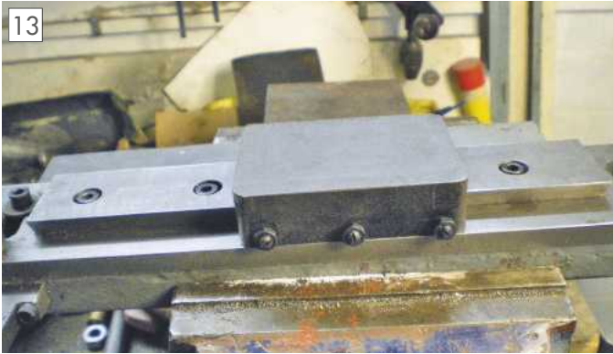
The sliding block in place on the finished swivel.
