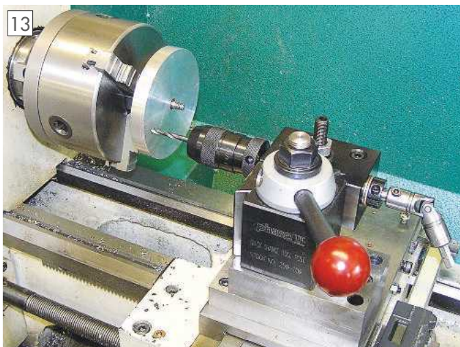
Using the drill along the lathe axis, note the universal drive joint.
