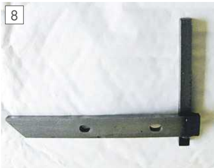
8 The simple guide that unfortunately does not align at 90 degrees.
