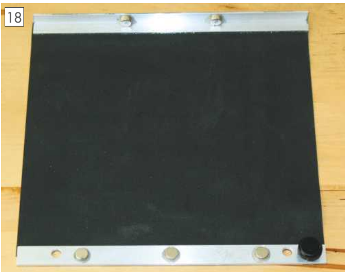
Simple swarf guard made of oil-resistant Viton rubber, with magnets on aluminium strips for fixing to the machine.
