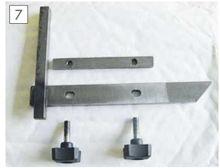
7 Alignment gauge and clamp components that were not really up to the mark.
