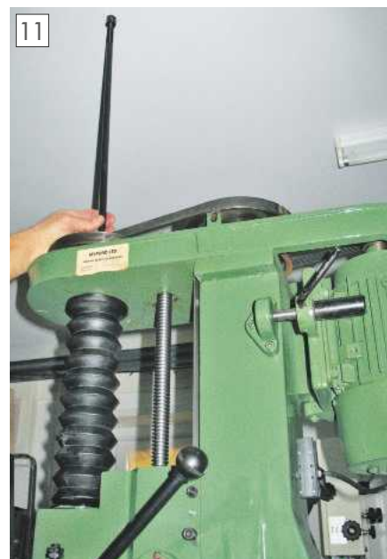
You need a decent ceiling height to extract the drawbar from a MKII VMB!
