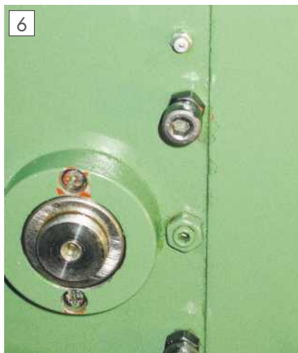
Gib adjusters on the head - initially gummed up with paint and immobile!
