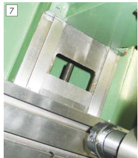
A pair of aluminium sash plates protect, and give access to the Y axis feedscrew.
