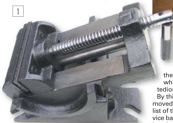
The original vice with the base trued up.
