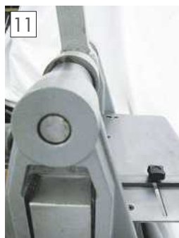
11 The end bearing of the main shaft in the cast end frame.
