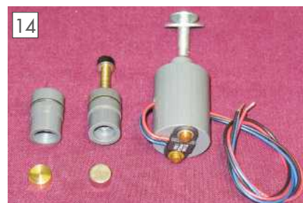
The plastic parts installed inside the belt casing. On the left are holders for the magnet and brass counterweight. On the right is the carrier for the Hall sensor: this is secured using the existing hole in the base of the casing seen in photo 15.
