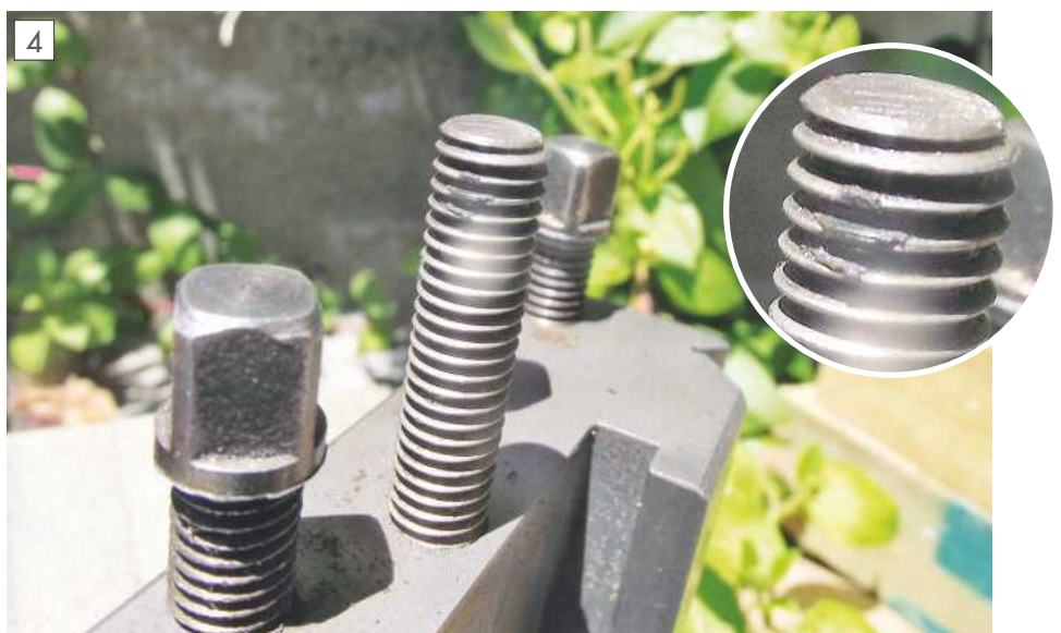
QCT height adjuster nylon insert in threads 3 and 4.
