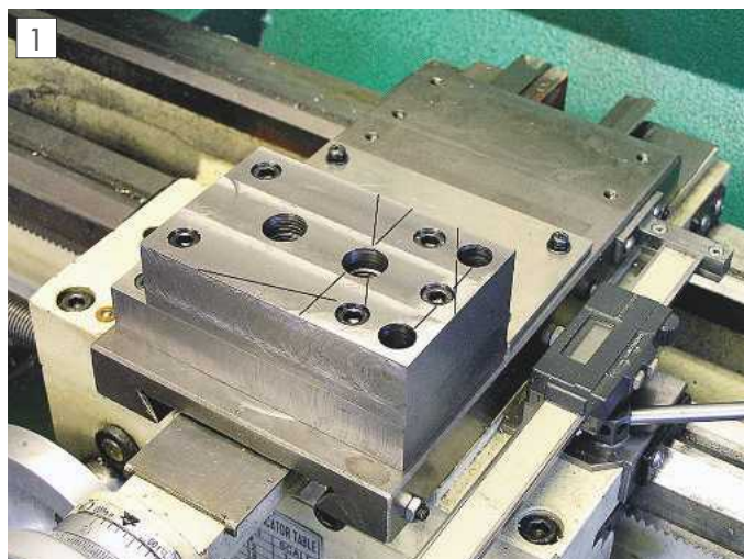
QCTP base fitted at the front of the cross-slide.
