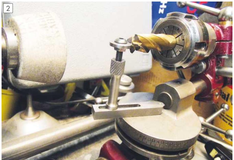
Improved Quorn end mill tooth setting gauge in use.
