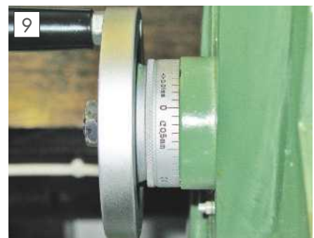
One turn of the handwheel on the head moves it up or down only 0.5mm! However, the graduations are a superfine 0.01mm which is useful for precision boring or milling.
