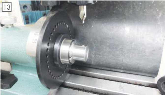
Drilling the dimple.
