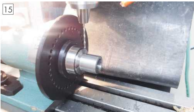
Drilling the hole for the first clamp screw.
