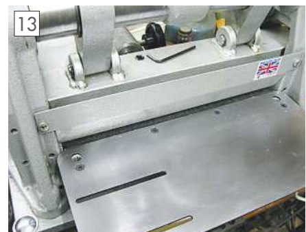
13 You can clearly see the 2 x 10mm threaded holes intended for a material clamp.
