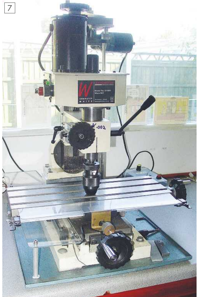
The spindle can easily reach the table when a keyless chuck is fitted.
