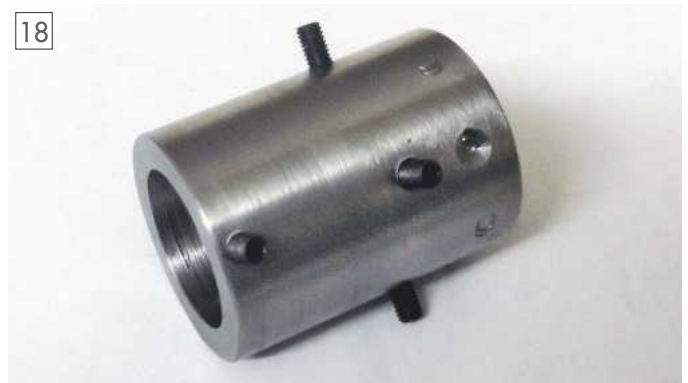
The completed housing.
