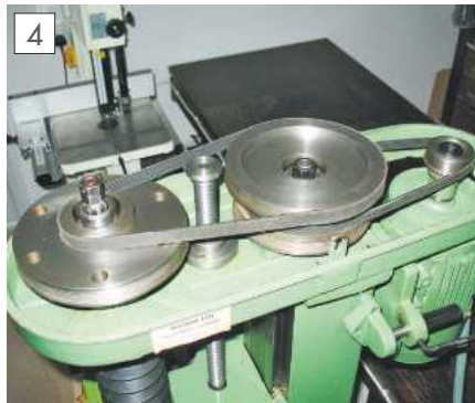
Motor, intermediate and spindle drive pulleys inside the head casing. The tachometer magnet and brass balance weight were inserted into diametrically opposite pulley holes.
