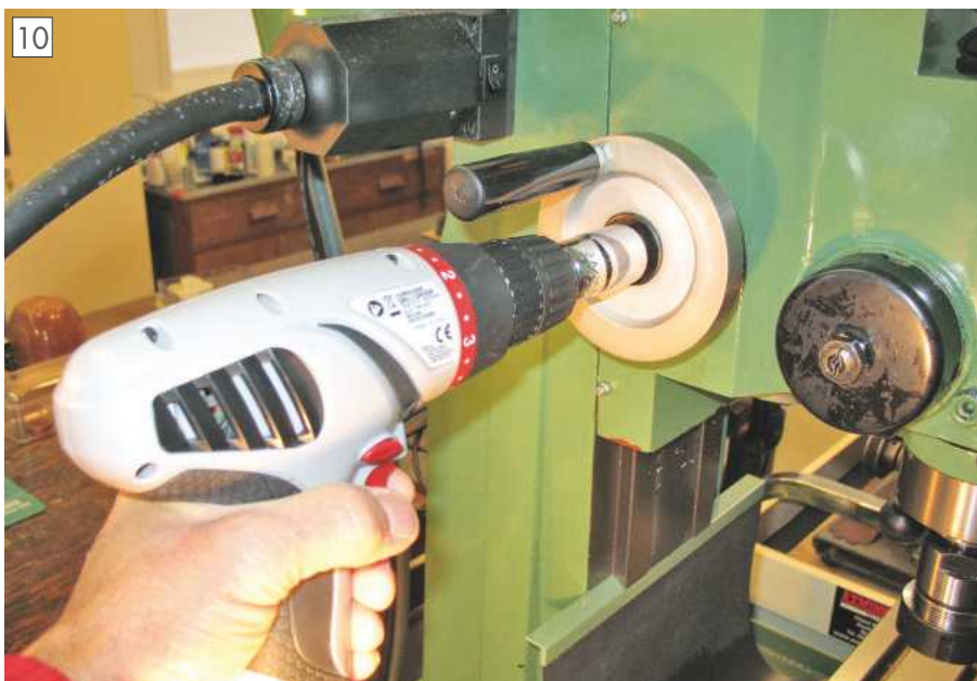
The tedium of moving the head manually is easily rectified by using a cheap cordless drill and \frac{3}{4} inch AF socket to rotate the handle.
