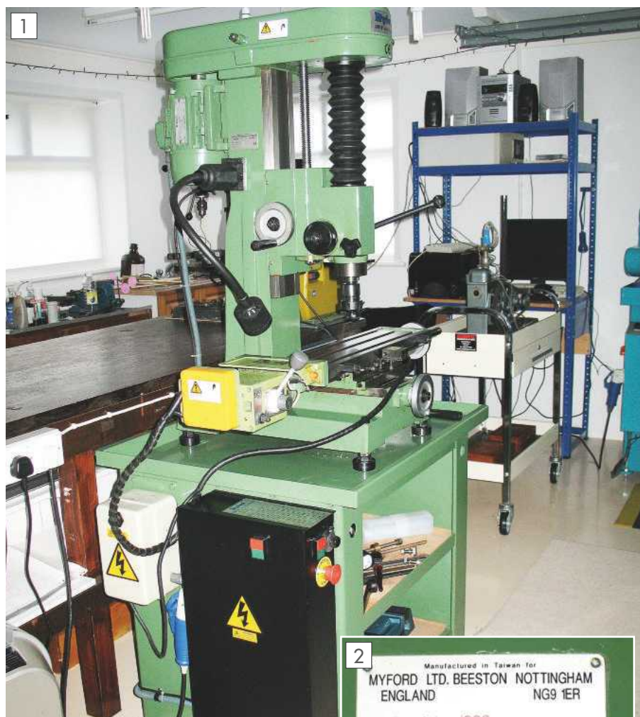
My VMB as originally supplied by Quillstar was fitted with an Align table power feed and associated 115V transformer in the grey box. This heavy drive unit has since been removed.
