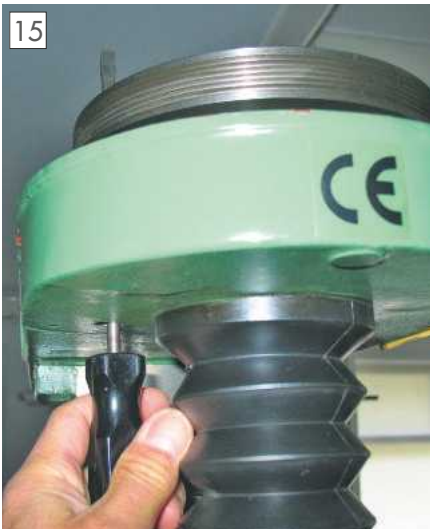
A hole in the base of the belt casing is provided to enable locking of the spindle pulley. This hole has been used to fit the Hall sensor carrier.
