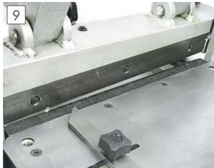
9 The safety guard removed to see the cutting blades and you can just make out the three securing screws of the moving blade.
