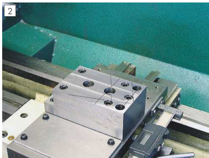
The QCTP base fitted towards the back.
