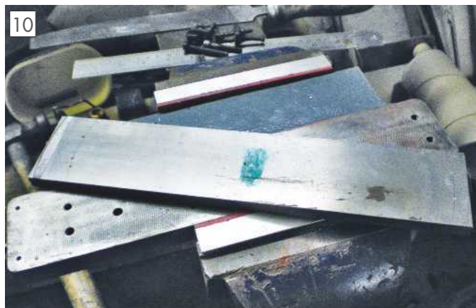
Marked out for the centre hole.
