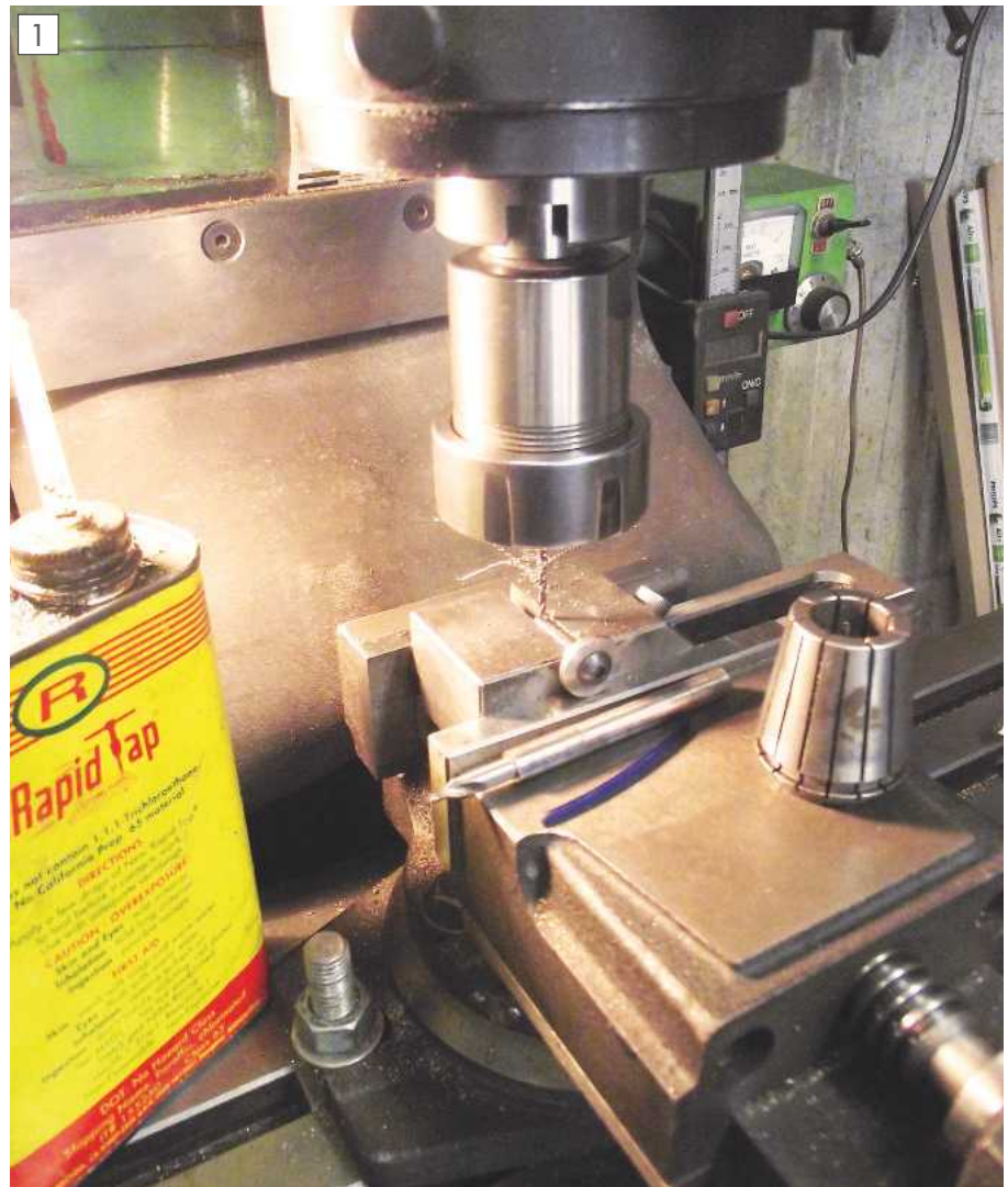
2mm dia. hole being drilled in end of M5 cap screw.
