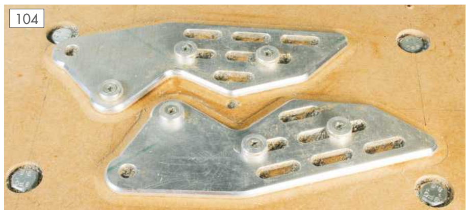
The guards secured to a backing plate.
