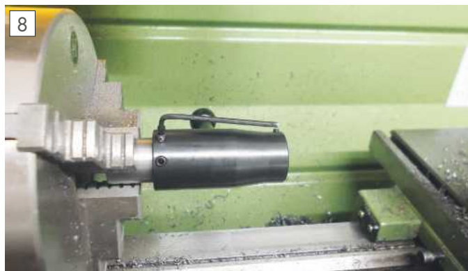
Marking for the location dimple.
