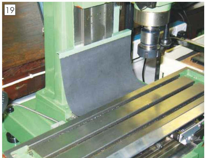
Swarf guard in place. Access to the Y axis oilers is retained via holes in the nearest fixing strip seen in photo 18.
