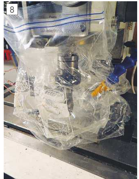
Magnets fix the bag to the head.
