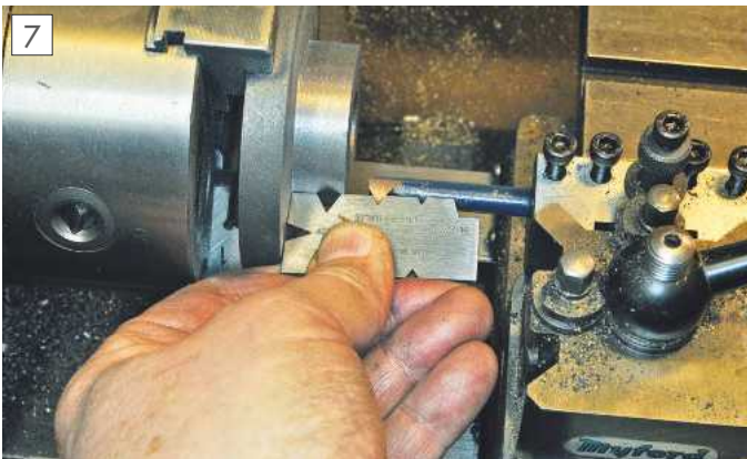
Setting boring tool square to lathe axis.
