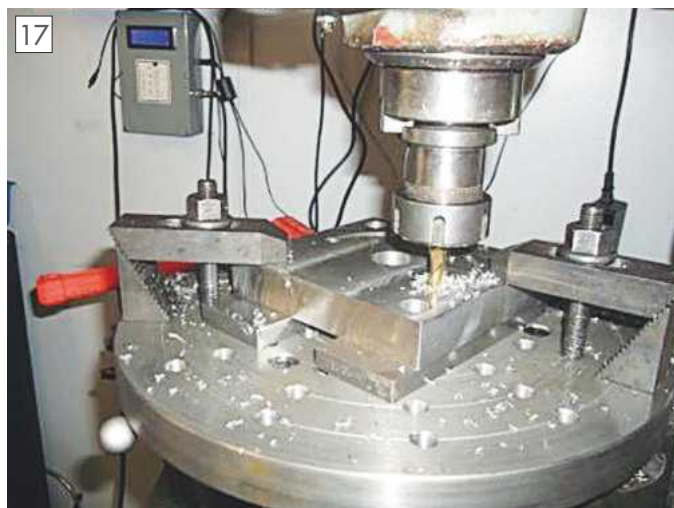
Putting tee-slots in the rotary base.
