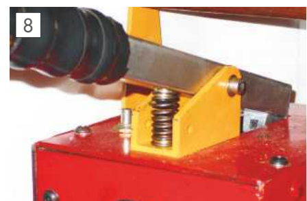
The handle return spring arrangement.
