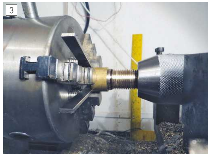
Adding support from the tailstock.
