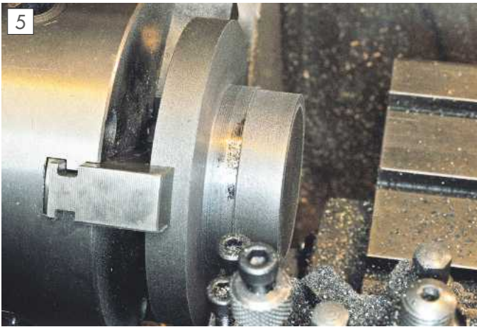
Turning backplate boss with shiny hard spot.
