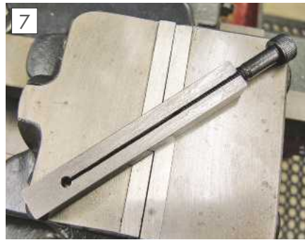
Prototype spring parallel.
