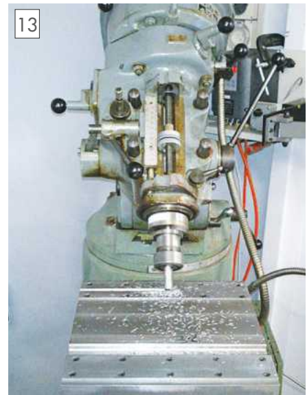
Machining the vee-way.
