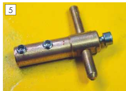
An electrode and electrode carrier.
