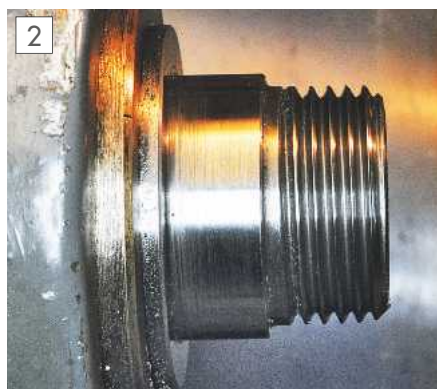
Myford spindle nose register and thread.
