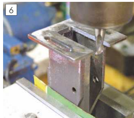
Truing up a fabricated bracket.
