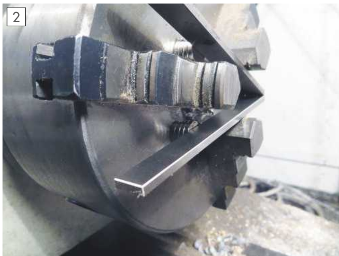
Parallels supported on stacks of magnets.
