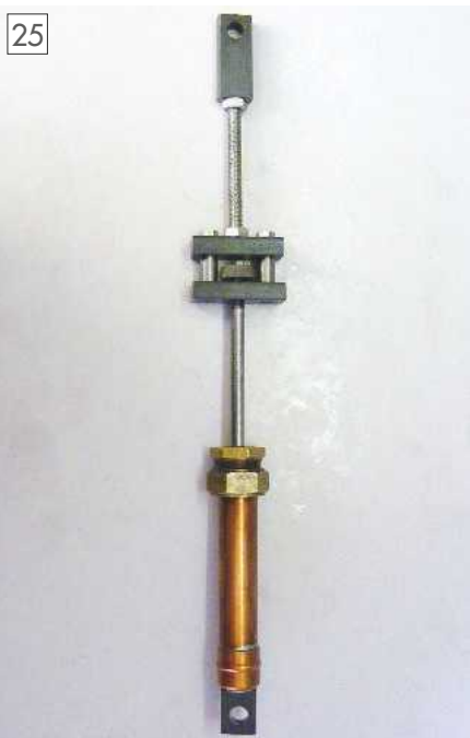
The cylinder and push rod assembly – open.
