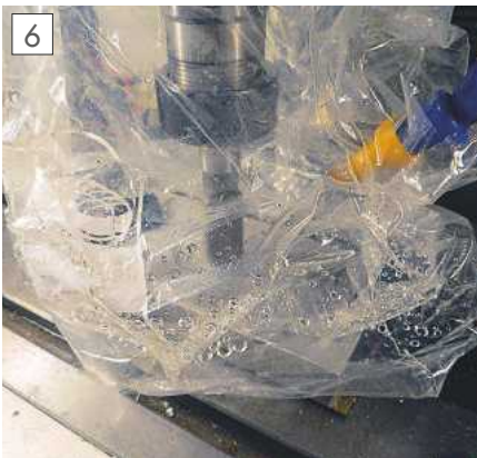
The magnetic bag solution to reducing coolant spray.
