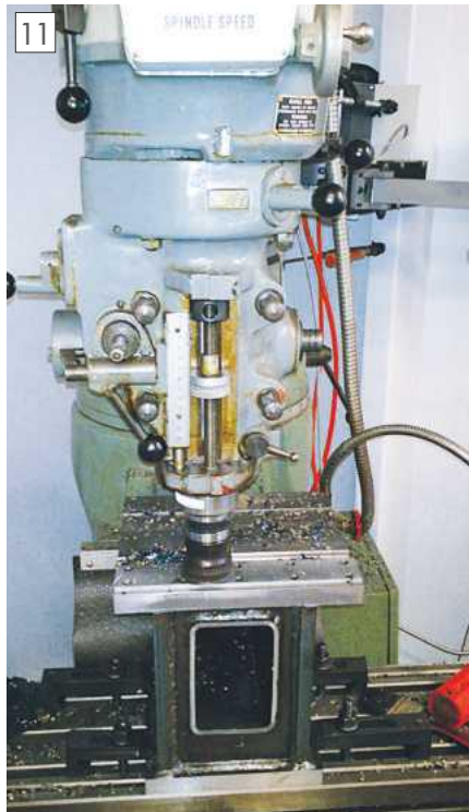
Machining the base of the extension.
