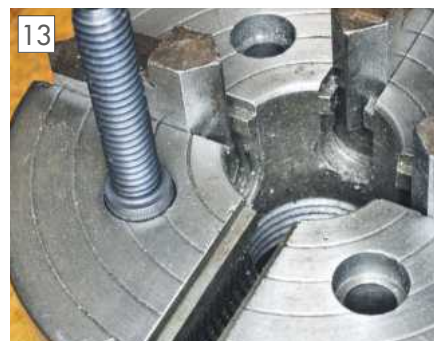
Determining amount of screw head to remove.
