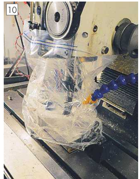
A hole is made for the coolant nozzle.
