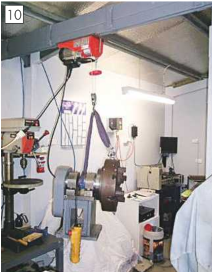
Lifting the headstock extension.
