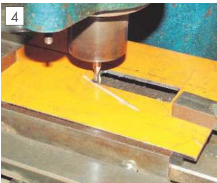
Milling the slot for the upper arm.
