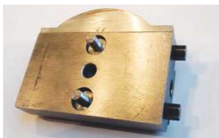
The underside of the modified topslide.
