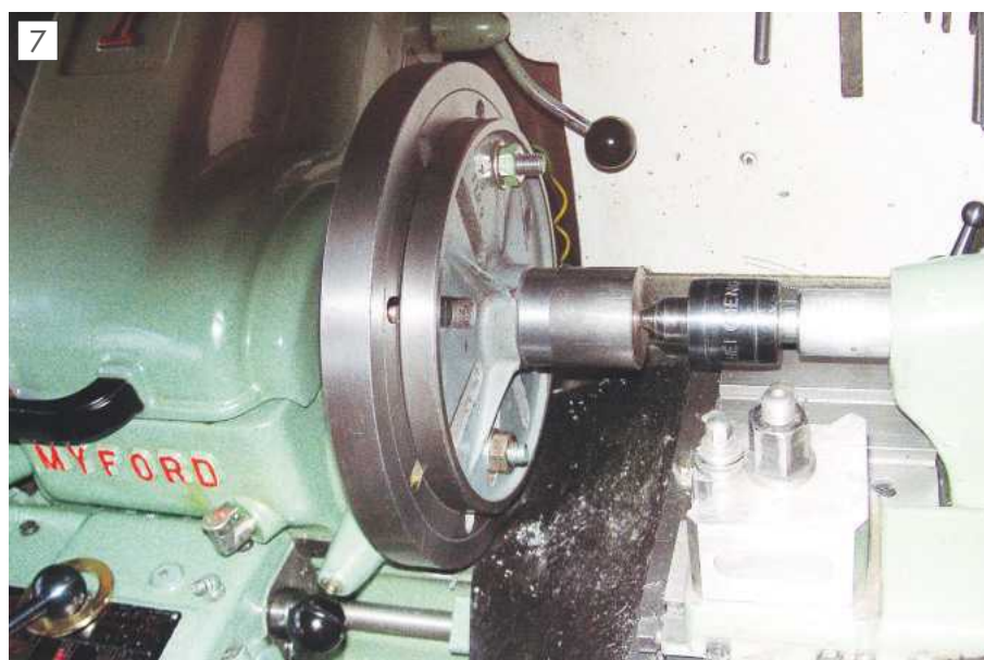
Using two faceplates back to back.
