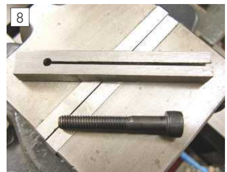
Prototype spring parallel, component parts. Simple shank without handle and cap-head expansion screw.
