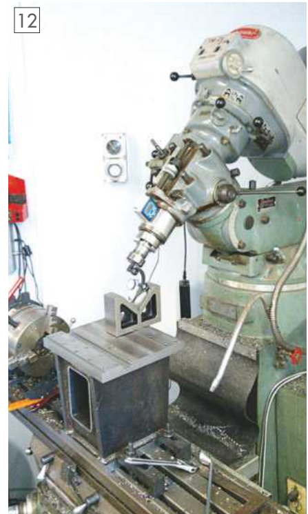
Setting the head angle ready for machining.
