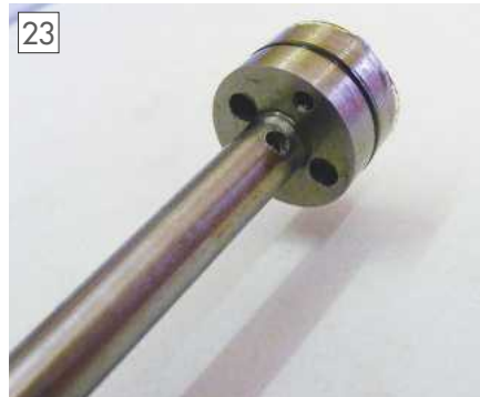
The piston showing screw holes and transfer holes.
