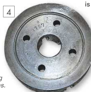
False nose with Myford thread and register.
