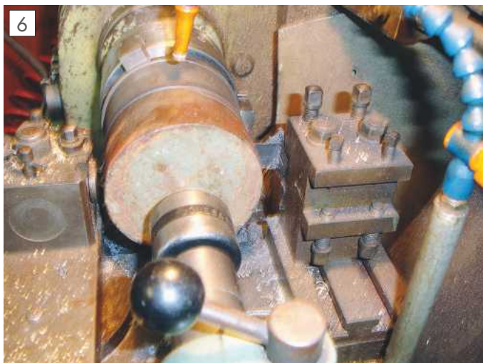
Parting off under power.
