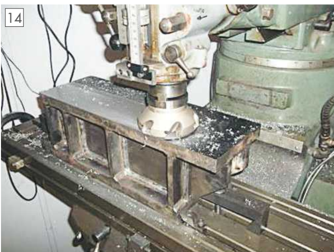
Machining the top of the saddle riser.
