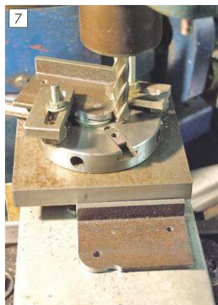
Set up for radiusing.
