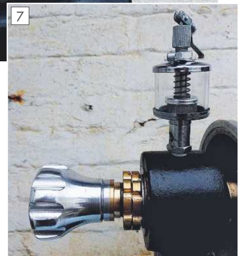
Spindle locking nuts and collar.
