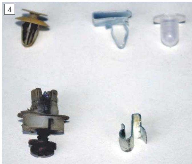
Various metal and plastic clips. Clockwise from top left : 1 & 2 clips for door cards, 3 may be used as hole liner for 2, 4 secures brake pipe to edge of sheet, 5 expanded by screw e.g. for headlamp retention.
