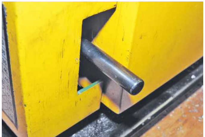
The lever extends through the front of the gear cover.
