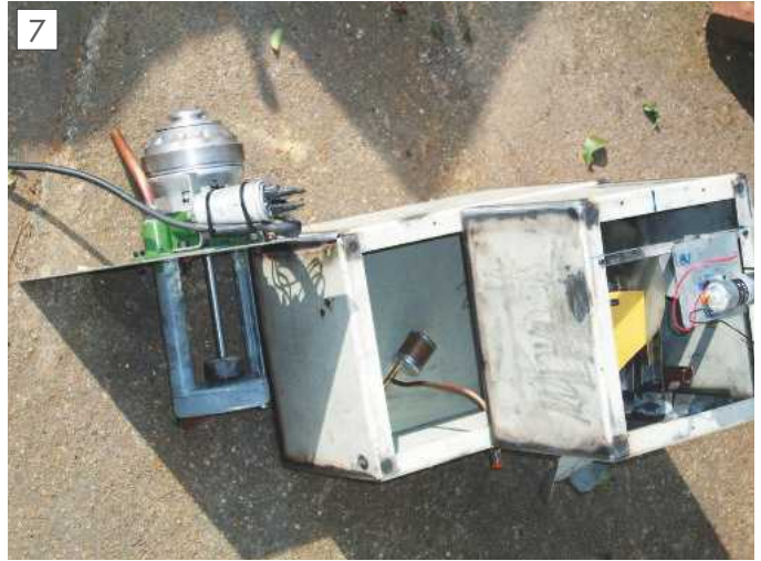
The complete coolant system with aerator fitted in bottom tank.
