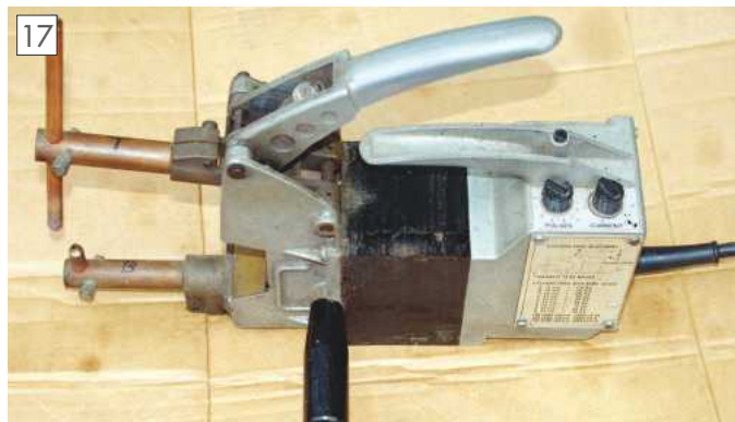
Electric spot welder with power and pulse count controls.
