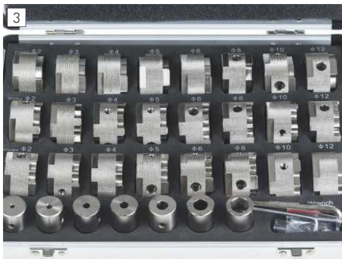
The collets and cams supplied as standard.
