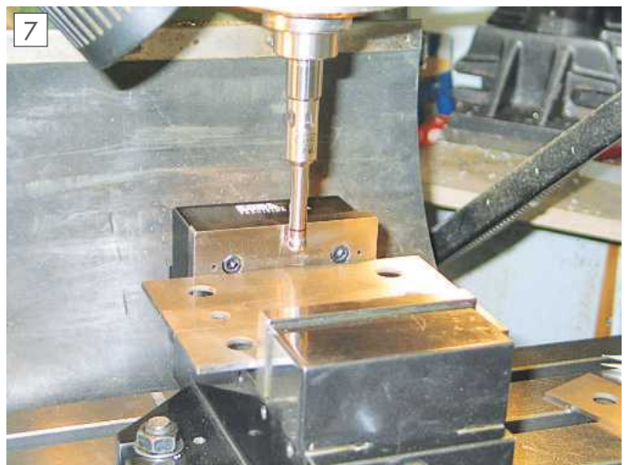
Measuring the jaw movements.
