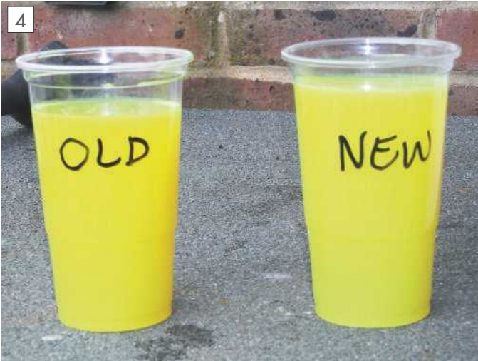
Comparison of old cleaned coolant and freshly mixed.
