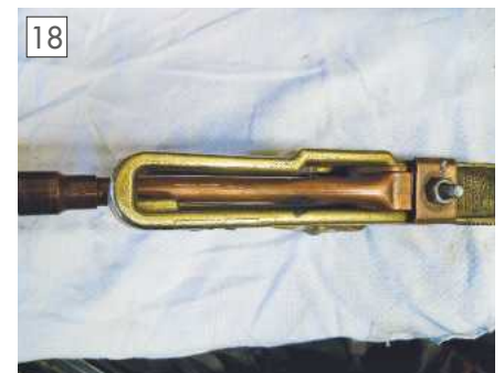
Welding set earth clamp repair.
