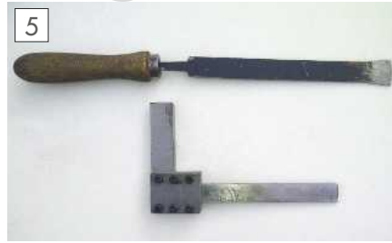
Tools from worn out files.
