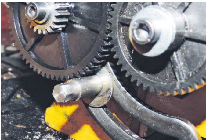
The extended nut and spring washer.
