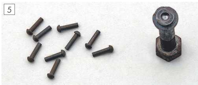
Several \frac{3}{32} in. rivets with home made snap.
