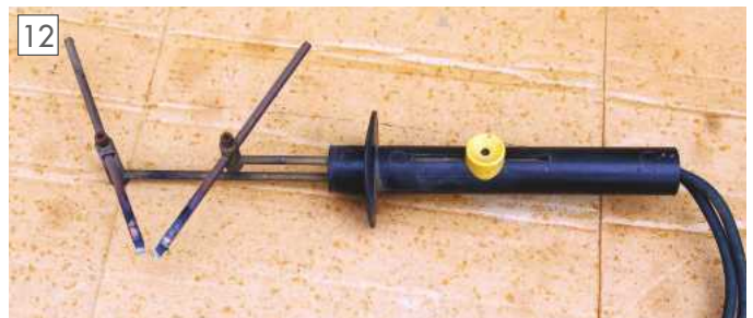
Twin carbon arc torch is powered by a basic arc welder.
