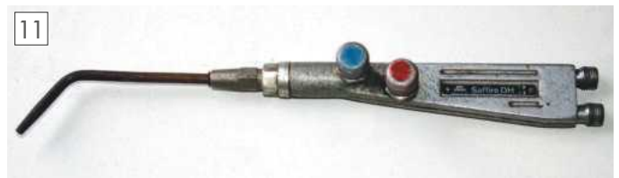
Gas welding torch.
