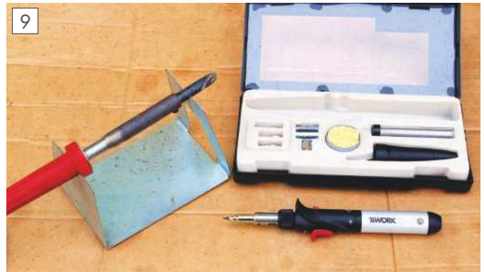
For heavier work, a 125 watt electric and 100 watt gas soldering iron.
