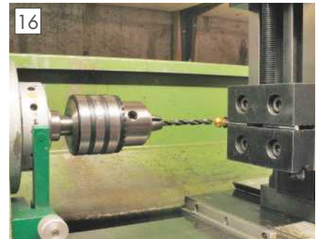
Drilling the pillar.
