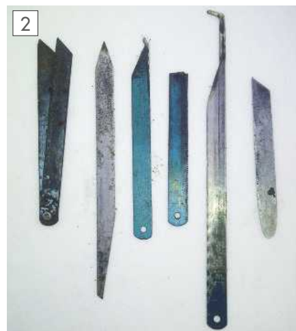
Squared edged tools from hacksaw blades.
