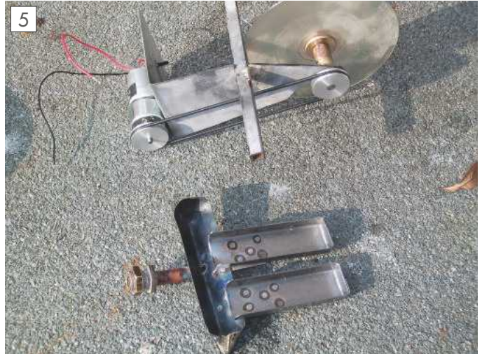
The main parts of the home-made coolant skimmer.
