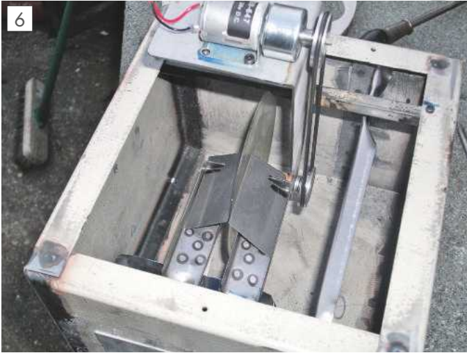
Skimmer unit fitted in coolant tank.
