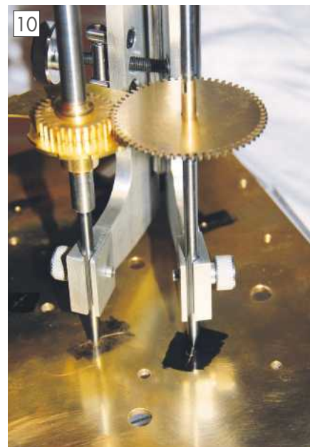
Using the depthing tool to mark out gear centres.
