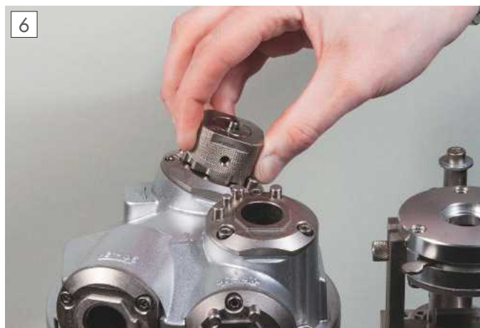
Putting on the secondary clearance.
