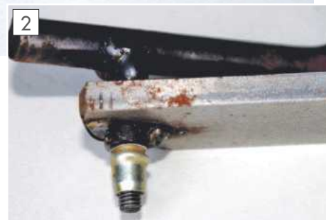
Deformation of M5 nutsert.
