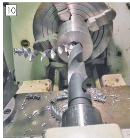
Drilling hole with 30mm drill.
