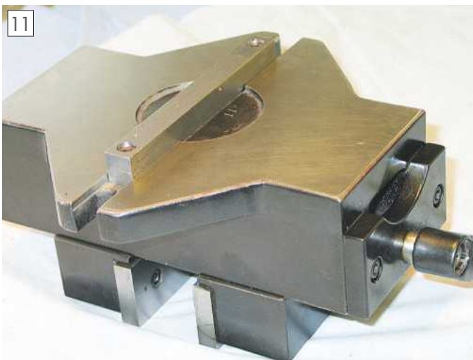
Tenon fitted to the self-centring vice.
