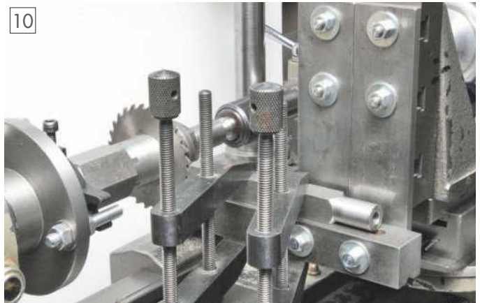
Method of clamping bar components.
