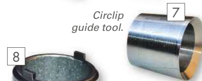
Slotted ring tool from a scaff bar.
