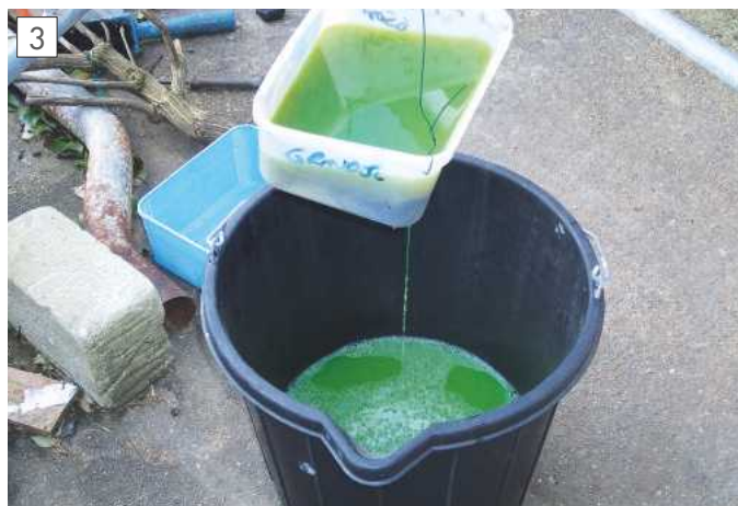
Filtering the partly cleaned coolant.
