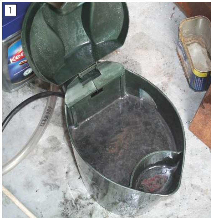
Nearly boiled coolant with tramp oil floating on the surface.
