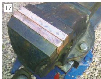
Finished soft jaws in position.
