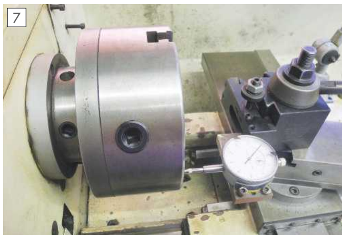
Setting chuck to run true.
