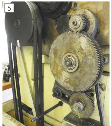
Greasy lathe change wheels.
