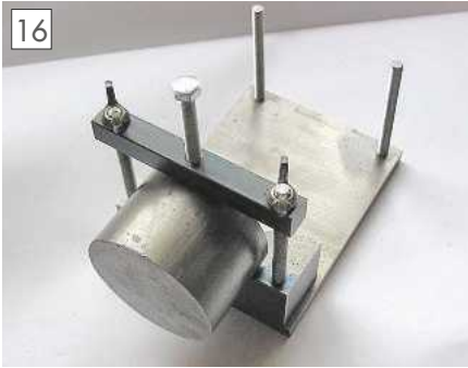
Clamping a 50mm bar.
