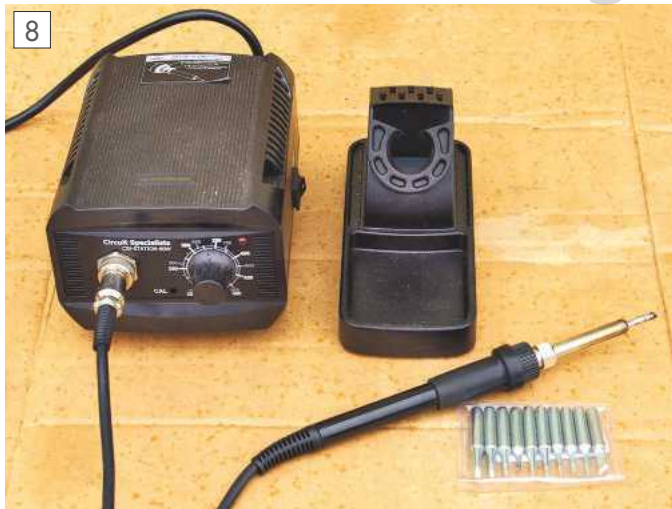
Temperature controlled soldering iron with selection of tips.
