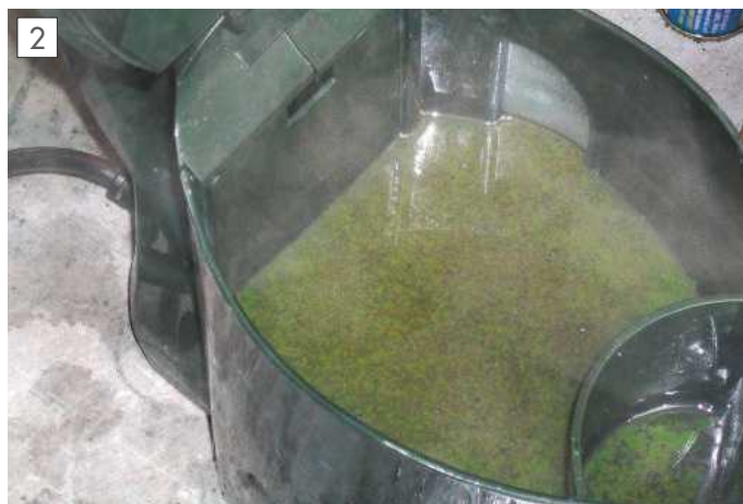
Tramp oil vacuumed off the top of coolant.
