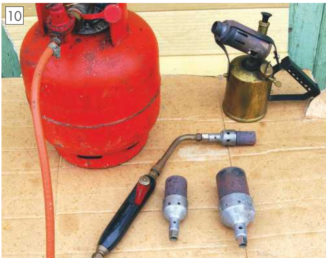
Propane cylinder, torch, interchangeable heads with older paraffin blowlamp.
