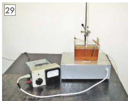
Electroplating taking place using the hot plate to ensure the correct electrolyte temperature.
