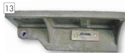
The modified fixed jaw.
