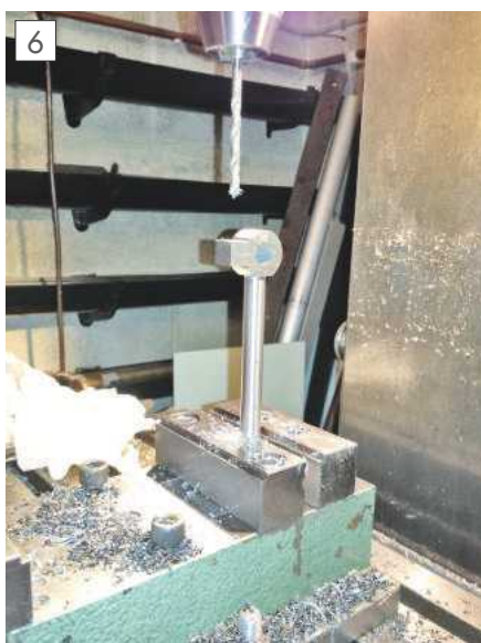
Drilling the clamp bold hole in the spindle.
