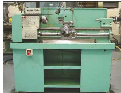
MYFORD Type 254S: Centre Lathe. 9" Swing over bed. 30" Between Centres. 1" Spindle Bore. Speeds 53 to 2000 rpm. £2,450
