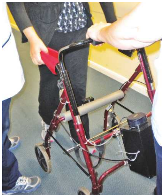
The walker in use. Note the black box on the front of the walker. This contains the electronics, servos and quick change battery pack.
