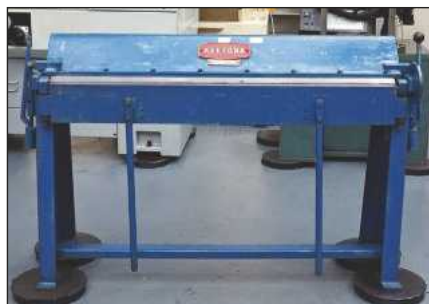
KEETONA: Manual Straight Sheet Metal Folder. Capacity 51" x 16swg. £850
