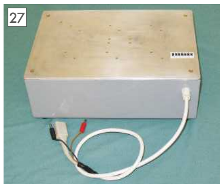
The completed hot plate with an LCD thermometer.
