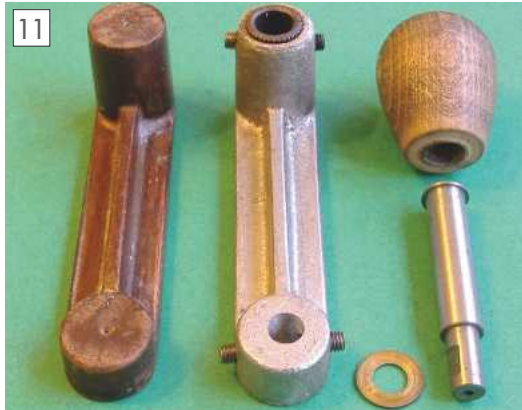
Handle casting and pattern.
