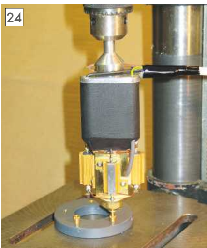
24 A series of M4 brass inserts being heat staked into a ring of PVC drilled with 5.6mm holes.
