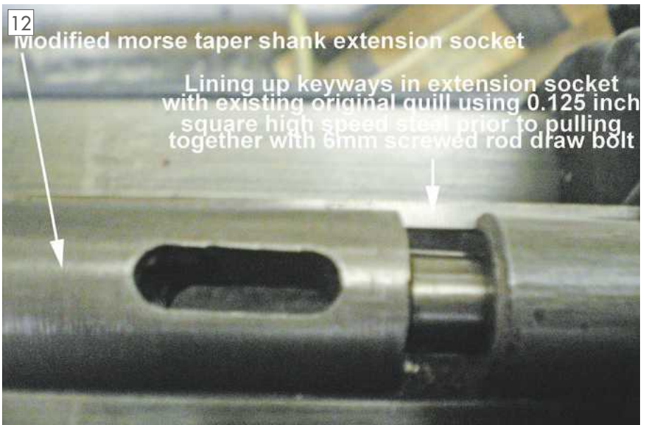
Using square HSS to align the components.
