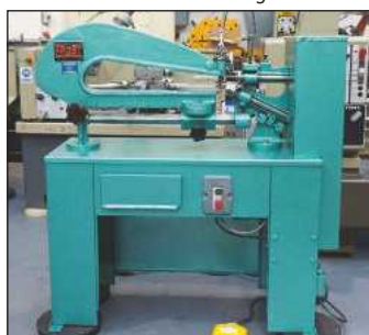
FROST Type 399: Power Circle Cutter. Maximum Diameter 48". Cutting Thickness upto 16swg. £2,250
