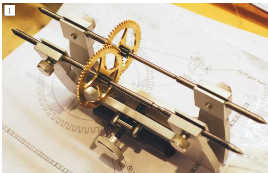
The clock gear depthing tool.
