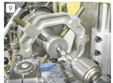
Using a fixed steady.
