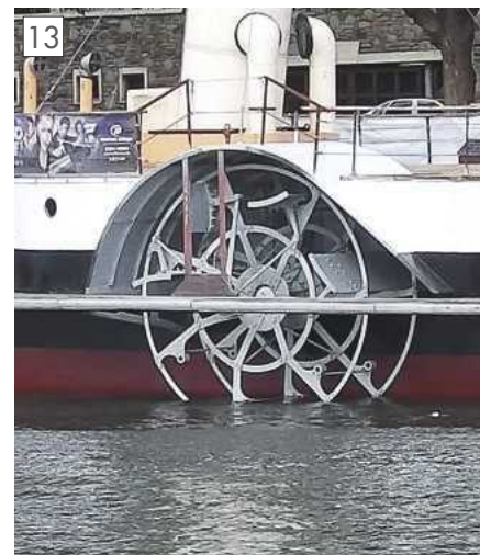
Paddle Wheel in situ clearly showing omitted floats - Richard Halton.
