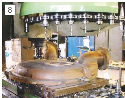
Machining the condenser casting (D. Abels).
