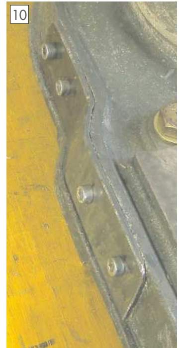
Reinforcing plates on the base.
