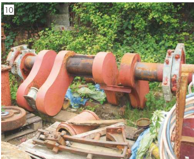
The unrestored crankshaft (R. Halton).
