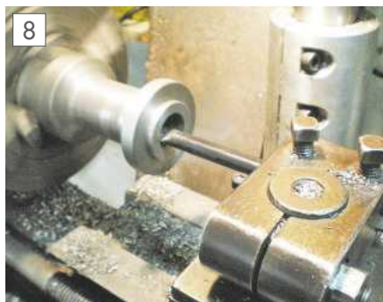
Boring to a good fit on the quill.
