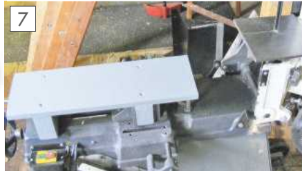
The seat clamped in the vice.
