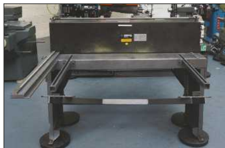
WALTONS Model UTG/50/16: Treadle Guillotine. Blade Length 1270mm. Capacity 1.6mm. 2 x Front Support Arms. Rack & Pinion Back Gauge. Year 2005. £1,750
