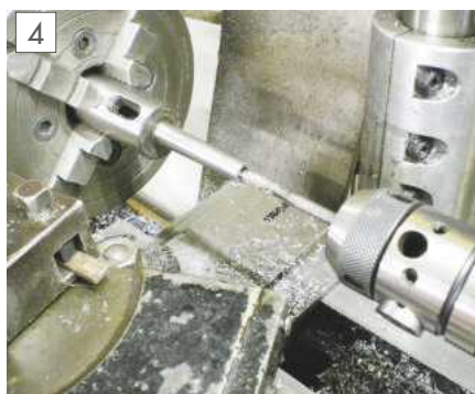
Drilling and tapping the Morse taper shank.
