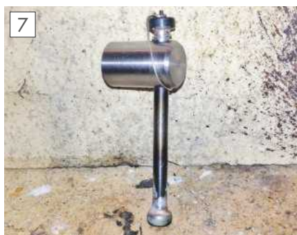
Set up to silver solder a handle.
