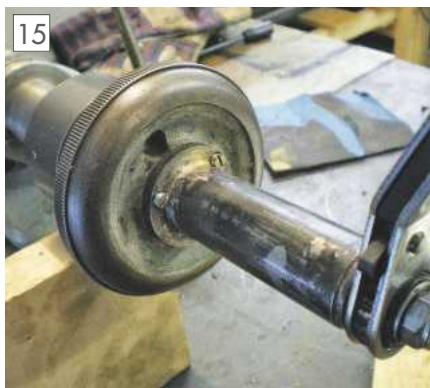
The ratchet fitted to the quill.
