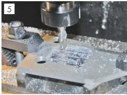
Machining the clamp plate inner profile.
