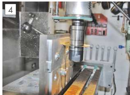
Cutting the slot for the bulldog spring.
