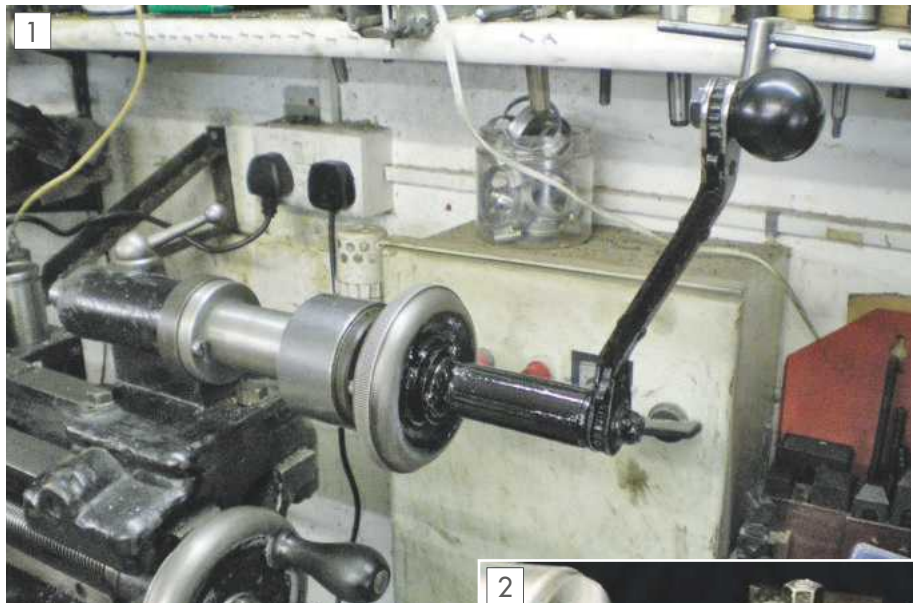
The completed tailstock modification.
