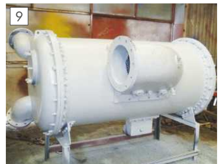
The completed condenser (D. Abels).
