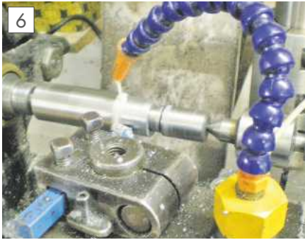
Machining the extension.
