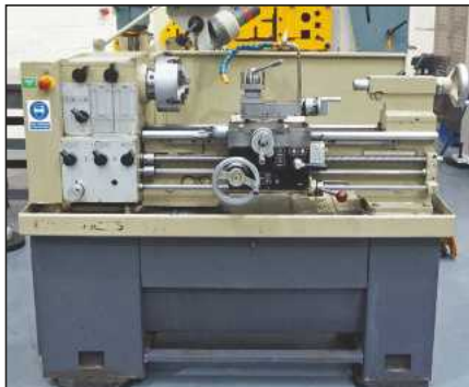
HARRISON TYPE M300: Gap Bed Centre Lathe. Swing 13". Between Centres 25". Spindle Bore 1 ½". Speeds 40-2500rpm. 3&4 Jaw Chucks. QCTP. £5,250
