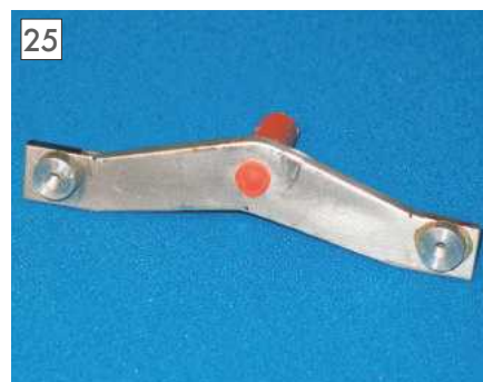
25 Red PVC pillar fixed to an aluminium bellcrank using a doming tool fitted to the heat stake device.
