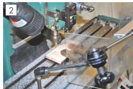
Machining the outer plate profile on a Tom senior machine.
