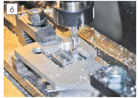
Machining the clamp plate outer profile.
