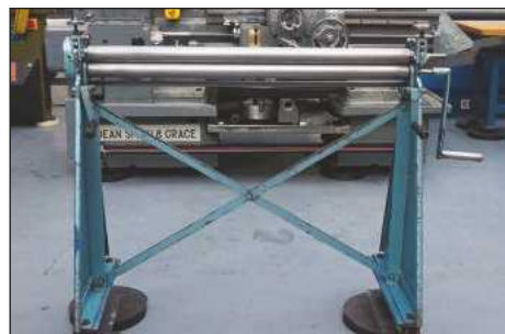
KINGSLAND INTIAL PINCH: Manual Sheet Metal Bending Rolls. Capacity 40" x 18swg. Roll Diameter 2". £950
