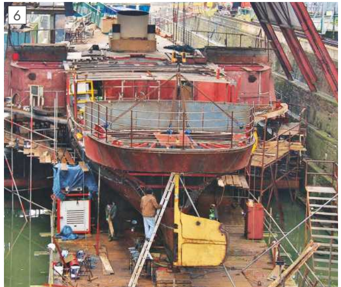
Installing the counter (B. Stokes).
