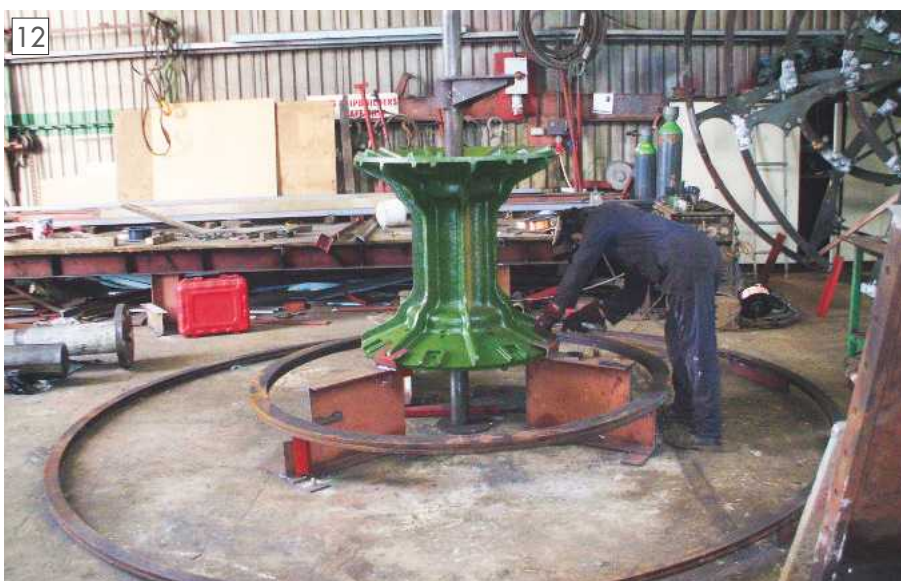
Jigging up a paddle wheel (R. Halton).
