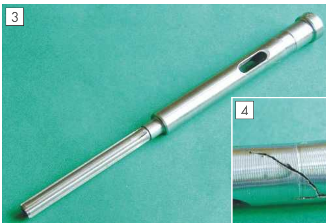
The damaged spindle.
