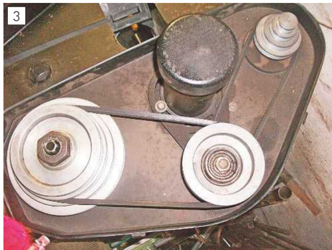
The drive belts and pulleys of the RF-25.
