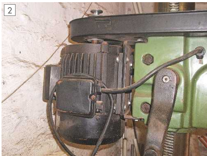
The 1-HP motor fitted to the RF-25.
