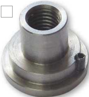
The nut with the dowel pin fitted...
