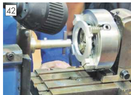
42 Shaping an internal gear.
