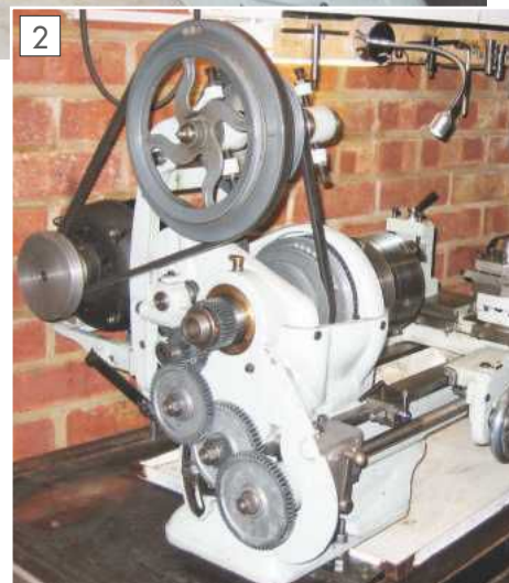
The lathes change gears and countershaft drive.
