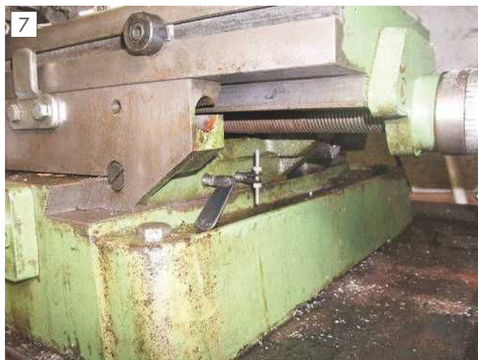
Y-axis original leaf screw and modified screw with T handle.
