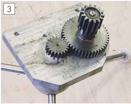
The gears on the tailstock apron.
