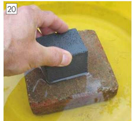
20 Finishing the Thermalite insulation block by sanding over a driveway pavior immersed in water.
