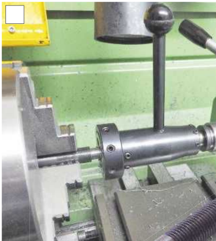
Threading the modified spigot.
