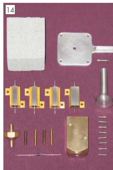
Main components of the heat stake. Not shown is a thin fibre insulating fibre washer that fits between the aluminium spigot and square top plate to reduce heat loss to the pillar drill.
