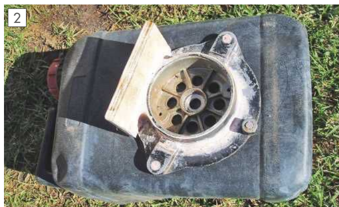
The pattern made using the original flange.
