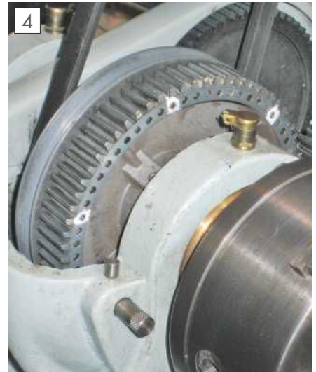
Bull wheel with indexing holes.
