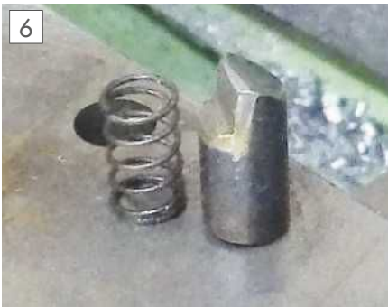
The detent and its spring.
