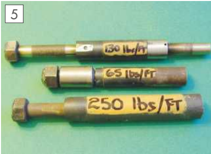
Three shrink fit test pieces.
