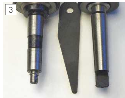
Tang Comparison and chuck removal drift.
