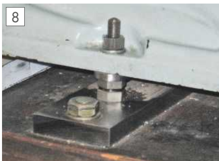
Adjustable feet fitted to the lathe bed.
