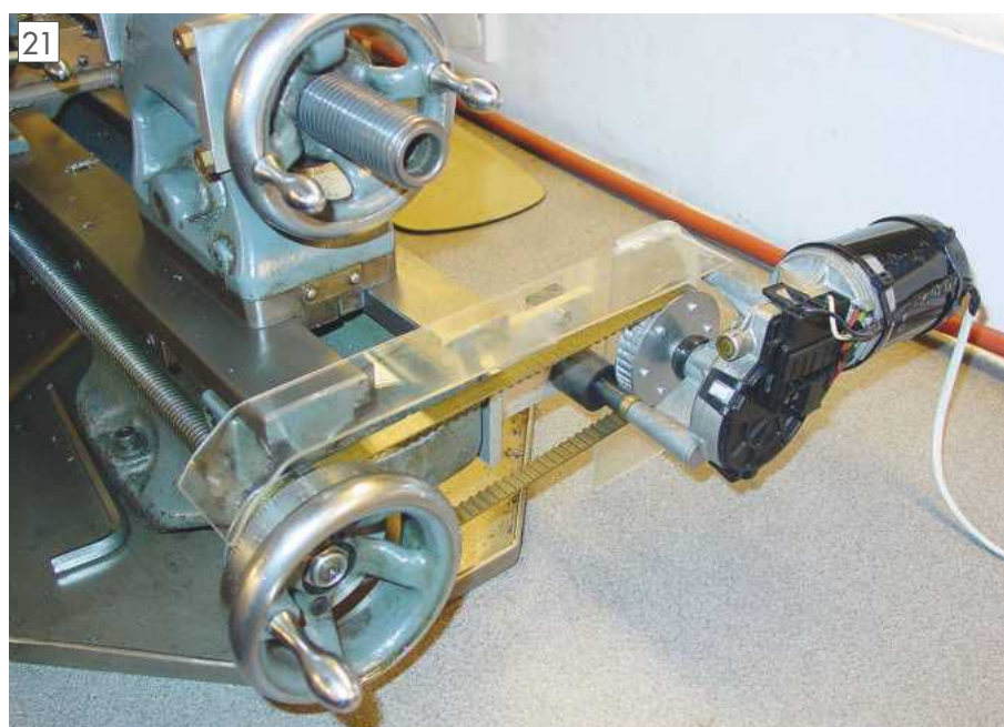
The final set-up with belt guard fitted.
