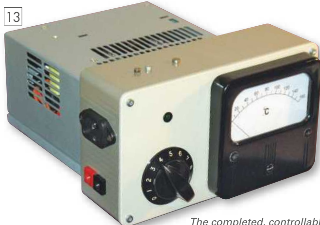
The completed, controllable ATX power supply with moving coil meter temperature display.
