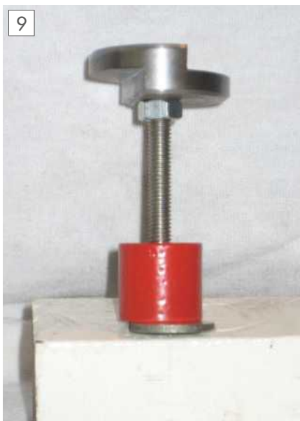
Some of the author's shop made accessories include this front and rear tool height gauge...
