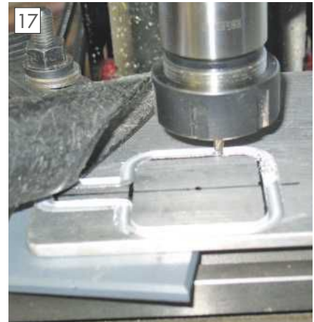
17 CNC machining the top plate for the heat stake.
