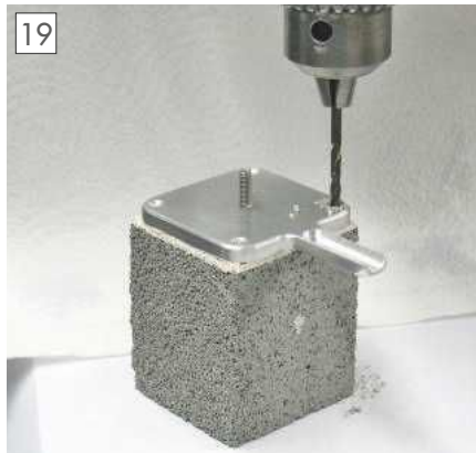
19 Drilling the four holes through the top plate and Thermalite block for wires that will connect to the heaters and diode sensor.
