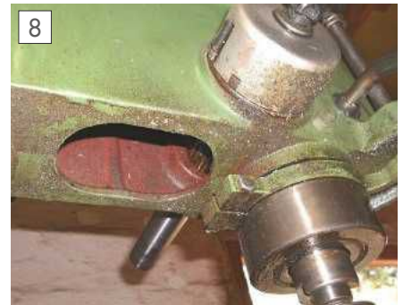
Cast in hole in bottom of headstock begging for a lamp.
