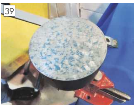
39 First steps in scraping.
