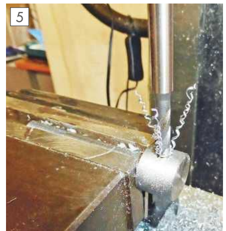
Tapping the lock bolt head.
