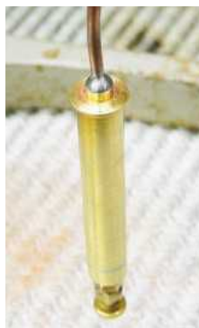
The new bulb with adjuster screw.
