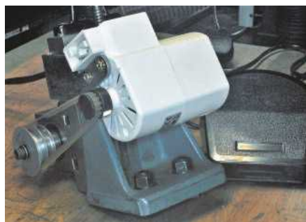
Arrand Motor – Rod Jenkins' sewing machine motor fitted to his Arrand spindle.
