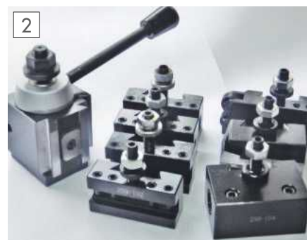
Quick change toolpost component parts.
