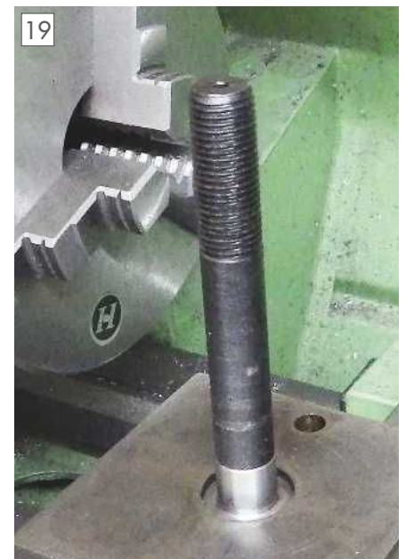
Toolpost securing stud assembled to spigot nut.
