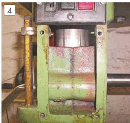
To lubricate the quill you need to remove the faceplate.
