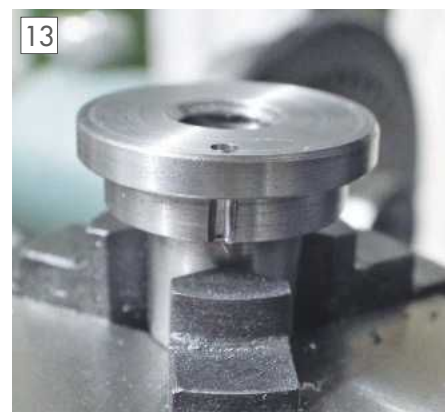
Location for the spring dowel.
