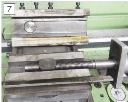
Compound/topslide removed from cross slide.
