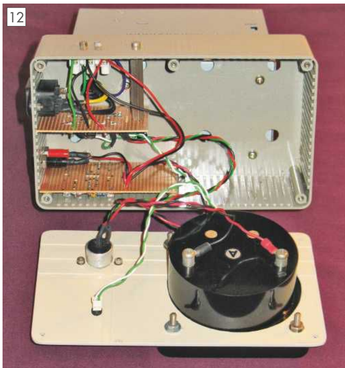
Interior of the Verobox showing the PWM circuit at top and temperature sensing circuit below. Heater current from the ATX unit is connected to a Europlug type of socket on the side of the case where a pair of 4mm sockets for the temperature sensor are also located.
