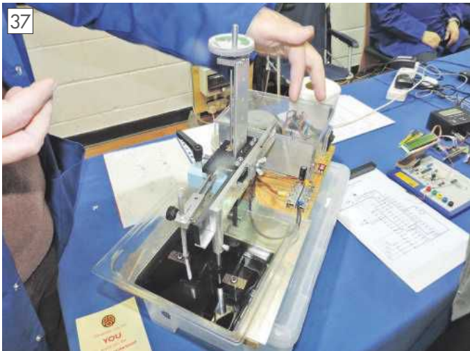
37 Demonstration spark erosion machine.
