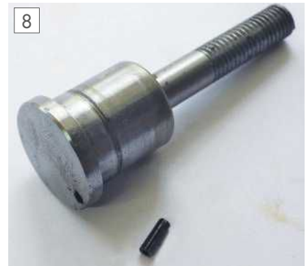
Locating spigot/locking handle stud & dowel.
