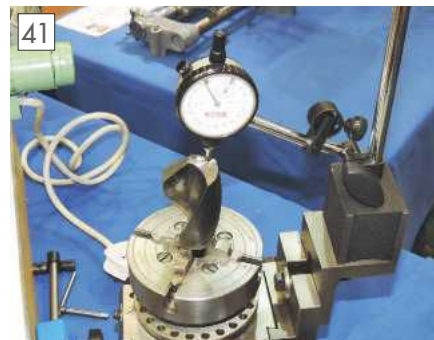
41 A drill accurately ground on a Quorn.
