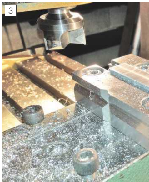
Reducing the jaw plates to 4mm.
