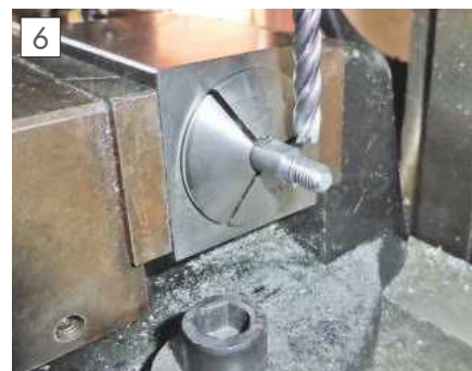
Milling flats on the operating handle.
