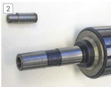
The chuck spindle extension.
