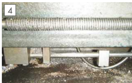
The stop bar of the leadscrew trip mechanism.
