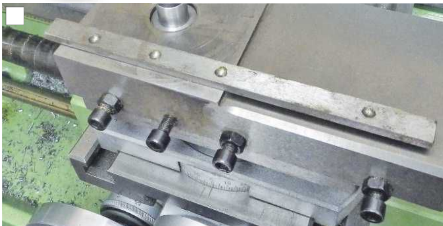
Compound/topslide jib strip.
