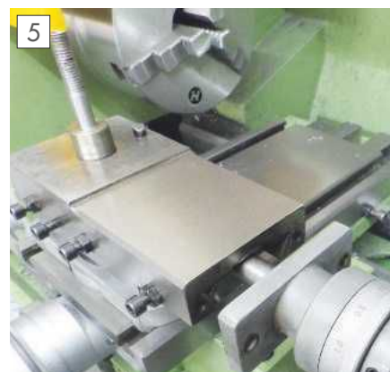
Compound/topslide during removal.
