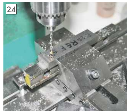
Mark out the holes from the reference edges and drill the holes.
