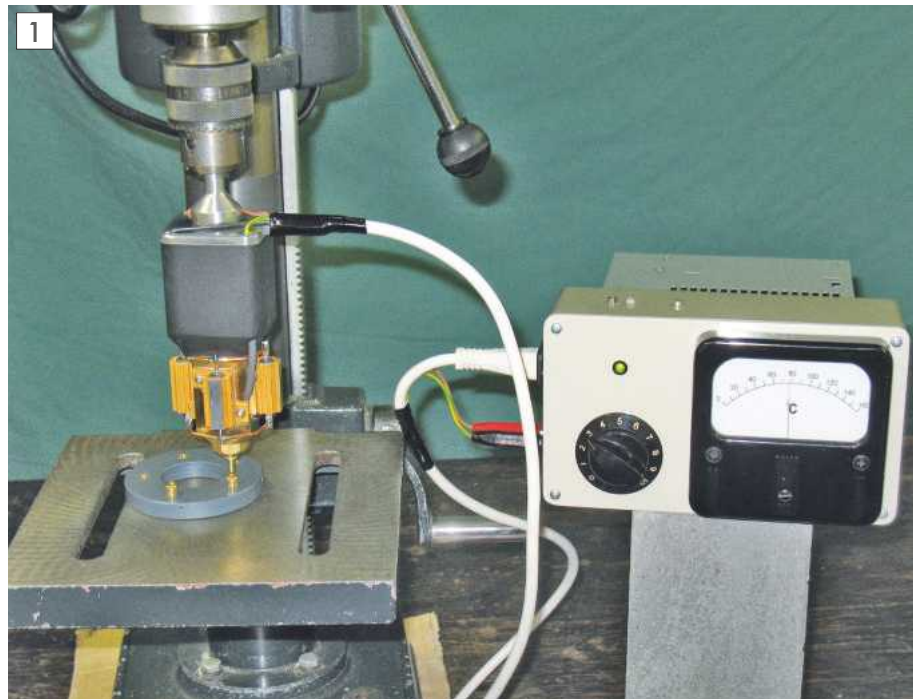
The heat staking tool in action. A set of brass M4 threaded inserts are being heated and emplaced into a PVC component. The ATX power controller also displays the stake's operating temperature.
