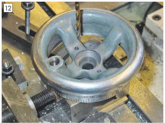
Drilling gear fixing holes in the handwheel.
