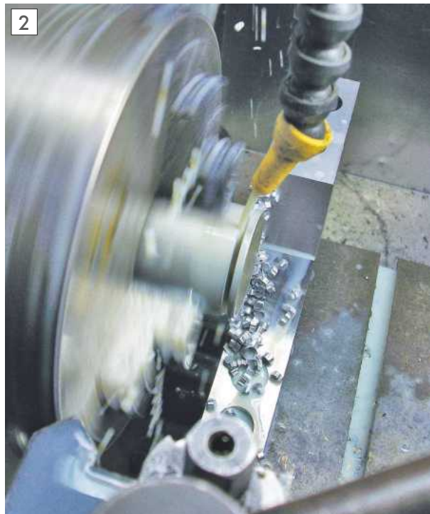
Parting off a washer with Reg's holder.
