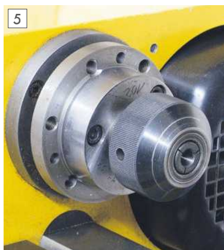
Collet chuck holder is secured by three M6 socket screws.
