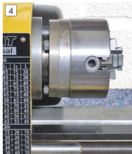
Custom face plate interfaces between flange and four-jaw chuck – note the M6 nuts that secure the chuck in the small gap between flange and head stock.
