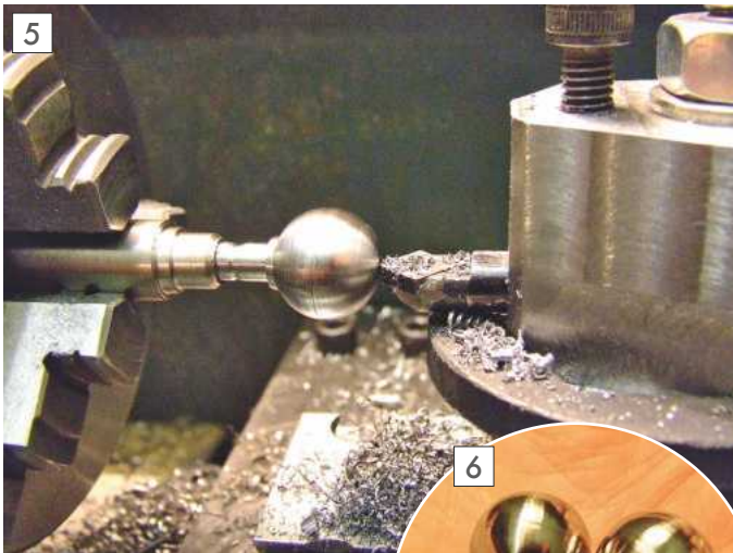
Set-up for completion of the ball.
