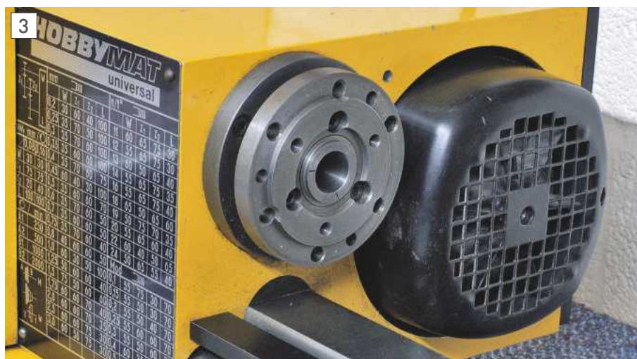
80mm flange with MT2 internal taper and adjacent motor.
