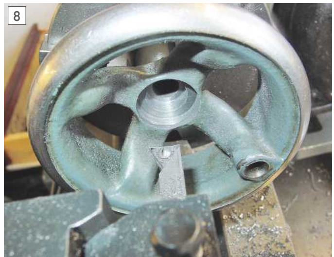
Counterboring the handwheel.
