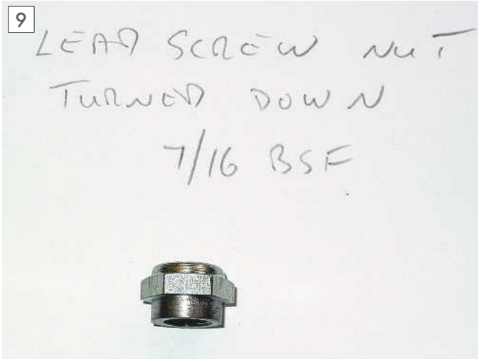
The modified leadscrew nut.
