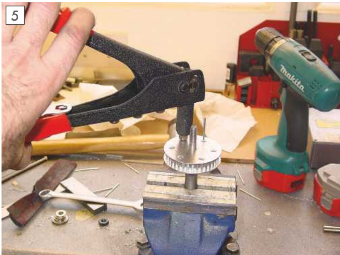
Pop riveting a flange.
