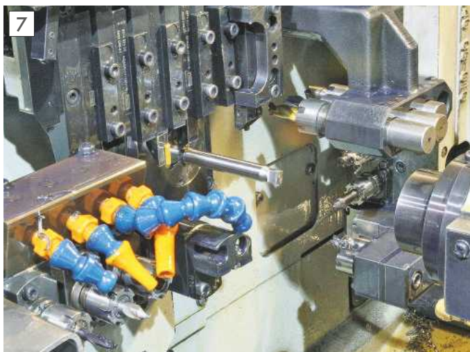
The automatic lathe used by Anchor Ltd for the production of threaded inserts.
