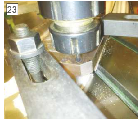
Drilling and counter-boring the holes.
