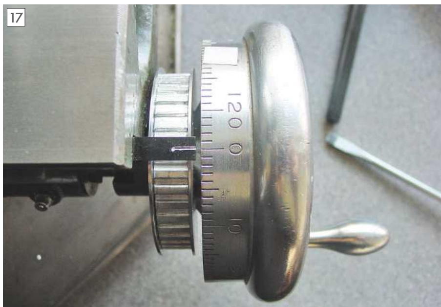
The new pointer is easily moved to allow belt fitting.
