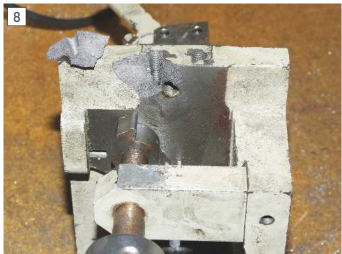
Damage to Main Casting.
