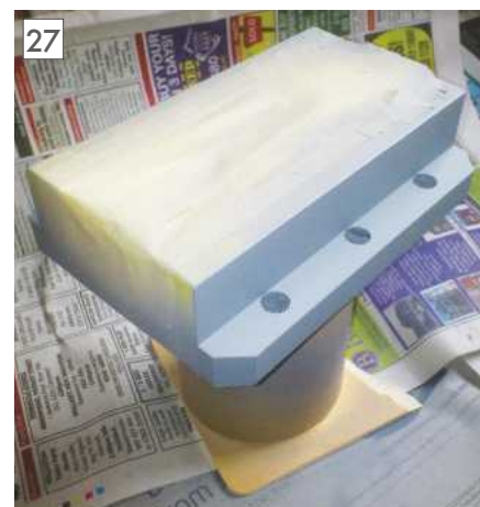
Masked base sprayed in primer.
