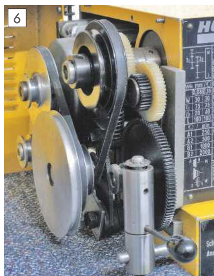
Space is limited in the transmission compartment – the slow speed attachment can just be seen at the bottom rear.
