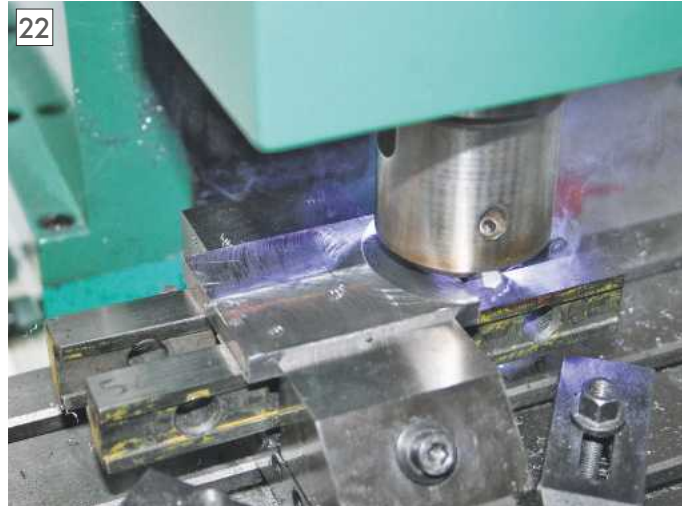
Machining the plate to the desired thickness.
