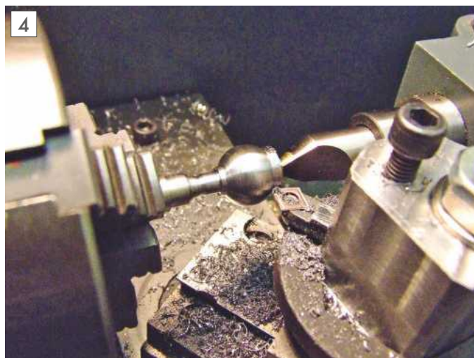
Optional set-up for the 2nd stage to finish the ball with a half centre support.
