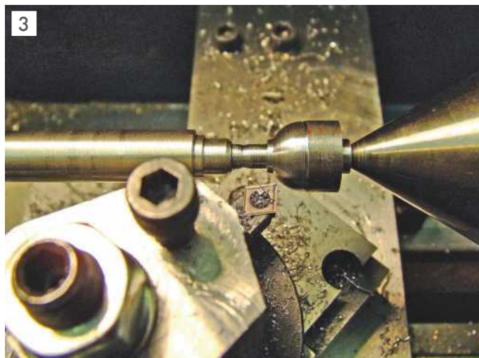
Turning the rear of a ball.
