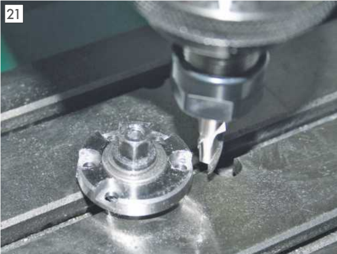
Milling the counterbore slots.
