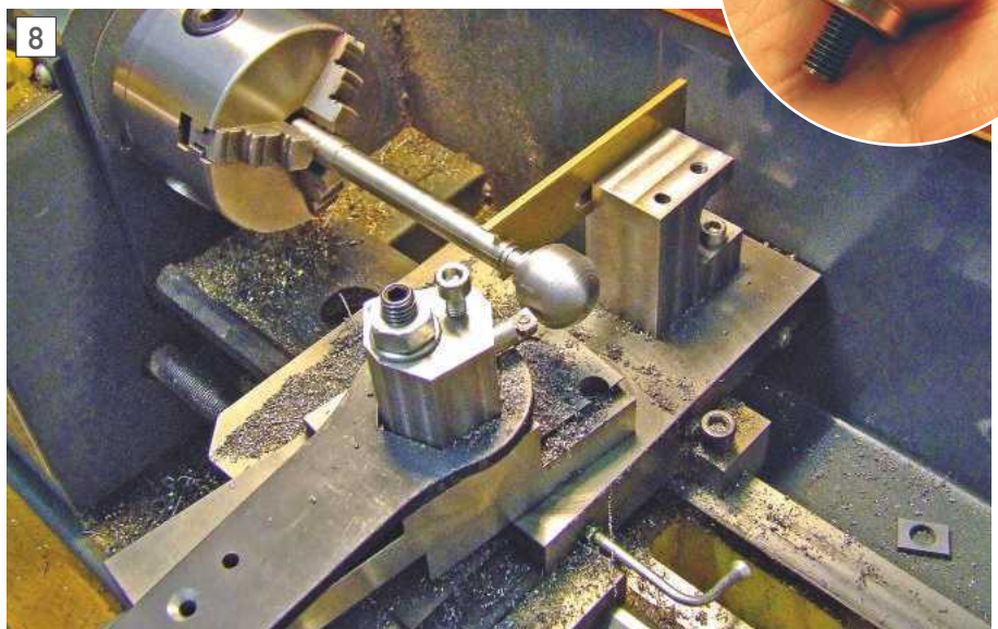
Set-up for turning a ball using a rear steady for support.
