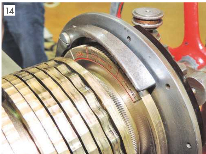
The rose engine's cams and micro-adjustment.
