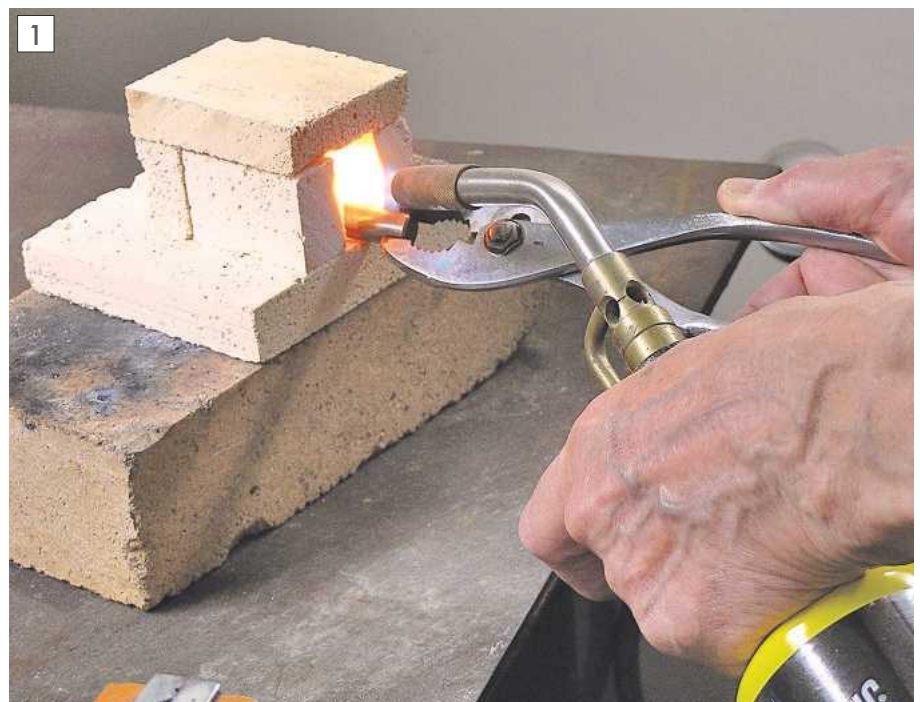
A mini-kiln for heat treating.
