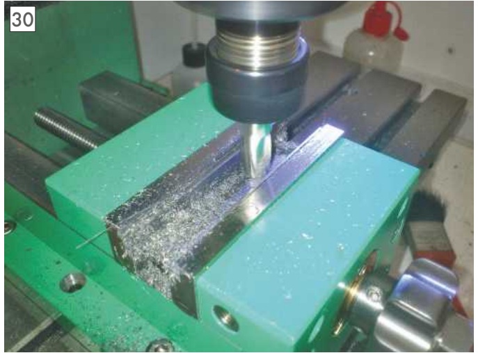
Milling steps in the jaws.
