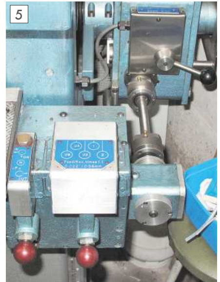
The power feed gearbox.
