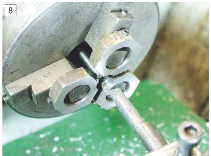
Boring a recess for the sprockets.
