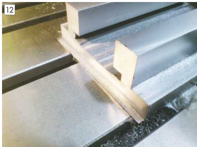
Machine the base sides, careful not to touch the milling bed!
