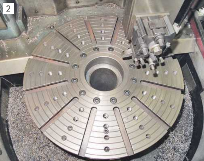
The lathe's large faceplate.
