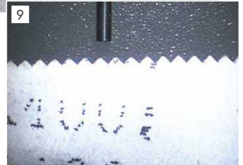
The cut edge compared against the shank of a 1 mm drill.
