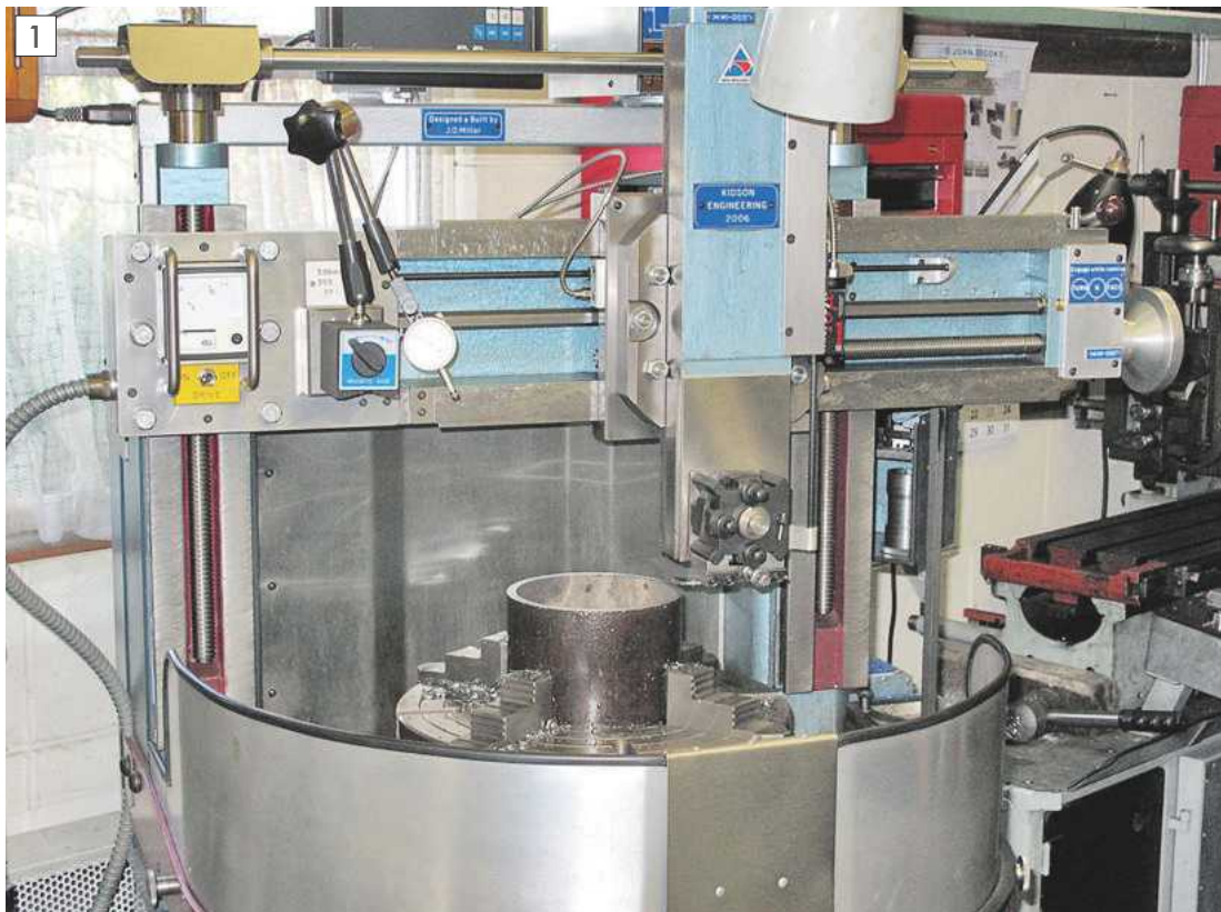
Jock Miller's shop-made vertical lathe.
