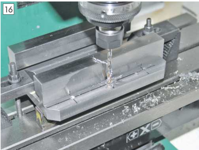
Drilling the mounting holes whilst raised off the milling bed.
