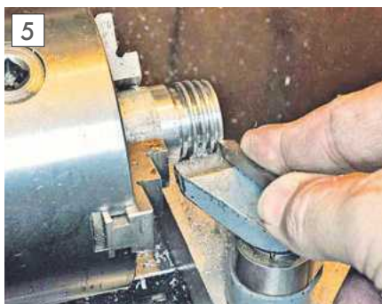
Using a hand graver to round the fins on a Dyno replica cylinder head.
