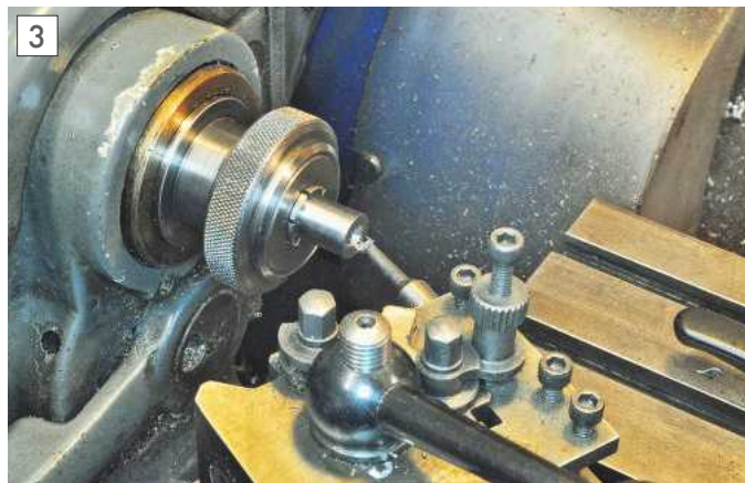
Turning a centre in silver steel held in a Myford Patent collet.
