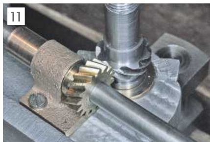
Helical gears driving the cam shaft on Wyvern gas engine.
