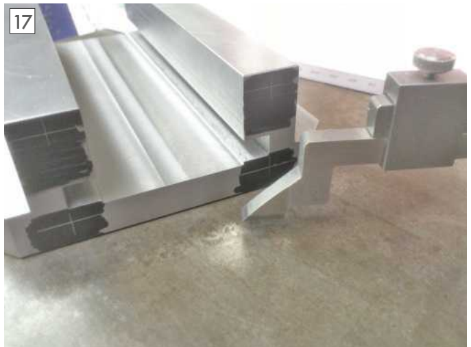
Marking out the mounting holes using a height gauge.
