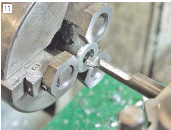
Boring a washer to size.
