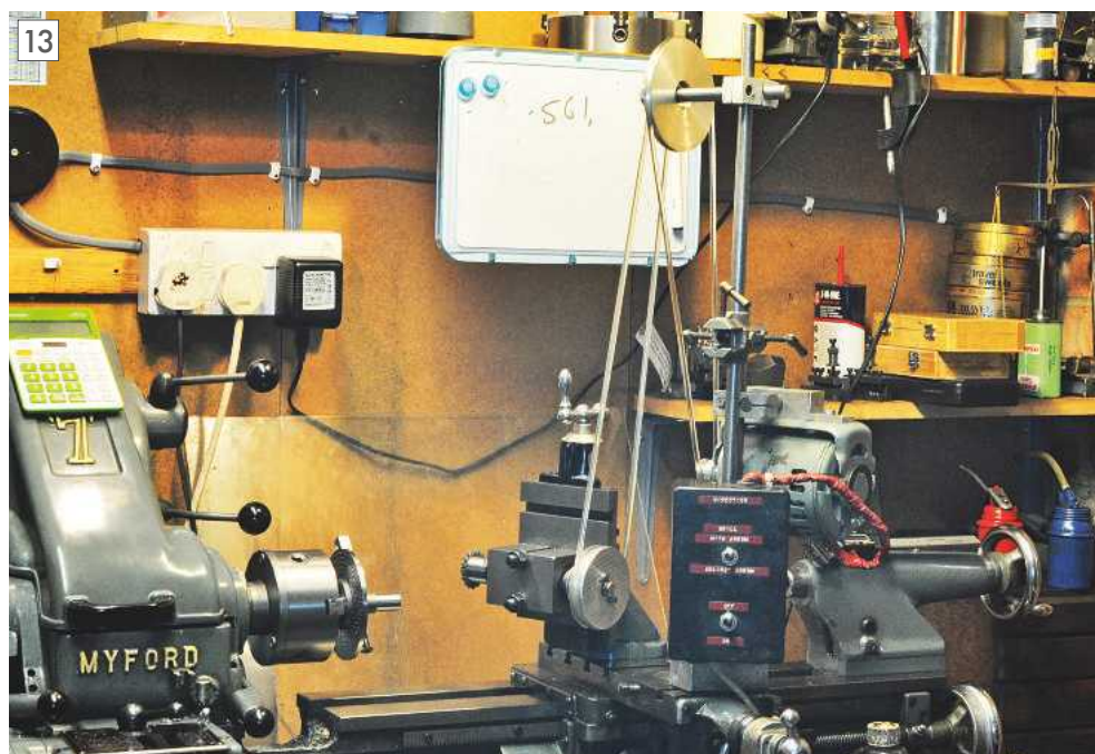
Boring the Wyvern cylinder using a fixed steady and tool held in the Gibraltar toolpost.
