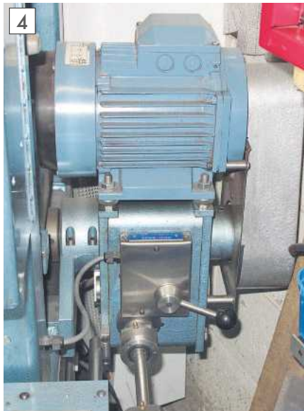
The motor sits above the gearbox.
