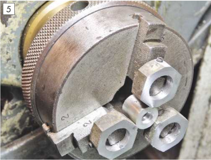
Using a spacer to hold the jaws open.
