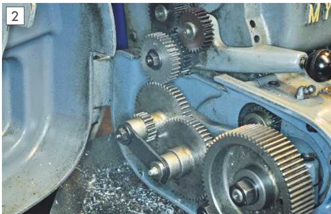
Standard gearbox banjo showing the cluster gear in the middle which is reversed for fine feed and a 34t gear on the tumbler stud for a metric thread.
