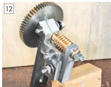
Purpose-made worm attachment for more complex dividing.
