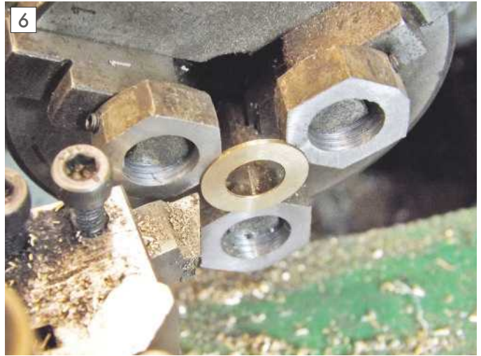
Facing a washer held in the 'soft jaws'.
