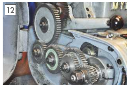
Gearbox banjo set up to give a lead of 0.885 inches for cutting a helical gear.
