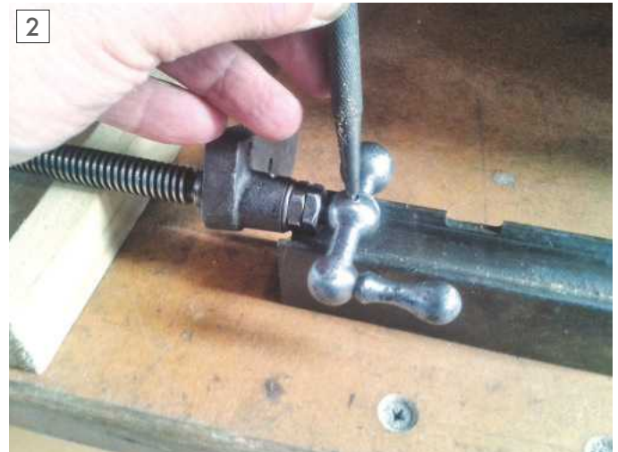
Removing the tapered pin in the handle.
