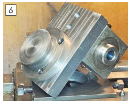
Milling spindle base fits in the top slide spigot hole.
