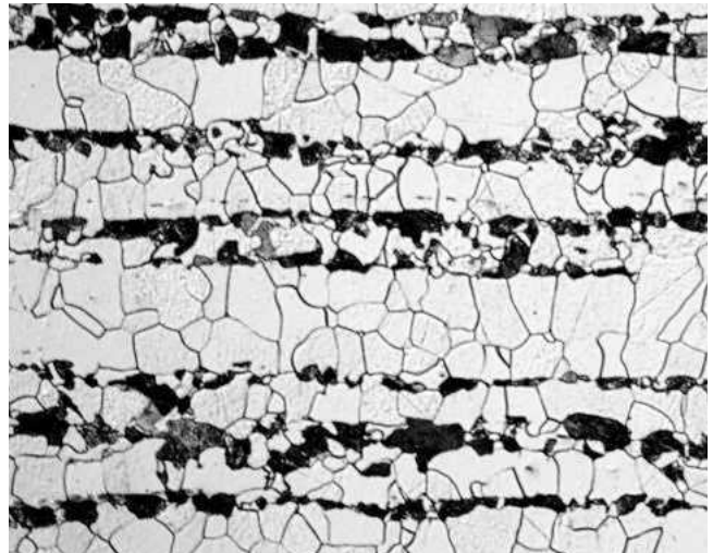
Micrograph 2: Slow-cooled 1018 (240x).
