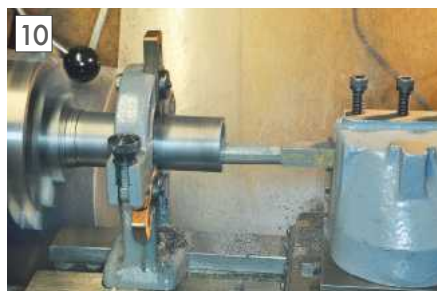
Boring the Wyvern cylinder using a fixed steady and tool held in the Gibraltar toolpost.
