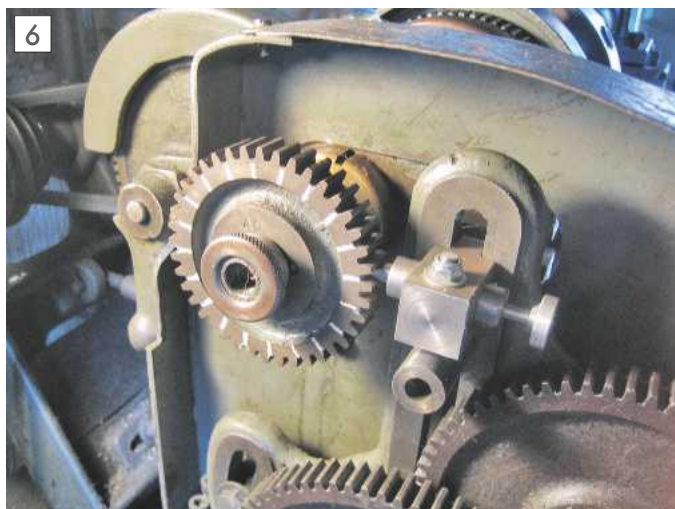
Direct indexing using a 40T gear wheel.
