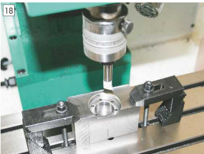
Boring the moving jaw for the leadscrew bush.
