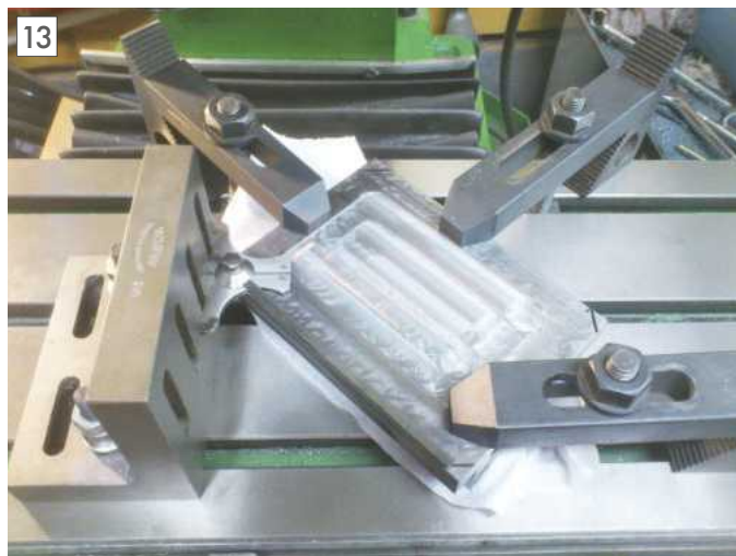
Mark out and mill the chamfers, no need for high precision!
