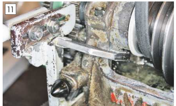
U-shaped clasp locating on the headstock rear bearing housing.
