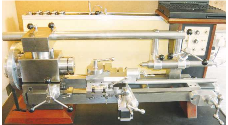
The finished Stepperhead CNC lathe.
