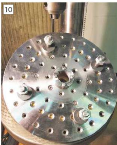
Finished Faceplate from behind. Halved hole on centre plug is just one of my mistakes. Wooden bowl is fastened on faceplate with screws.
