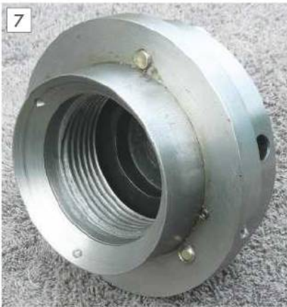
Backplate for ER 25 collets, with traces of a former life.
