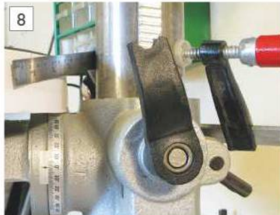
Poor Man's Dividing Head (PMDH). Rule is fastened to drill press pillar.
