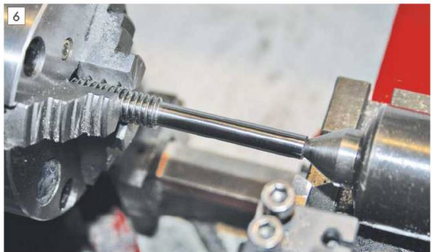
Turning the lead screw shaft.
