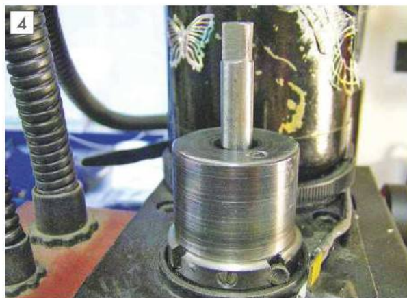
New drawbar and top cap fitted to the mill.
