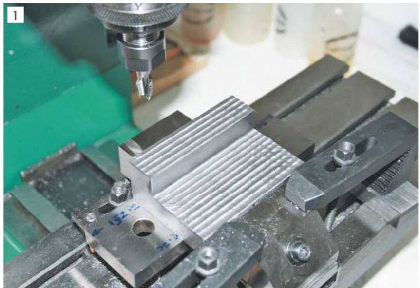
Milling the fixed jaw mating faces.
