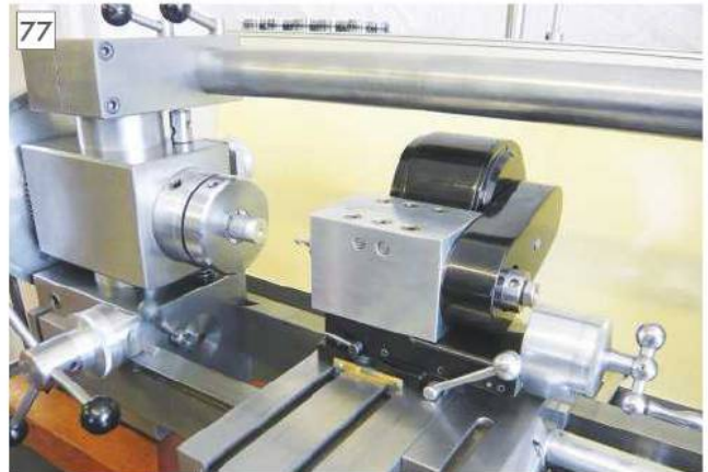
77 Another view of milling head on the topslide.
