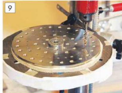
Fastening holes are drilled. Upper plug holes are left from a previous project and serves no purpose on current job.
