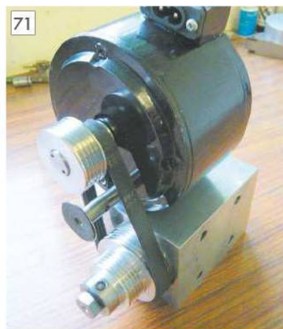
71 Milling head with belt cover removed.
