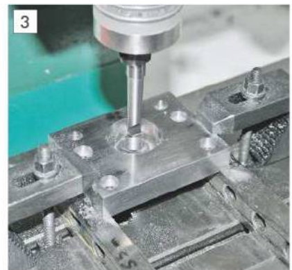
Boring the fixed jaw for the leadscrew bush.
