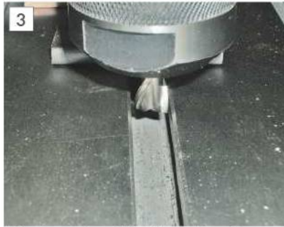
Aligning a slot drill with a table t-slot.
