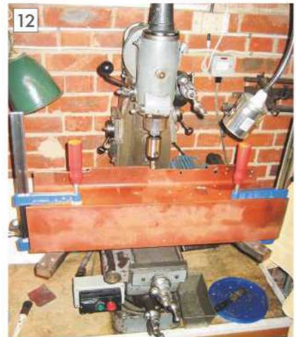
The RSJ mounted on the extension bars for machining.
