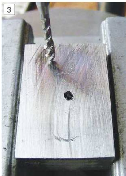
The 2.5 mm hole prepared for threading.
