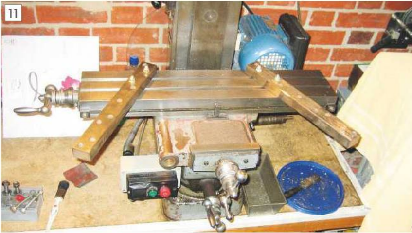
Method for temporarily extending the mill bed.
