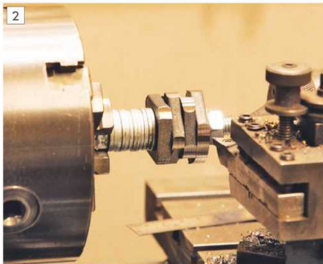
Washerplate billets are turned on M10 bolt in the lathe.
