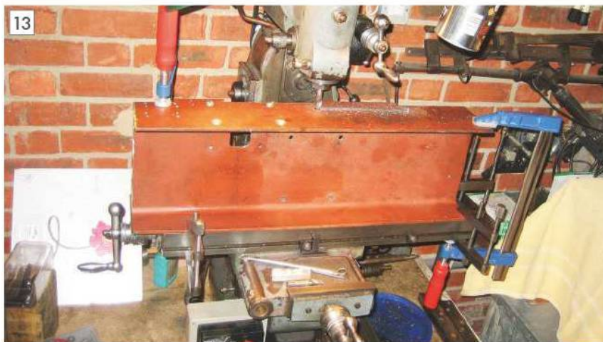
Using a collet to maximise mill headroom.
