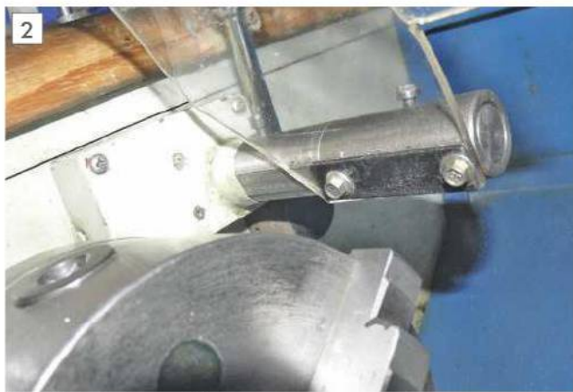
Modified chuck guard fittings.
