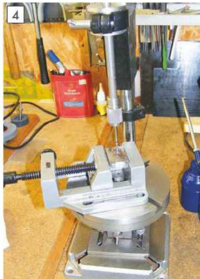
The tap set up in the pillar tool.
