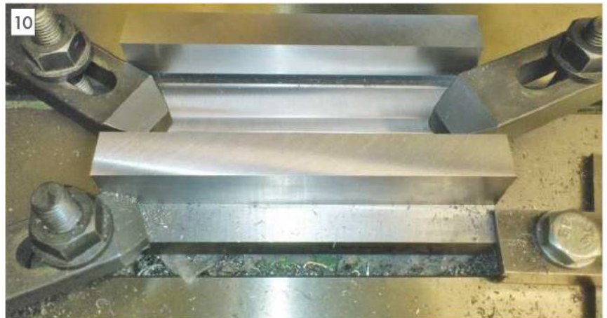
Fixing of the vice base during machining.
