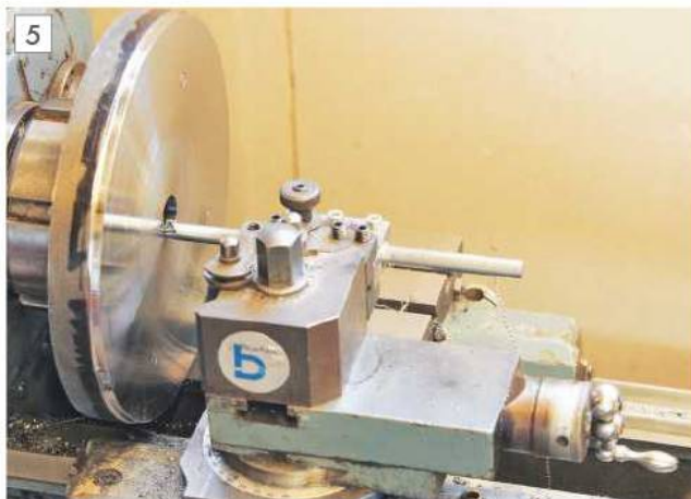
Boring 25mm hole.
