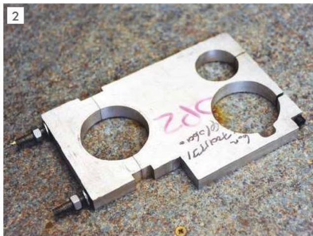
The top of the adaptor plate with an extra hole...
