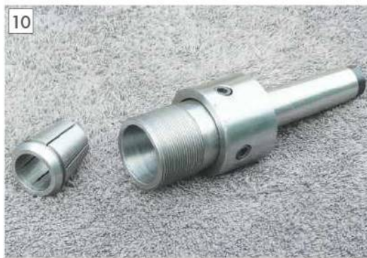
Floating reamer holder with 3MT ER32 style collet.
