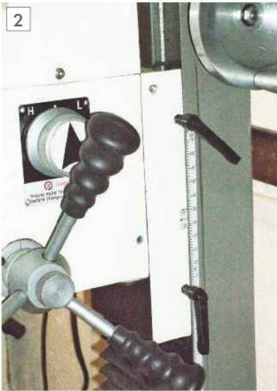
Align the head with the column by eye.
