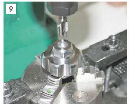
Machining the counterbore.
