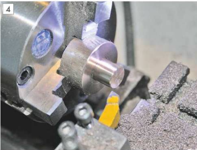
Turning the lead screw bush.
