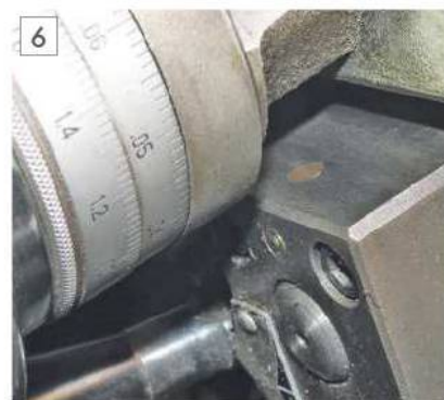
Repositioned ball oiler.
