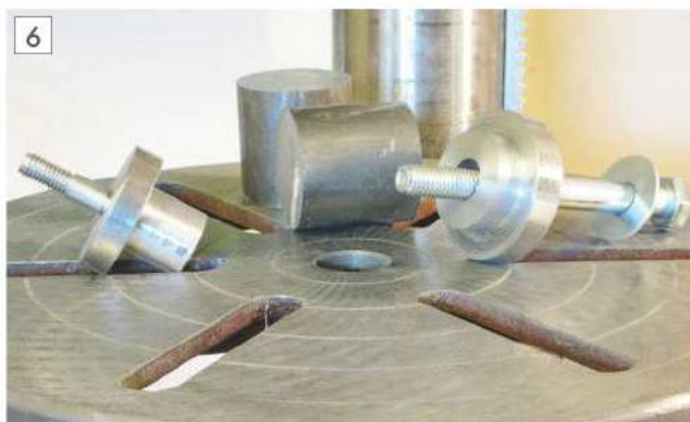
Upper plug and lower plug with bolt. This picture is from a previous project. The upper plug has threaded rod not needed and the two short steel stubs are unnecessary.
