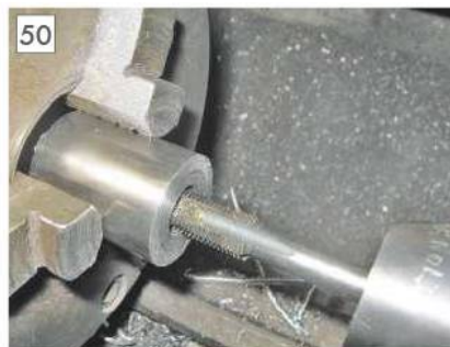
Tapping to fit shaft.
