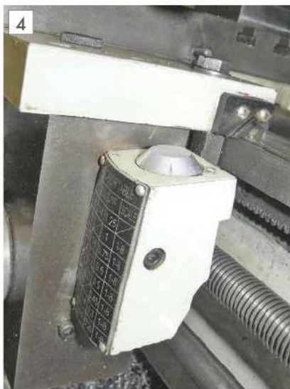
Relocated thread cutting dial.
