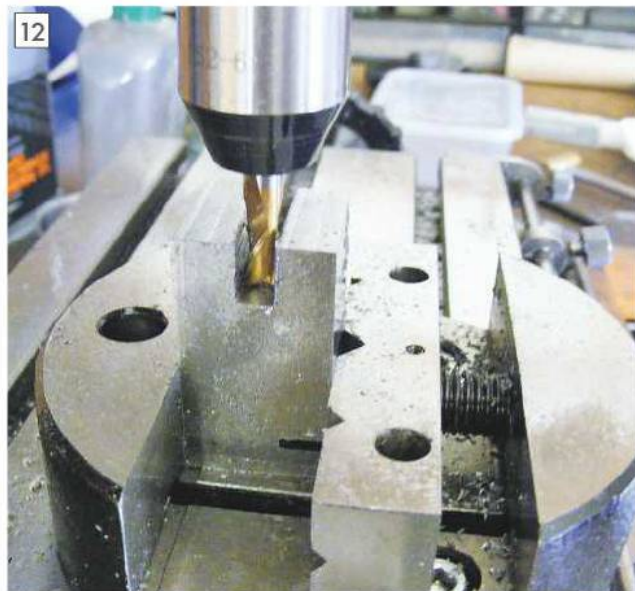
12 Preparing the slot for the cutter.
