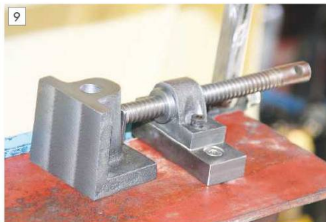
9 A sleeve nut recovered from a broken G-clamp.
