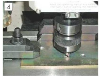
Drilling a hole with minimal quill extension.
