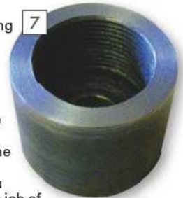
7 Inside of top cap showing 16-tpi left hand thread.
