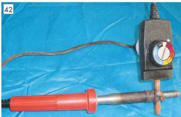
Thermostat monitoring a soldering iron.
