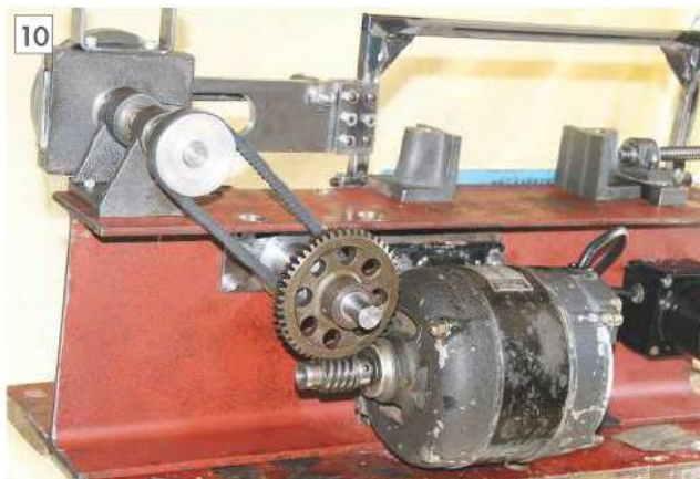
10 First assembly of the hacksaw showing the base from an RSJ.
