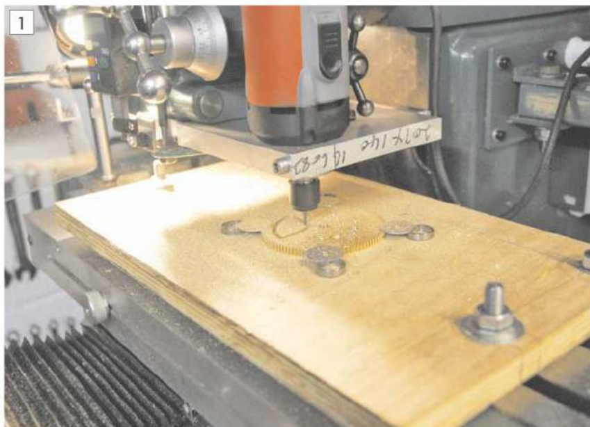
The adaptor plate with the Kress spindle.
