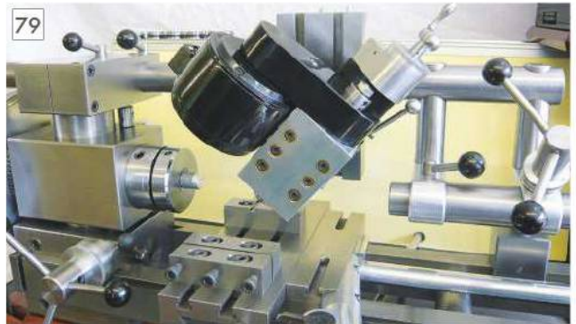
79 Milling head angled on the overarm.
