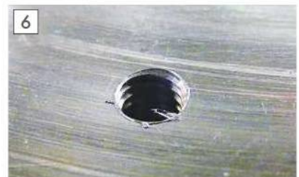
The threaded hole. Note the minimum burr around the tapped hole.
