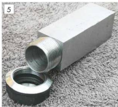
ER 20 drill holder for wooden cutter grinder.
