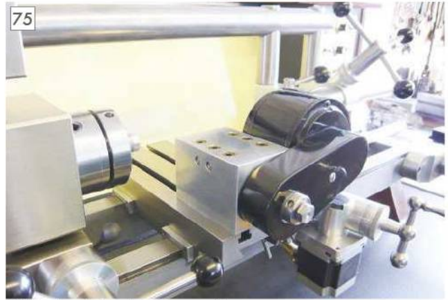
75 Milling head directly on cross slide.
