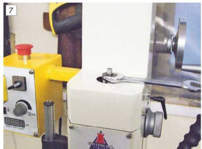
Using a spanner to turn the spindle.
