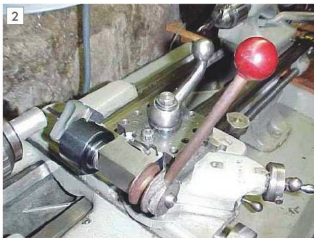
A ball turning tool made from a boring head.
