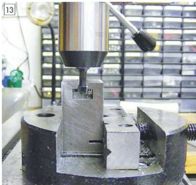
13 The finished tee slot.
