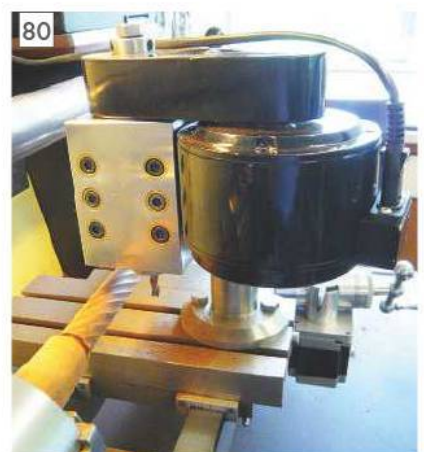
80 Milling head mounted on vertical column.
