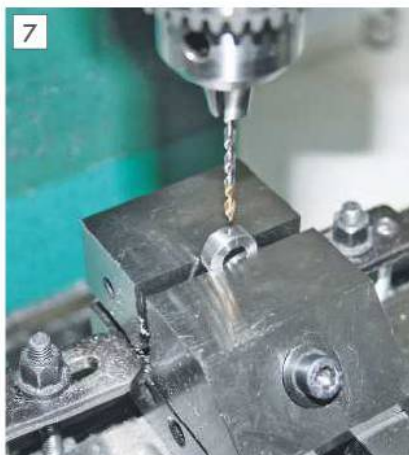
Drilling the leadscrew collet.
