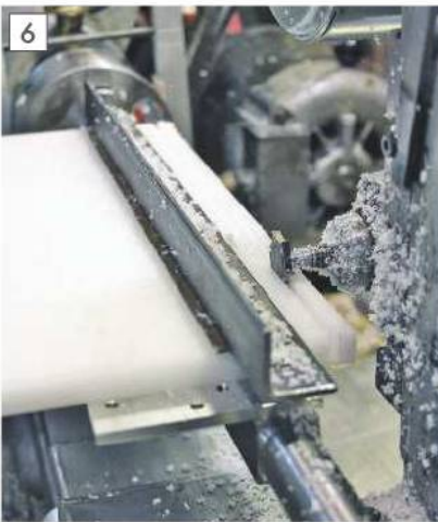
Deep groove being milled in the strip of track links.
