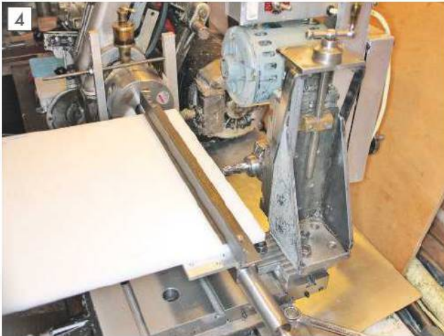
Milling the edge of a large acetal plate to make track links.
