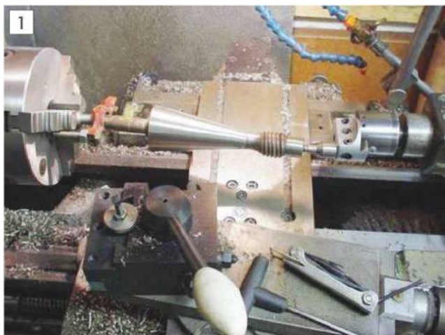
Using a boring head for taper turning.
