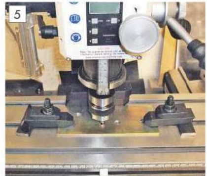
Lowering head with quill at maximum extension.
