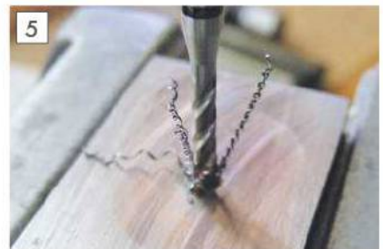
The swarf exits as long coils.
