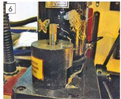
6 Modified spindle end cover, object at lower right is a hall-effect sensor for a tachometer.
