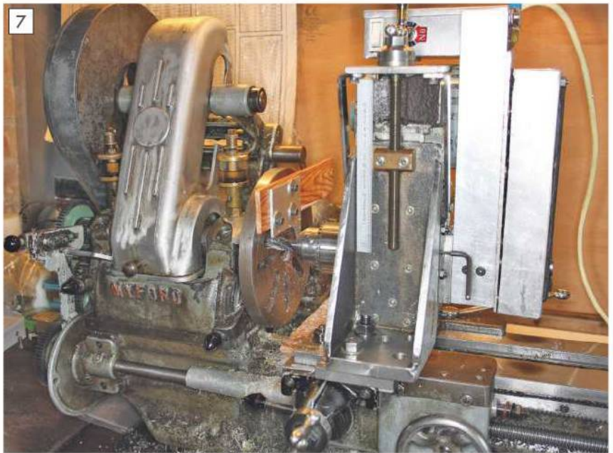
Milling spindle mounted at front of long cross slide for axial milling.
