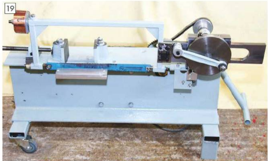
Finished saw showing support platform.
