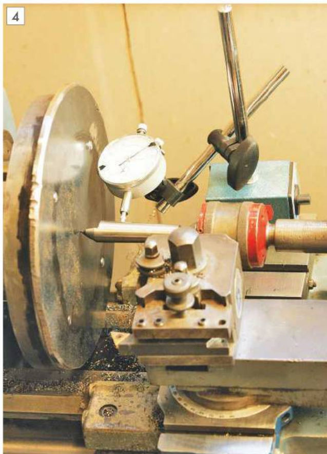
Faceplate is centred with clock and half centre between centre pop.
