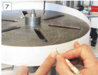
Also from previous project. Paper belt is wrapped around drill press table and two lines are marked to measure its diameter.
