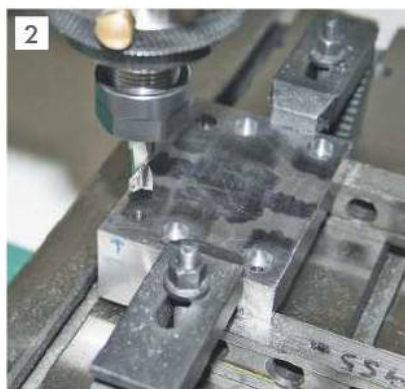
Drilling counterbores in the fixed jaw.
