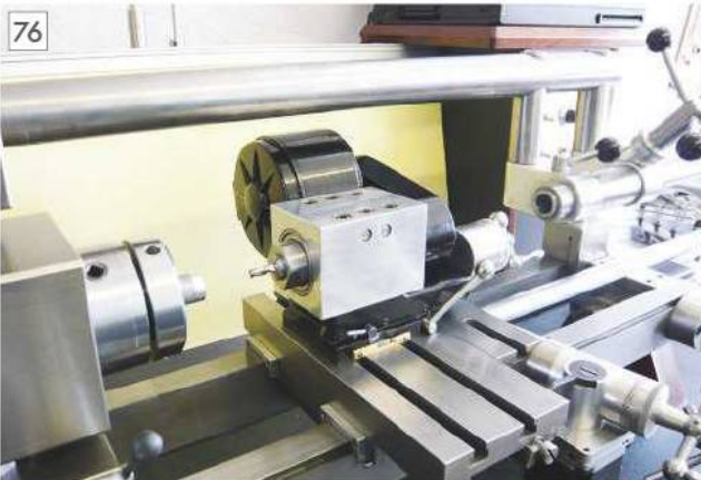
76 Milling head mounted on topslide.
