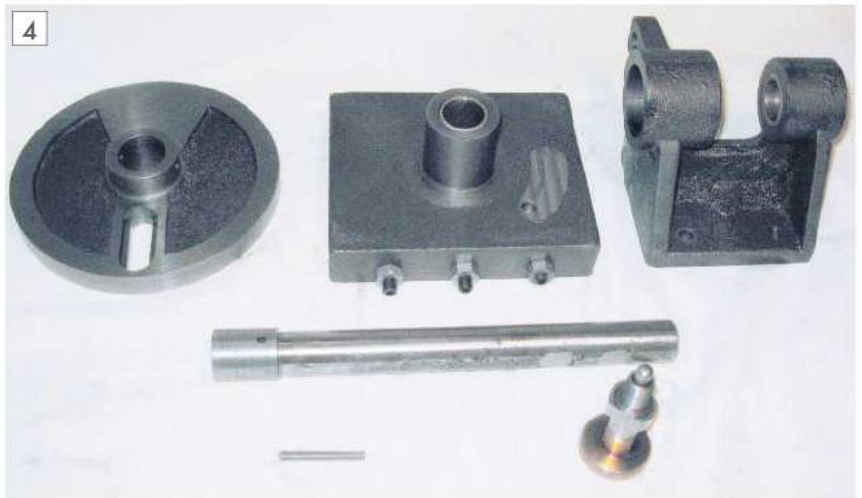
Machined headstock components.
