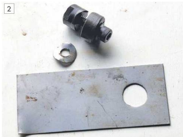
Q Kit punch set with work piece.
