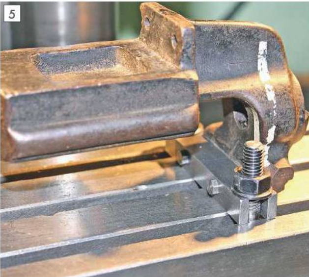
Fastened to the mill using the bar.
