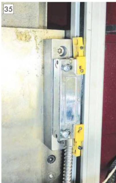
35 The Z axis slider attached to the mounting block. The yellow spacers were removed afterwards.
