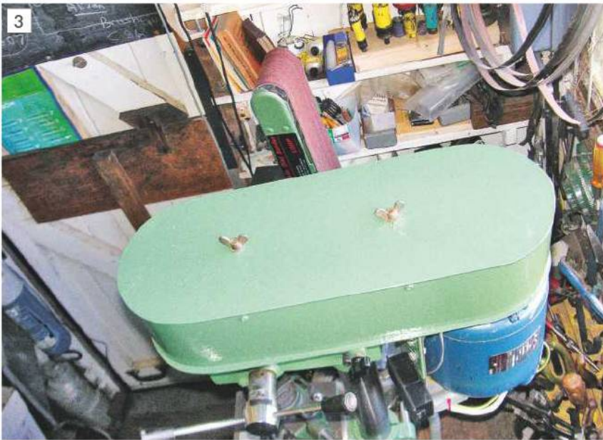
The new belt guard.
