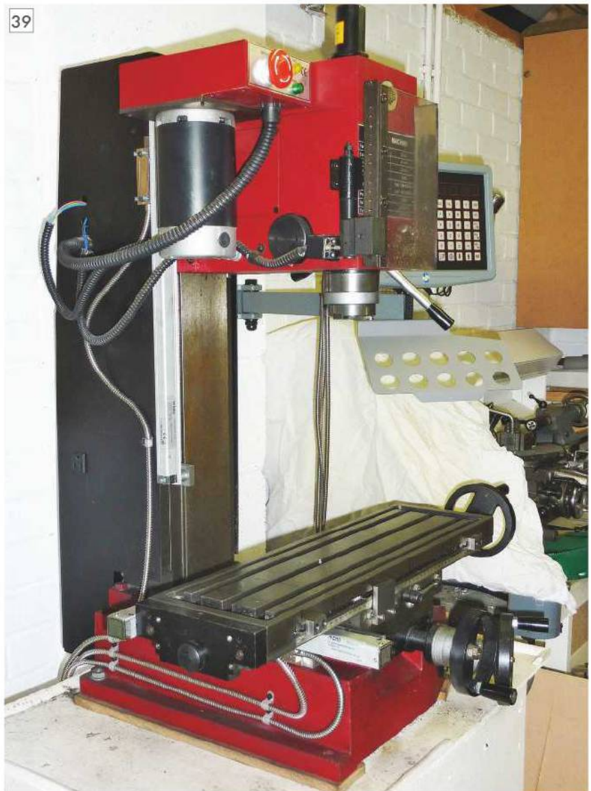
Another view of the X3 with the DRO fitted.
