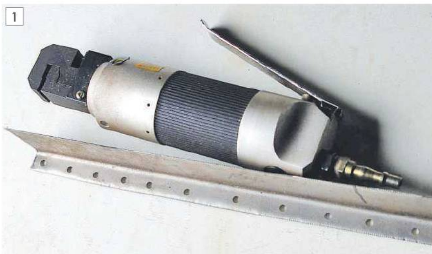
This air powered gadget punches holes or creates joggle.
