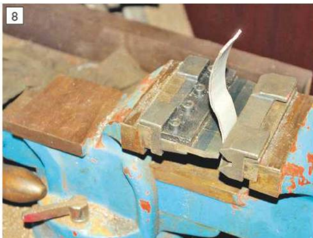
Repeated light bends with the Warco device.
