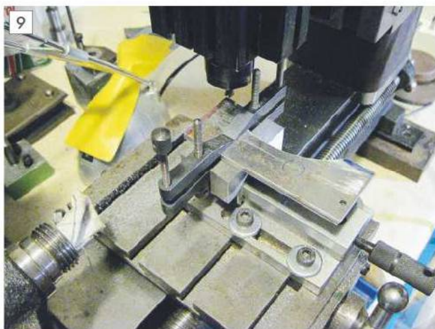
Milling frame spacers to width.
