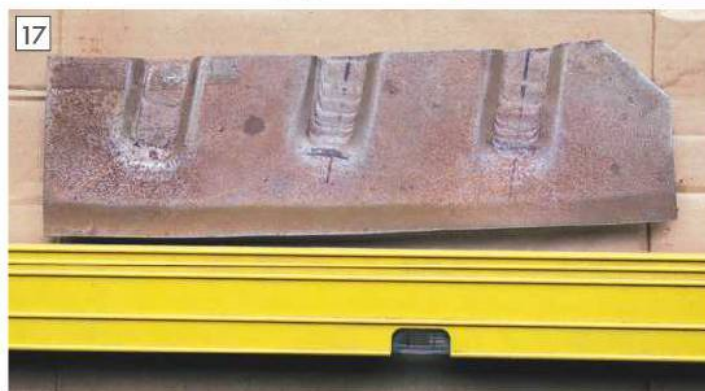
Wrong order of folding caused distorted panel.
