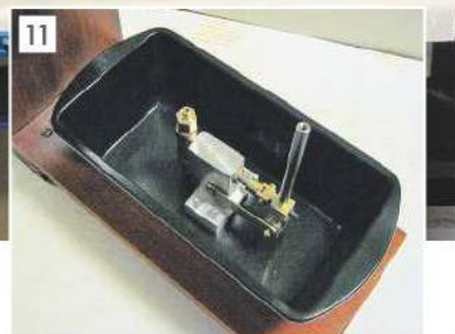
A hydraulic test rig under construction. The pump was built on the EW, as will be the remaining fittings.
