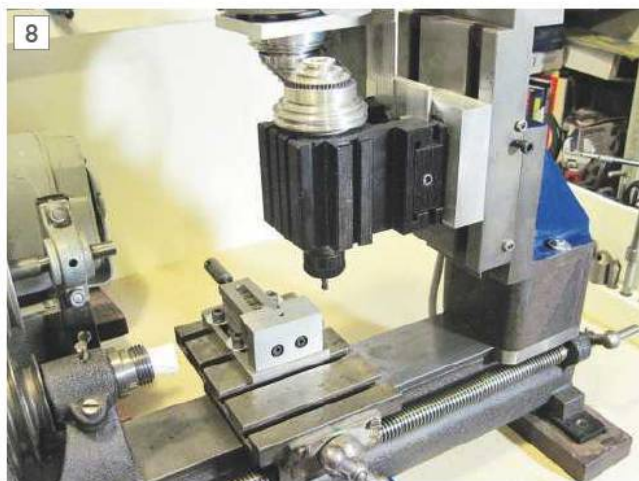
Taig milling attachment clamped to the EW bed.
