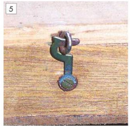
Catch arrangement used for the hinged lid.
