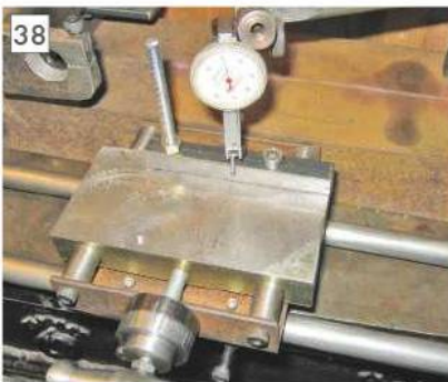
Clocking the back stop
