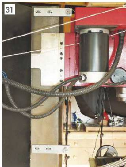
31 The Z axis scale mounting brackets. After this photo was taken, the mounting brackets were lowered by around 50mm. The column cover is loosened and temporarily held in place with string.
