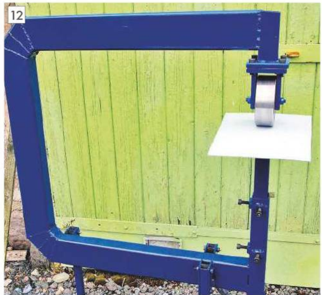
Wheeling machine with slightly domed aluminium workpiece.
