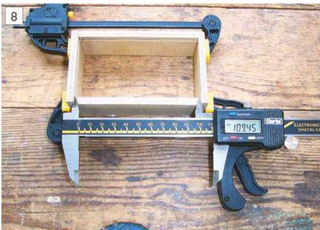
Lid width being measured on the box, dry assembled and clamped.
