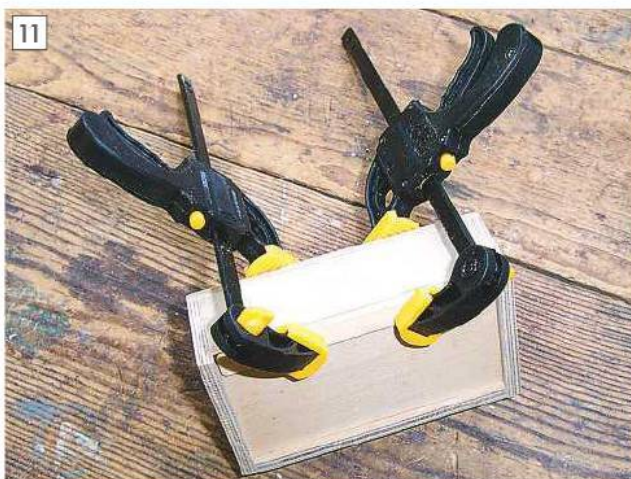
Assembled box with the lid grip glued and clamped in place.
