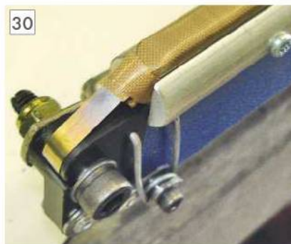
Insulation around the radius 1.
