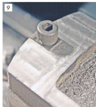
The small area left unmachined.
