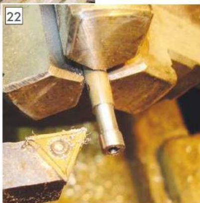
Machining ball spigot.
