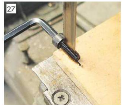
Cutting slot in SHCS - finish.
