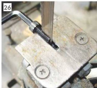
Cutting slot in SHCS - begin.
