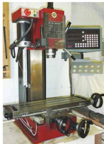
The X3 milling machine with DRO system installed.
