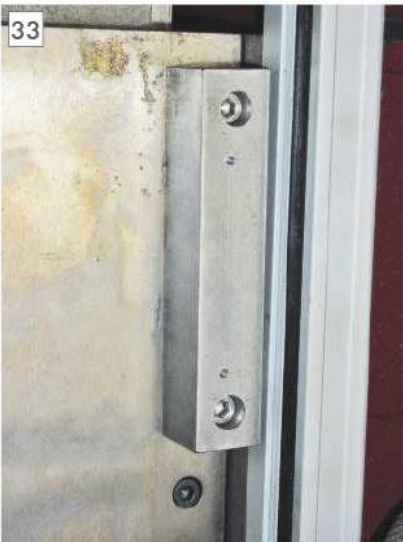
33 The mounting for the Z axis slider.
