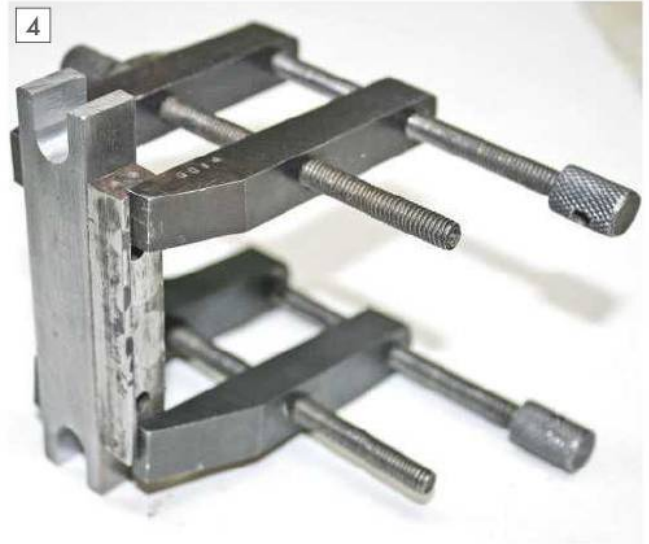
Using the loose jaw to align holes.
