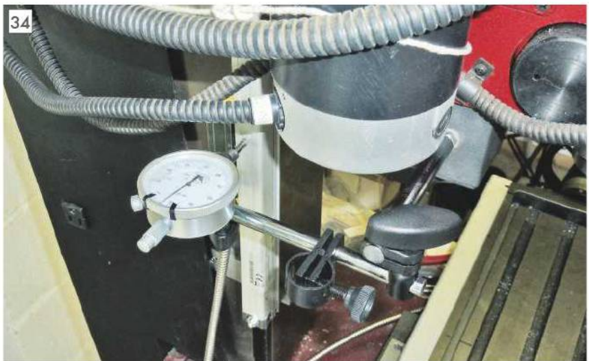
34 Checking the alignment of the side face of the scale. The back face was checked in a similar fashion.
