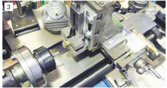
Milling with the vertical slide and ER32 chuck.
