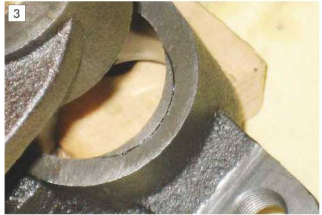
How a boring error was corrected.
