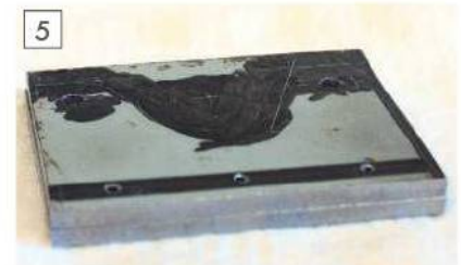
Marking out the side plates.
