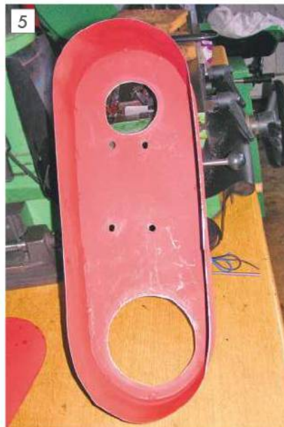
Base of the new belt guard showing tack welds.
