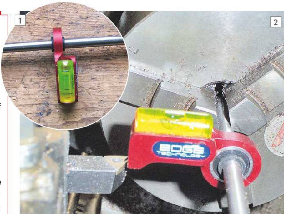
Lathe Tool Height Setting Gauge in use. INSET: View of the Gauge.
