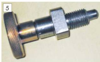
The ram guide support plunger.
