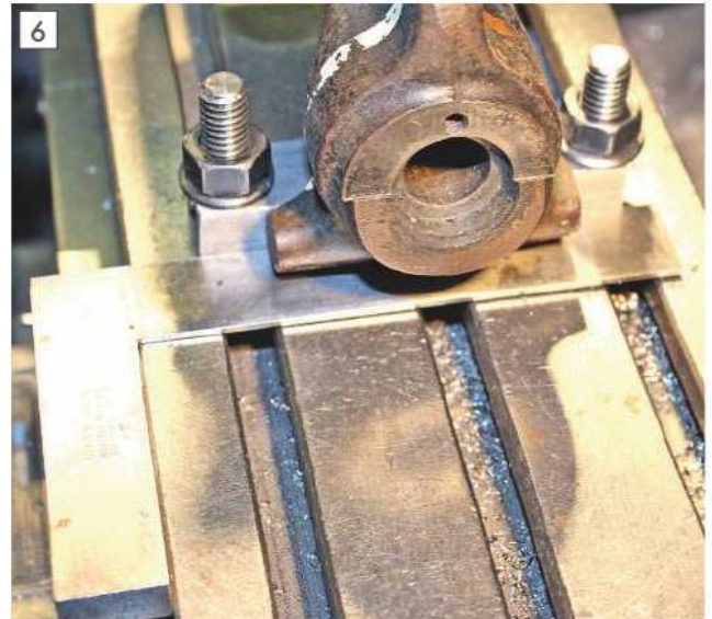
Using a set square to align to the mill table.
