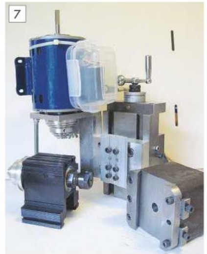
Major units of the Taig milling attachment. ➤
