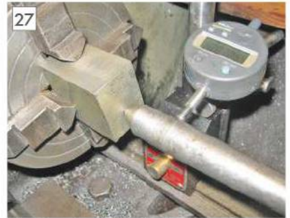
Clocking the tap holder body.
