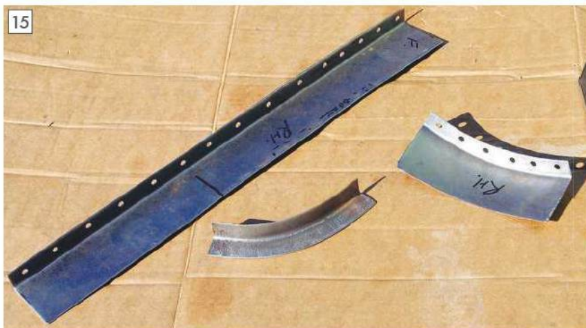
15 Three patch panels, one folded and punched, two folded then curved on the stretcher/shrinker.
