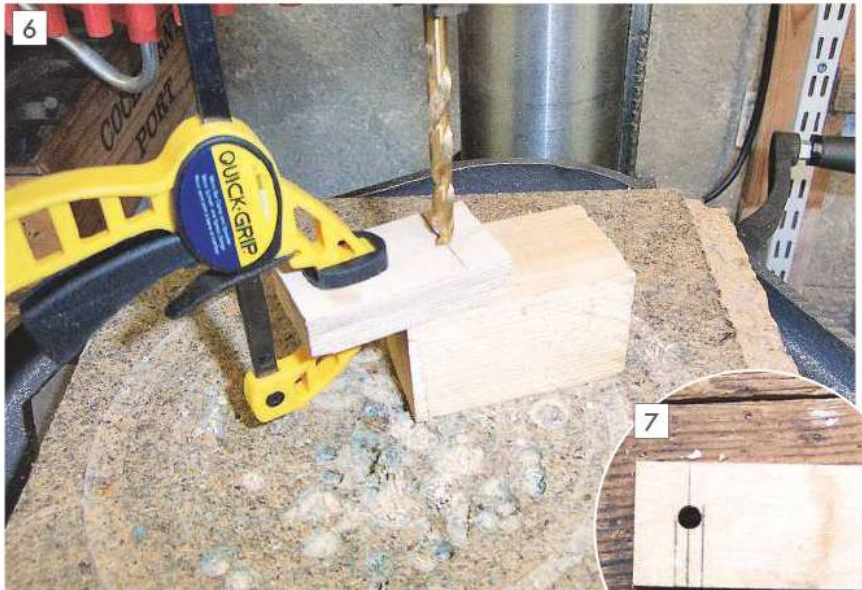
Drilling the \frac{1}{4} inch hole in both inserts simultaneously. INSET: Insert marked ready for sawing to provide the openings.
