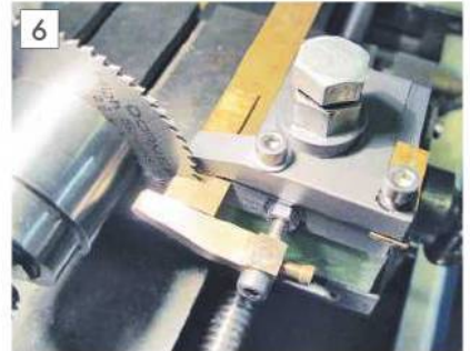
Sawing brass sections with the depth stop.
