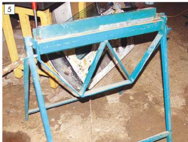
Home made sheet metal bender.
