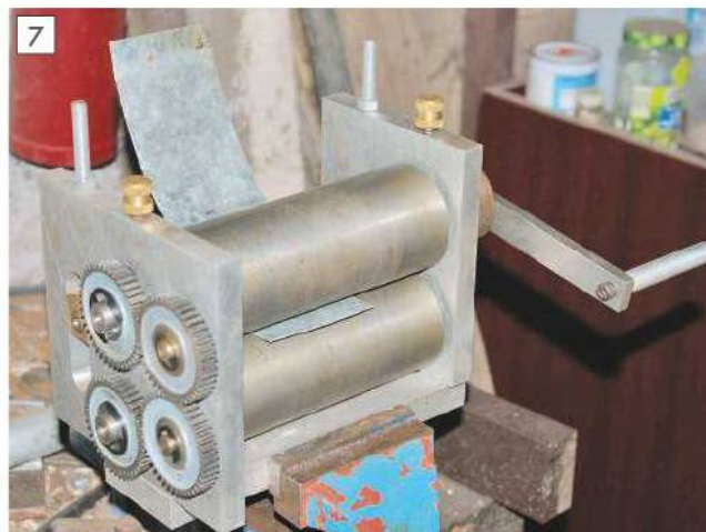
Small set of home built rolls.
