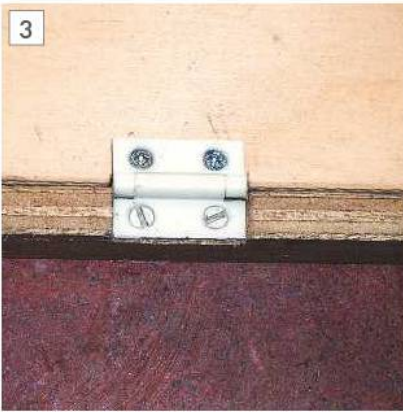
An alternative hinge arrangement for the lid.
