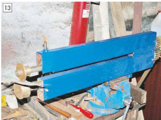
13 Bead roller with dies for folding up a flange.
