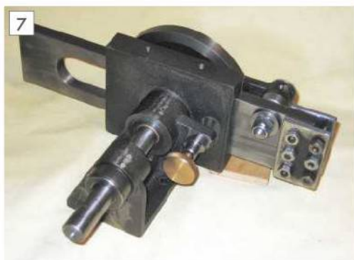
The ram mounted on the headstock.
