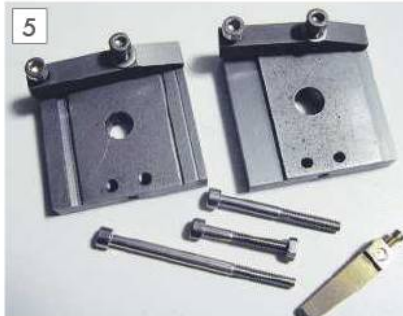
Two sawing tables (for round and flat stock) and their accessories.
