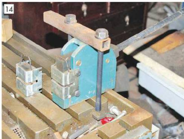
14 Stretcher/shrinker with second set of dies.
