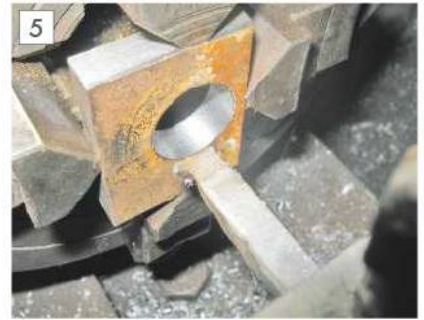
End support boring.
