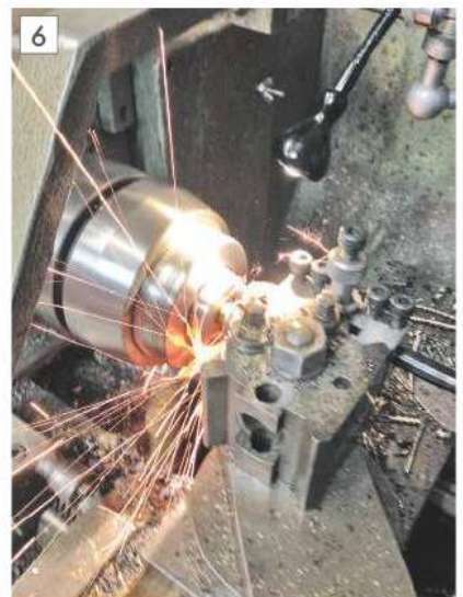
Machining hardened ballnut.
