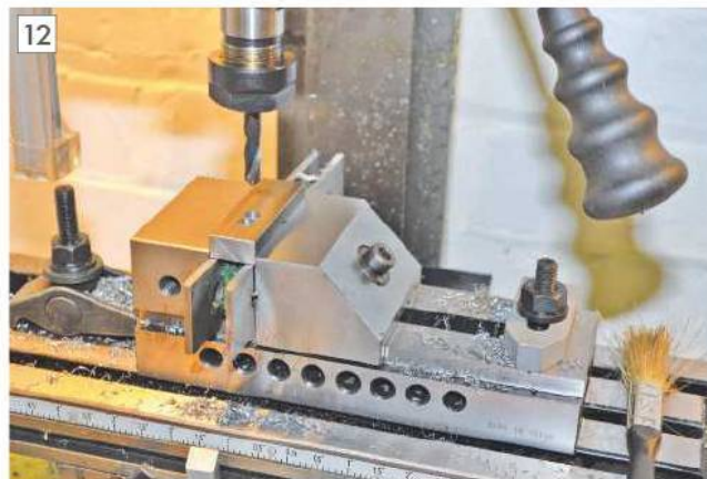
Drilling the end holes.
