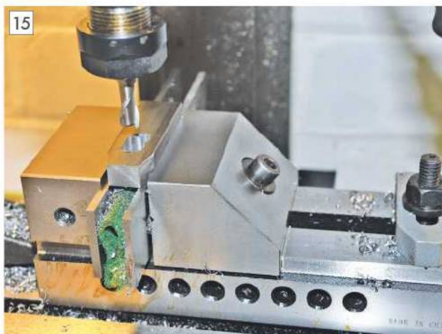
Finally machining the width of the slot.
