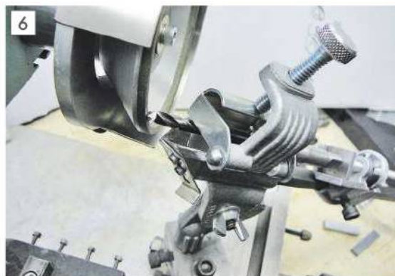
The short 5mm 1MT drill packed with 2 lots of .200 inch Pitters to allow the taper shank to clear the V bed.
