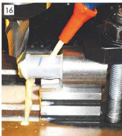
The adapter clamped in a v-block ready for machining.
