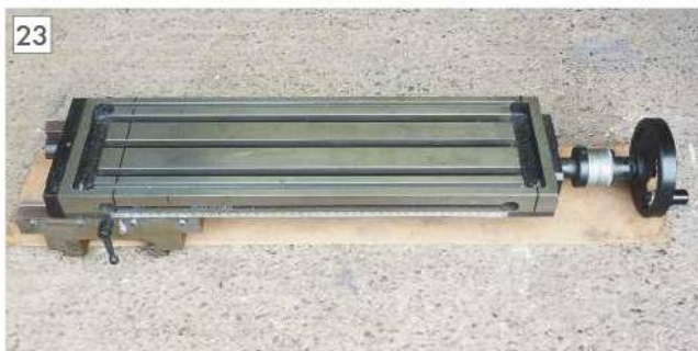
The mill table at one end of its travel...
