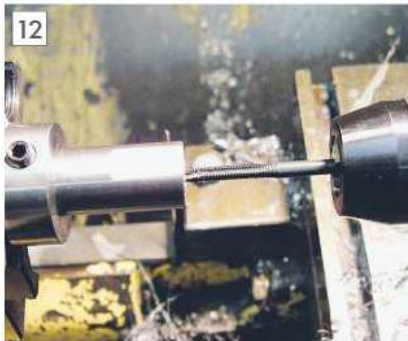
Reverse the adapter and tap the end hole.
