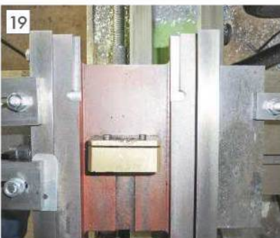
The rebates milled into the saddle to provide clearance and a stop for the modified bearing housing.
