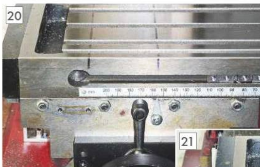
The saddle being set up on the Warco lathe/mill ready for machining. Further clamps were added after aligning the saddle with the DTI.
