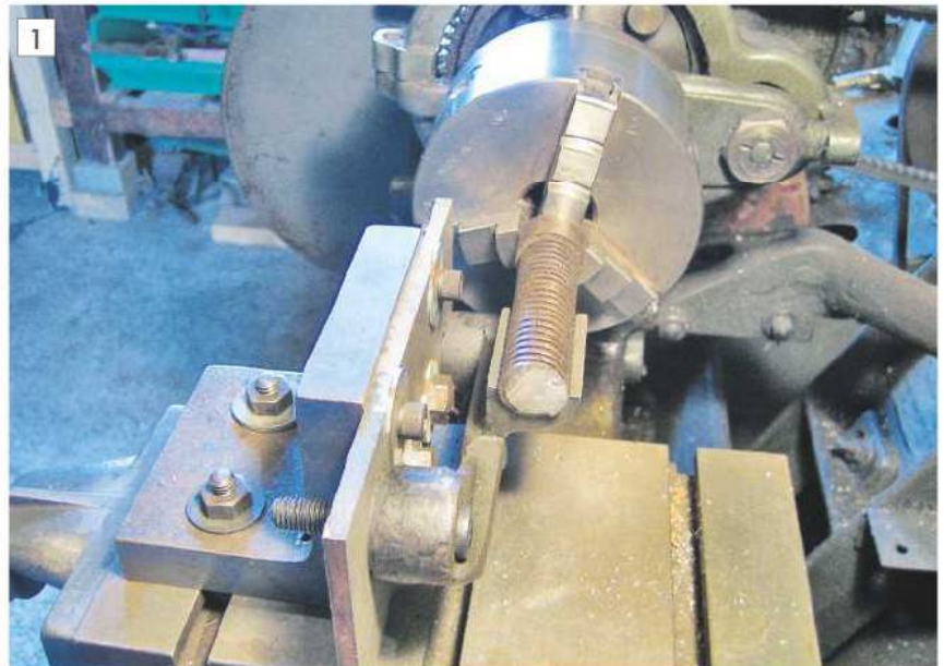
Half nut aligned on the centre line of the lathe.
