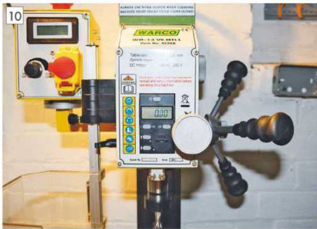
Use the Z readout to see how deep you are going.
