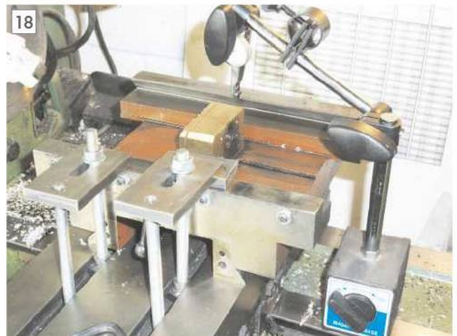
The saddle being set up on the Warco lathe/mill ready for machining. Further clamps were added after aligning the saddle with the DTI.
