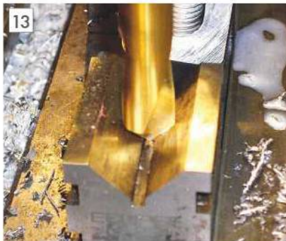
Aligning the v-block with the spindle.
