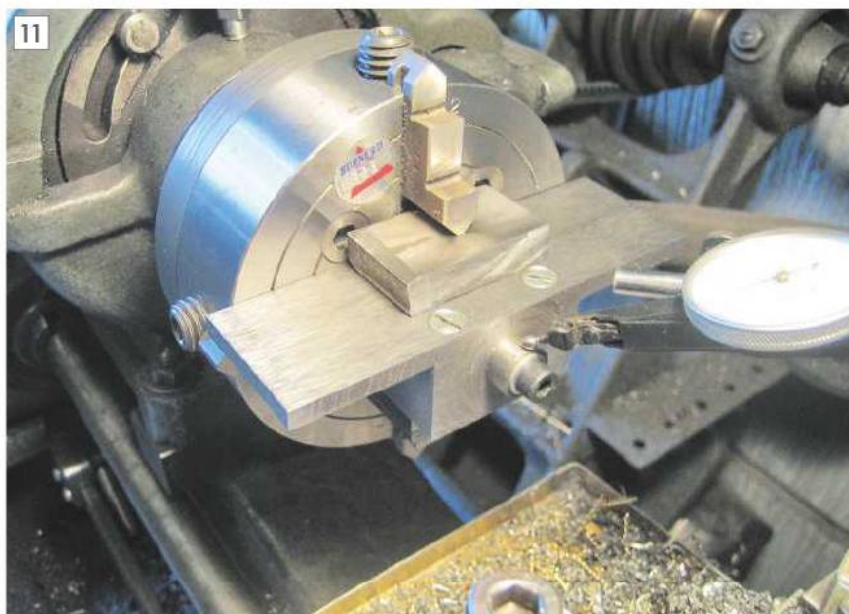
Centring the toolmakers button in the 4 jaw chuck.
