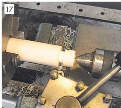
Both faces of the PTFE inner bearing spacer were machined in one operation to ensure parallel faces.
