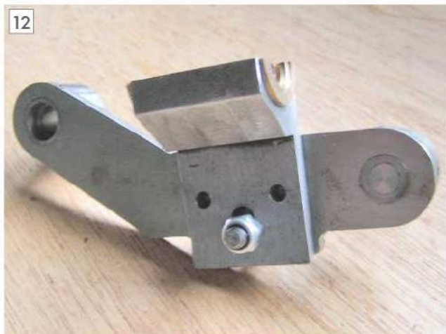
Bracket and bobbin fixed to the arm for setting on the lathe.
