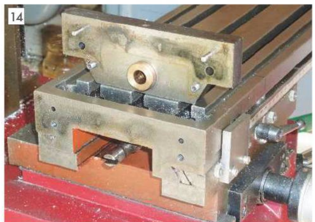
The bearing housing removed from the machine.
