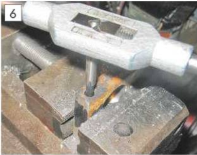
Tapping the clamp thread.
