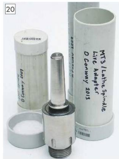
Enclosures made from PVC plumbing pipe and fittings provide excellent protection.
