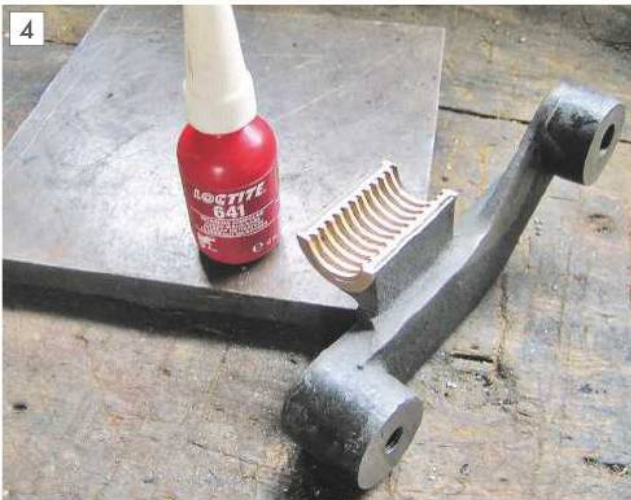
Bobbin secured in place with loctite.
