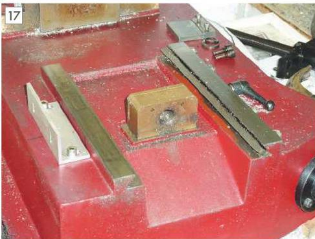
The milling machine with table and saddle removed.
