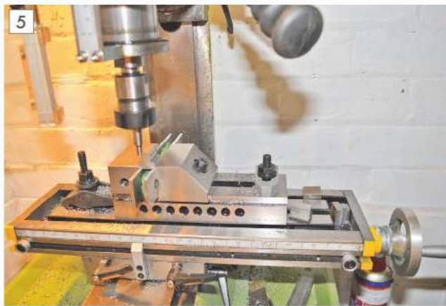
Using a wobbler to find the centre of a hole.
