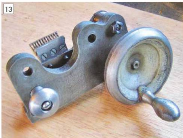
Completed half nut attached to the apron.
