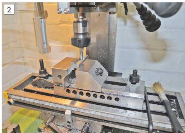
Machining the sides of the tee-nuts.
