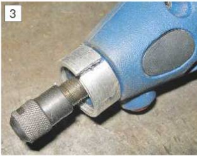
The protective nut fitted.
