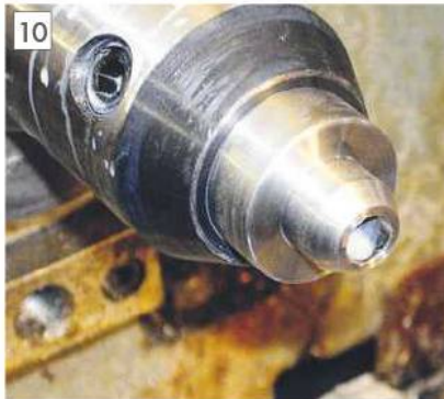
Drill the holder undersize...
