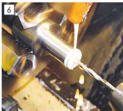
Drilling for the tapped hole.
