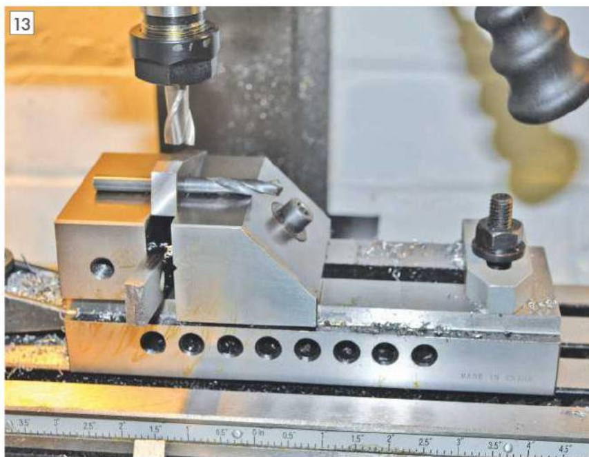
Milling the angles on the end of the clamps.
