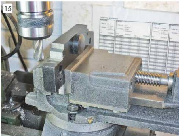
Modifying the bearing housing.
