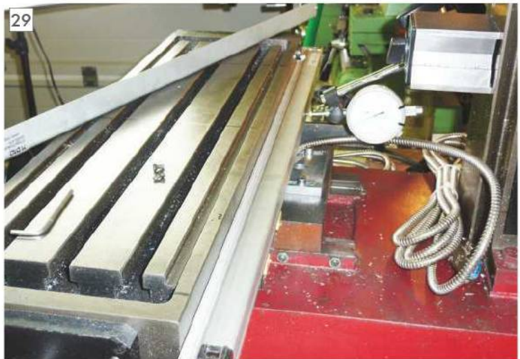
Checking the scale's alignment with the X axis.
