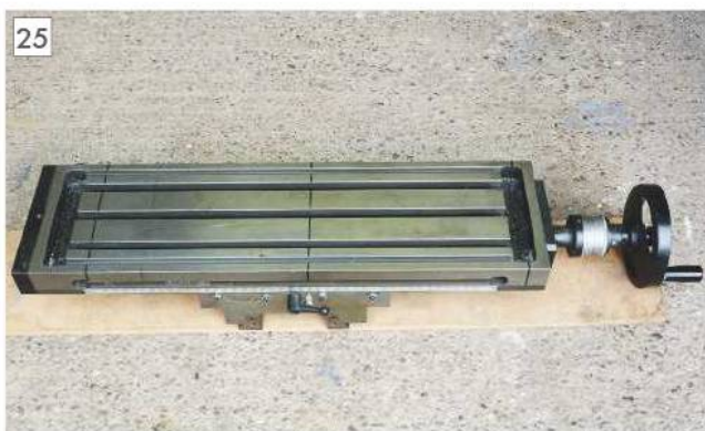
The centre of the X axis travel marked on the mill table. It is easier to fit the X axis scale with the table removed from the machine.
