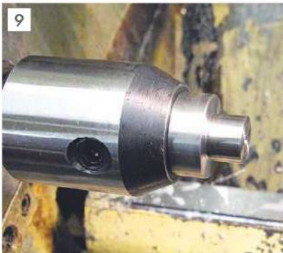
An adapter fitted in the MT3 holder.
