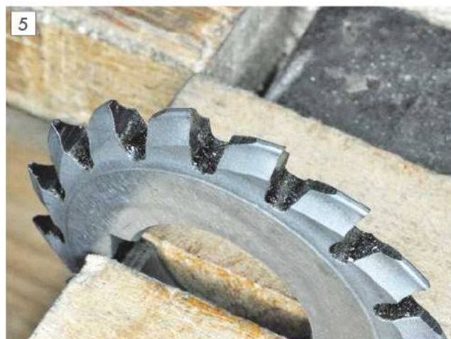
Sharpened tooth face and ground interference on back of tooth.
