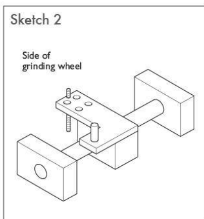
Sketches of suggested simple beds for using the Picador with a bench grinder for 4-facet grinding.
