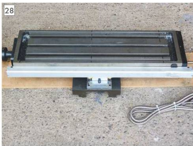
The scale and cover in position on the mill table.
