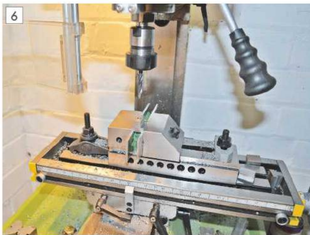
Drilling the tee-nuts.
