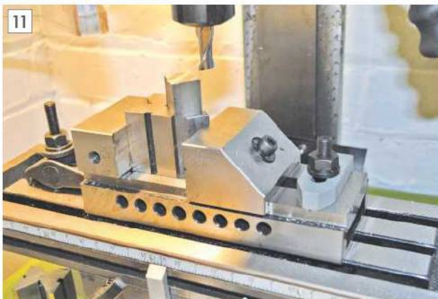
Milling the ends of the clamps in a vee-block.
