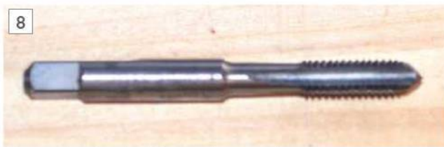
The tap showing the difference between the original and extended flat.
