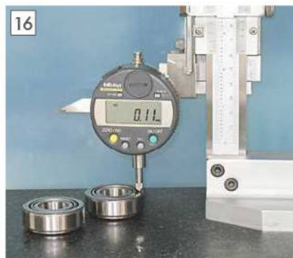
The inner and outer bearing races were compared to determine the correct spacer widths.
