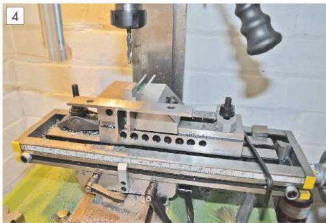
Using a parallel against the vice as an end stop.
