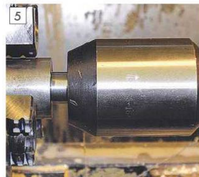
The adapter tail is a close fit.
