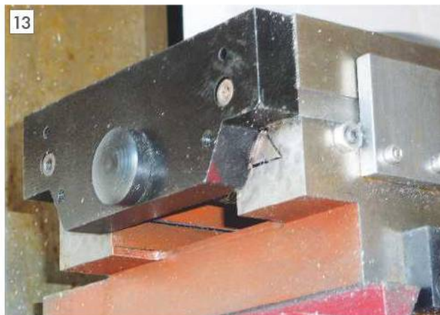
The leadscrew bearing housing, showing how it fouls the end of the slide and limits X axis travel.
