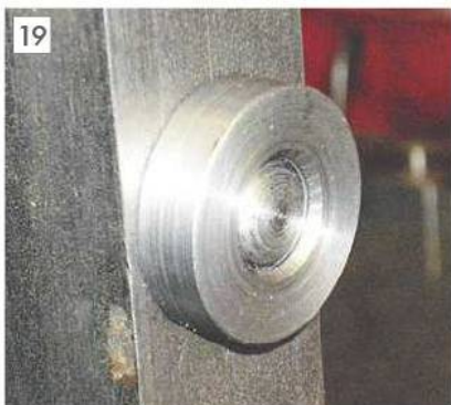
Checking the fit of the mounting collar.
