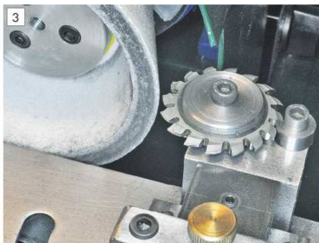
Cutter mounted on Worden toolholder.
