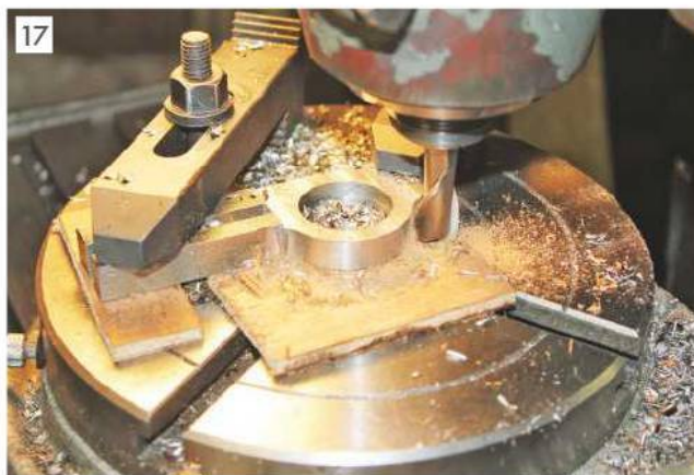
Profiling the work on the rotary table.
