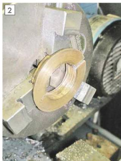
A temporary collet from a plumbing fitting.
