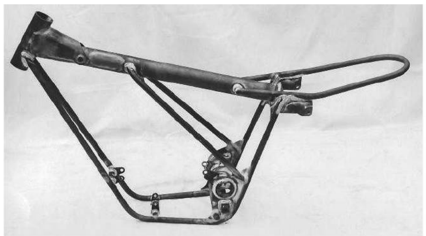
Norton Villiers Trials Scrambling frame from March 1968, with a large single top tube.
