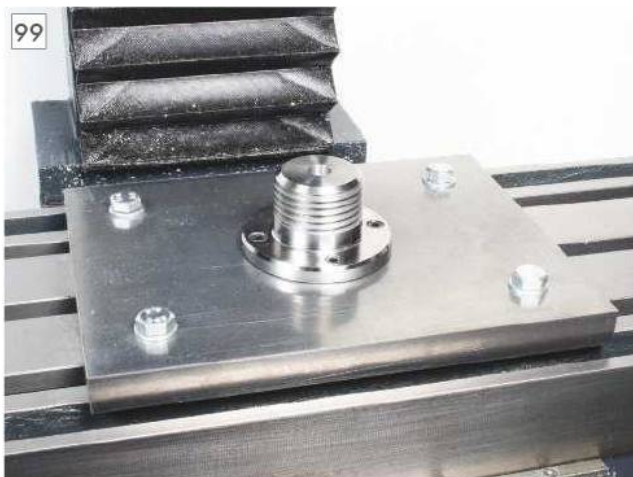
A plate-mounted chuck spigot...
