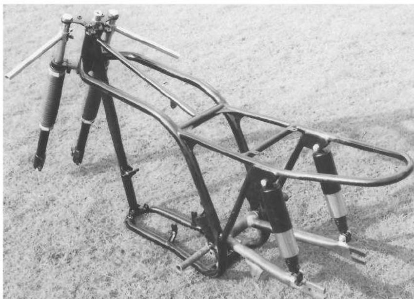
A 1958 Reynolds Duke Velocette frame of duplex design with a single downtube.
