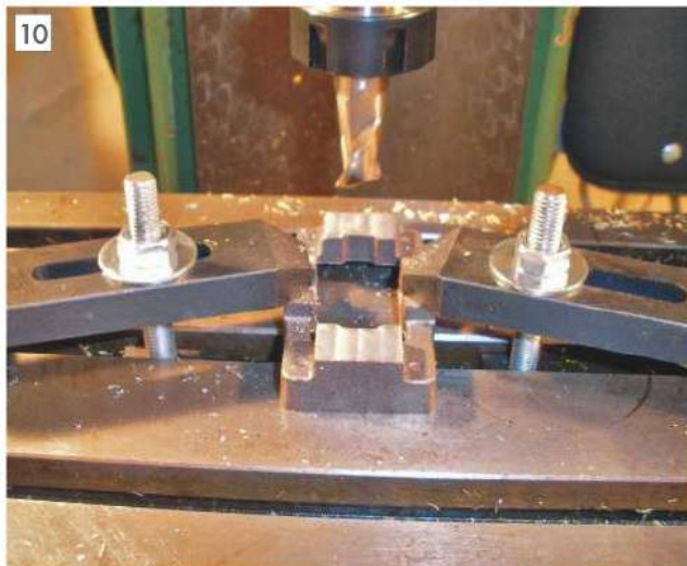
10 Milling the standard mounts.
