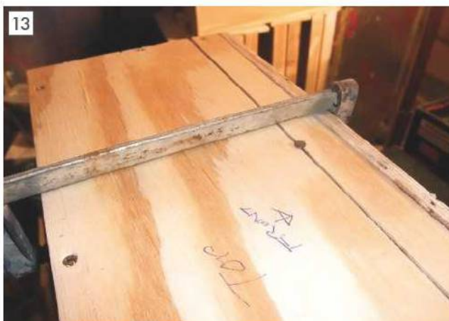
Using a spacer and clamp to maintain both rigidity and a gap.
