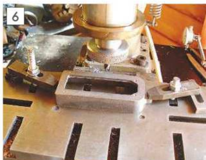
6 Box bed clamped to the mill.
