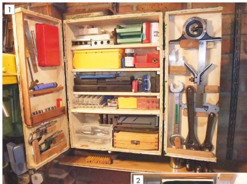
Milling machine tools in cabinet with storage in doors.
