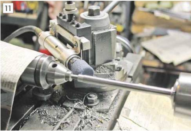
Grinding the shaft to size.
