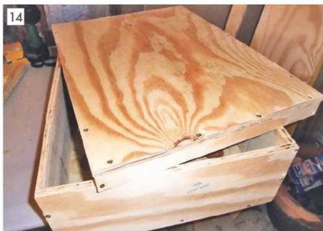
The door cut from the main box.
