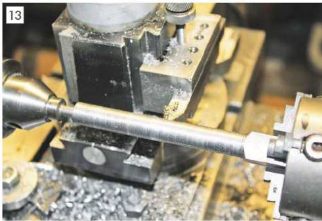
Roughing the support column.
