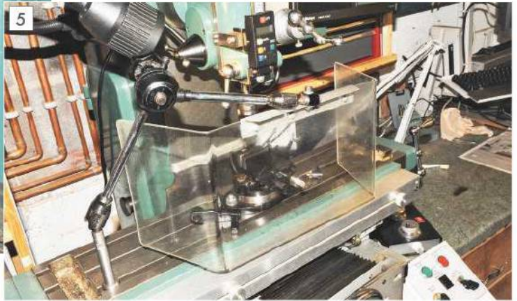
Acrylic guard fitted to milling machine.
