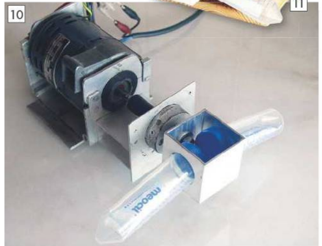
The simple working parts of the centrifuge.
