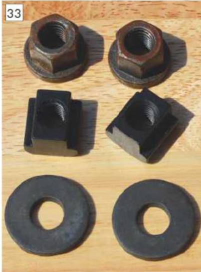
Tee nuts, top hat nuts and washers are required to clamp work and vices down.
