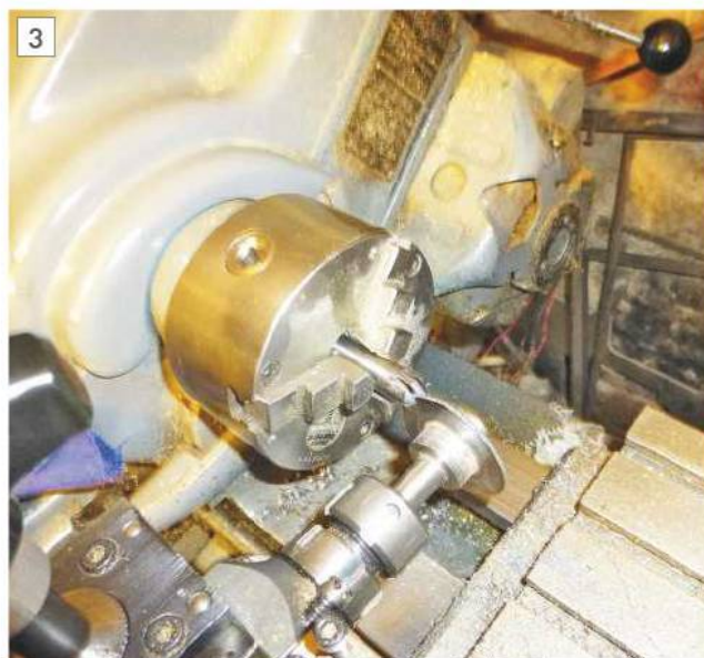
Shaping the tip of the drill.
