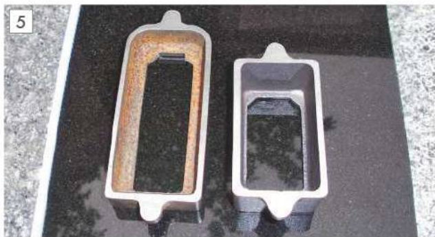
5 Comparing the horizontal and vertical box beds.
