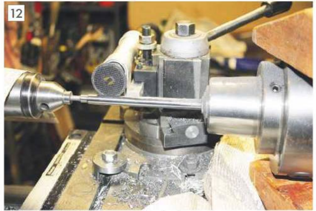
Using a cutoff disc to groove the shaft.
