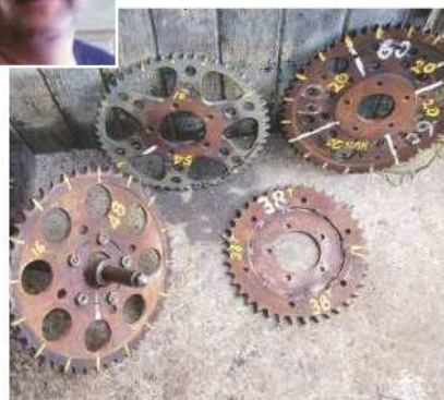
38 and 54 tooth sprockets ease awkward division problems.
