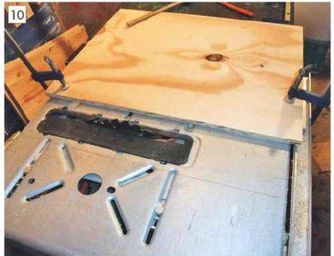
Fence set to correct position for removing front of box.
