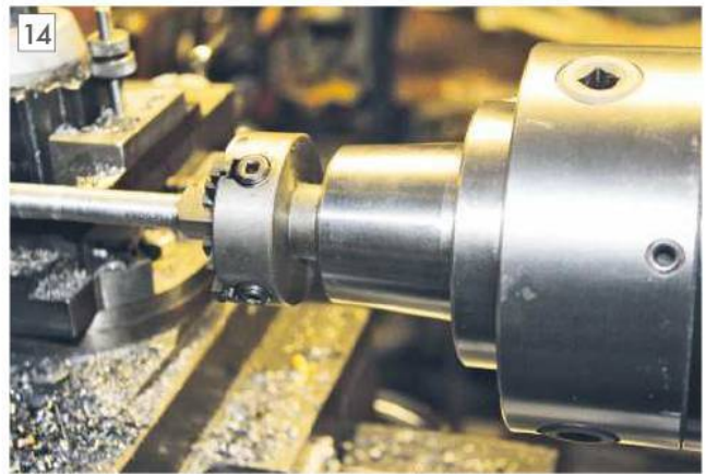
Holding a second chuck using a stub shaft.
