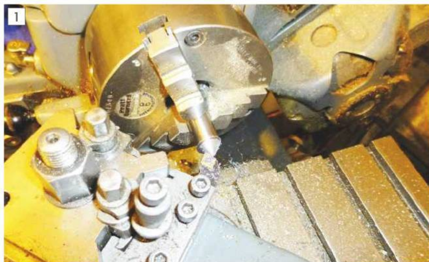
Tapering the end of a silver steel rod.
