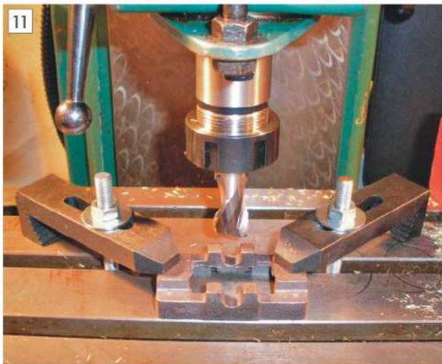
Milling the top of the bearing housings.
