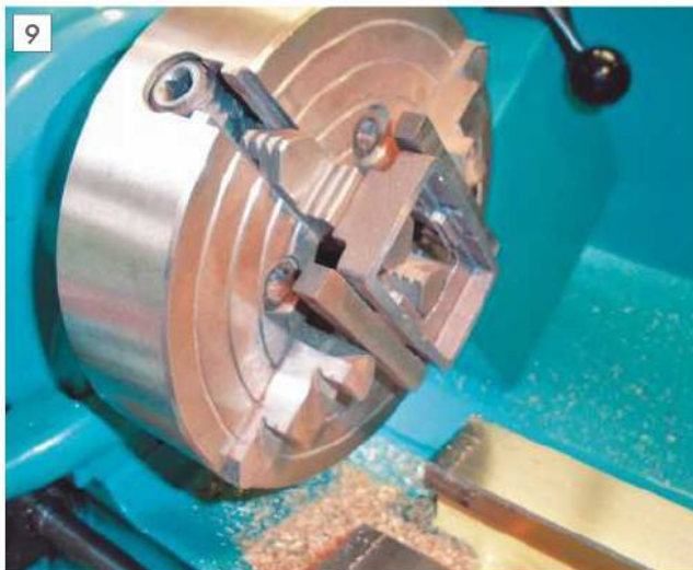
9 A lathe can be used to machine flat surfaces.
