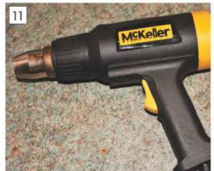
A hot air gun as used for shaping acrylic guards.
