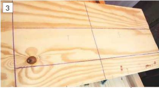
12mm ply marked ready for cutting.
