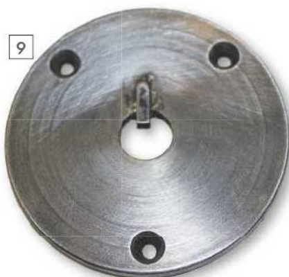
The disc after silver soldering the tooth.
