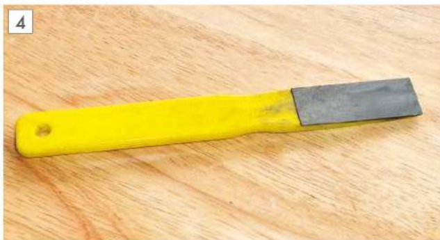
4 A diamond lap, fitted with a handle.
