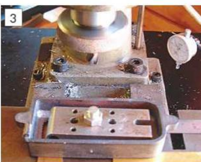
Machining under the box bed.
