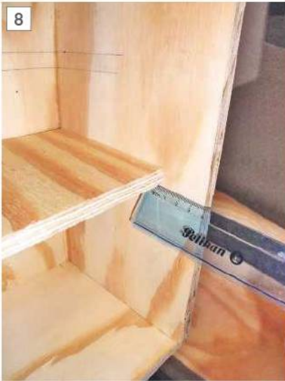
Checking shelf clearance before securing the front piece.
