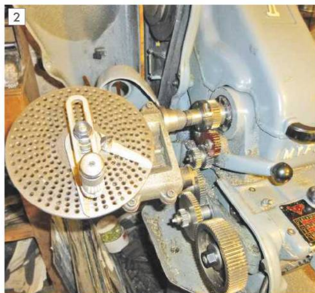
The dividing head at the back of the lathe mandrel.
