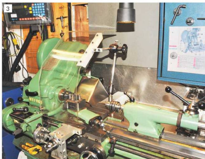
Acrylic guard fitted to myford lathe.
