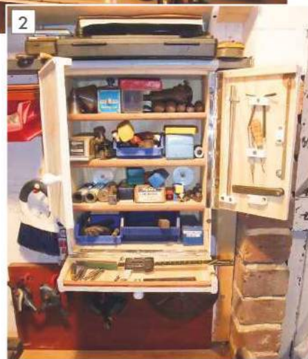
Lathe tooling in cabinet with drop-down shelf.
