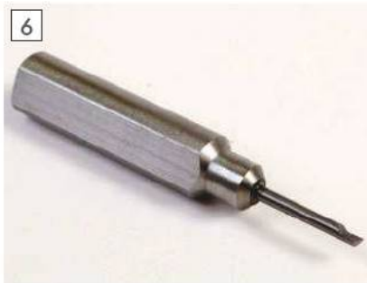
A mild steel mounted tungsten carbide boring bar.
