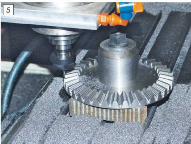
Inner Bevel Gear Machining.
