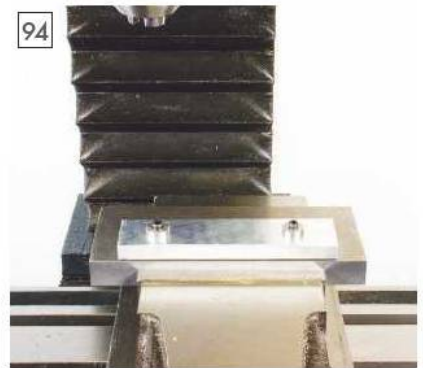
Workpiece screwed to a sacrificial base.
