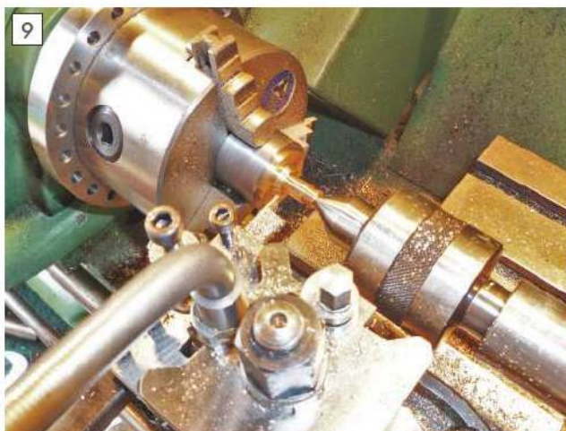
Turning a brass component with the Mini-Thin tool.
