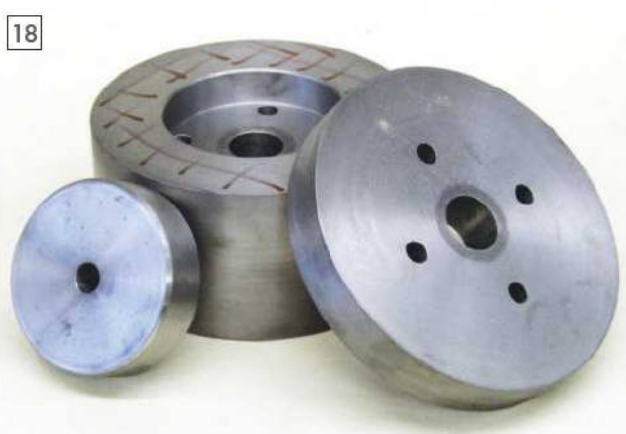
The three finish-turned blanks ready for the rotary table.
