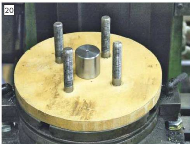
The protective packer used when drilling the stud holes in the baseplate was used to locate the holding down studs.
