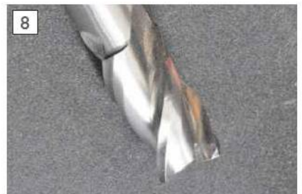
The damaged edge of this cutter re-ground and used for a radiused edge.
