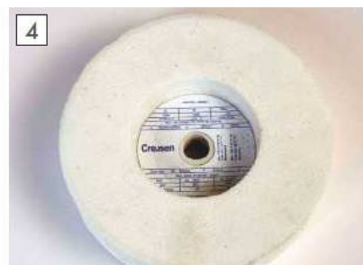
A recessed grinding wheel suitable for grinding on the side of the wheel.
