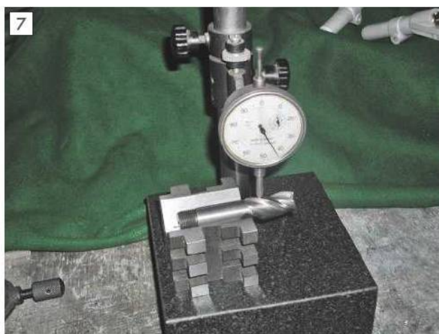
7 Measuring the diameter of a ground 3 flute cutter.
