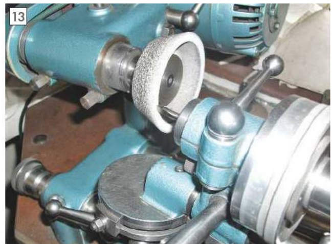
Grinding the radius on a lathe tool.
