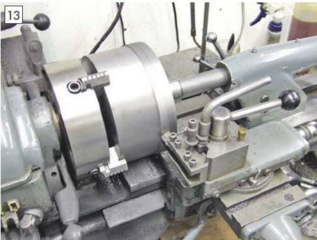
13 Now that the blank can clear the front of the saddle the LH tool can be used in the conventional position, turning from left to right.
