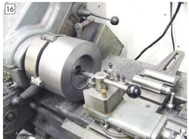
16 Boring the 1 inch diameter through hole in the main body.
