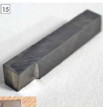
A tool for brass does not have top rake.
