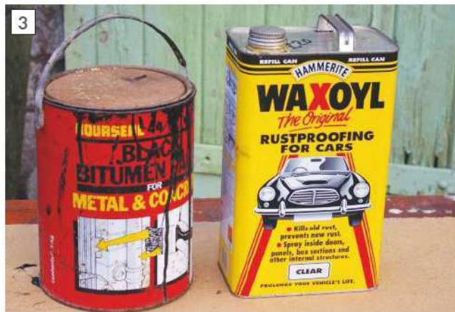
Black underseal (left) and Waxoyl (right) which is available either black or clear (much less messy).
