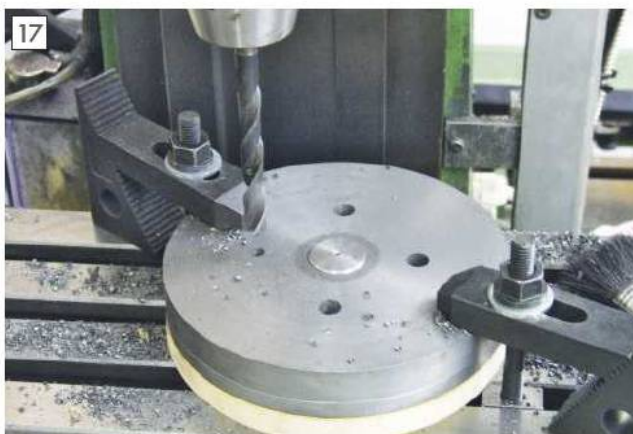
Drilling the holes for the studs which will hold the baseplate onto the rotary table.
