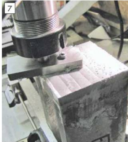
Flycutting the bracket base.
