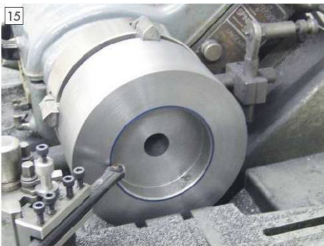
15 Chamfering the entry to the recess.
