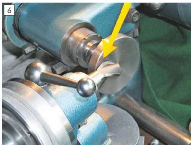
6 Facing plate fitted to grinding head used to check the clearance angle.
