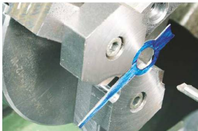
Harold's two-jaw technique gives just enough support for the light cuts needed to finish this tricky task.
