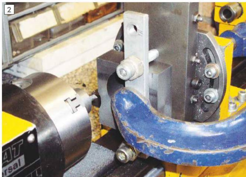
Machining clearance for the leadscrew protective tube.
