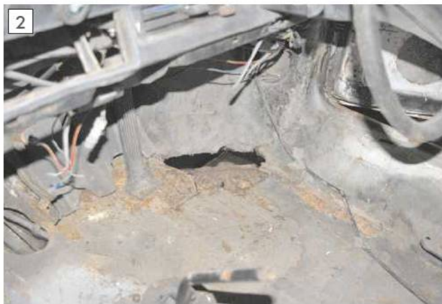
Showing the gaping hole at the footwell/A post area.
