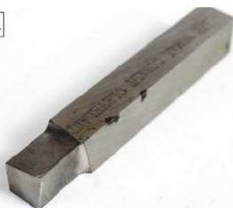
A typical HSS turning tool for steel, note the top rake.
