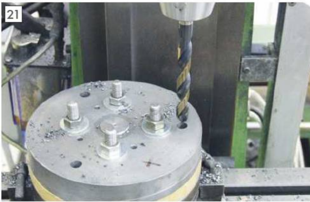
21 Drilling the 10.5mm hole reminded me exactly why I was doing this job - the drill point only just cleared the baseplate, so drilling the much thicker main block should prove interesting.
