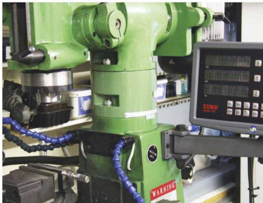
The Raising Block fitted to the VMC Mill.
