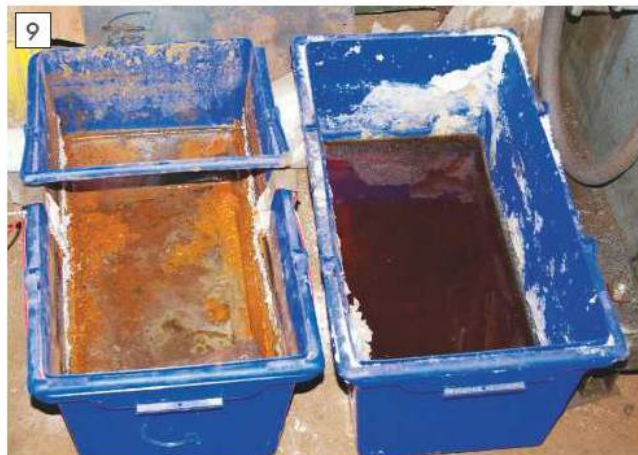
Tub on right contains caustic soda, that on left has washing soda solution and is equipped with plate steel anodes. Both will need topping up with water for larger.
