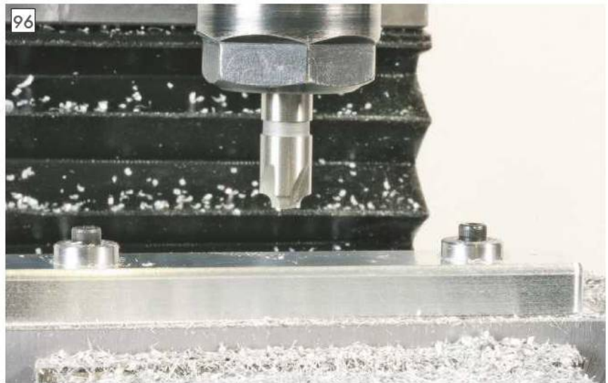
A rounded edge achieved using a form cutter.
