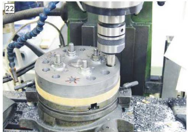
22 Opening up the counterbores to 16mm diameter.
