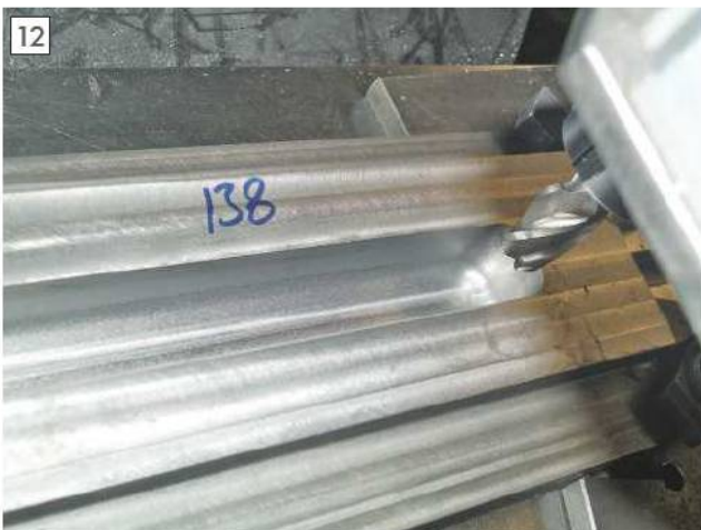
Radius edge cutter used in lead screw clearance slot.
