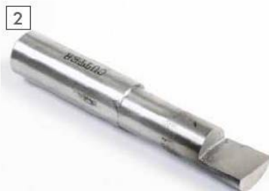
A boring bar ground from a round piece of HSS.
