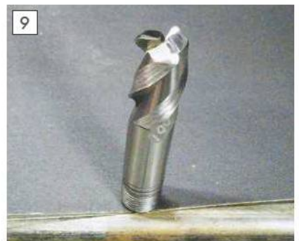
Cutter restored and ready for use.
