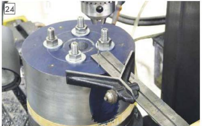
24 Using the rule and vee from the combination set to mark a centre line which will be transferred to the opposite face of the main block to position the studs which hold the turret in place. Note that the inner extent of the pocket has been scribed onto the face of the main block.
