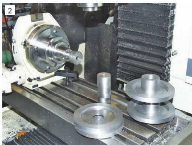
CNC Mill Setup and Cast Iron Blanks.
