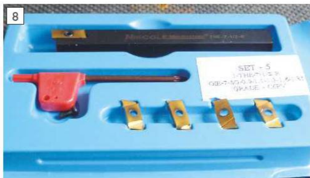
A Mini-Thin grooving and parting tool with a selection of tips.
