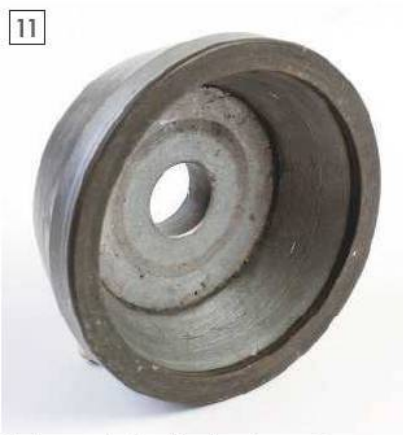
A diamond wheel for lapping tools.
