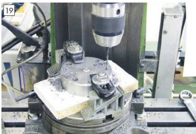
The spigot was the first part on the rotary table to drill and counterbore the holes for the M6 capscrews. The operation shown here is pilot drilling the spigot for roll pins. Note the centring plug and the packing underneath the spigot.
