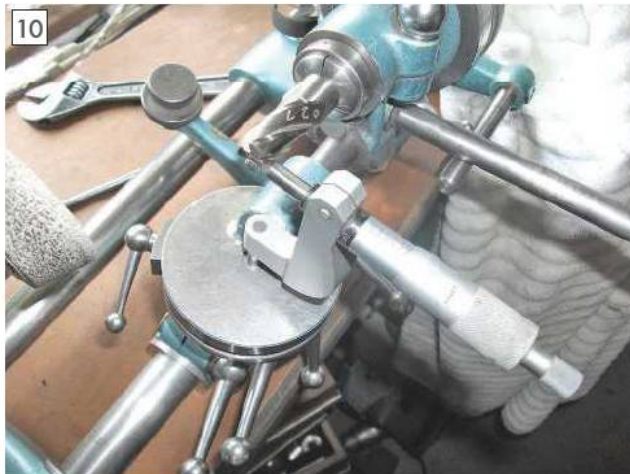
Setting cutter first position for corner radius.
