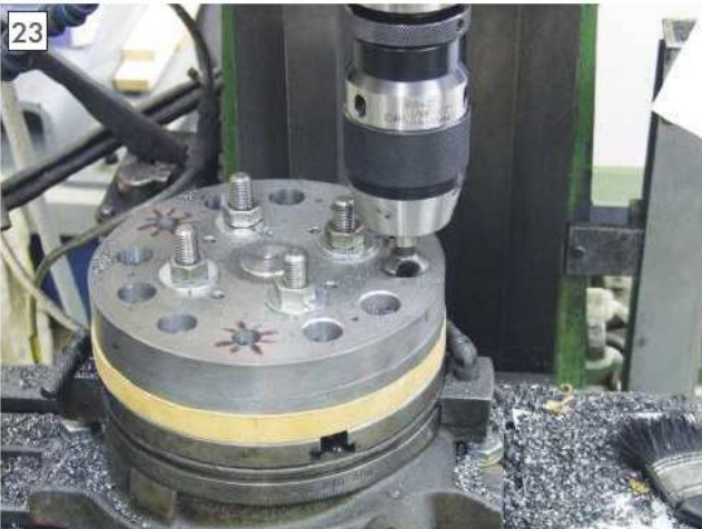
23 This face will be skimmed at the final assembly stage, so a countersink cutter is being used to avoid any sharp edges later on.
