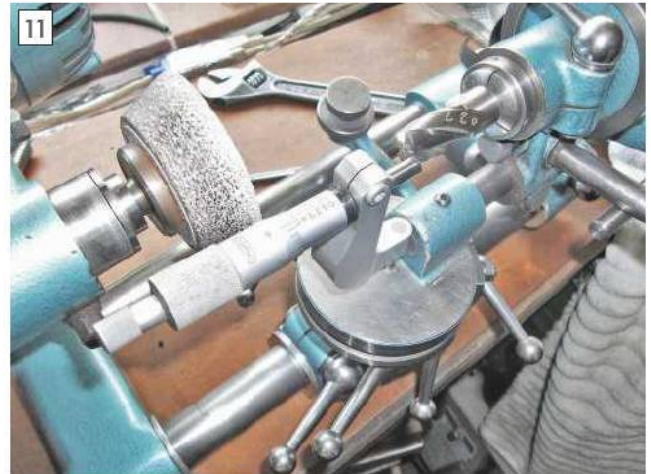
Setting the position of the cutter grinding allowance.
