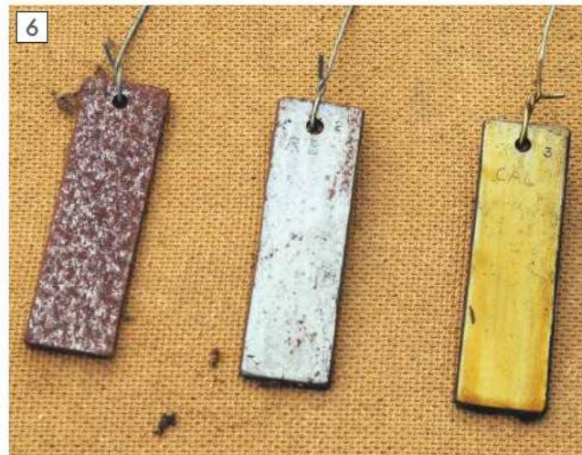
The three test pieces after seven years.
