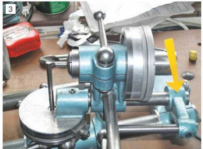
Setting the axis of the workhead and rotating base.
