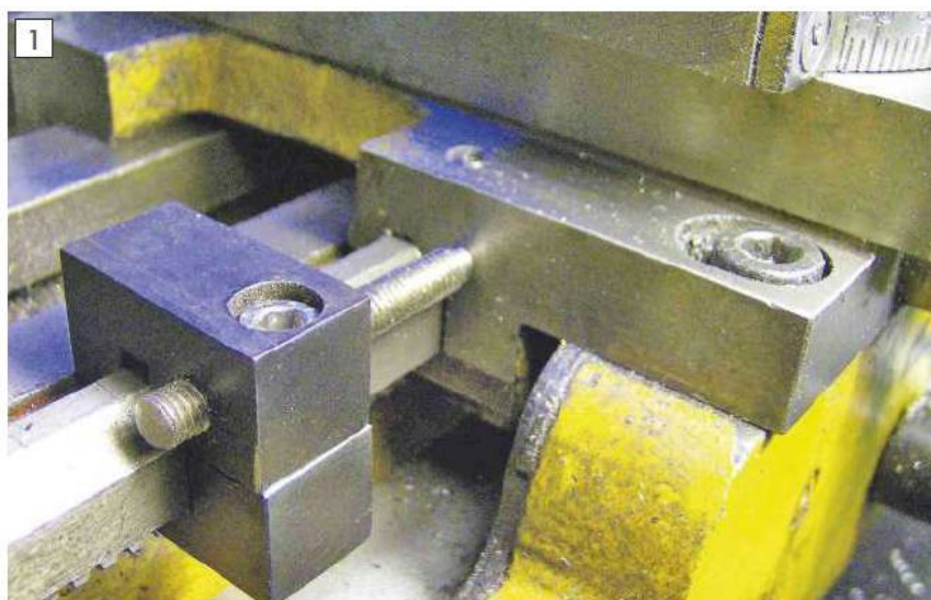
How the stop bears against the saddle.
