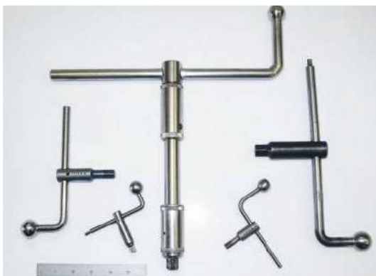
LEFT: A selection of modified chuck keys. BELOW: A modified chuck key in use.
