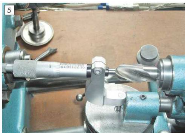
Setting the grinding allowance of the ball nose cutter.
