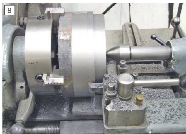
Confidence is increasing - turning a longer second section of the outside diameter.
