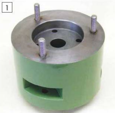
The finished raising block - the angular scale would be fitted after assembly onto the machine.
