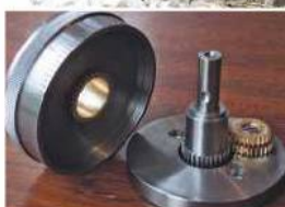
Components of a handwheel dial for my lathe.
