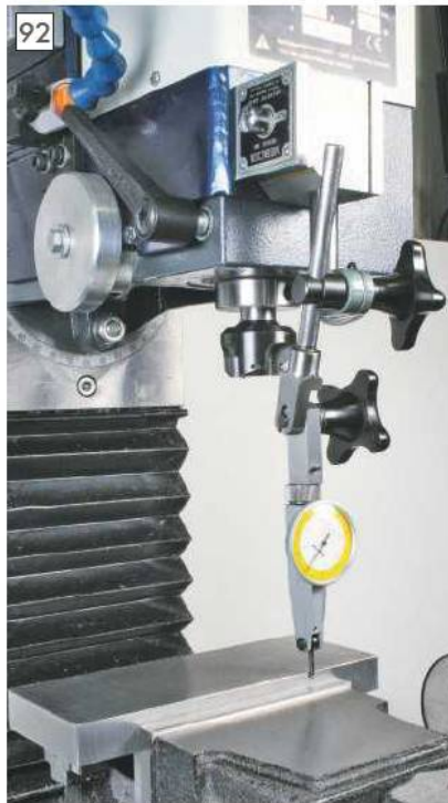
A lever action DTI is used to clock the front edge of the material parallel to the X axis.
