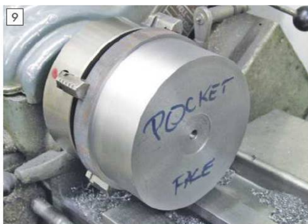
The first face has now been completed - this is the face in which the pockets will be milled.
