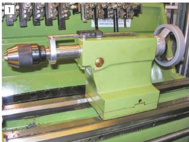
The digital scale fitted to the tailstock.
