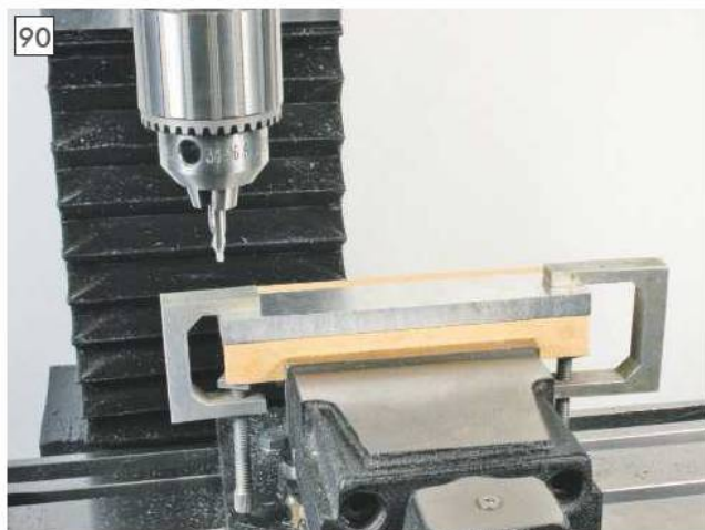
MDF plate in position to support the main parts as the locating holes are drilled and reamed.
