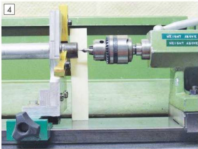
A close up of the centre drilling arrangement.
