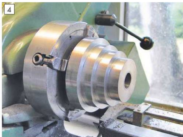
Small end and bore completed.
