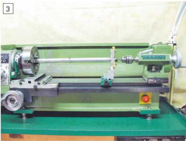
The set-up for centre drilling the ends of the bar.
