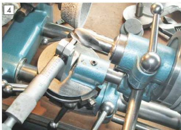
Checking the set position of a ball nose cutter.
