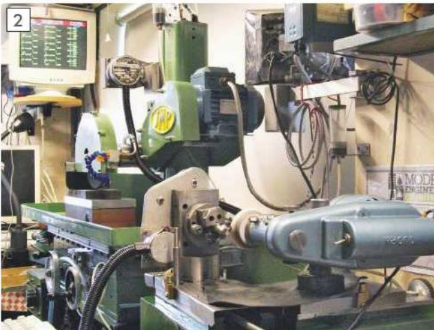
The cnc cutter grinder in action.
