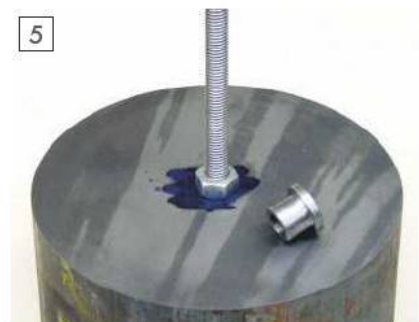
The 'drawbar' fitted to the main block, shown together with the reducing bush.
