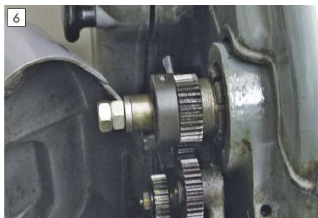
View at the rear of the Myford spindle showing the reducing bush, M10 stud and nut used to secure the main block blank.
