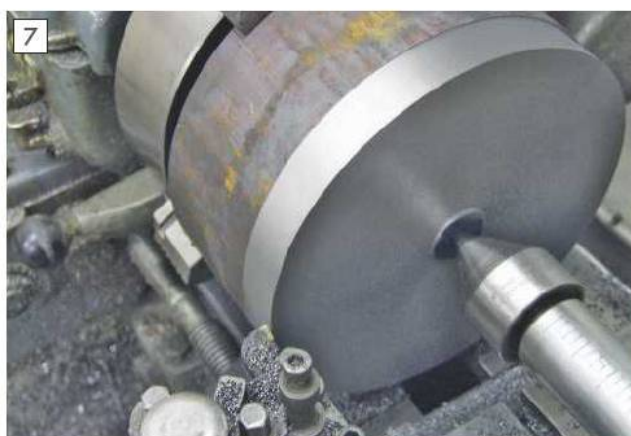
Turning the main block to finished diameter using a left-handed tool. Note the tailstock centre is in use as an additional security measure.
