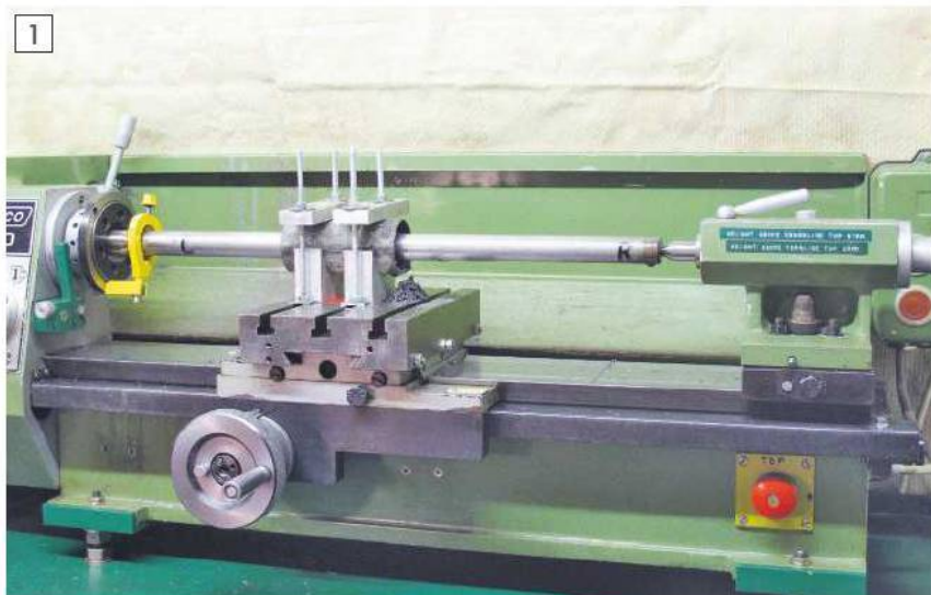
The finished boring bar in use on lathe.
