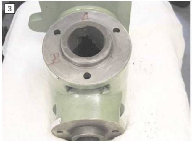
The underside of the turret.
