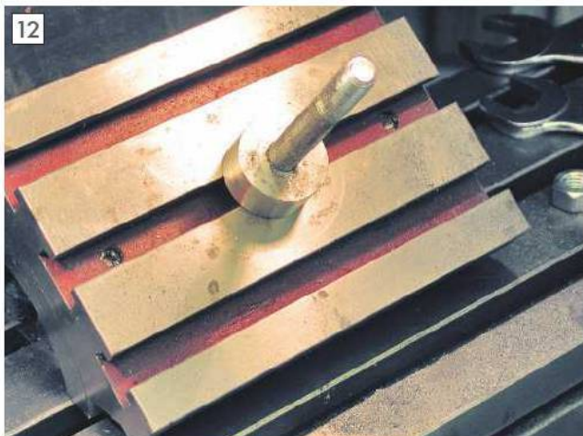
Mounting for the spindle pulley at 40 deg.
