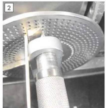
The sector arm trapped on both sides.
