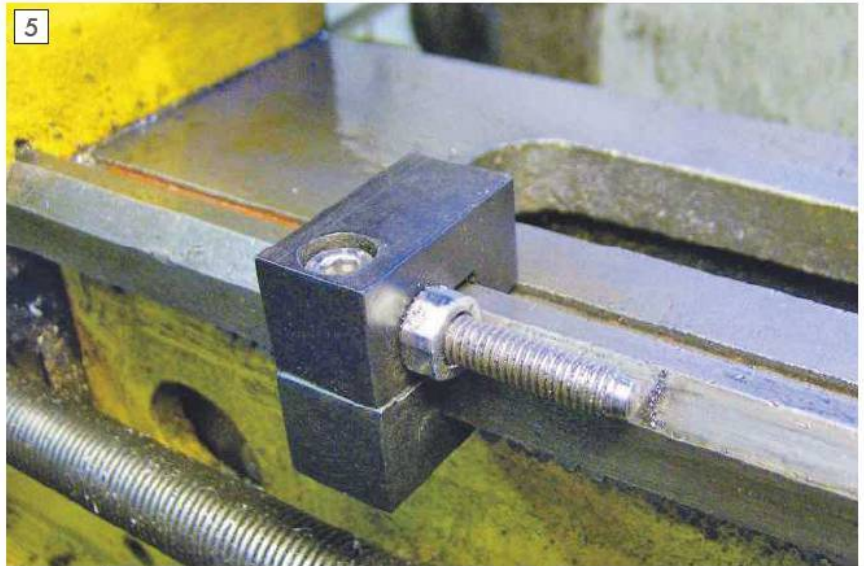
The stop fitted to the bed of the lathe showing the stop bar.
