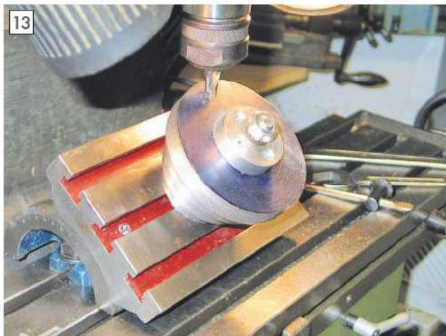
Boring the 40 deg. hole.
