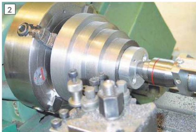
Set-up showing the aluminium support pad.
