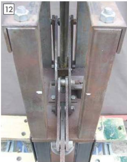
Details of lever arm, tie link and upper lever.
