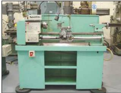
MYFORD Type 2545: Centre Lathe. Swing Over Bed. Between Centres 30". Spindle Speeds 53-2000 rpm.
