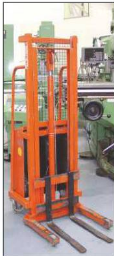
WILMAT Type 16: Manual Electric Lift Fork Truck. 300kg Capacity. Fork Length 20"
