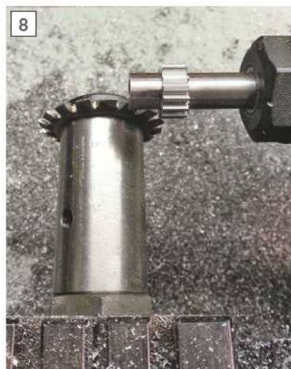
Cutting the 16 tooth gear.
