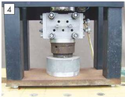
Mould clamped in position under cylinder.
