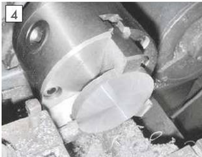
Facing a gear blank.
