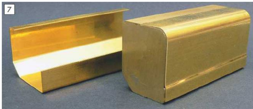
A complex shape done on the press.
