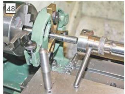
48 The finished thread.
