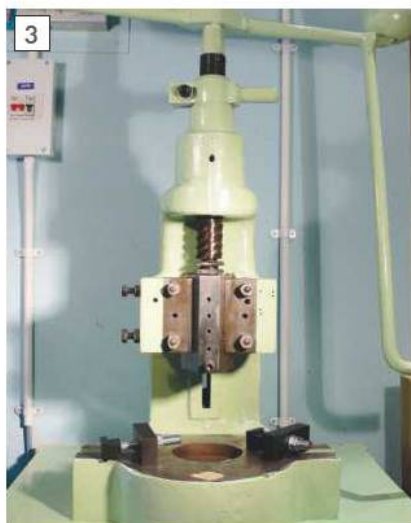
A typical fly press.
