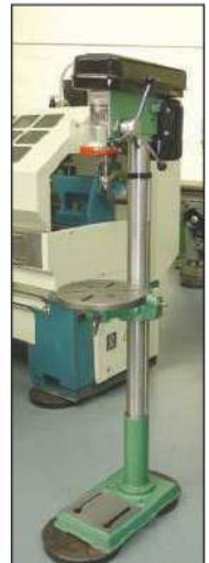
NUTOOL: Pillar Drill. 1/2" Capacity. 11" Diameter Table. Single Phase.
