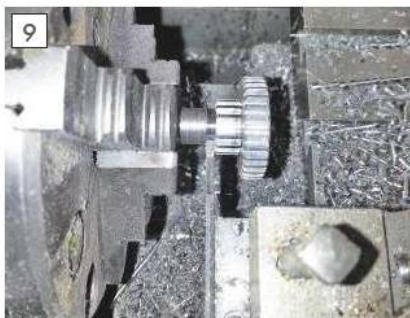
Parting off the gear assembly.
