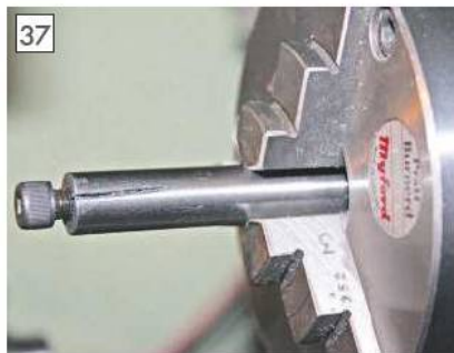
Expanding mandrel to take the casting.
