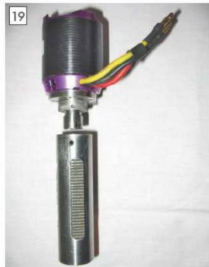
The motor fits onto the flange.
