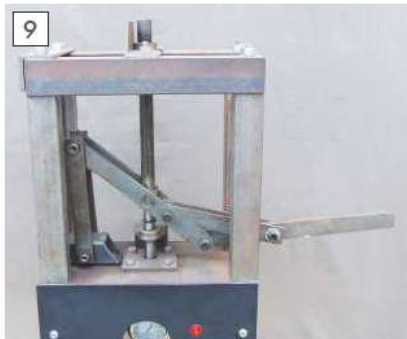
Ram at bottom of stroke.
