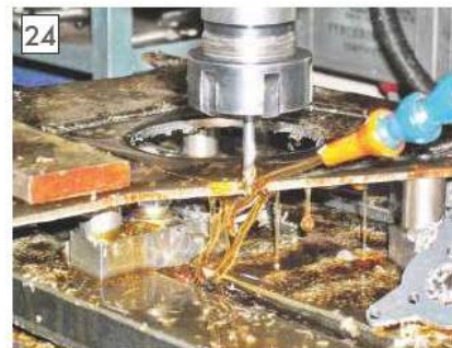
Milling the mounting plate.
