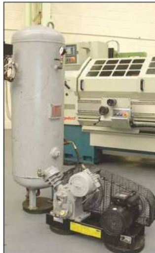
INGERSOLL RAND: Twin Cylinder Compressor. 2.2KW Single Phase Motor. 17" x 48" Air Receiver.
