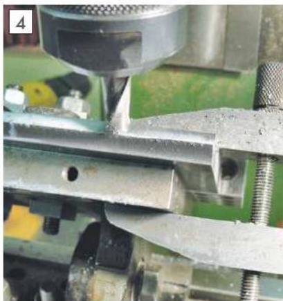
Machining the angle on the Vee tool.
