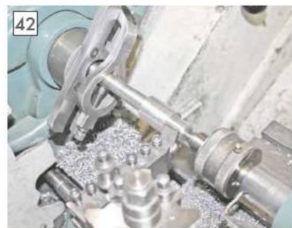
Roughing out the bar.
