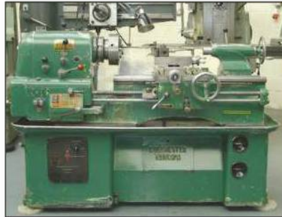
COLCHESTER TRIUMPH 7 1/2": Between Centres 30". Swing Over Bed 15". Spindle Bore: 2" 3 Jaw. 2.83 Point Steadies. Quick change tool post.
