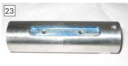
The rack slot milled and drilled.
