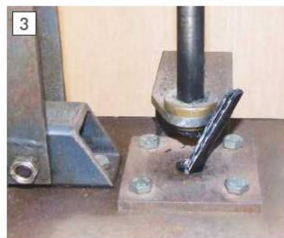
Plastic strips loading into cylinder mouth.
