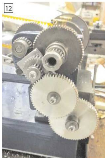
The gear train from the end of the lathe.
