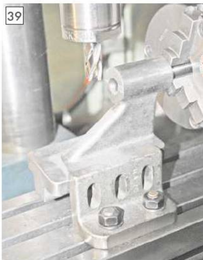
Machining the boss.
