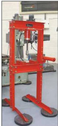
SNAP ON: Garage Press. 20" Between Uprights. 35" Max Daylight. Capacity 15 Ton (Approx).
