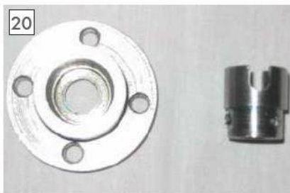
The motor flange and drive dog.
