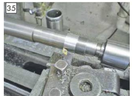
Skimming the spindle to fit.
