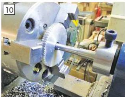
Slotting a gear.
