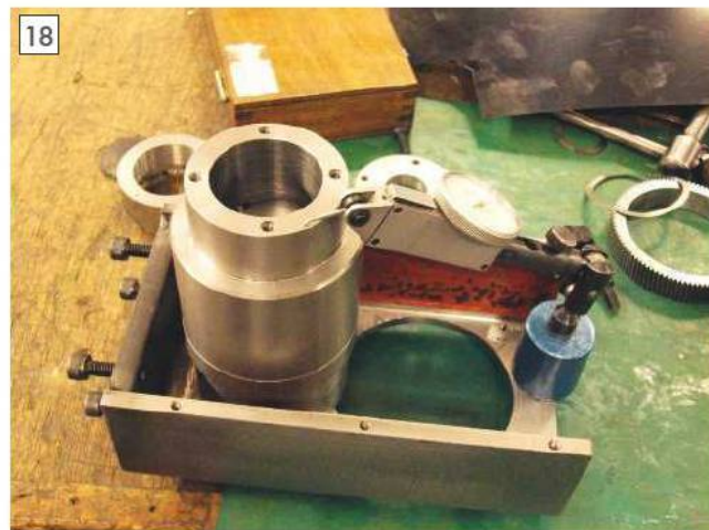
Checking the end float.
