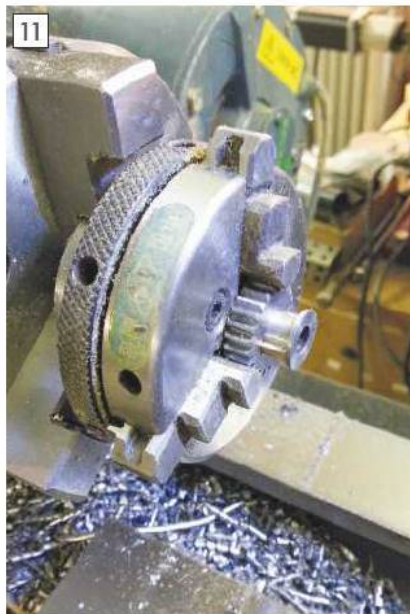
Checking the gear's fit on a bobbin.
