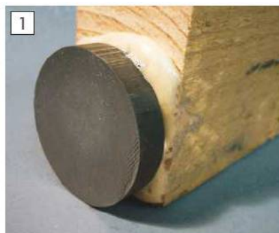
A typical joint all glued up; the swollen appearance of the glue is from the foaming action.
