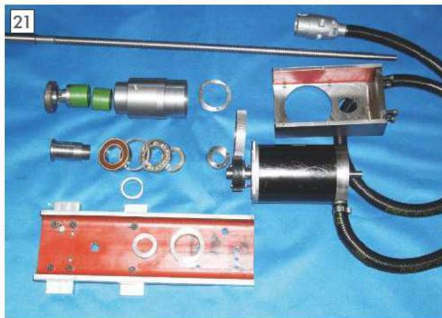
The saddle drive components.
