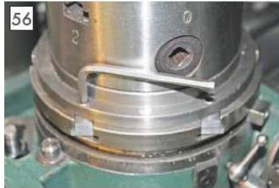
Clamp the chuck to the rotary table.
