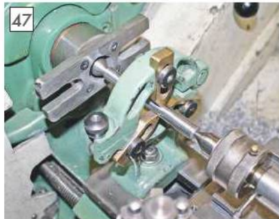
47 Ready for threading.
