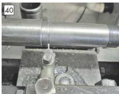
Turning the circlip groove.
