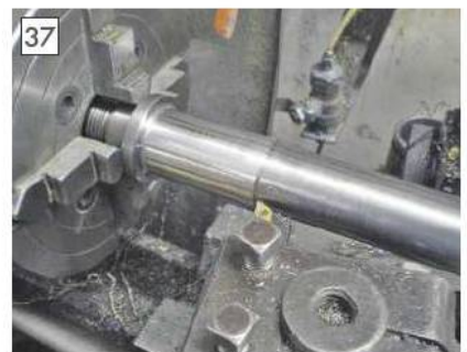
Skimming spindle headstock bearing diameter.
