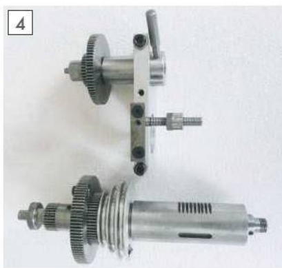
Spindle and back gear subassemblies.
