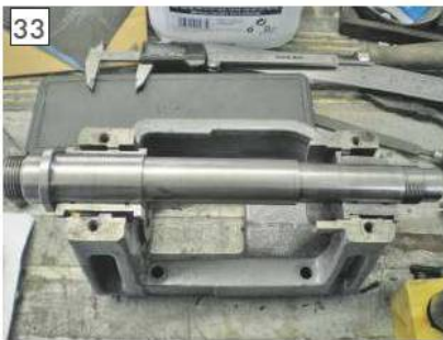
Checking length for mild steel bushes.
