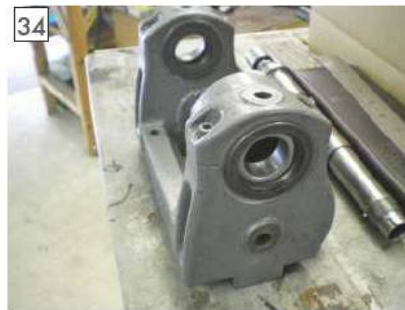
Bushes and seals temporarily fitted.
