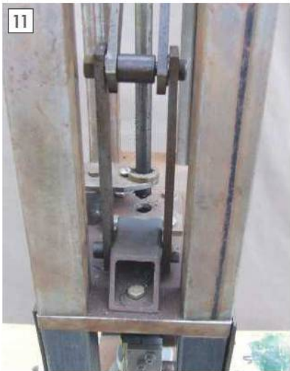
Details of drop link mounting and lever pivot, note spacers.
