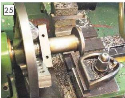
Machining the cross slide leadscrew bracket.
