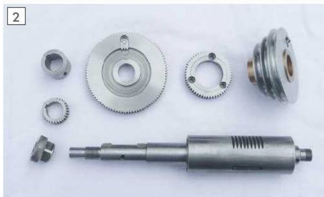
The new spindle components.
