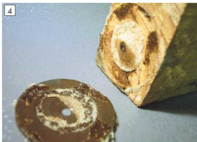
The joint after separation.
