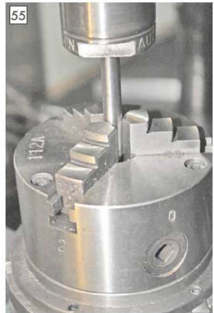
Aligning the chuck on the rotary table.
