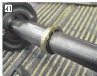
Circlip and brass washer fitted.
