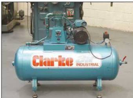
CLARKE: Industrail Air Compressor. Model SEI 6C150 Garage Type Max Working Pressure 10.3 Bar. Single Phase.
