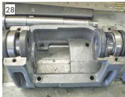
Trial fit of bearings and seals.
