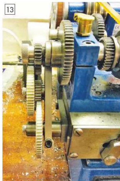
The gear train from the front of the lathe.
