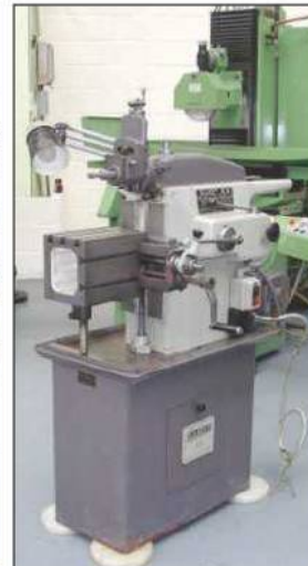
ELLIOTT Type 10M: Horizontal Shaper. 10" x 7" Tilting Table. 10" Stroke. With Vice.
