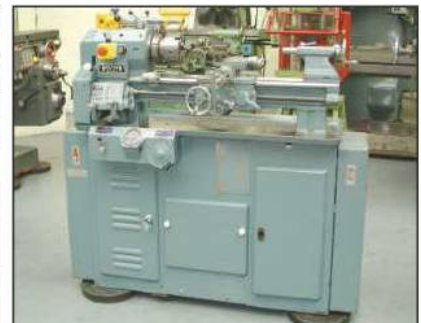
BOXFORD VSL: Variable Speed Centre Lathe. Swing Over Bed: 9". Distance Between Centres: 20". Collets & Drawbar.
