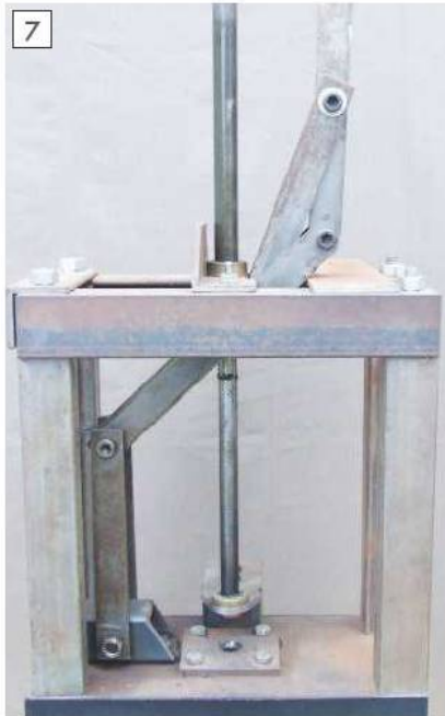
Ram at top of stroke, note drop arm angle.
