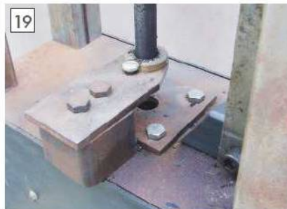
Lower ram bushing and support plate, note bushing retaining screw.
