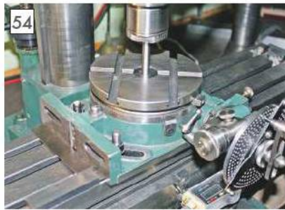
Aligning the rotary table.
