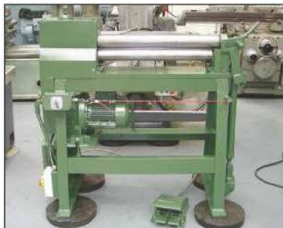
BARNES Intial Pinch Powered Bending Rolls. Rolls Size 24" x 3" Diameter
