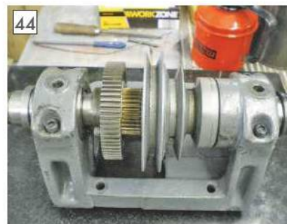
...with the bearing caps fitted.
