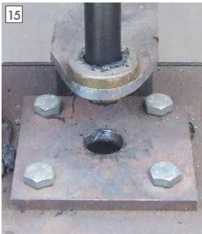
Cylinder top plate, note four bolts rather than the two shown on drawing.
