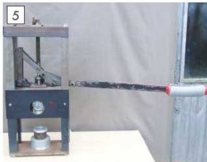
Ram in lowest position, note lever extension tube.
