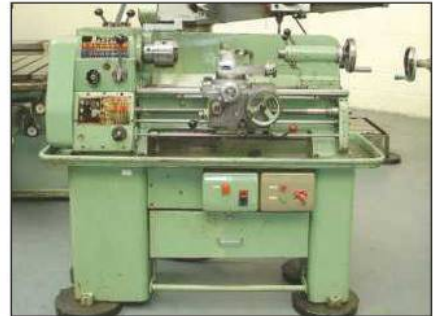
COLCHESTER BANTAM 1600: Centre Lathe. 11" Swing Over Bed. 20" Between Centres Speeds 35 to 1600 rpm. 3&4 Jaw chucks.
