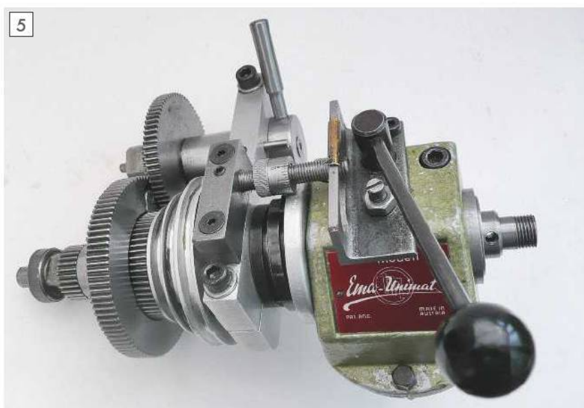
The assembled headstock.
