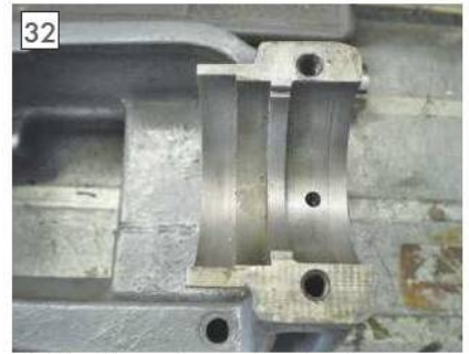
Finished bore changewheel end.
