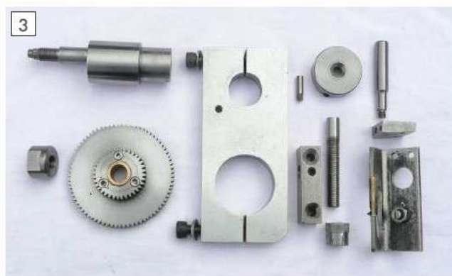
The back gear components.
