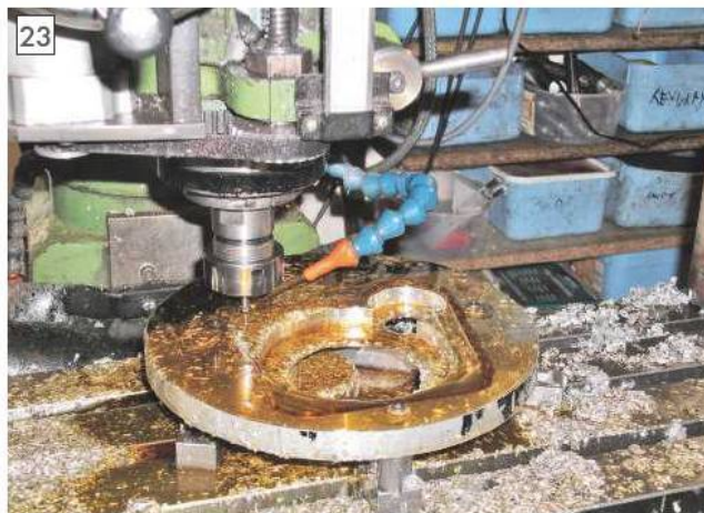
Milling the cover plate.
