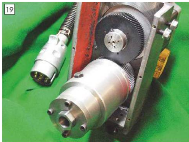
The X axis drive assembly.
