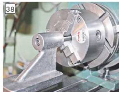
The casting on the mandrel.
