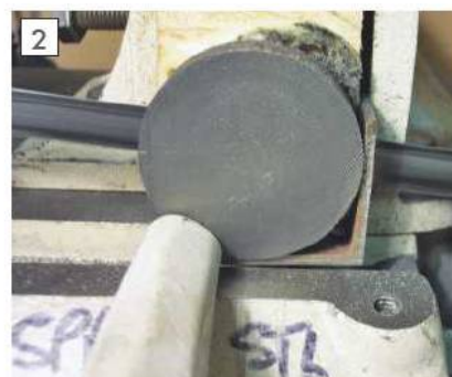
Sawing in progress, note the angle iron support.
