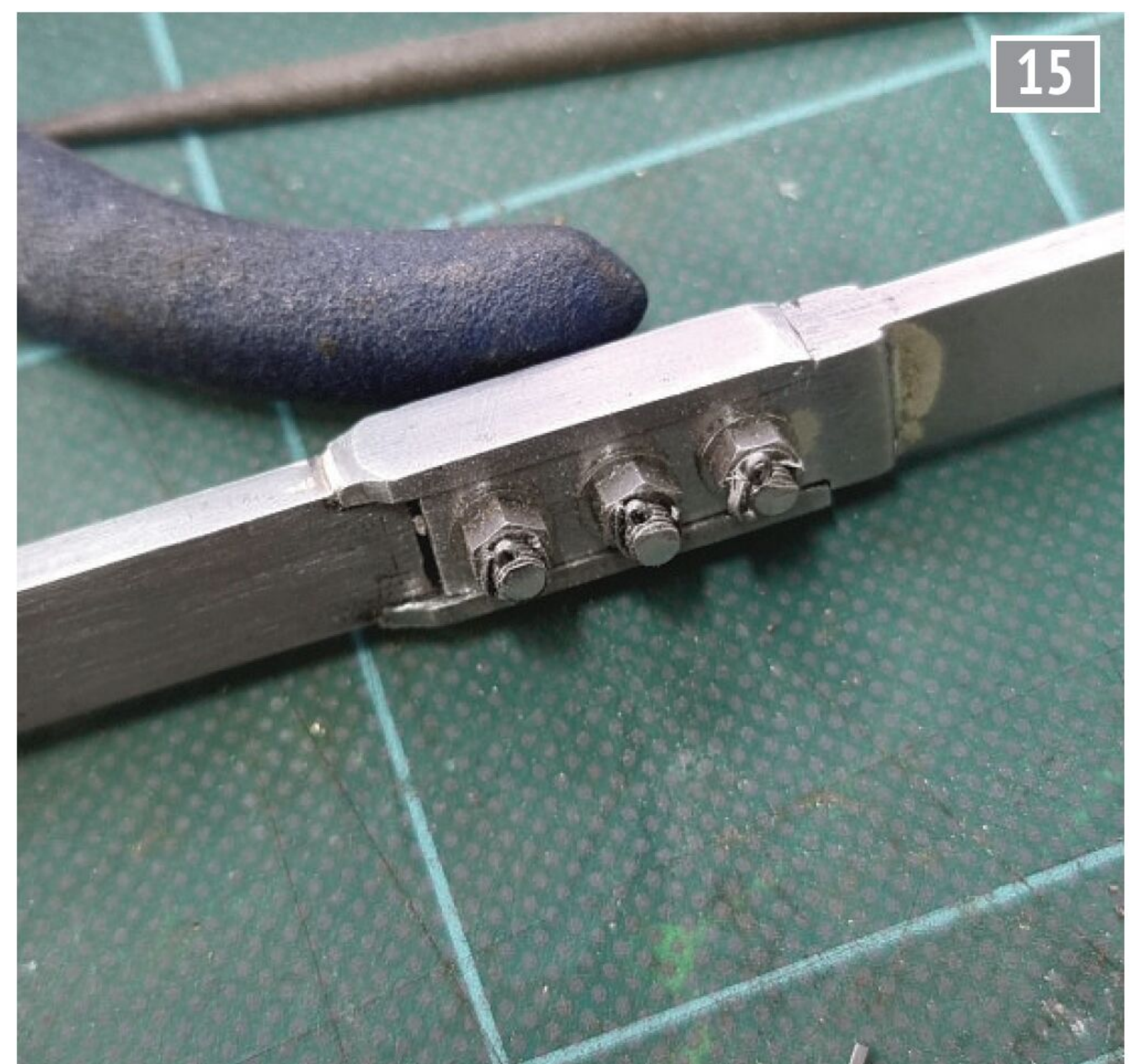
The completed reach rod joint.
