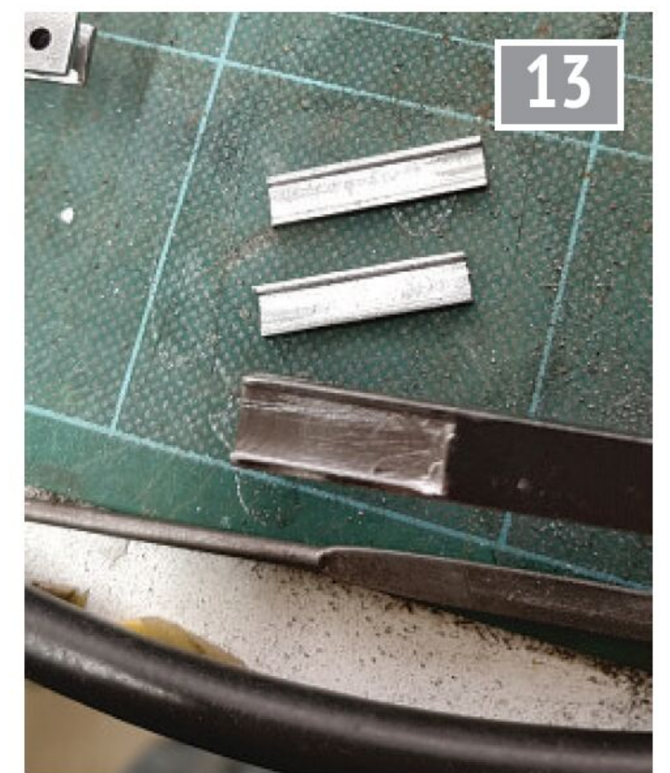
Two pieces cut to form the bulge in the joint.
