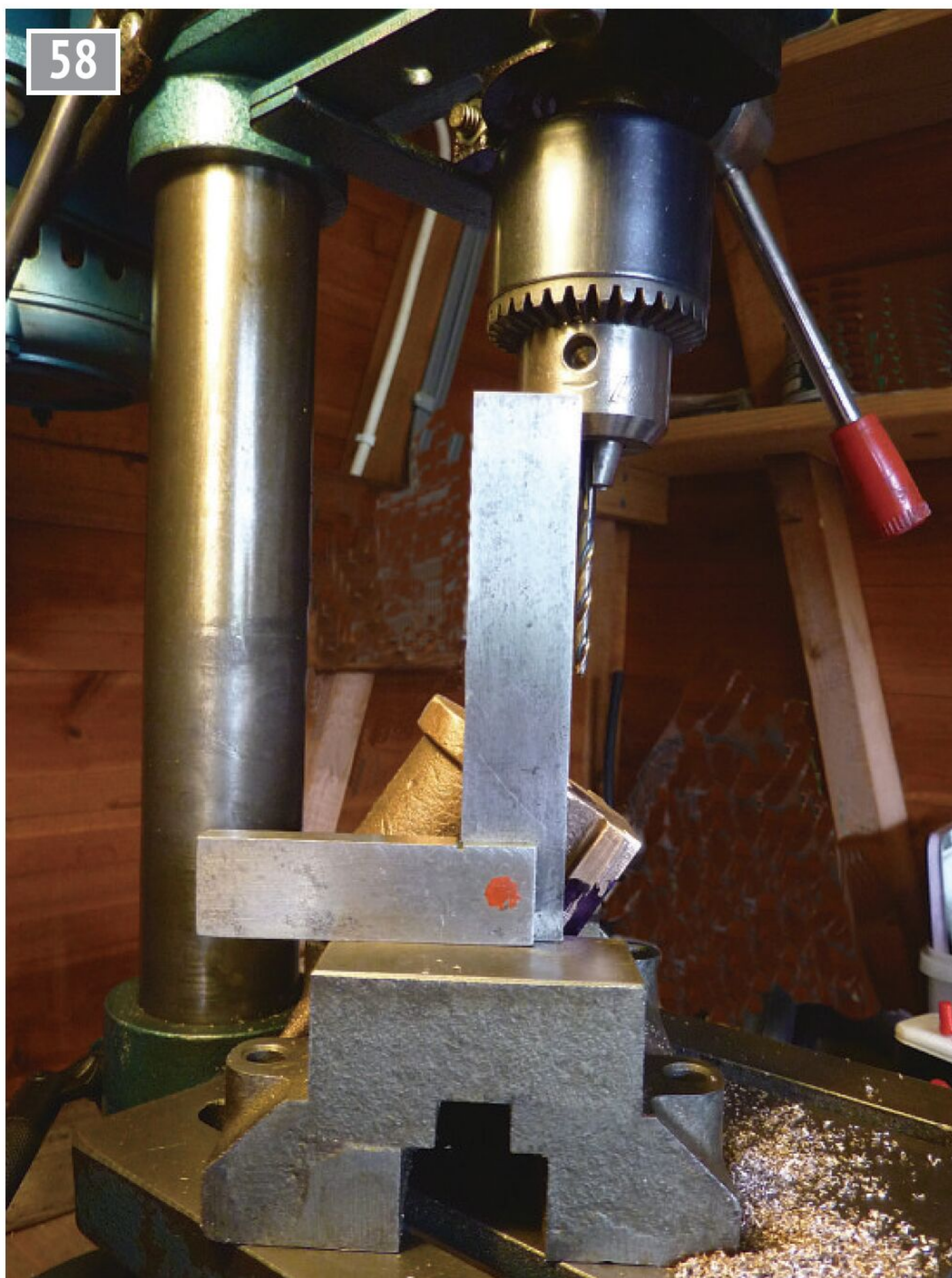
Lining up for drilling the passages.
