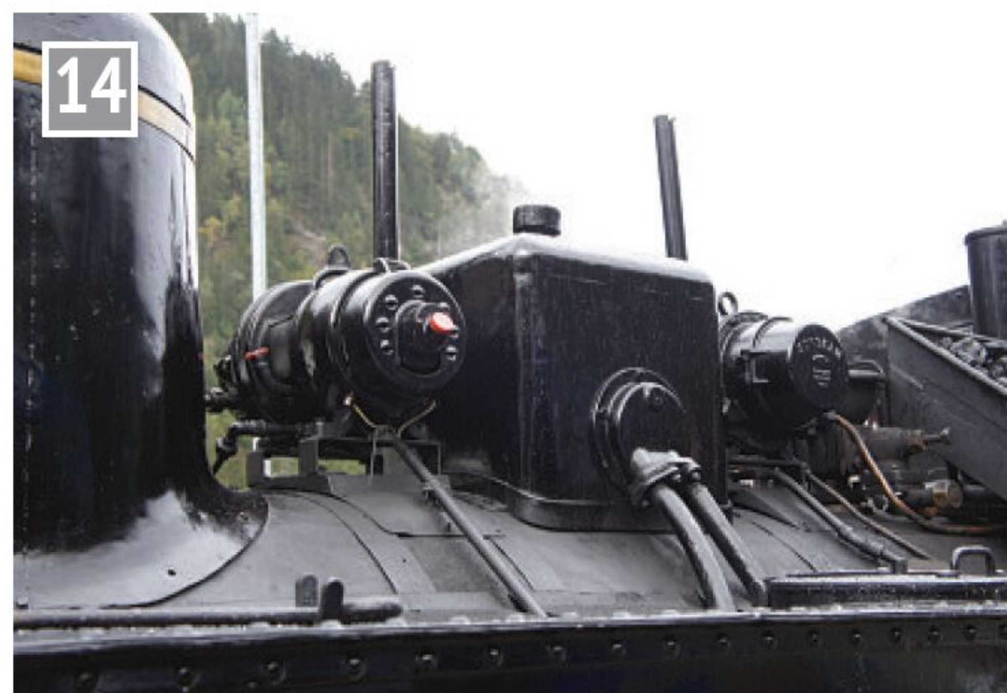
Locomotives have substantial boiler mounted sandboxes and turbo generators as seen on No. 3.
