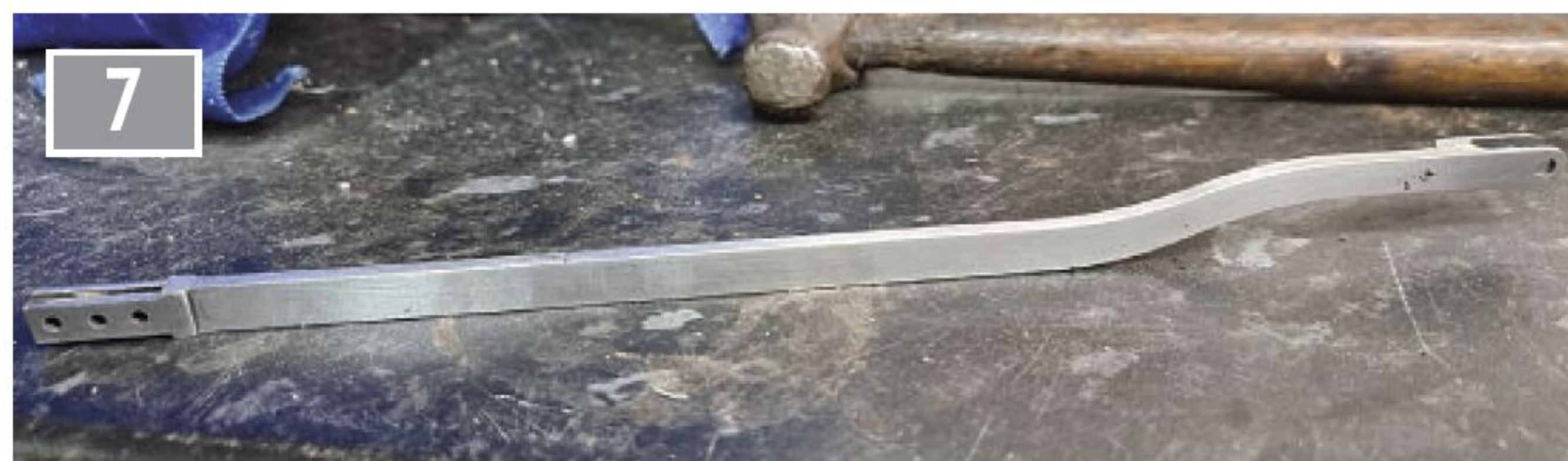
Front half of the reach rod, showing the tongue with the extra pieces added to the sides.
