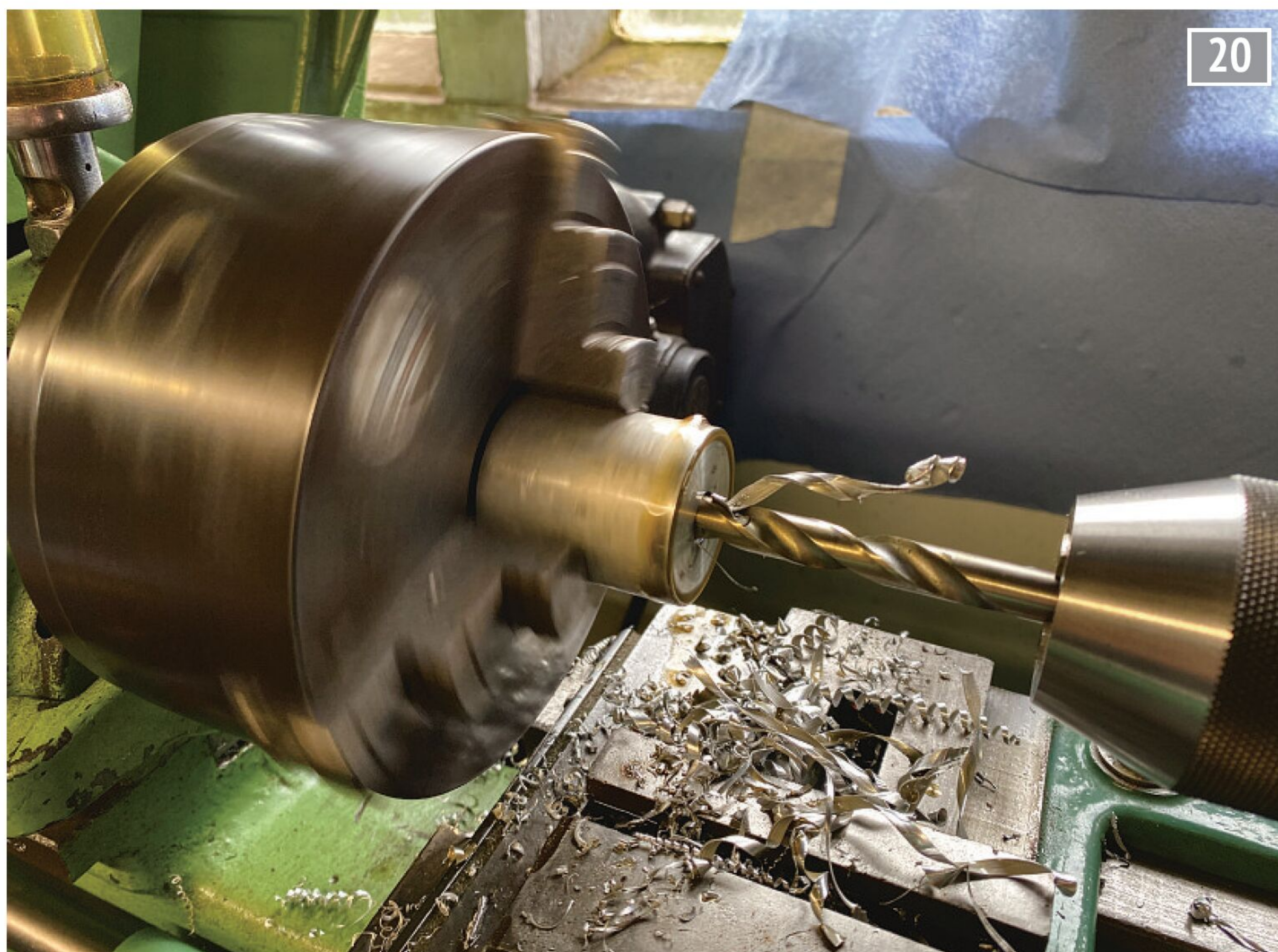
The countersink centres a large drill.
