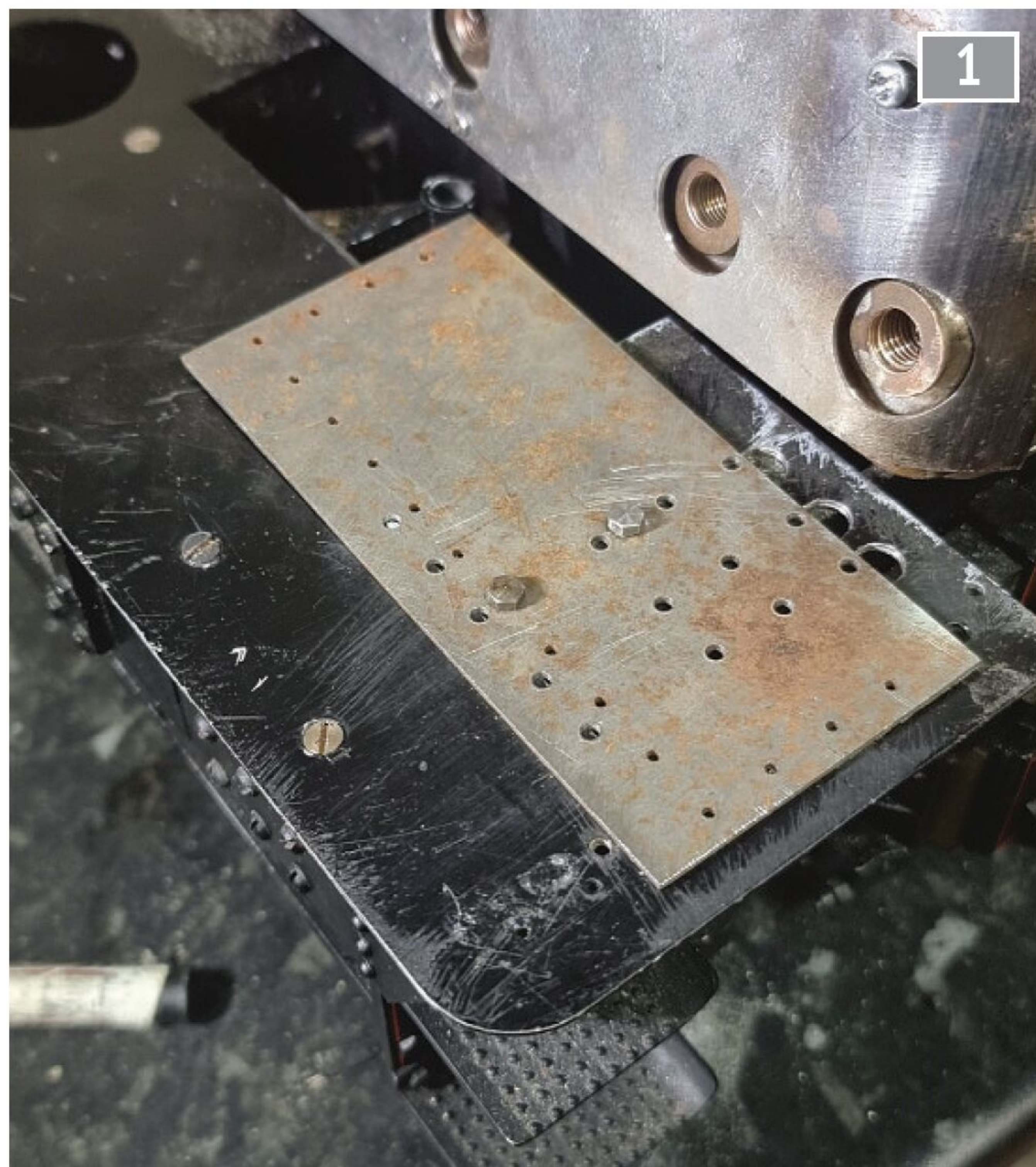
Jig for relocating the reverser stand holes.
