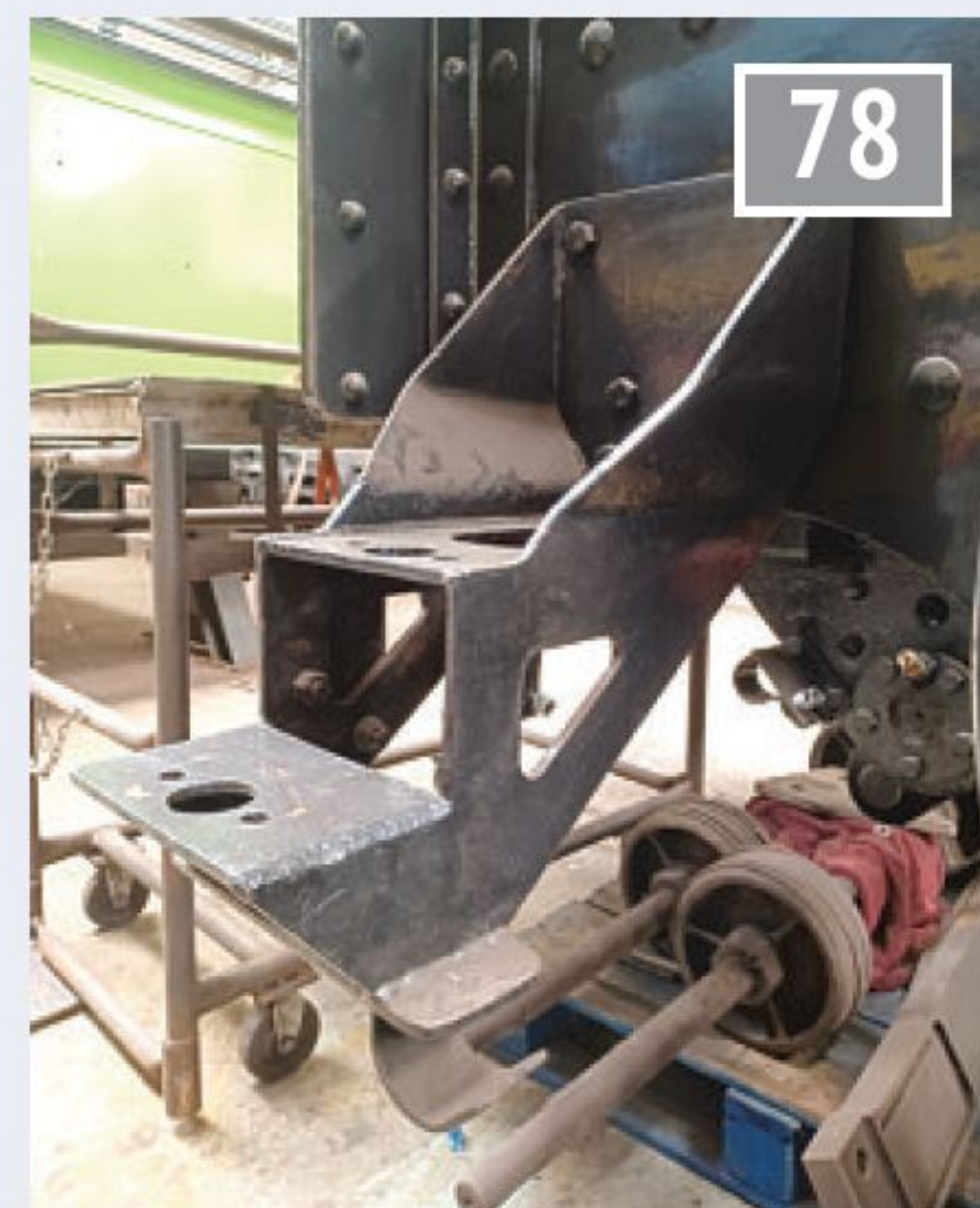
Right-hand injector bracket (Toddington Standard 4MT).
