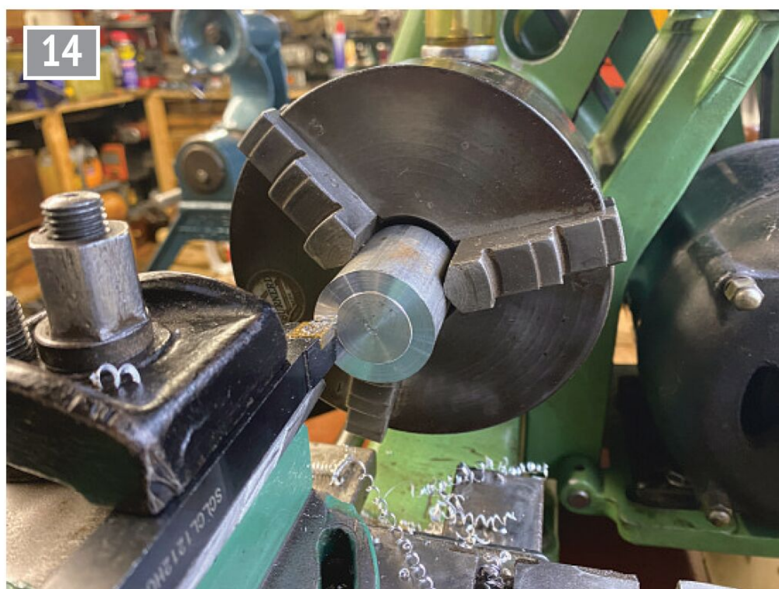
Squaring off the end of the work before drilling.
