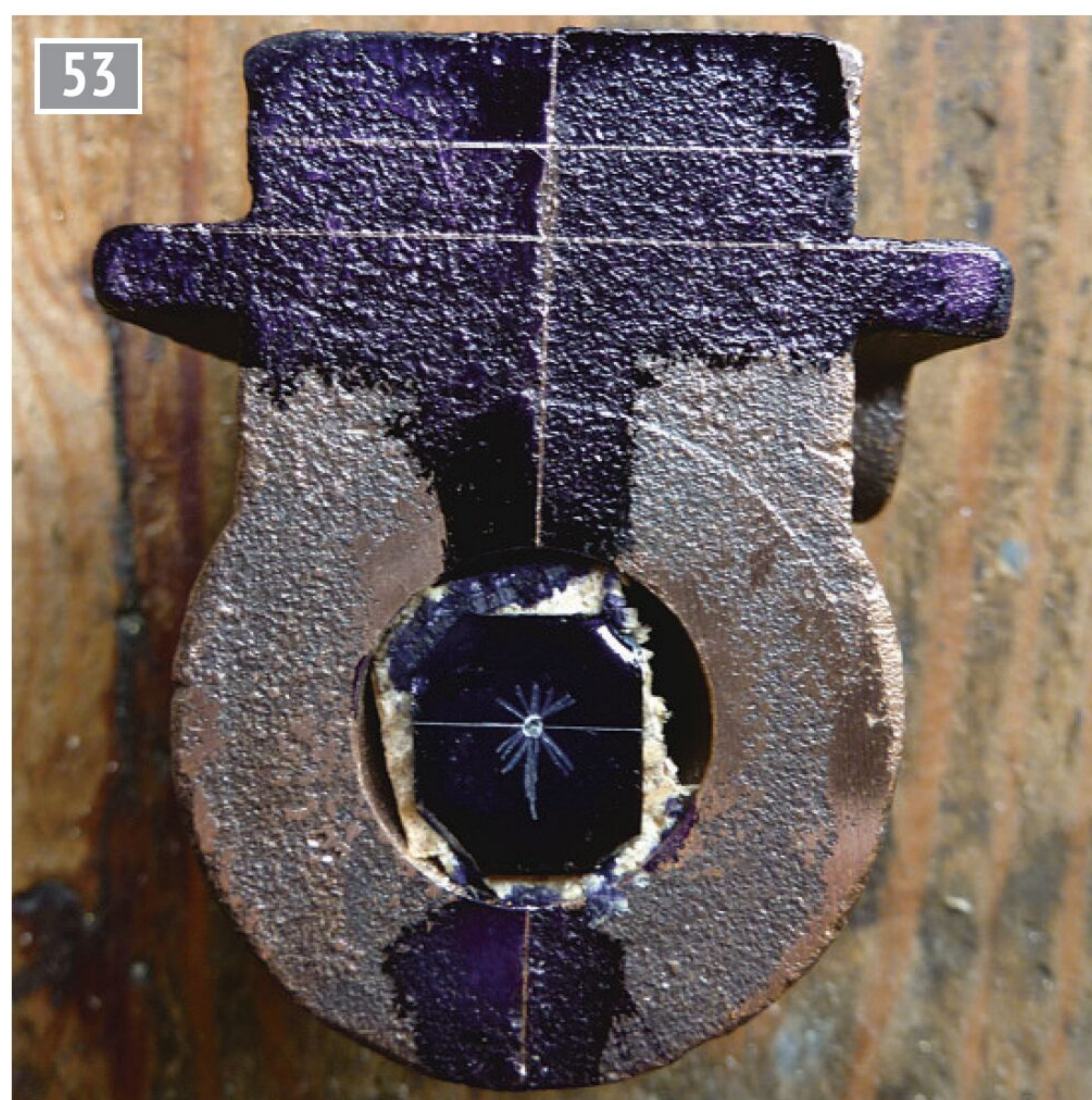
Finding the centre of the bore and marking out the port face.
