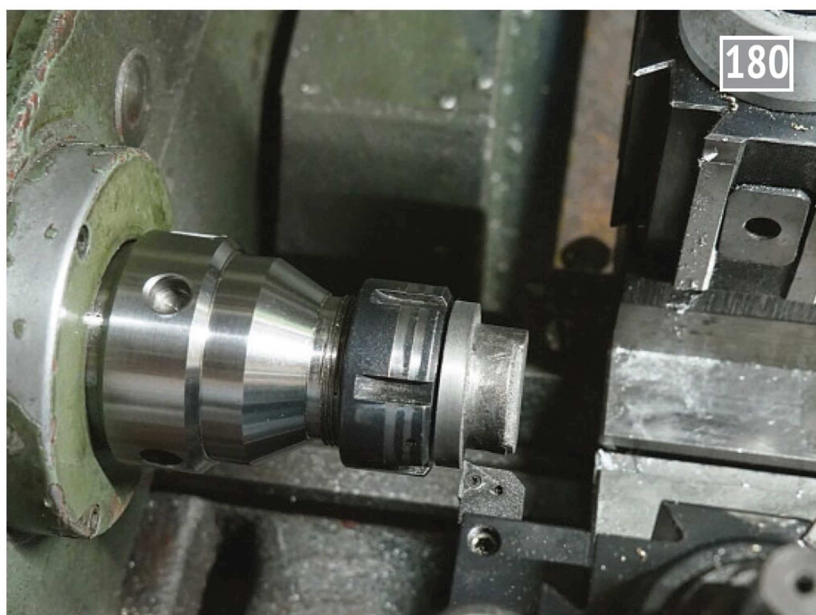
Then the bits that fit inside the bore were turned.
