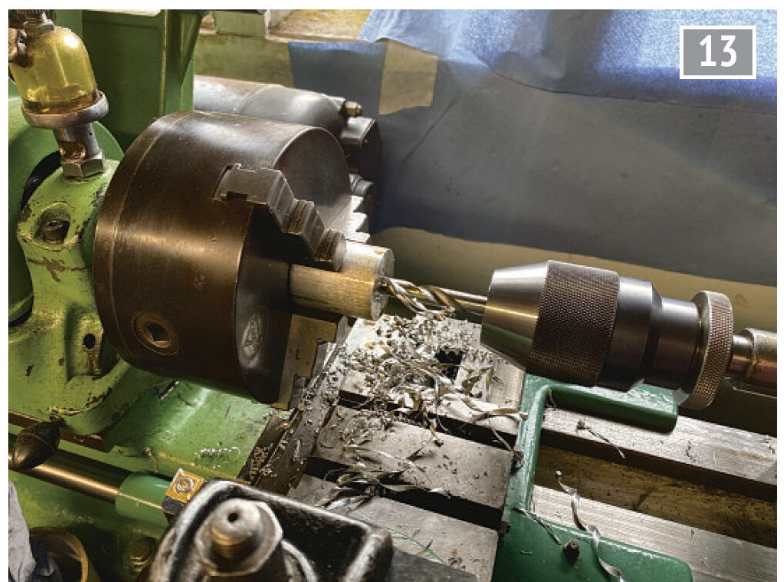
Drilling the lathe is carried out horizontally.
