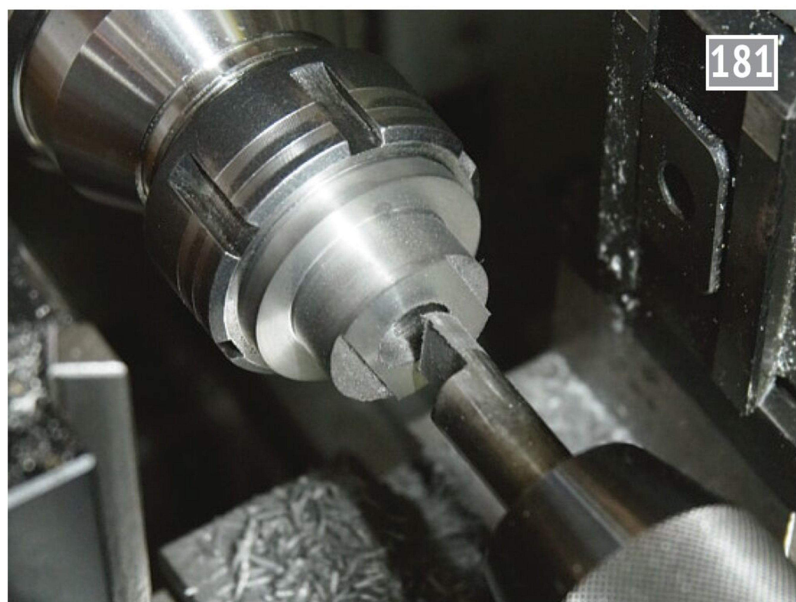
The rear cover needs clearance for the piston locking nut.
