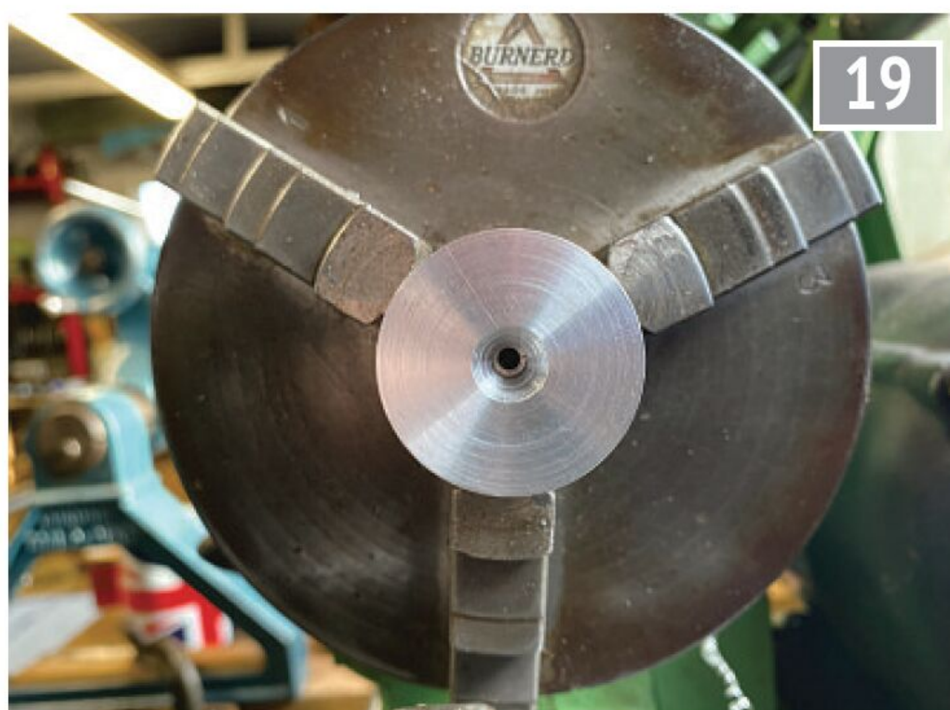
A countersink formed by a Slocomb drill.
