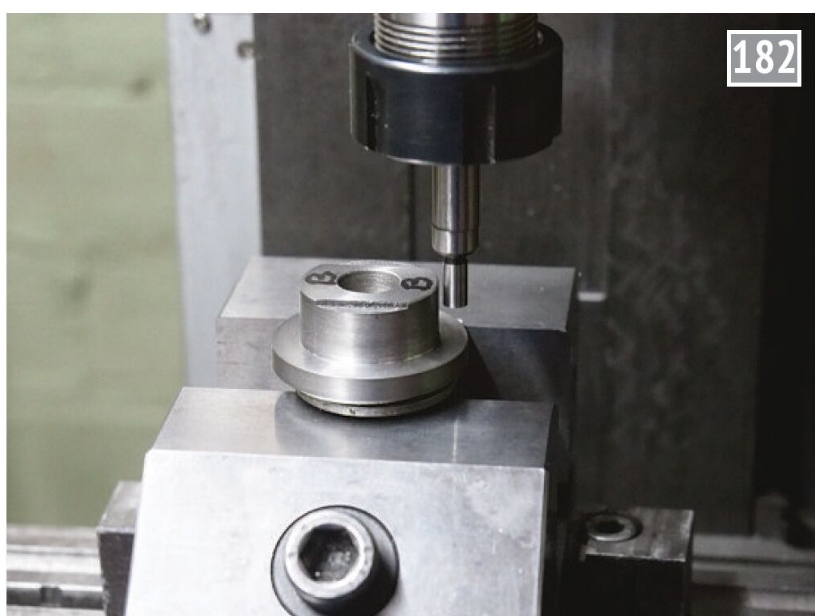
The chucking piece is left attached and is held in a V-block so that a edge finder can be used to align the axis of the with that of the mill spindle ...
