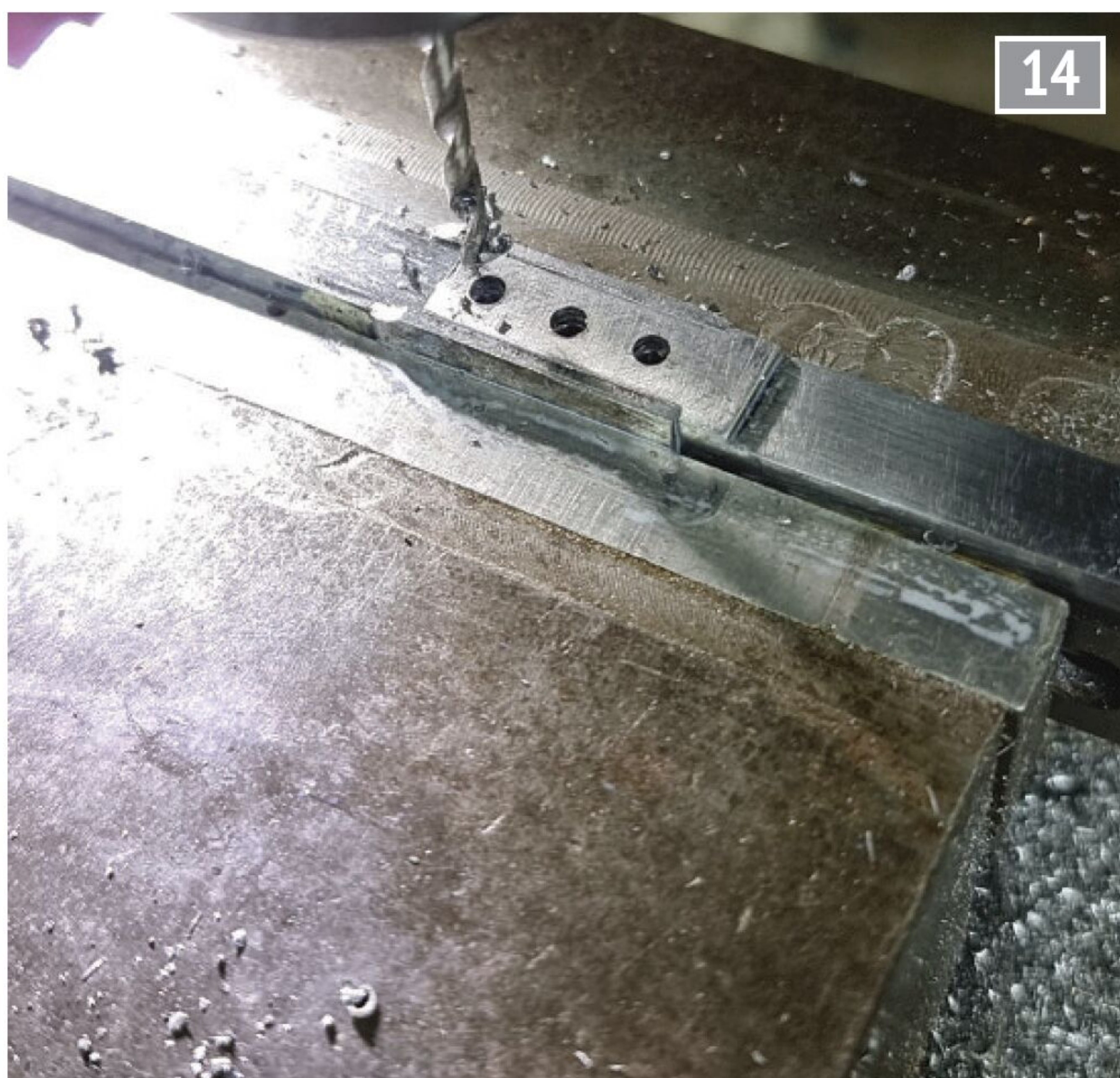
With the bulges added, the fixing holes are drilled.
