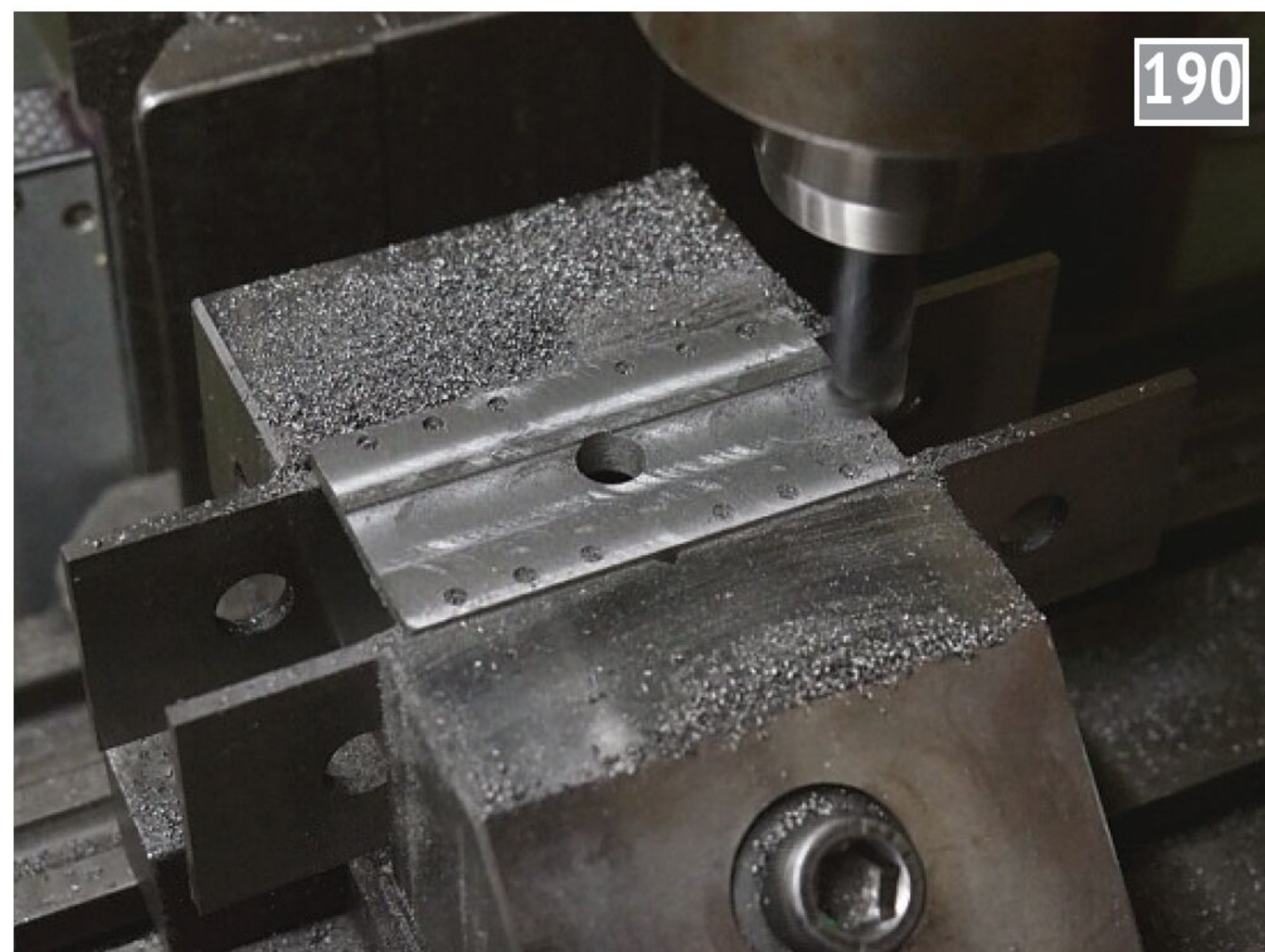
Drilling through released the chucking spigot and the part was brought to finished thickness.
