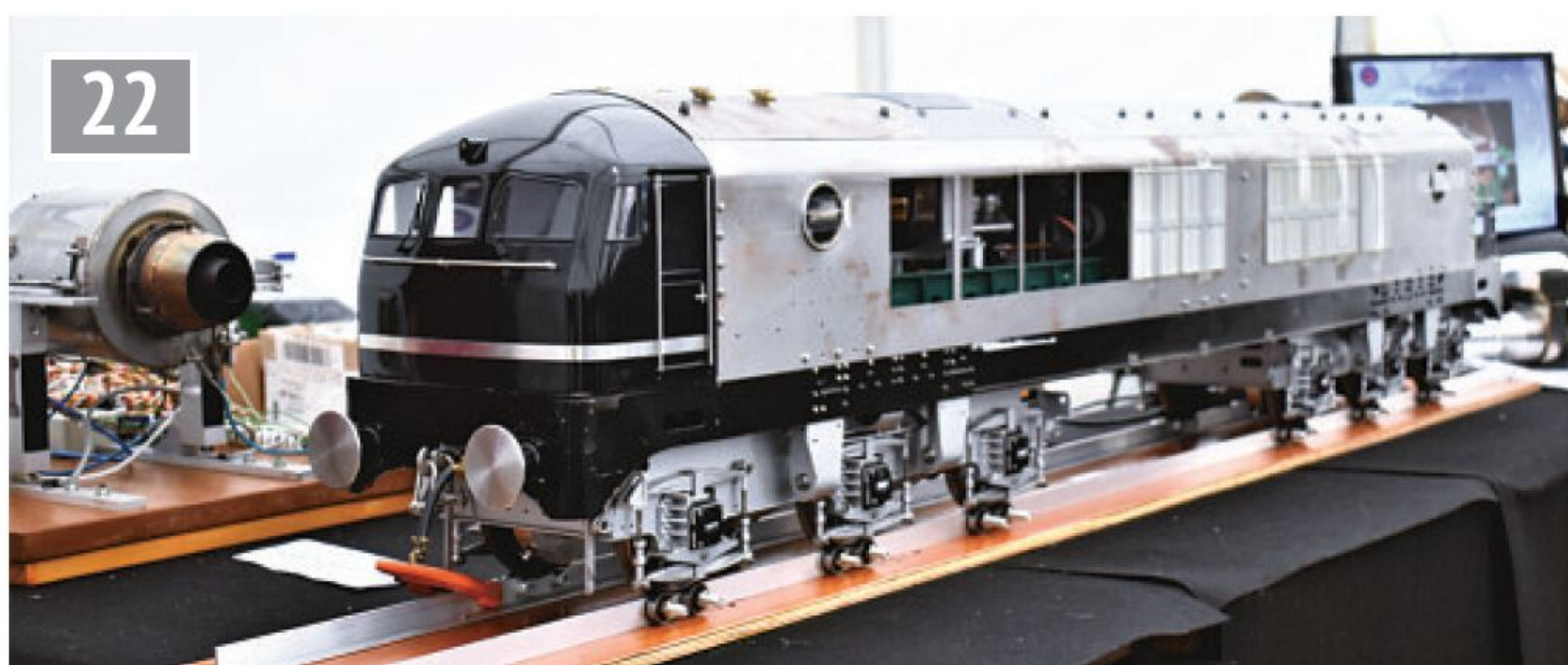
The turbo-electric locomotive No. 18100 almost complete.
