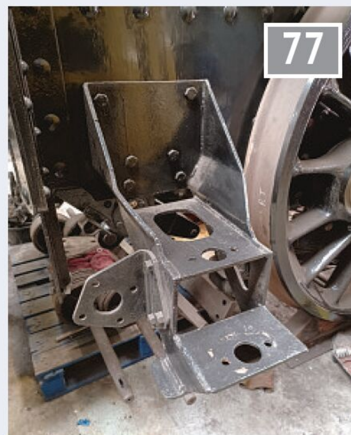
Right-hand injector bracket (Toddington Standard 4MT).
