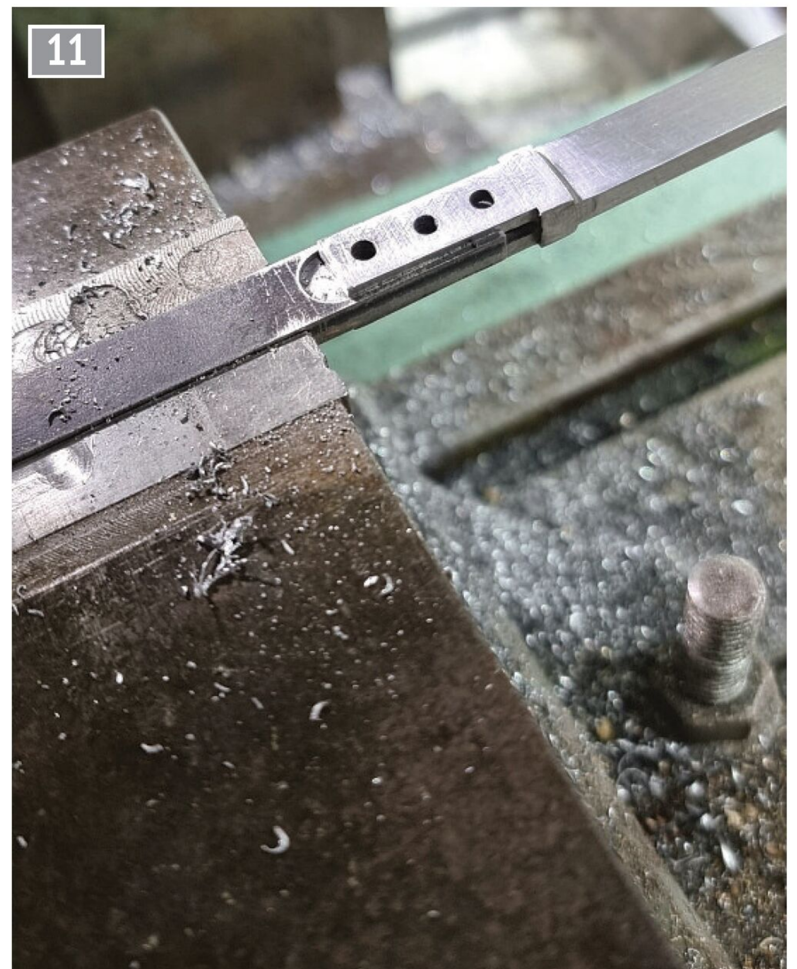
Test fit of the reach rod joint.
