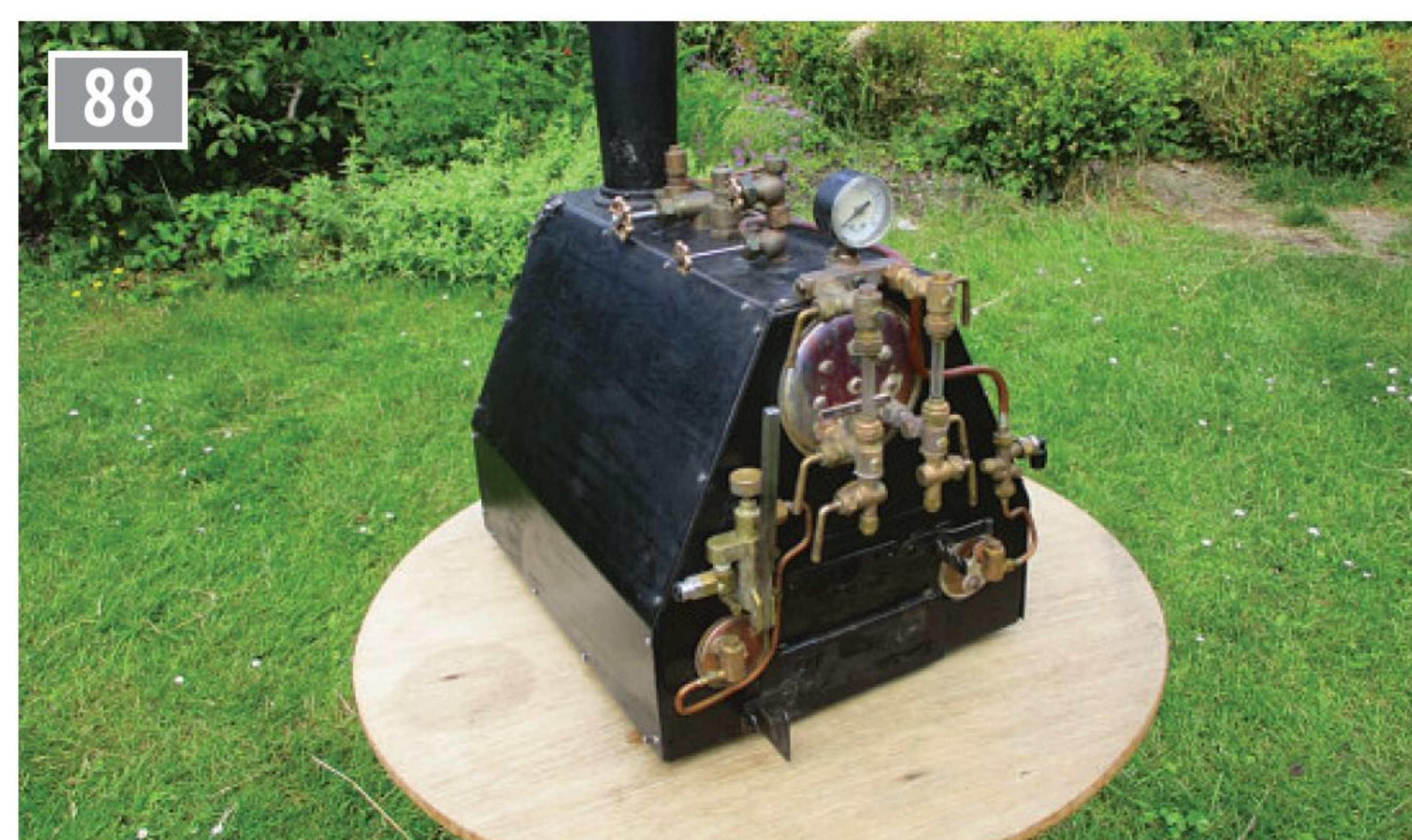
Steam is supplied by a Yarrow boiler.
