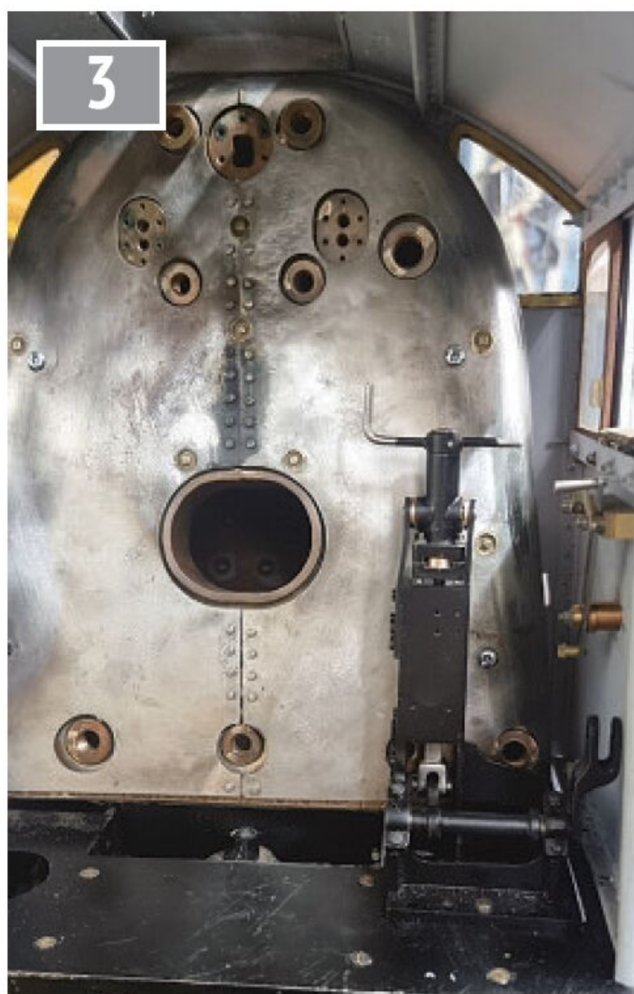
The reverser correctly located in the cab.
