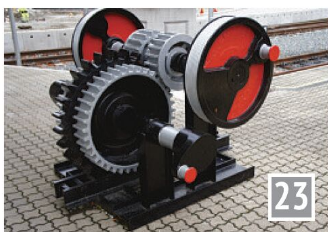
Demonstration of how a rack locomotive works at Jenbach. The Achenseebahn uses the Rigenbach system with a ladder like rack in the centre of the track.
