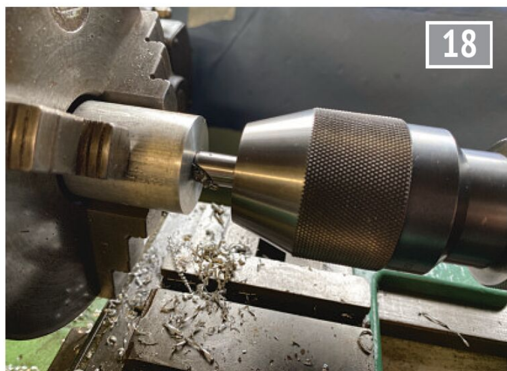
Using the Slocomb drill to form a countersink.
