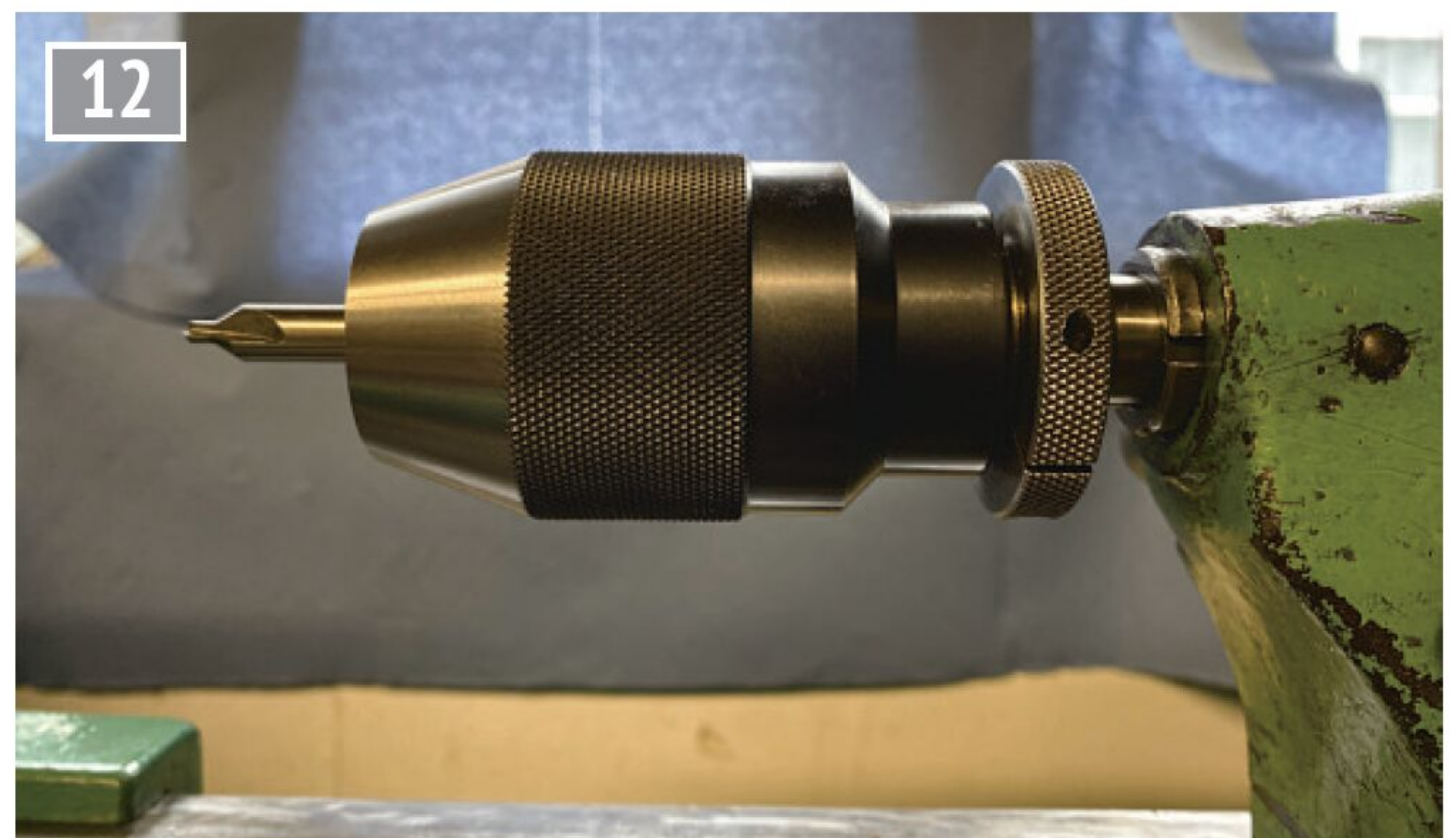
A quick release chuck mounted in the tailstock.
