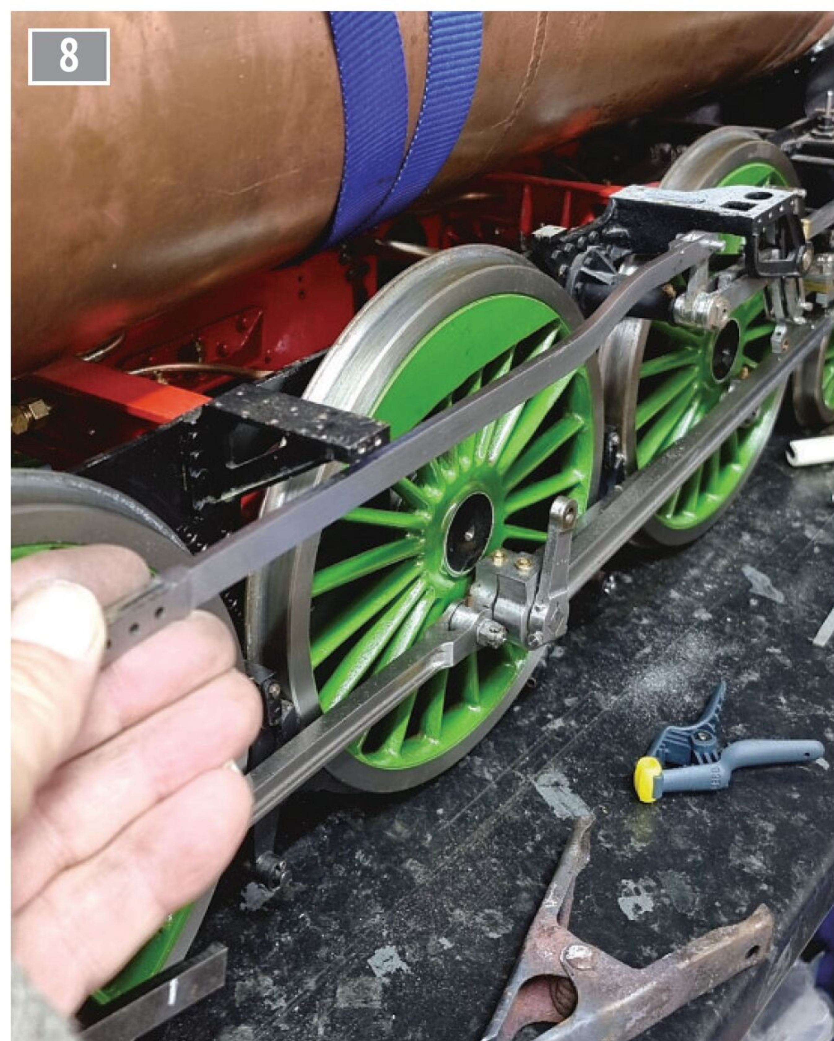
Test fitting the front end of the reach rod.
