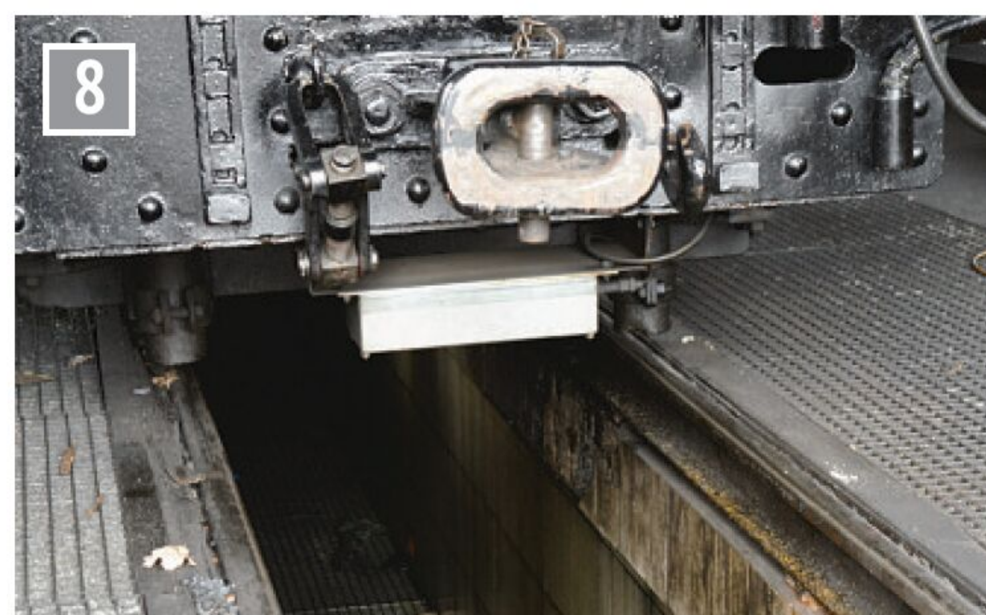
Balises like this are fitted to locomotives to enable exact locations to be known.
