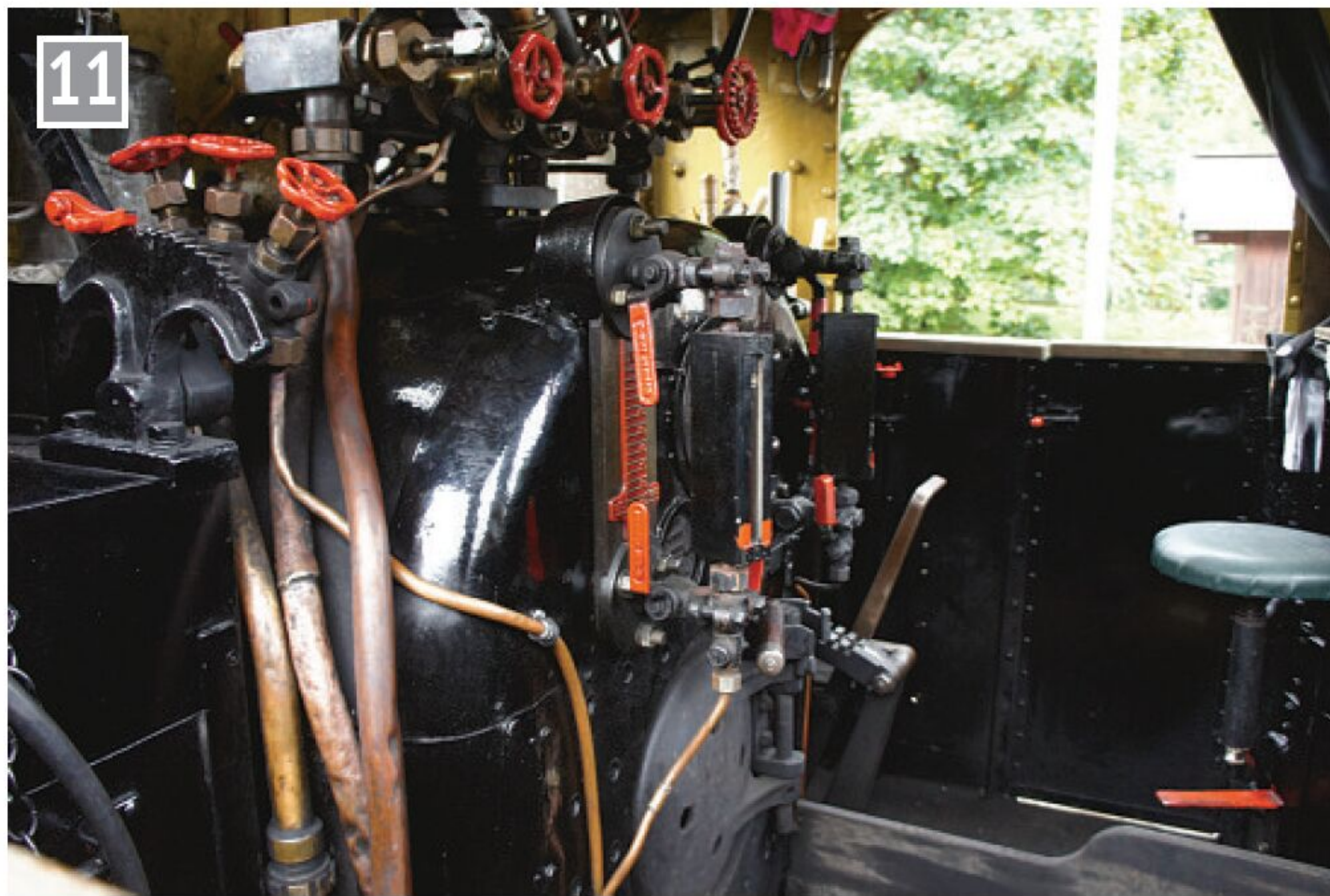
Cab picture No. 3 - note the weight on the cut off lever.
