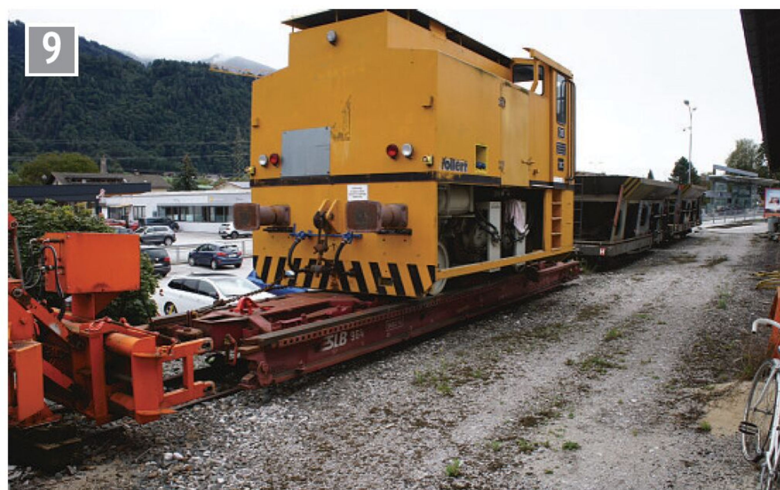
Standard gauge shunting locomotive on a transporter wagon. The ZB has a short length of standard gauge track at Jenbach.
