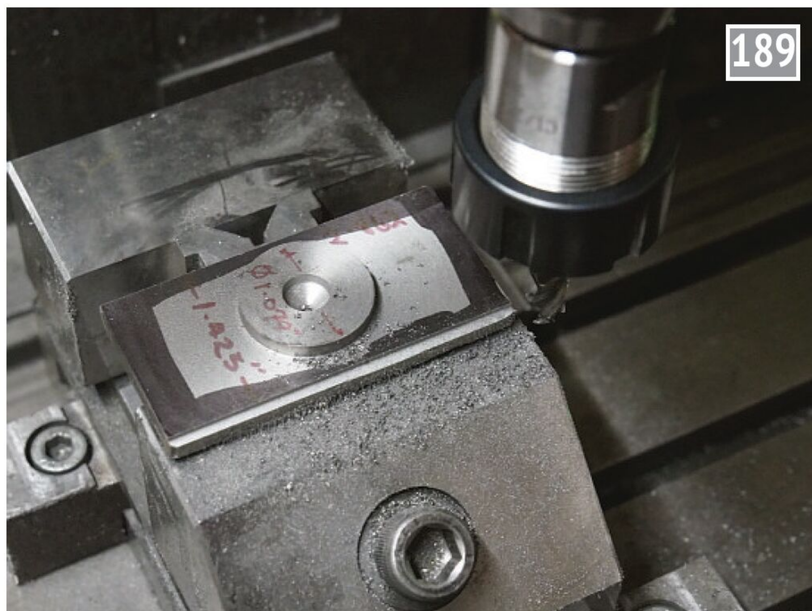
... so that it could be used to align the part for milling the edges square and drilling the securing holes.
