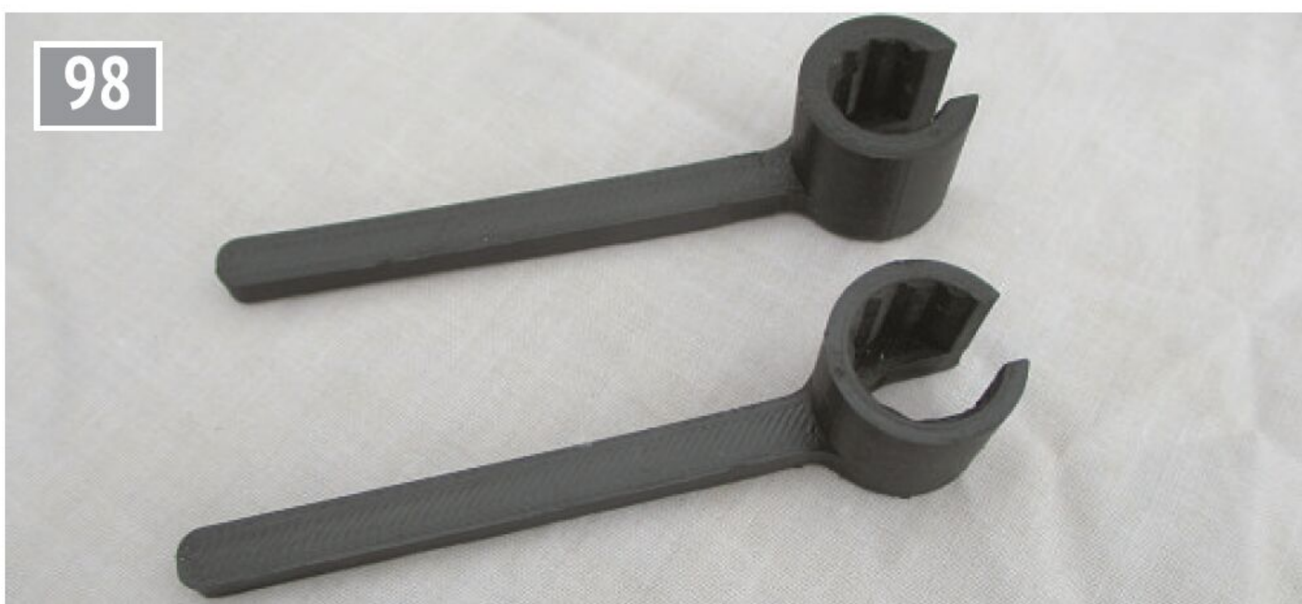
3D printed custom spanners for gland nuts and lock nuts.
