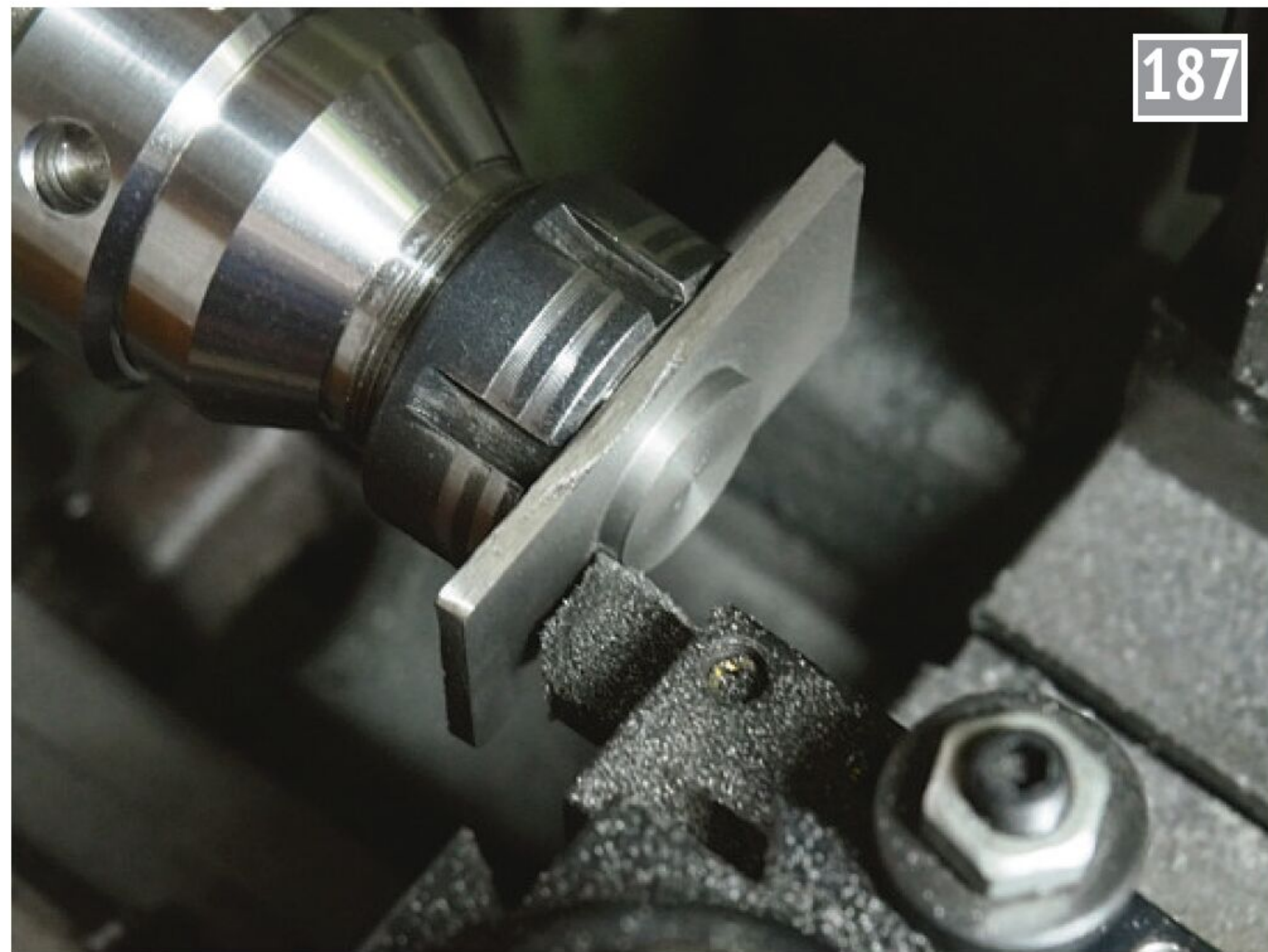
With a clean chucking spigot, holding the piece to machine the outer surfaces is easy.
