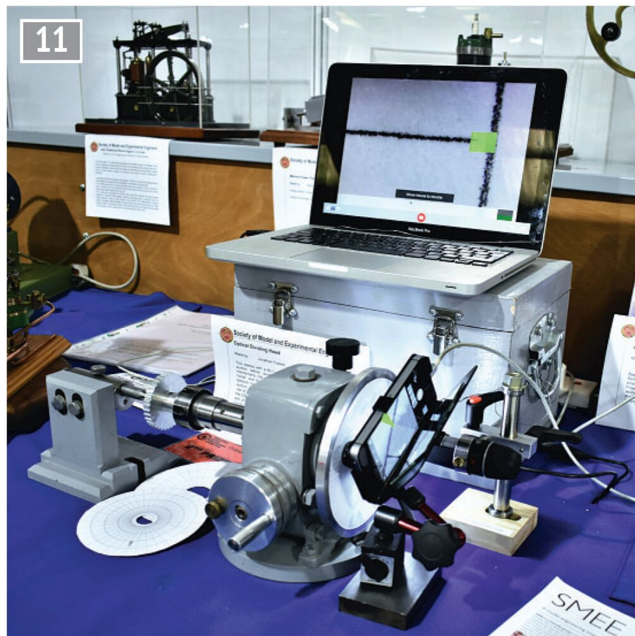
An optical dividing head based around an existing worm drive gear box.
