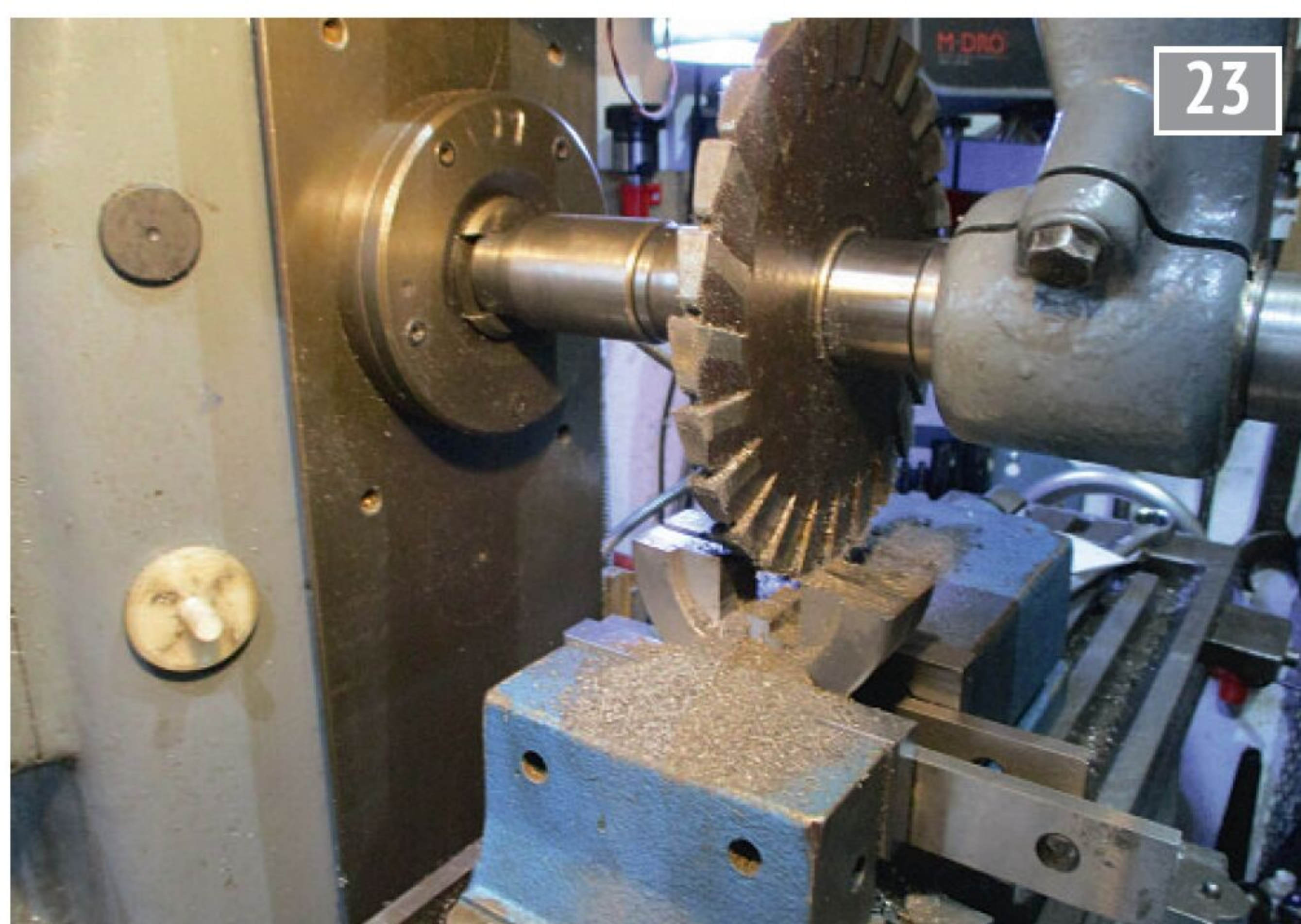
Finishing the counterweights.
