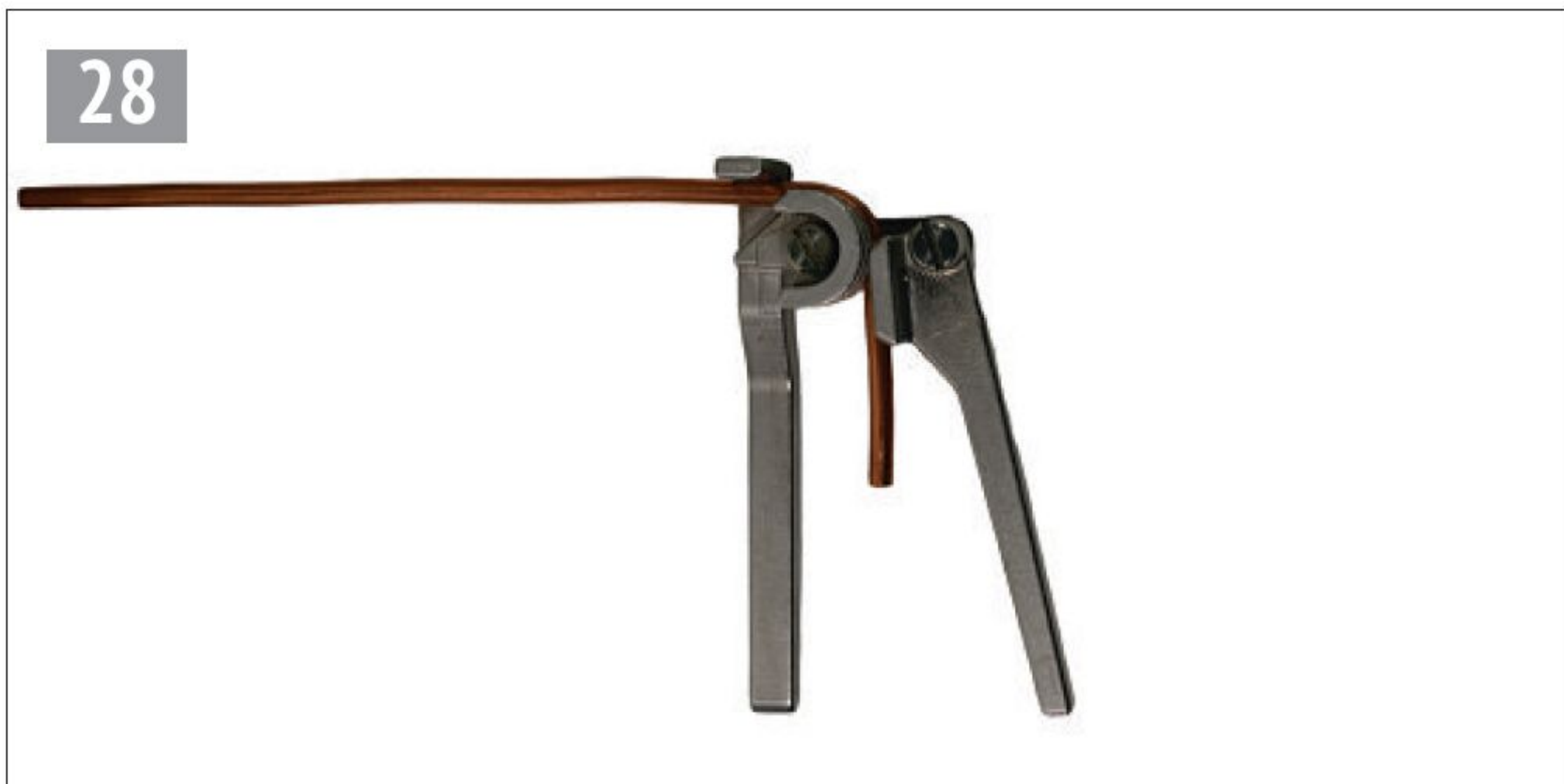
Pipe bender in action.
