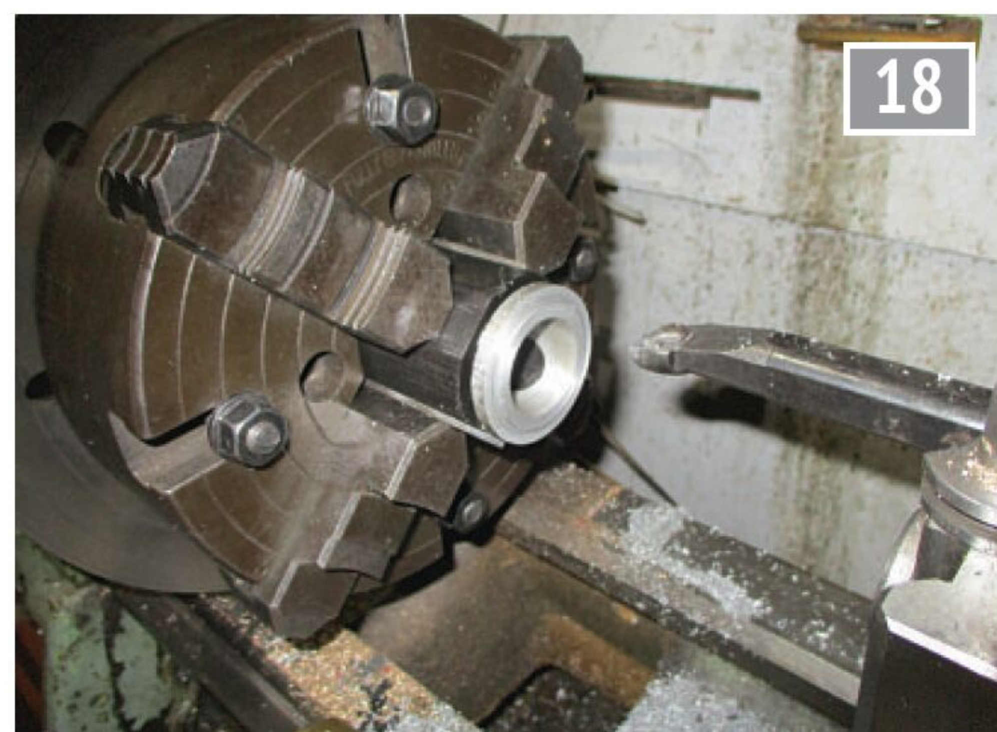
Boring the crosshead guide.
