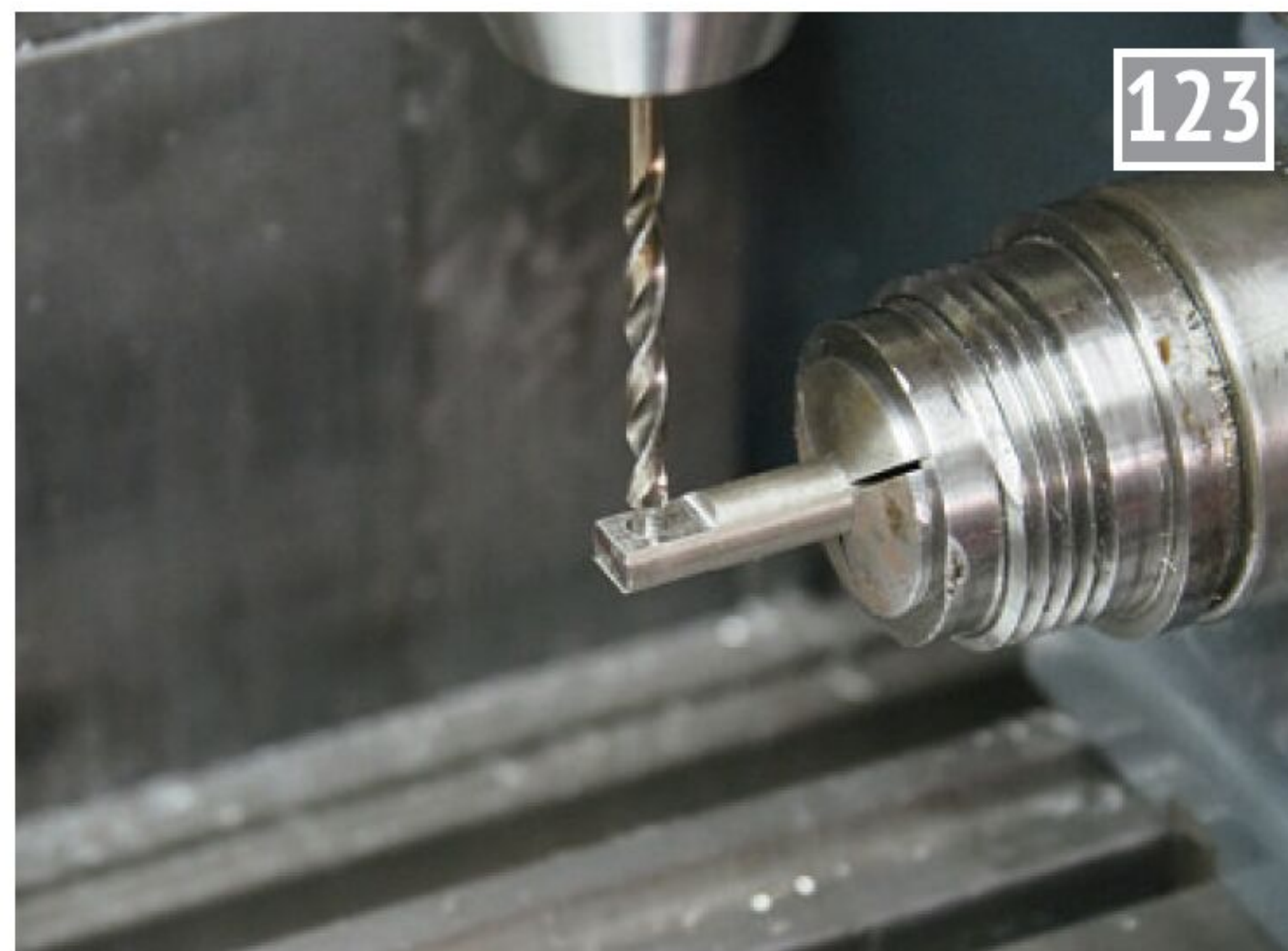
... then turning through 90 degrees to drill the pivot hole.
