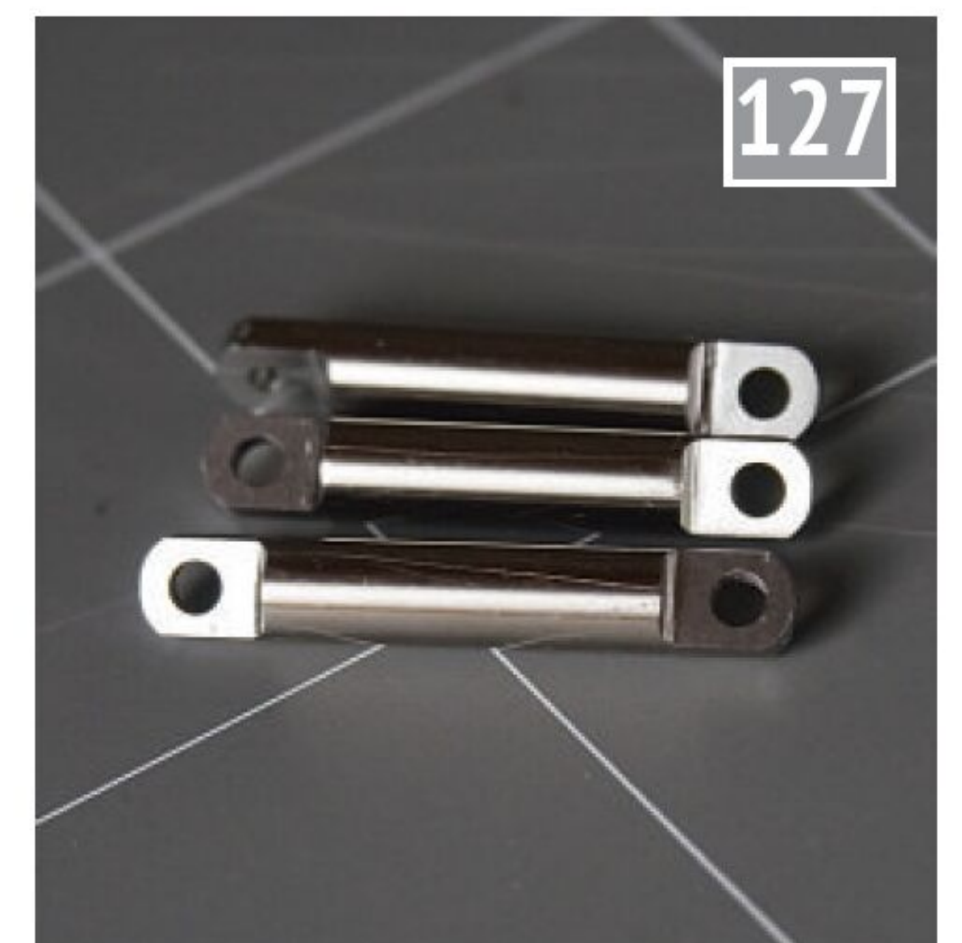
Making the rods' ends in pairs is a big help when it comes to keeping hold of them. After the stage shown here, they are cut apart, machined to length and the axial holes drilled and tapped.
