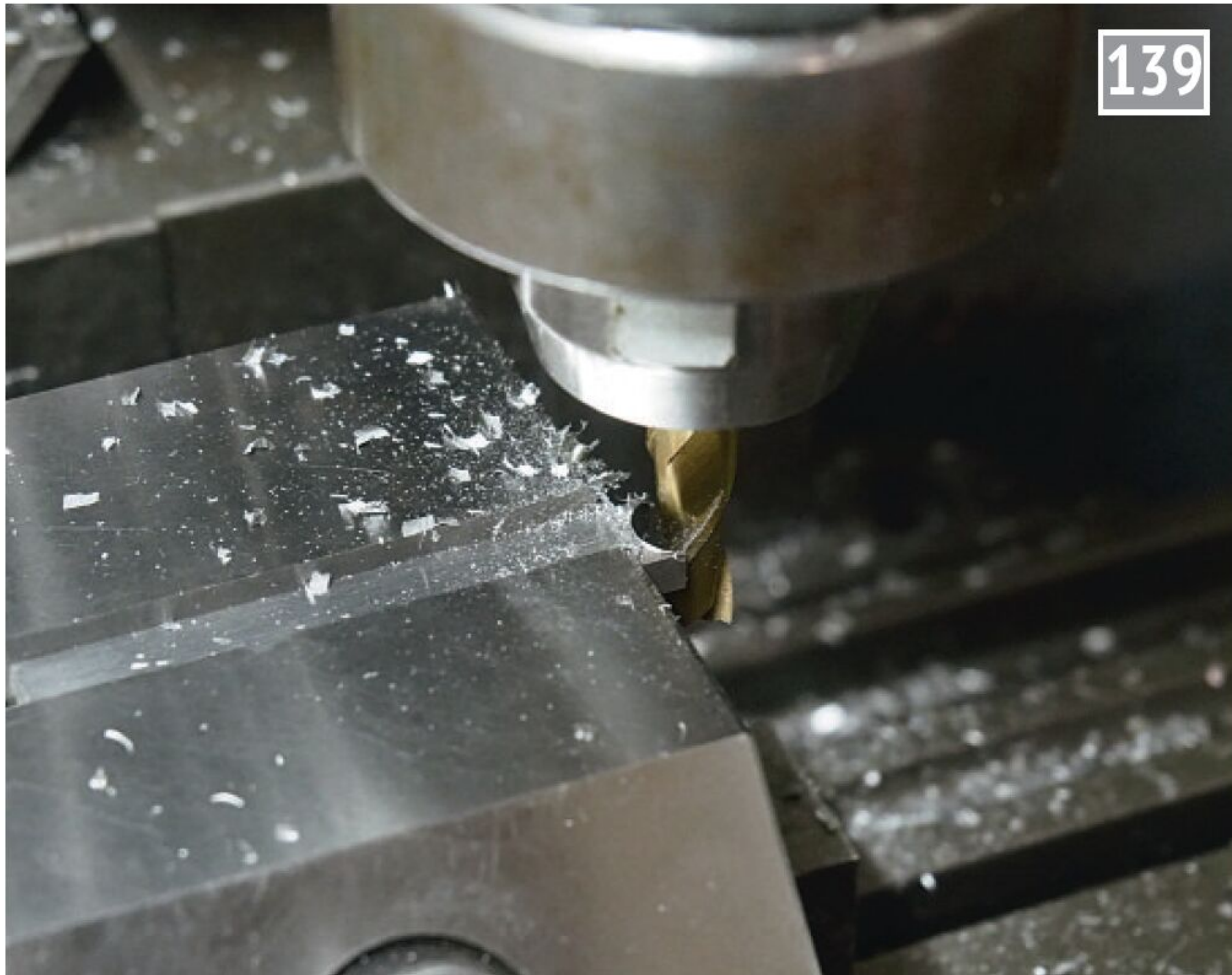
Cutting the scallop in the lower end of one of a pair of uprights ...
