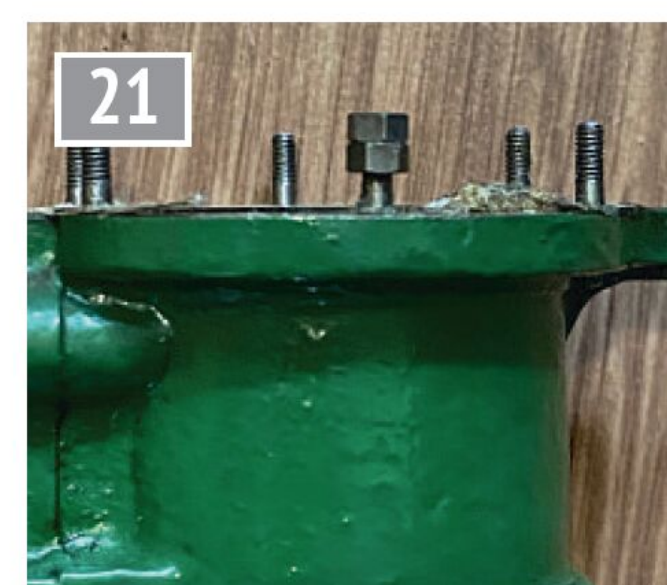
21 It's easy to remove studs without damage by running a pair of nuts tightly together - your spanner in this instance needs to be working on the lower nut.
