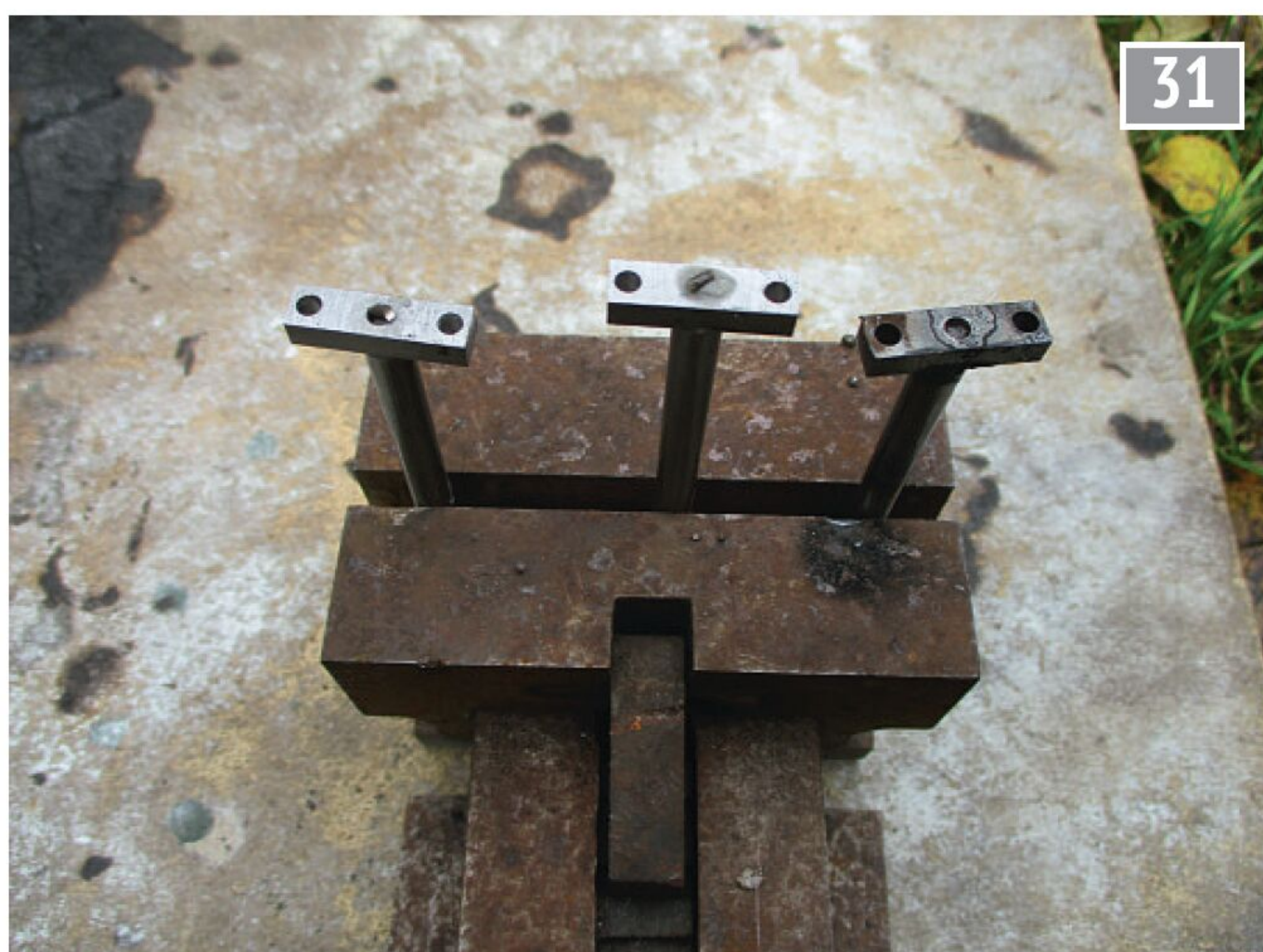
Silver soldering the ends to the rods.
