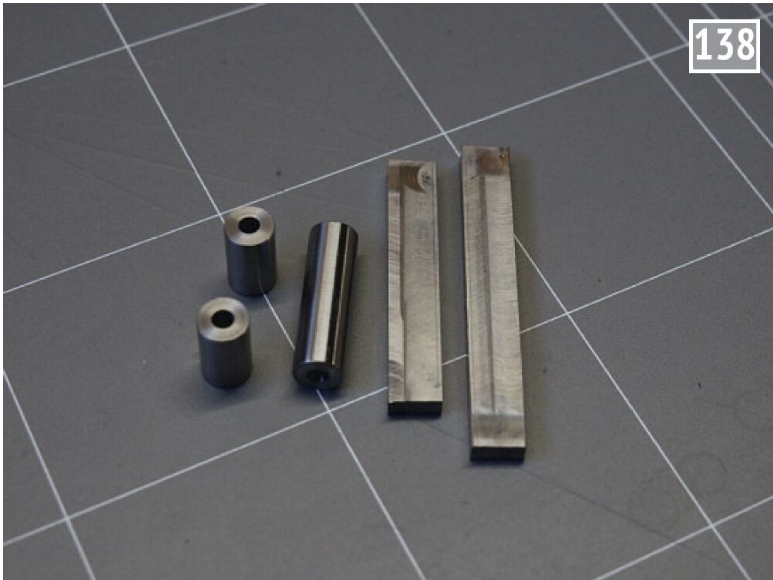
The rockers were built up from stock round bar and flats milled to size.
