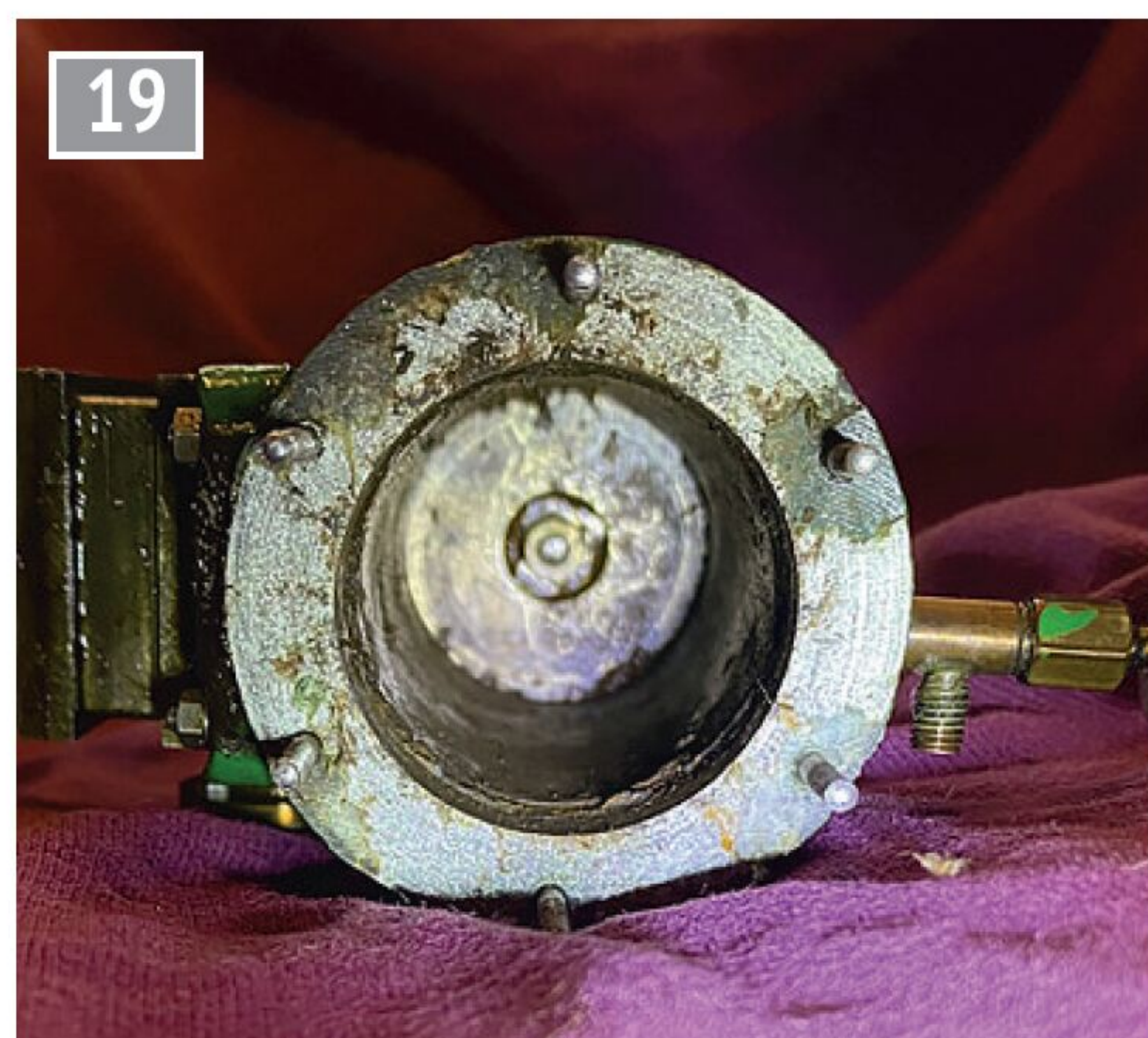
19 A ray of hope - the cylinder bore wasn't a write off and there was a nut visible on the underside of the piston.
