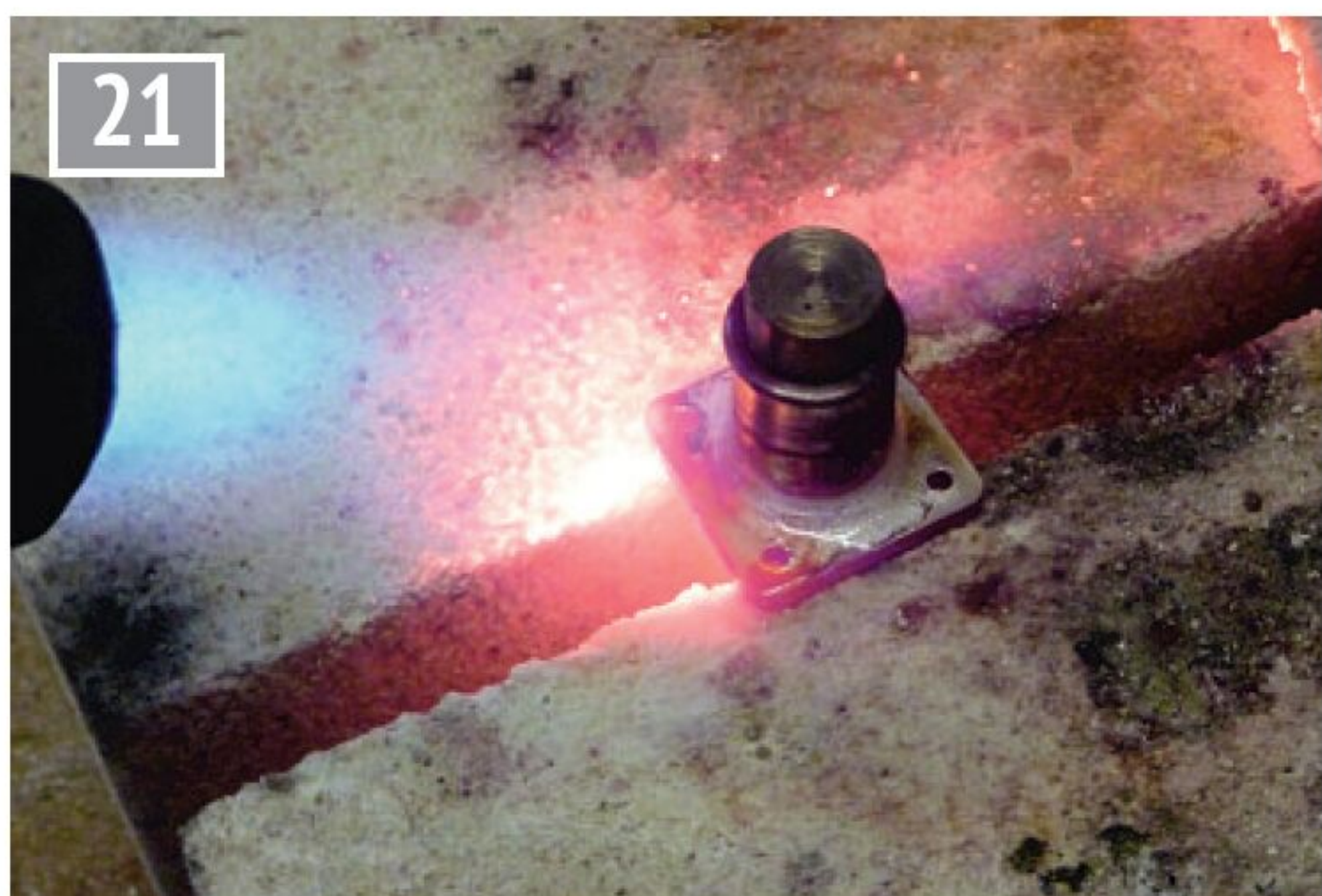
21 Silver soldering a buffer stock.
