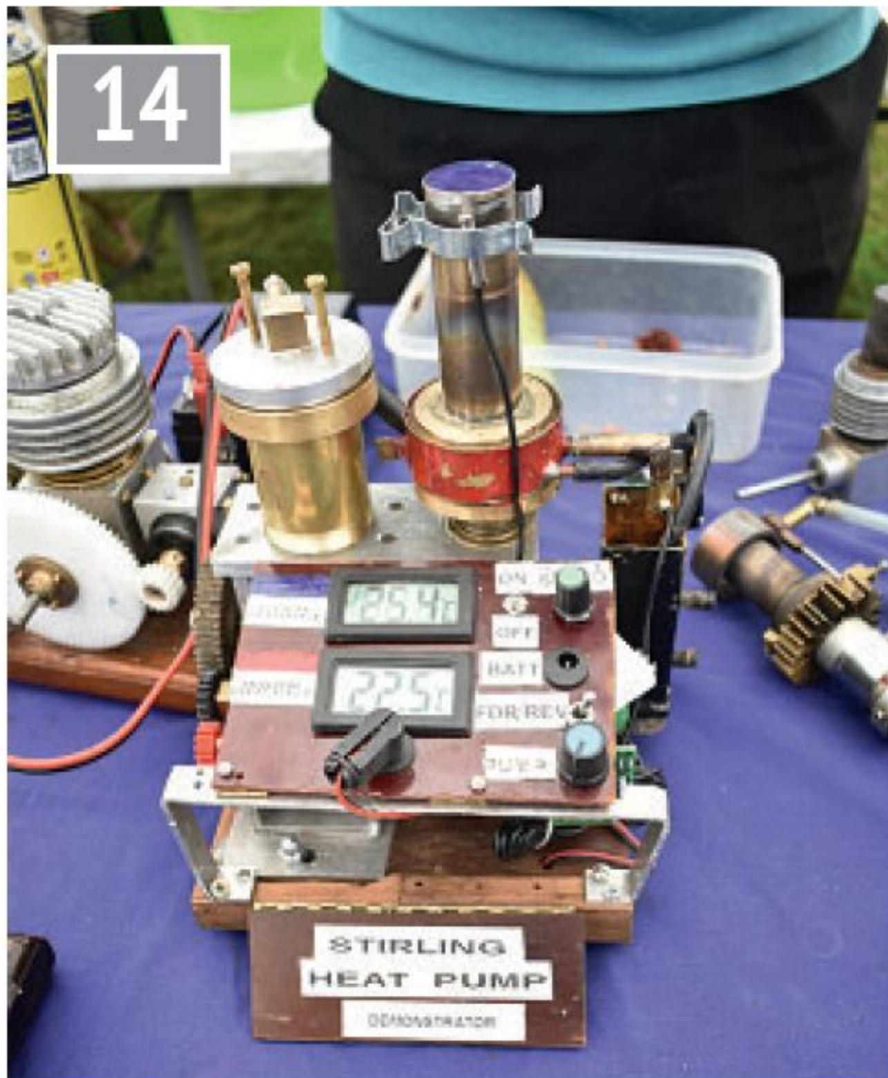
Julian Woods latest experimental engine is this hot air heat pump.
