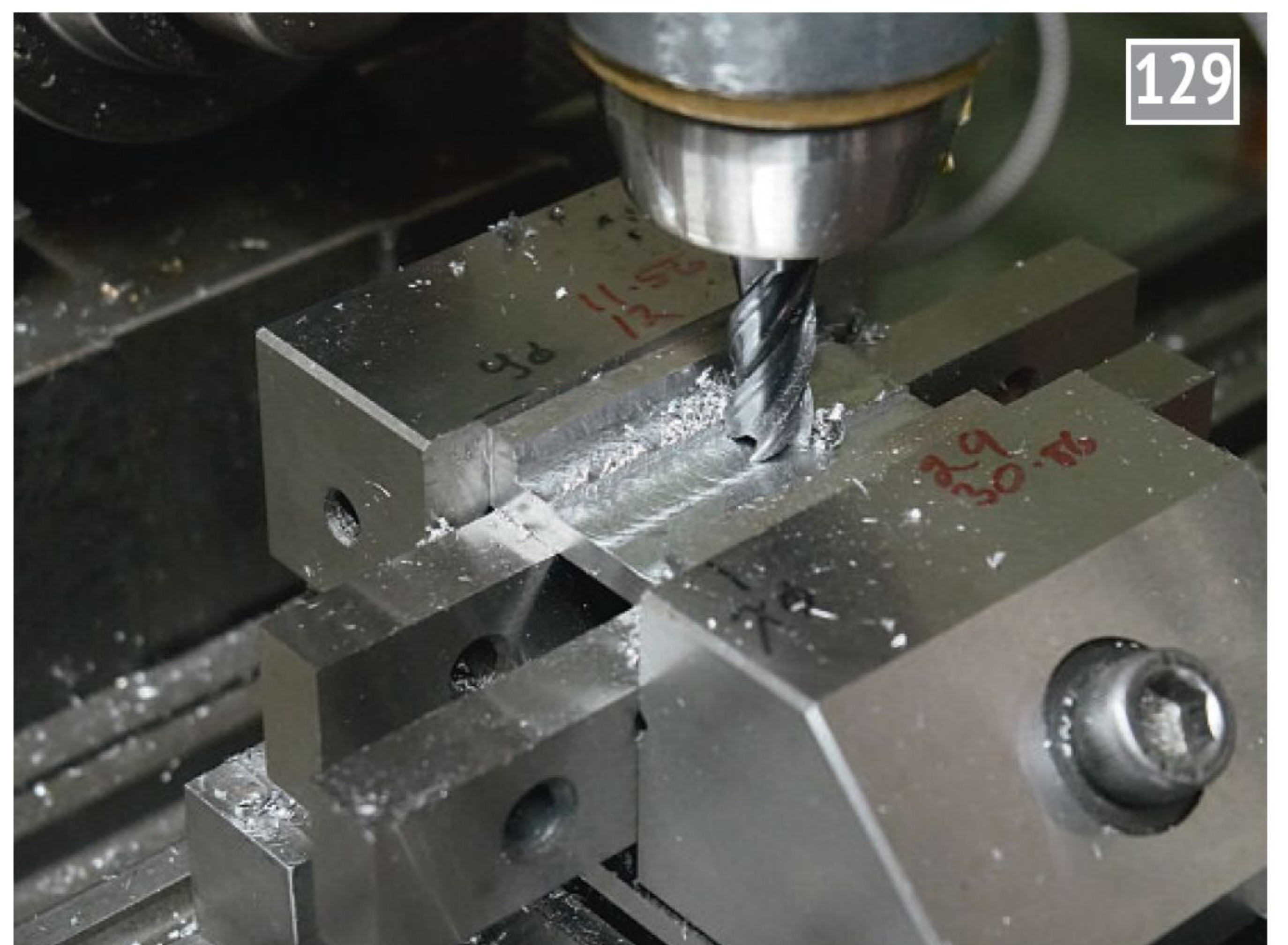
The two fulcrum brackets were carved from the solid as a pair – first the central trough.
