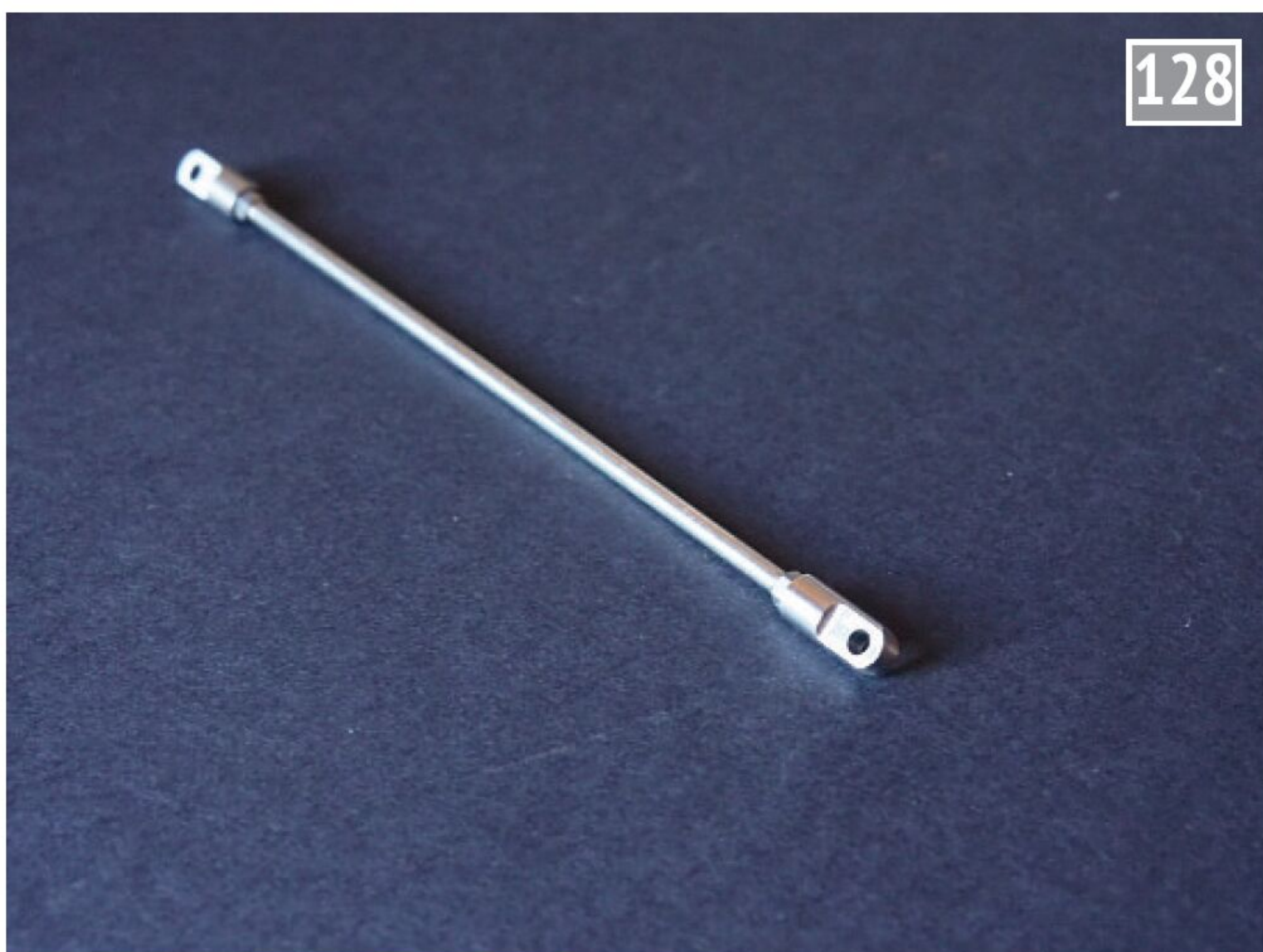
The rods are made from stock and the ends attached. Thin locknuts of the correct appearance will need making.
