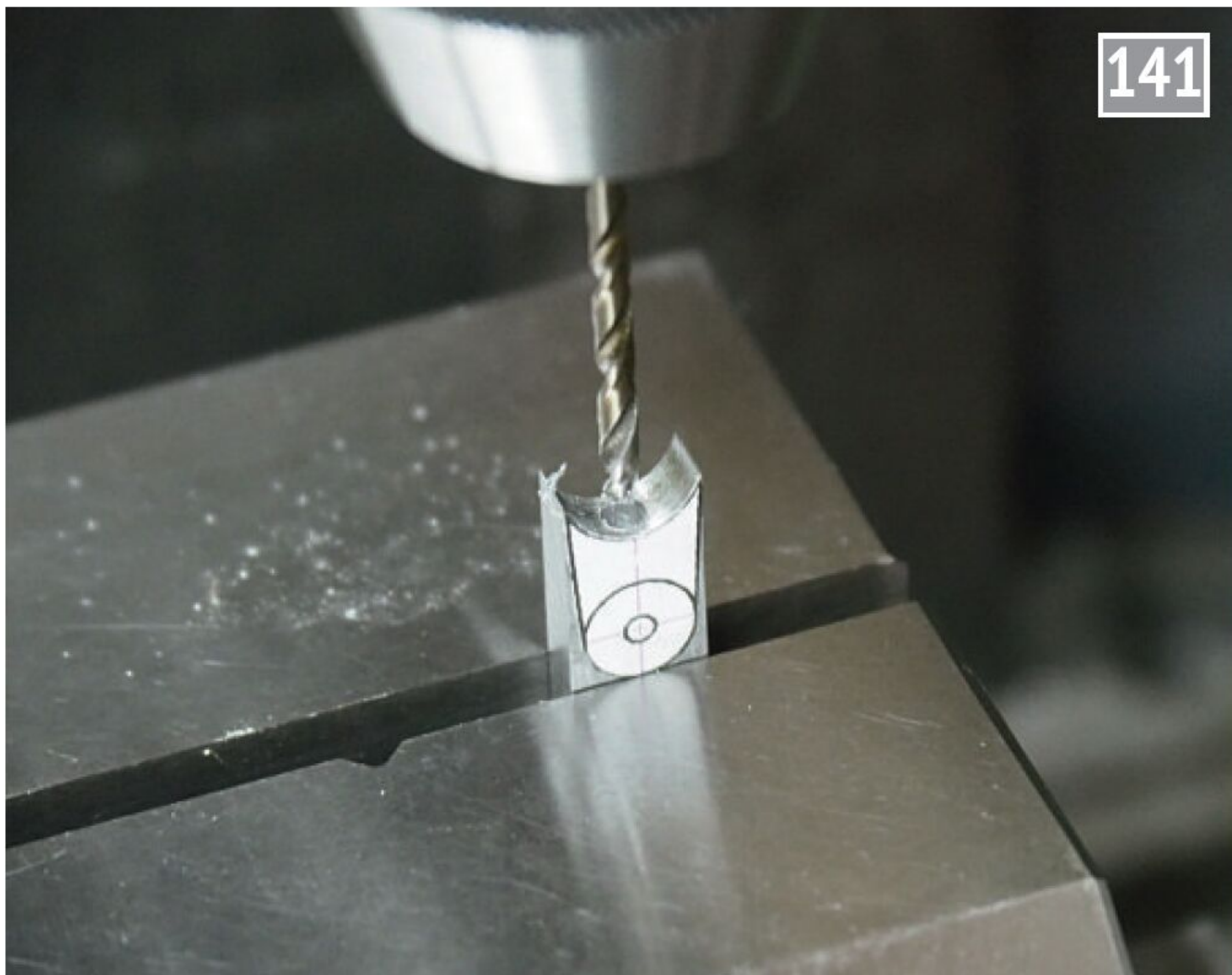
... and drilled axially for a peg to hold things together during assembly.
