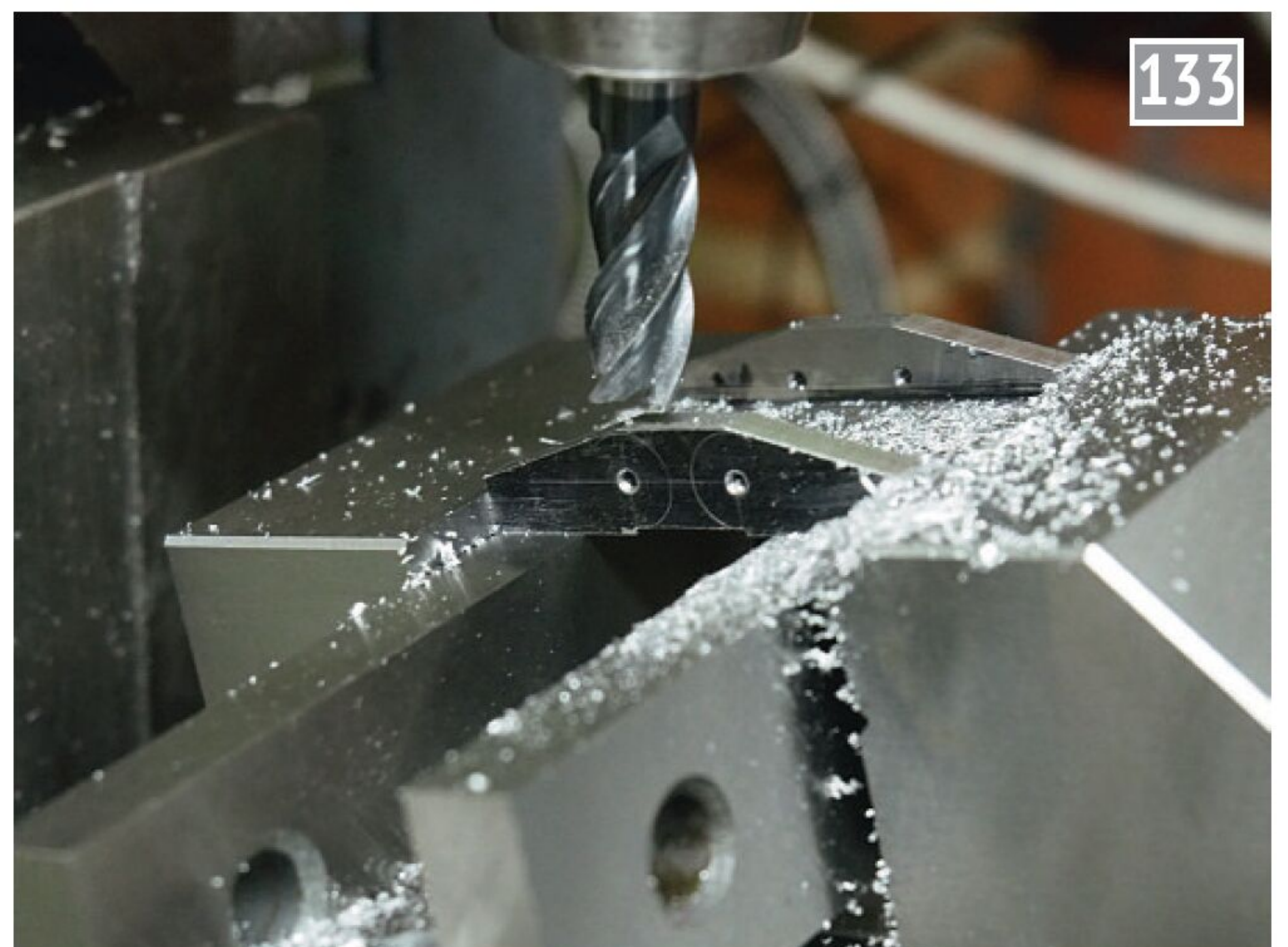
A sine vice makes it easy to set up the slope of the sides, but the parts could be gripped in an ordinary vice just as readily.
