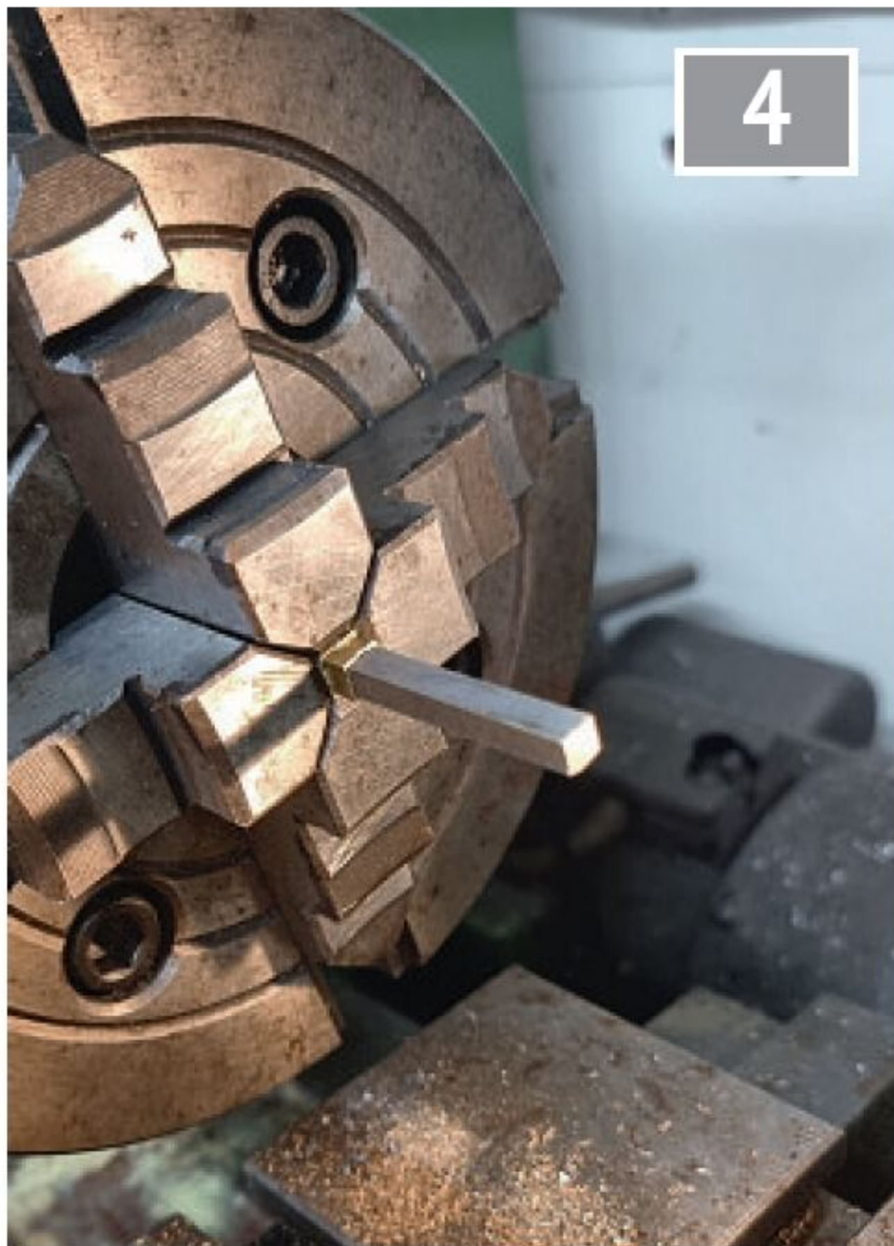
Using square brass tube to hold the work.
