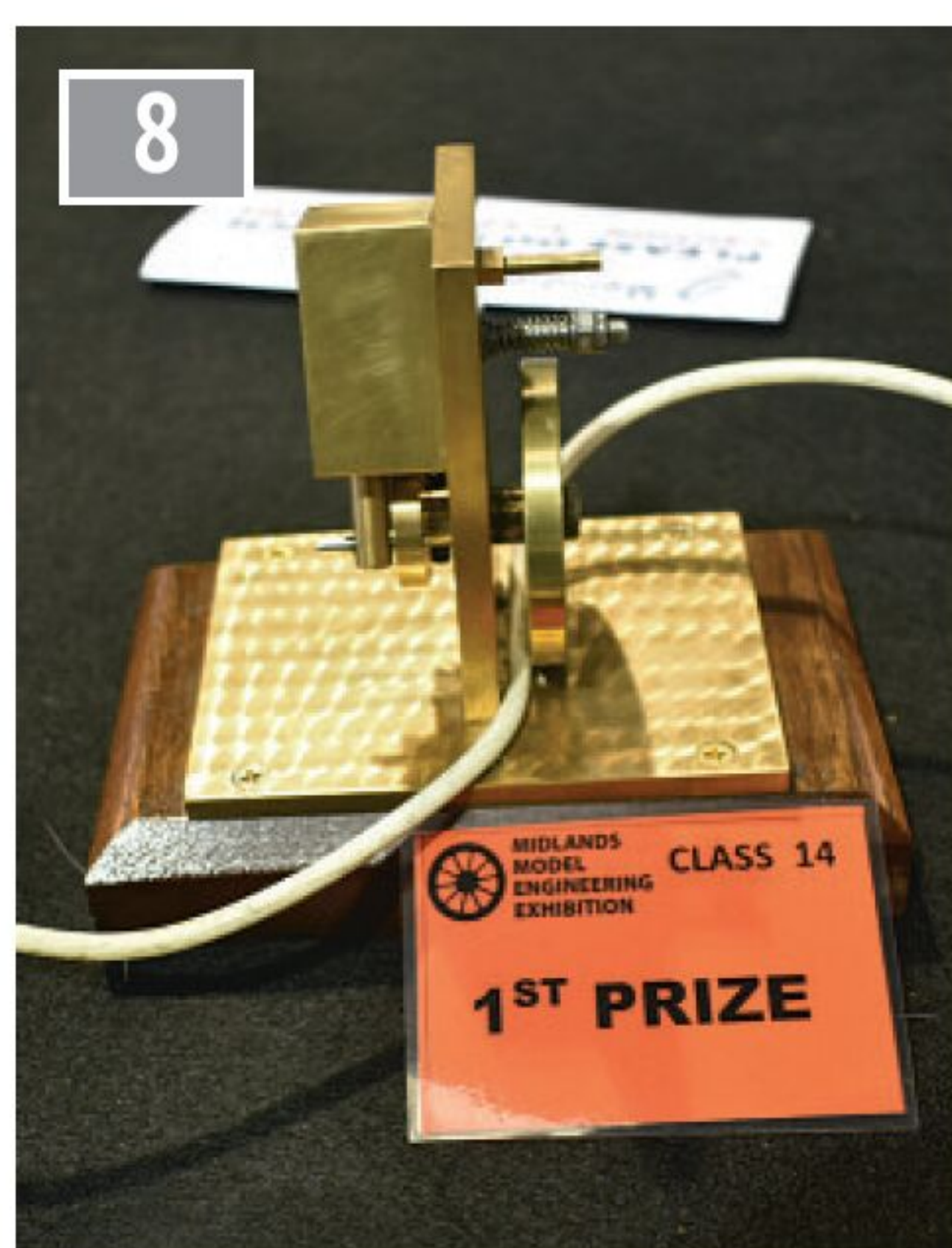
Twelve year old Tommy Pugh-Bodman built this small oscillating engine from scrap material.
