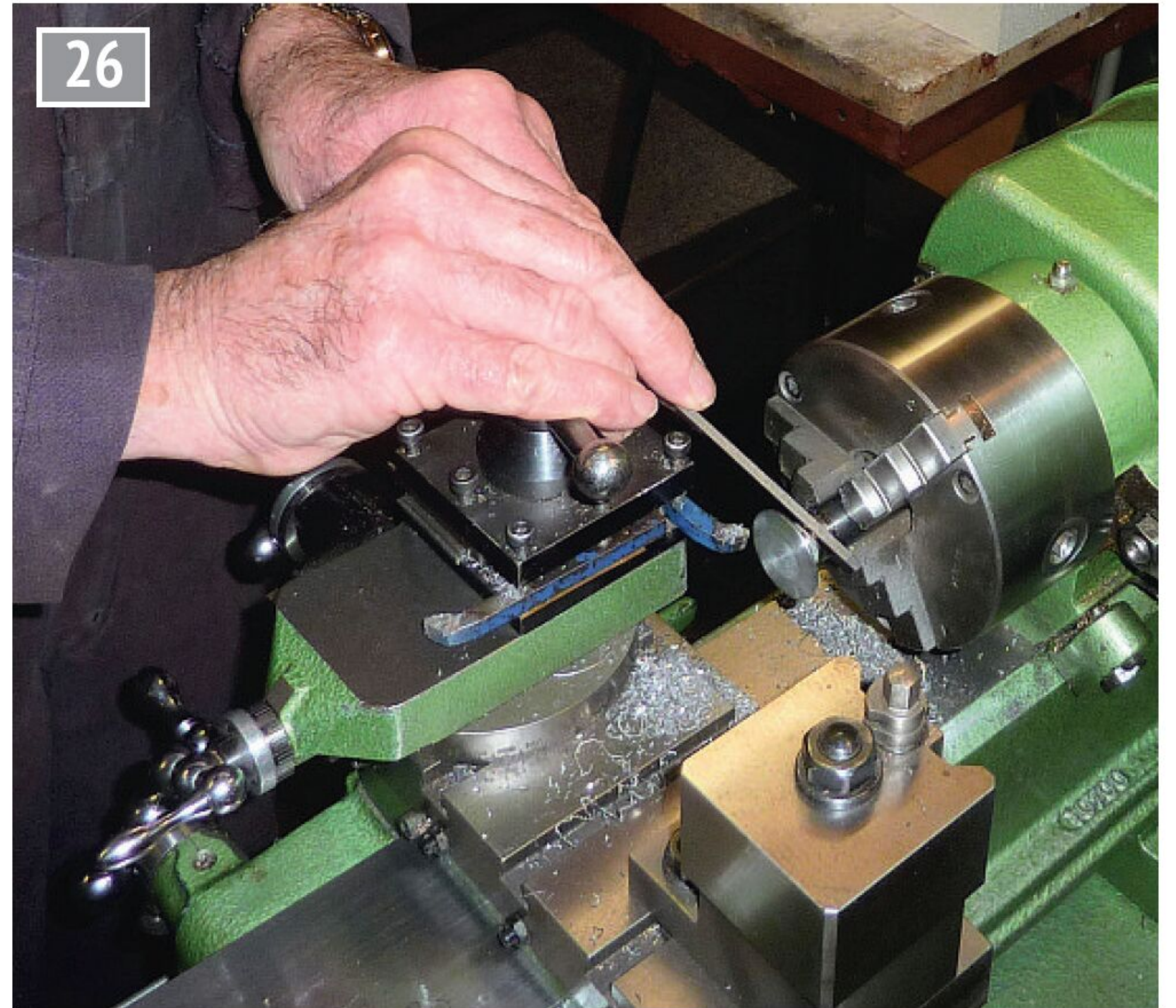
Shaping the edge of the buffer head.
