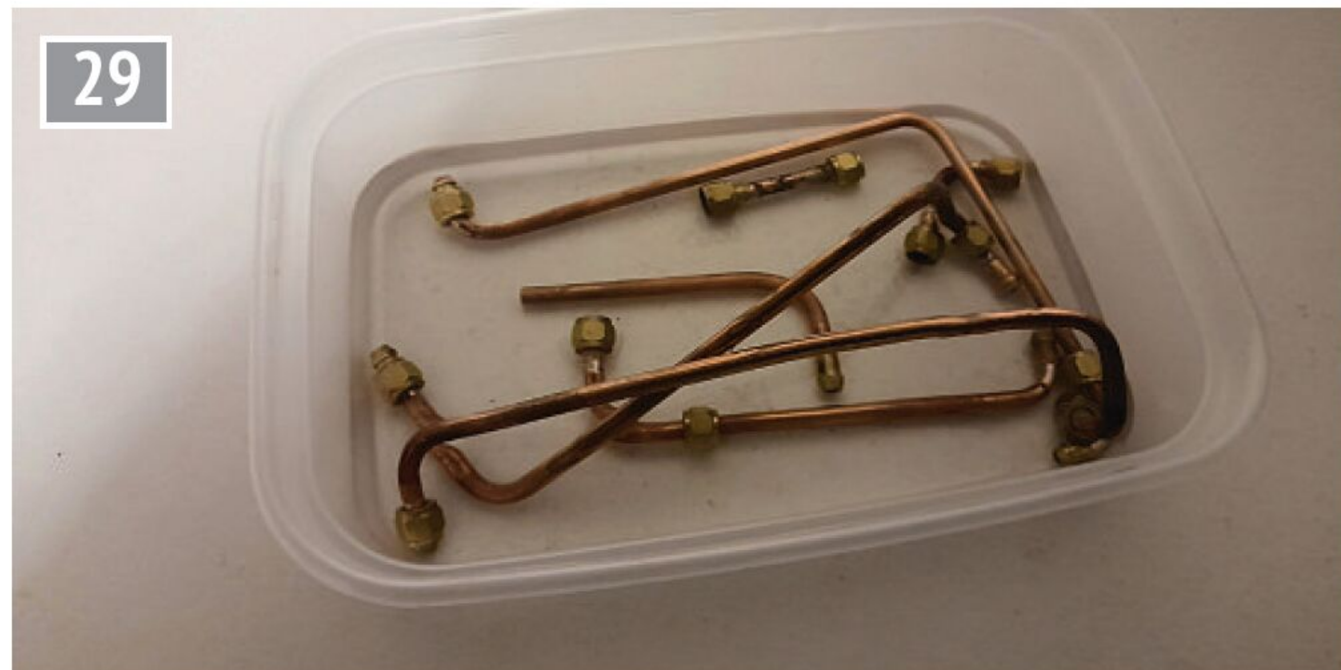
Pickling the pipework.
