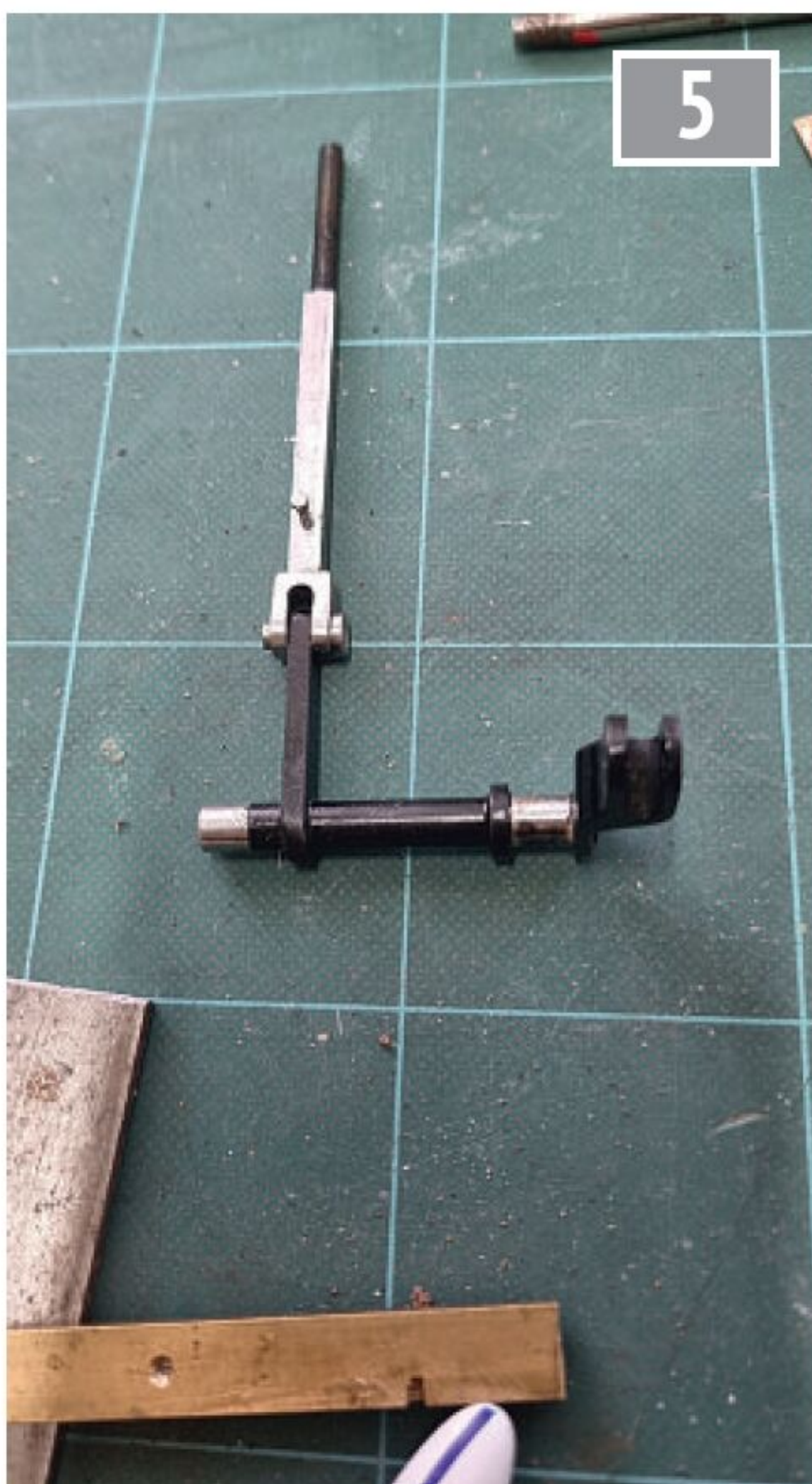
Screw and shaft temporarily assembled.
