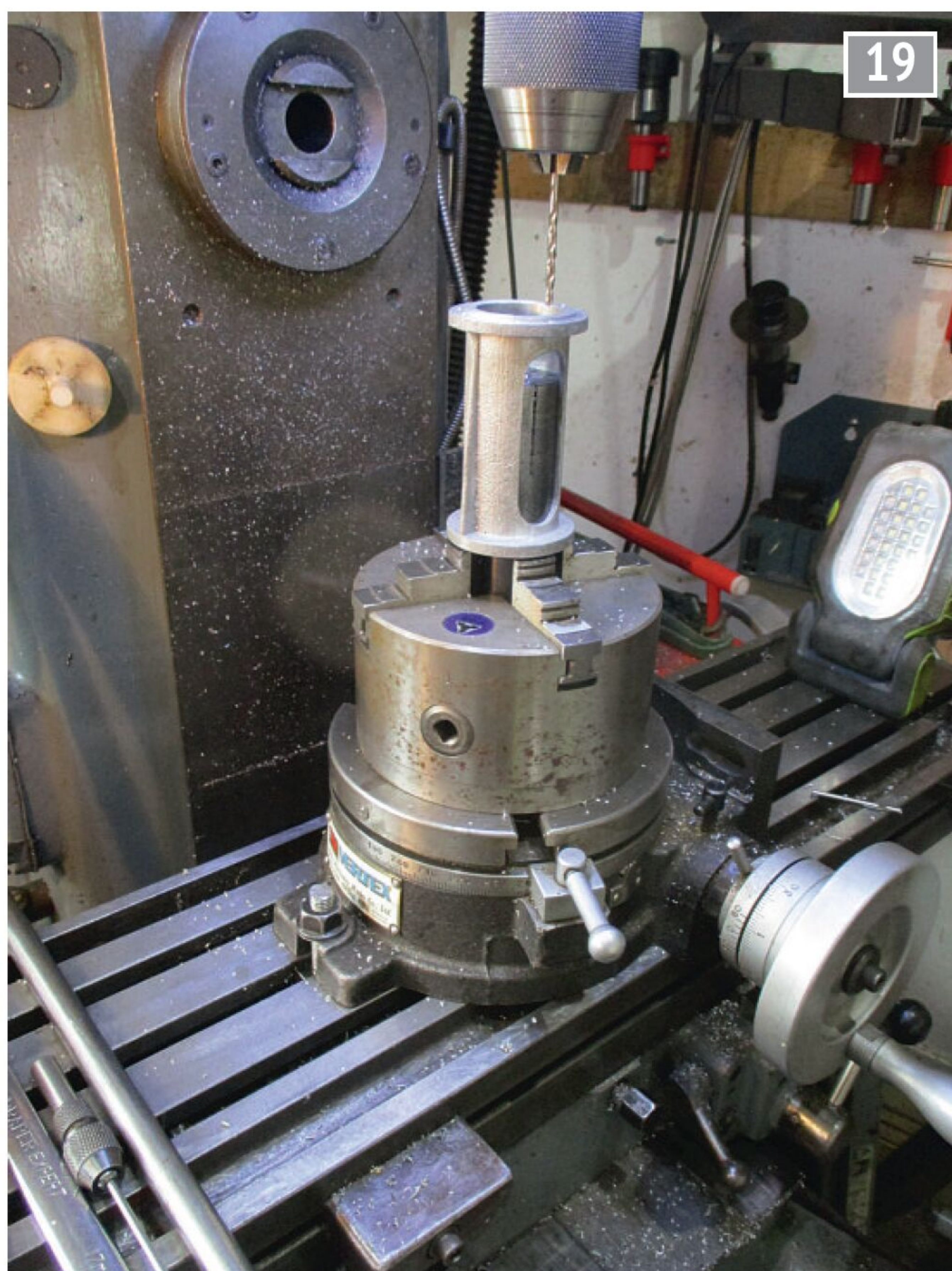
Drilling the fixing holes.
