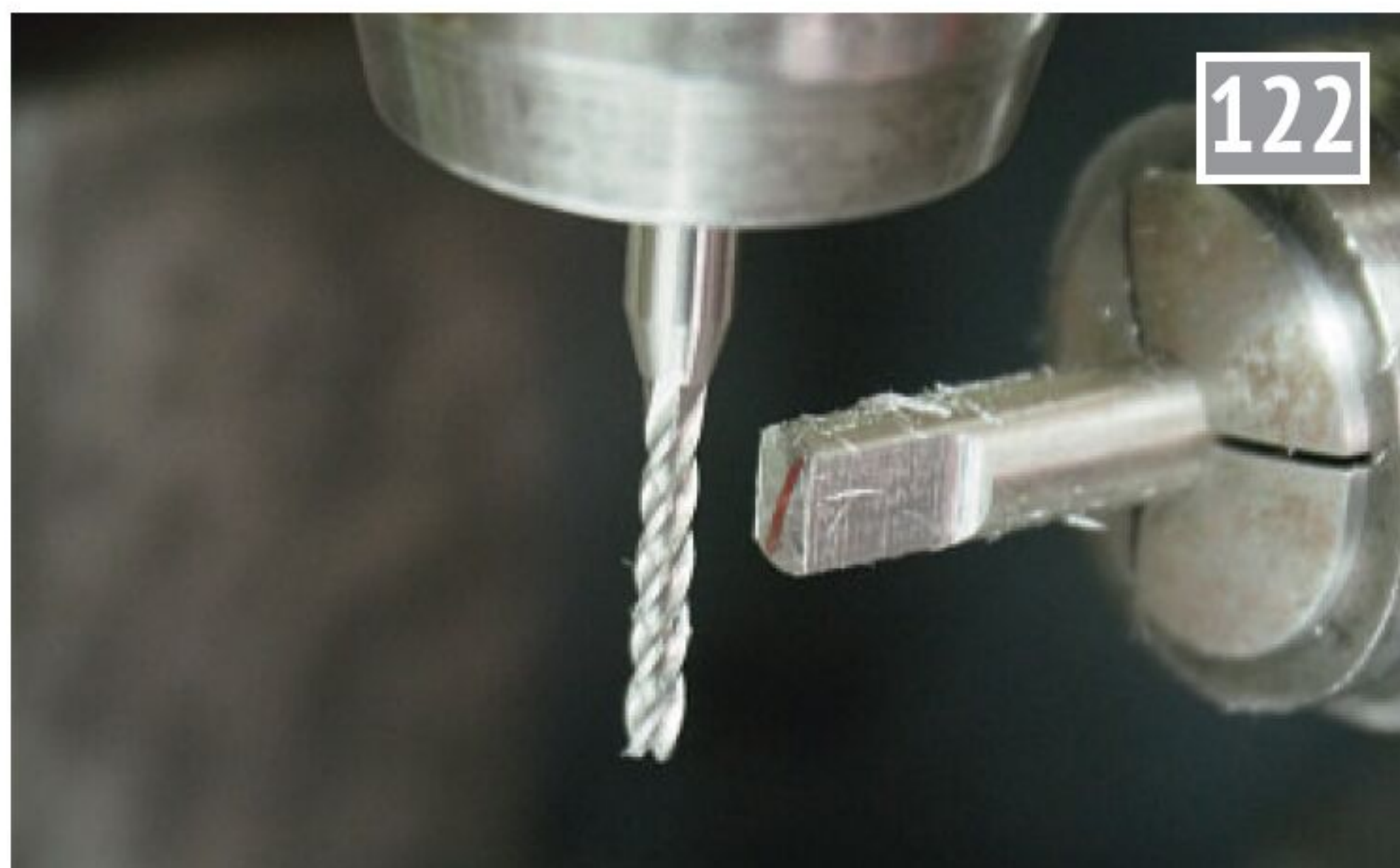
One useful way of making rod ends and clevises is to mount the stock in a dividing head (or collet block) and start by forming the flats ...
