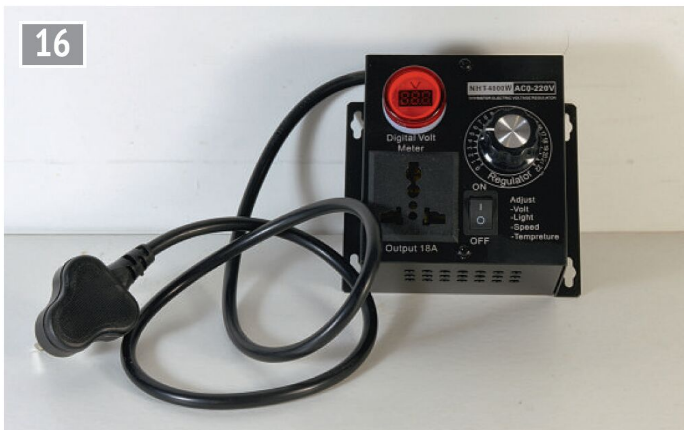
The boiler voltage control unit.
