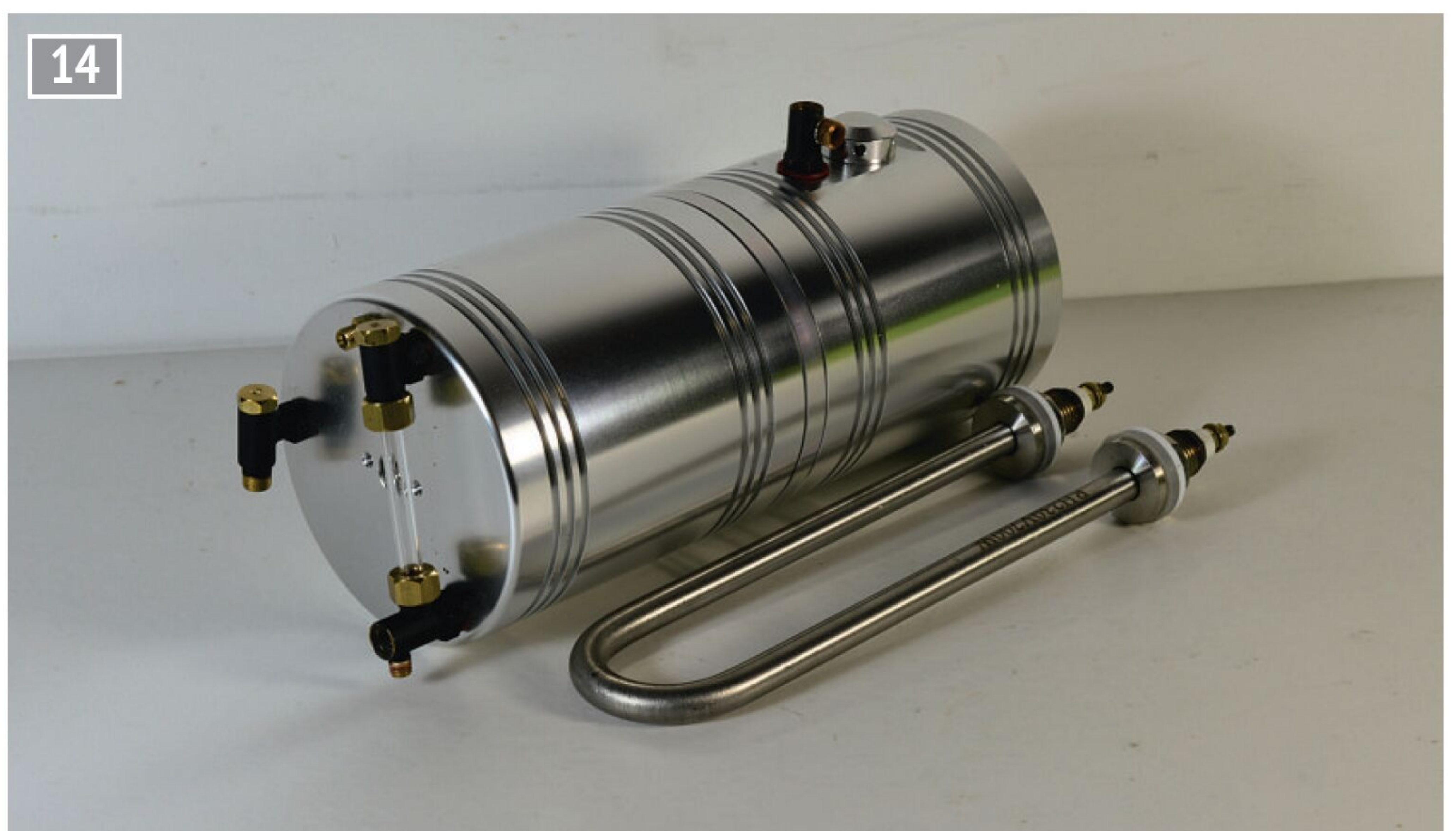
The boiler shell and heating element.
