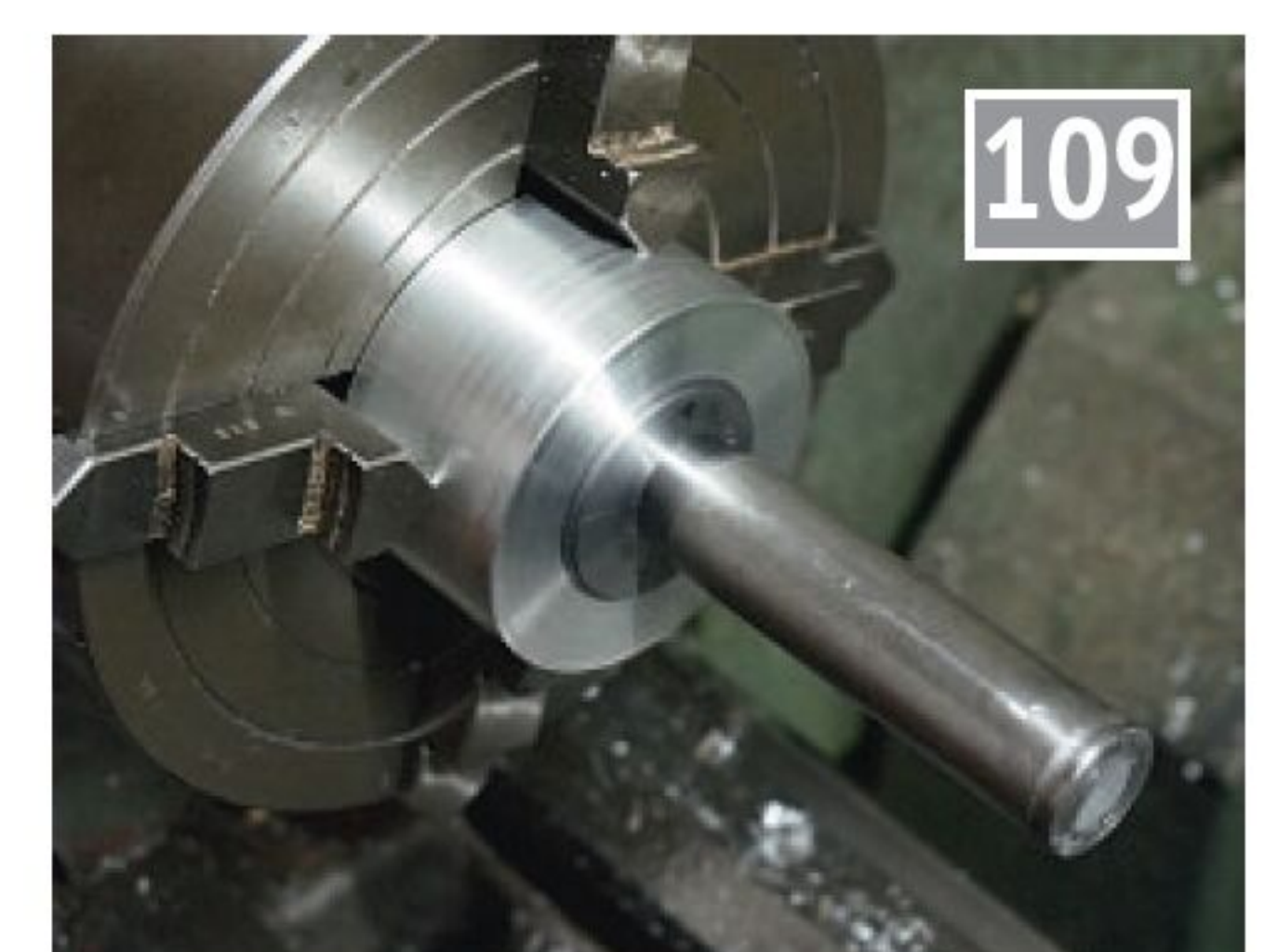
Plug gauges had been made when the crankshaft was turned.
