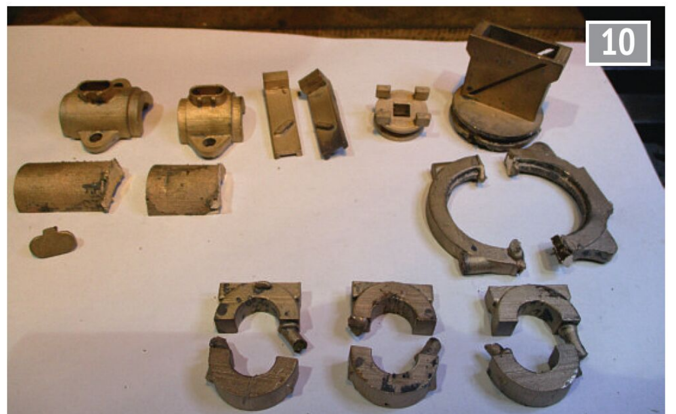
The results of the 'lost plastic' process.
