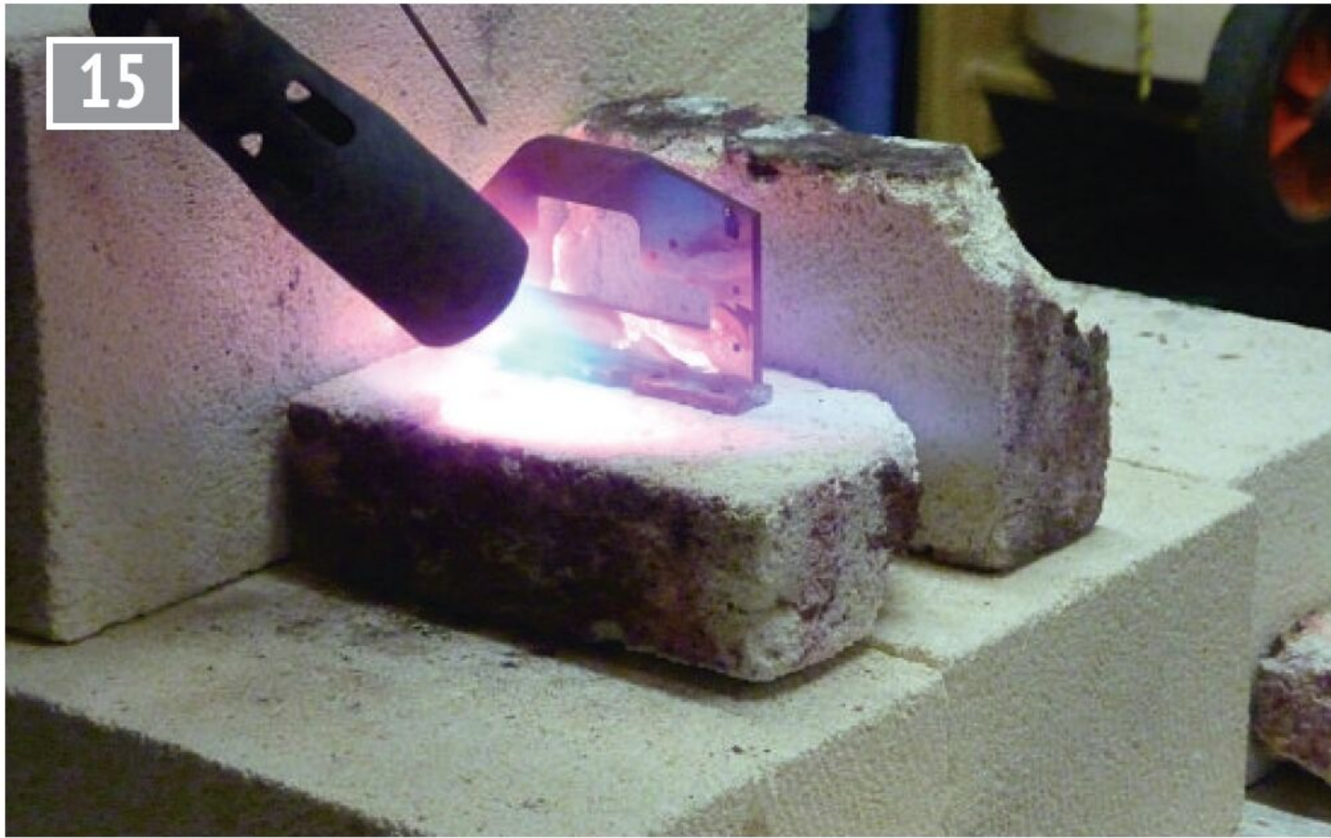
Brazing the motion bracket.
