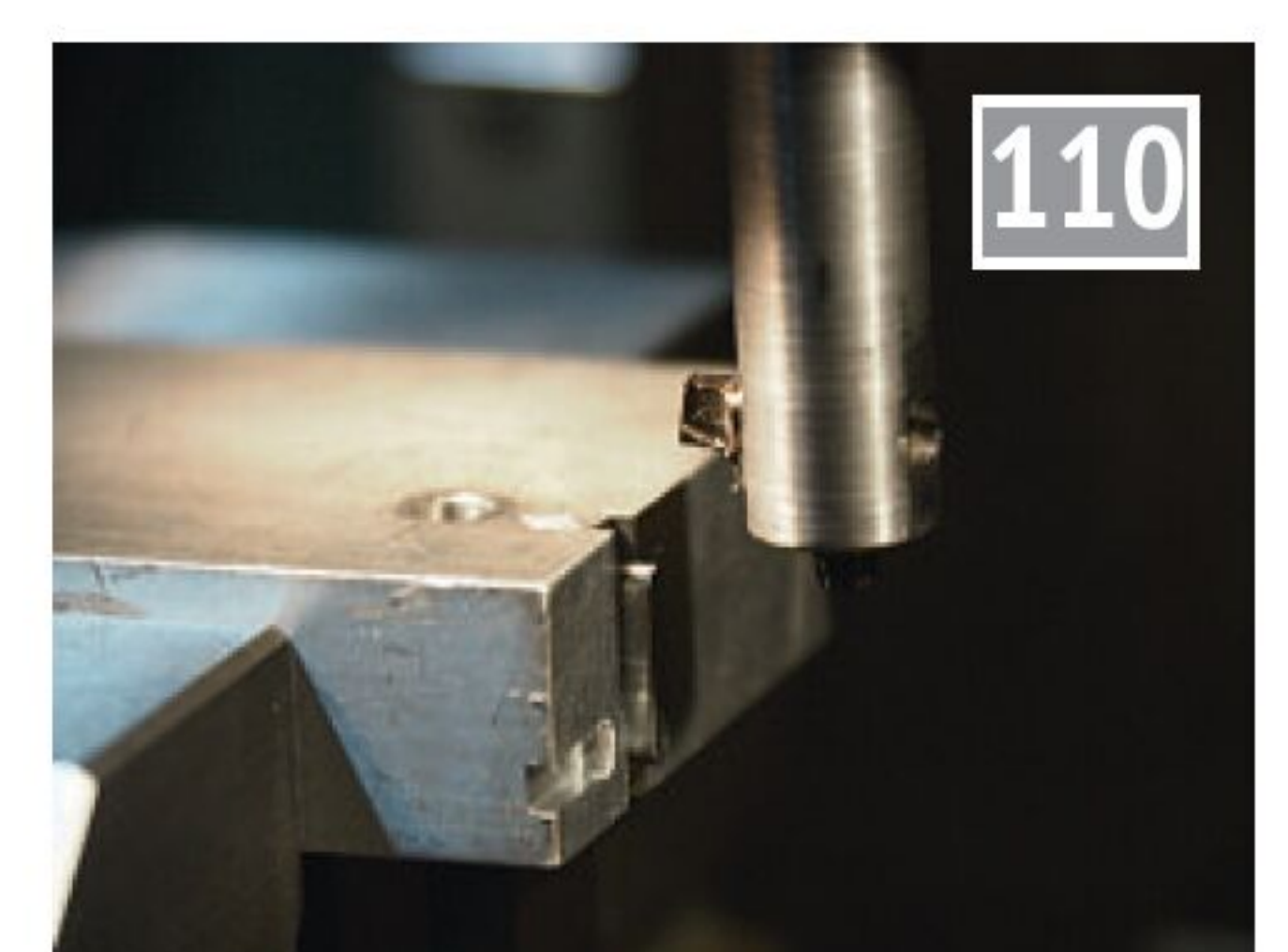
Test cut with the slotting tool for the eccentric keyways. The key is a light push fit.
