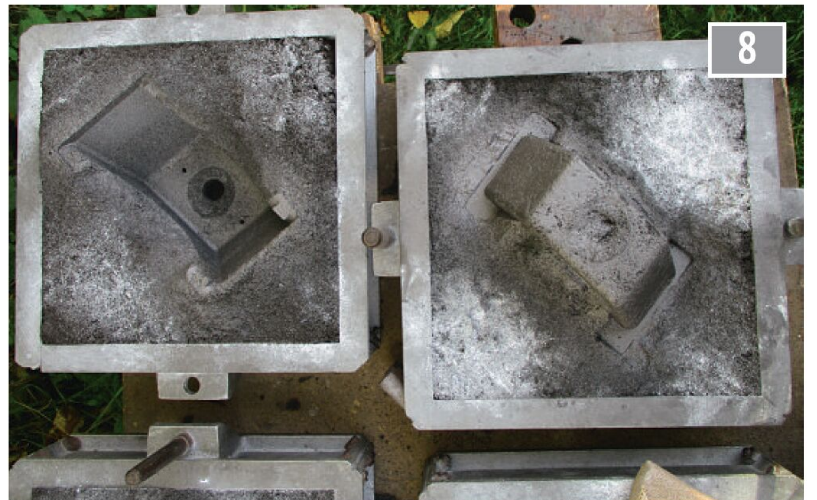
Ready for pouring the upper section.
