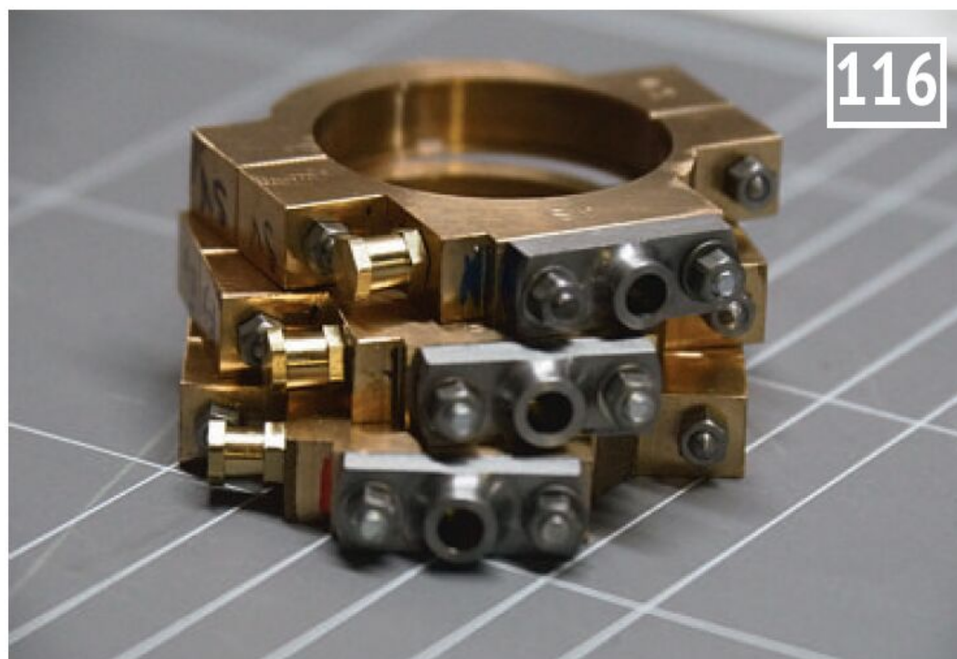
The three assemblies with studs and dummy oil pots fitted. All parts have been letter-stamped to prevent future errors.
