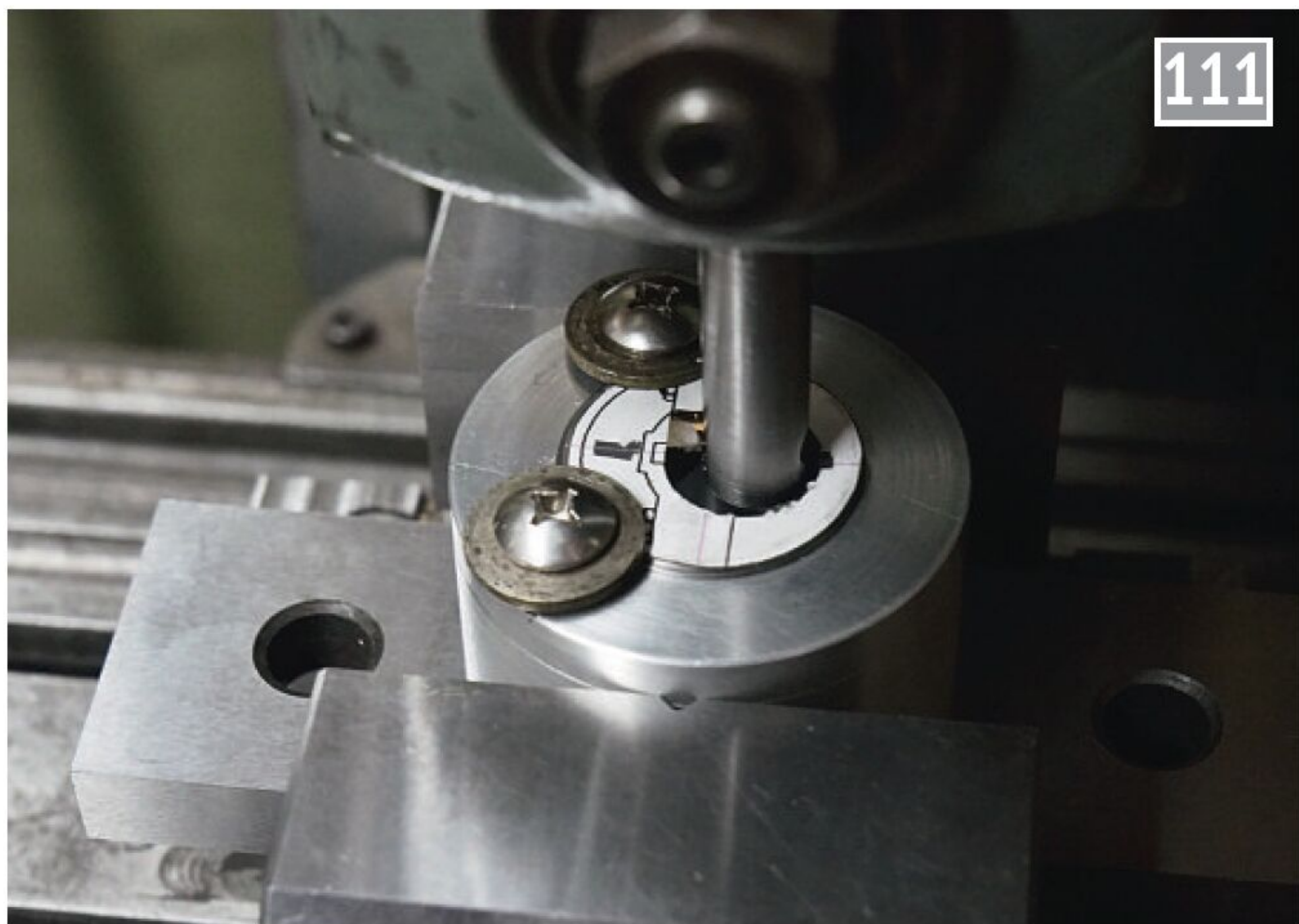
Two screws were added to the pot chuck to hold down the eccentrics. The slotting tool was aligned by measurement; the paper guide is a sanity check.
