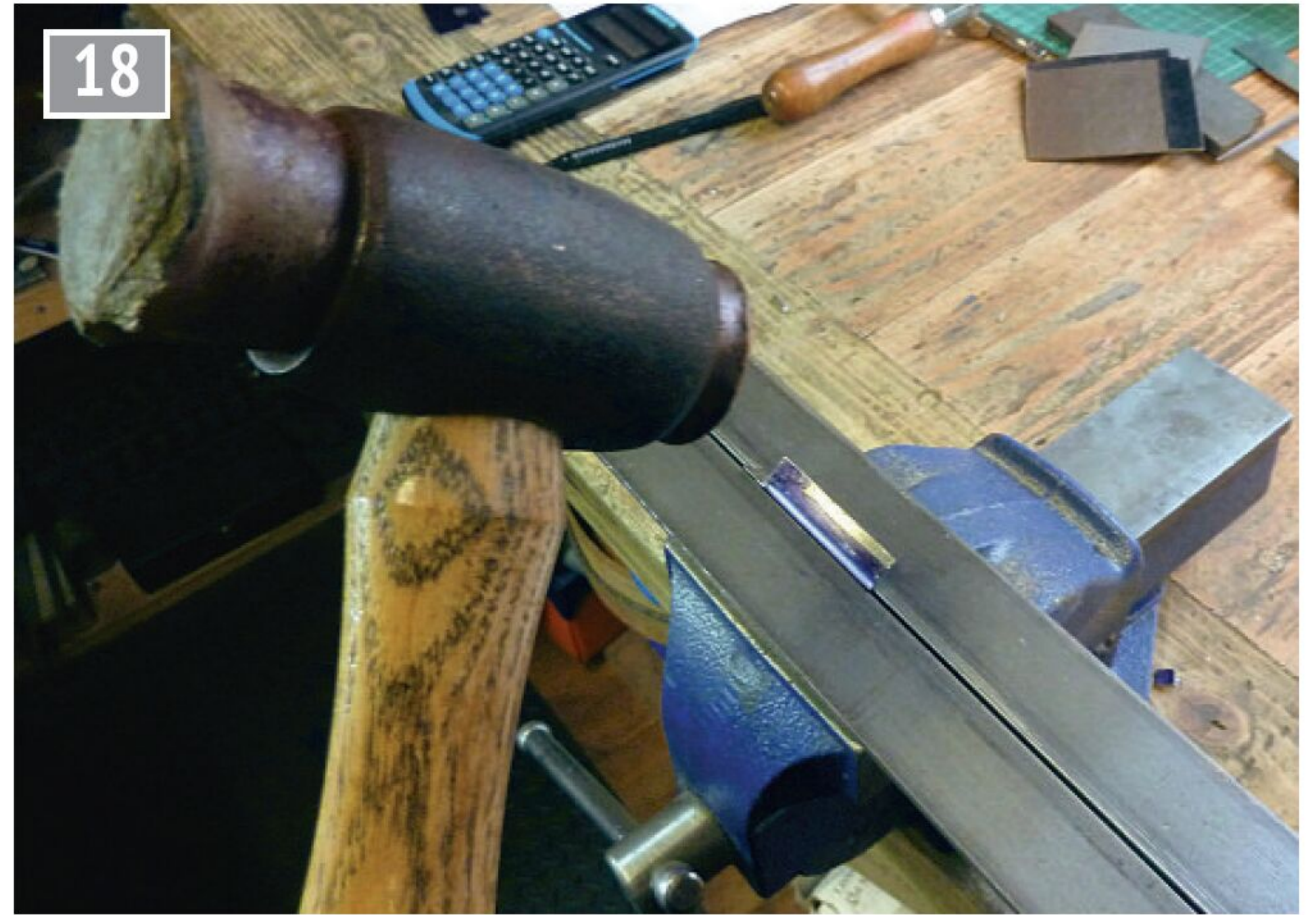
Knocking over a footplate bracket.
