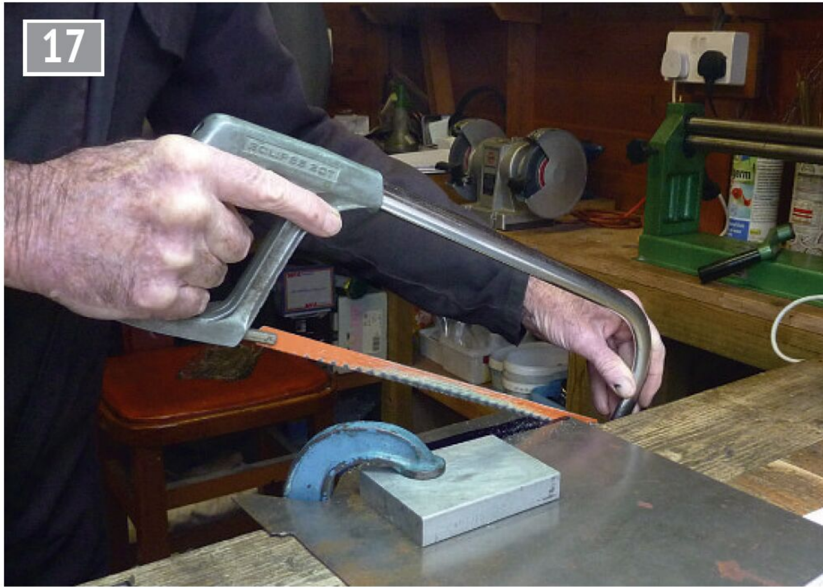
Cutting sheet metal on the bench.
