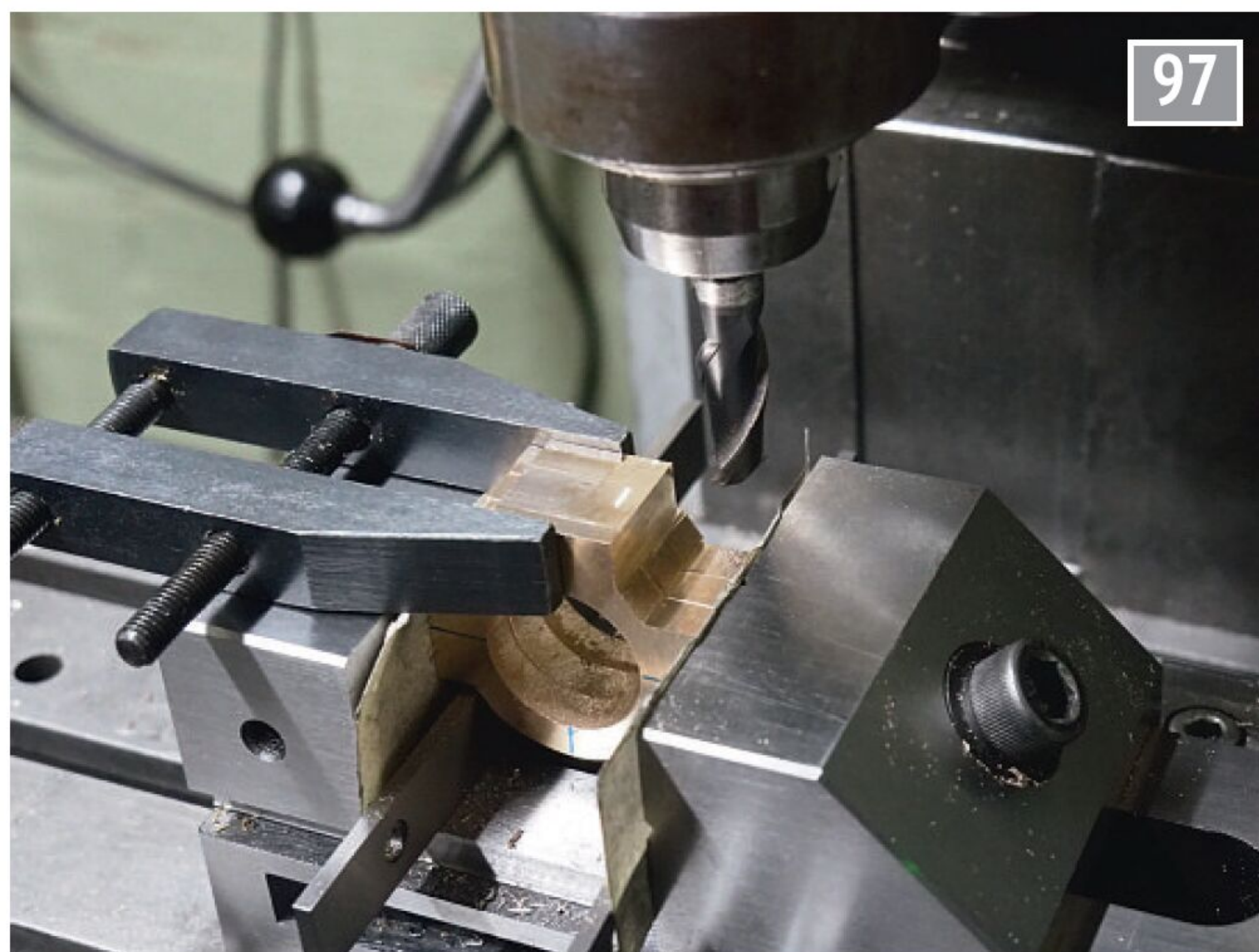
Milling the attachments for the eccentric rods.
