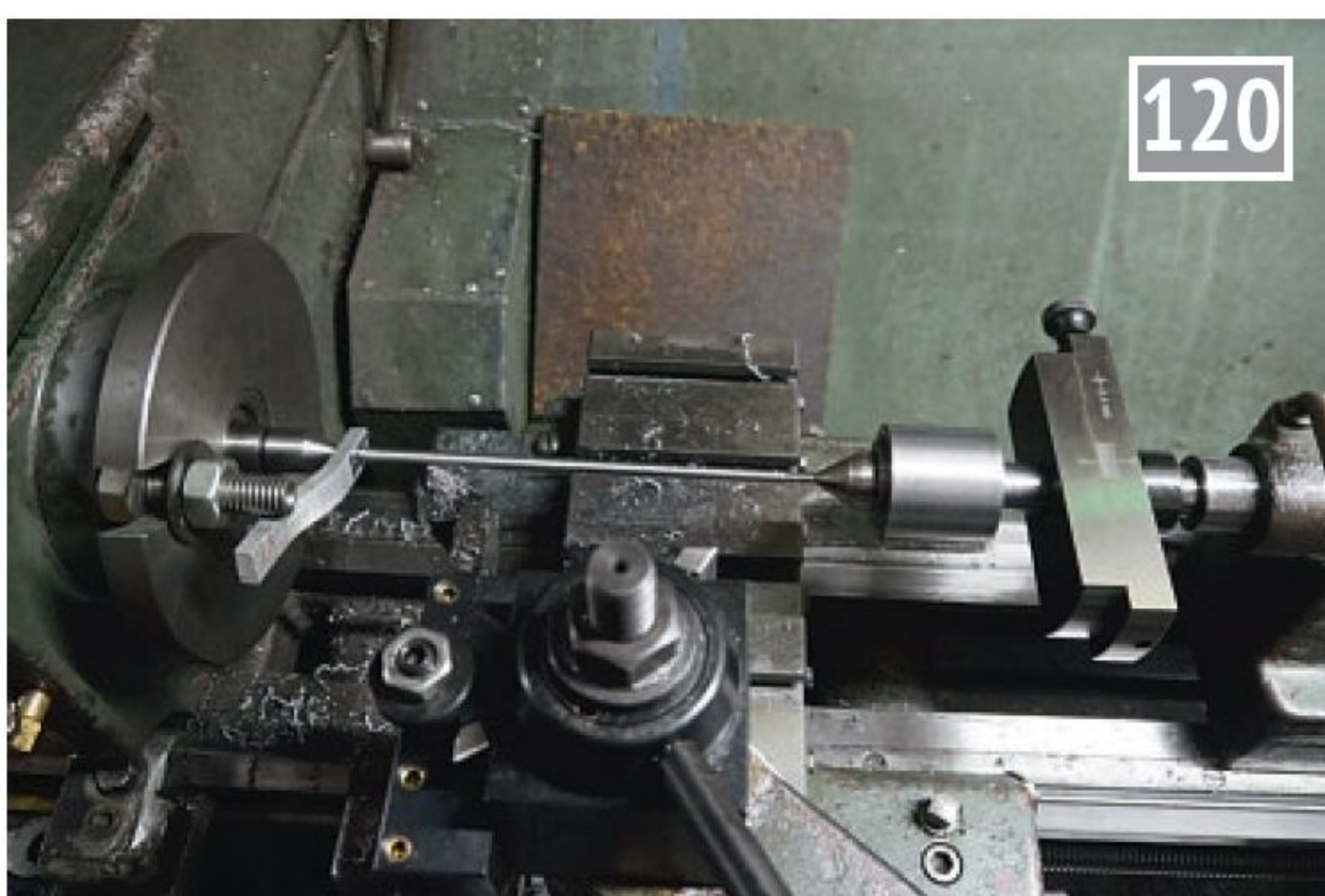
The taper on the three eccentric rods was achieved using a set-over tailstock.
