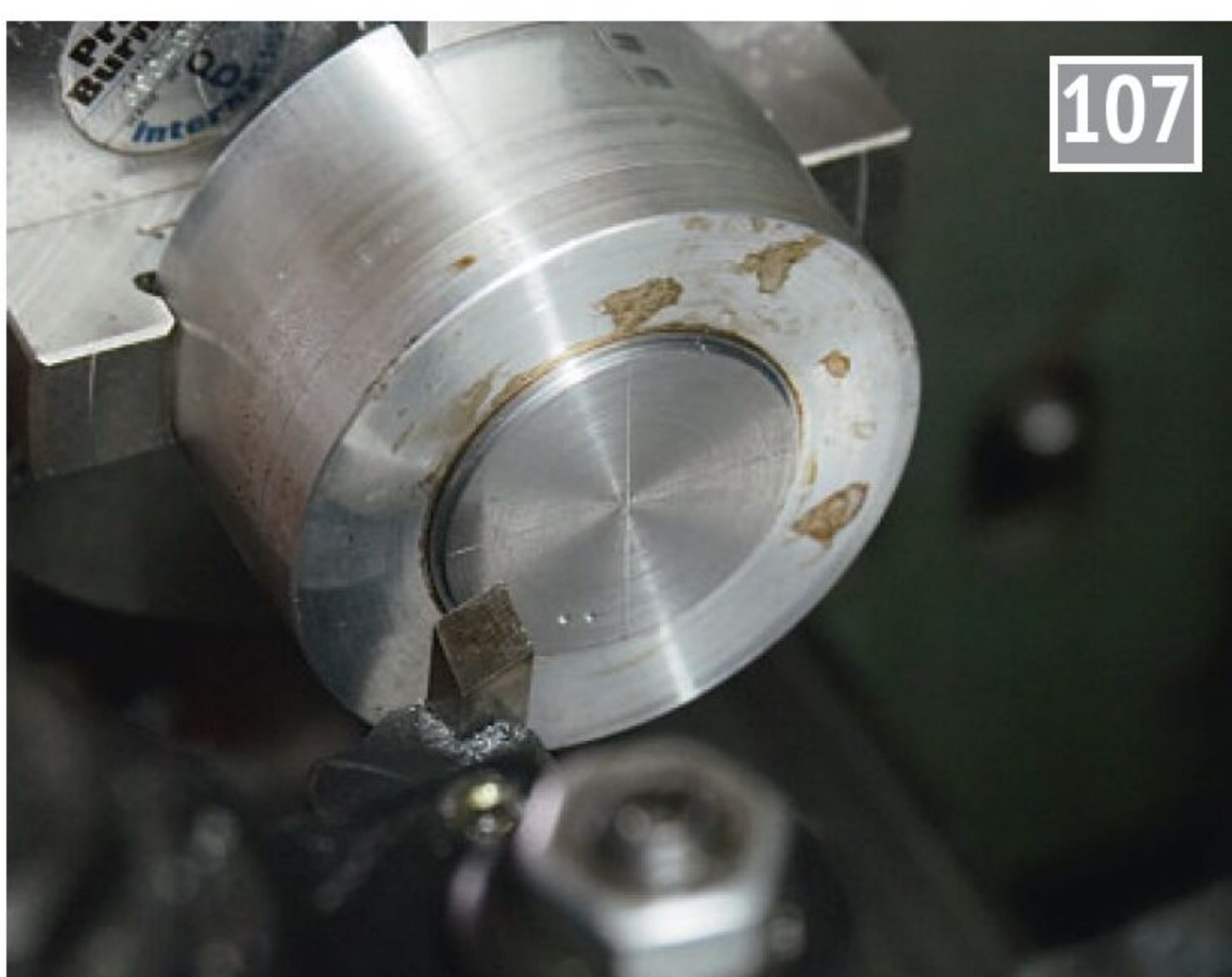
...but cyanoacrylate worked very much better for gripping the eccentrics for marking in the centre lines. Note that the chuck is a self-centring four-jaw, and also the identifying centre dots.
