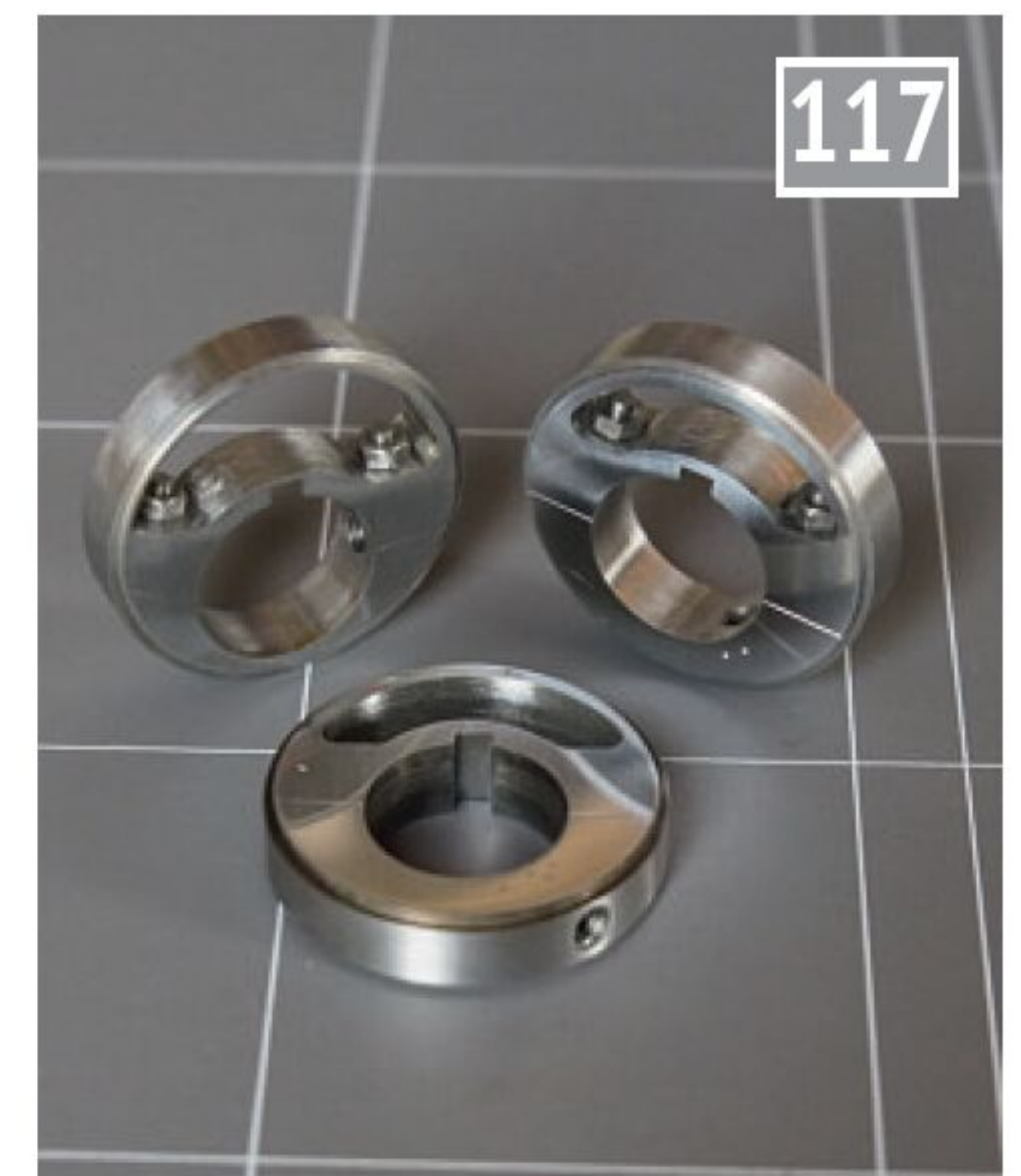
In actual use the eccentrics stay in place on the crankshaft by friction but there was room for grub screws just to make sure.
