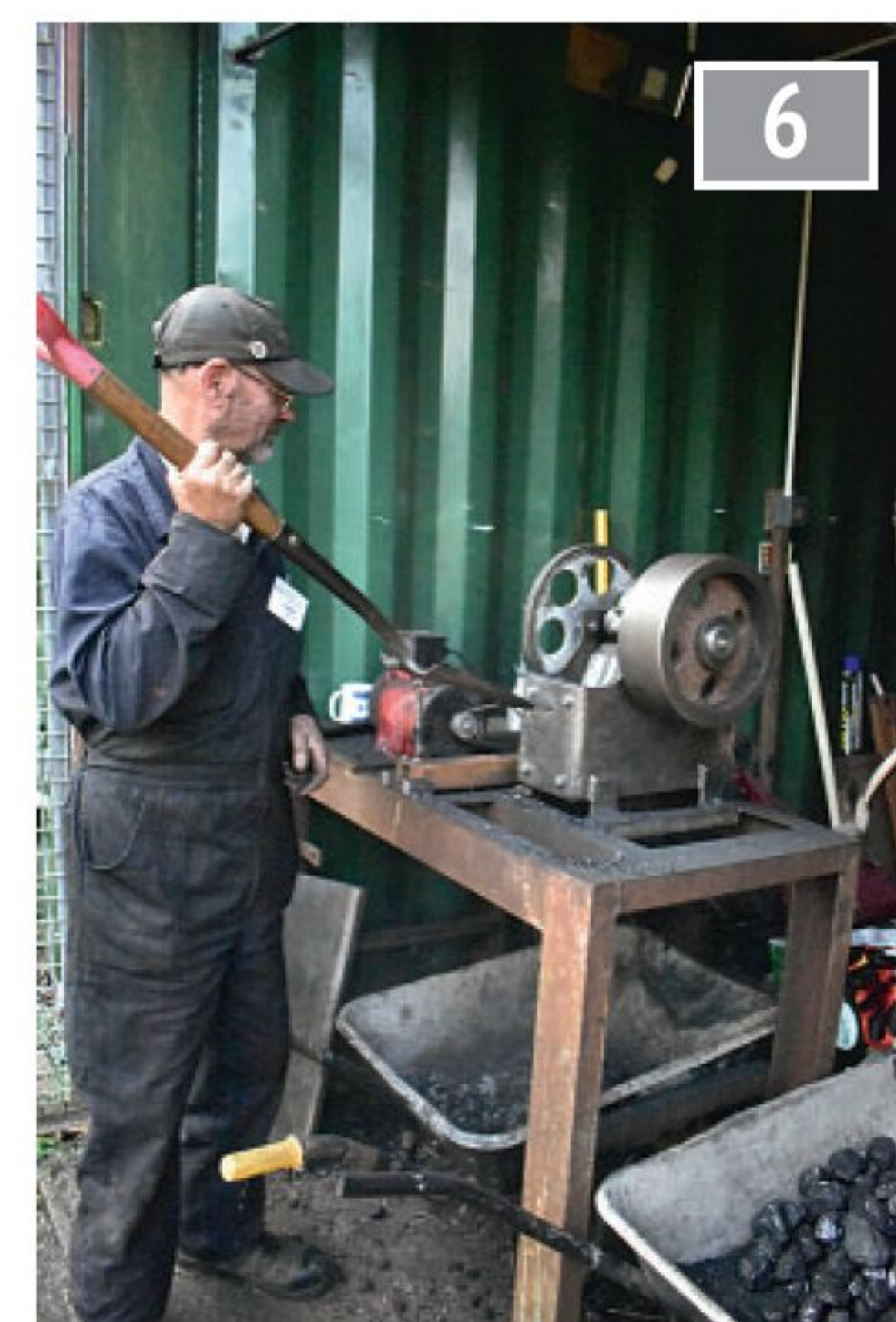
Phil Hancock built the coal crusher to do its job during the weekend.
