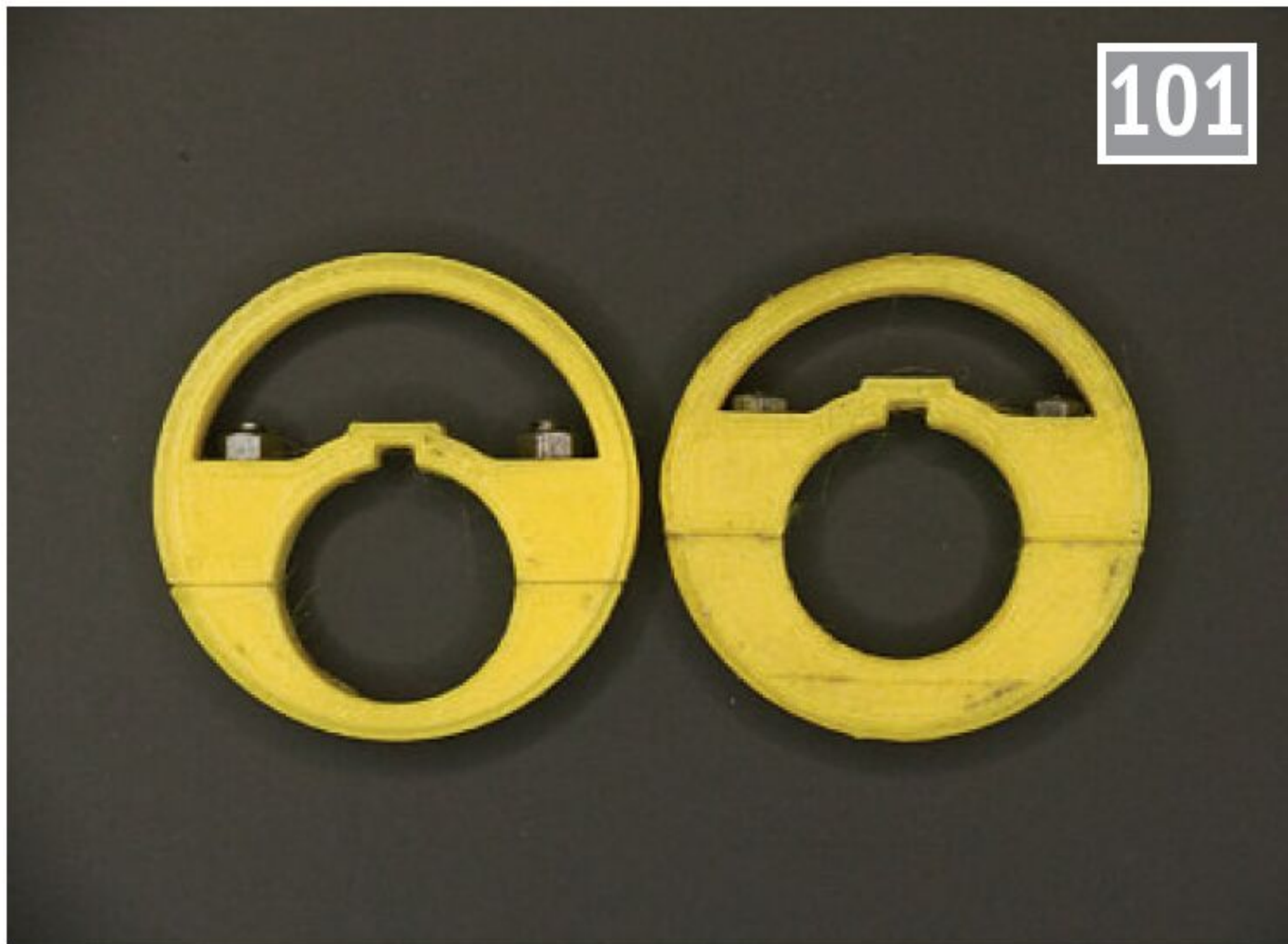
3D prints of eccentrics to the original design. Getting a spanner on the nuts was going to vary from very difficult to impossible.
