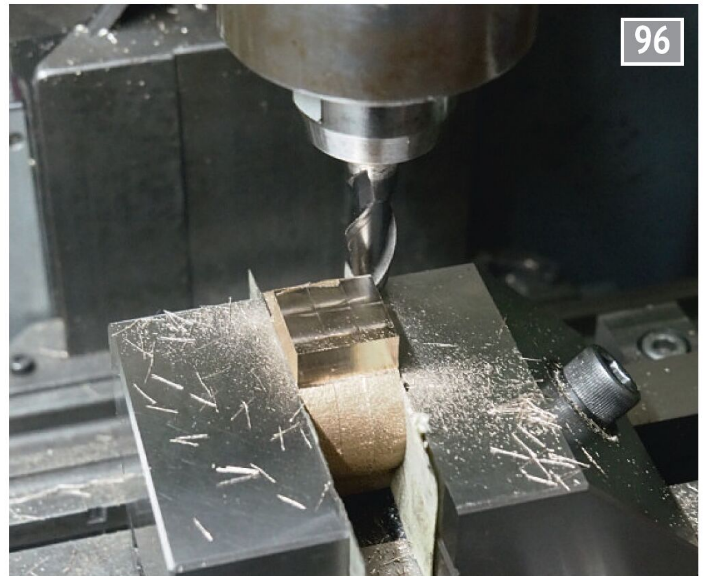
Cleaning up the edges of the clamping bolt bosses.
