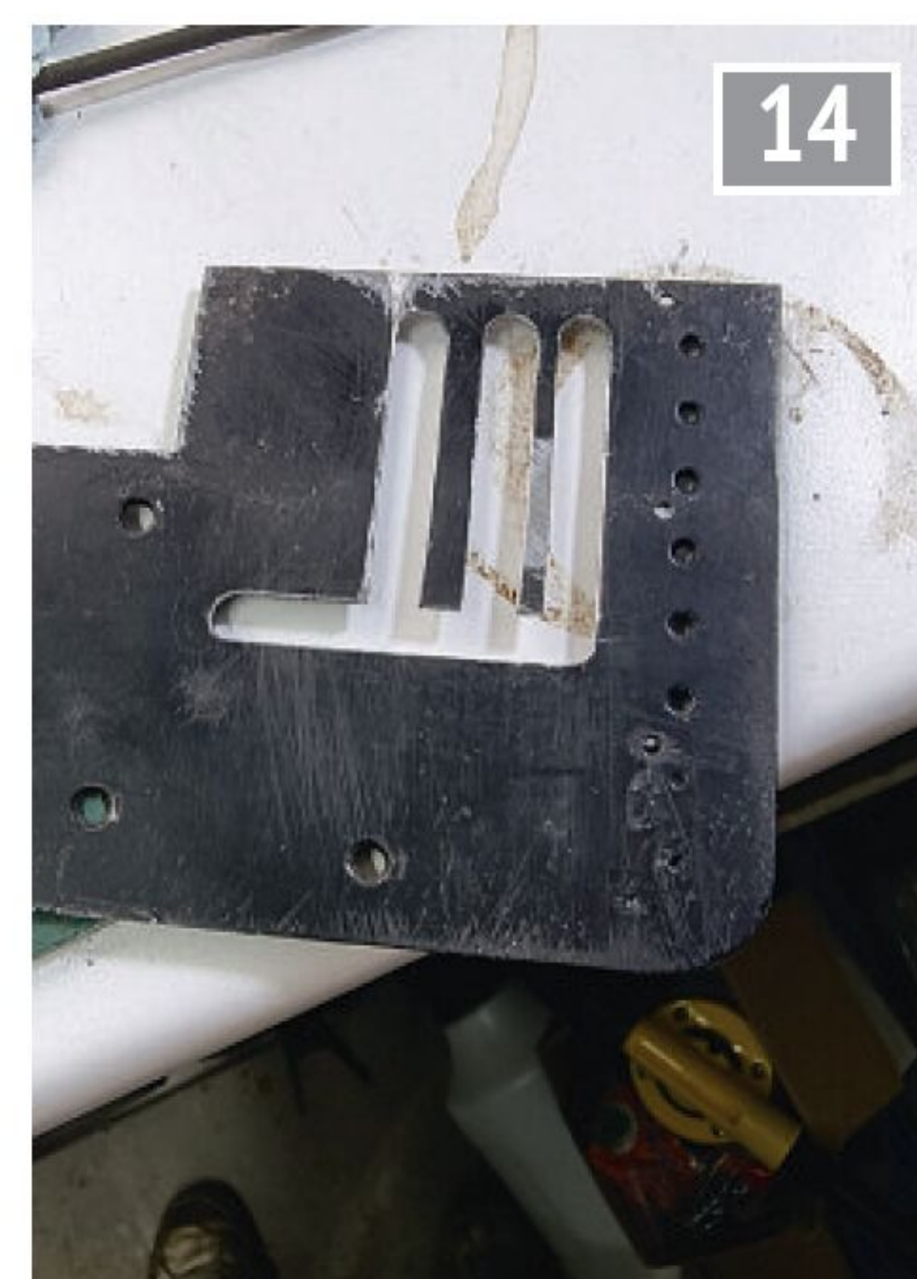
Clearance slots in the cab floor.
