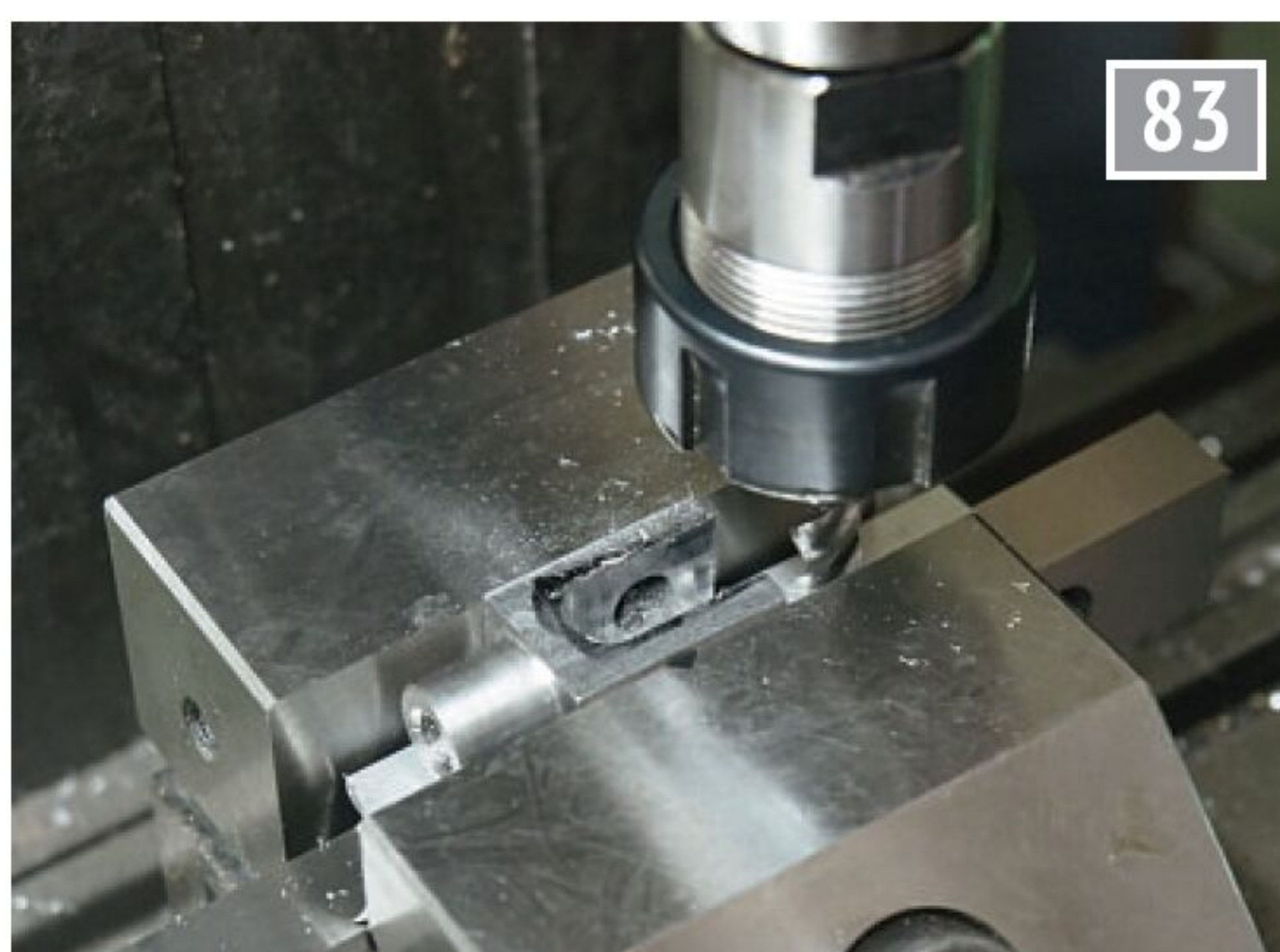
Starting the slot in the crosshead for the connecting rod ...
