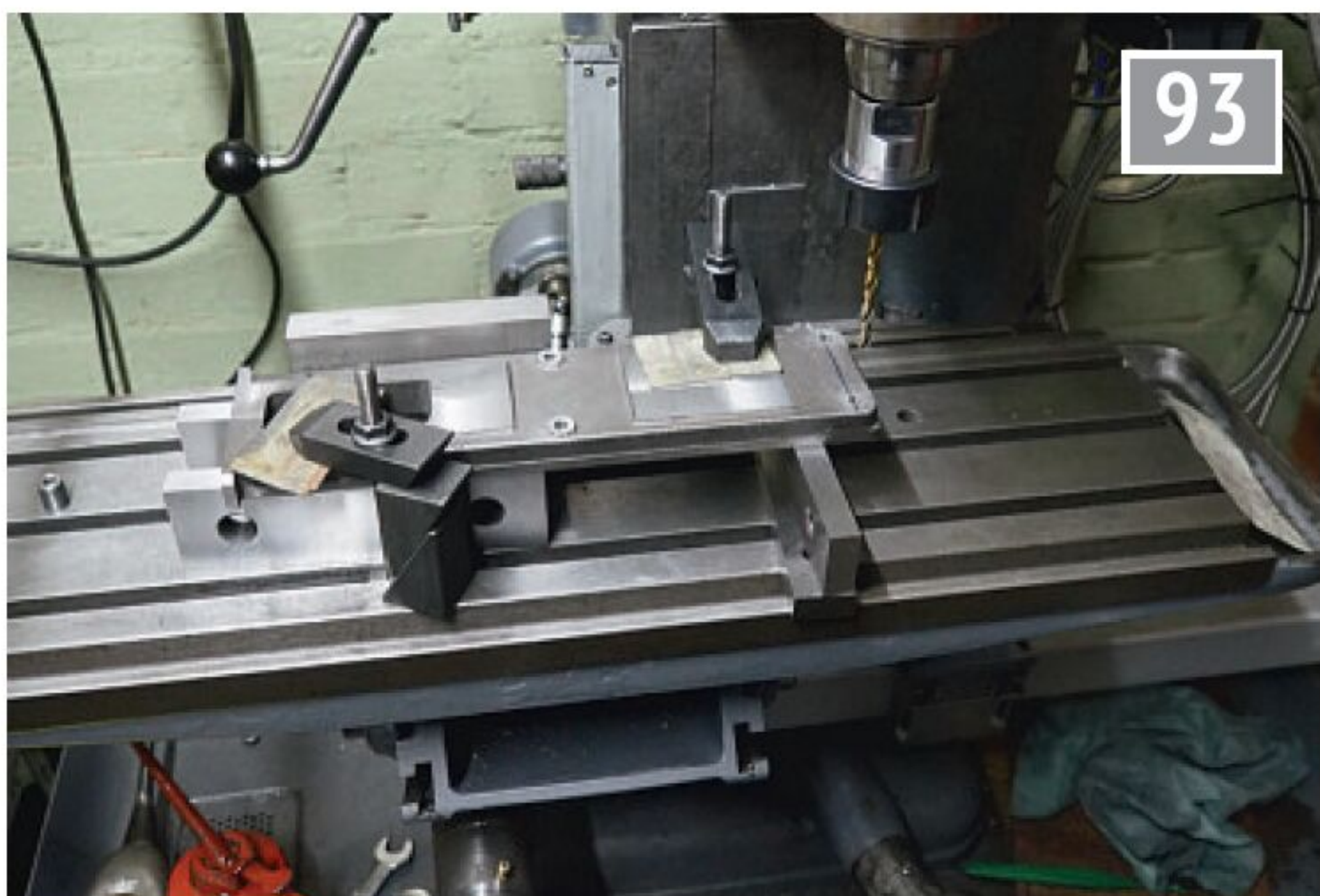
93 Two of the bosses for foundation stud nuts were missing from the casting. Holes were drilled in appropriate places and ...
