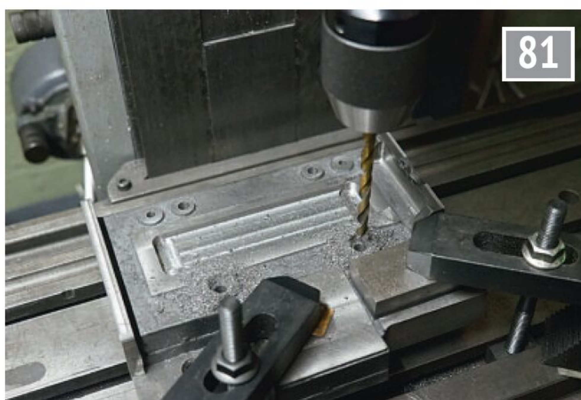
The casting was aligned with the mill axes, the datum surfaces located and the DRO axes set to zero at these. Holes for the foundation bolts and for the handrail stanchions were drilled by coordinates.
