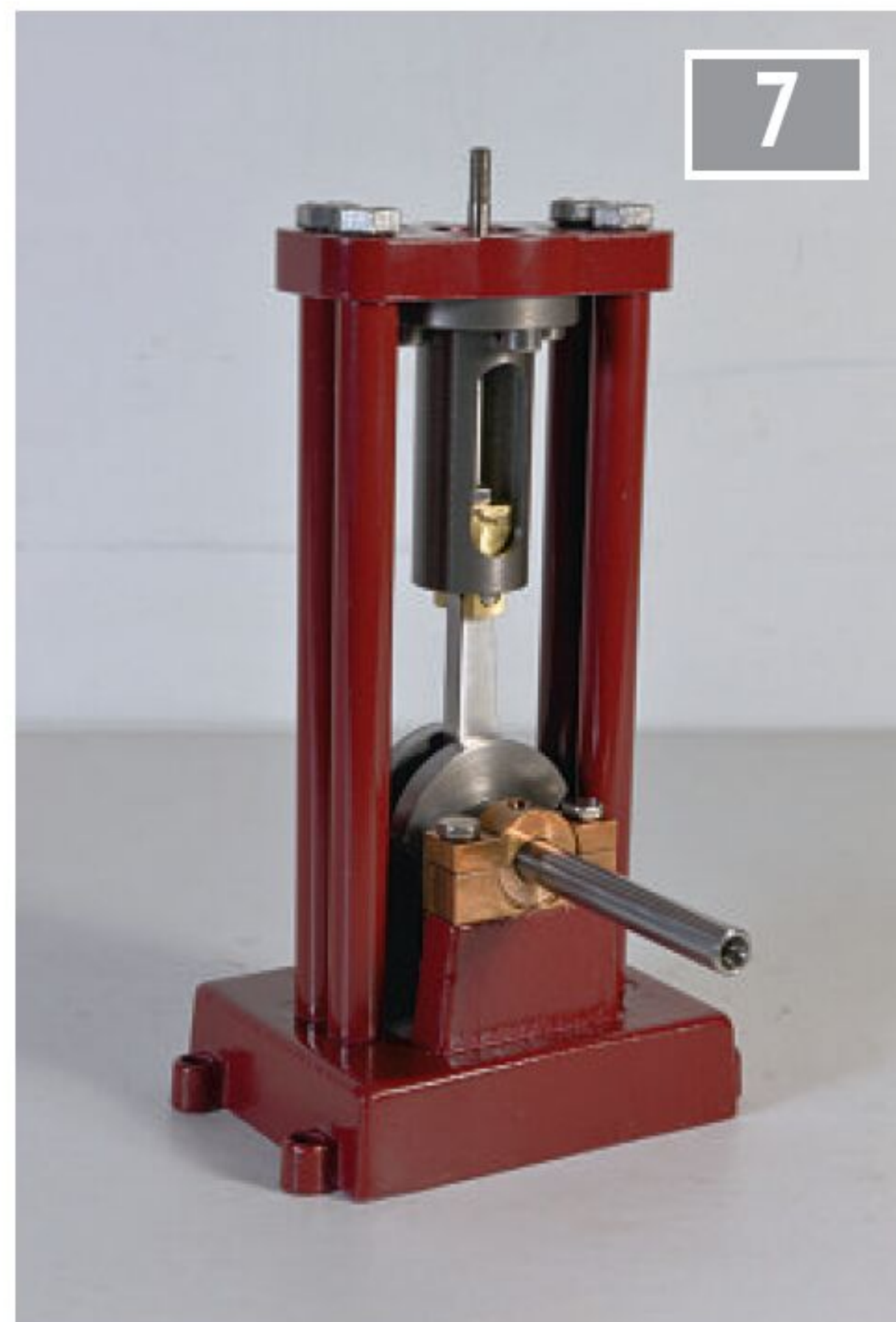
The crosshead guide is fitted.
