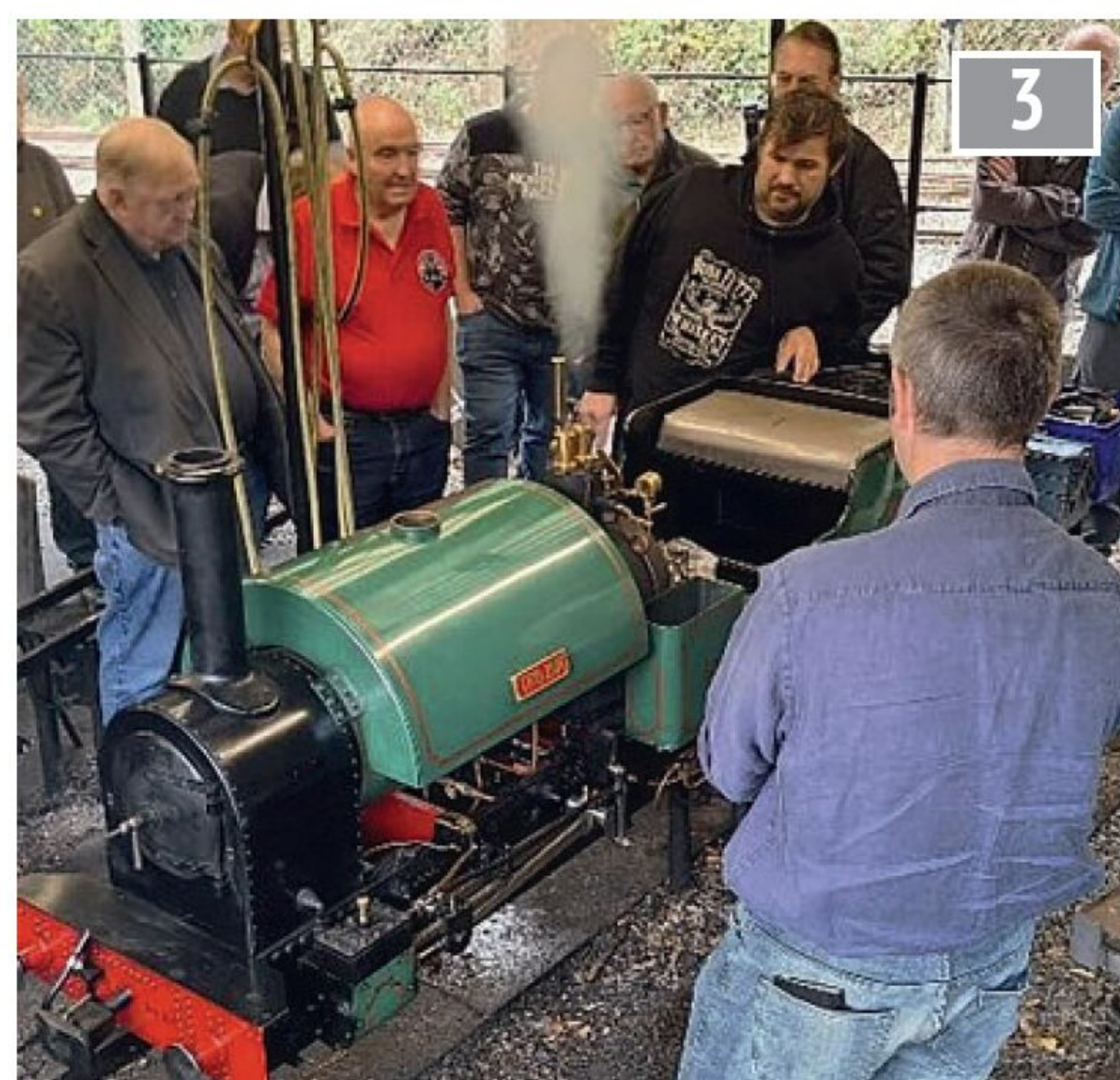
Undergoing a steam test.
