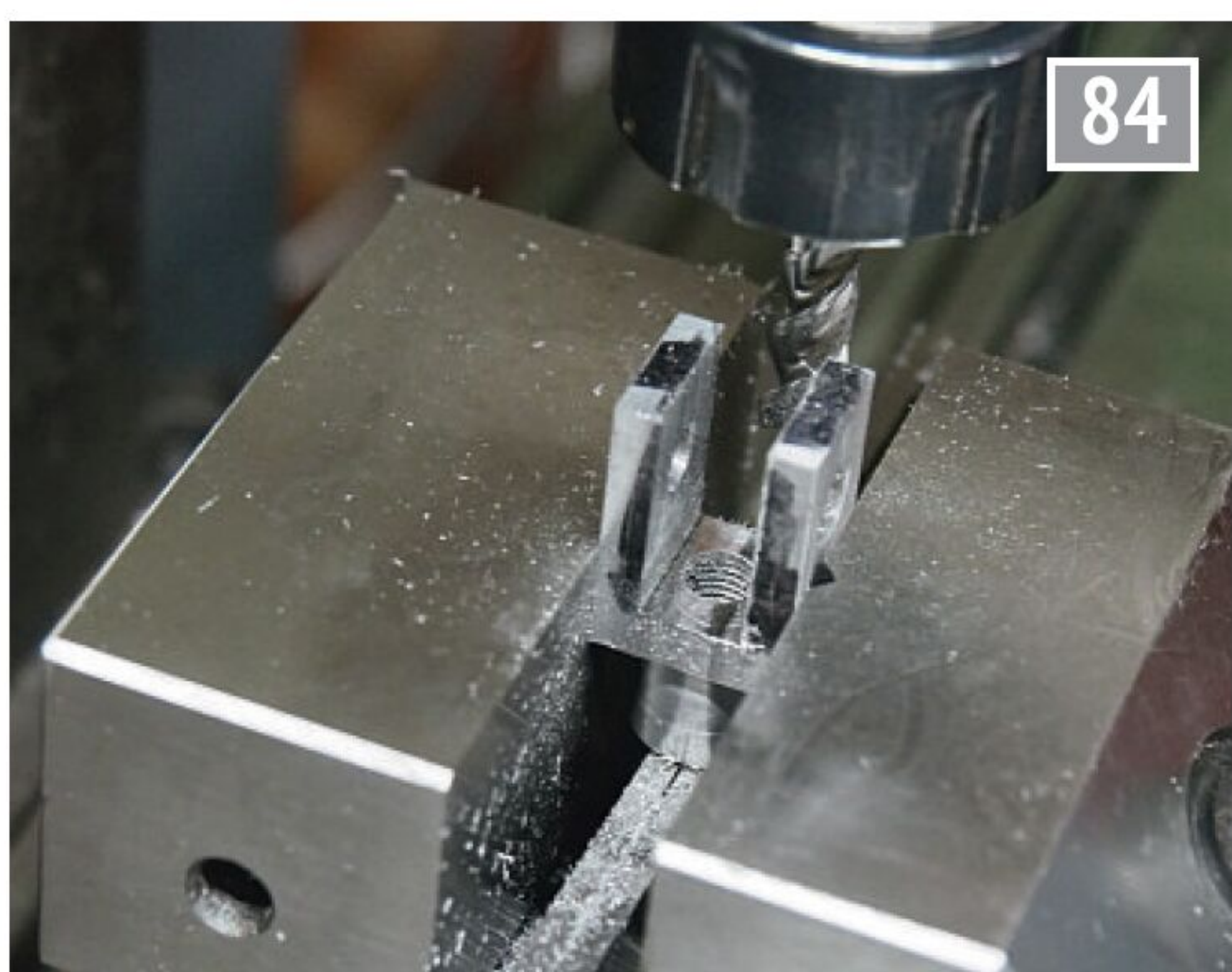
... which is then turned through 90 degrees to square off the end.
