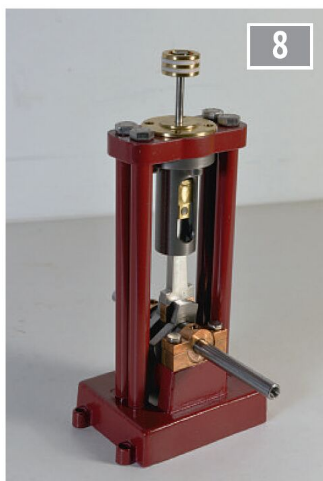
The cylinder end cover and piston are added...
