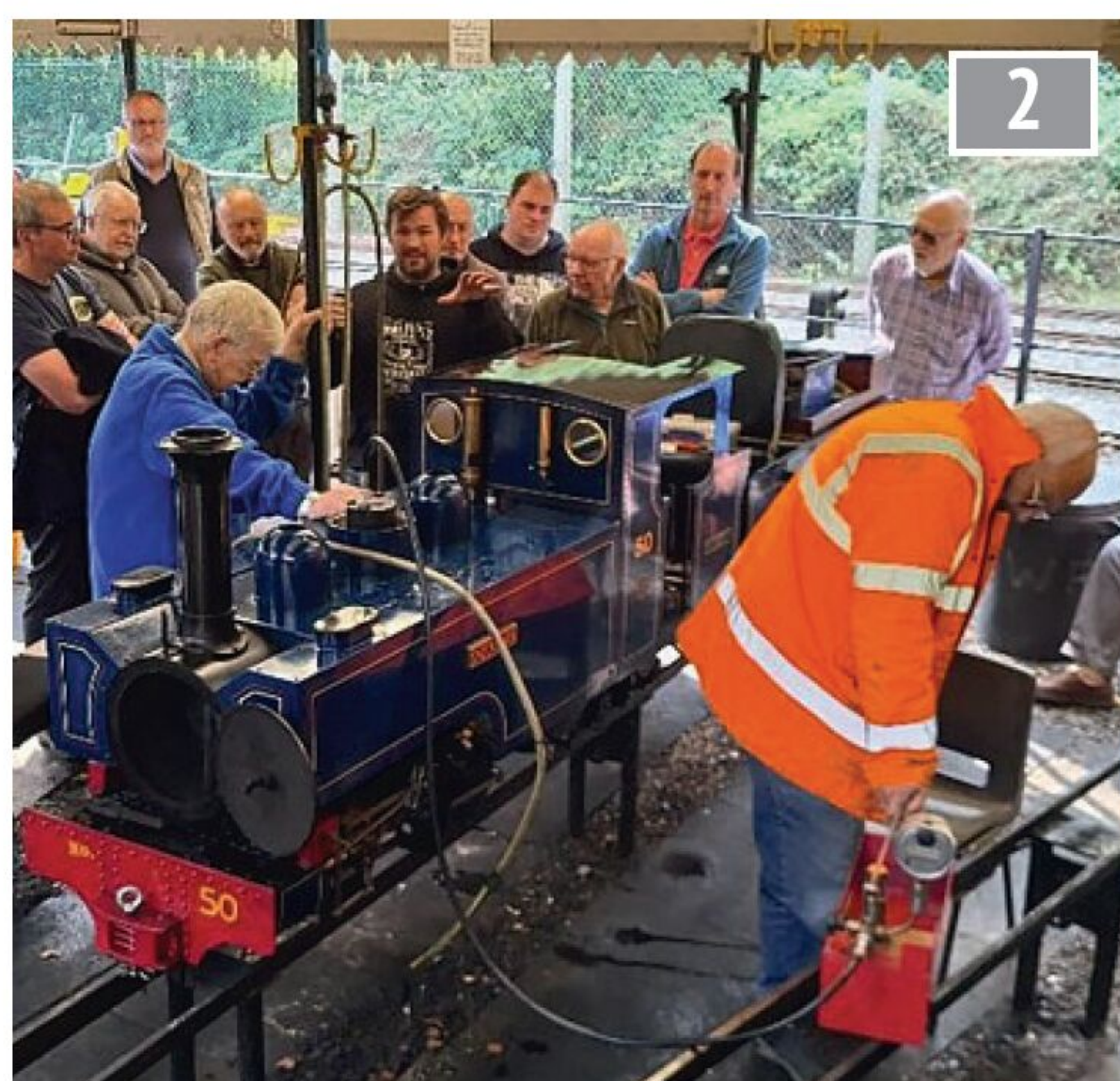
Ben Pavier demonstrates hydraulic testing.
