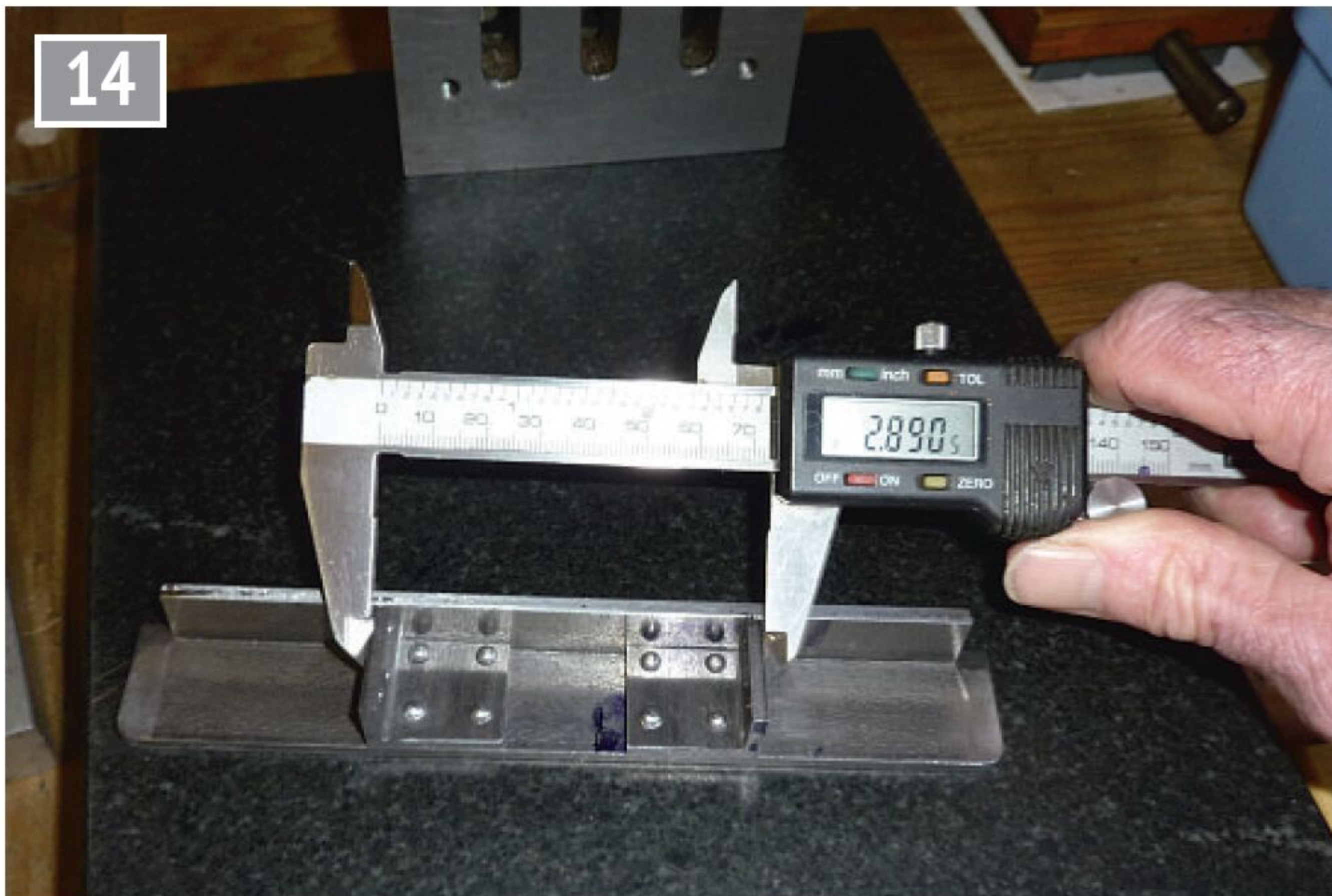
Rivets done - angles dimension near enough right.
