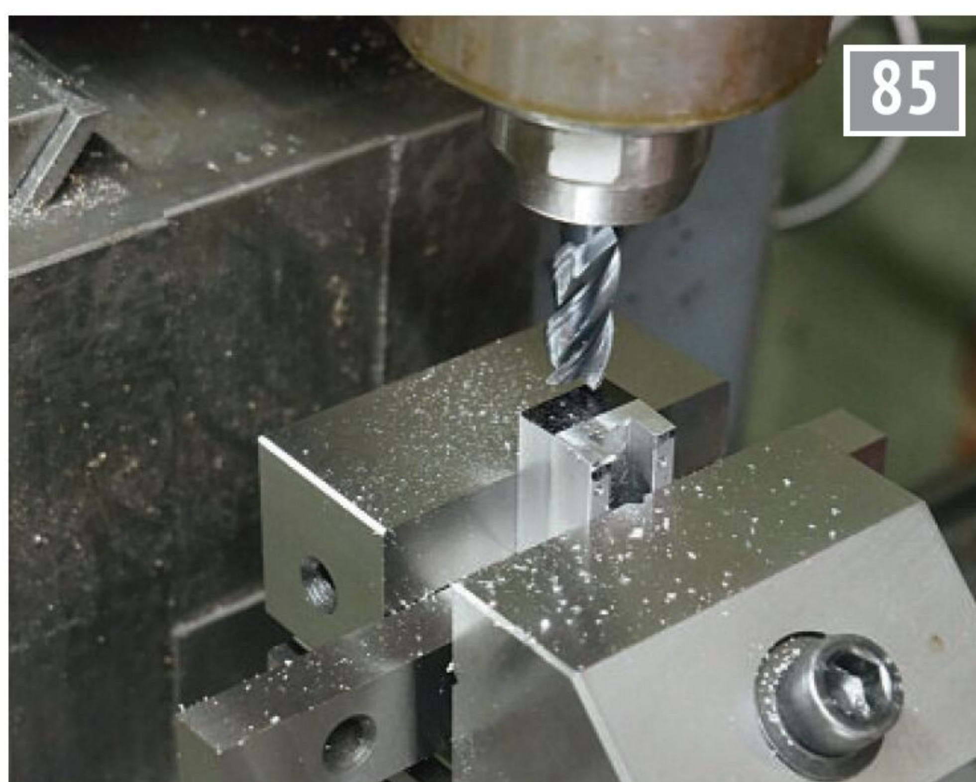
For the sake of appearance only the slipper has angled ends. Here the part is set up in a sine vice with the end coated with marker pen to show where the cut has reached.
