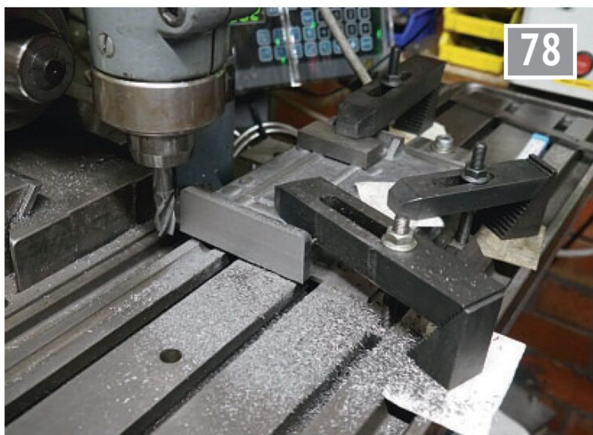
... and the crankshaft end and outside edge (not visible) of the casting milled flat. These surfaces are the X and Y dimension datums.
