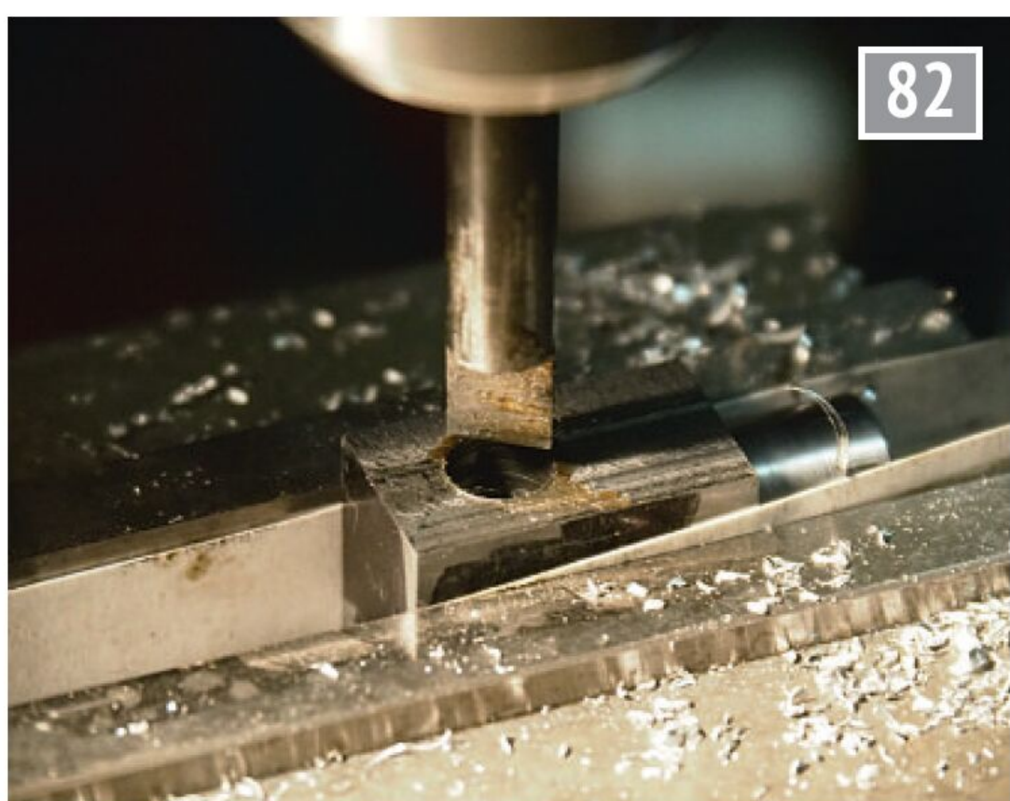
Counter boring the crosshead for the gudgeon pin.
