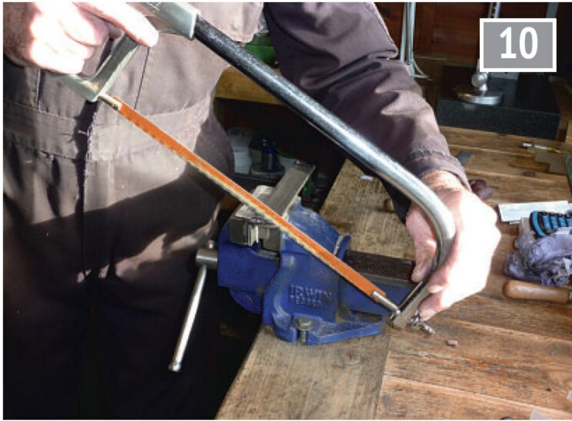
Hacksawing the buffer beam rebate.
