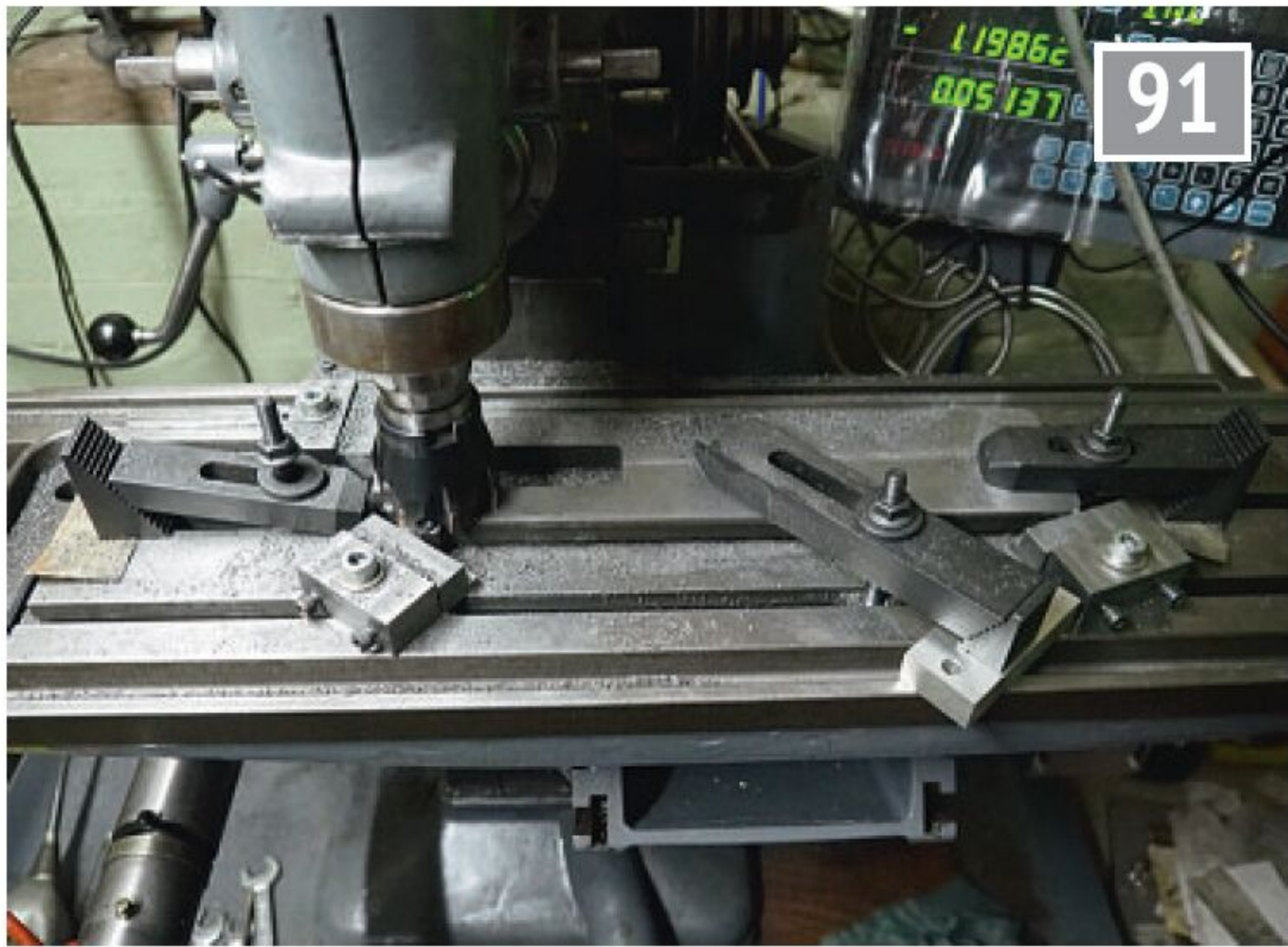
91 As with the slide the top projecting surfaces of the soleplate were filed to give stable clamping then the underside cleaned up. This required a lot of clamp juggling. Making a set of those low-profile clamps locating the corners of the casting is a very good idea.
