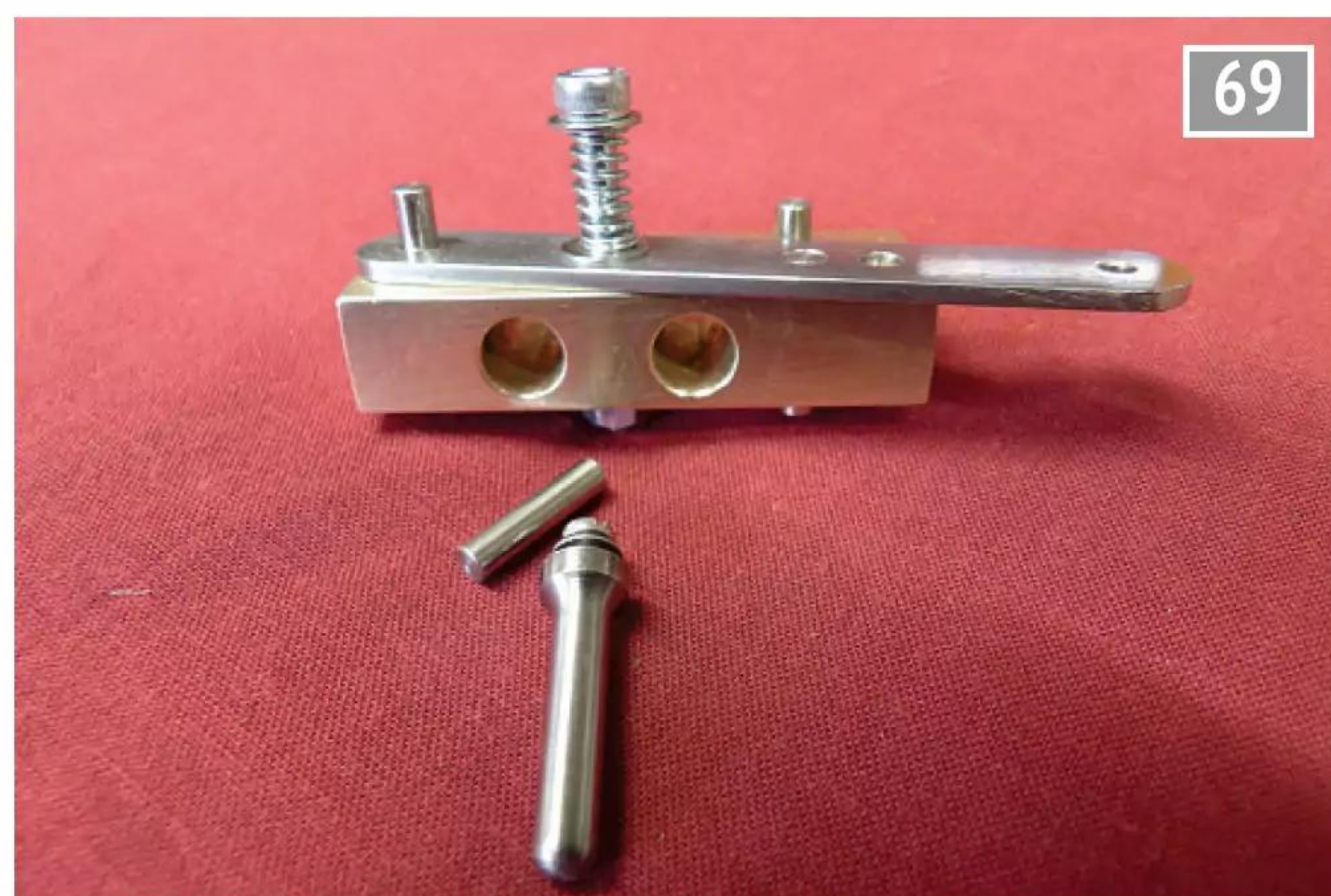
Forward/reverse control lever.
