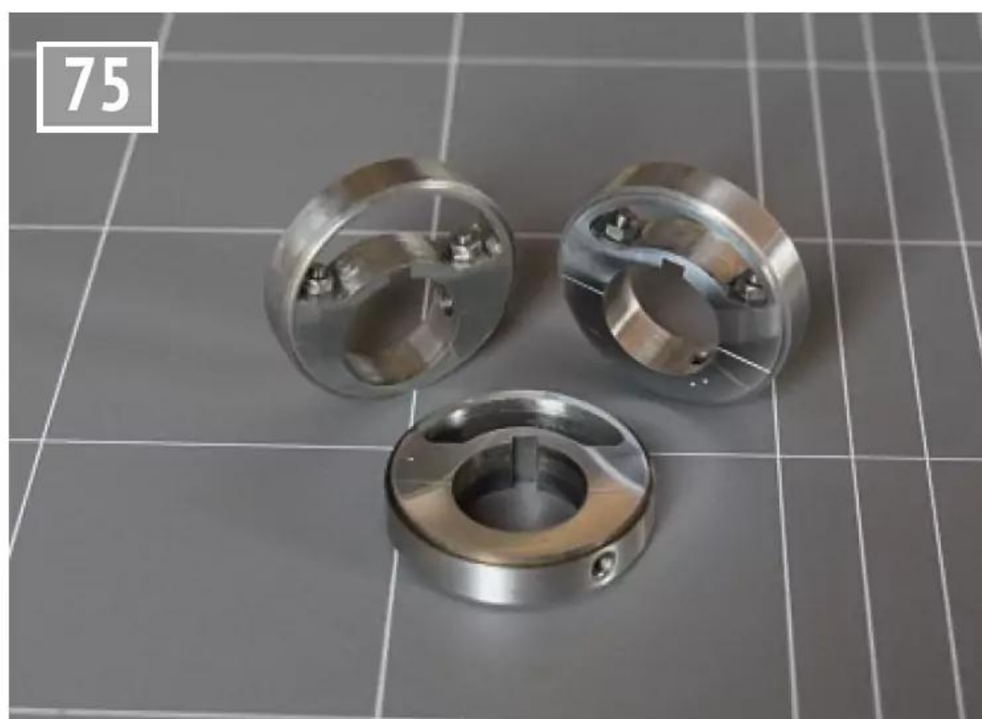
The marking out lines were polished out and the dummy joint line scribed in. The 'nuts and studs' are glued in dummies.
