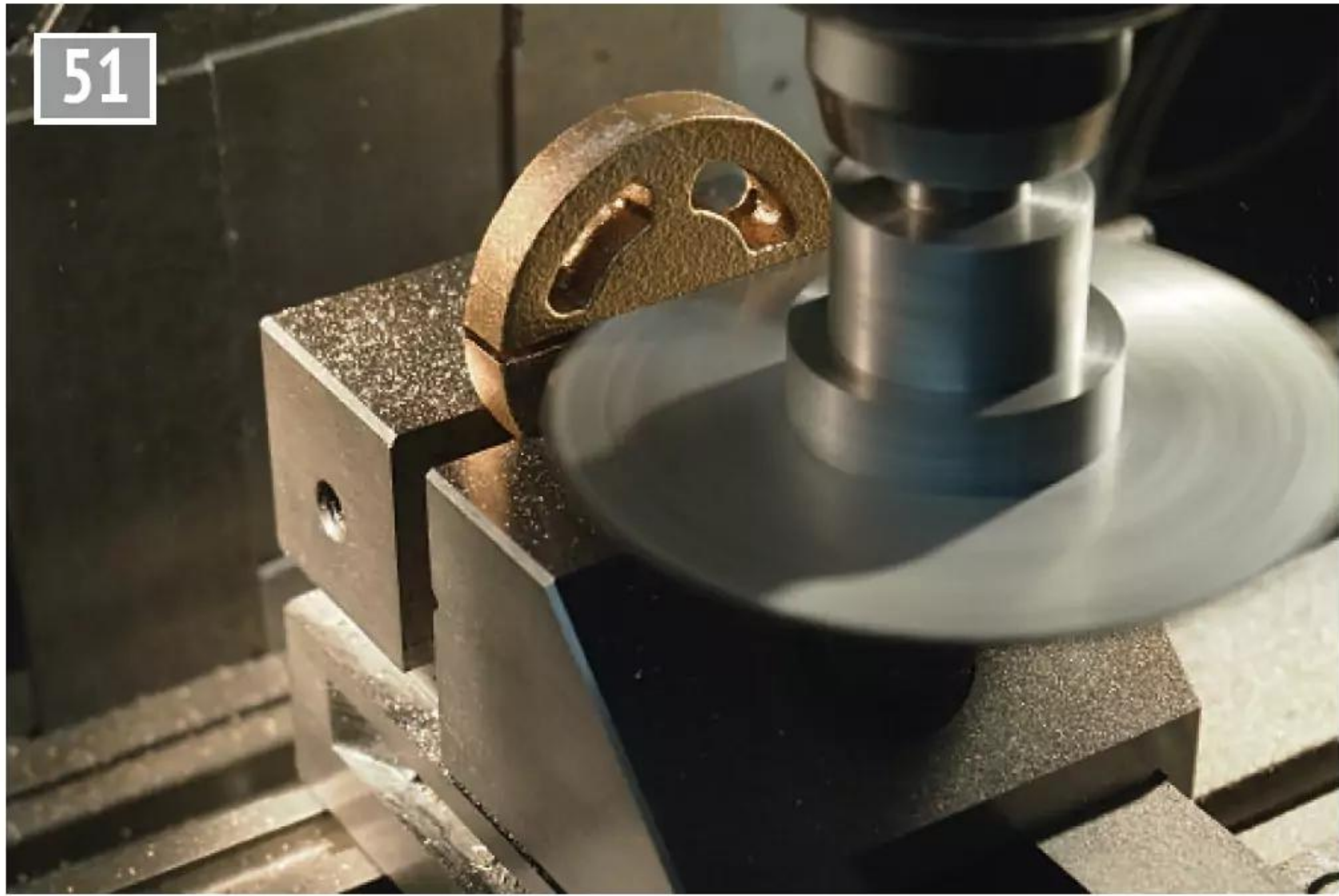
Separating the pulley casting halves.
