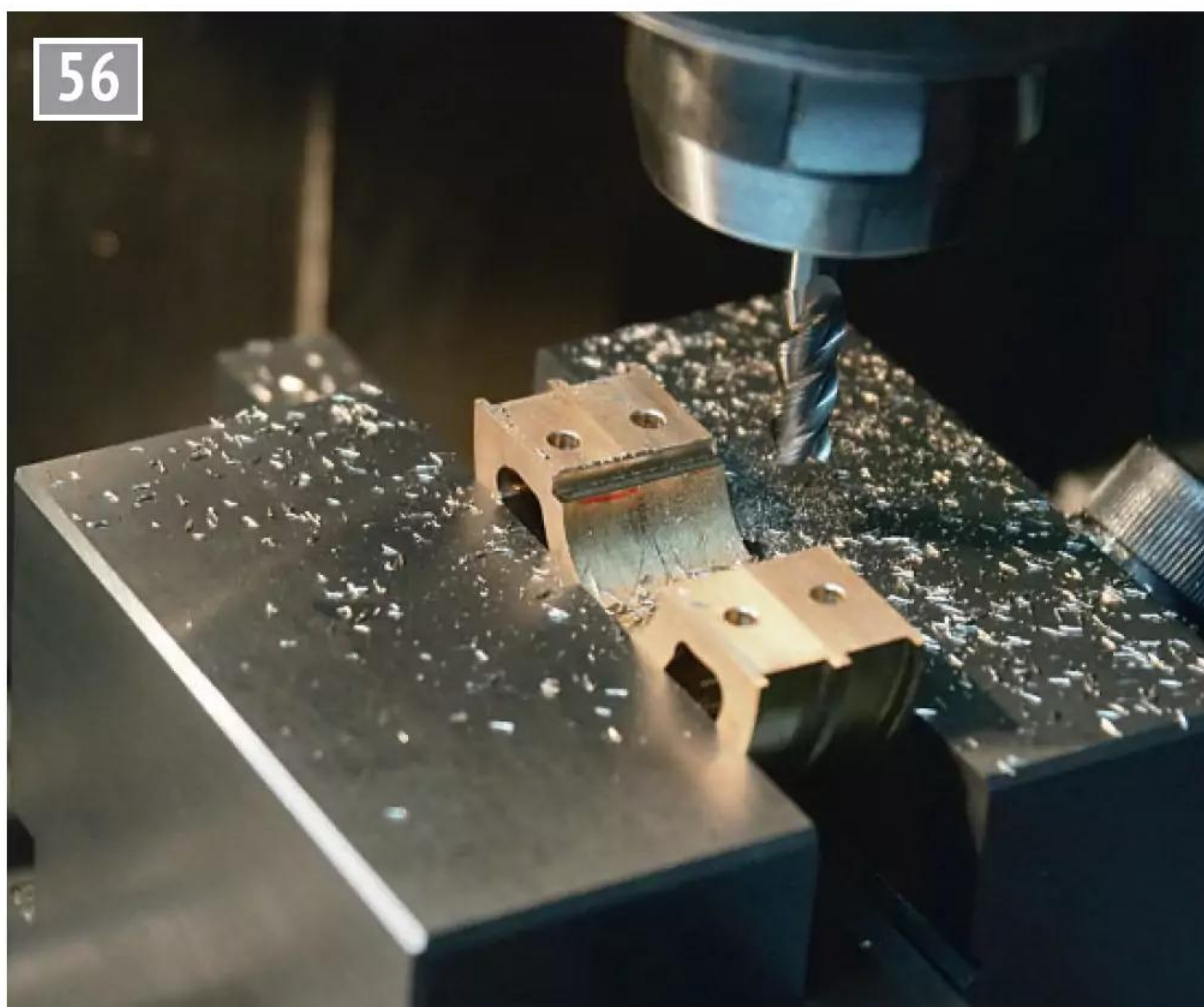
Set-up for machining the keyway in the pulley and drilling the stud holes.
