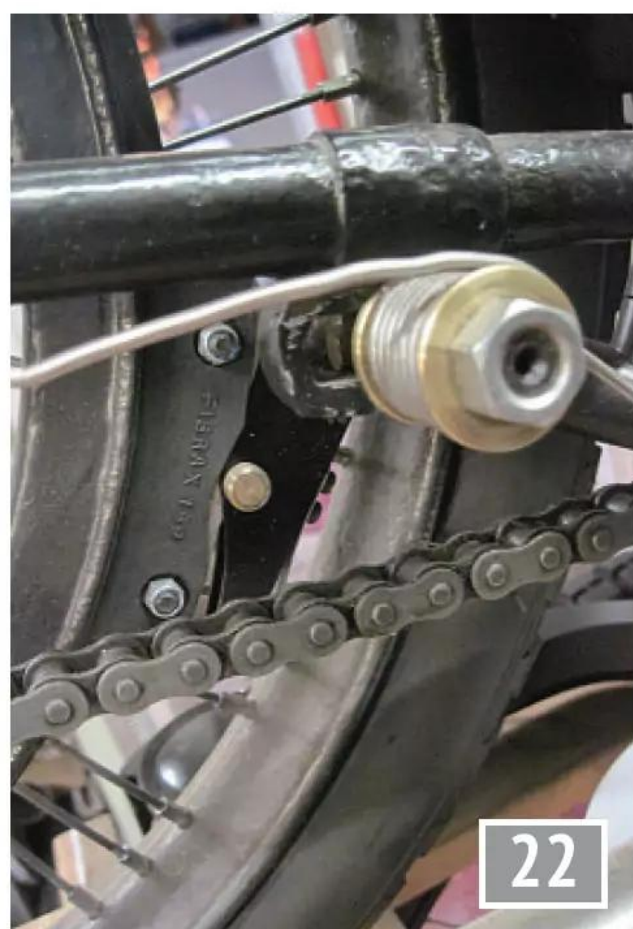
Rear brake. Rubber 'wedge' in centre of the picture.
