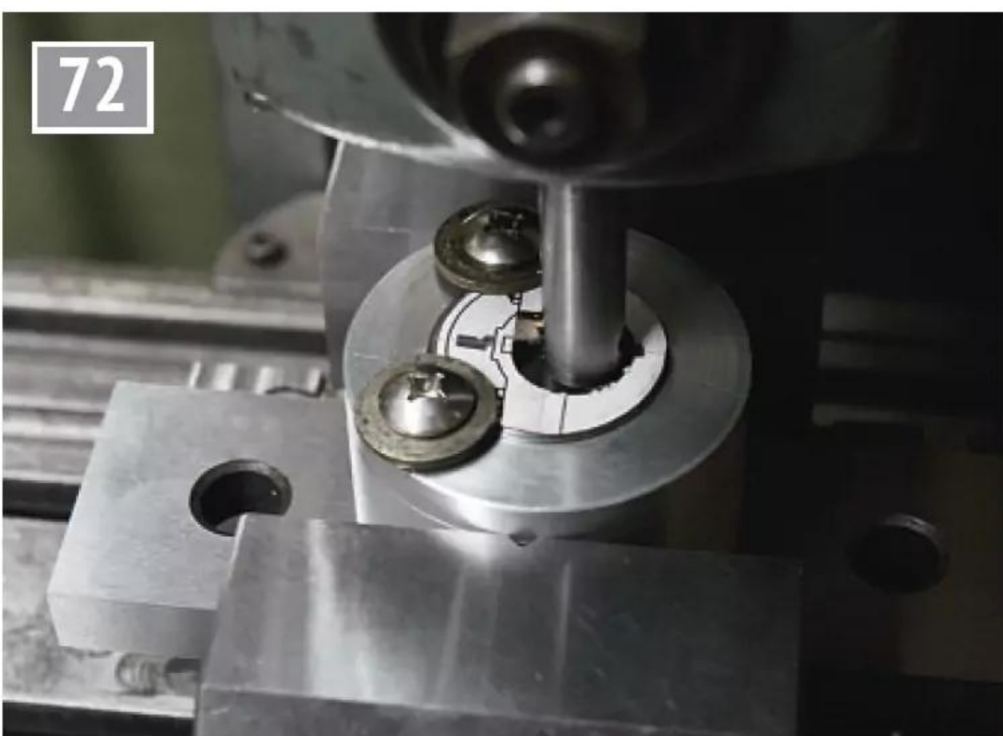
CA glue wasn't strong enough to hold the eccentrics for slotting - two M6 screws were.
