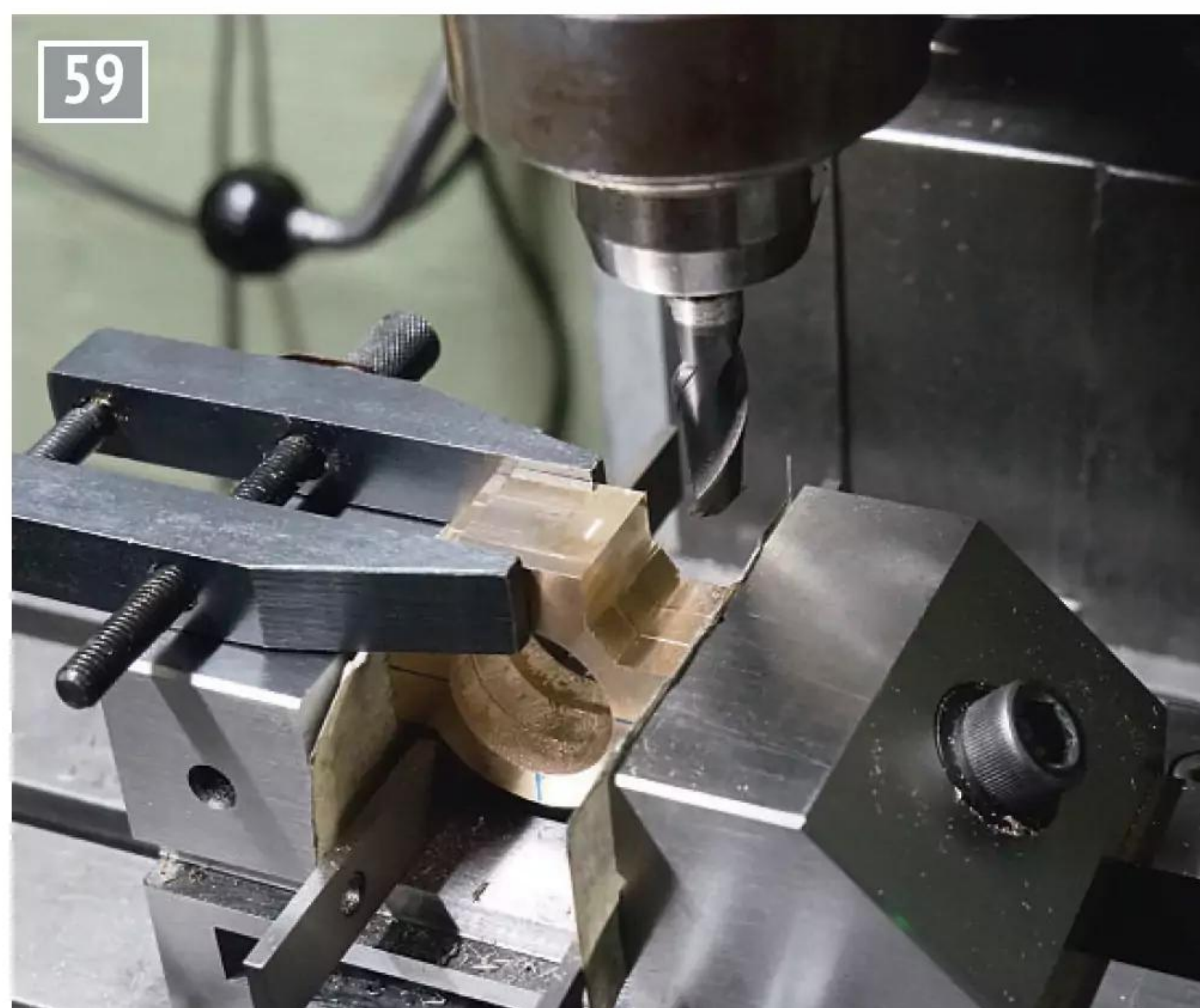
More work on the outer surfaces of the eccentric strap castings.
