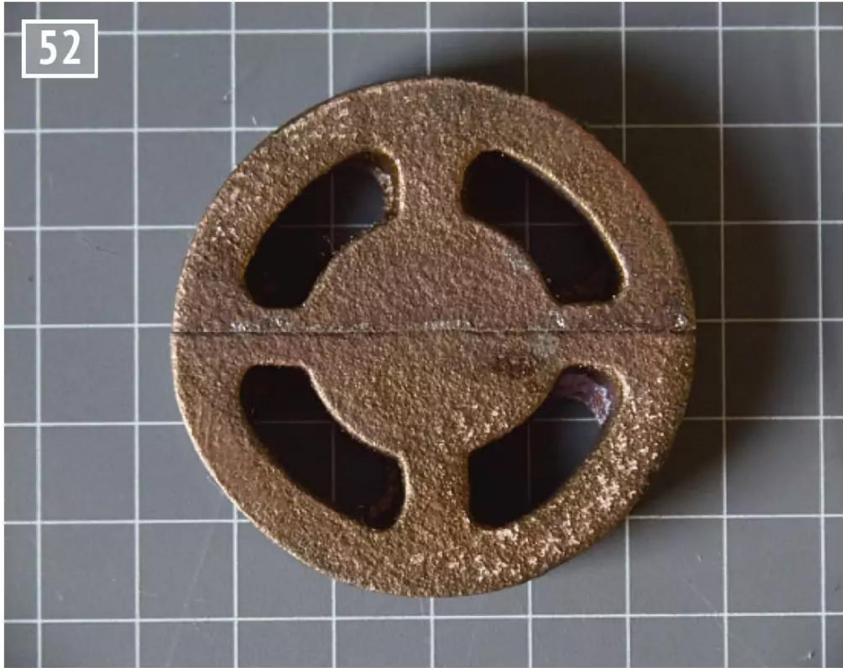
Pulley re-assembled with soft solder.
