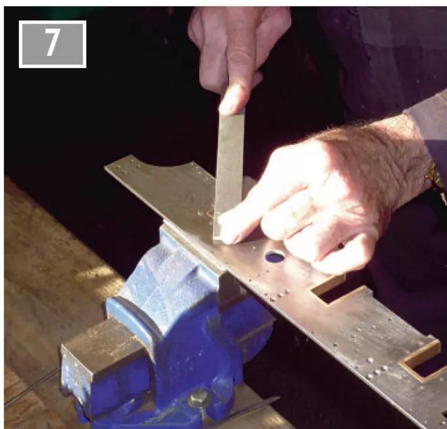
Filing the horn retaining rivets flush.
