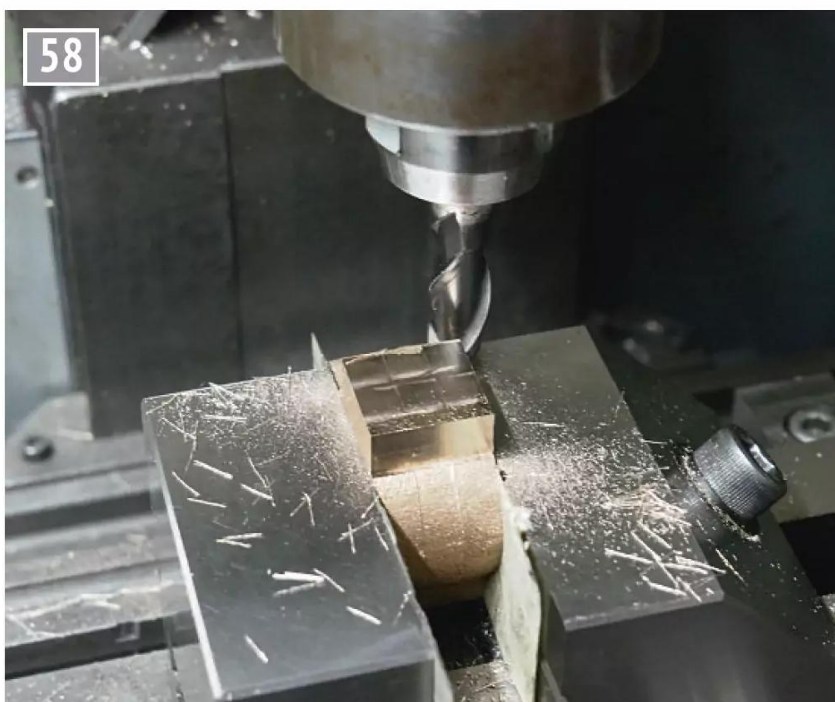
After facing both sides of all three castings they were machined as a group.
