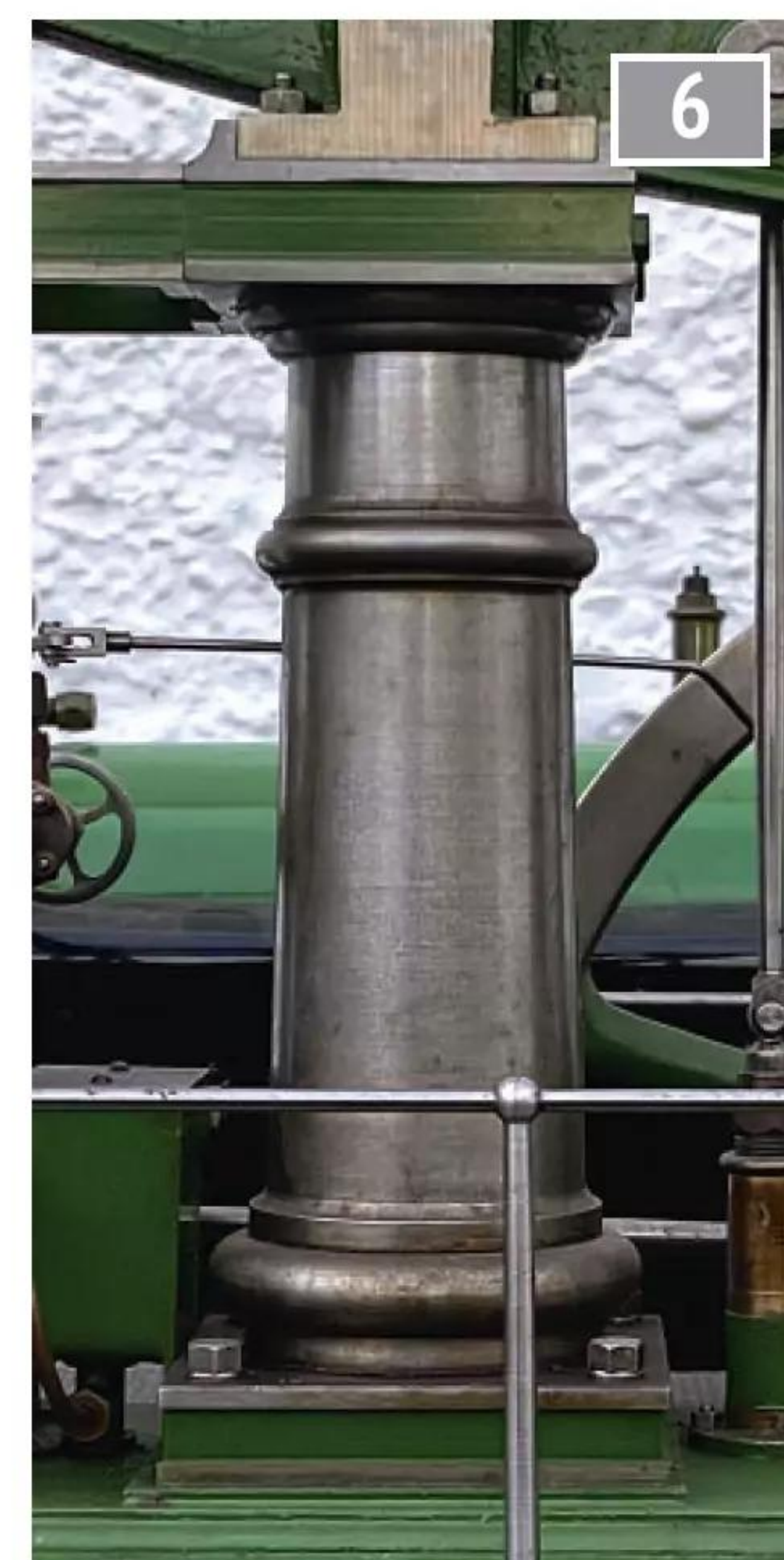
The column has its two decorative rings – known as tori – turned to near perfection.
