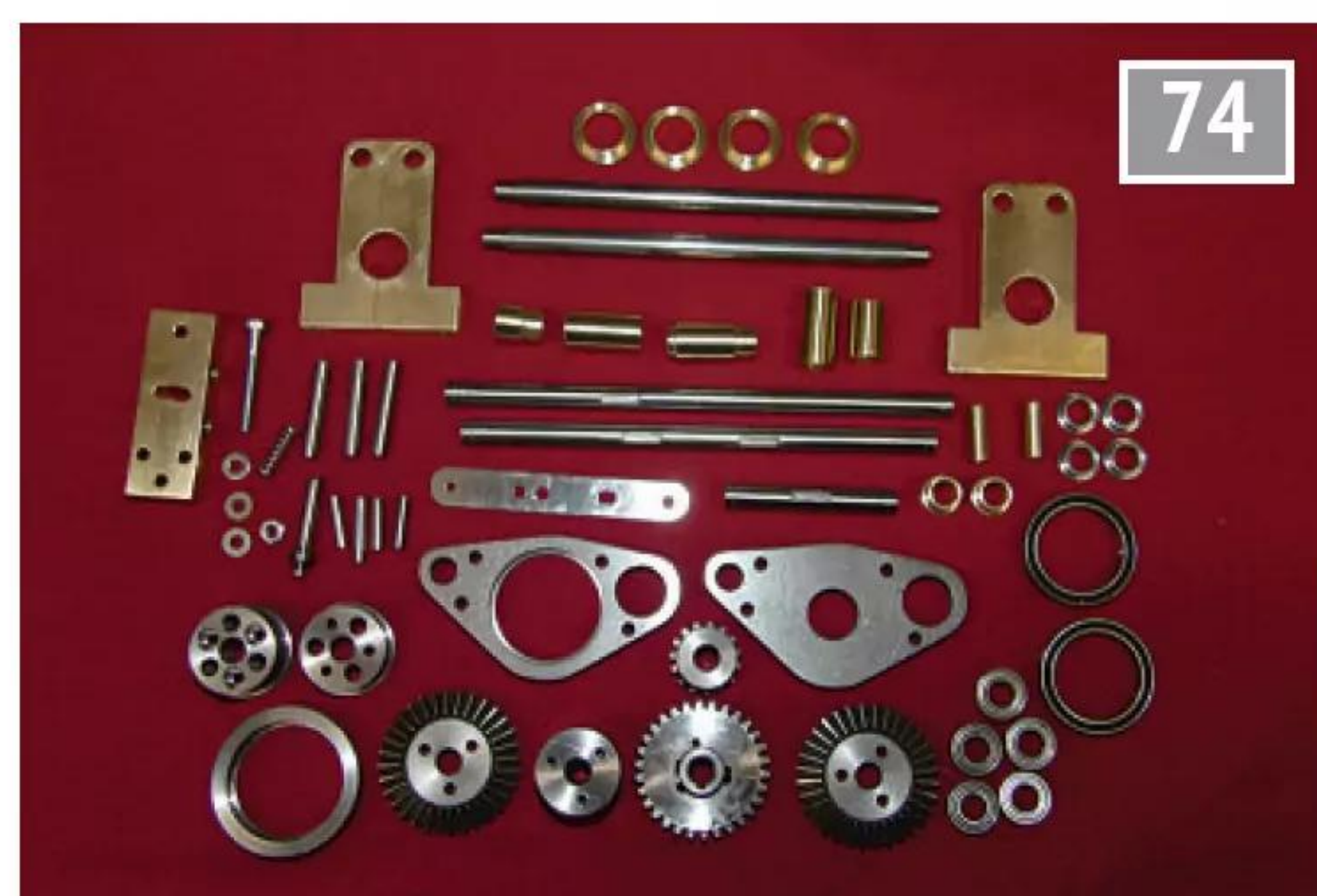
Array of parts for output of transmission and forward/reverse gear change. Hoped for a simple sub-assembly...
