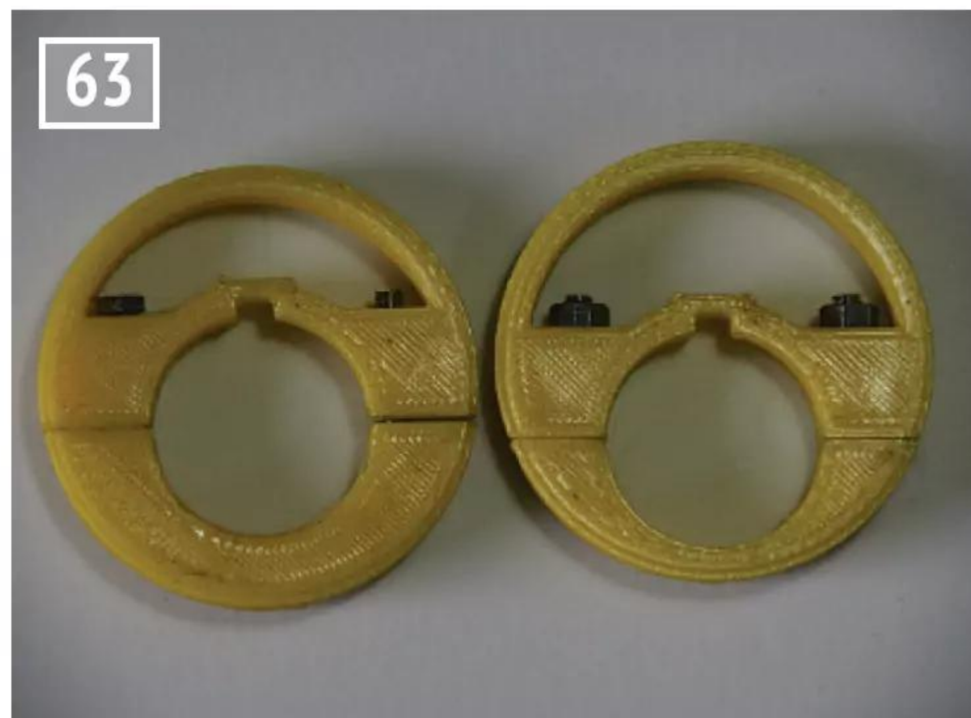
3D printed dummy eccentrics used to help work out how to make these parts.
