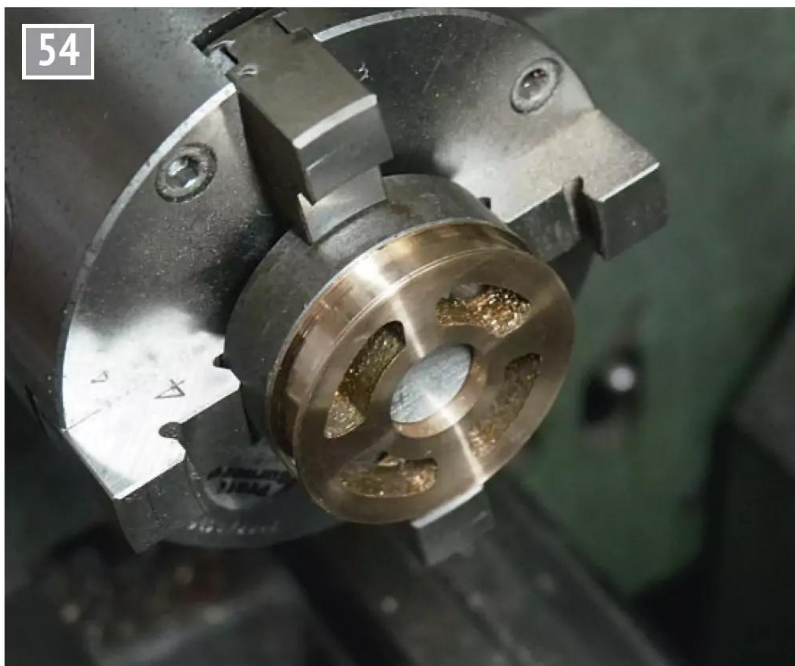
The pulley glued to a steel mandrel with CA glue in order to machine the other face and the belt groove.
