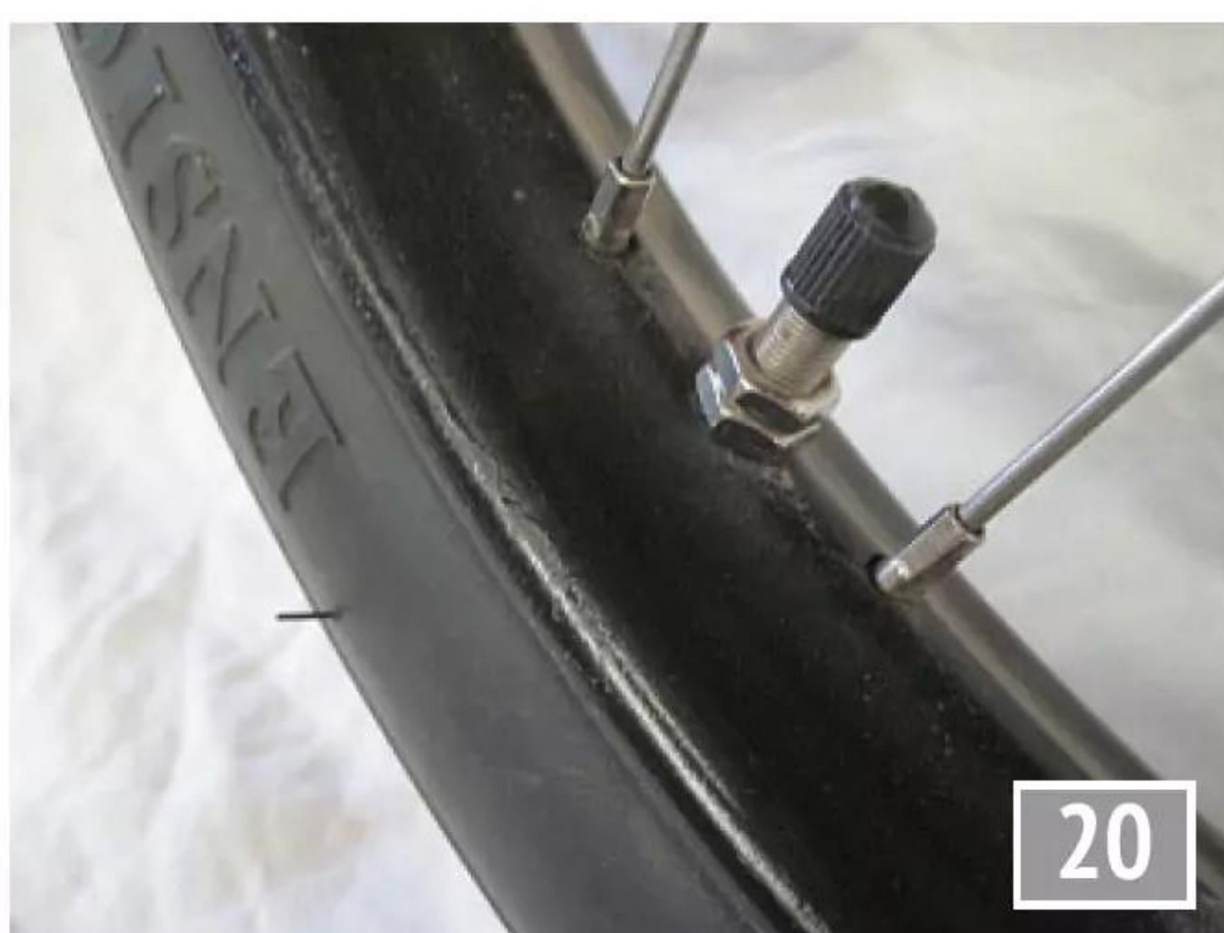
Flat rim carrying the bead edge tyre.
