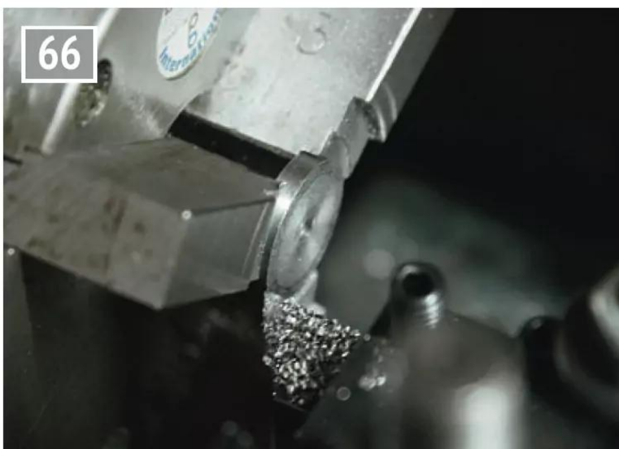
Soft jaws were used in the three-jaw chuck to face the other side of each eccentric.
