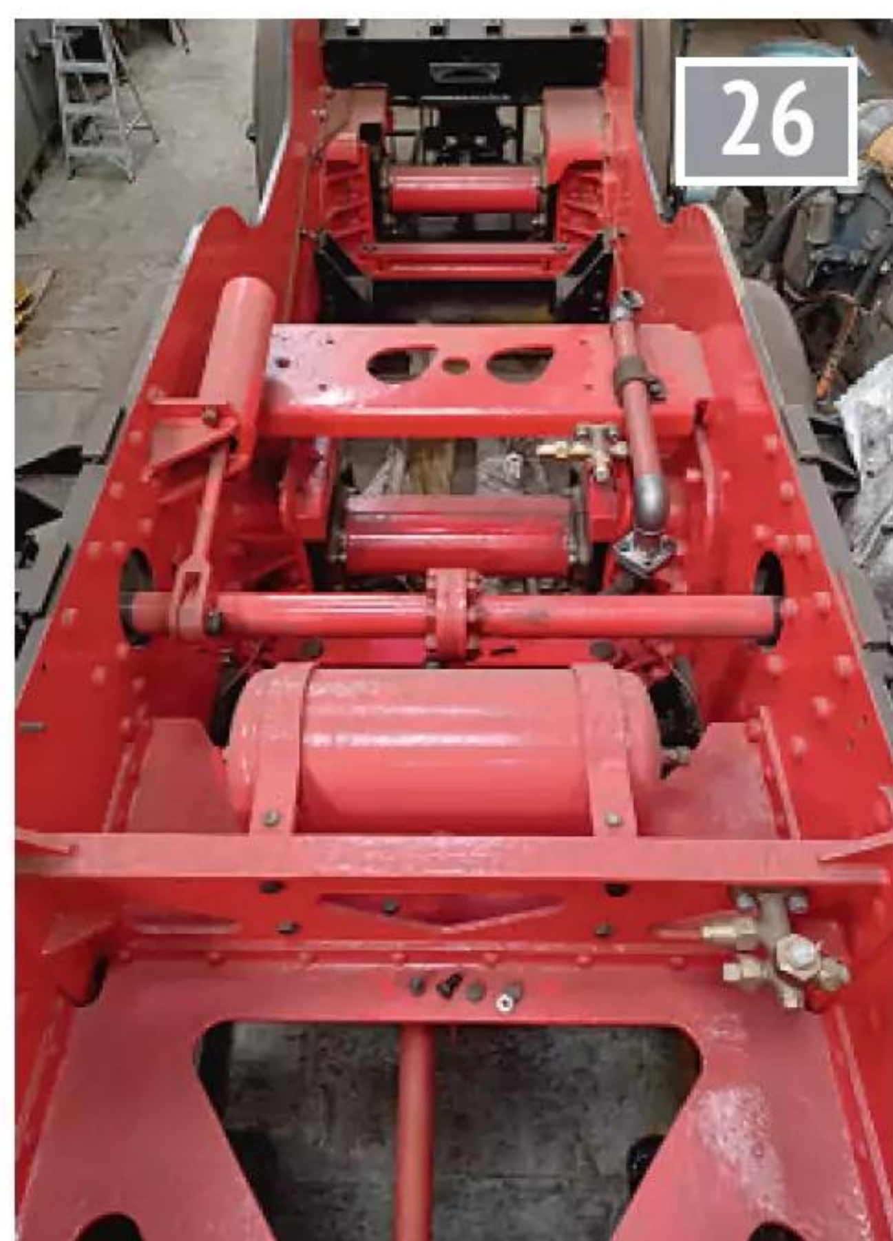
The vacuum reservoir (photo: Toddington Standard Loco Ltd.).
