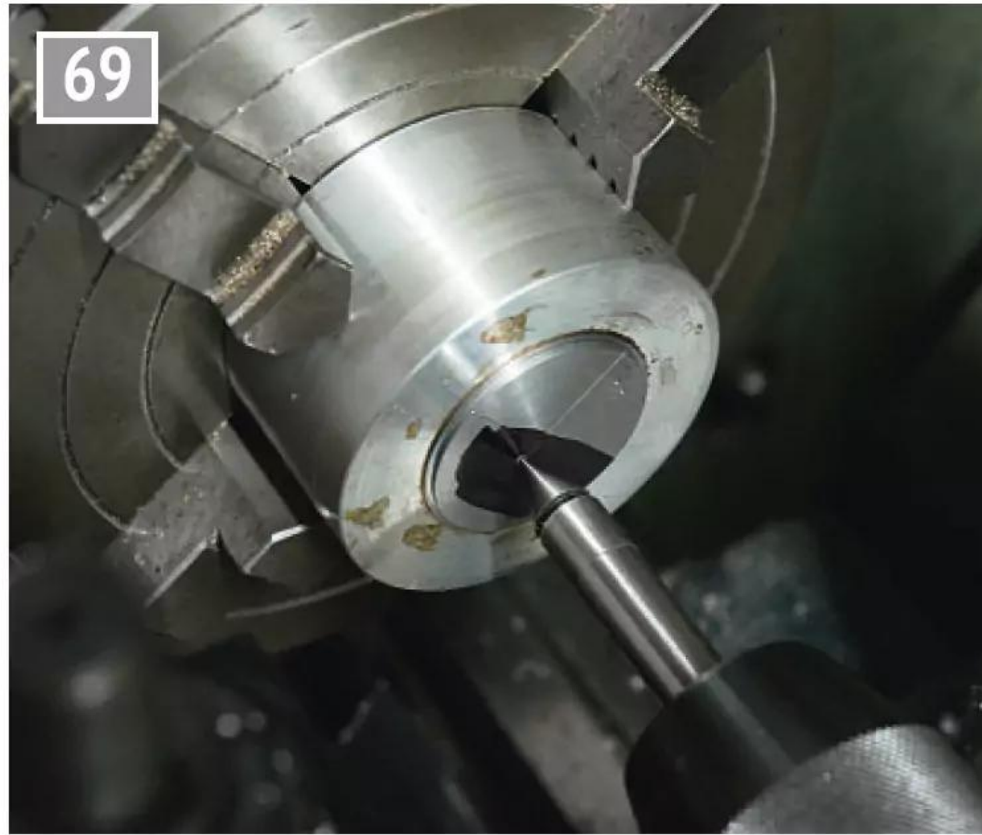
... and the centre for the bore marked out then the pot chuck set up in the four-jaw.
