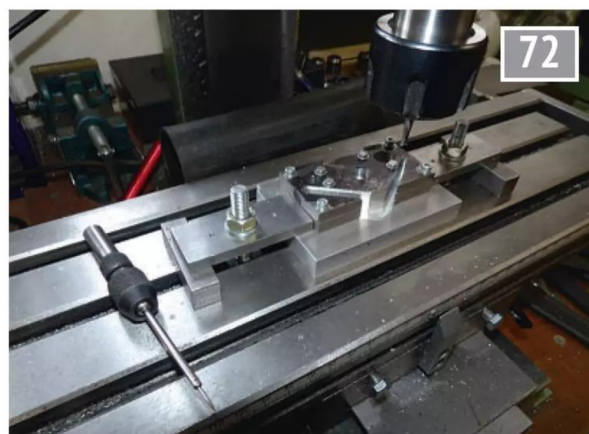
Cutting away outer profile of cheek plates on the mill to reduce hacksaw and hand filing work.
