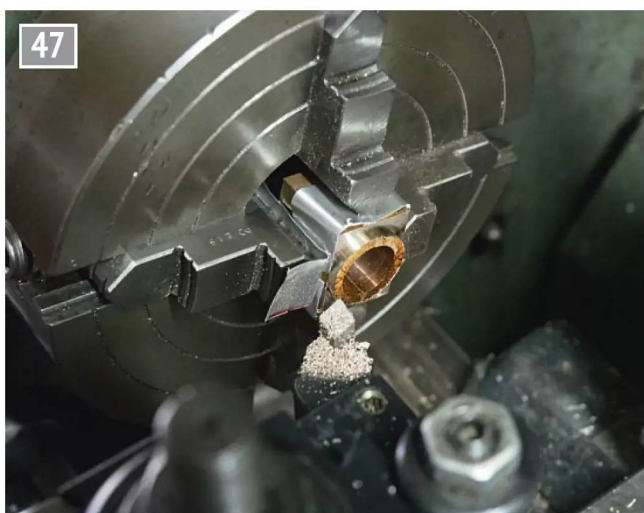
Then the clearance for the oil rings was turned on the other half of the bearings.
