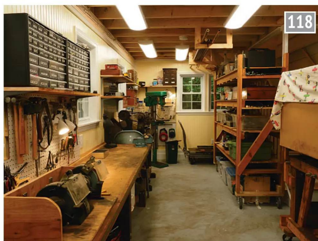
The finished workshop with everything in its intended place. A simple rack for the very longest materials hangs from the ceiling joists above.
