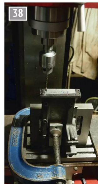
Drilling the bolt holes in the rear flange. Careful measurement from the datums is vital as the holes in the mating flange on the slide have to align.
