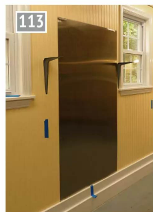
A strategically positioned spatter guard, ready for the lathe's imminent arrival.
