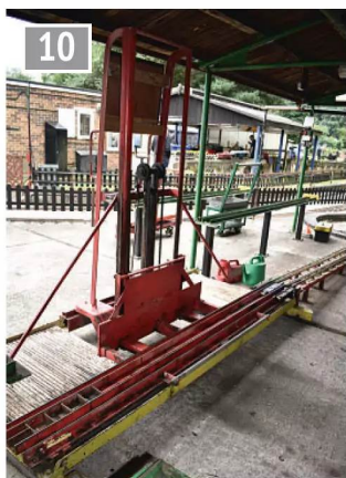
A good sized lifting table for the ground level engines.
