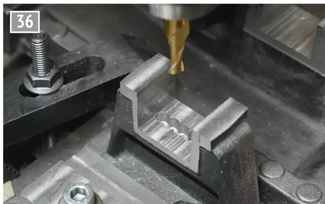
The bottom of each bearing housing needed an oil reservoir.
