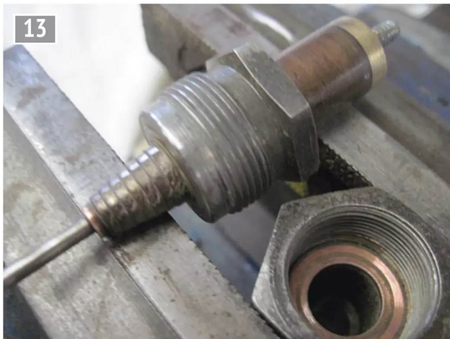
...and dismantled. Note the mica insulation.
