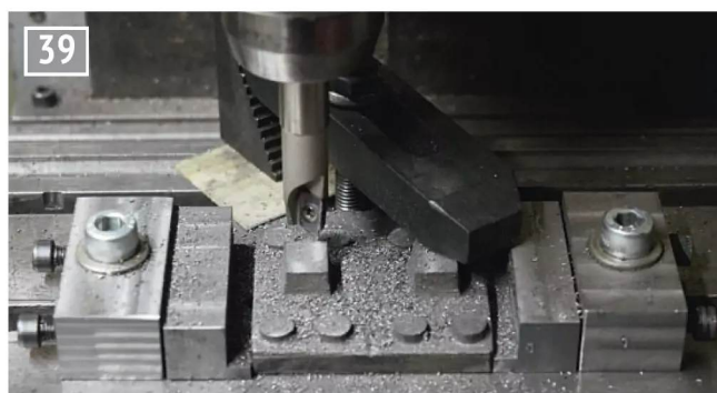
The bearing caps come cast as a pair. The bosses for the nuts and the tops of the oil pots were roughed out ...
