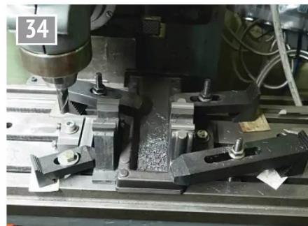
Set-up for machining main bearing housings.
