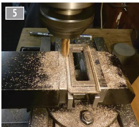
Milling the toes of the horns.
