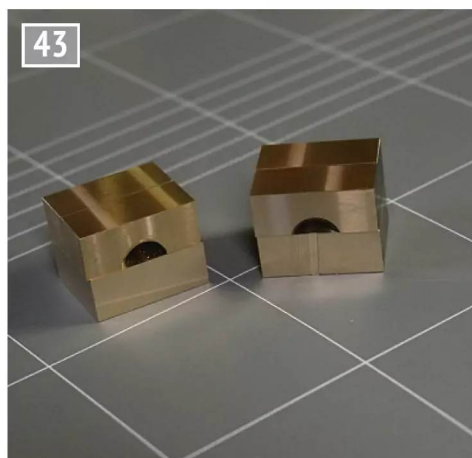
Recycling hoarded material is good but can lead to difficulties. Those half-round holes didn't make good places to start the drilling and boring.
