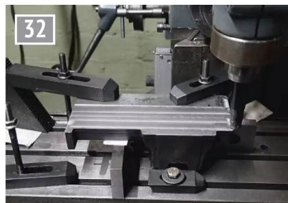
Machining the base of the bedplate. This is the datum for vertical dimensions.
