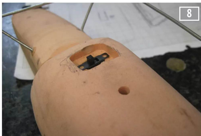
Fitting the switch.
