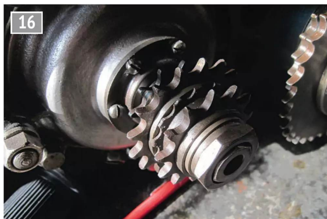
The patent slipping clutch - inside the drive sprockets.
