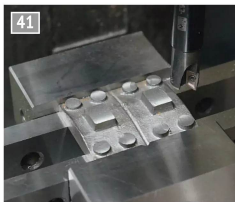
Going back to the top and facing off parallel to the now smooth base.
