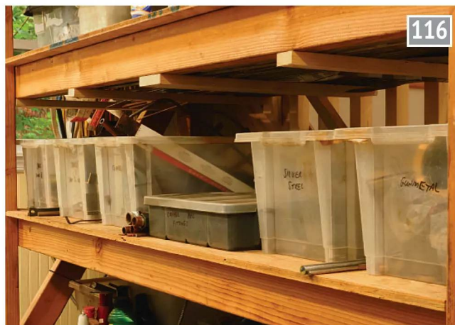
Offcuts of each metal type are stored in segregated containers. Longer items - up to 2 feet long - lie adjacent with their ends visible for quick identification.
