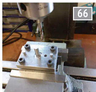
66 Set up on the mill to accurately match crank pin drilling.
