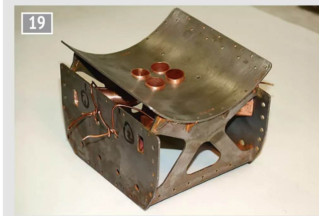
19 Exhaust ways wired ready for silver soldering (photos: Geoff Whittaker.)
