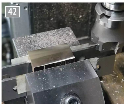
Whatever the original form of the bearing brasses they need to be squared up to size.
