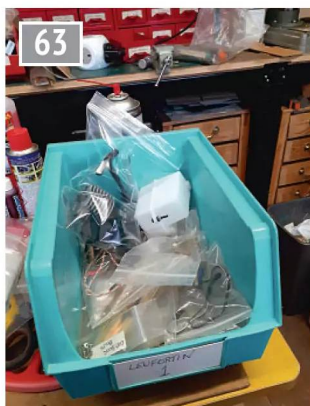
Bagging and tagging all of the disassembled components and isolating salvageable parts.
