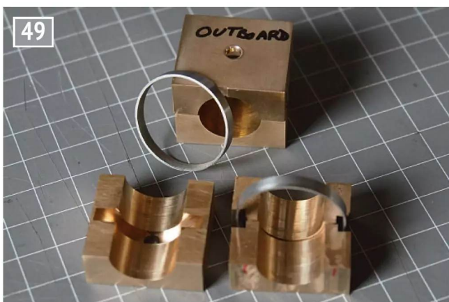
The sets of bearing bits came together to look like this. They are interchangeable but I marked them anyway in case of differences due to wear in the future,
