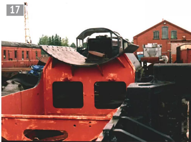
17 Rear view showing the four stiffeners (photo: Toddington Standard Loco Ltd.)
