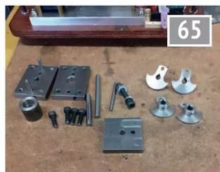
65 Completely new flycranks with keyways and the tooling to ensure all were identical.
