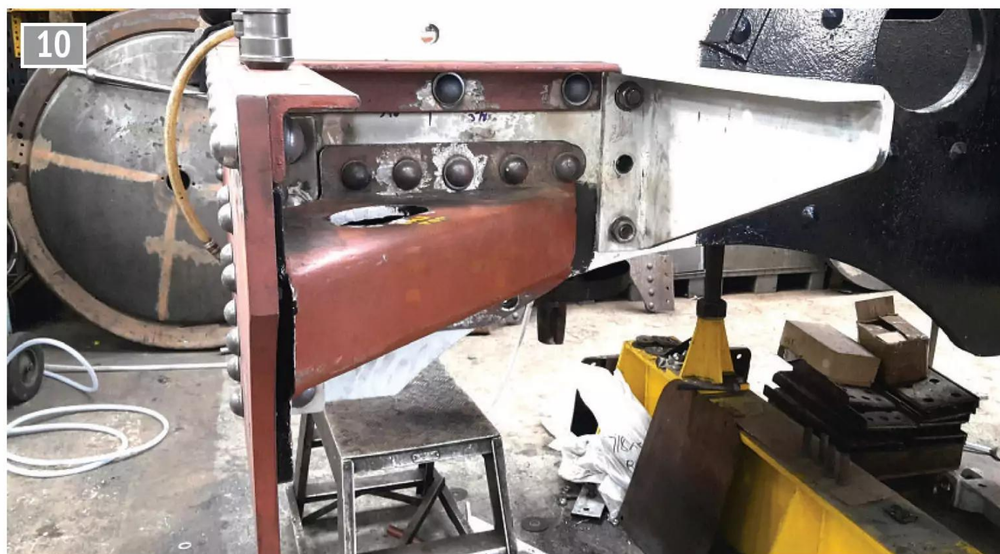
Buffer beam support bracket (later type). photo: Gloucestershire and Warwickshire Railway
