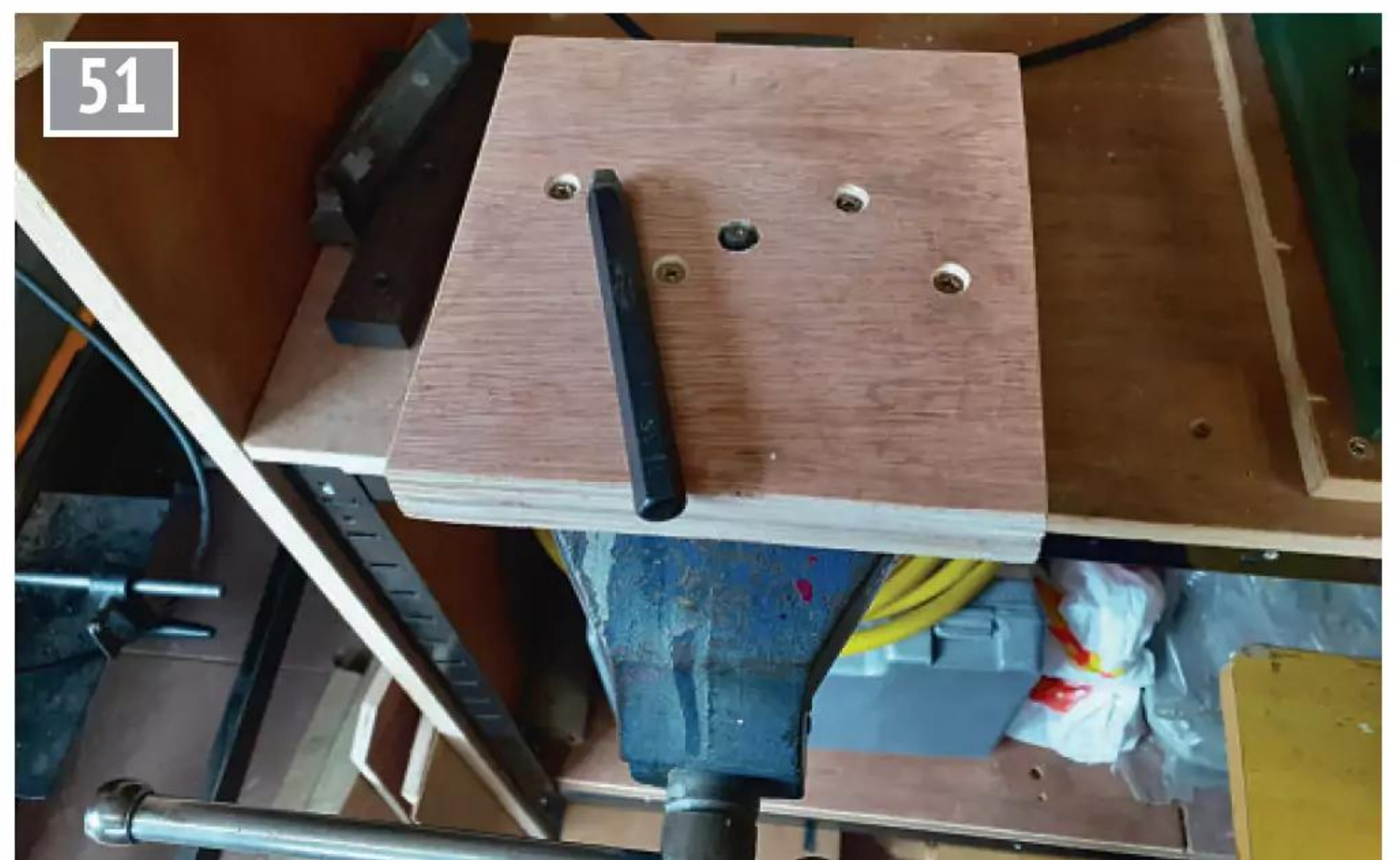
Riveting 'table' for cab alleviating the need to grow an additional hand.
