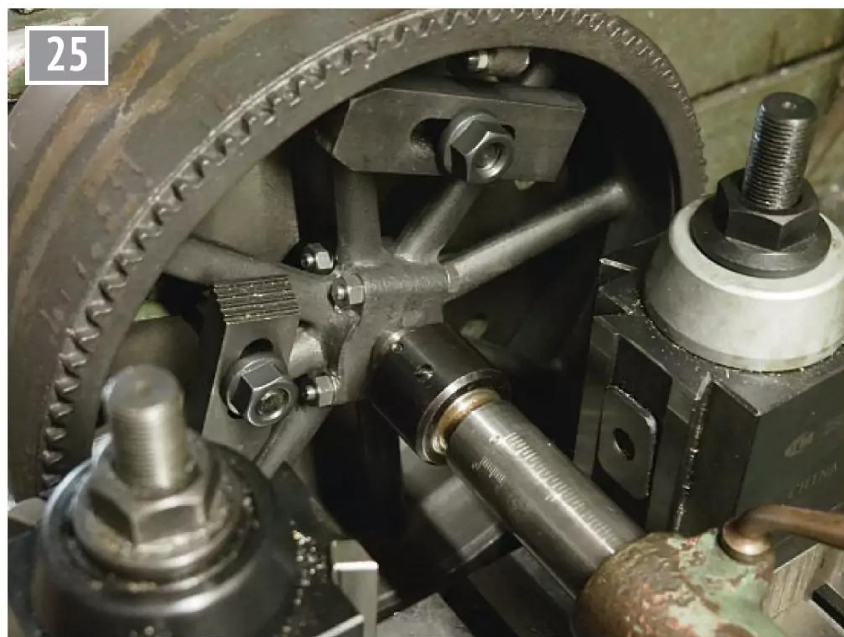
Using the pre-drilled hole to align the flywheel on the faceplate for boring.
