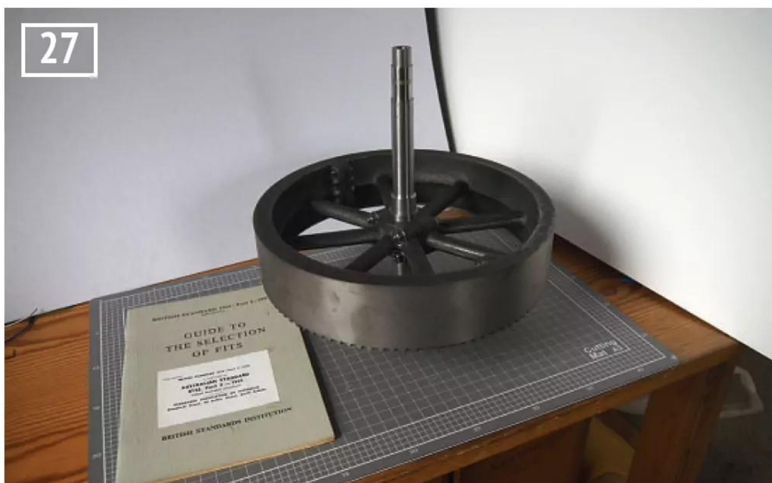
27 Crankshaft and flywheel fitting together as they should, but it didn't last.
