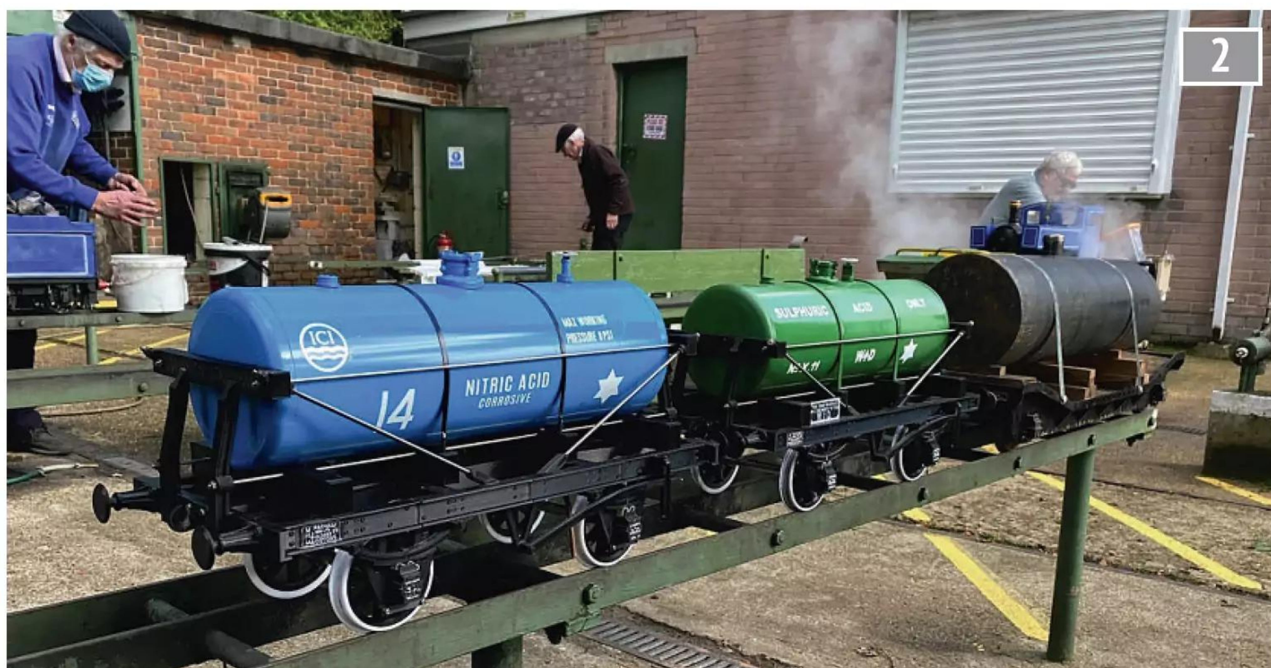
A pair of 3D printed tank wagons, made with minimal machining, almost entirely 3D printed.
