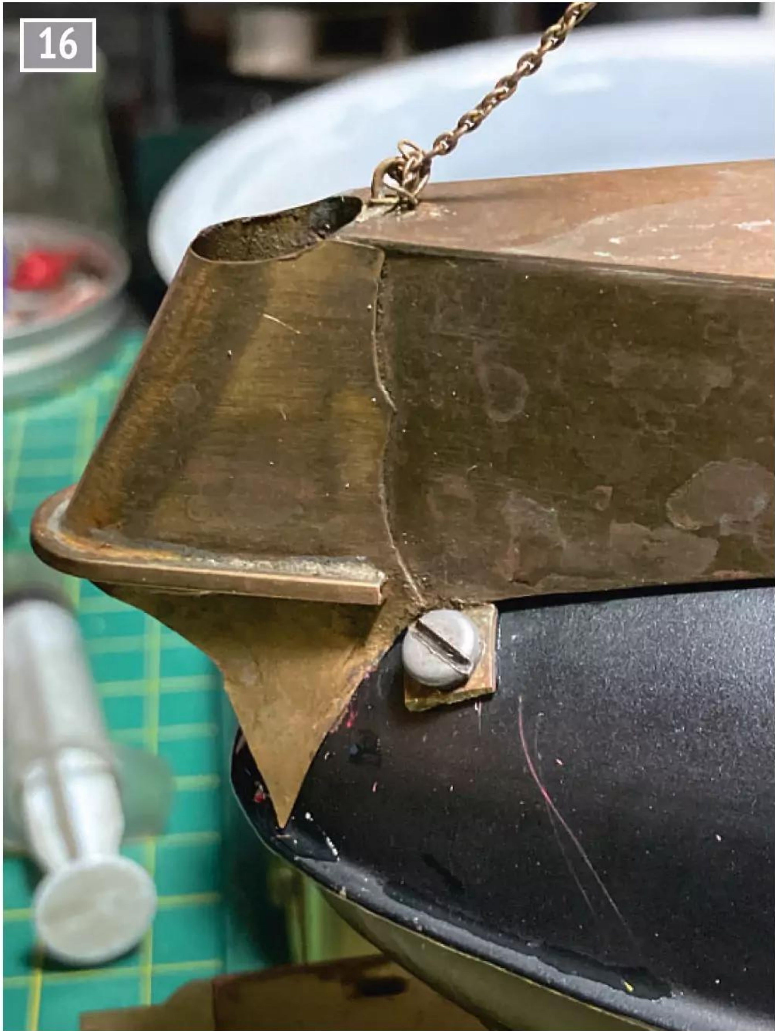
One of the two screws that hold the deck down on the bow is evident here.
