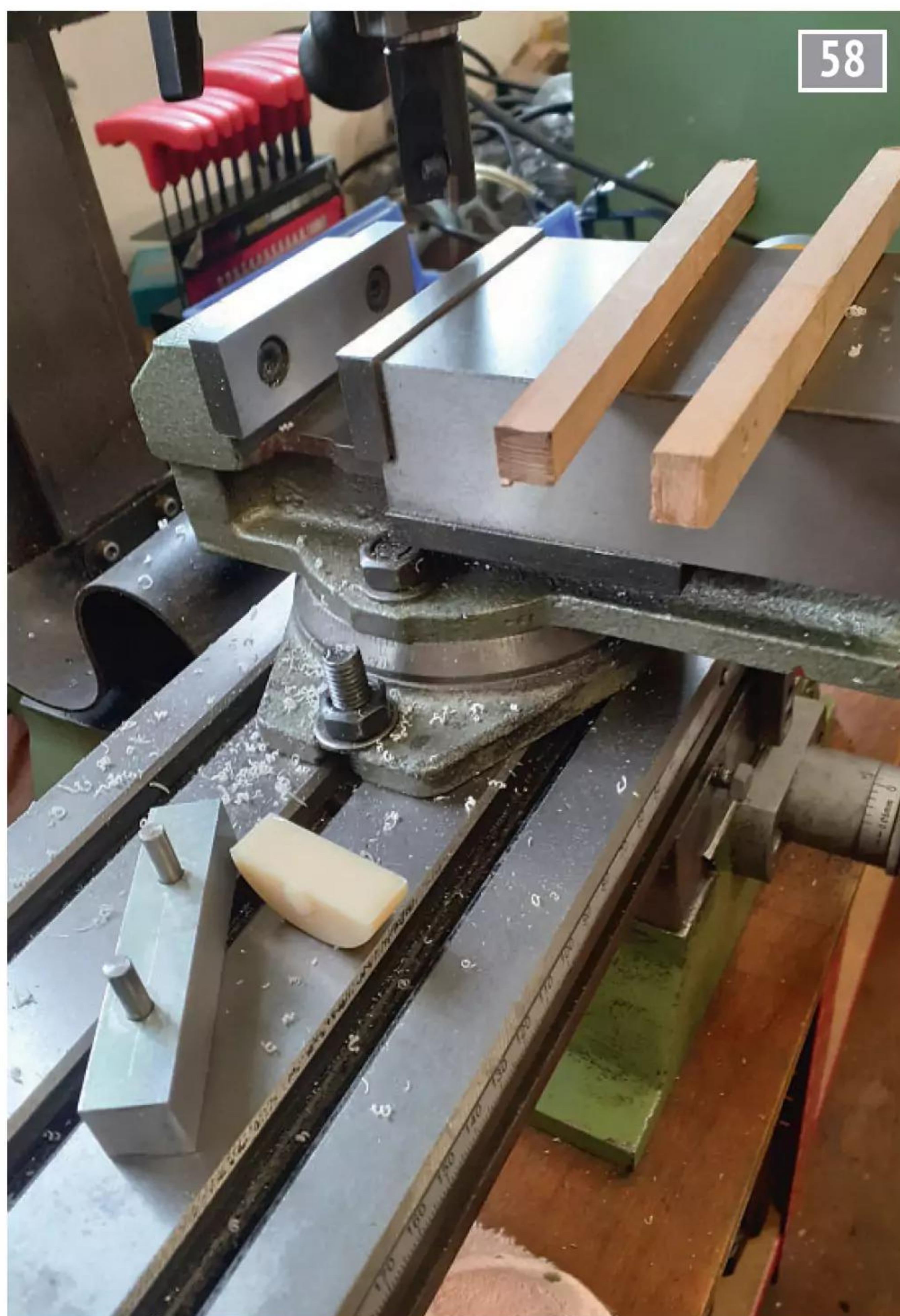
Milling operation for dumb buffers.
