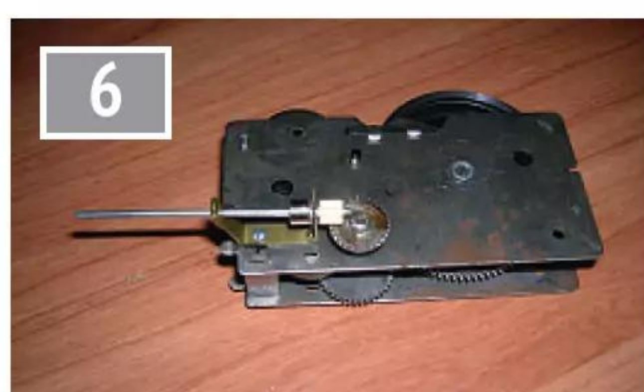
Sprocket gear is mounted on drive axle with JB Weld epoxy.
