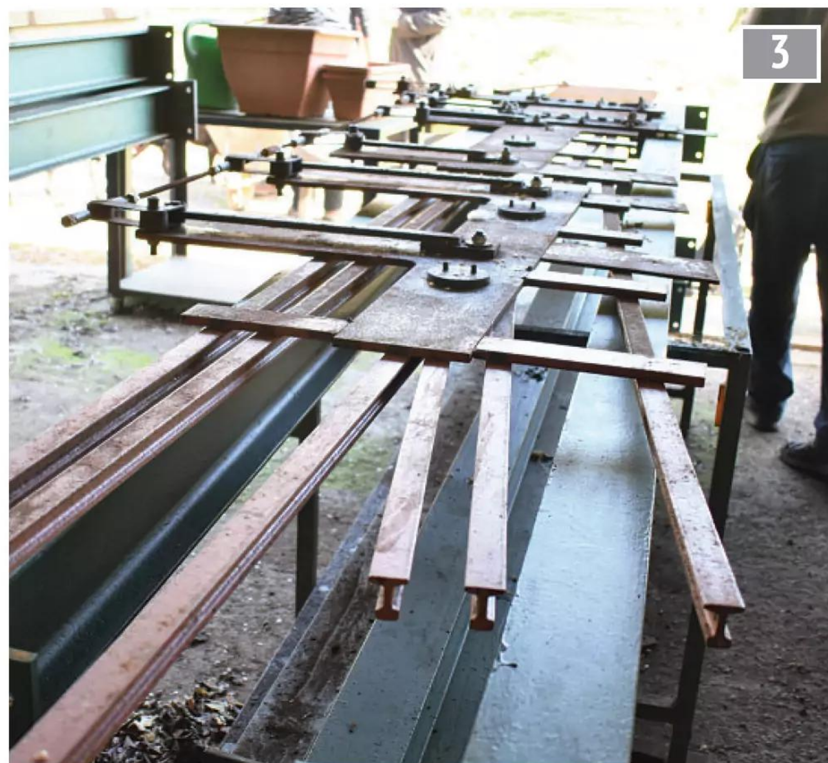
The underside of one of the new points showing the cams and operating levers.
