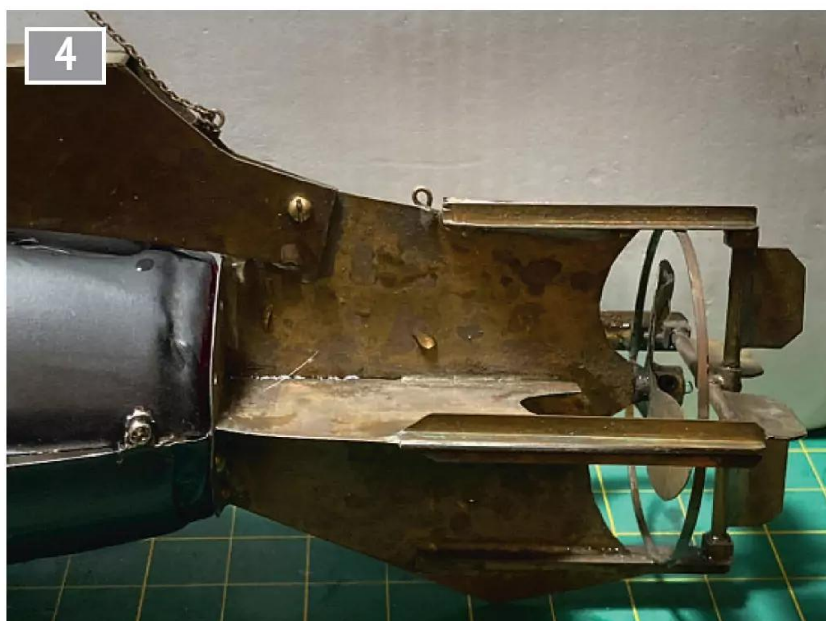
Of note is the single bolt holding the rear deck on and the sheet metal screw in the tab fastening the hull halves together
