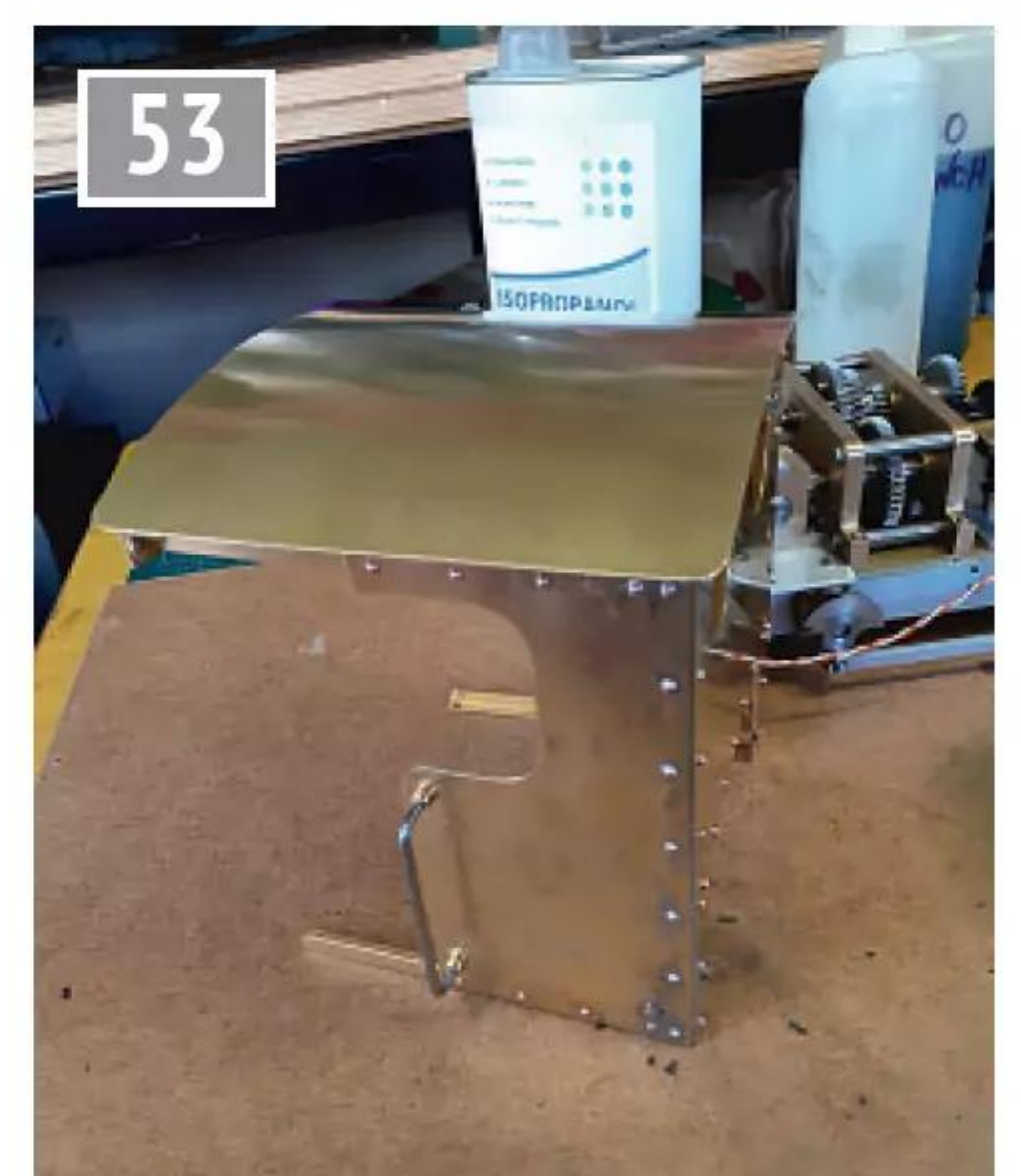
Cab roof finished and trial fitted.
