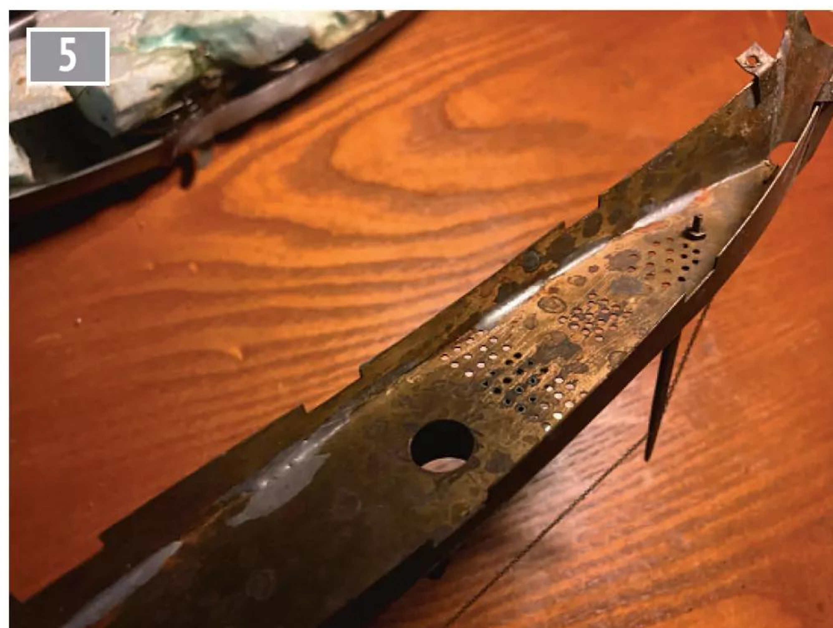
The two mounting tabs on the bow can be seen here and these are for mounting the deck to the hull.
