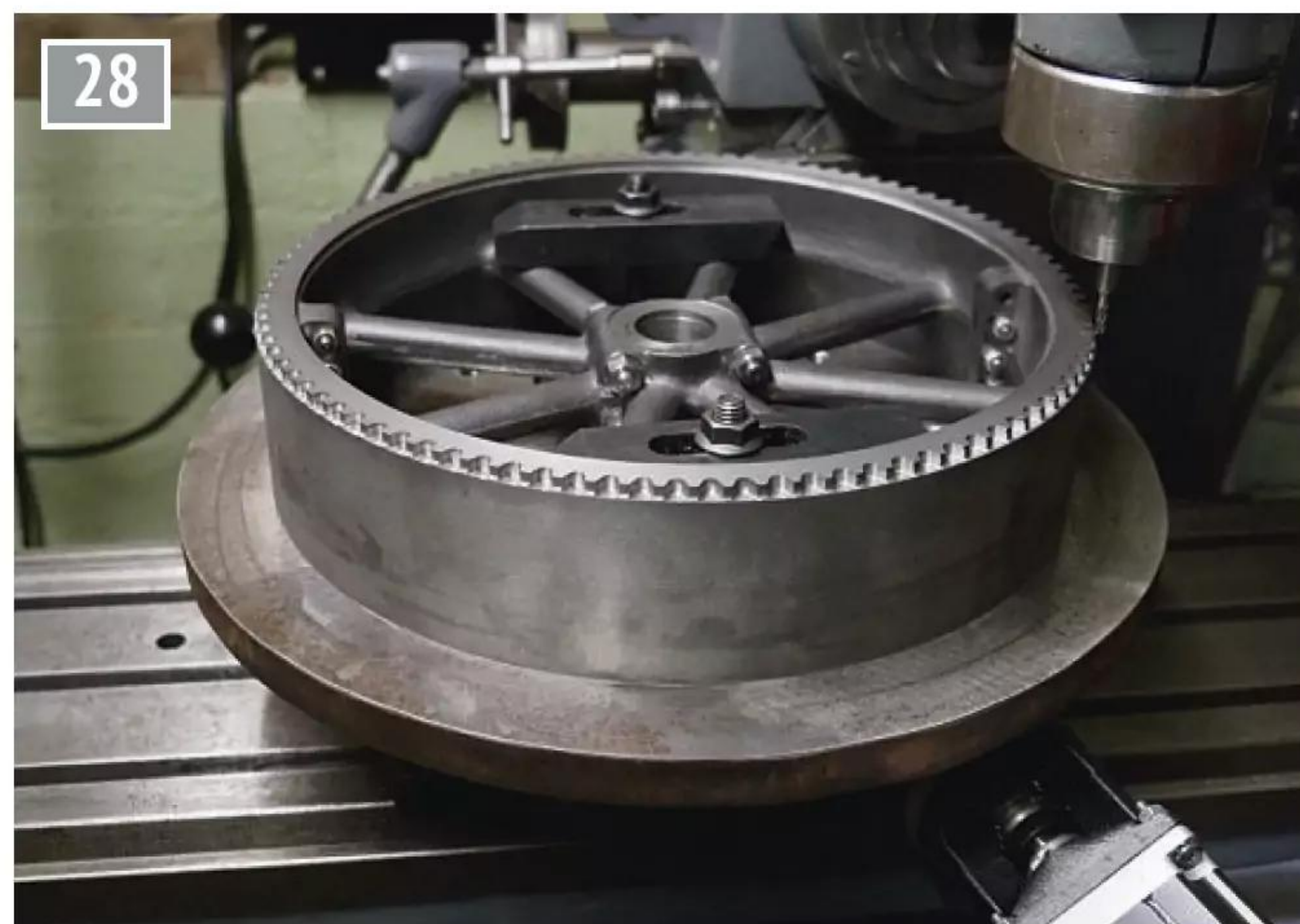
28 Re-cutting barring teeth the slow way.
