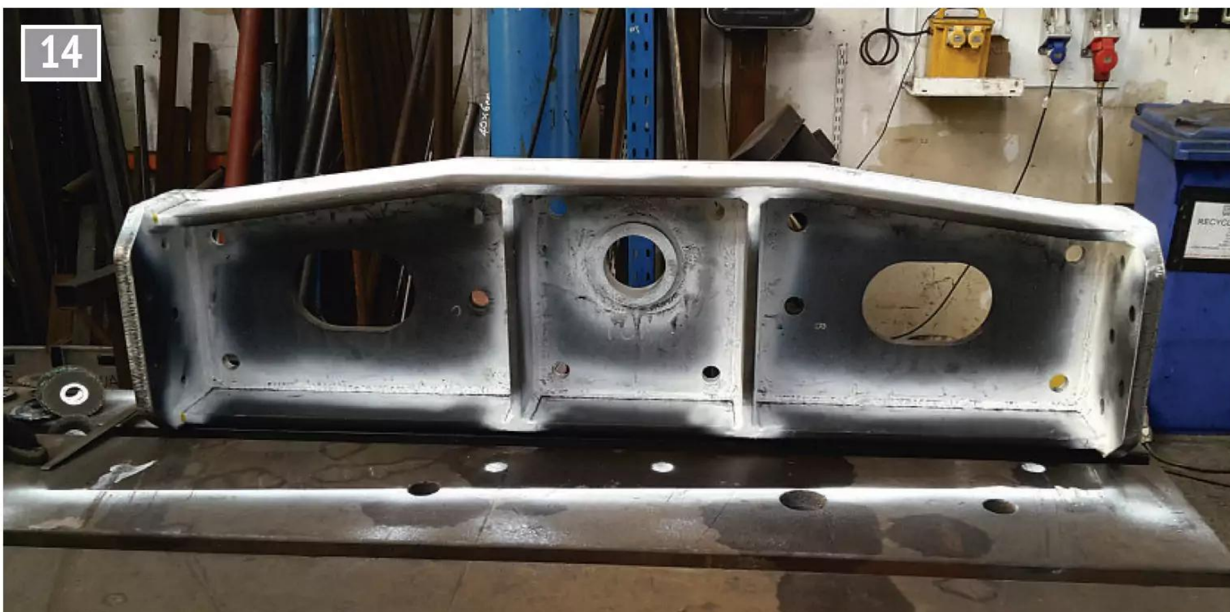
Pony truck pivot support. photo: Gloucestershire and Warwickshire Railway
