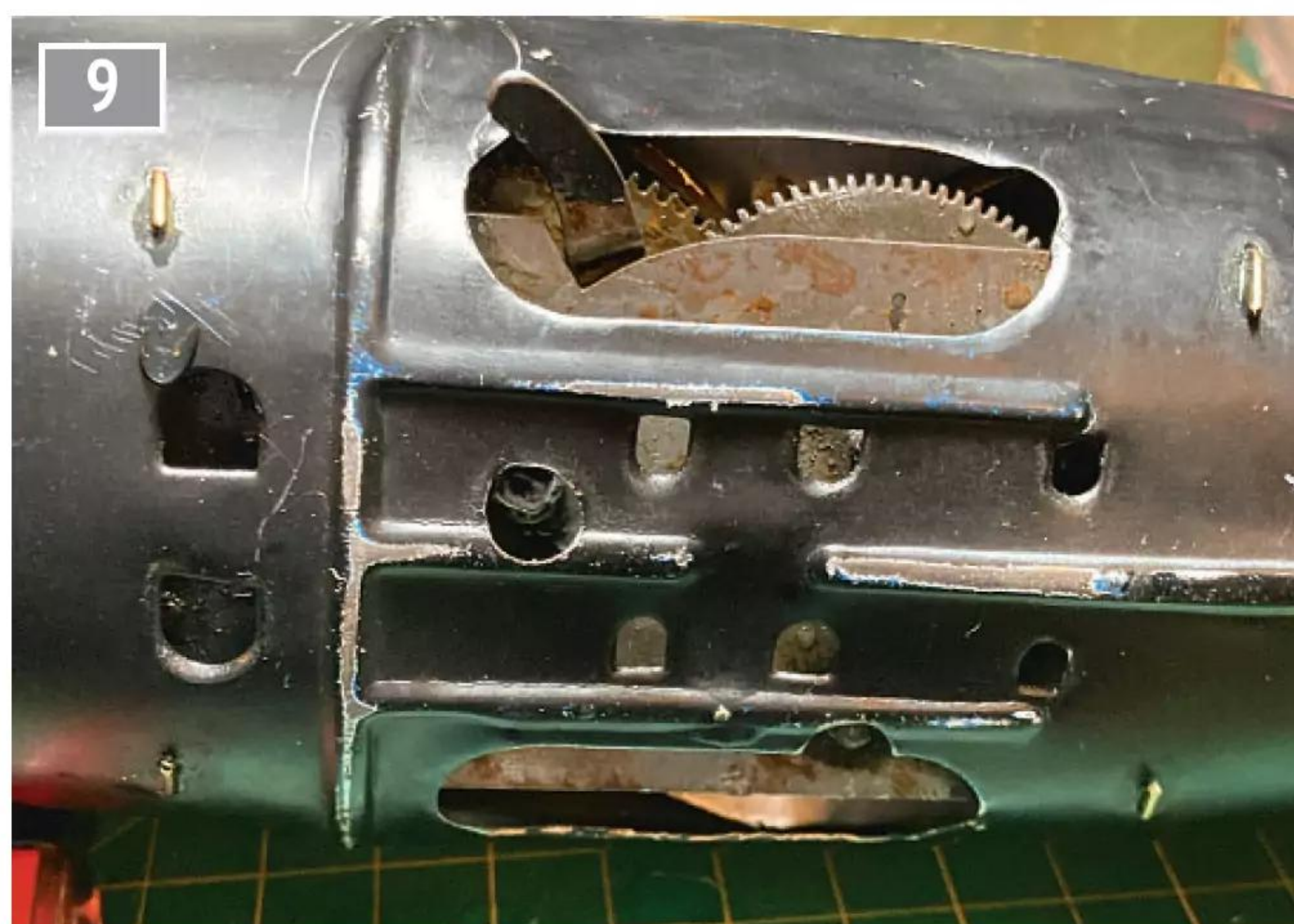
The brass wire holding the wind-up unit to the bottom of the hull is visible here.
