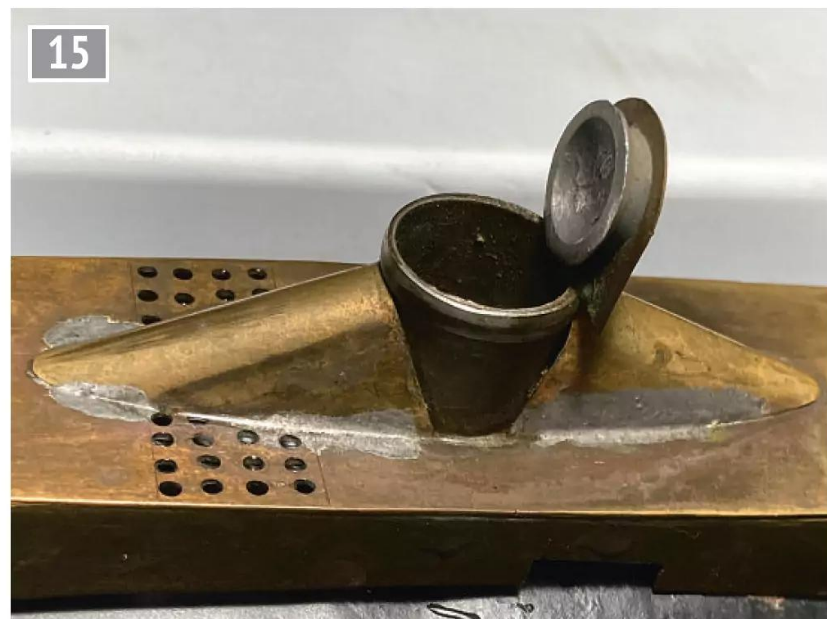
Very thin brass sheet for the coamings makes bending much easier.
