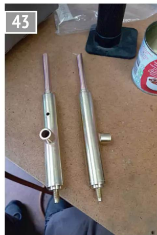
Two exhaust resonators pickled, cleaned and ready for final silver soldering operation.
