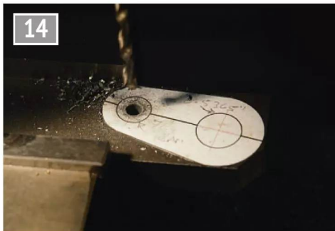
Crank material set up for drilling and reaming.
