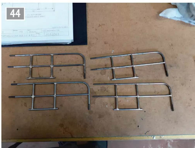
Four completed side handrails.
