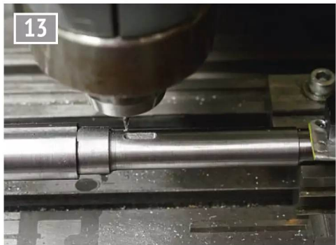
Cutting the governor pulley keyway. You need to approach the correct width a little at a time using a piece of key material as a gauge.
