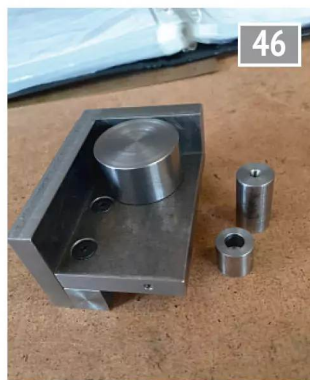
Over engineered handrail bending fixture.
