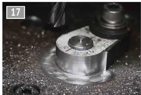
Crank located on the sub-table for rounding over the larger end with a central pin and cap screw through the hole for the crankpin.
