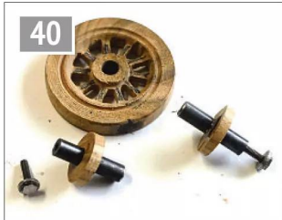
Rear wheels and stub axles.
