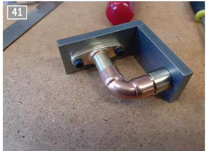
Exhaust manifold 'dry-run' in silver soldering fixture.
