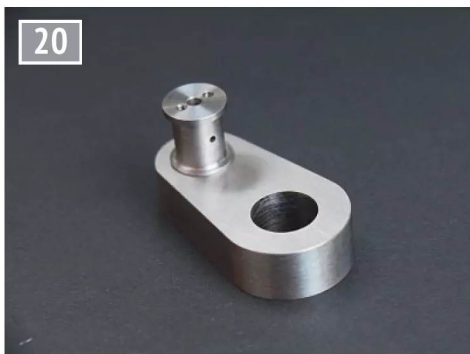
Crank and crankpin assembled.
