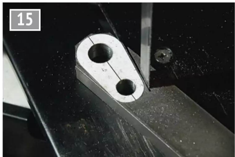
Bandsawing the crank from the stock.
