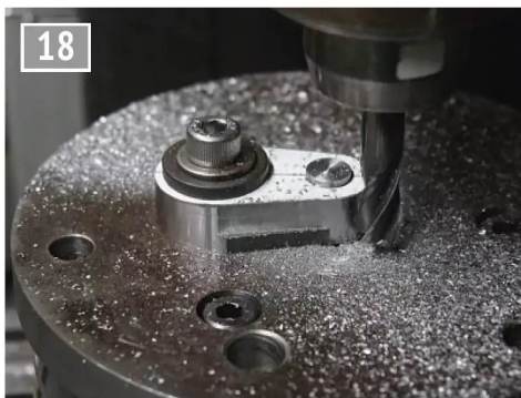
Finishing the sides of the crank.
