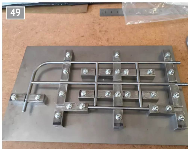
First handrail dry run at assembly.
