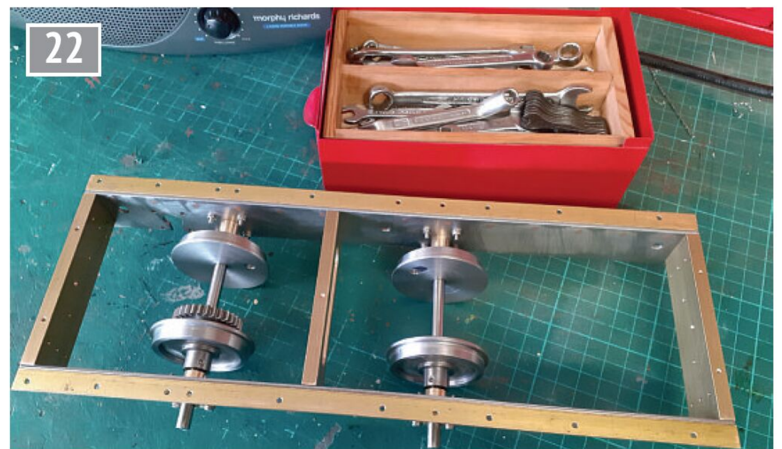
The chassis on its wheels having been 'dry run' assembled to get axle centres for coupling rods.
