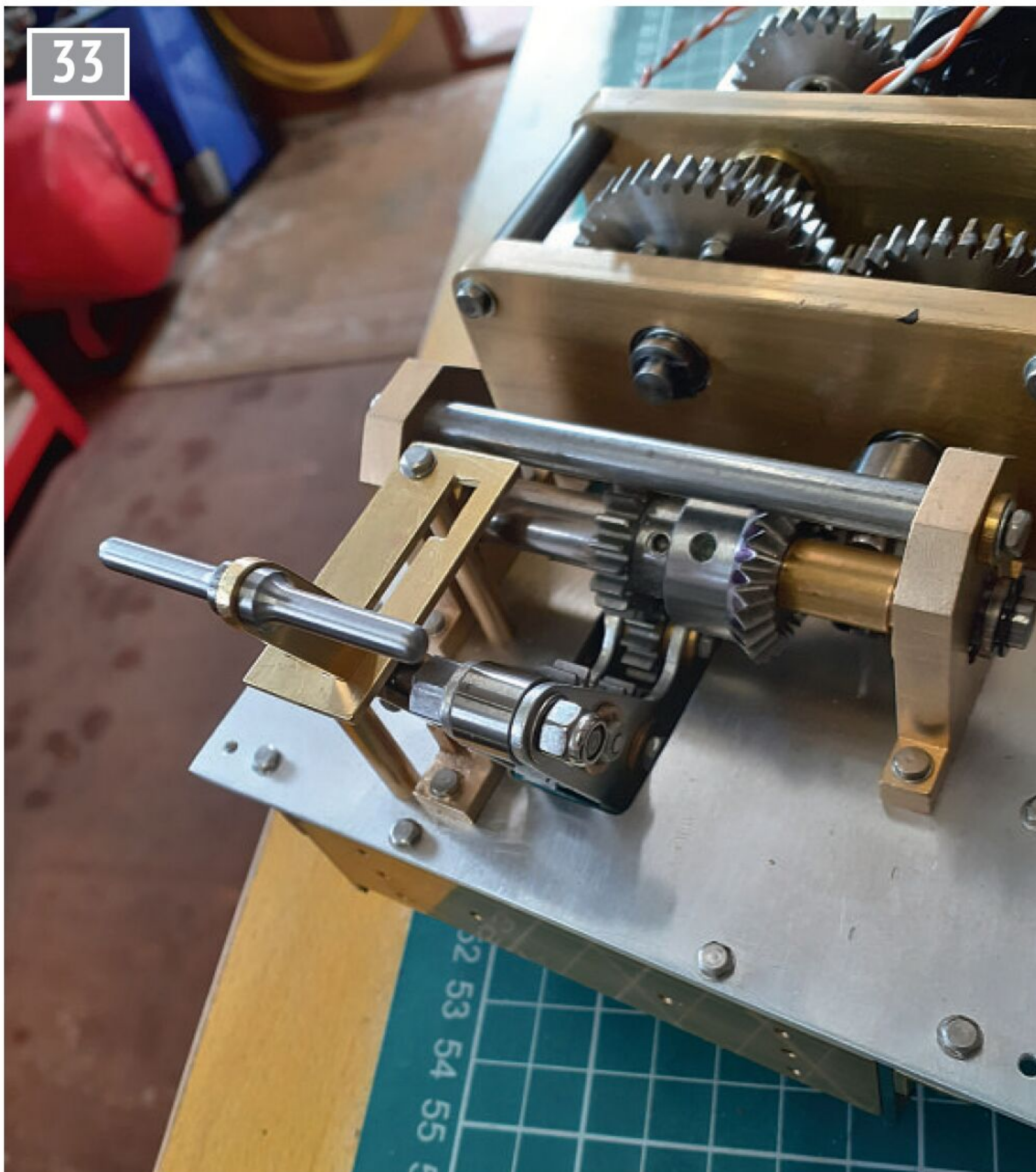
Right hand side view of Fwd/Rev change mechanism.
