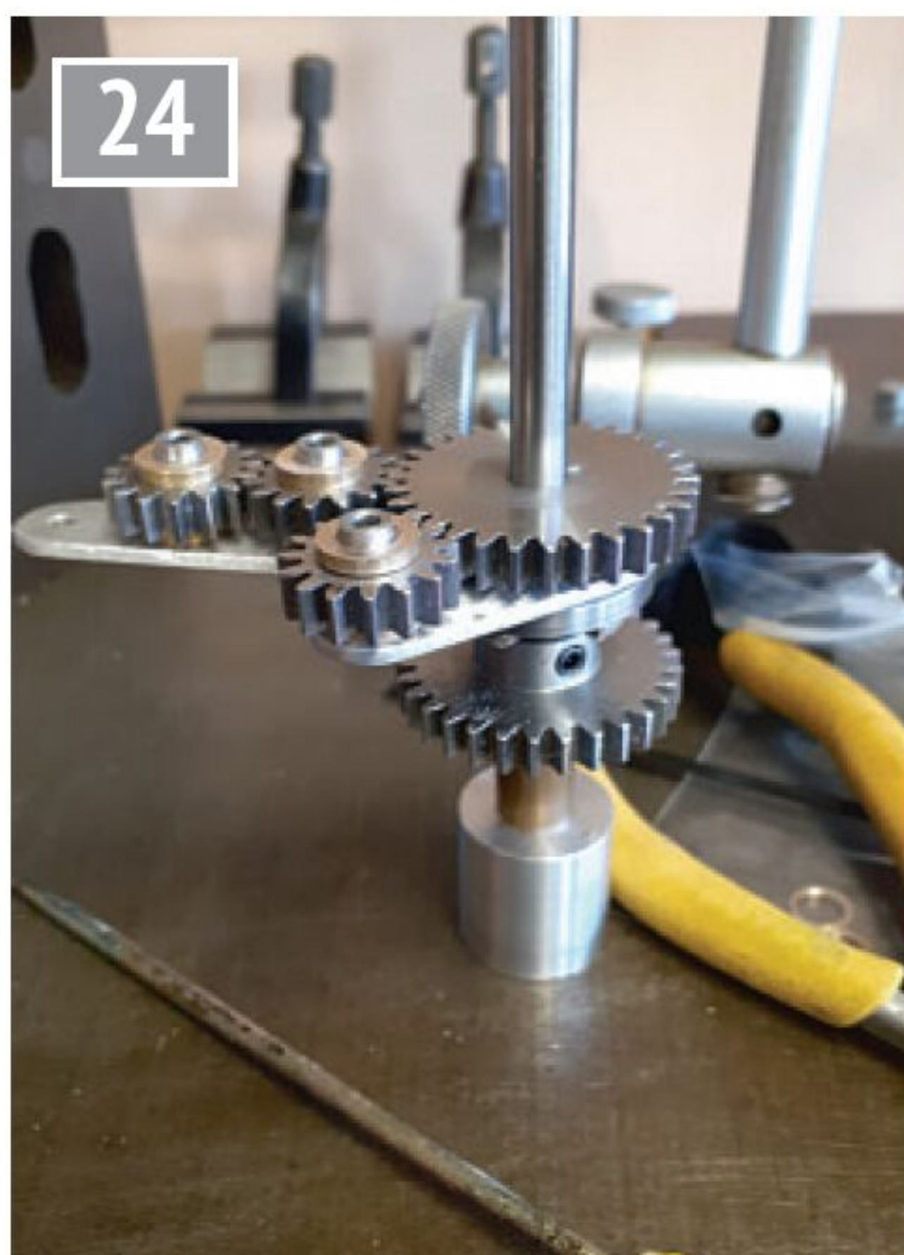
Jackshaft and gears assembled.
