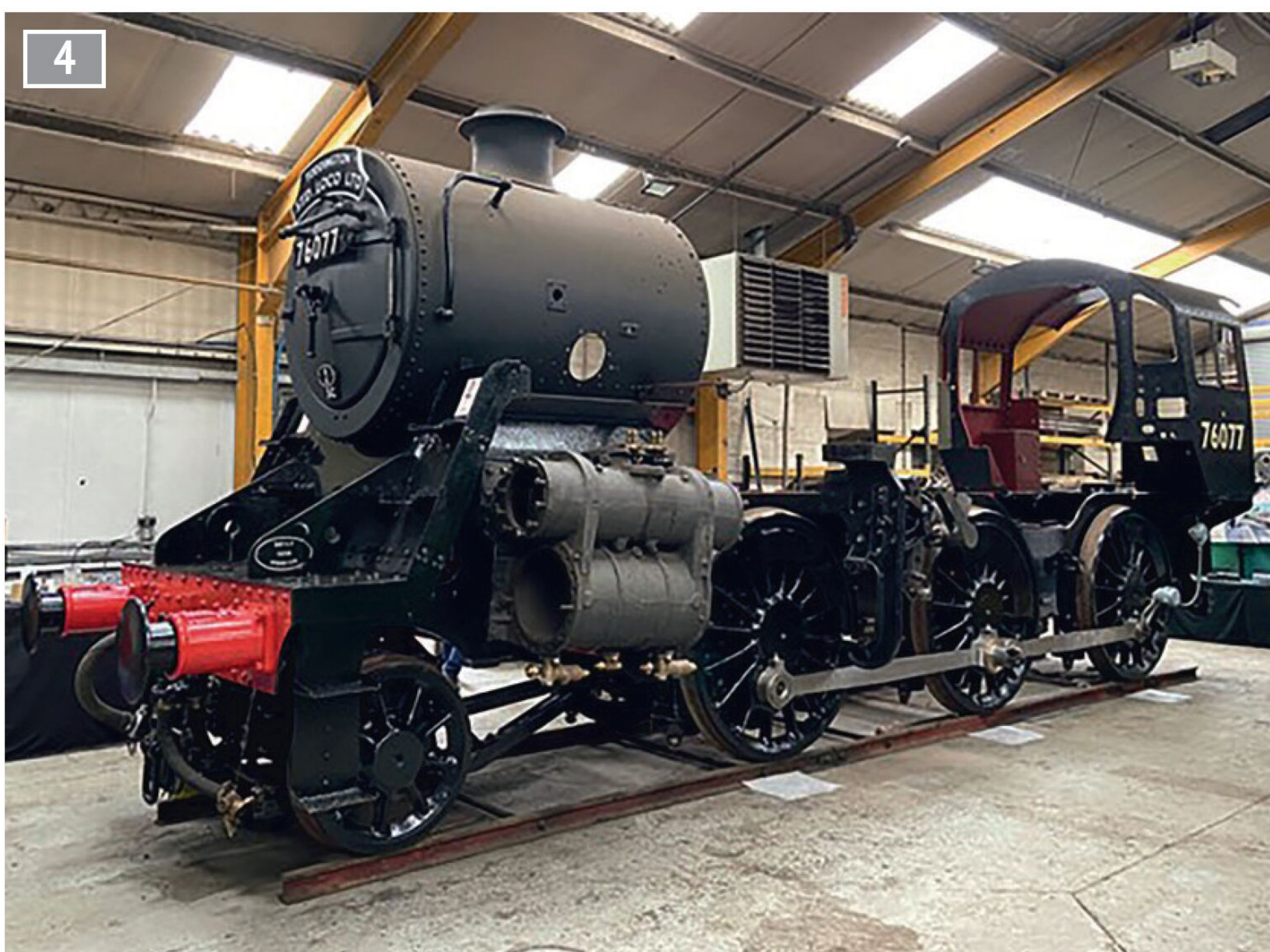
Subject locomotive with a new cab.
