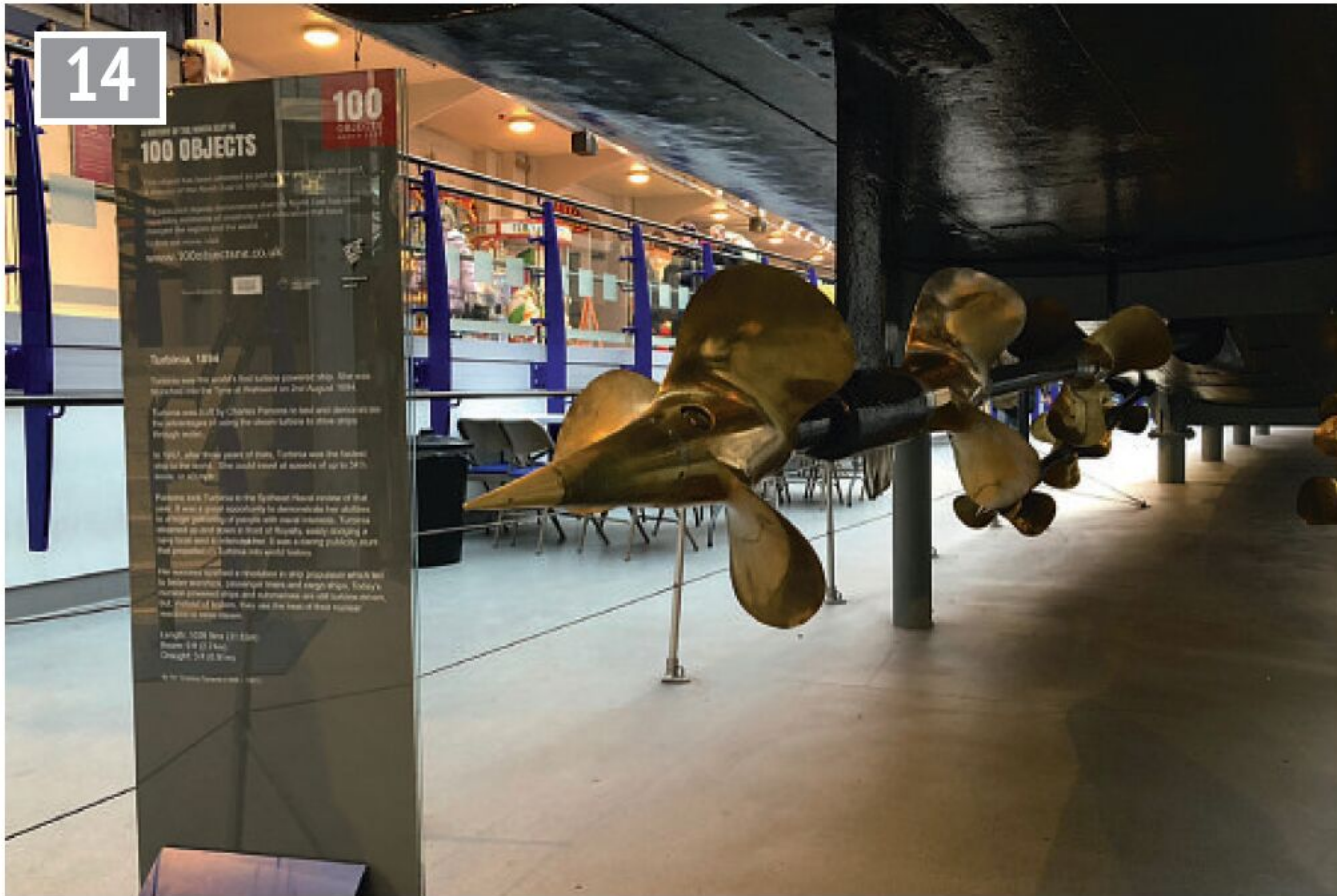
In a later form Turbinia had three propellers on three drive shafts. (© Mike Tilby 2024.)
