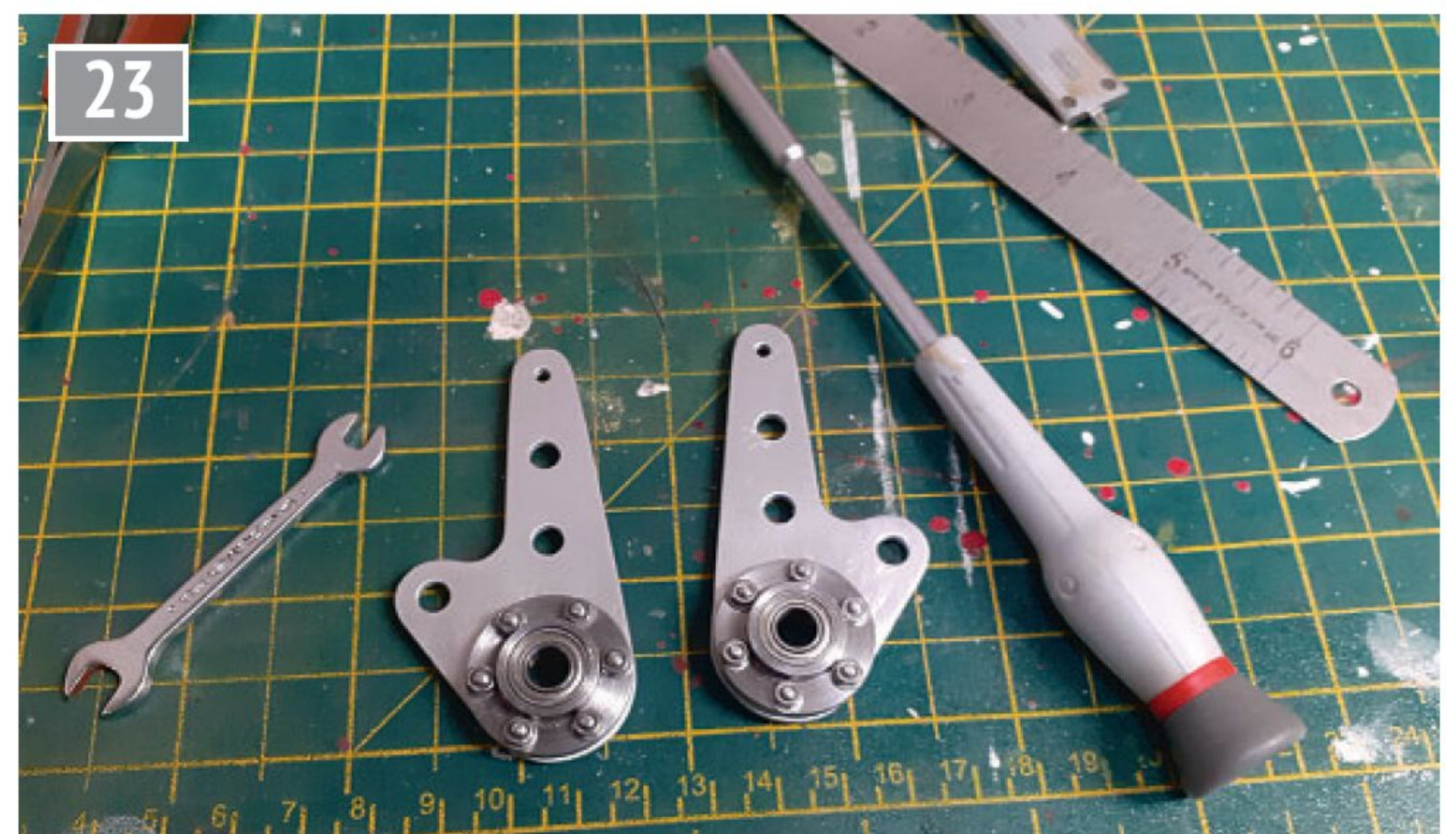
Assembly of forward/reverse tumbler gear yokes.
