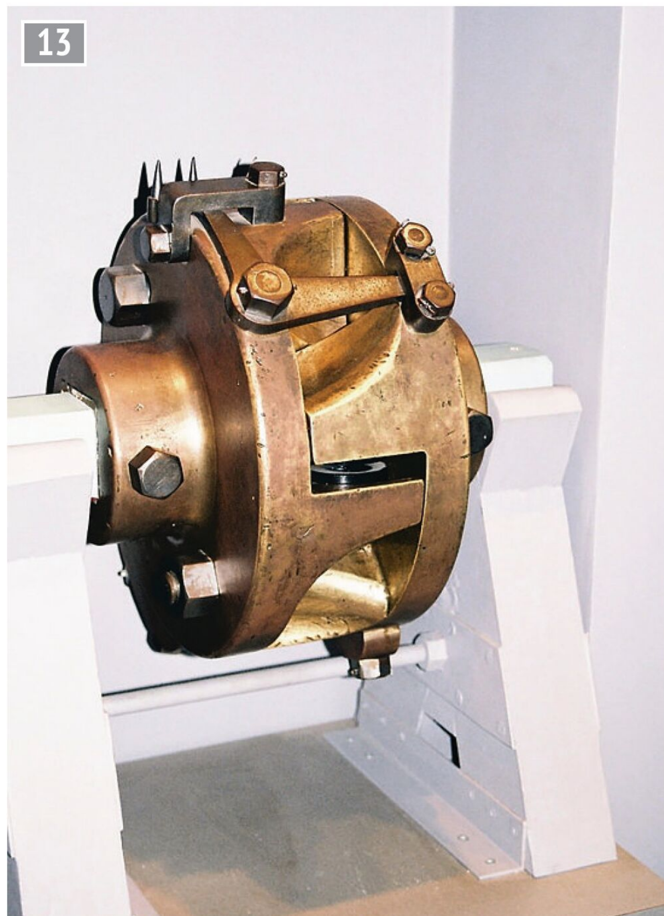
Torsion dynamometer developed by Charles Parsons to help development of his revolutionary steam turbine.
