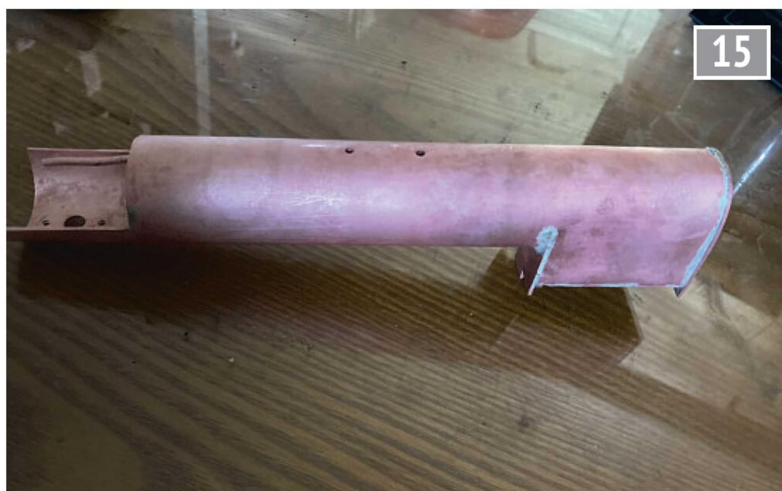
15 The boiler awaiting safety and Goodall bushings to be turned, threaded and soldered on.
