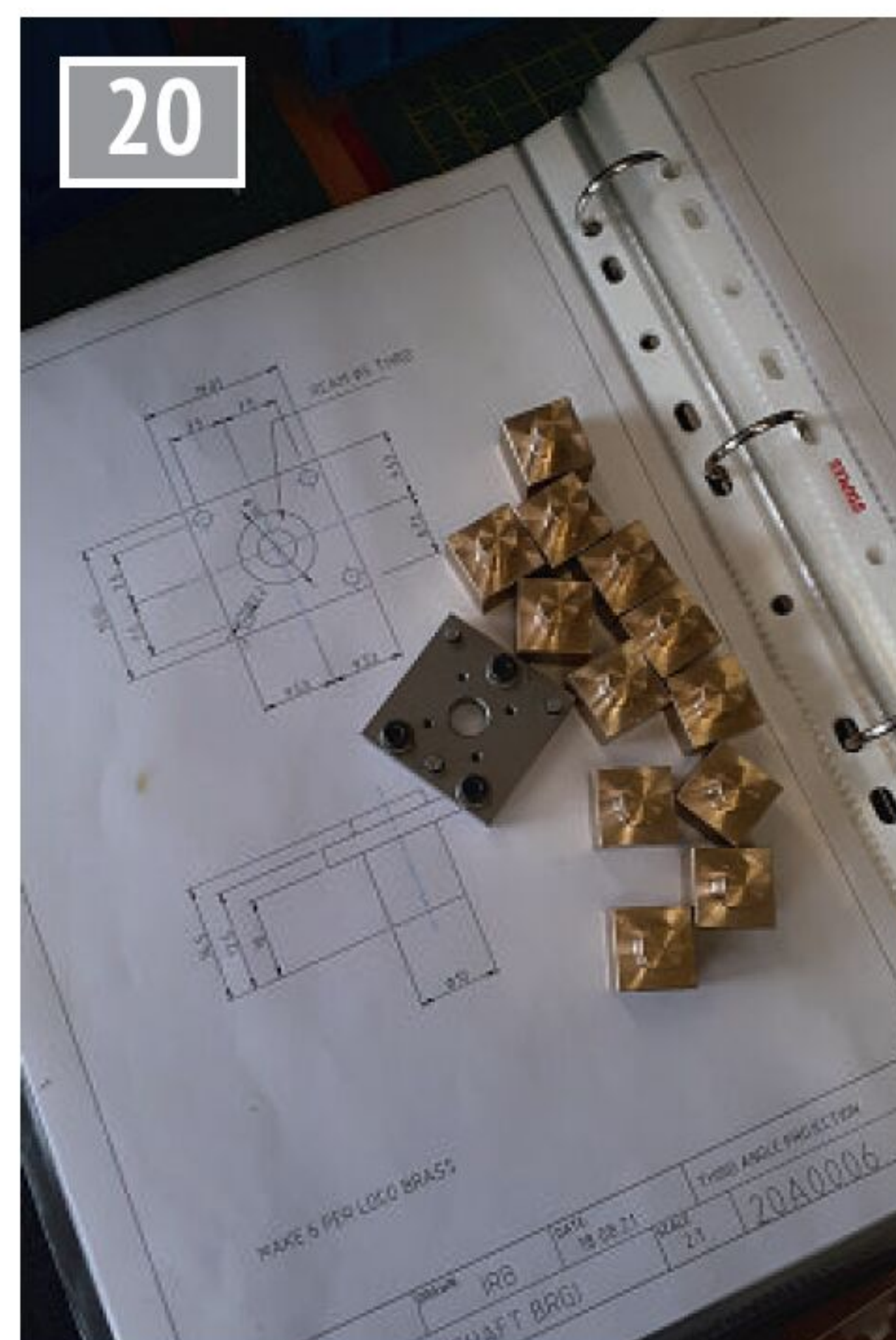
Part finished axle boxes sitting on their project book drawing with drill jig.
