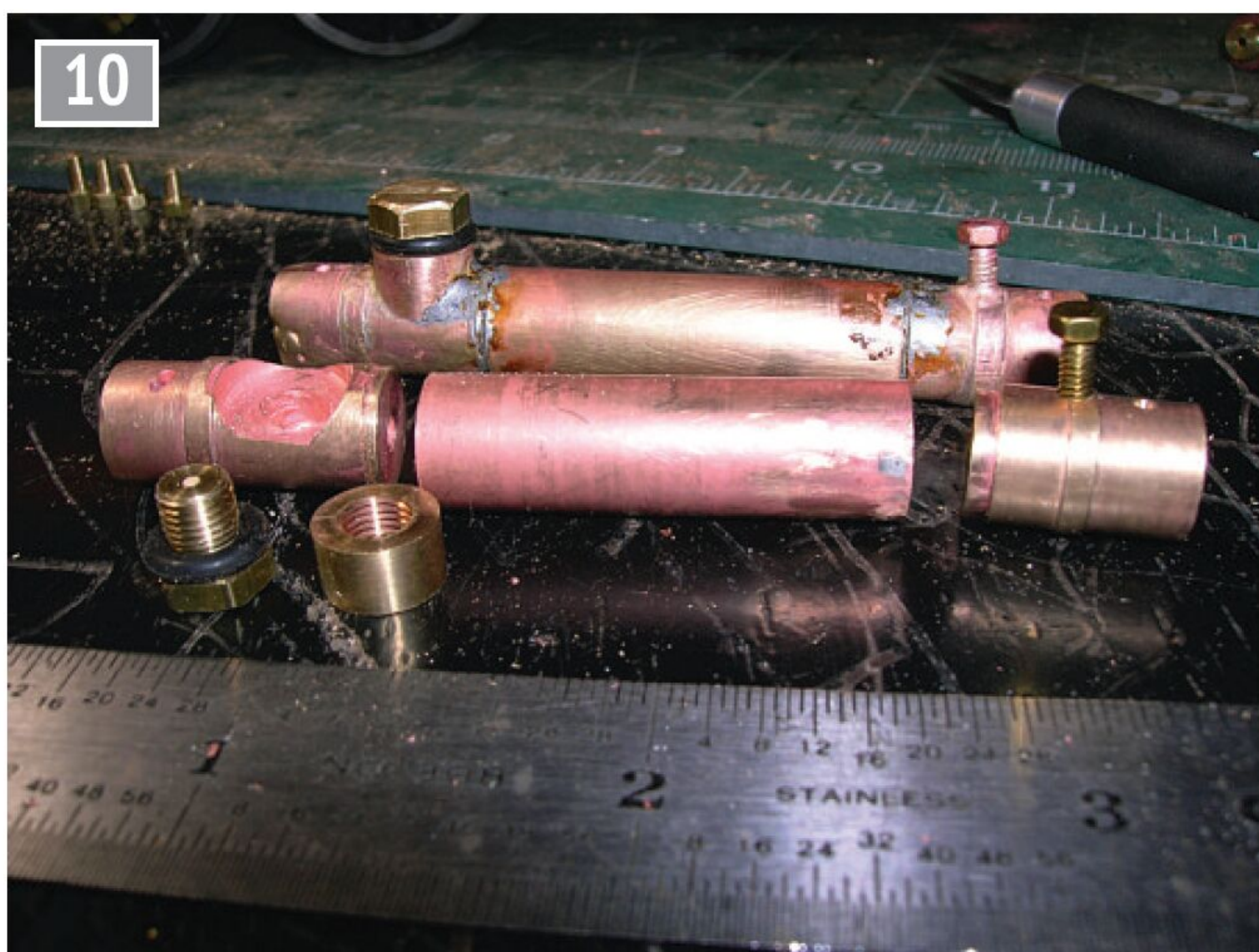
Oil tanks turned on a mini lathe and soft soldered.
