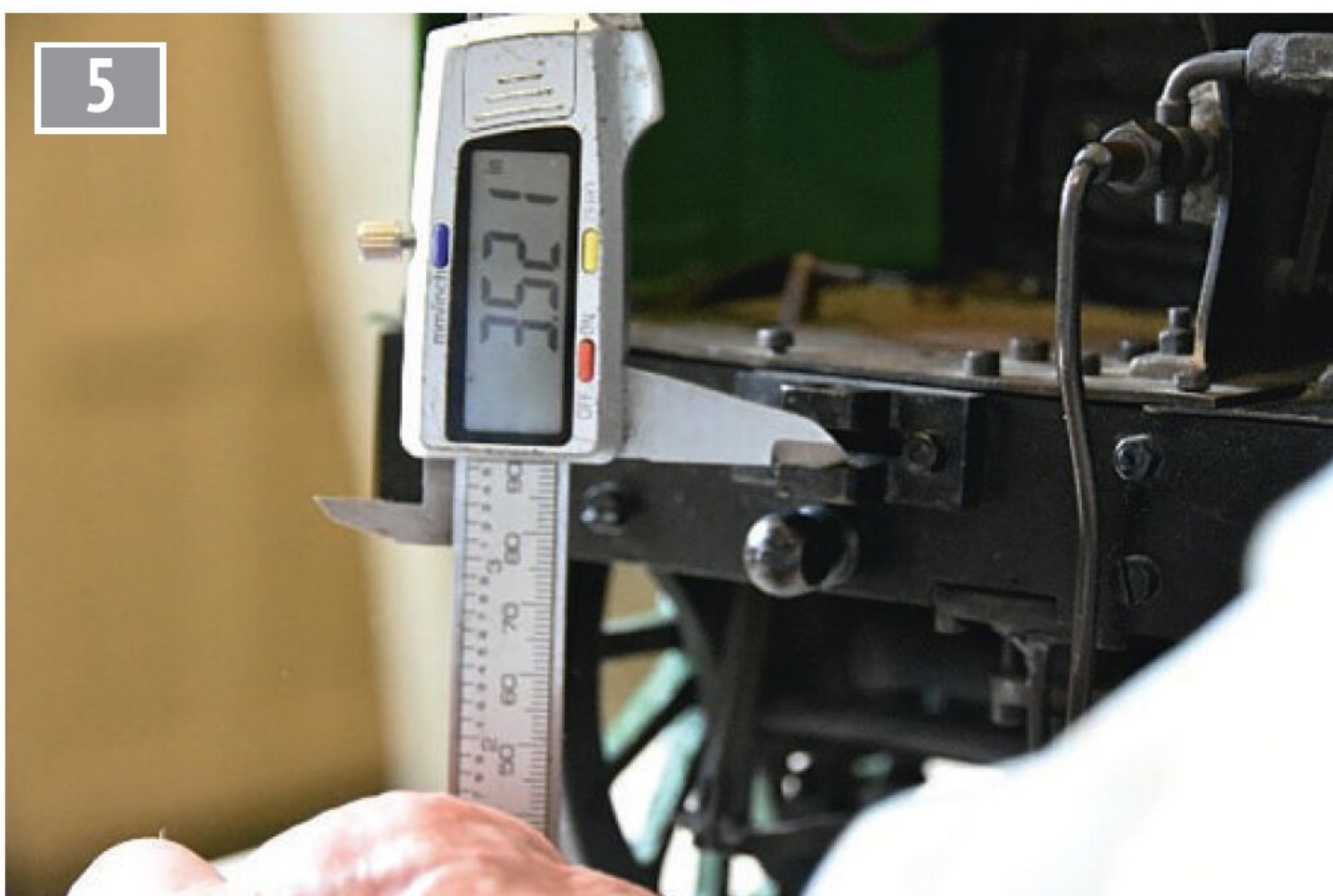
Measuring the locomotive's tender hitch height.
