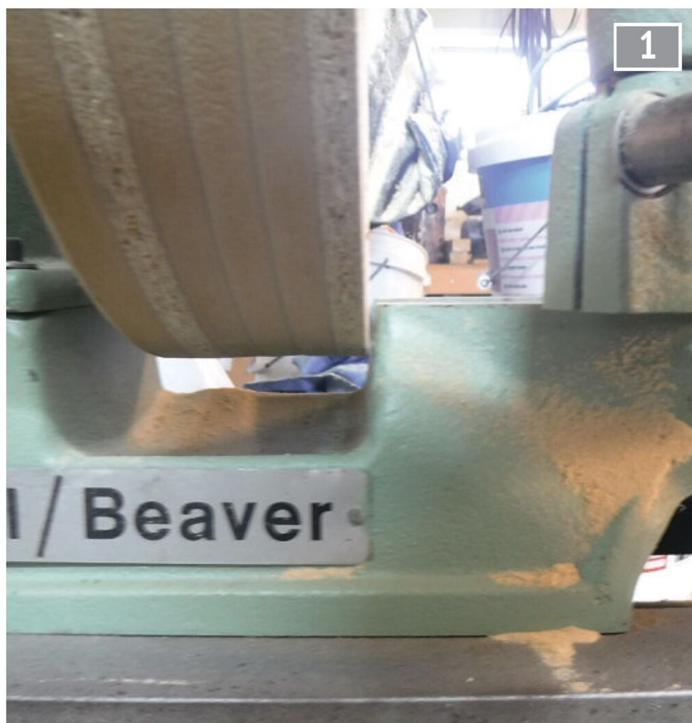
Note the narrow gap between mould and lathe bed.
