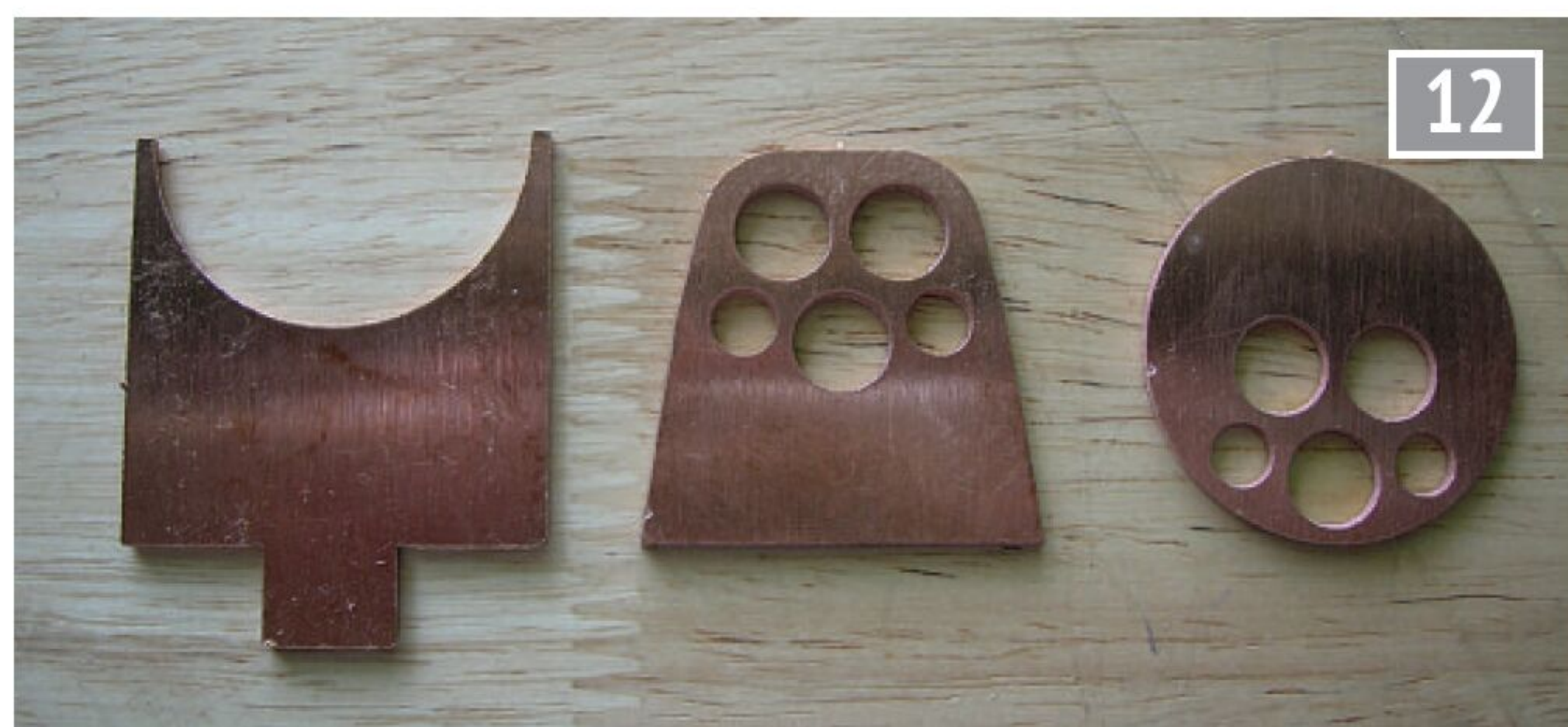
Water jet cut parts are worth every penny and made the second boiler go together faster and much more accurately.
