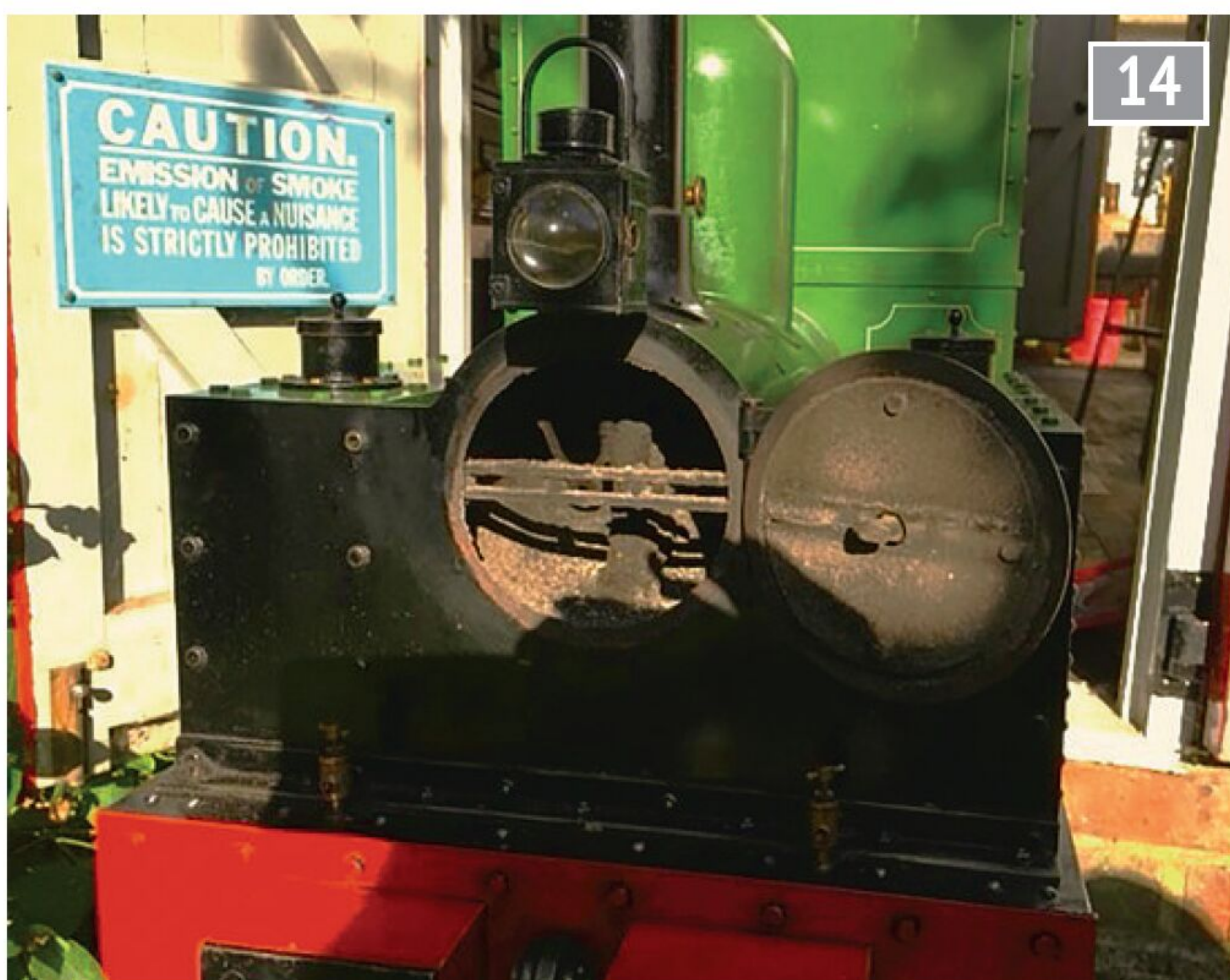
Unused coal and lots of ash needs to be removed, the tanks drained and everything oiled up until its next run.
