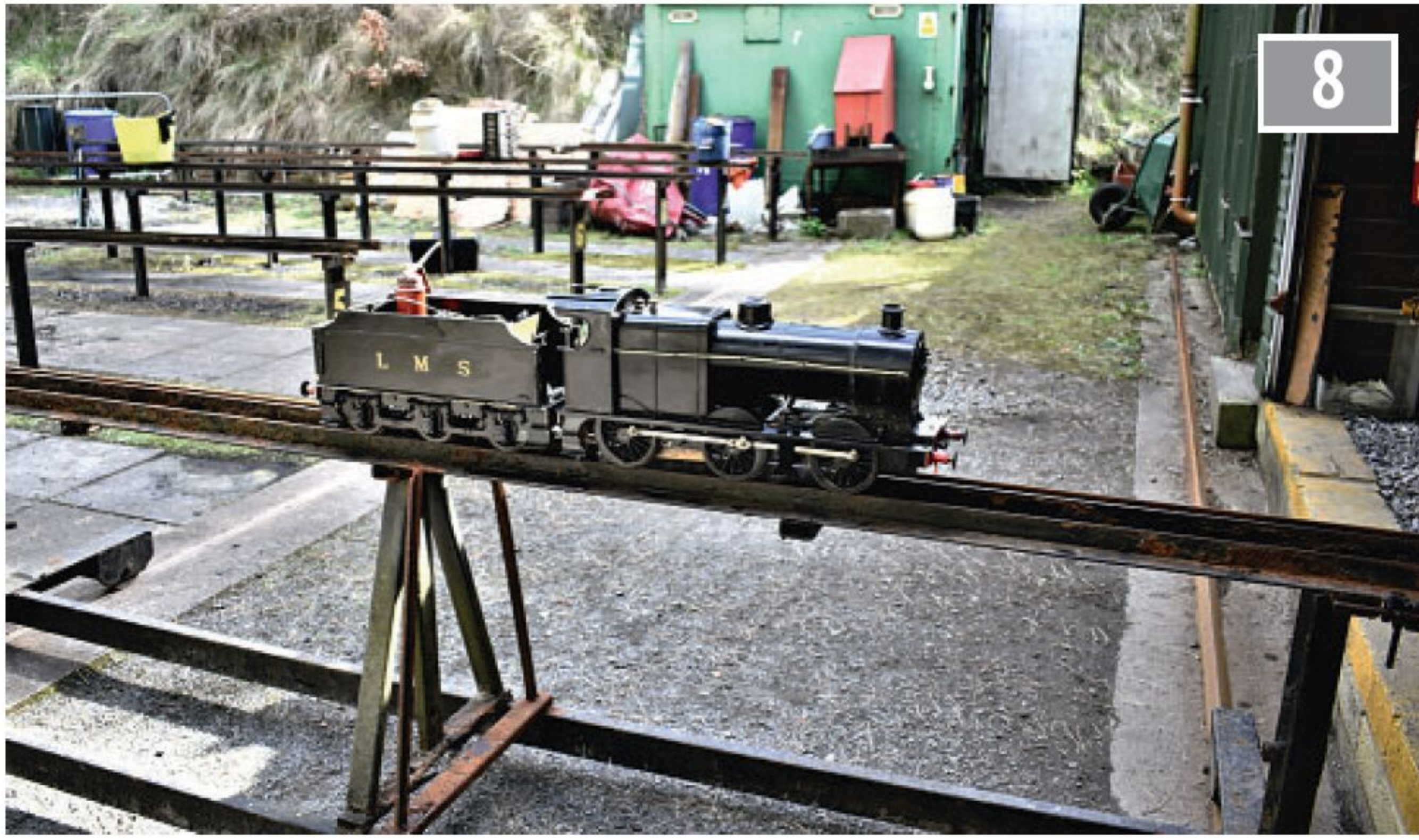
A good length access traverser outside the main storage shed.
