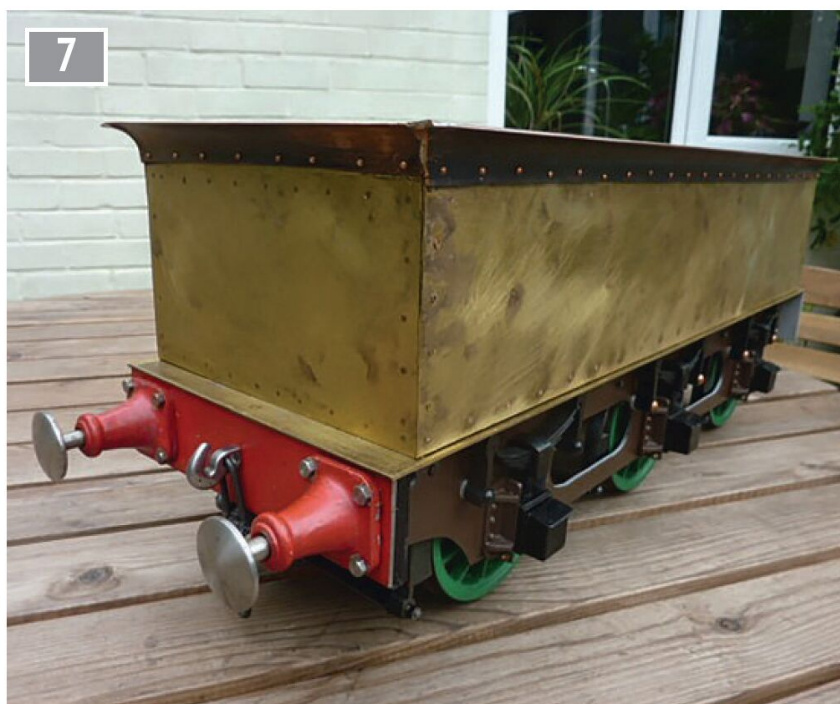
Restored tender chassis united with its new body.
