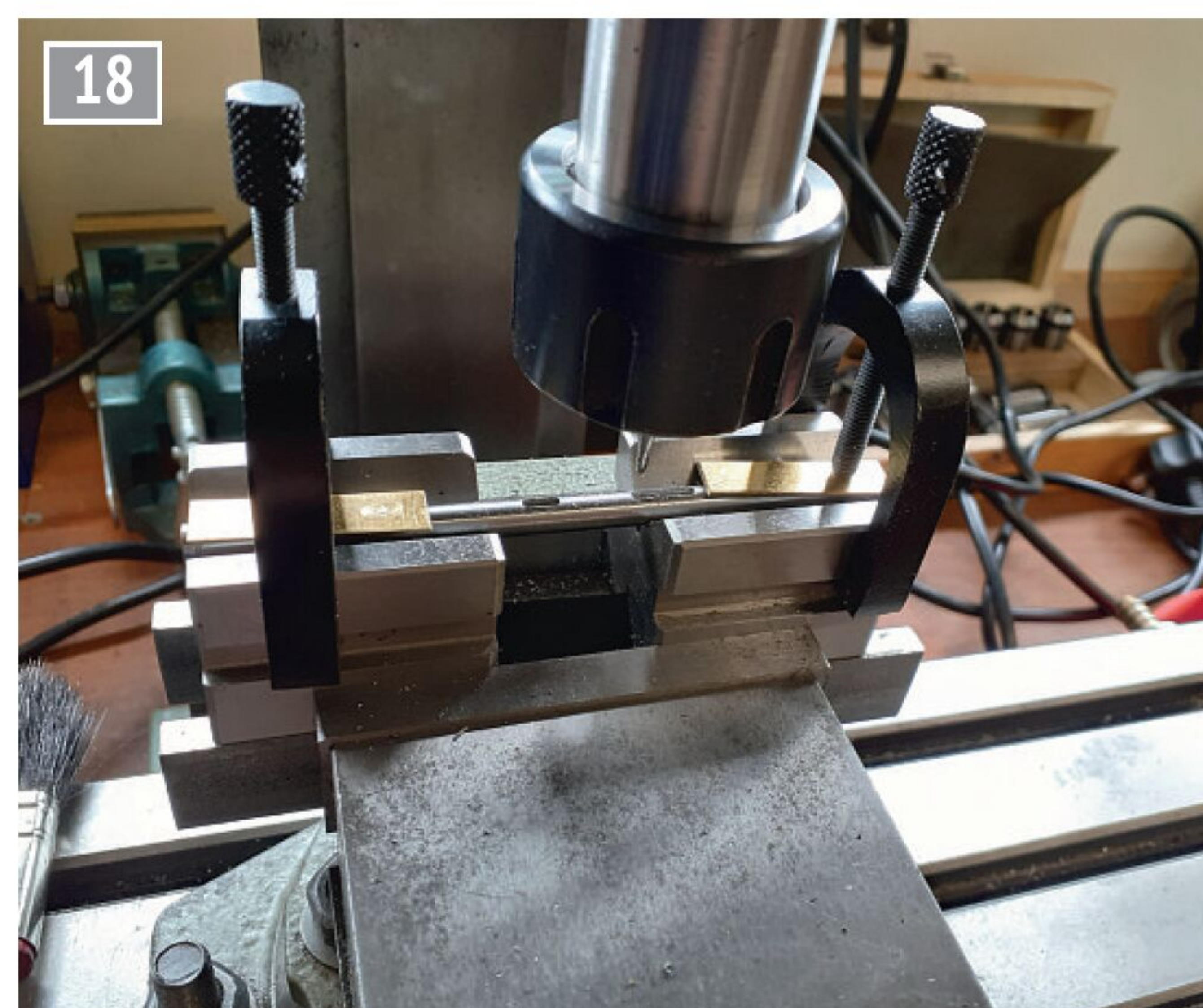
Cutting axle keyways in the first iteration of the model.
