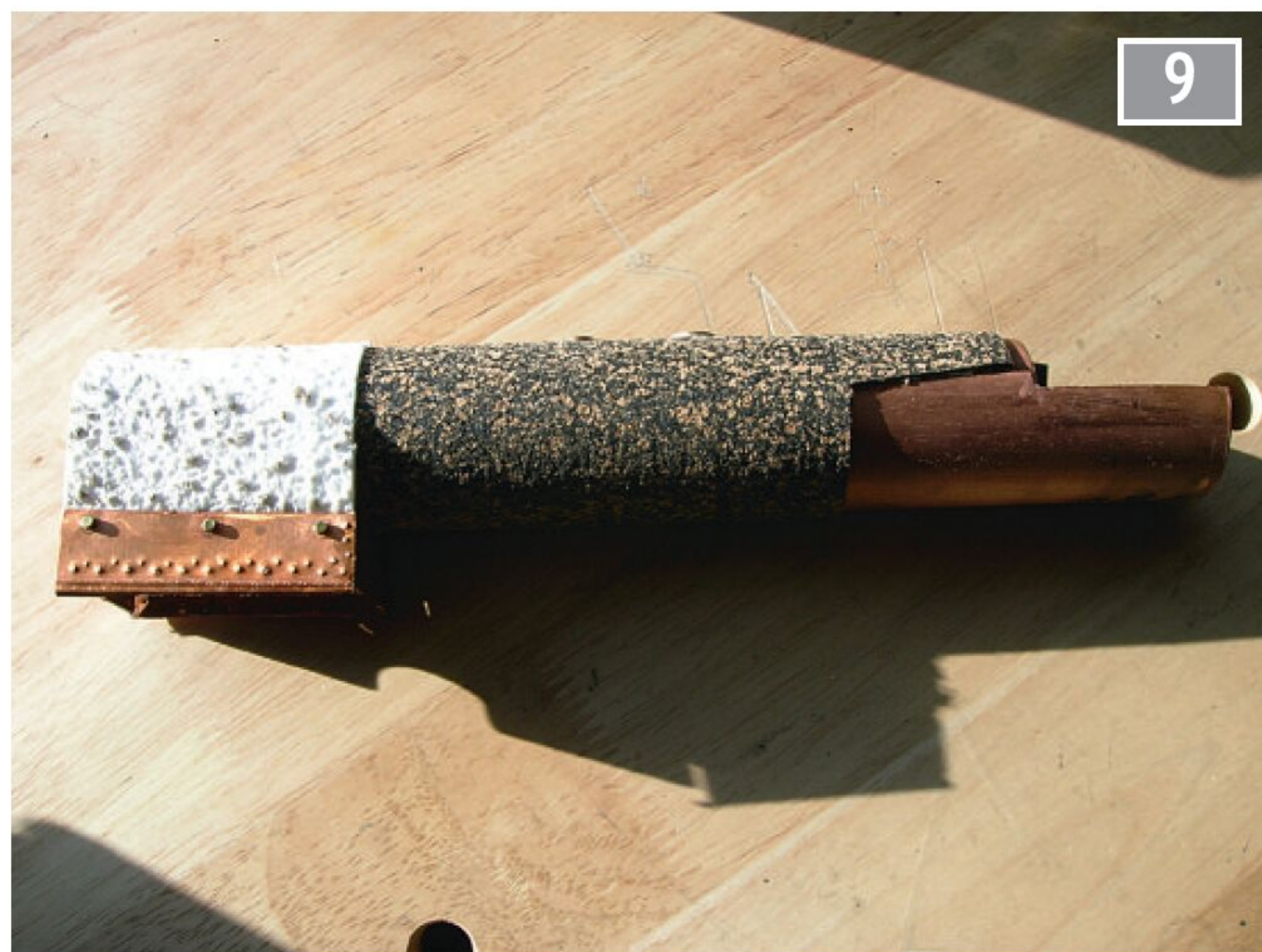
The boiler is insulated with cork in the wet areas and ceramic blanket around the firebox area.
