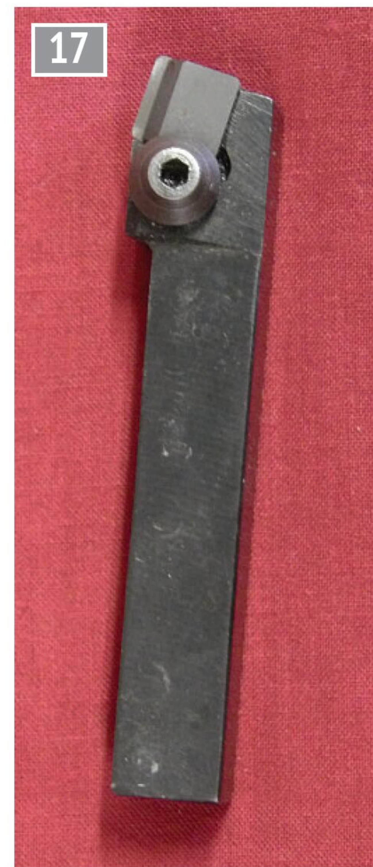
The old tipped bar turning lathe tool explained in the text.
