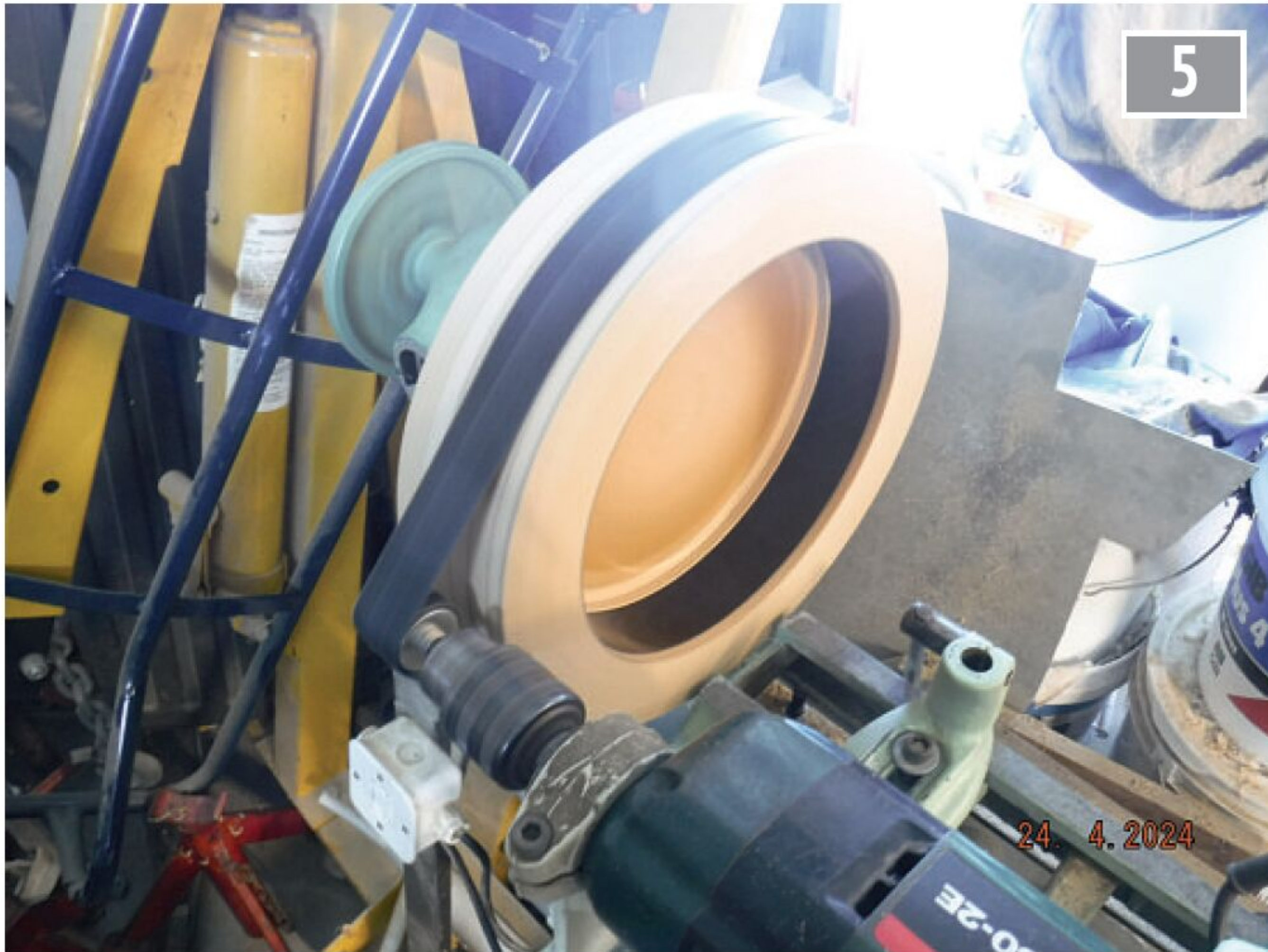
Cast tyre curing in the spinning mould.
