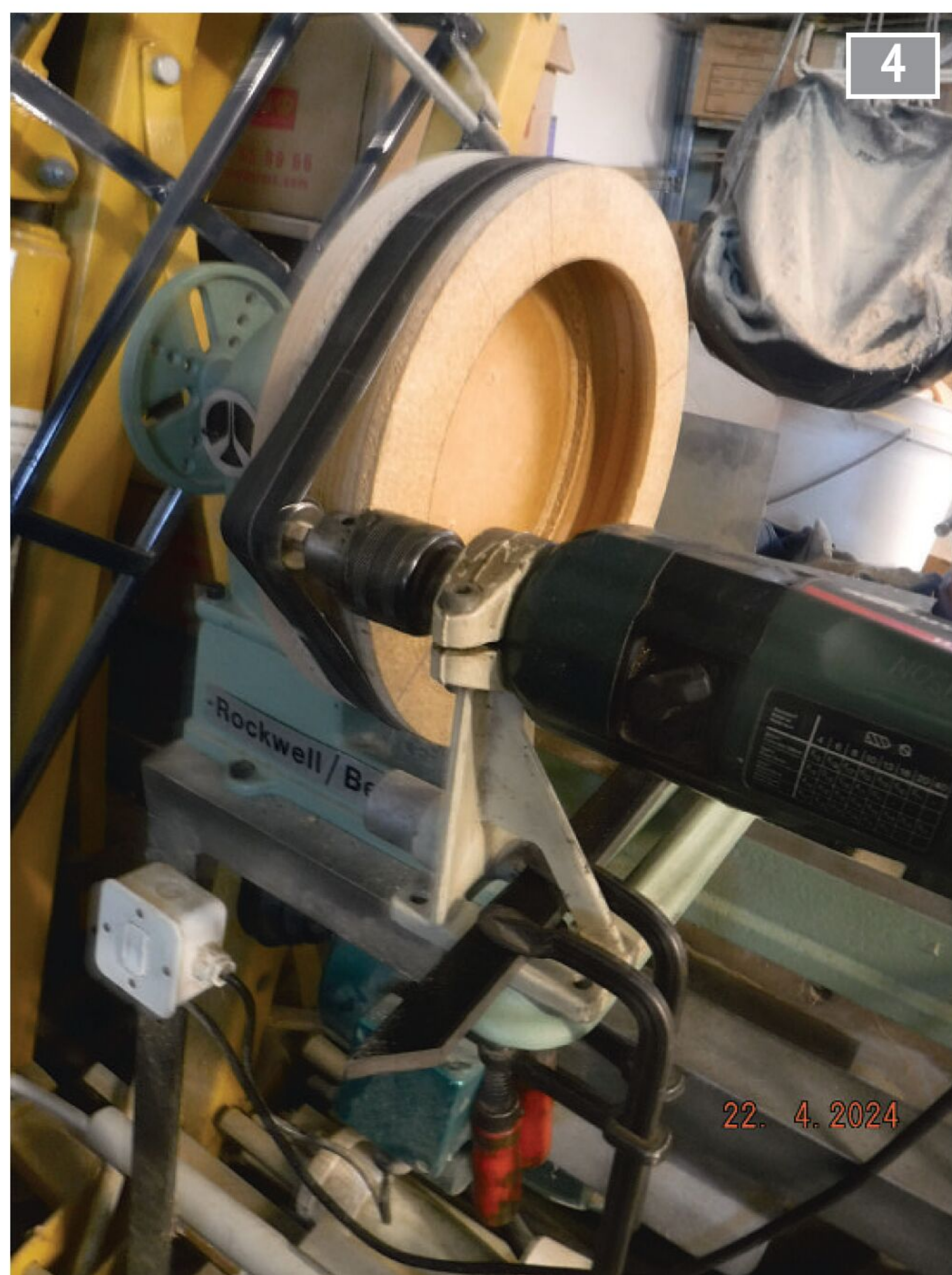
Spinning the mould with belt from bicycle inner tube.
