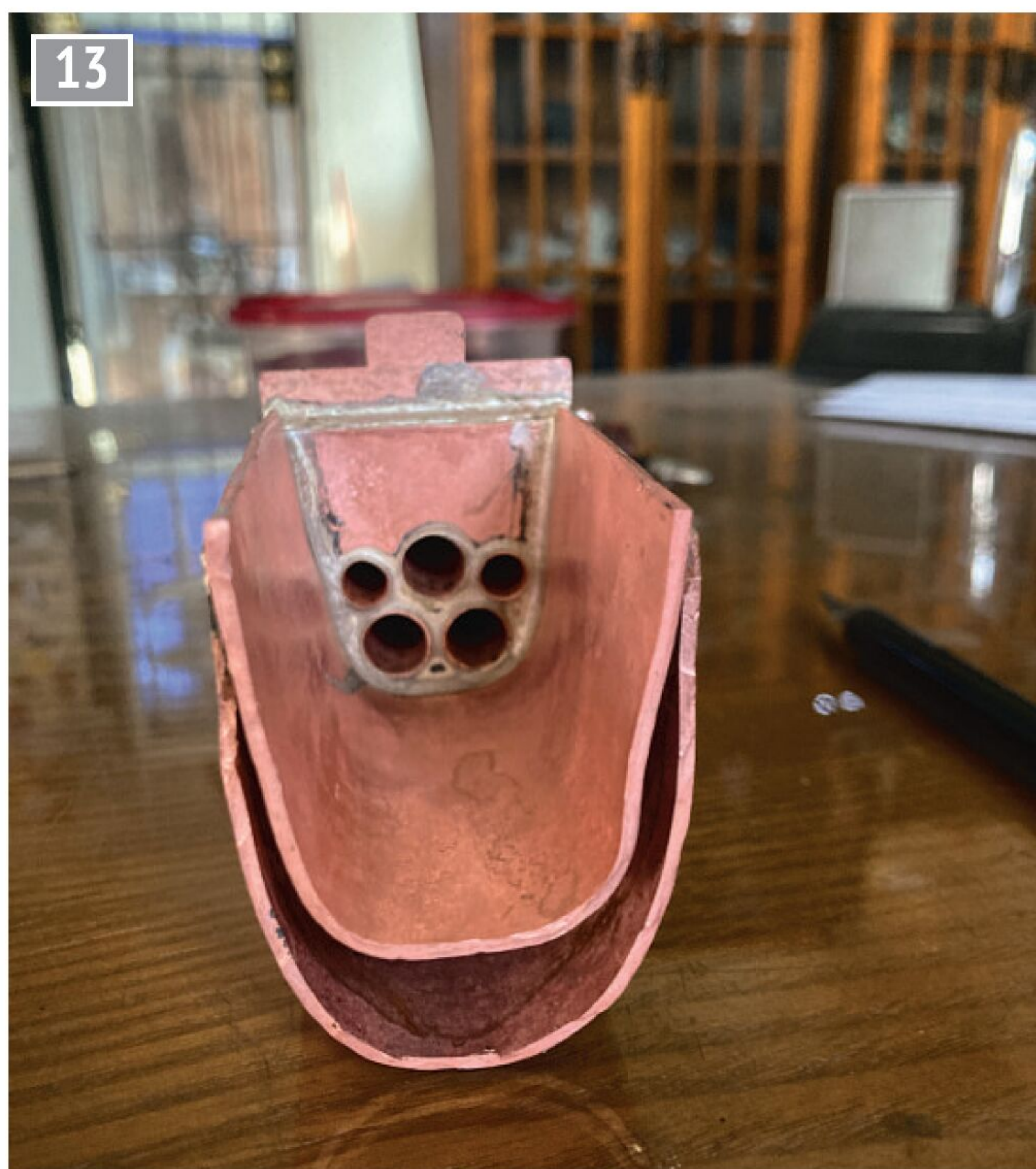
13 New boiler with wet legs. The slanted sides take advantage of the ceramic burner's radiant heating characteristics.
