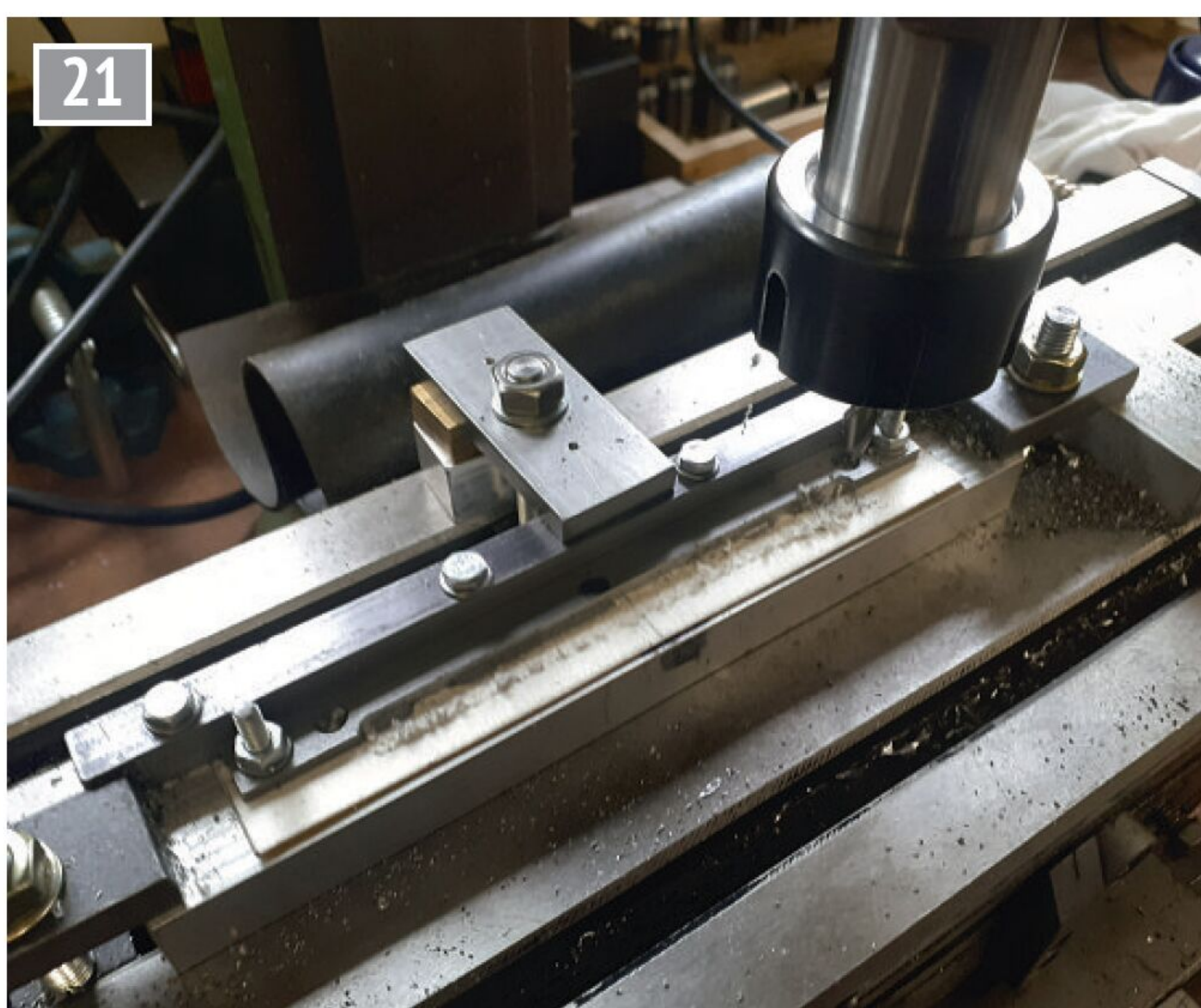
Profiling and drilling coupling rods on the mill. These had been drilled out of 'sync' with the text but proved successful.
