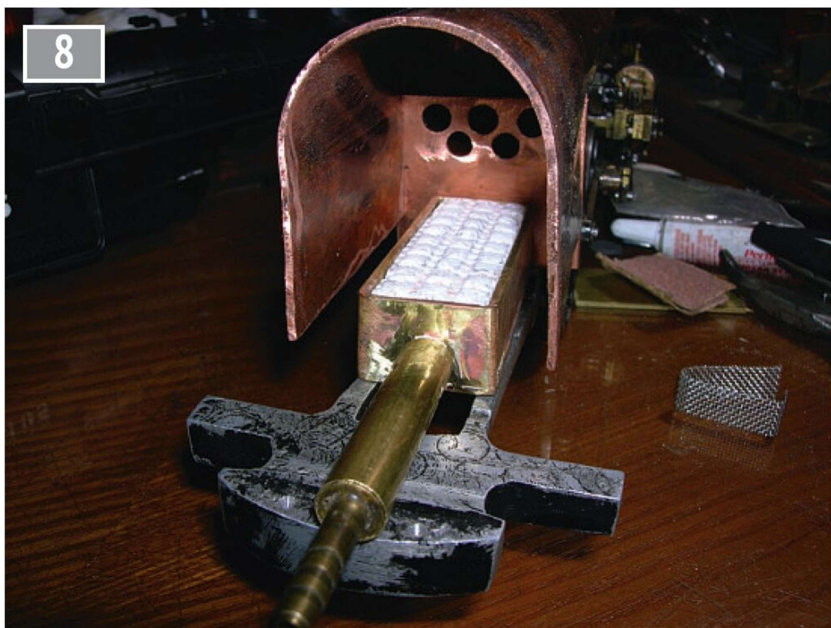
Test fitting the boiler to frame and firebox items which include the throat plate and ceramic burner.
