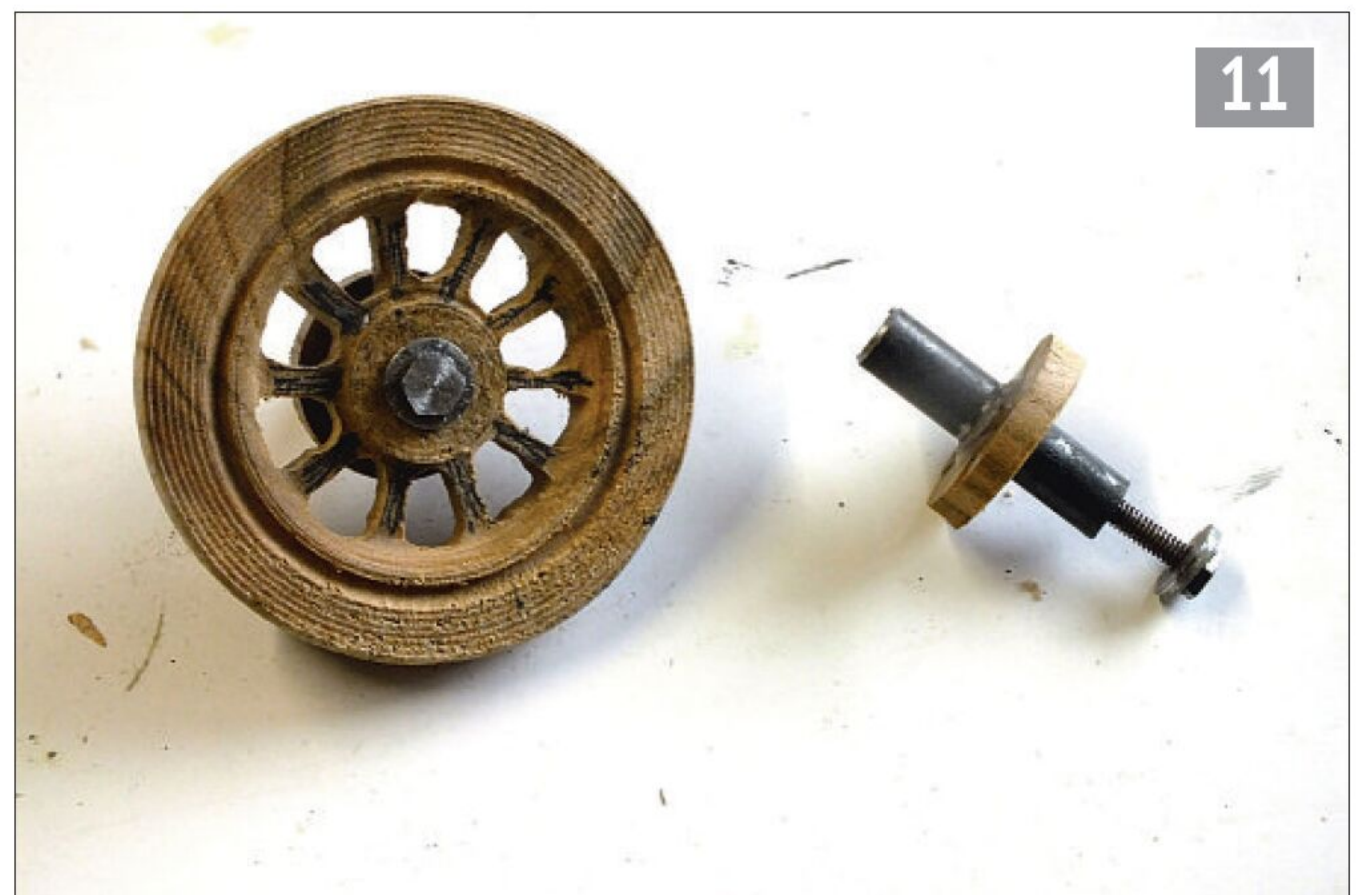
Spokes drilled out and finished by filing.
