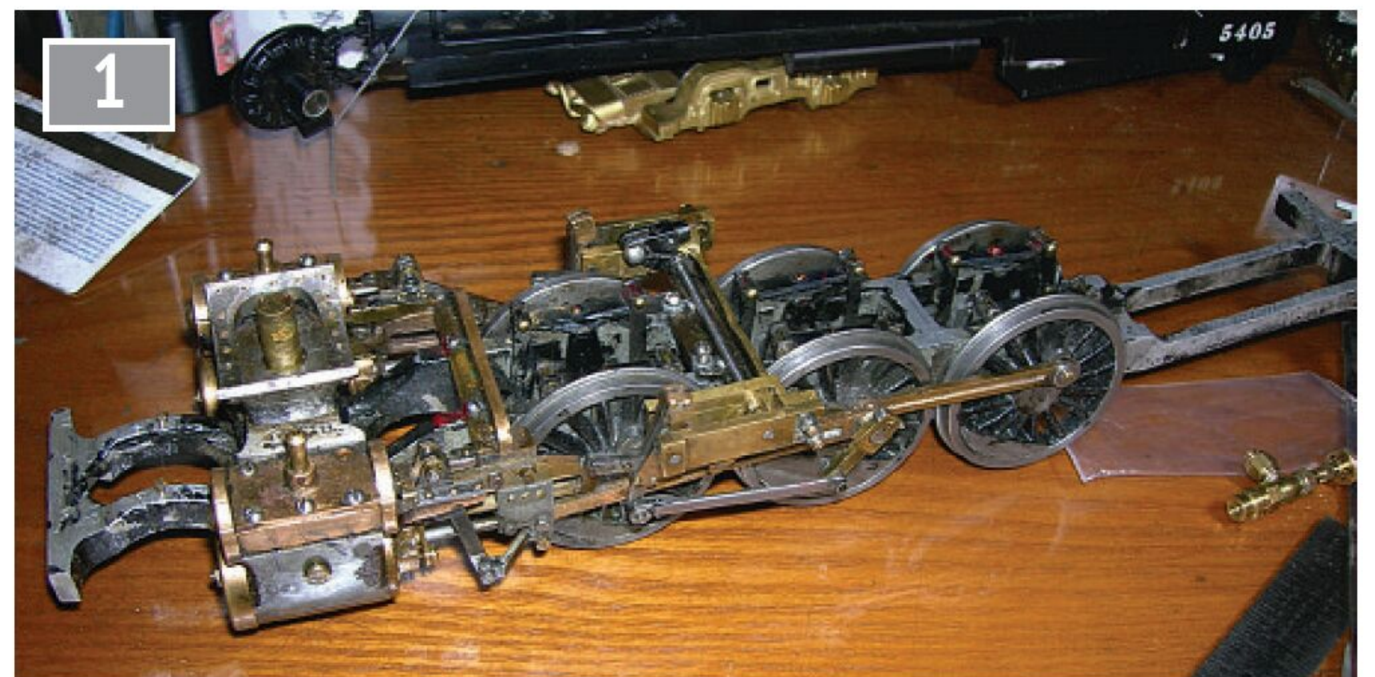
The chassis as received. The radius rods have been removed, awaiting installation of the slightly longer rods. The Williams brass shell is in the background.
