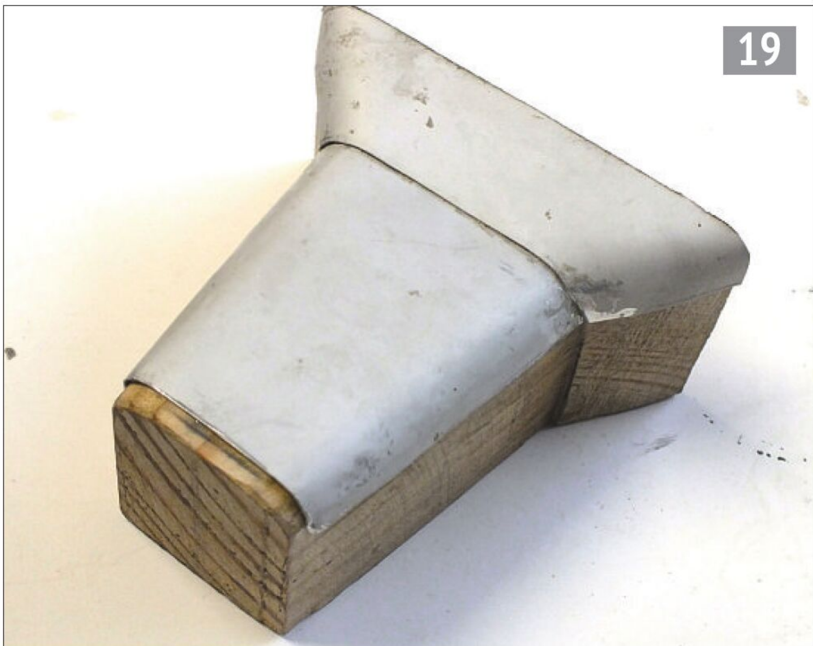
Aluminium bonnet and scuttle shaped over a former.
