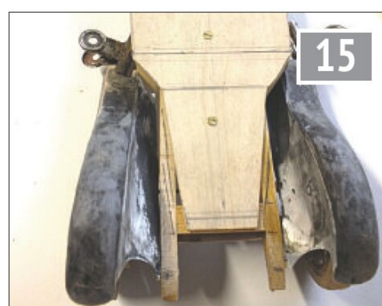
Mudguards are made from ply and aluminium.
