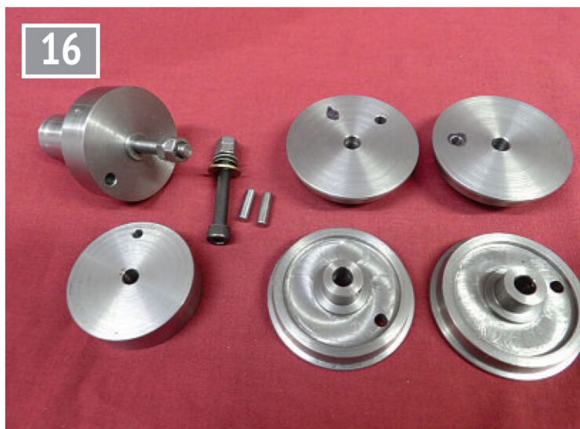
A completed wheel set with the tooling made for the job.
