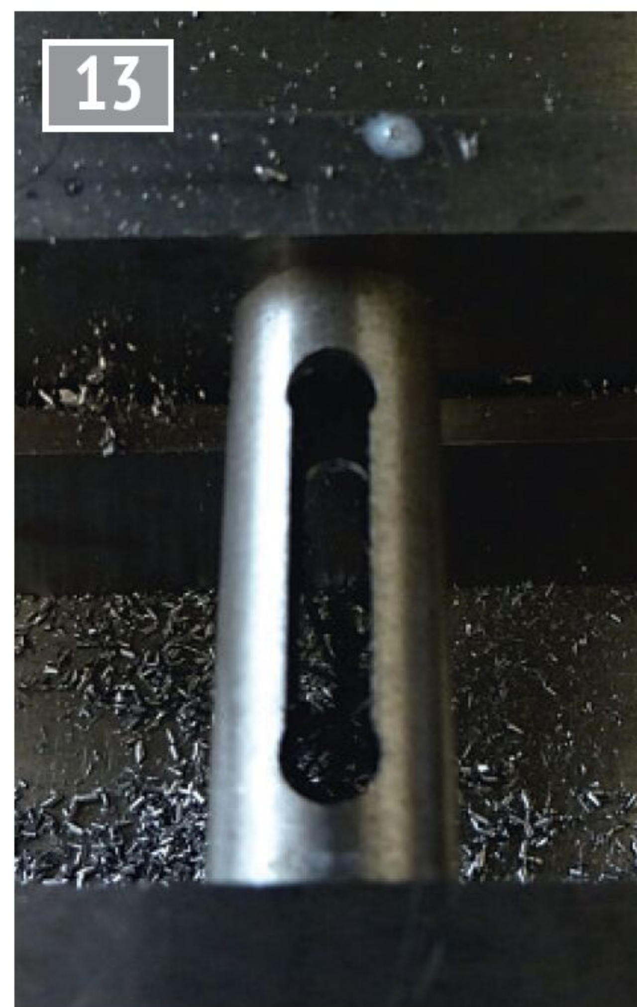
Trunk guide slot ends drilled and central slot milled.
