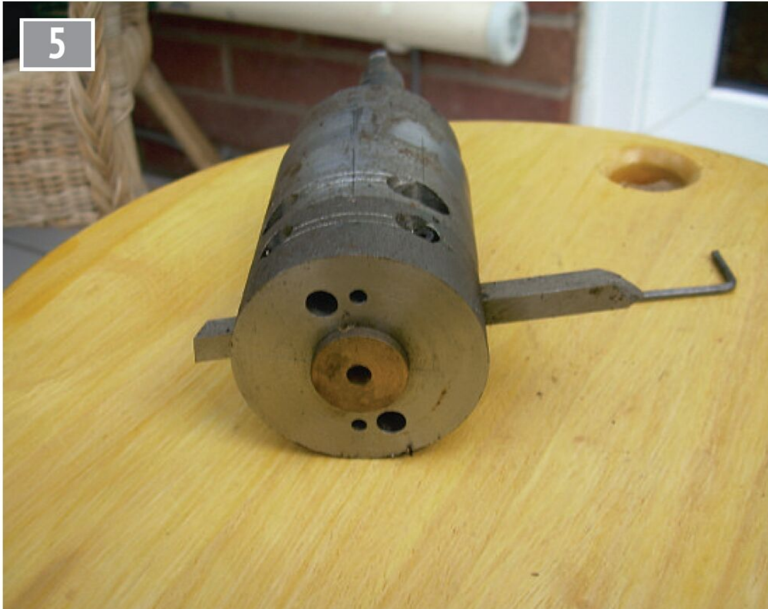
The cap. Showing one of the steady bushes in place; the larger of the two pairs of holes are to take the heads of Allen cap screws, the smaller ones are the dowel holes.
