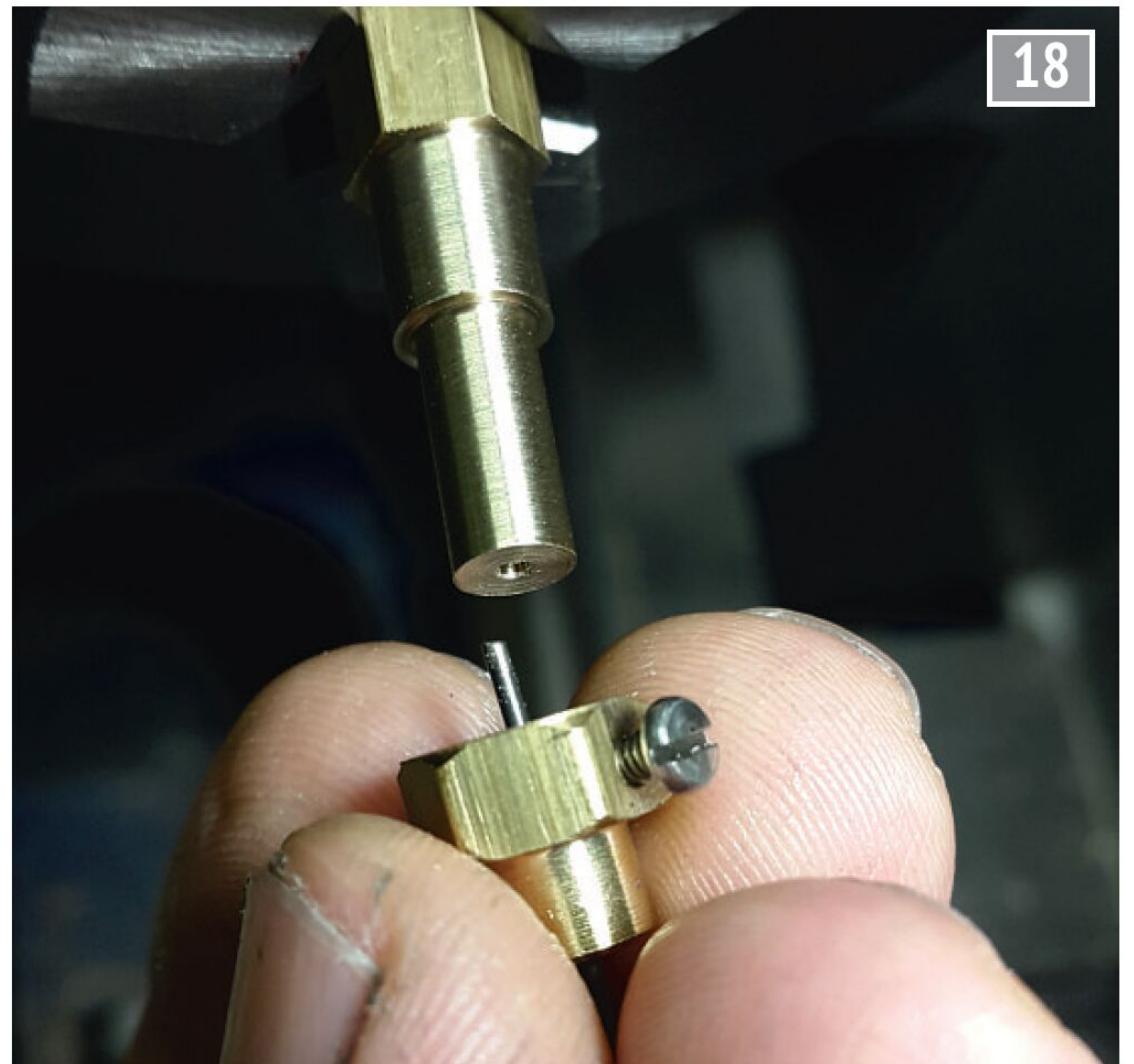
All cone depths on my injector designs are measured using a 1mm drill 'depth gauge' to check for proper taper length and assembly depth. This takes away any tolerance issues with using multiple gauges and standardizes on the measurements.
