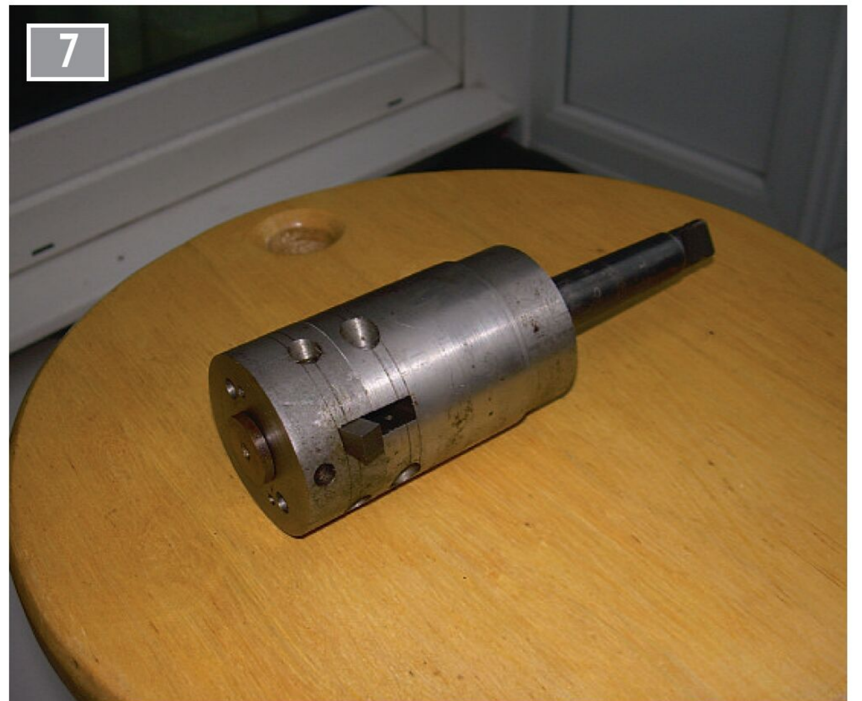
The unit. Showing the disused tool bit slot in the body – useful as it allows the swarf to clear. The single hole in front of the tool bit is for a screw to clamp the brass guide bush but I haven't had need to use it.
