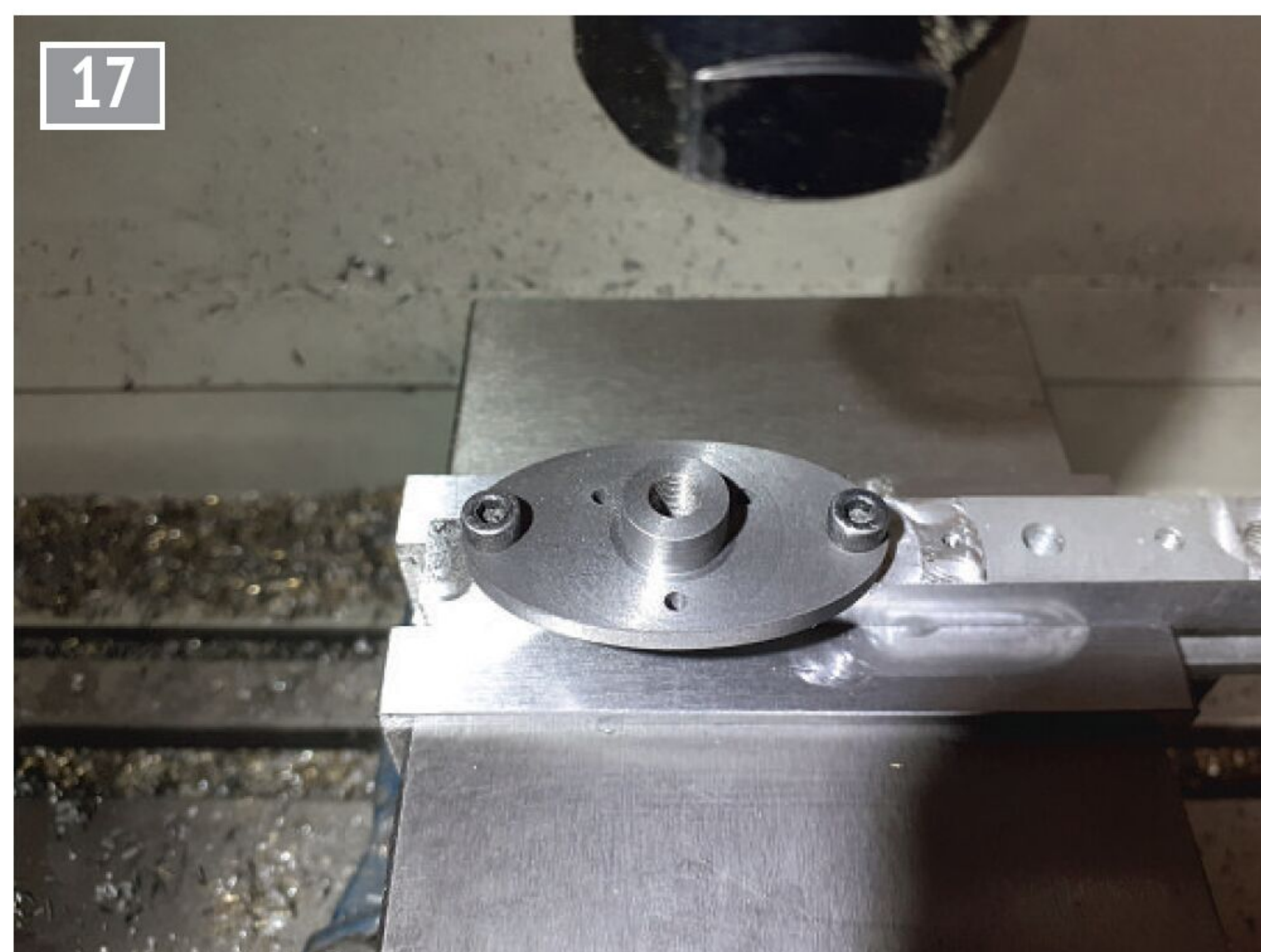
Profiling bottom cover.
