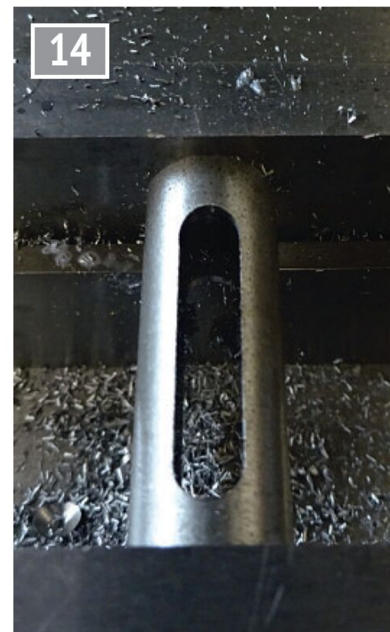
Slot widened to 5mm.
