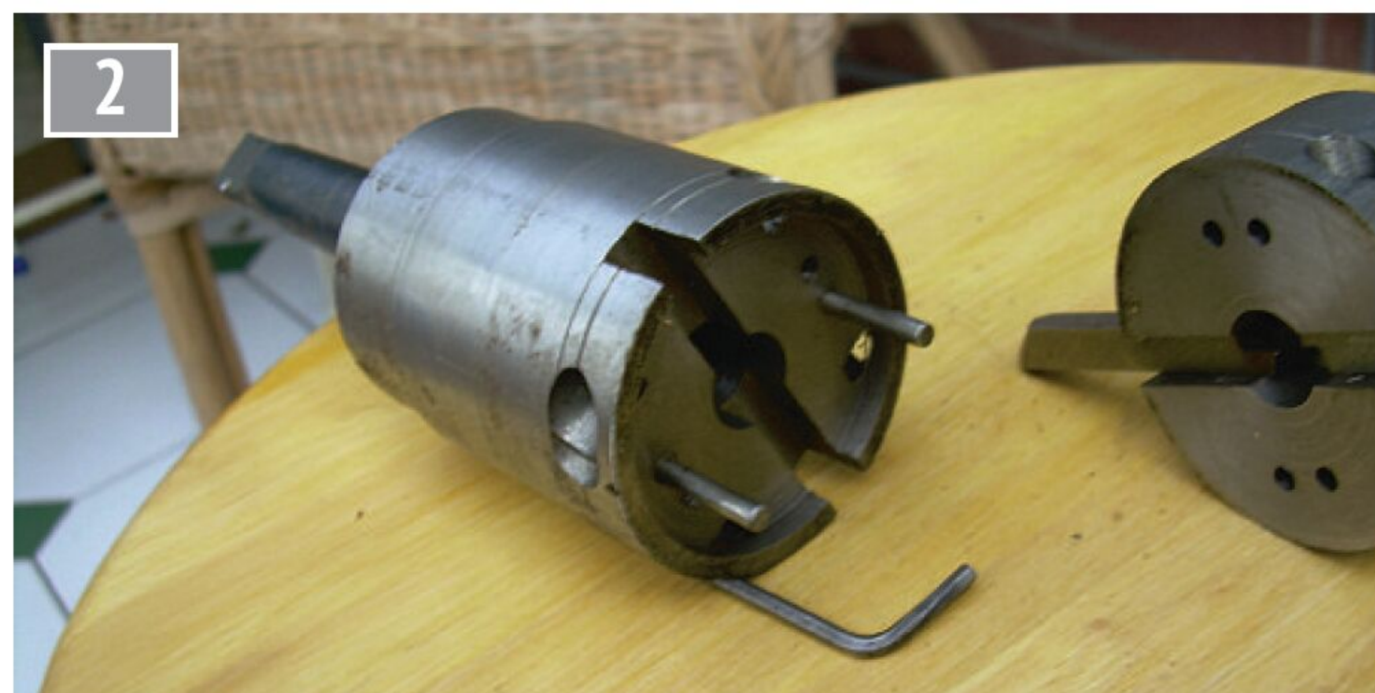
Cap and body. The slot and tool locking screw holes are where I changed my mind. After I'd cut/drilled these it dawned of me that if I put the tool bits in the cap I could set them so much more easily. The two dowel pins are shown.
