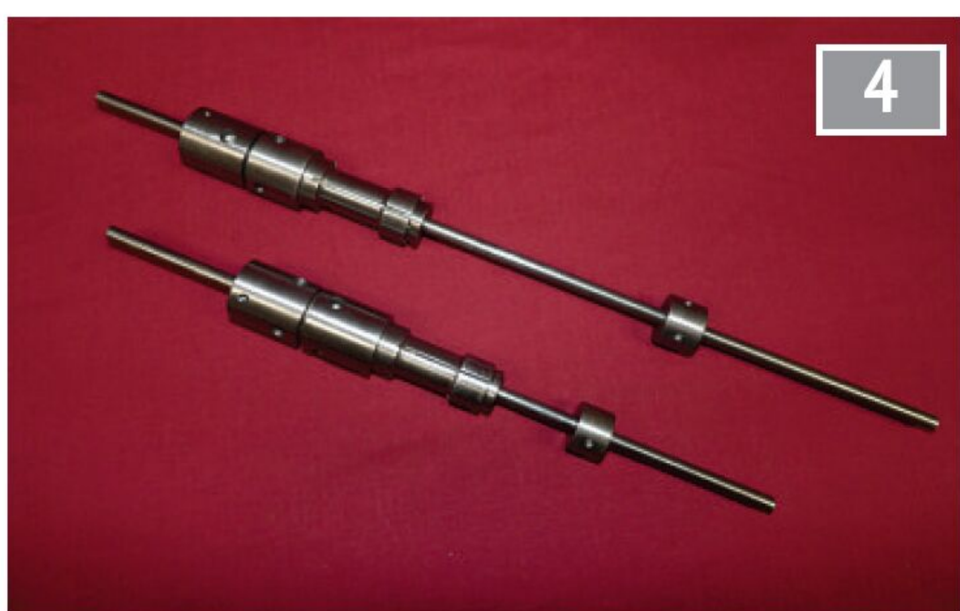
Lathe mandrel back stops to Harold Hall basic design.
