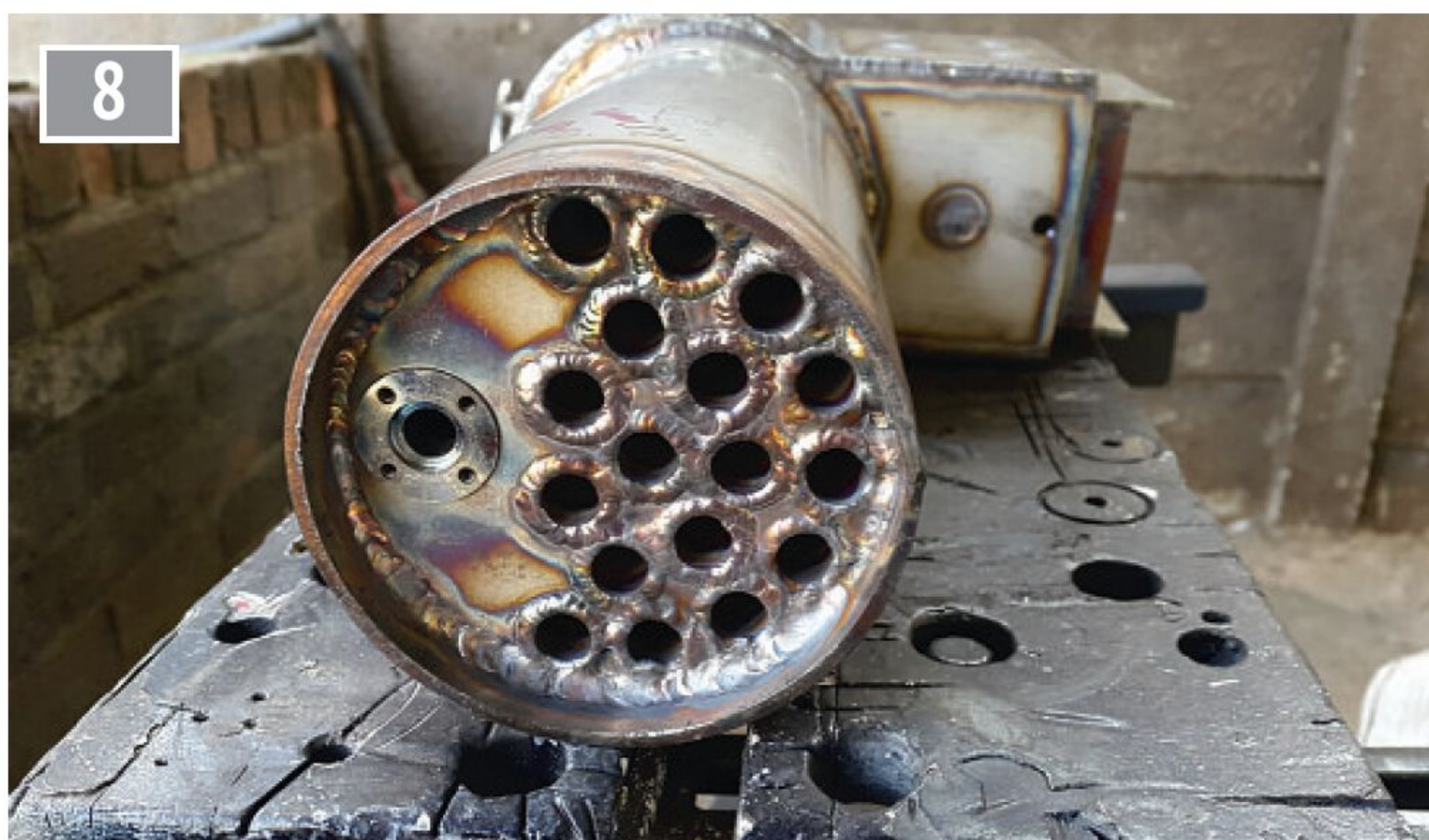
A stainless steel boiler specifically designed for a live steam model.
