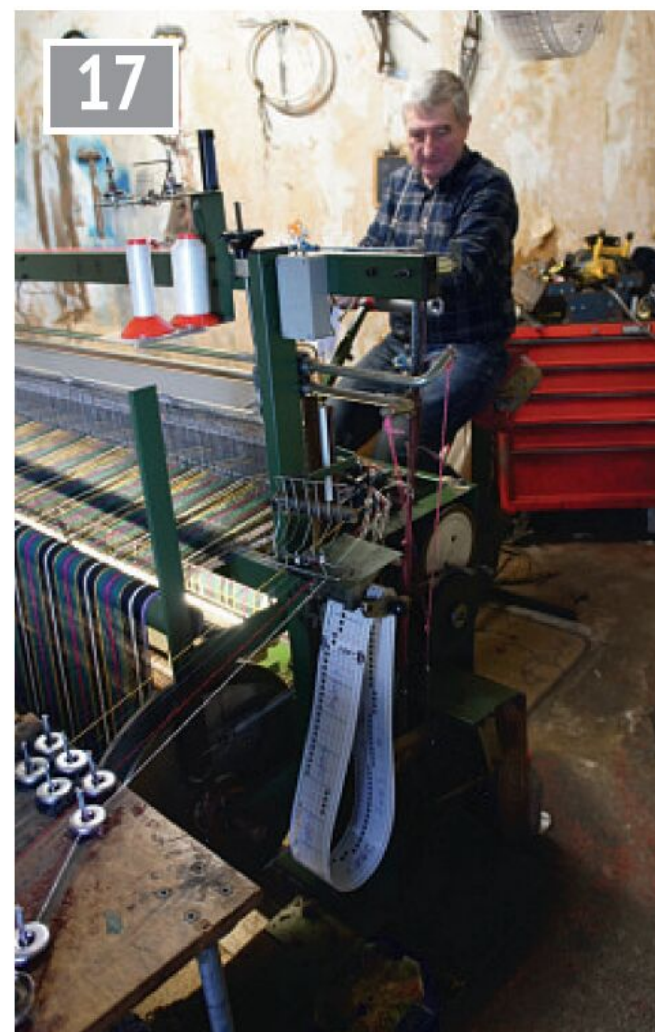
17 Another view of the controlling punched tape. White bobbins above carry a nylon thread to make a selvage.
