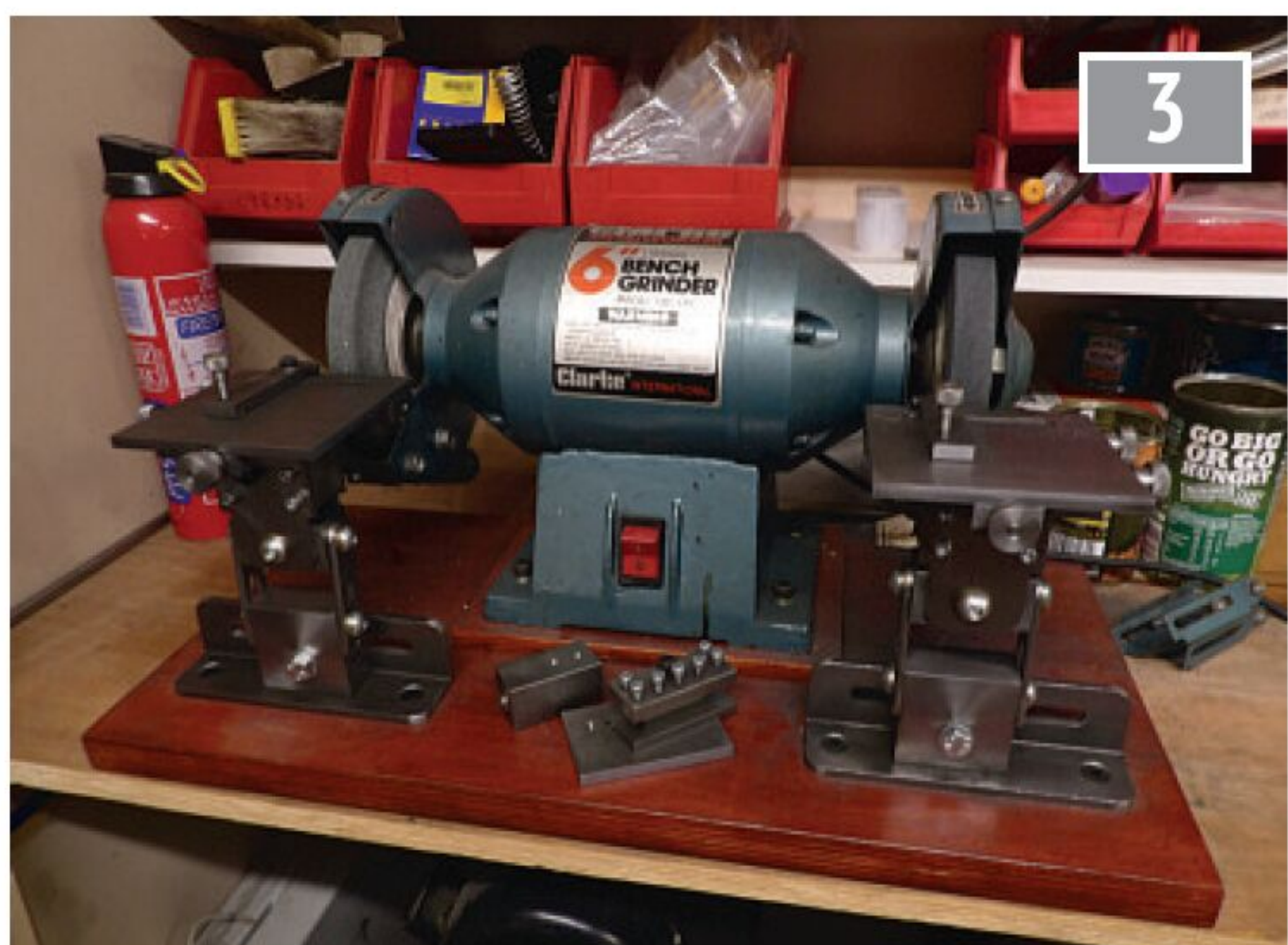
Upgraded basic 6 inch bench grinder to enable basic tool and cutter sharpening.
