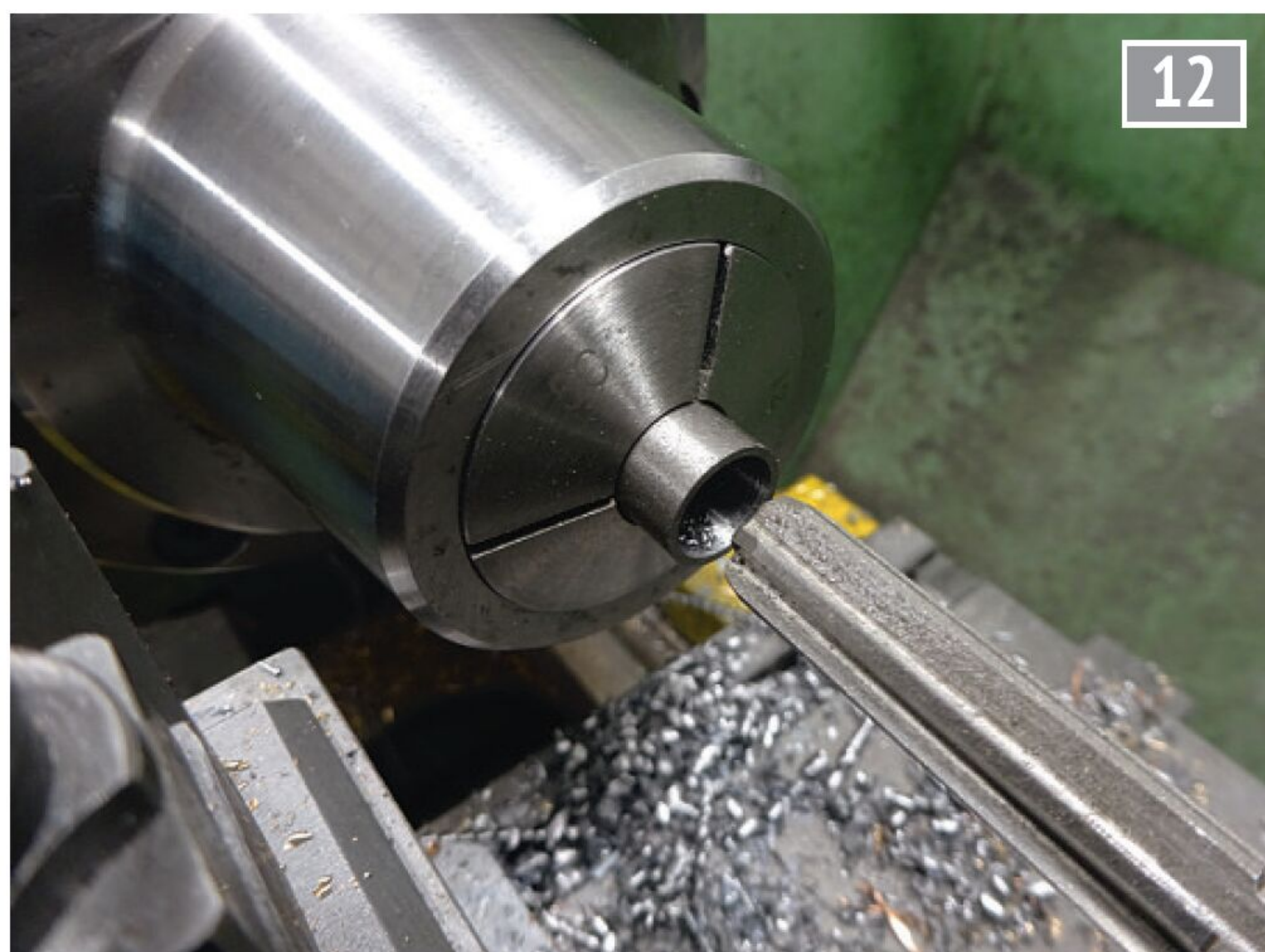
Reaming the trunk guide.
