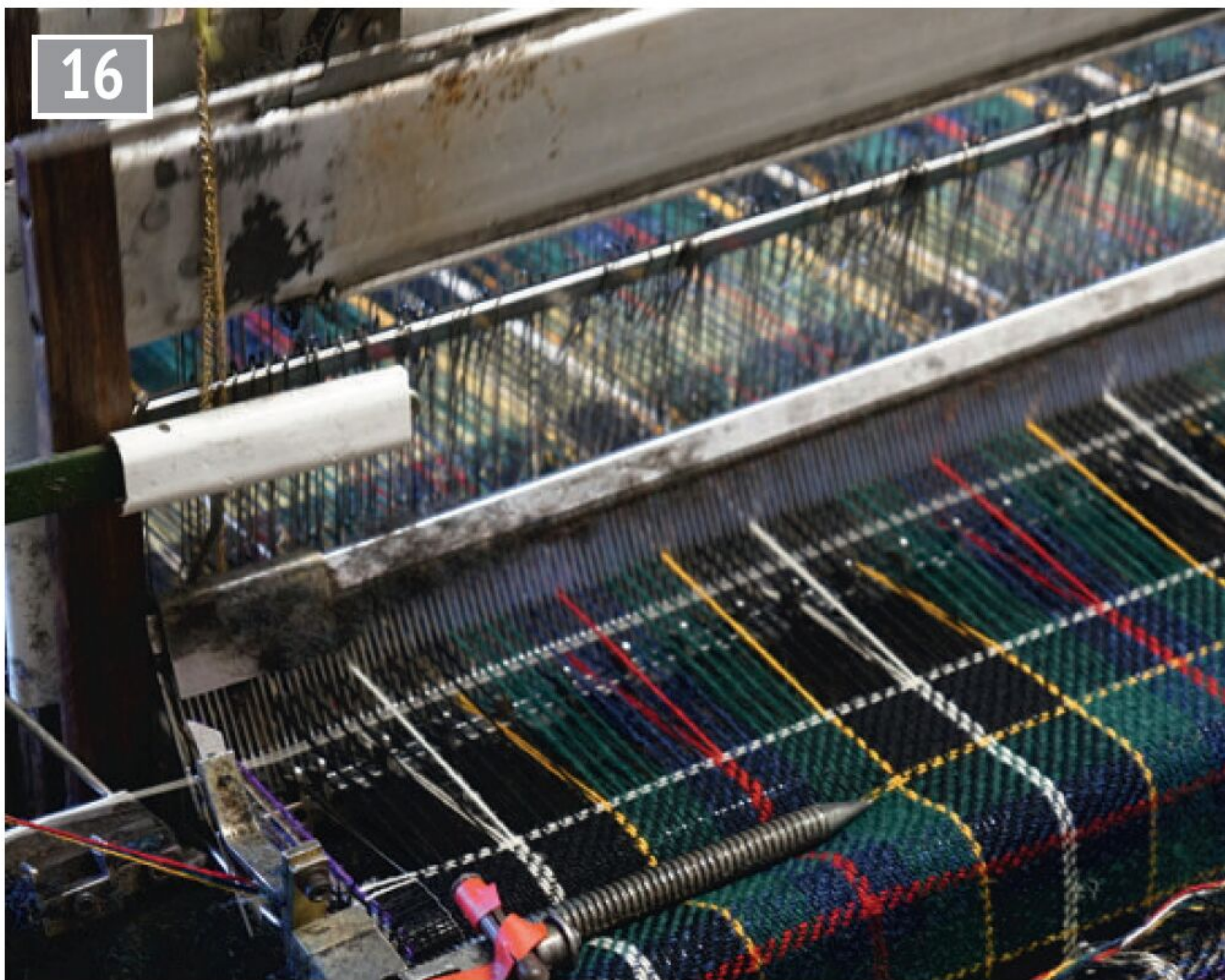
16 Weaving happens fast on a rapier loom! The rapier has picked up a white thread and the beater (metal with vertical slits) is moving towards the camera to 'beat up' the just woven thread. Behind the beater the boards (aluminium tops) are moving up and down forming the shed for the next weave by the rapier.
