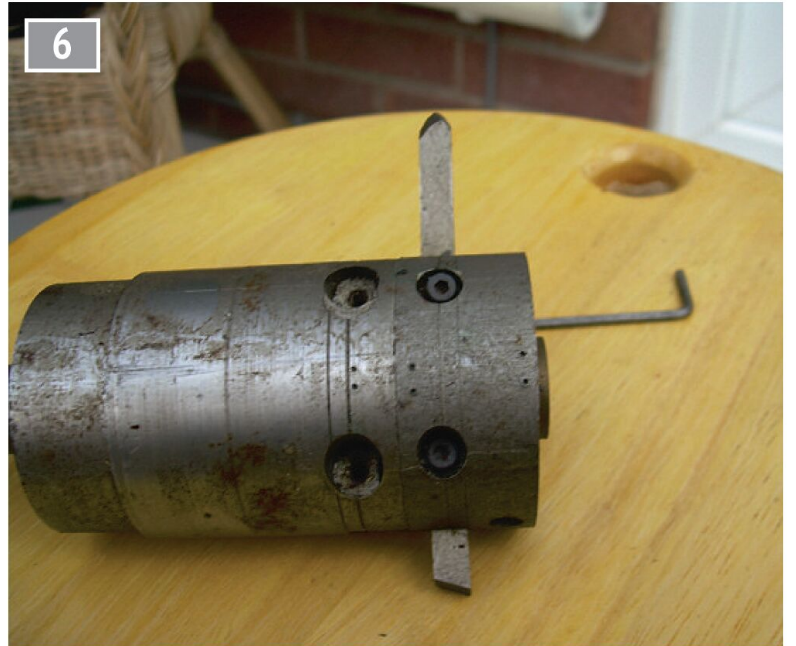
The unit. Showing the disused tool clamping screw holes in the body. The pop marks are to make sure that I get it the right way round when I put it together.
