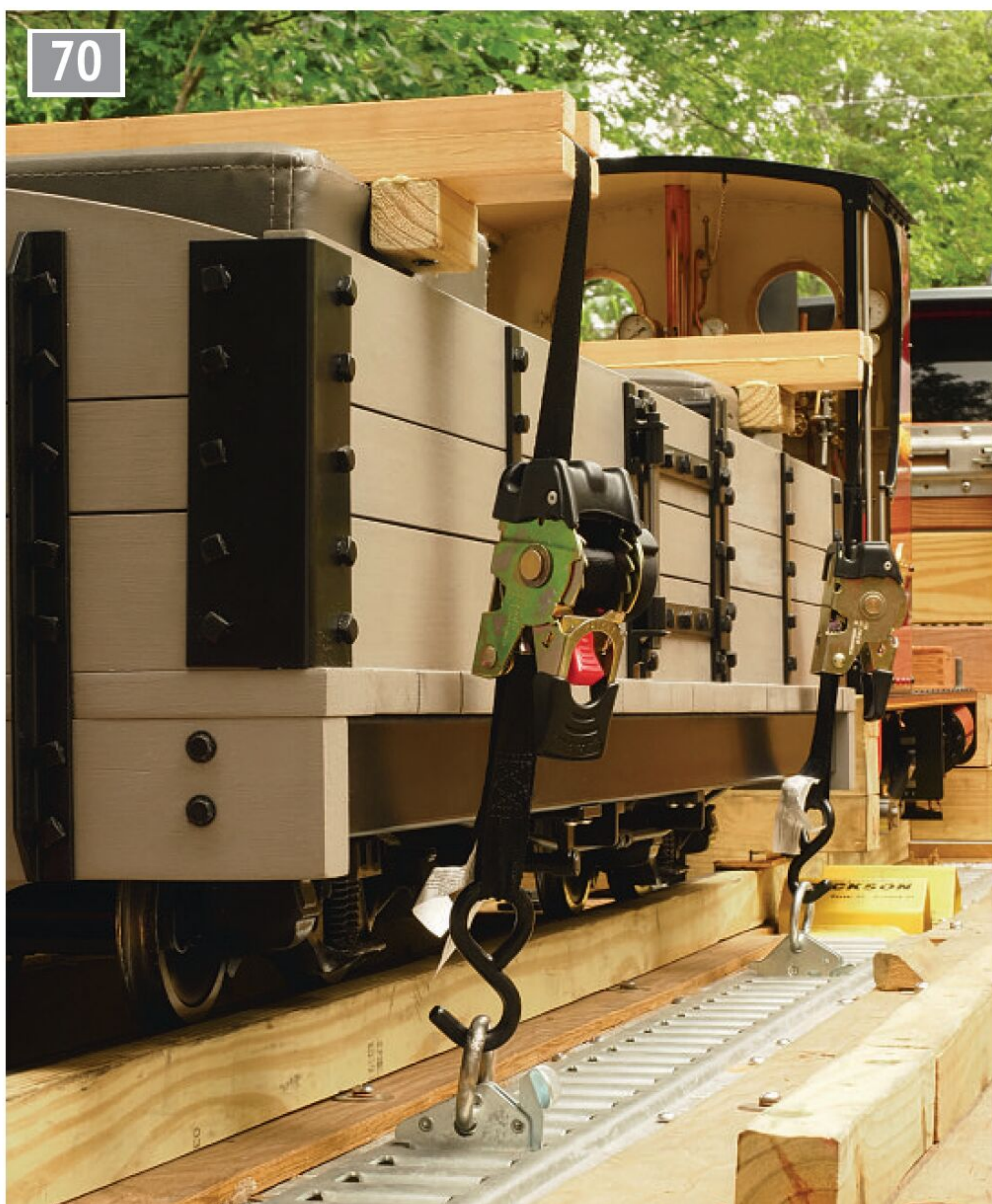
Ratchet straps tug the driving wagon down onto the wooden rails.
