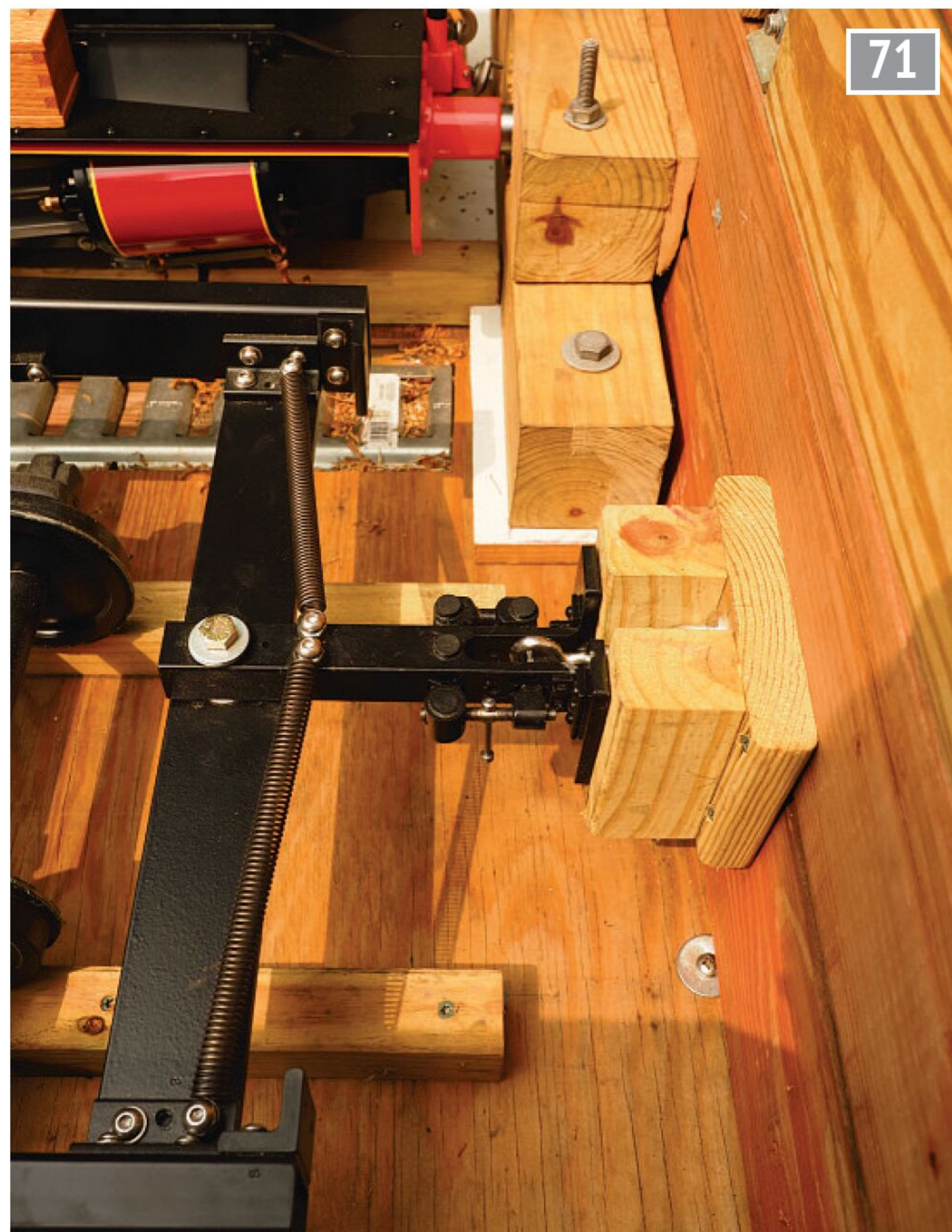
A passenger wagon chassis sits in the trailer with its frontmost buffer against another wooden block. While the just-visible silver hook holding the buffer has no structural purpose, it does prevent the wagon from rolling out of the trailer and disappearing into the sunset when the author is distracted. Eventually, another wooden block will be added behind the rear of each passenger wagon to keep it securely in place fore-and-aft while on the road.
