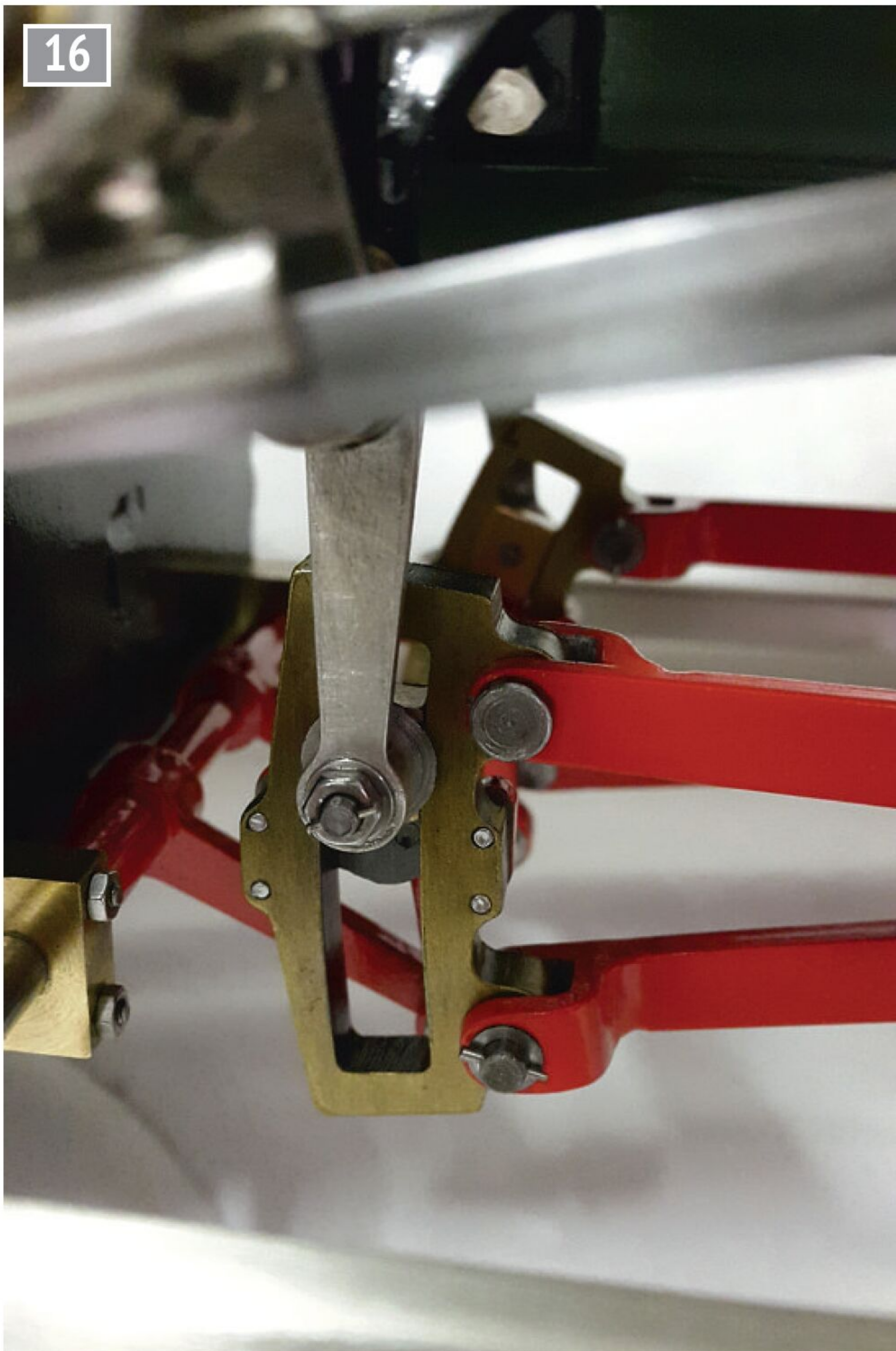
One of the oddest things I've done as a model engineer was to make a strong component look weaker to fit the prototype. Brass plating steel components is relatively easy in the backyard; it's not a new process but as far as I know this method has never been used to plate an expansion link.
