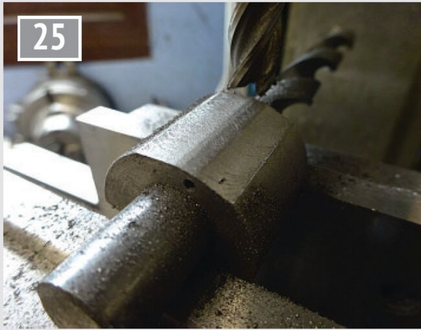
Shaping outside of cylinder.
