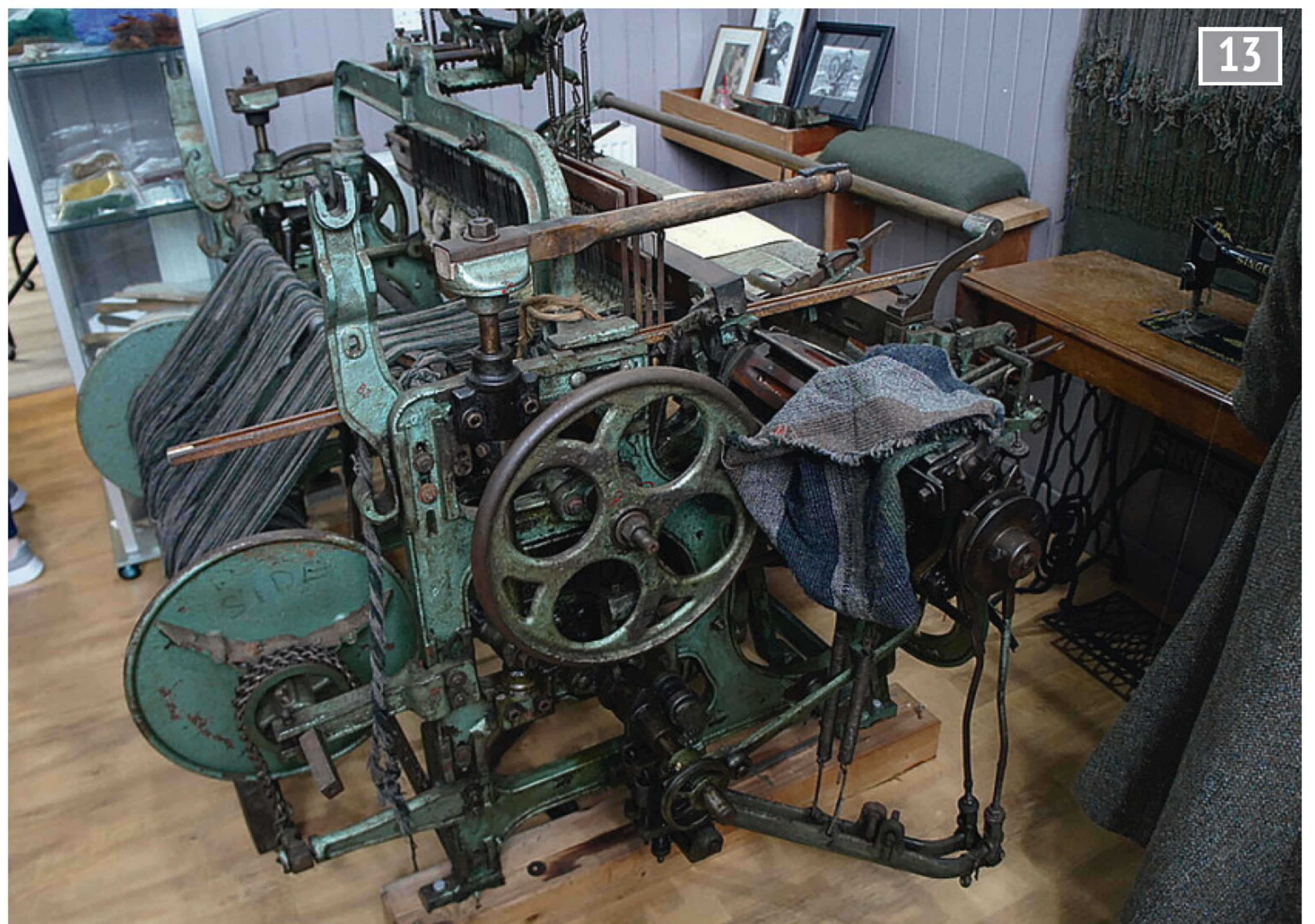
Hattersley iron loom displayed at the Harris Tweed shop in Drinishader. Unfortunately it is not currently set up for weaving. Introduced from 1919, these looms transformed tweed weaving.
