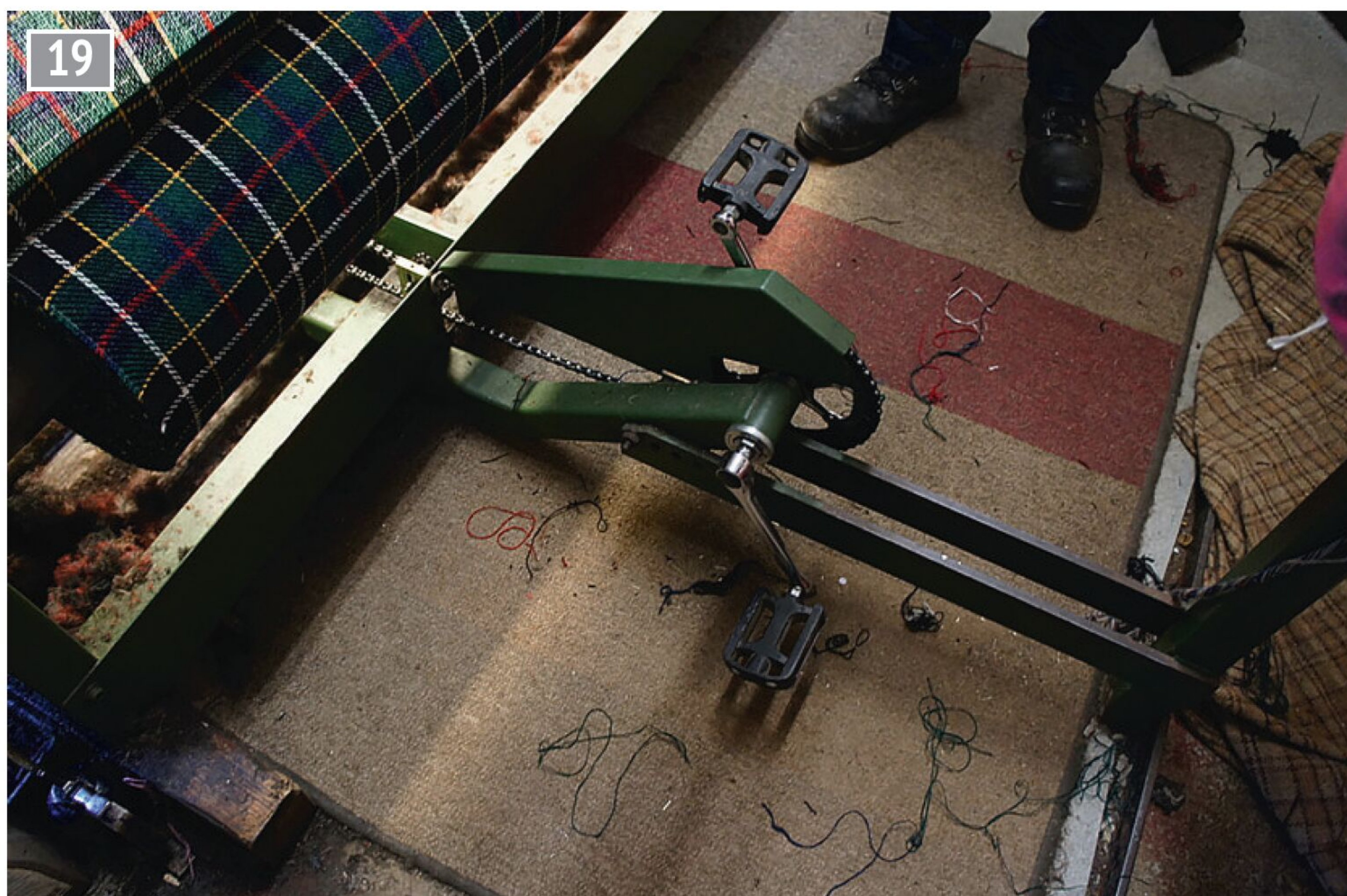
Rapier loom pedals - muscle power still dominates Harris Tweed weaving.
