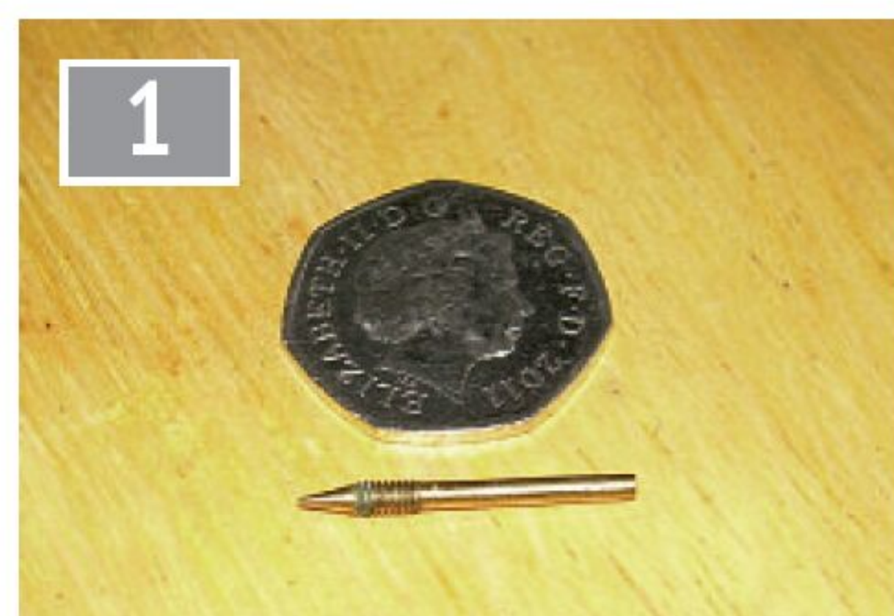
Regulator spindle. Thread is 5BA ( \frac{1}{8} inch), spindle is 2.2mm.
