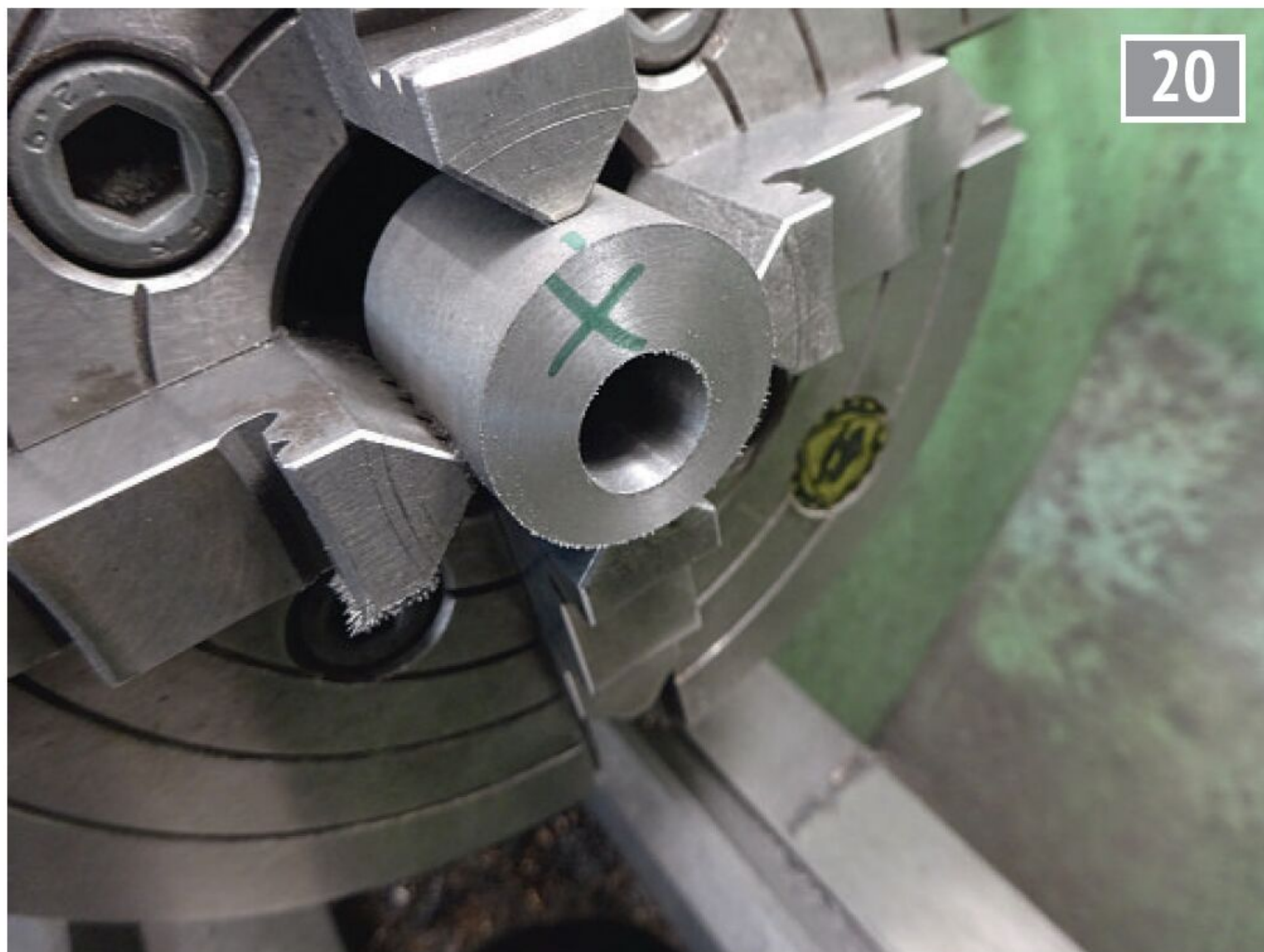
Cylinder bored and faced.
