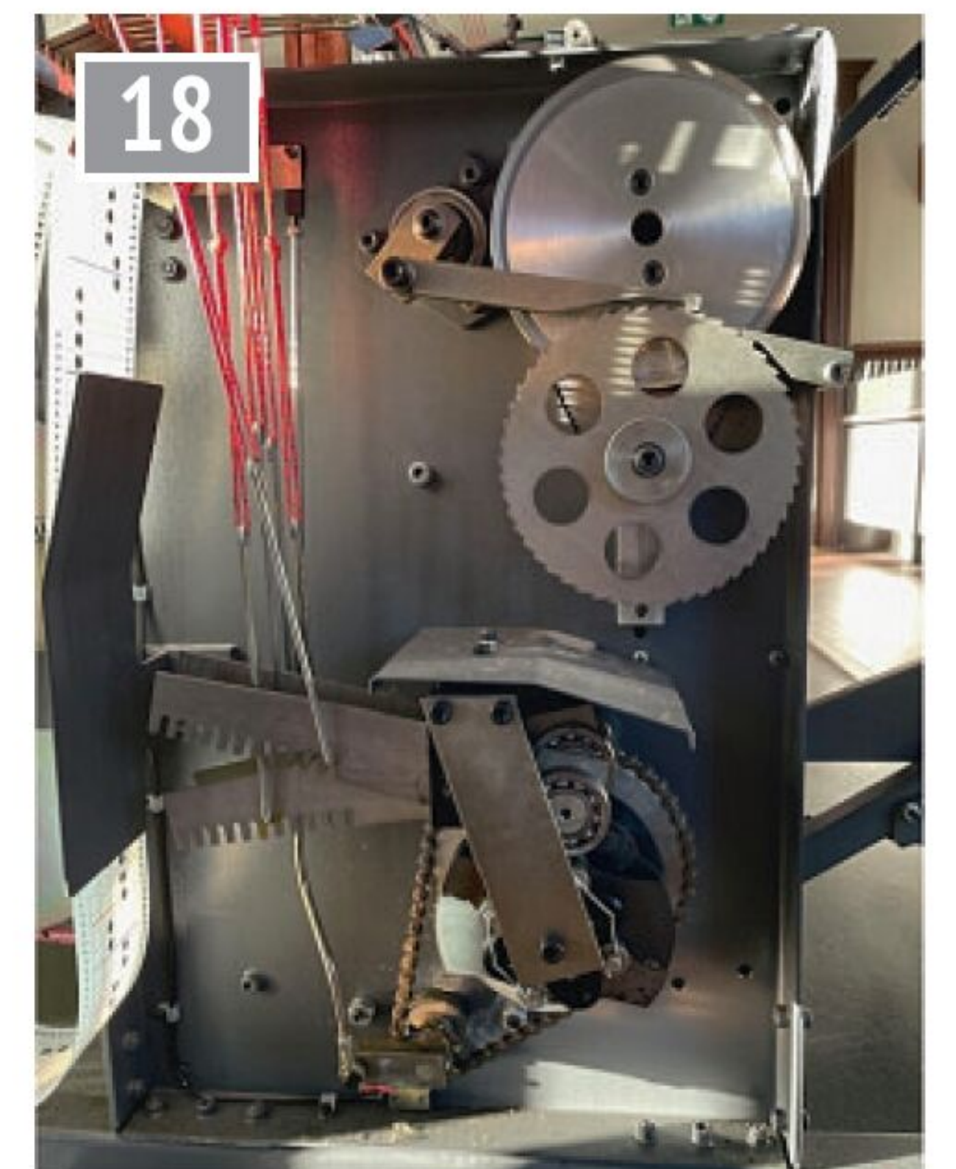
18 Tappets and brackets pull the appropriate cord to lift boards. (Photo: Harris Tweed Authority 2024. Thanks to Kristina Macleod for this picture of the rapier loom in the Harris Tweed Authority offices.)
