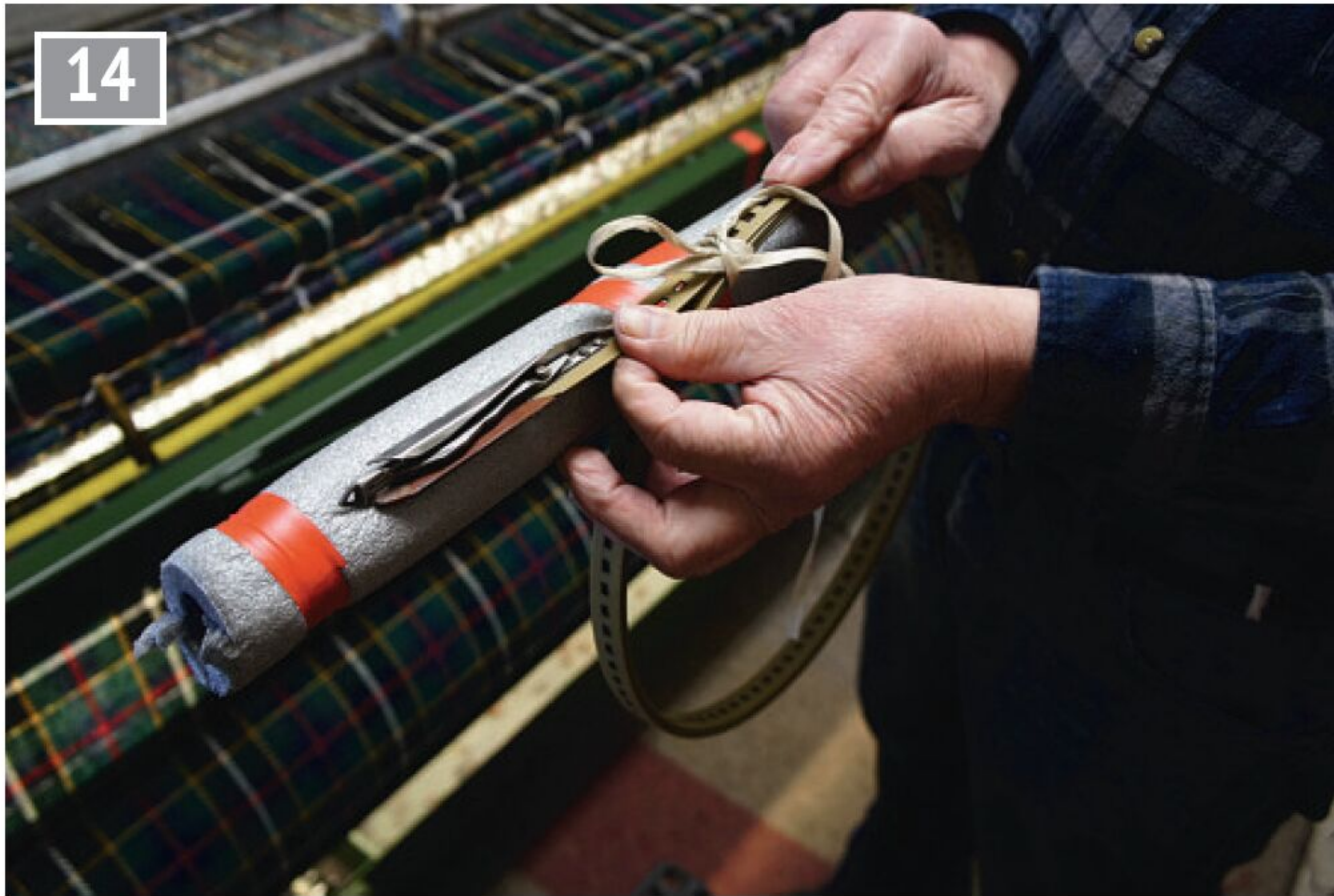
14 Rapier on a single rapier loom shown by Kenny MacLennan. It is fixed to the coiled strip which guides it across the loom where it will pick up one of the weft threads.
