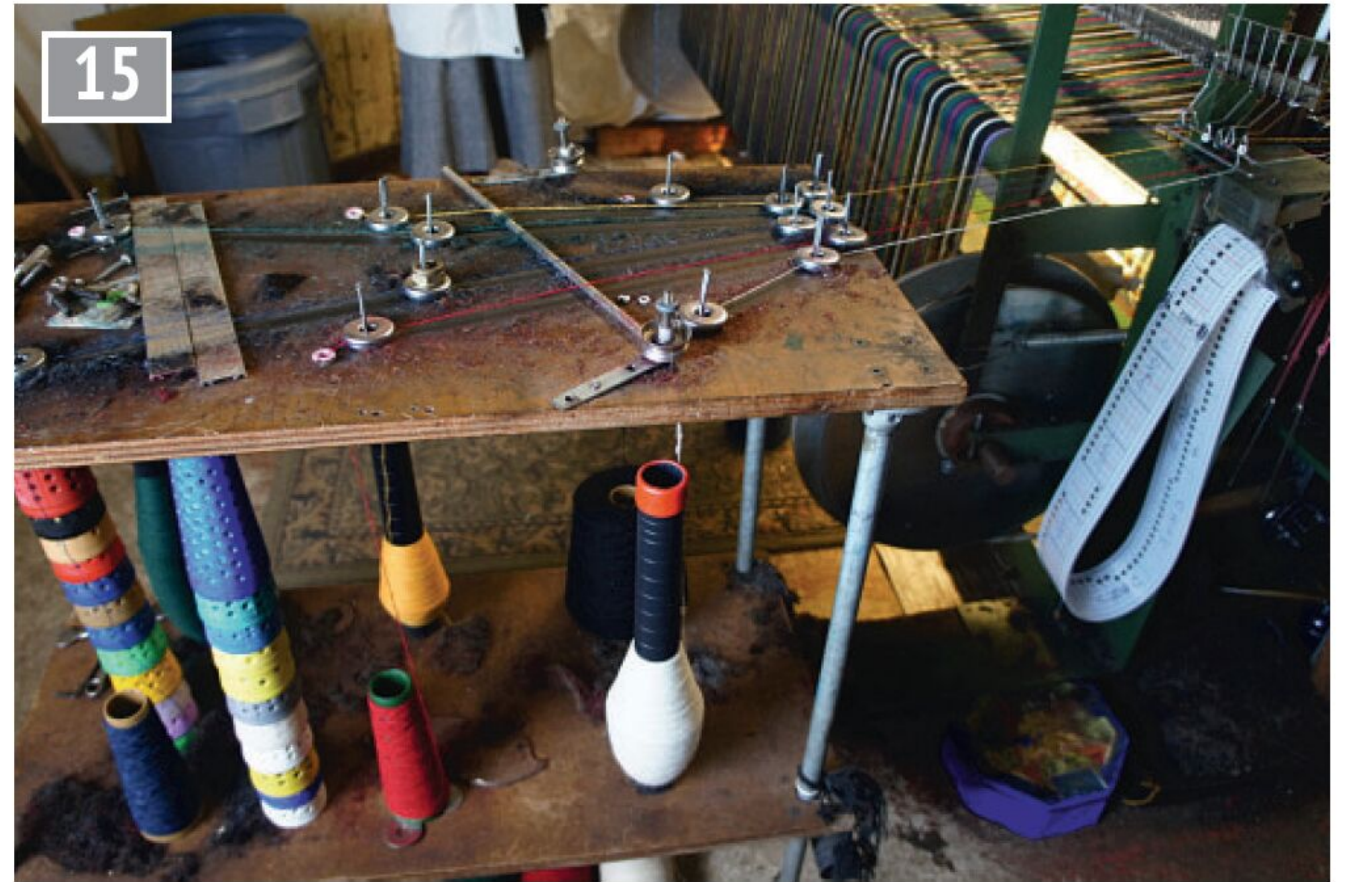
15 Weft threads pass from the bobbins below the table to be picked up by the rapier. The device to lift weft threads is in the top right of the picture. The punched plastic strip and selects the weft thread to be picked up by the rapier. Board lifting is controlled by the tappet levers.
