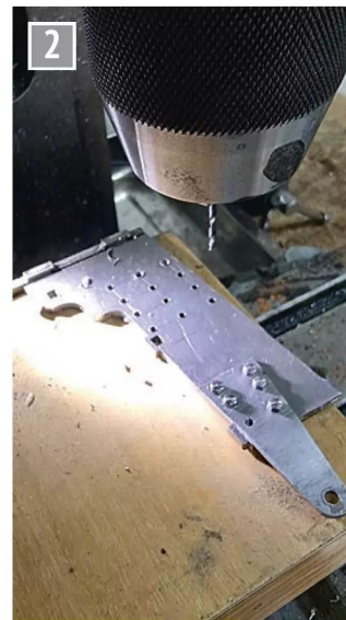
Drilling the array of bolt holes on the inside of the assembly.
