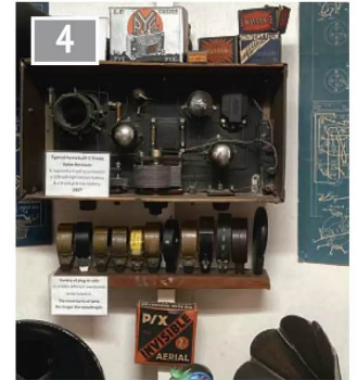
A typical 3 triode receiver from 1927.
