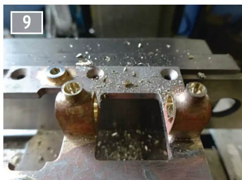
Drilling the oil holes.
