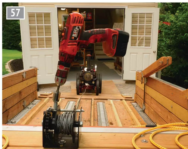
The winch with portable drill in position, all ready for use.
