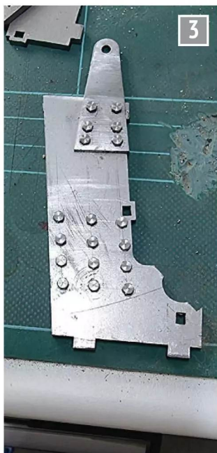
Trial assembly of the bearing plate.
