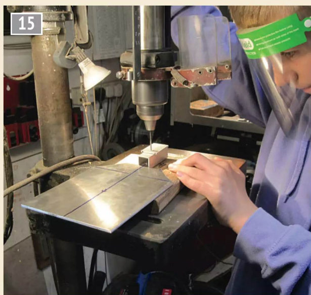
Gluing rather than clamping for spotting through.
