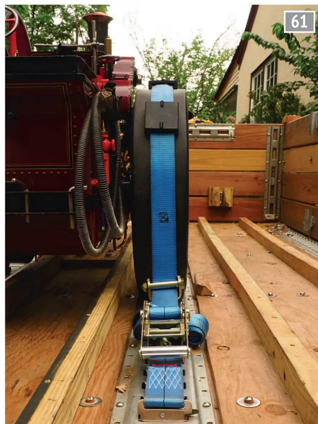
For the rear wheels, the Ratchet Strap with Roller Idler kit includes three rubber wheel pads having triangular protrusions on each side, ideal to locate with the groove between Ruby Swann's vulcanised tyres.
