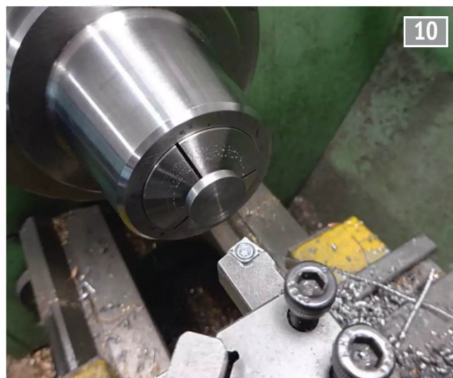
Facing crank disc to final thickness.
