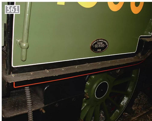
Tight radius at the corner of the cab on 1306 (photo: John Thompson).
