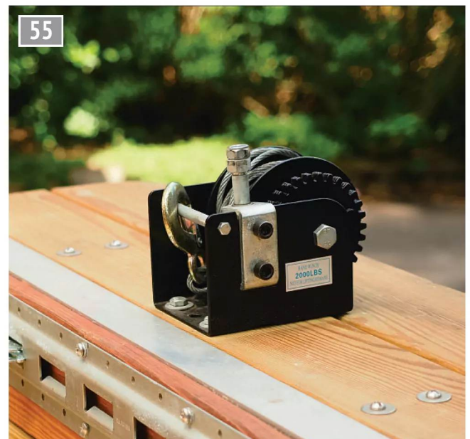
55 The worm drive winch, its handle removed and replaced by two locked nuts.
