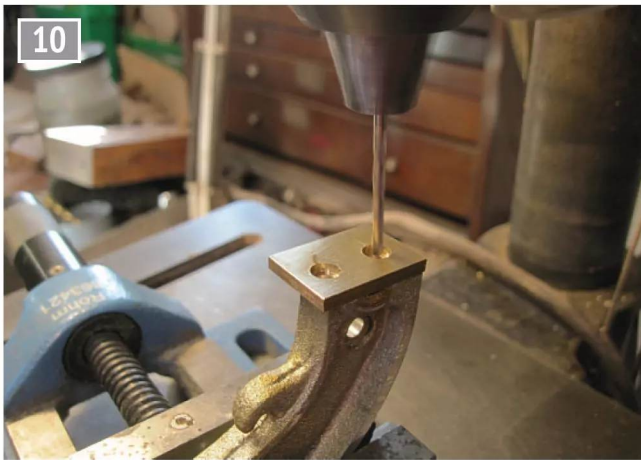
Drilling and fitting pressure pads.
