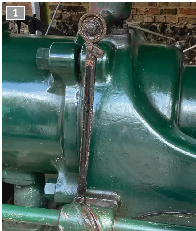
Lubricator drive on the Tangye gas engine.
