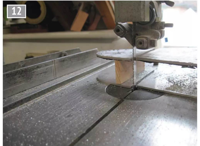
Cutting the plates on the bandsaw.
