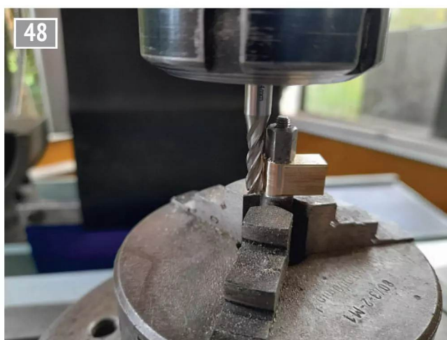
Milling the radius on a knuckle.
