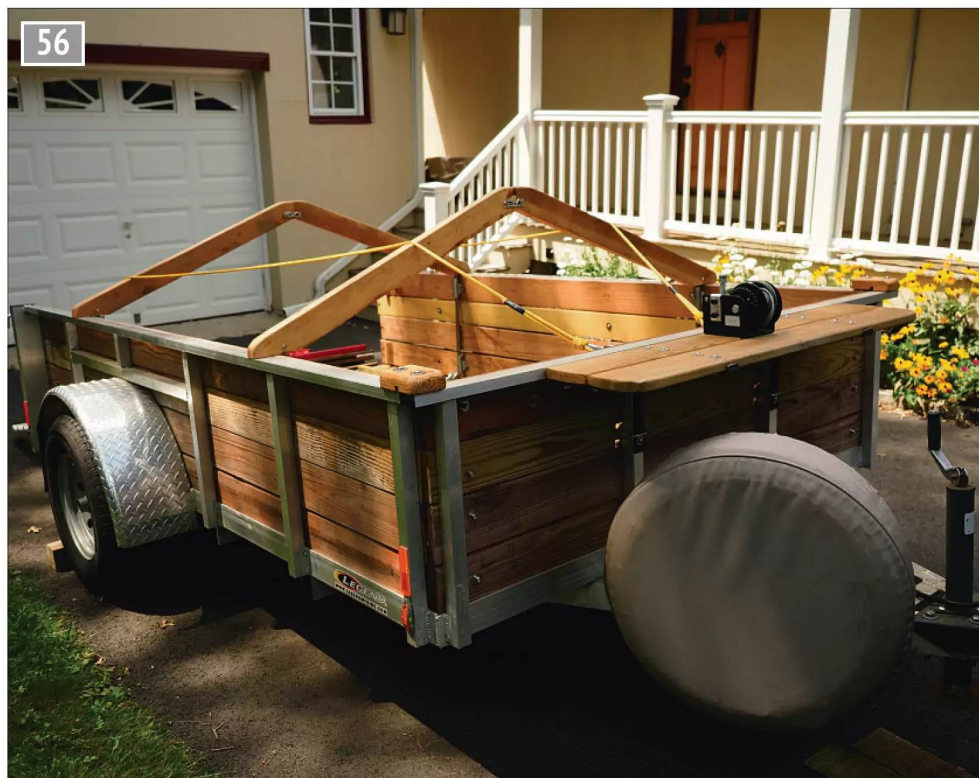
The winch is bolted to a substantial shelf above the towbar; readily accessible without consuming valuable payload space.
