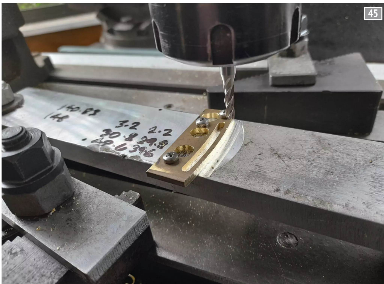
Milling the outside radius in the quadrant.
