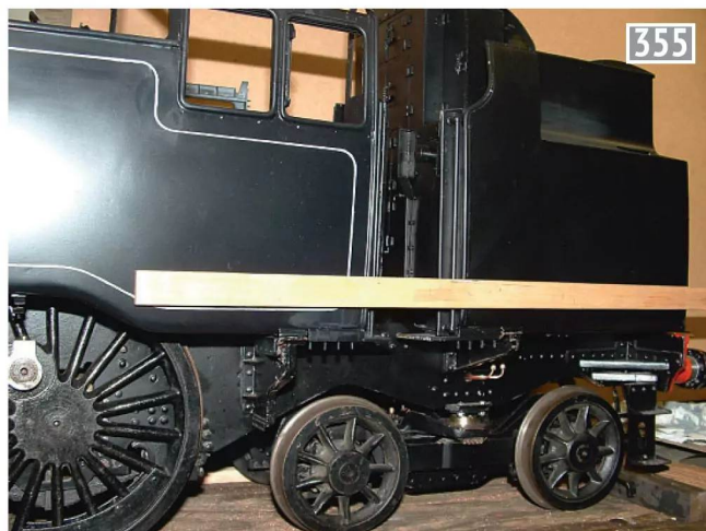
Lining up to add the grey line at the bottom of the tank.
