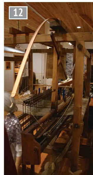
Wooden loom displayed at the excellent Kildonan Museum, South Uist. The wooden lath springs the flying shuttle across the loom. Tops of the boards are visible.
