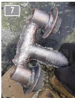
Copper is one of the more difficult metals to cast because the chance of blow holes, due to gas pickup, is very high.
