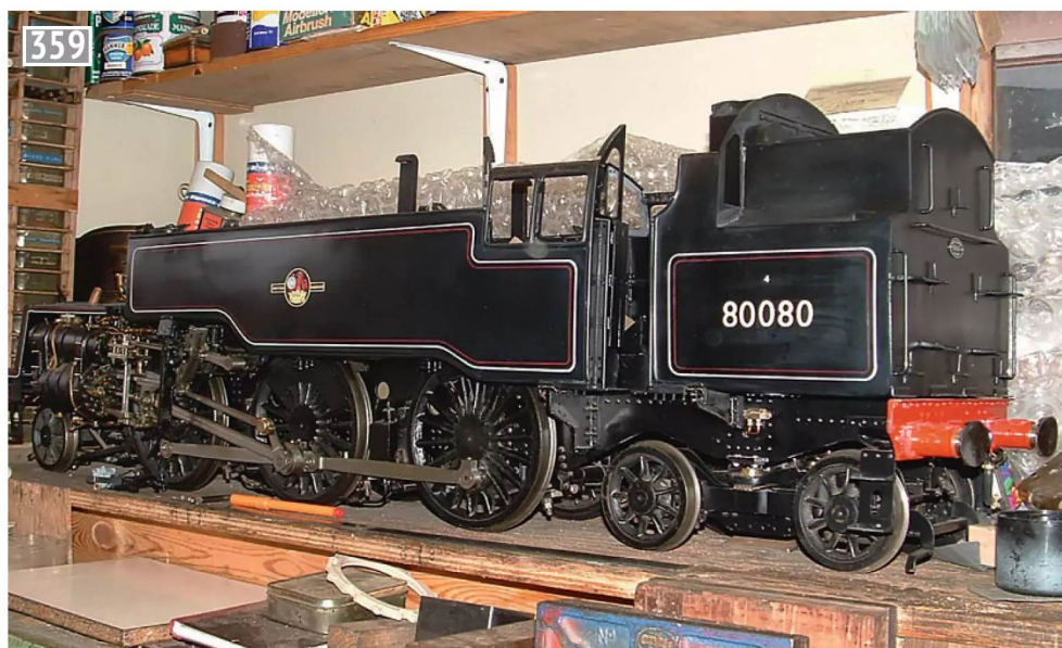
Lining finished on the 4MT.
