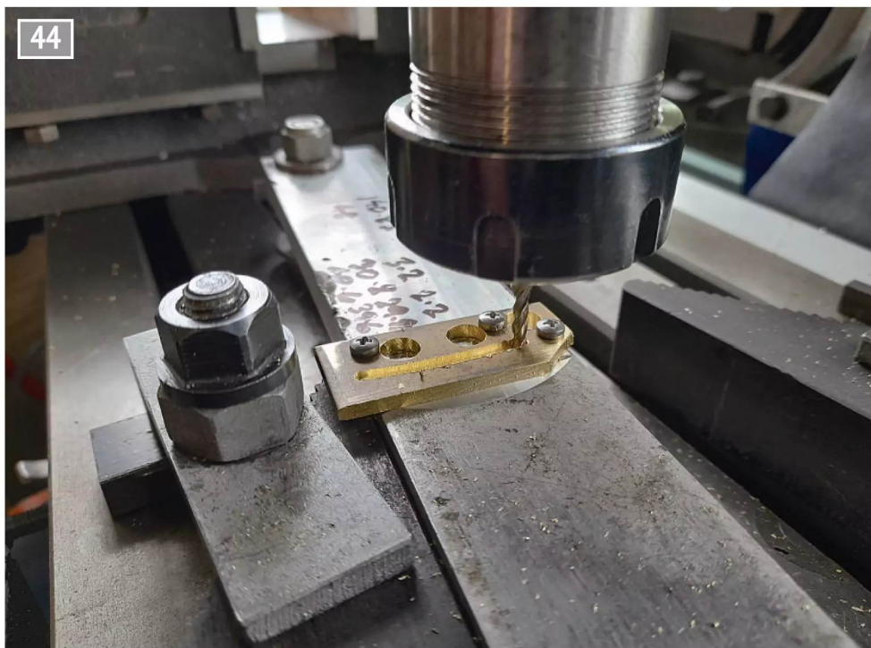
First stage milling the quadrant slot.
