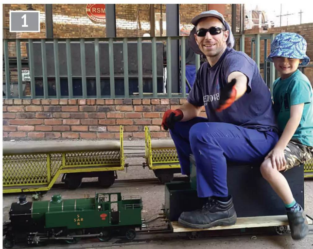
My little William, a 2-6-2T engine designed by Martin Evans. I built this locomotive very close to drawing, but found that it tended to run with a colder fire and had an uneven beat. The valve timing and grate was modified to bring it in line with my newer methods; now this little locomotive is a pleasure to drive.
