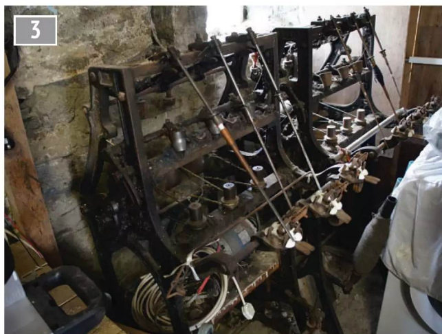
Pirn winder once used to wind thread on to pirns used in shuttles. Pirn winding was once Kenny MacIennan's job after school. His mother was also a weaver.
