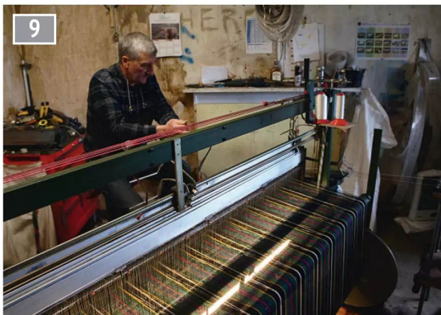
The aluminium strips are the tops of boards. Earlier versions were made of wood. As demonstrated by Kenny MacLennan on his Bonas-Griffith loom, they move up and down to create the shed for the rapier. The light underneath helps show any imperfections in the weave.
