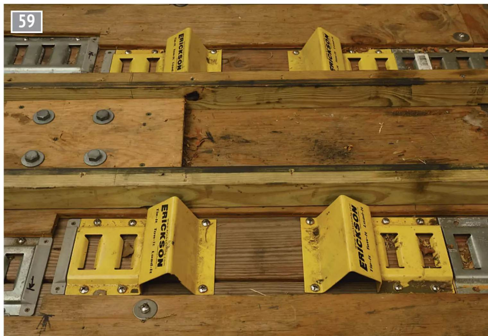
Erickson's ATV (All-Terrain Vehicle) wheel chocks were ideal for securing Ruby Swann's front wheels.
