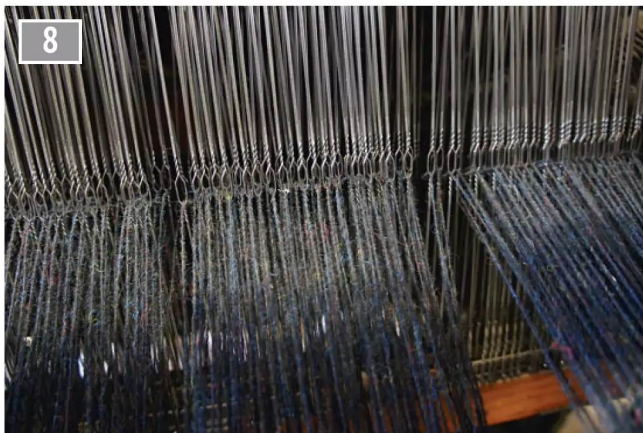
Each warp thread is passed through an eyelet in the heddle (heald or board). Boards are lifted alternately to form the shed. By using several boards, patterns can be created.
