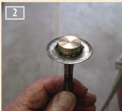
Using superglue to attach a centre for facing a valve.
