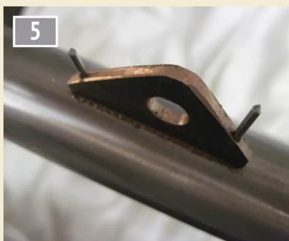
Holding a bracket in place for brazing using superglue. Note – the hanger is on the underside of the pipe.
