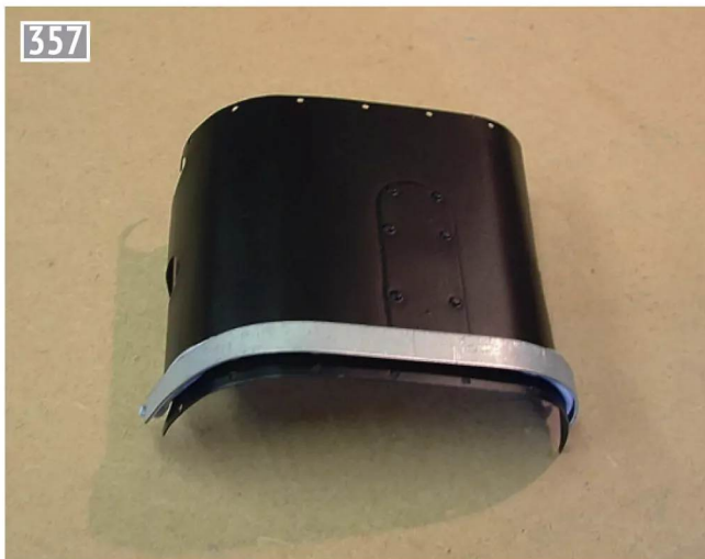
Guide strip for lining the cylinder covers.
