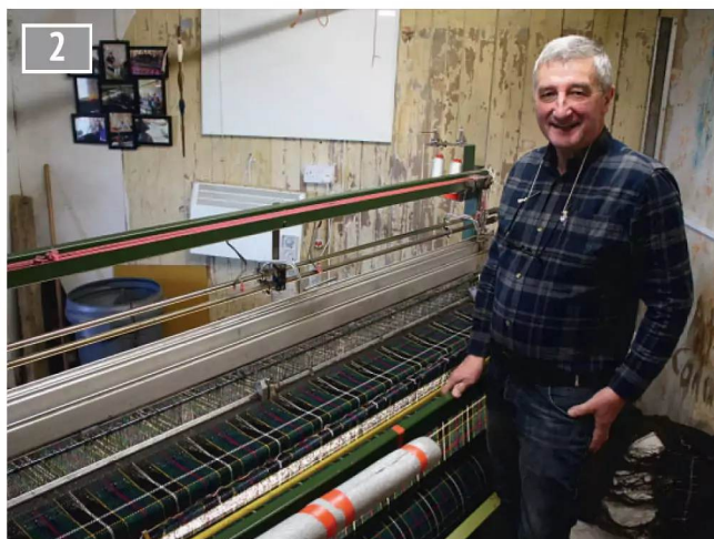
Kenny MacIennan with his rapier loom. He has been a weaver all his life and describes the loom as 'like a large knitting machine'. Many colours now used are much brighter than the original natural dyes used by islanders.
