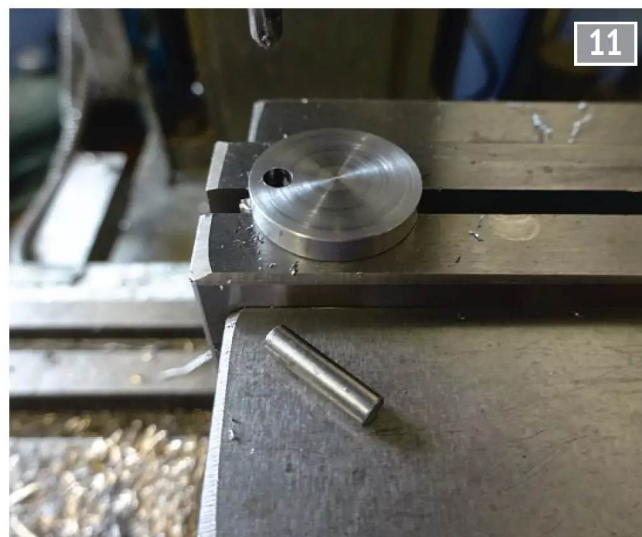
Drilling for crank pin location.
