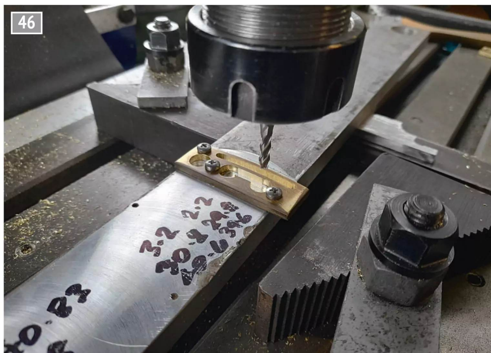
Milling the inner radius.
