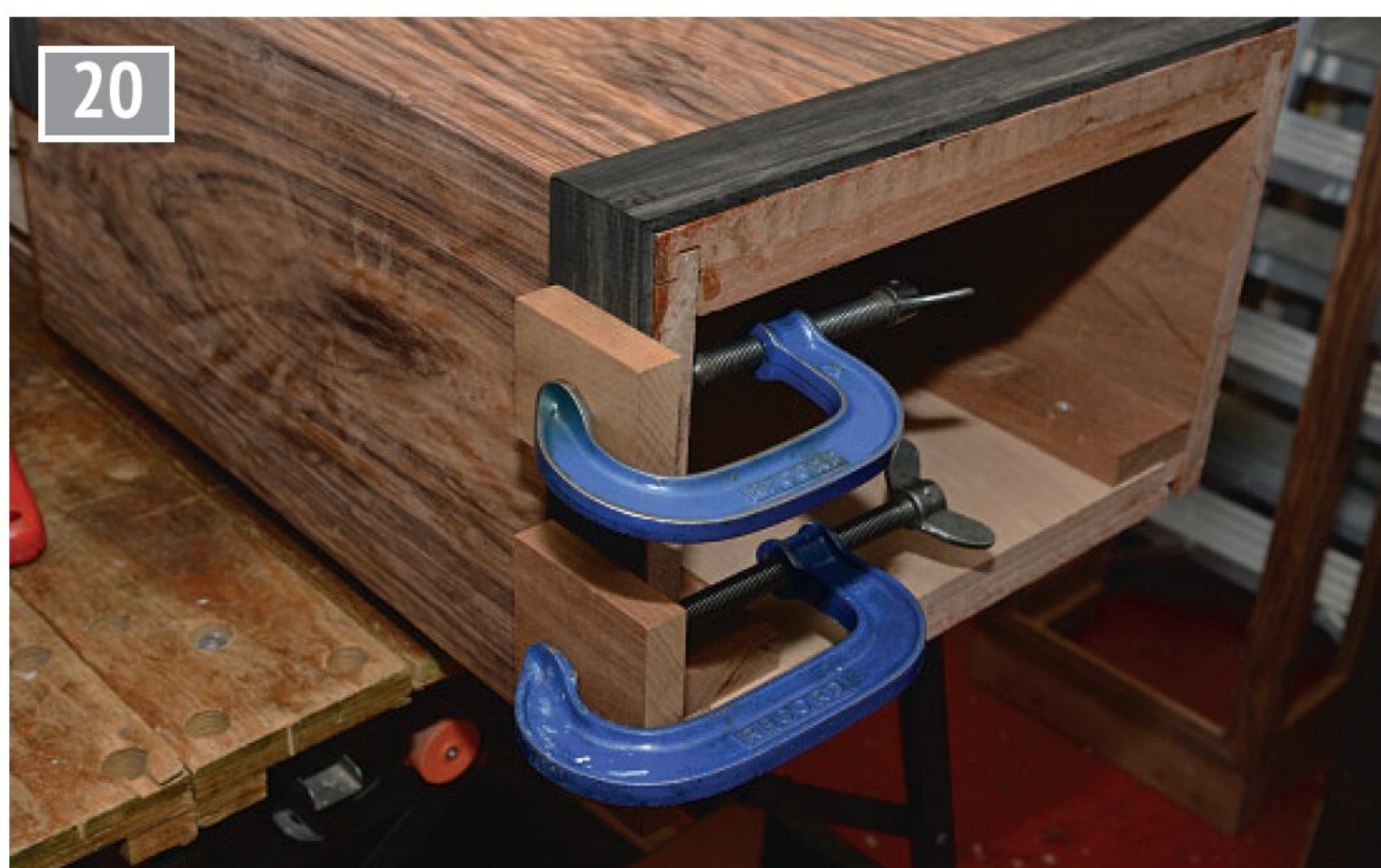
Mitred Ebony edging being glued in place after the veneer is dry.
