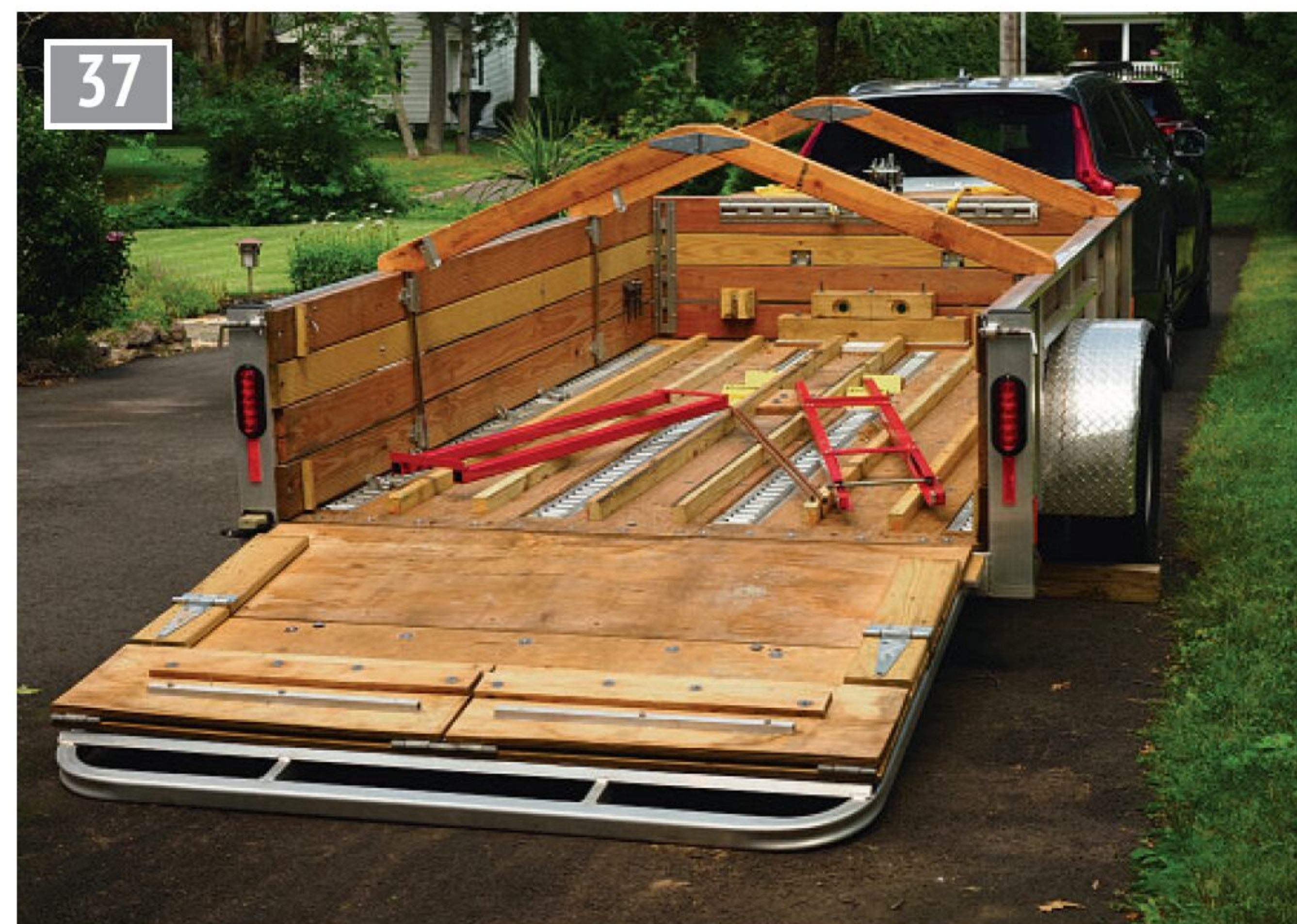
With the first part unfolded, the ramp does not quite reach the ground.
