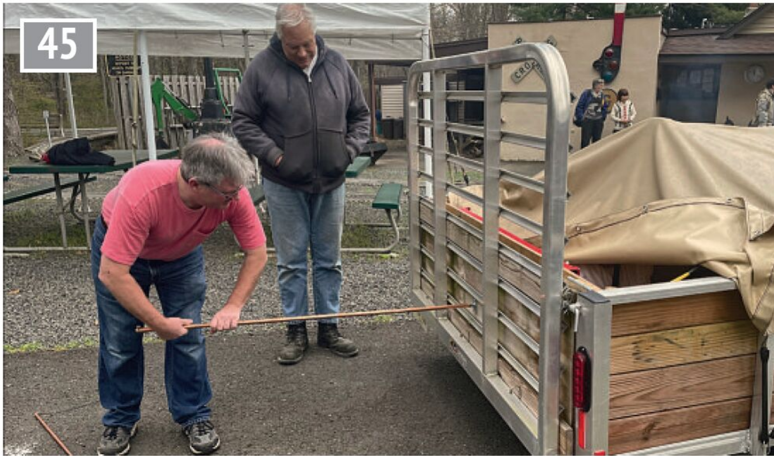
45 Ignoring comments about unicorns, the author attaches one half of the adjustable tell-tale pole to the trailer's rear end, ready for reversing towards the turntable. The second half of the pole, lying on the ground beside his right foot, slides into the first to be secured by a simple knurled thumbscrew (photo: Helen Munro).
