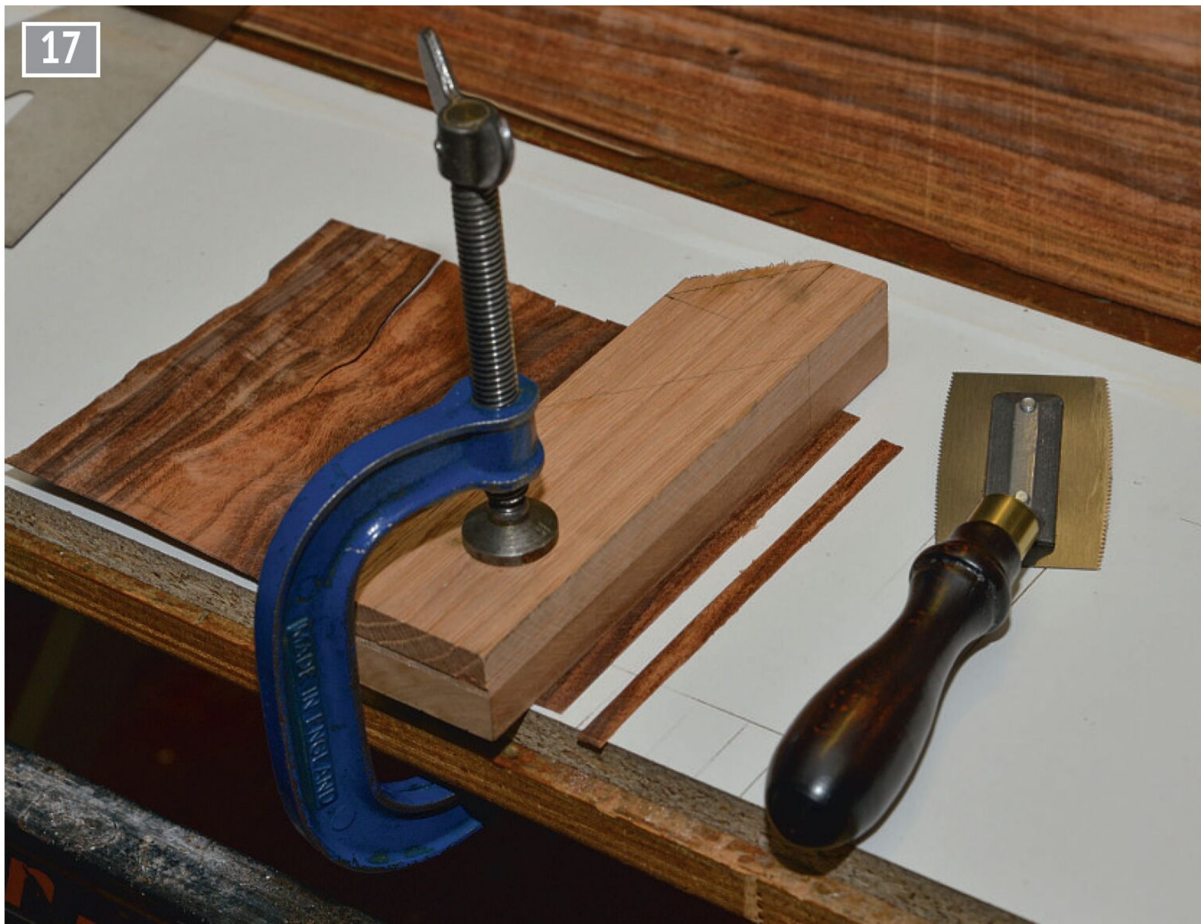
Cutting strips of veneer for the cross bars of the sides using a veneer saw.
