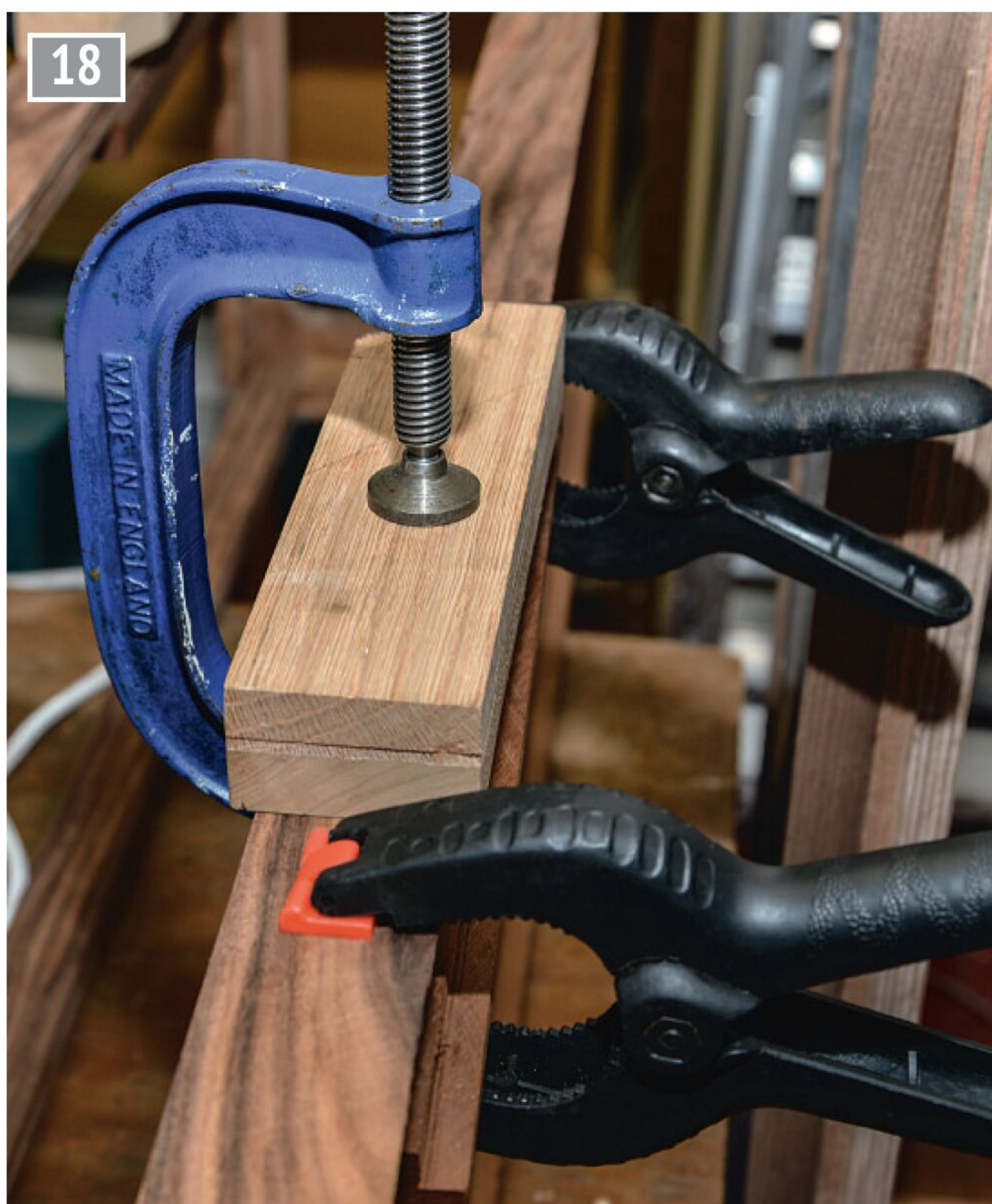
Where the veneer forms bubbles heat from an iron is applied and the area is clamped for about five minutes.
