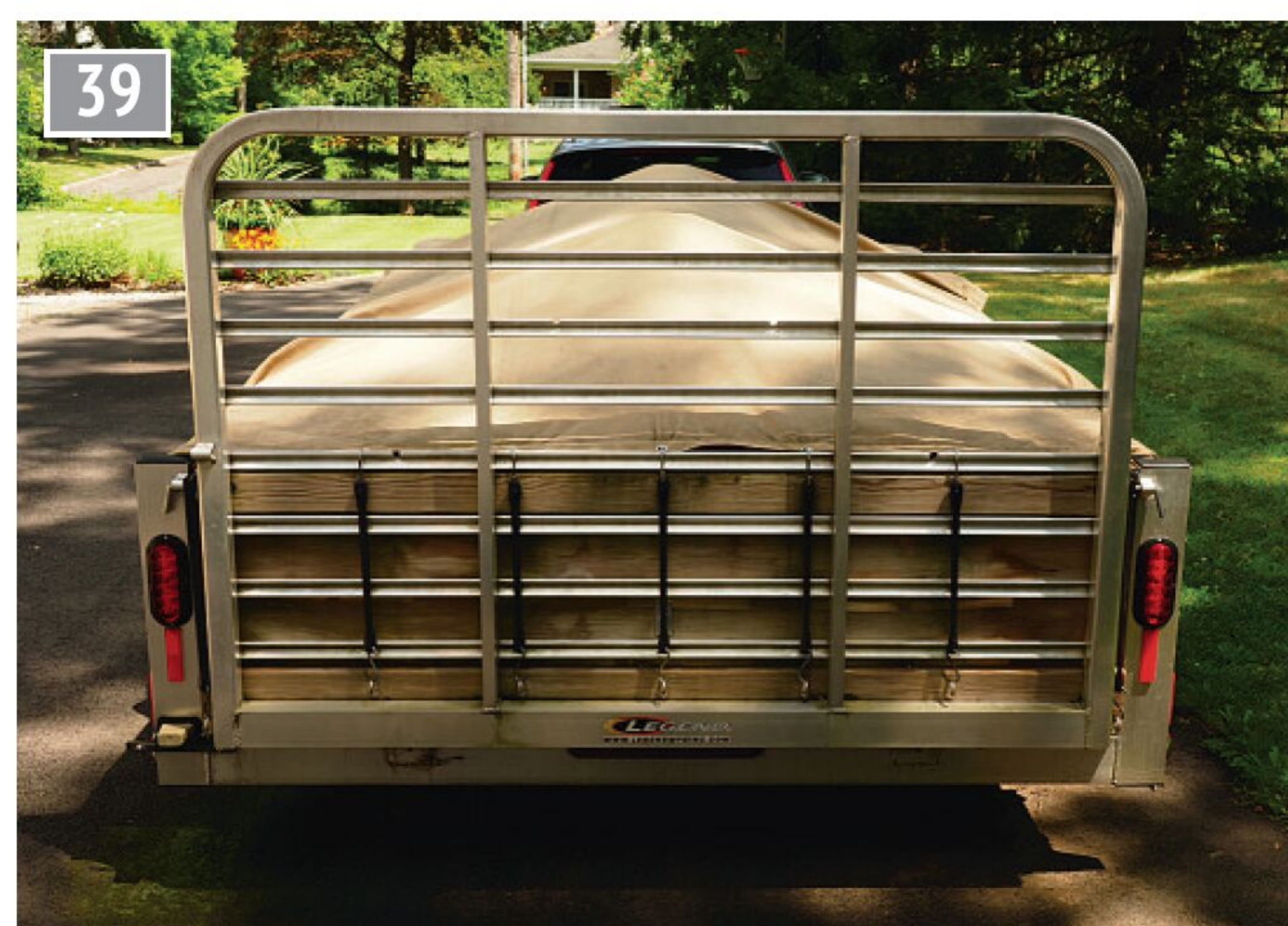
With the gate raised, the folded ramp encloses the rear of the trailer while leaving its aerodynamics unaffected.
