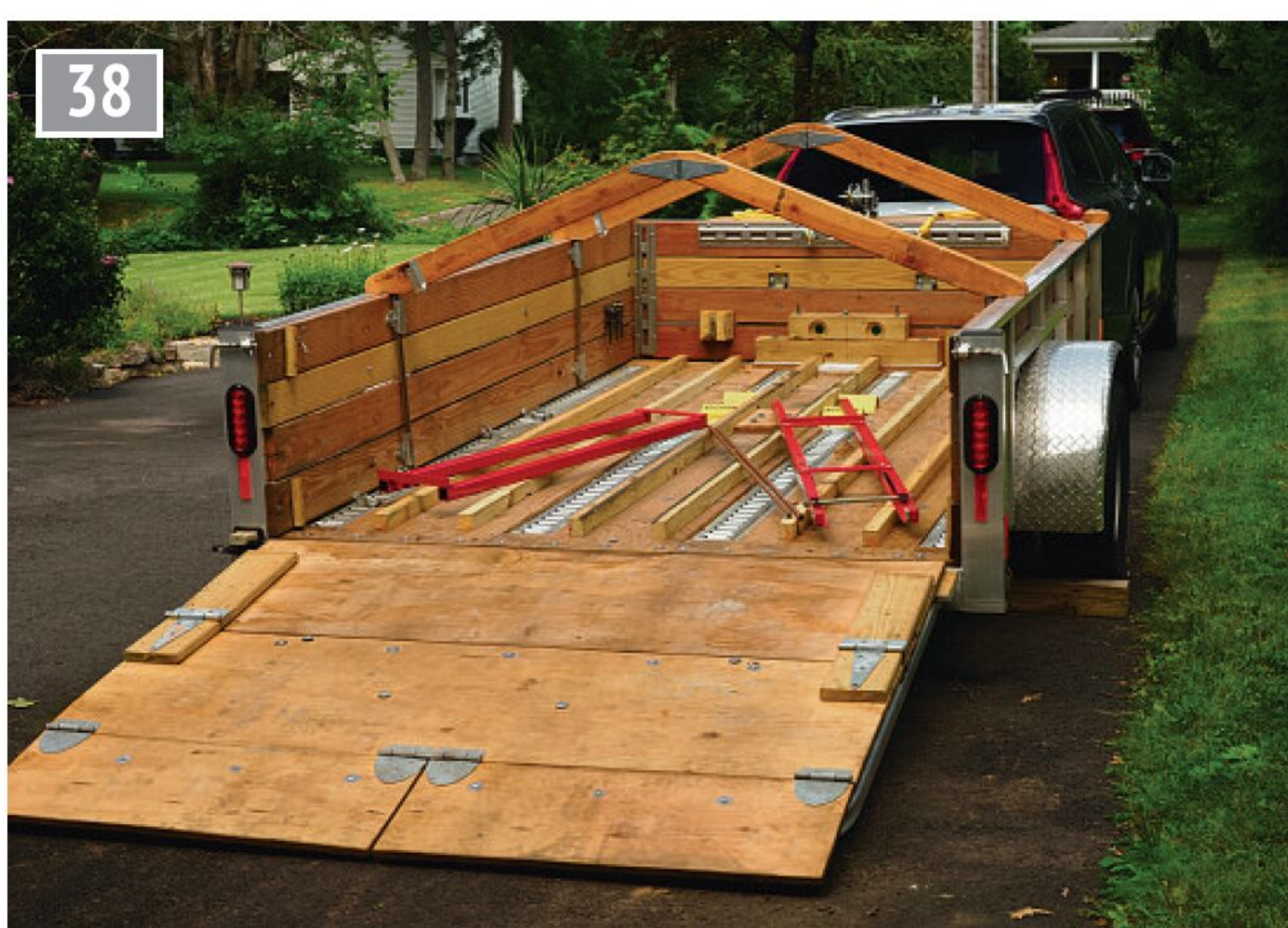
With the side-by-side lowest portions unhinged, the ramp meets the ground and gives flexibility to cope with uneven surfaces.
