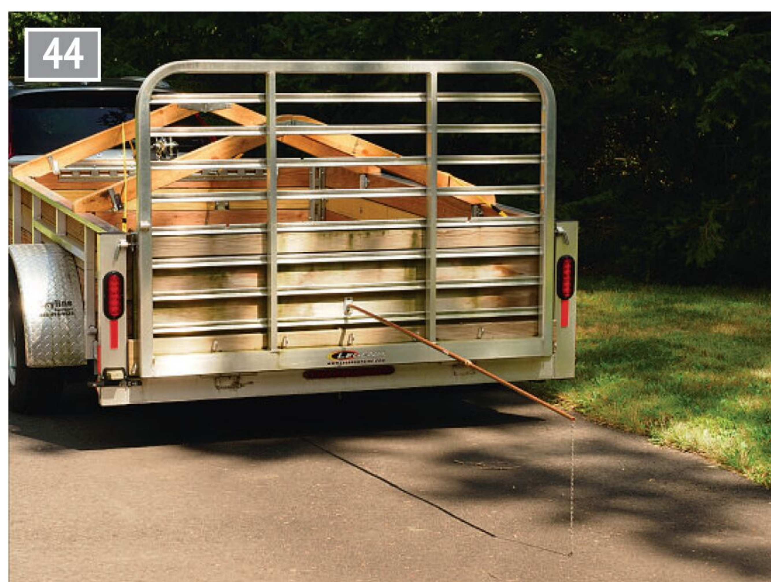
A tell-tale pole takes the guesswork out of the reversing process.
