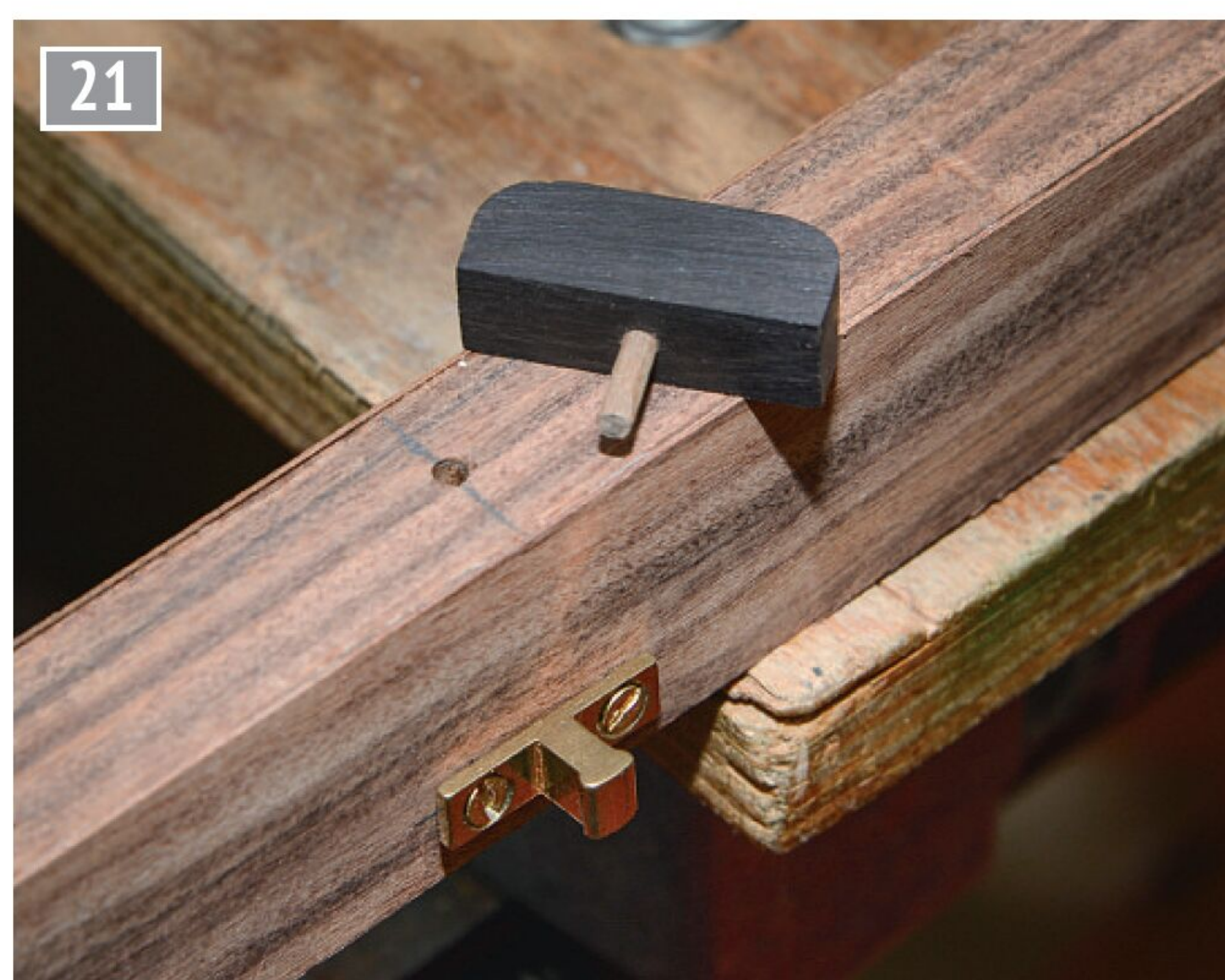
Ebony handles and brass catches. The former were cut from some spare stock and fitted via a short dowel to the door side whilst the latter are commercial items.
