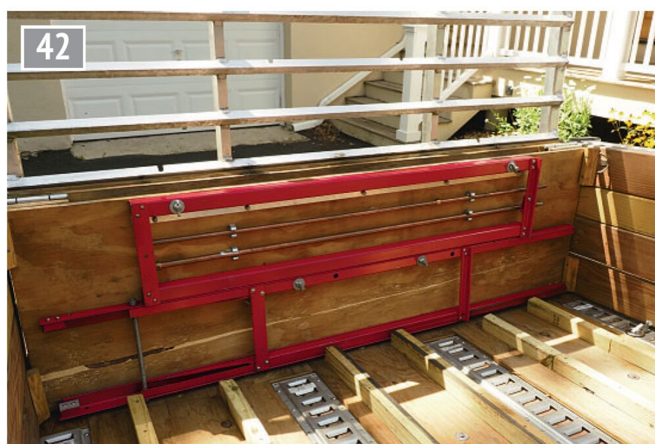
The railway bridge, attached to the folded ramp and hidden within the trailer during transportation.
