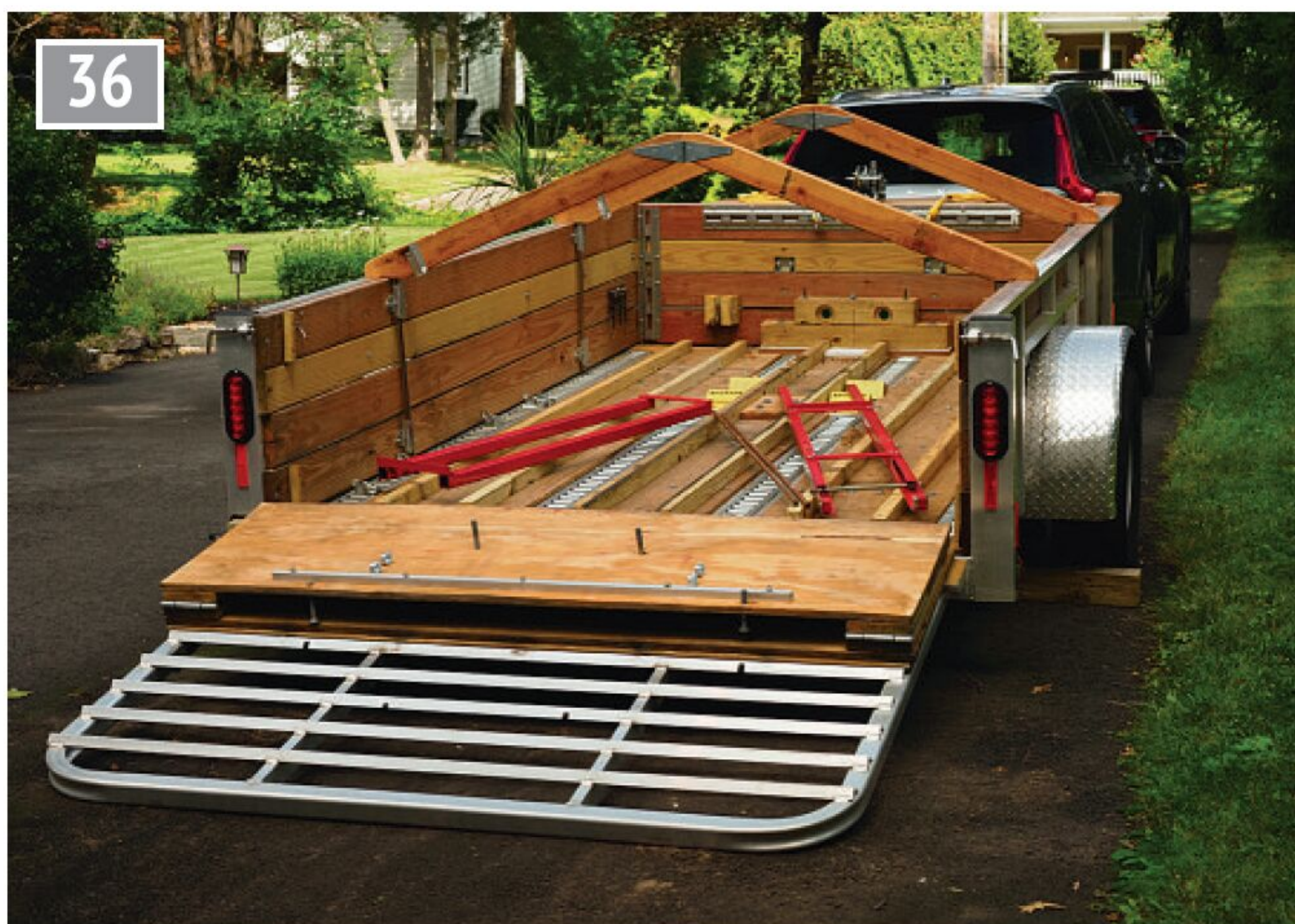
The plywood ramp attached to the rear gate, folded and ready for deployment.
