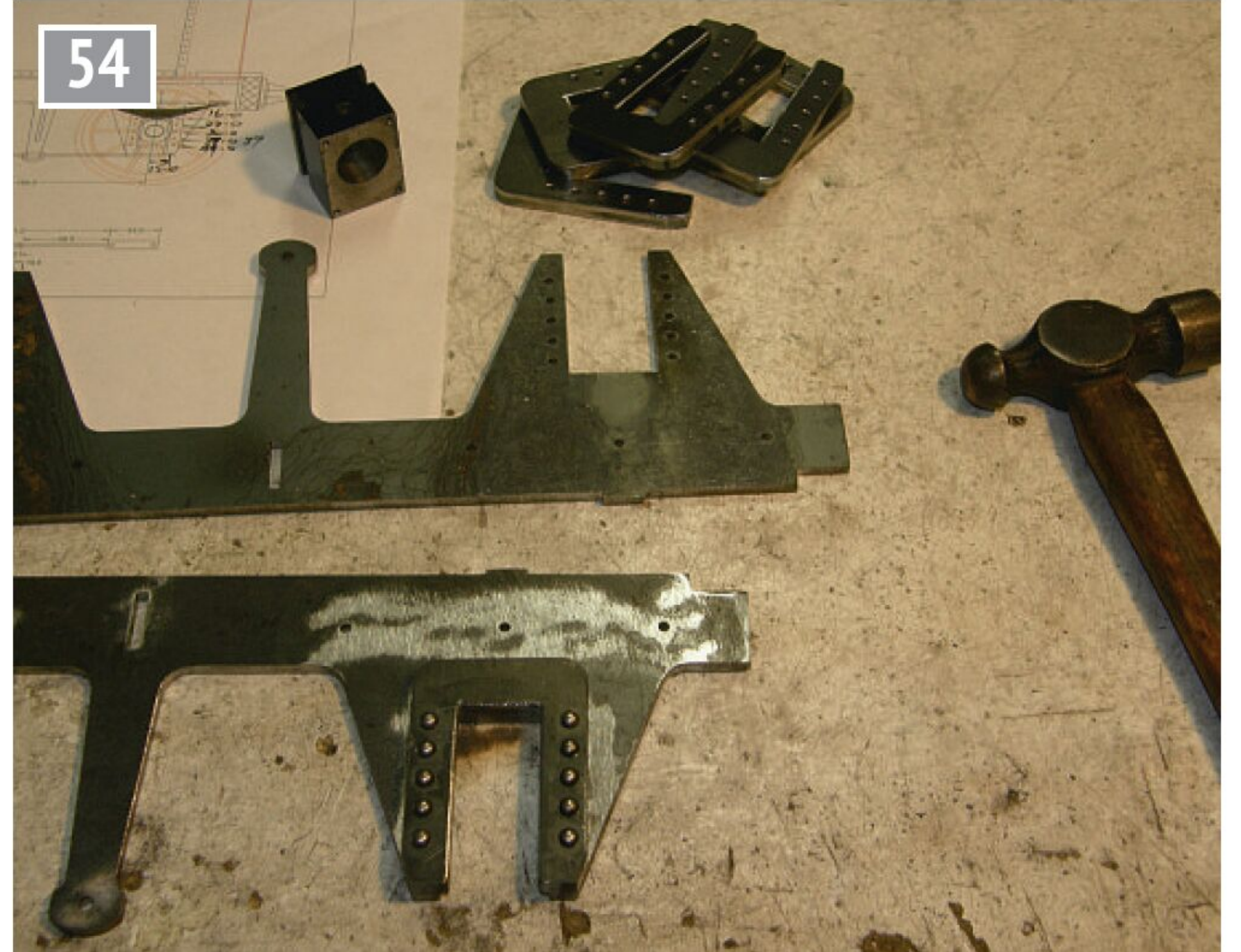
Assembling the axle hornblocks.
