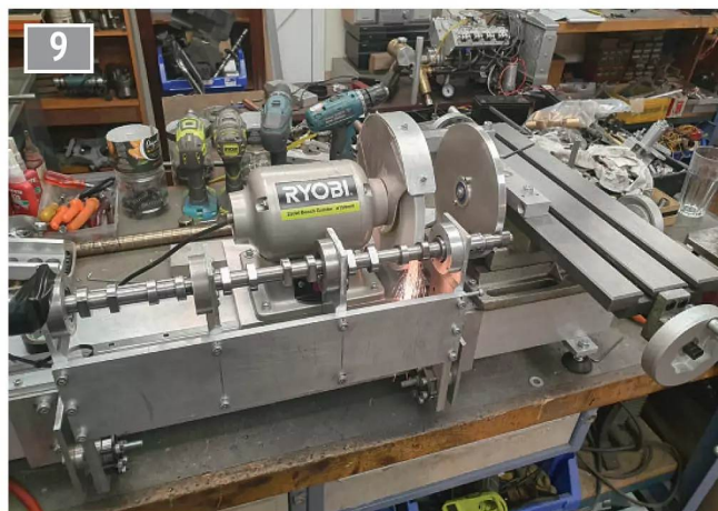
Home-made camshaft grinder.
