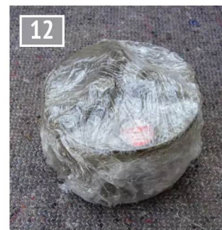
A lathe chuck that was over-wintered, between October to April, in a damp workshop that was heated occasionally. The chuck was old and previously very rusty before being renovated a few years ago – here it is oiled and wrapped in cling-film.
