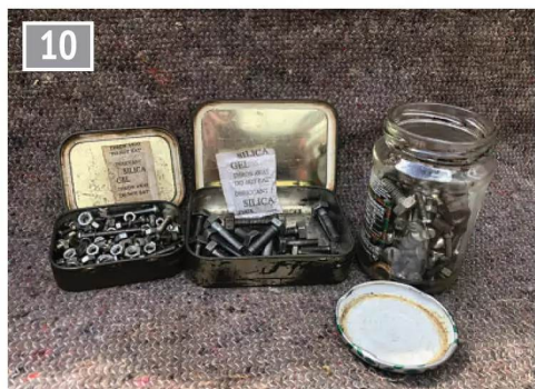
Small well sealed tins and jars are excellent containers to keep nuts and bolts rust free. Sprayed with WD40® and stored with a packet of silica-gel.
