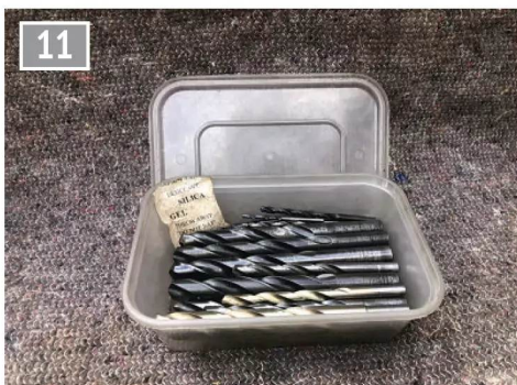
Plastic containers work well for storing larger items such as drill bits. Items were oiled and stored with a packet of silica-gel.
