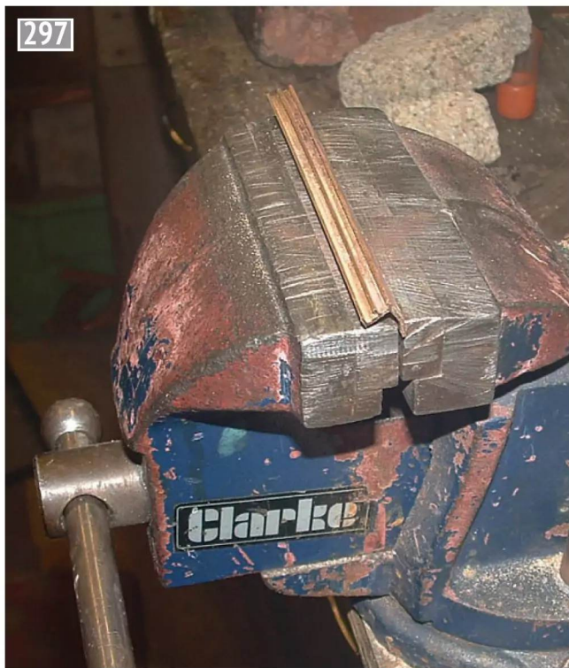
Bending over the upright on a window slide.
