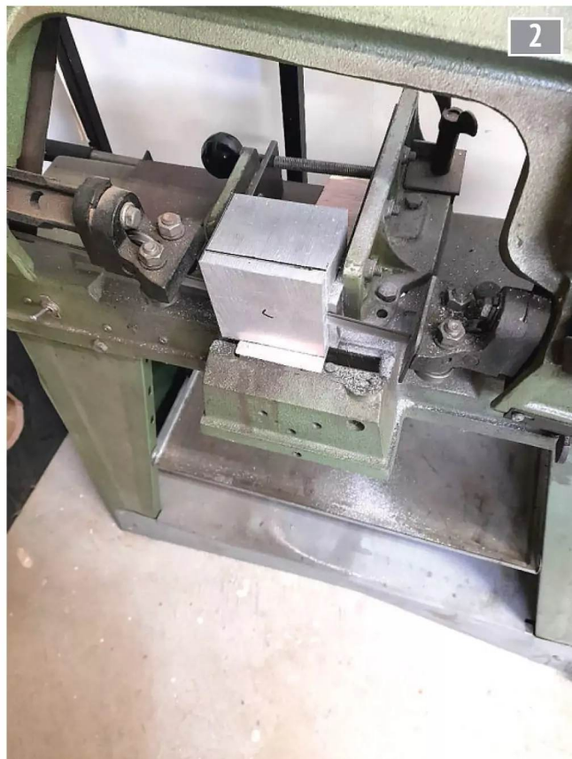
Band sawing the aluminium block to size.
