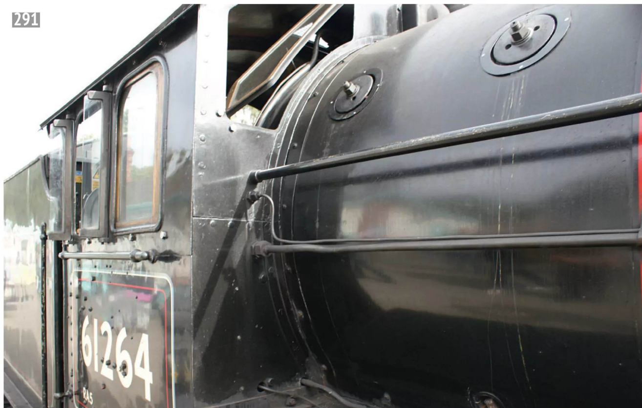
Close up showing the construction of the windscreens.
