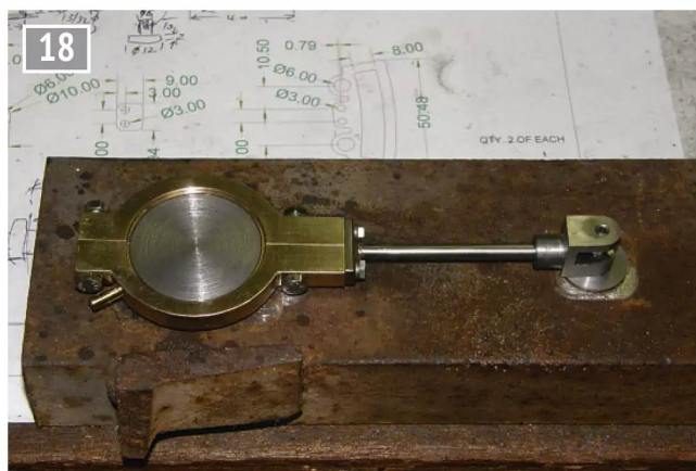
Here is one complete eccentric strap, valve rod and clevis, finish machined and sitting on the jig that was used to ensure the correct valve rod length.
