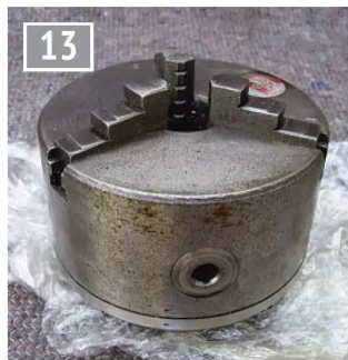
The chuck on unwrapping after winter and showing the worst area of corrosion.
