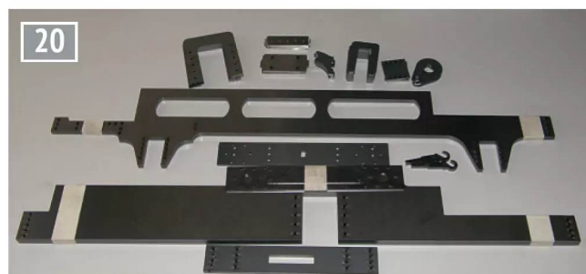
A kit of mild steel plates ready to be put together.
