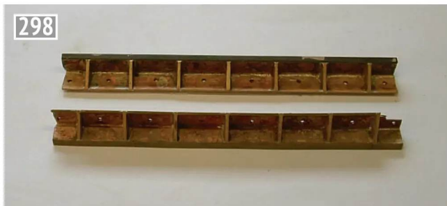
Triangular stiffeners soldered in.
