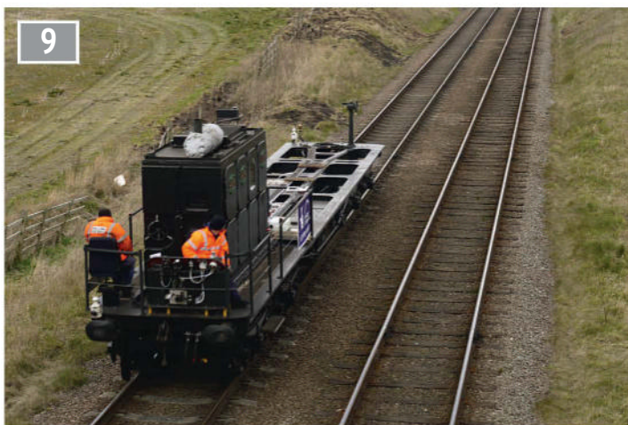
9 Underframe with Cummins engine under test on the Great Central Railway. Photo: Alan Chandler, 2016.
