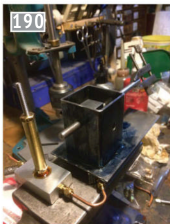
Testing the oil pressure release valves.
