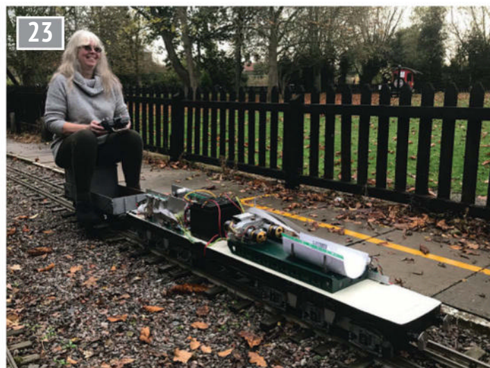
Helen gives the chassis a run at our local club track. The radio control system seems to work well, with good control of the locomotive, both forward and reverse.
