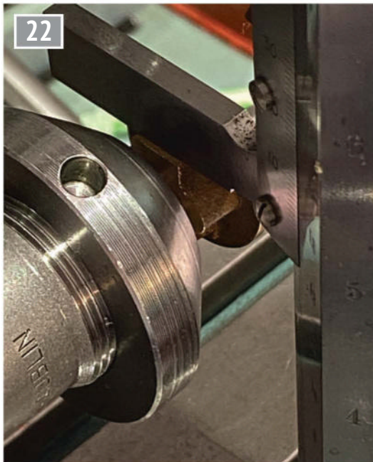
Setting the flats using the height gauge.
