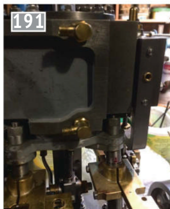
The two support brackets on the columns.
