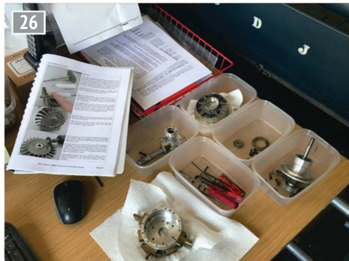
This shows some of the many parts of the turboshaft engine and reduction gear box.
