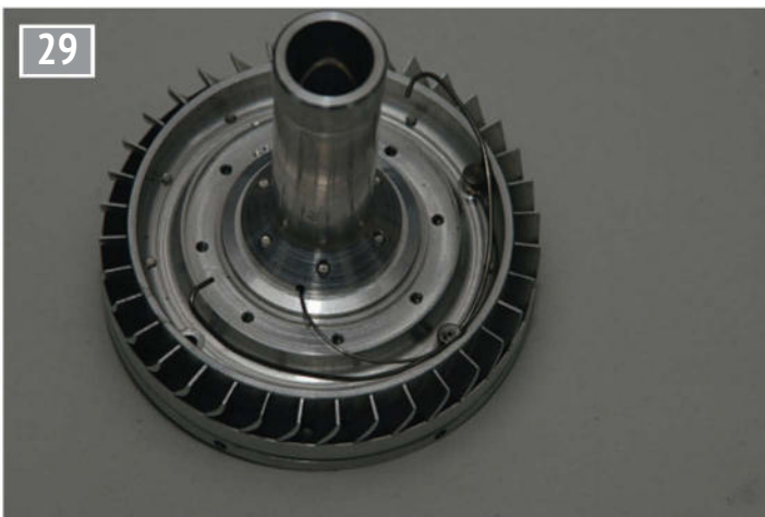
The diffuser and shaft tunnel united.
