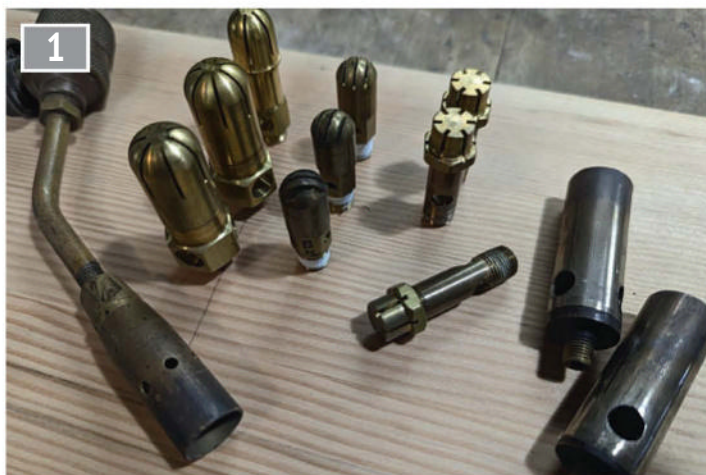
1 A group of Barber jets, star and fan pattern. With a couple of jet burners and a propane torch head as well.
