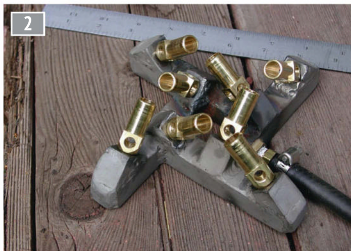
2 A home-made eight jet impinged burner with temporary gas connection for test.
