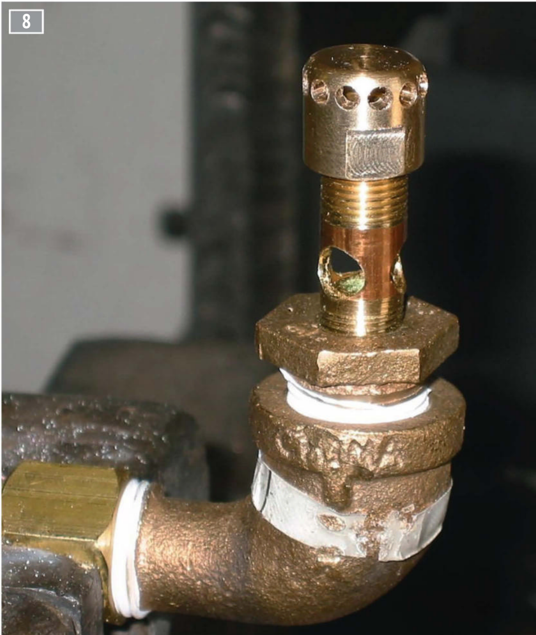
And I have to show this - Ken Brunskill was dissatisfied with the Marty burners he made and so he devised another top cap. I've named it the 'Brunsen Burner' and it works really well. It took a lot of experimentation but it gives a really good flame pattern.
