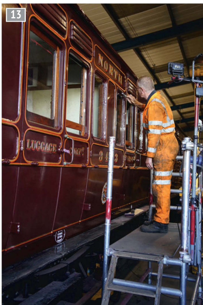
NER Autocar Trust volunteer, John Furness has done all the painting, varnishing and lettering and is seen here varnishing the trailer.
