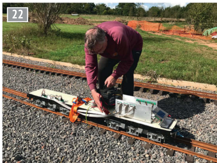
John Freeman connecting up the temporary traction batteries prior to the first test run of the complete chassis, on the Taunton club track.
