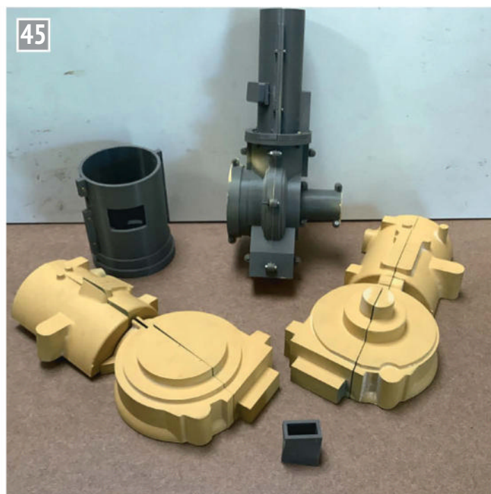
Engine pattern and core box.
