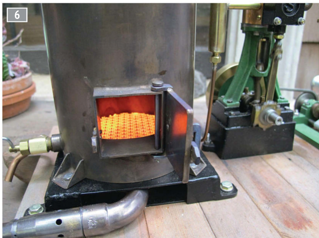
Here's a ceramic burner in a 4 inch diameter vertical boiler using a propane torch burner as a mixing system.
