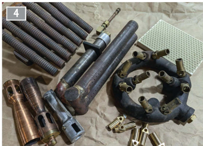
4 A really extravagant and a simple bar burner. A ten-jet impinged burner with extra, smaller jets that create less heat. Also, a ceramic burner tile and mixing venturis both home-made and salvaged.
