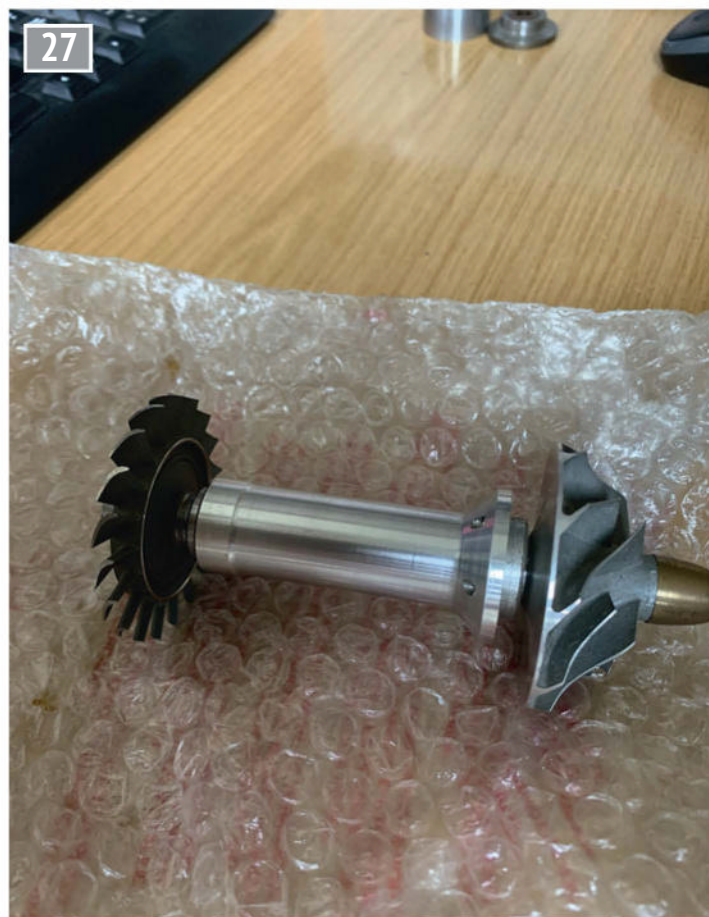
This is the heart of the turboshaft engine, the compressor, shaft tunnel and turbine wheel.
