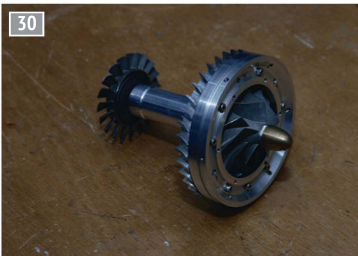
The compressor and turbine now fitted to the diffuser section.
