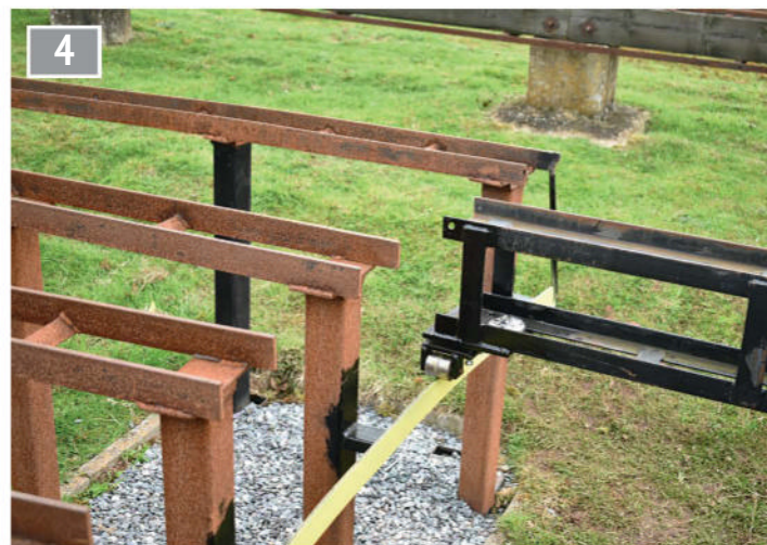
A smart roller keeps the traverser inline.
