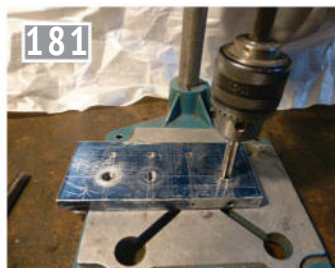
Tapping the bottom oil gallery plate.
