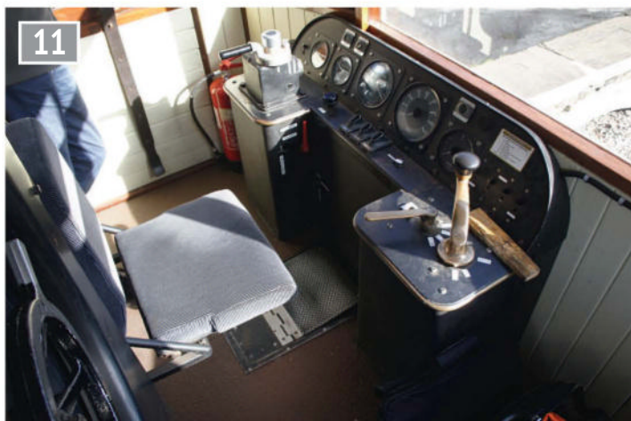
View of the driving position. Control arrangement is similar to British Rail era diesel locomotives.
