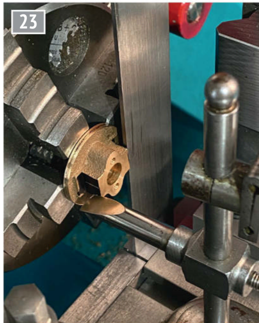
Scribing the centre of the flat to receive the slide bar assembly.
