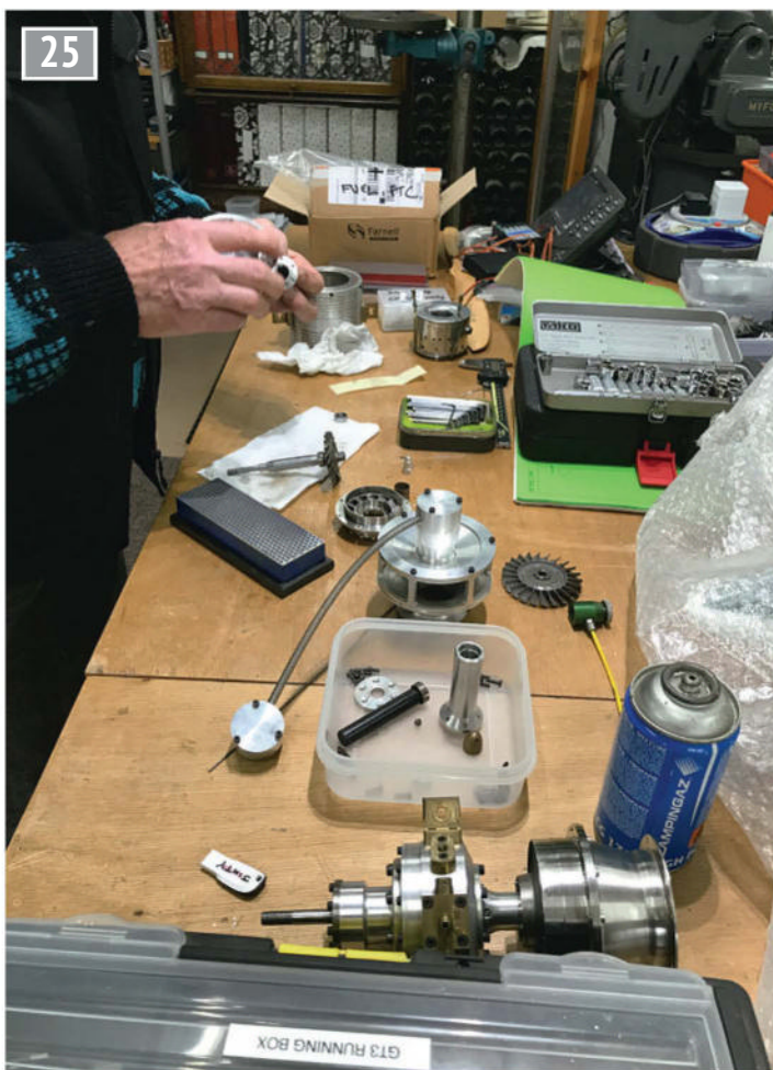
The turboshaft engine dismantled on James Hill's work bench. It turned out that quite a lot of work was needed to get the engine into running condition.
