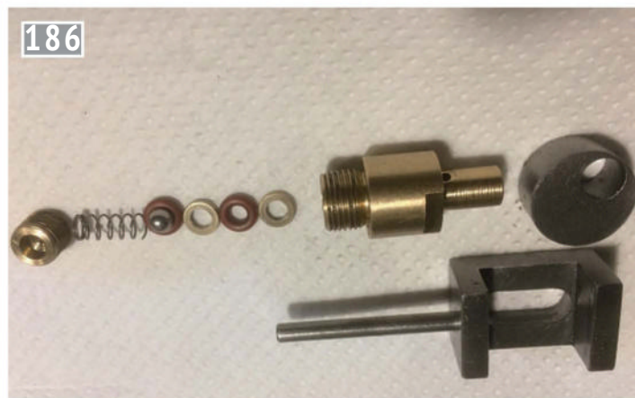
186 Pump components and ram.
