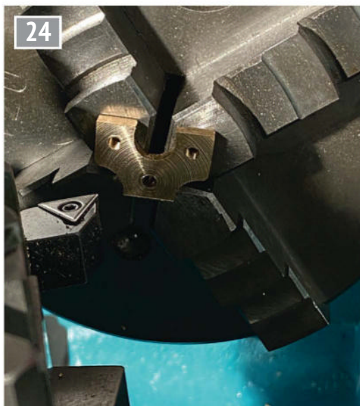
Facing an anchor block.
