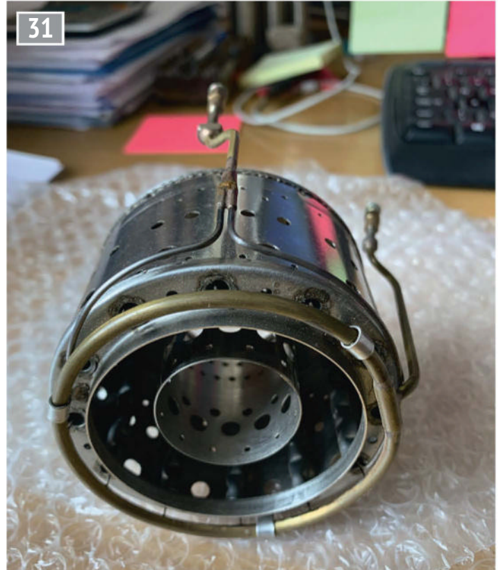
This is the 18 kW combustion chamber, as viewed from the back of the engine. The brass ring is the fuel supply to the 'sticks' which deliver vapourised fuel into the chamber.
