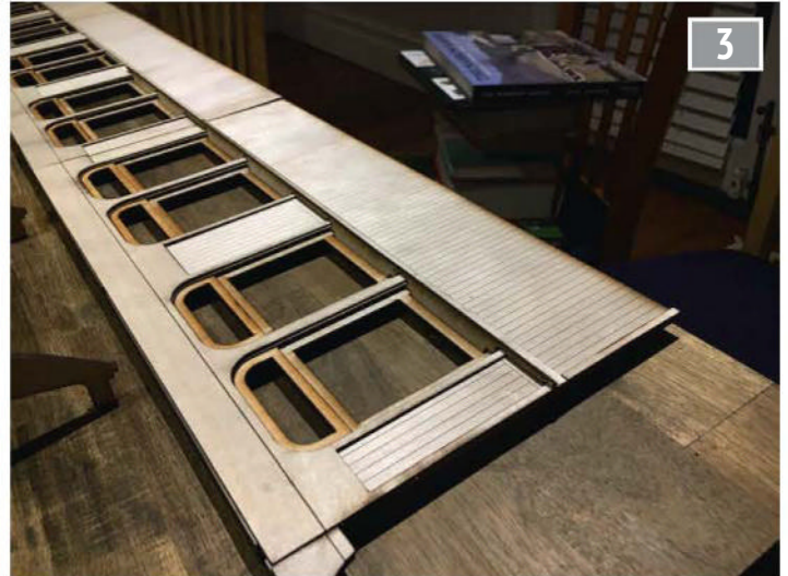
The sides were laminated out of laser cut plywood of thin sections.
