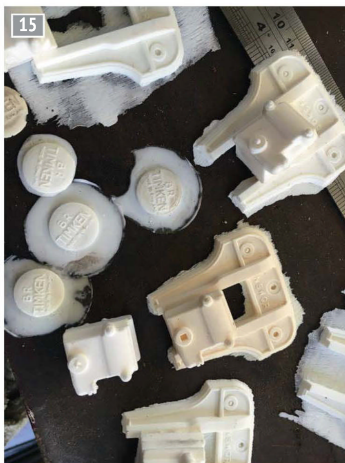
The 3D printed masters and moulds for the horn faces and axleboxes.
