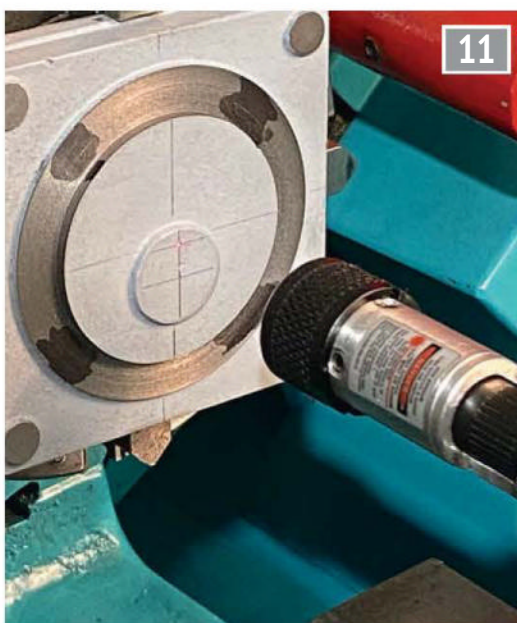
Laser used to establish centres on the base.
