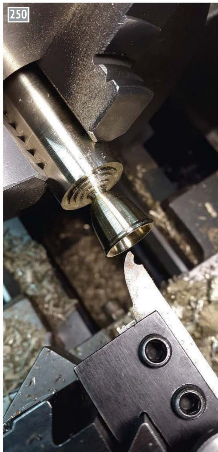
Using the second former to cut the inside of the sanding box.
