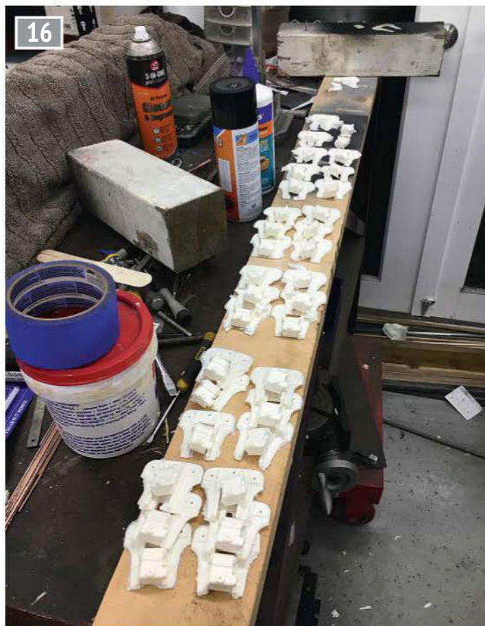
Here are the resin castings in groups making sure we had enough.
