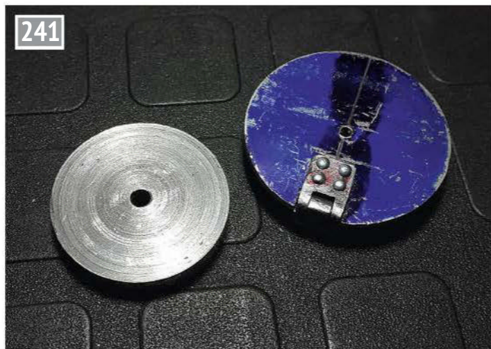
The tender filler cap with the backing bar for riveting the hinge. The hole in the middle was used for alignment and this was welded closed right at the end. Those little rivets were made from nails.
