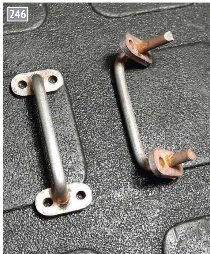
A completed handle on the left, and on the right, one that still needs to be trimmed and filed flush on the underside.
