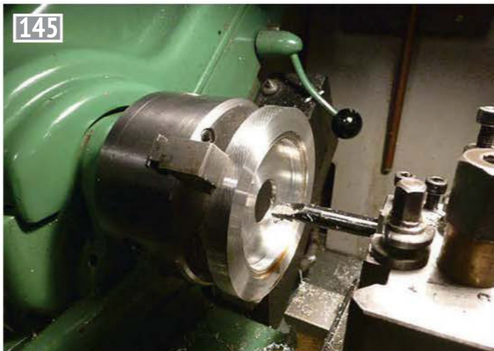
Boring out one of the end flanges.
