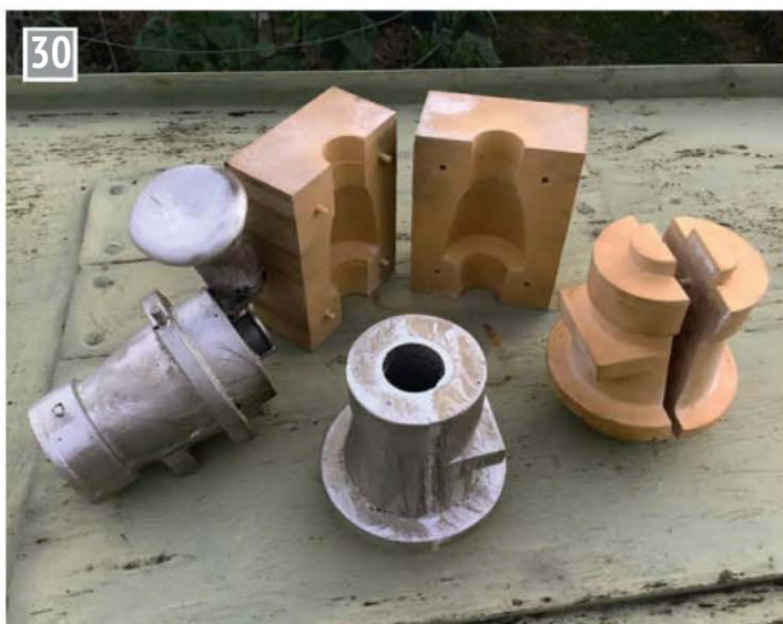
The pattern, core box and casting for the rear axle support. These bolt on each side of the gearbox.
