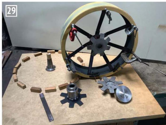
The wooden jig used to centre the rim and hub and help in fitting the spokes.
