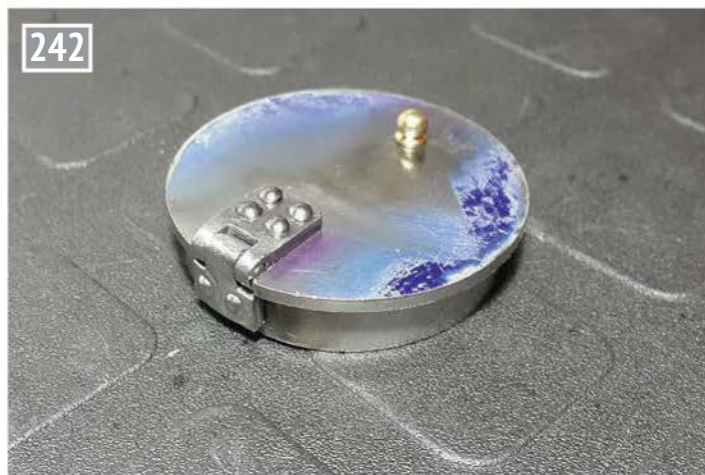
The completed filler assembly with the lifting knob fitted. I left this as brass because I thought it made a nice feature.
