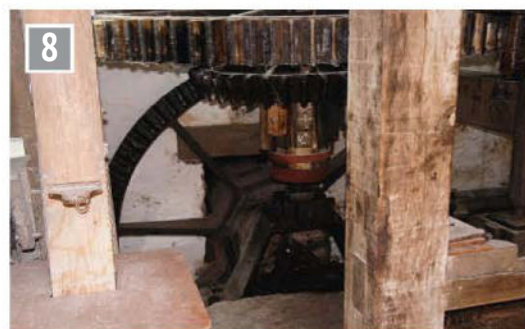
Inside the mill the vertical pitwheel, in the distance, is powered directly by the waterwheel. They are mounted on the same axle.
