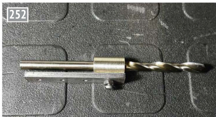
Brake lever bearing carefully aligned with the base plate (eyeballing is good enough), and a retaining screw at the bottom to keep it in place during soldering.
