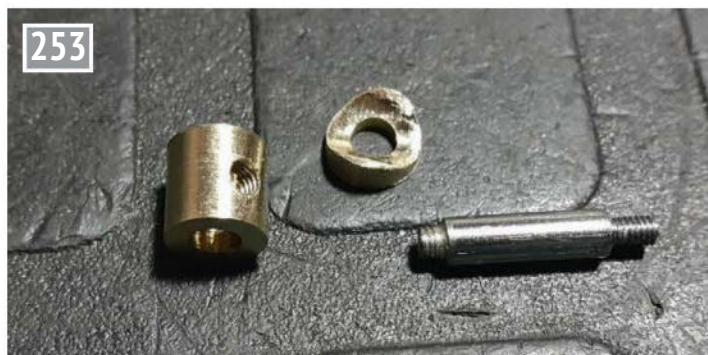
The T-piece for the top of the brake lever. A silver steel shaft screws through the bearing and the shoulder of the bearing, with a small amount of silver solder used to keep the lot together.
