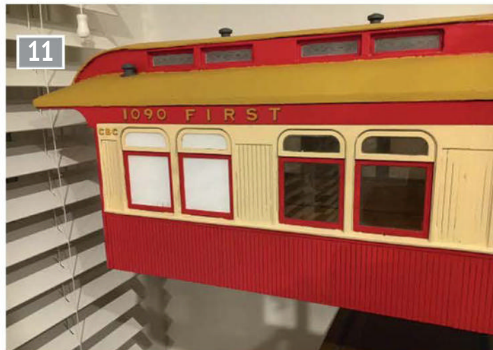
Waterslide transfers in the NSW font were commissioned from a supplier who made them for HO scale but enlarged them to suit our scale.
