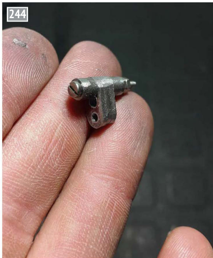
The handle mounts that were filed in a stack using radius guides.
