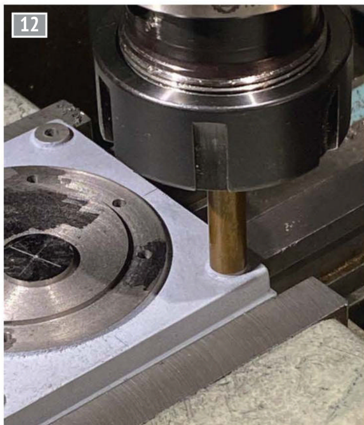
Alignment procedure to find the centre of bolting spigots.
