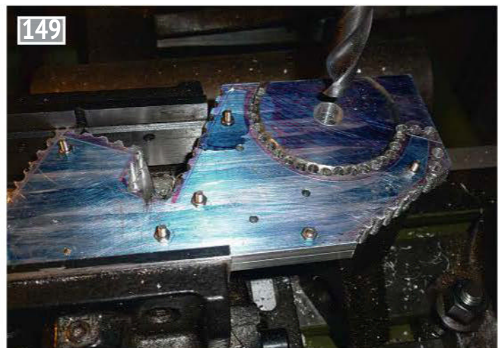
Drilling the centre of the chain drilled plate to allow the use of a boring bar.
