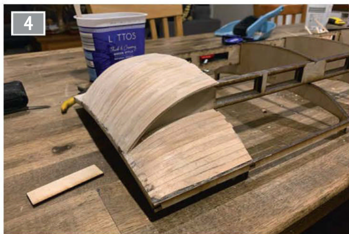
The ends were fabricated out of thin planks. Here the planking is complete. Each plank was steamed and dried to shape prior to gluing on.
