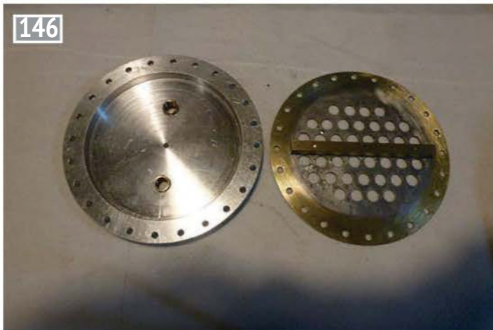
An end cap and its tube plate. The brass strip which forms the coolant divider is fixed on the tube plate but is also screwed to the cover on assembly.
