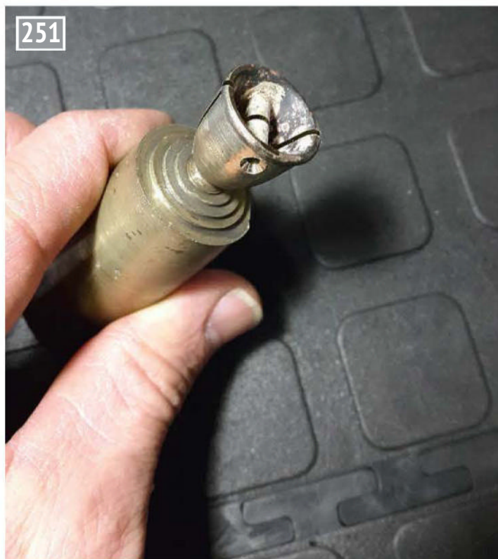
The centre screw guide (for assembly repeatability) soldered in place and the two sanding bars split using a thin slitting saw.
