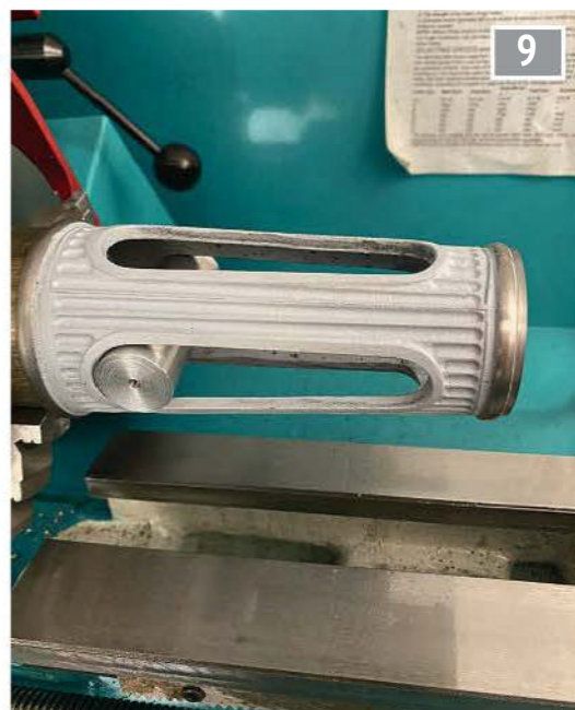
Column bolted to brass spigot to machine the top surfaces.
