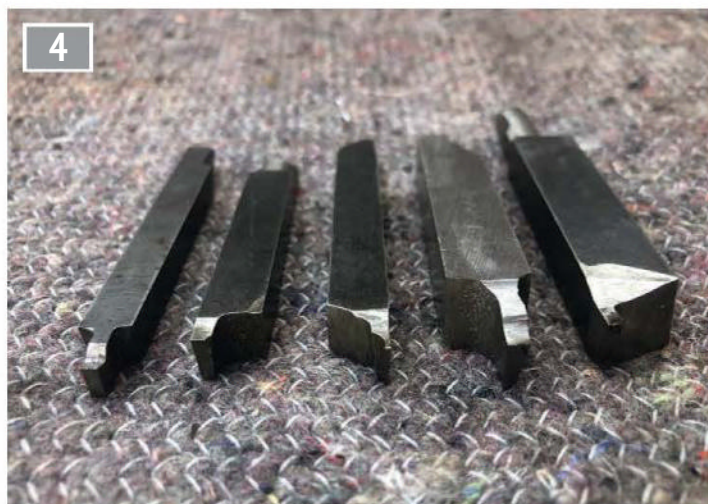
Collection of HSS parting tools formed from HSS blanks. The tool positioned 2nd from the right was the one used to perform the parting cuts discussed in the text beneath.
