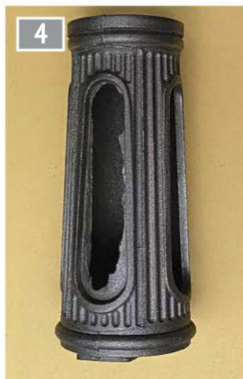
Thin hard flashes around openings in the column.
