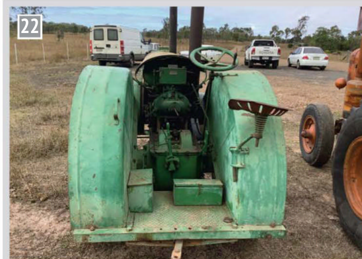
22 A rear view of the tractor showing the gear lever selector handle and the top cover of the gear box. One of the tool boxes on the floor houses the blow lamp for heating the hot bulb for starting the engine.
