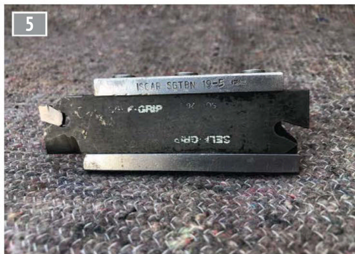
A carbide insert parting tool positioned in a toolholder. By using a separate toolholder the narrow blade is able to extend deep into the parting cut.
