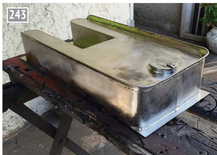
The completed tender tank, ready for a little beautification.
