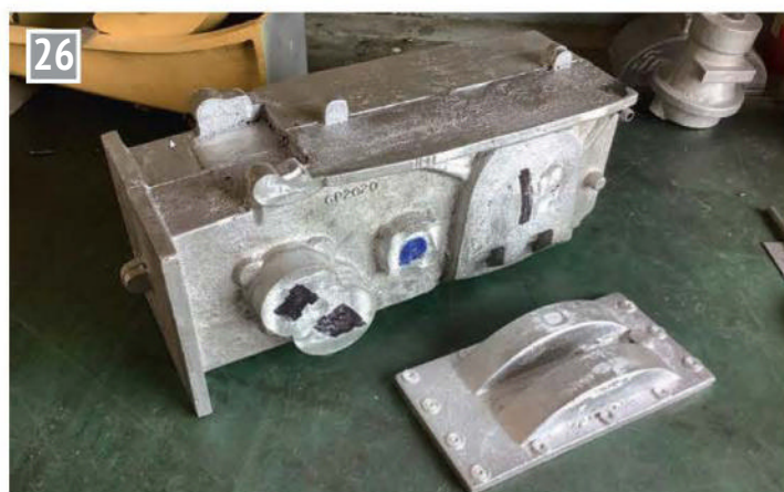
26 A dry assembly of the gearbox with the cover casting in the front. The top of the box has yet to have the opening cut into it.
