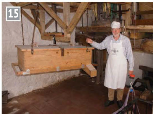
Mill gearing also operates this jigger. It shakes and grades oatmeal. Seen here with Neil Hannah, the miller on duty at the time of my visit.
