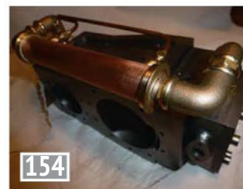
Trial fit on the cylinder block.
