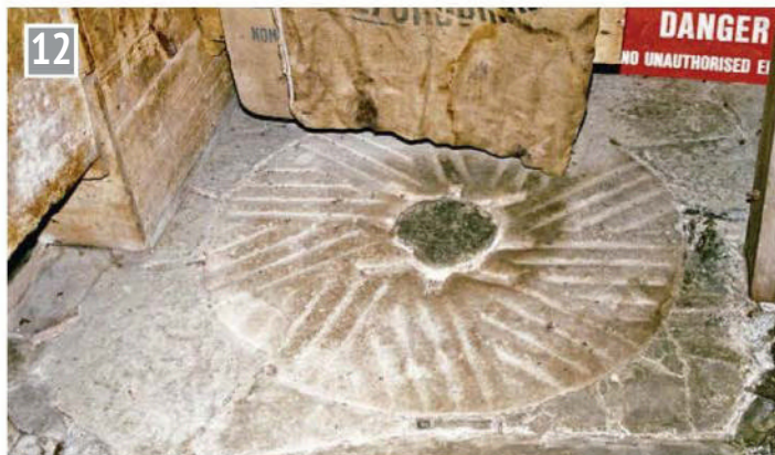
Millstone at Acorn Bank mill showing grooves directing flour or oatmeal outwards.
