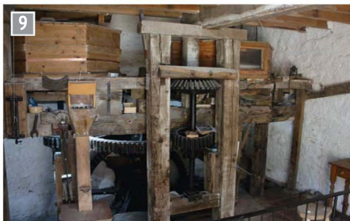
The great spur wheel is the large horizontal gear wheel. The smaller is in front of a stone nut, temporarily disengaged. Boxes above and behind hold the pairs of millstones. That on the right has a window to show operation.
