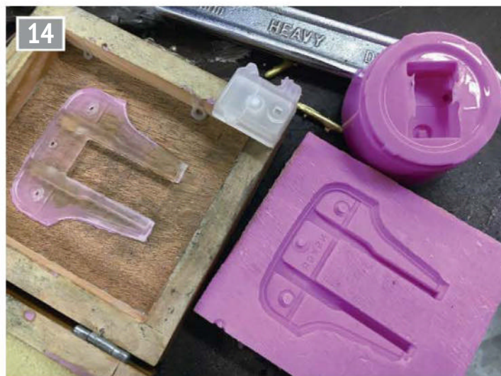
The 3D printed masters and moulds for the horn faces and axleboxes.
