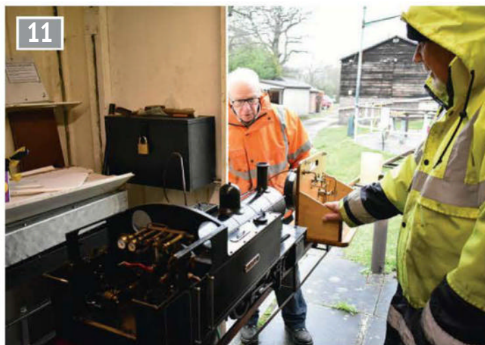
David Shrimpton's Simplex undergoes its boiler test.
