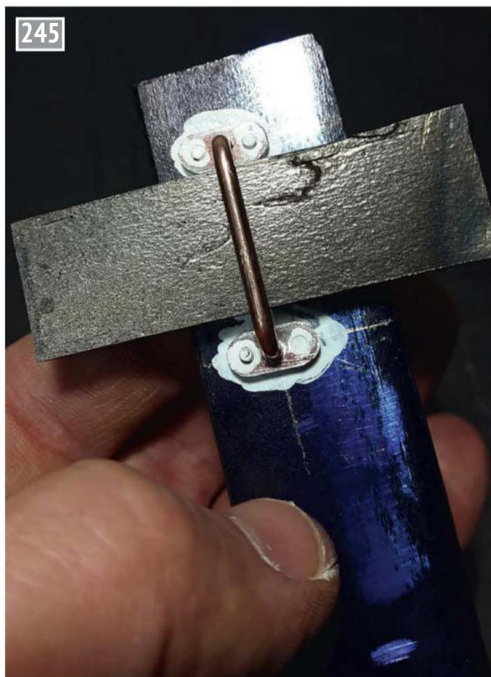
The handles being soldered together using a jig and Tippex to keep the solder away from unwanted areas.
