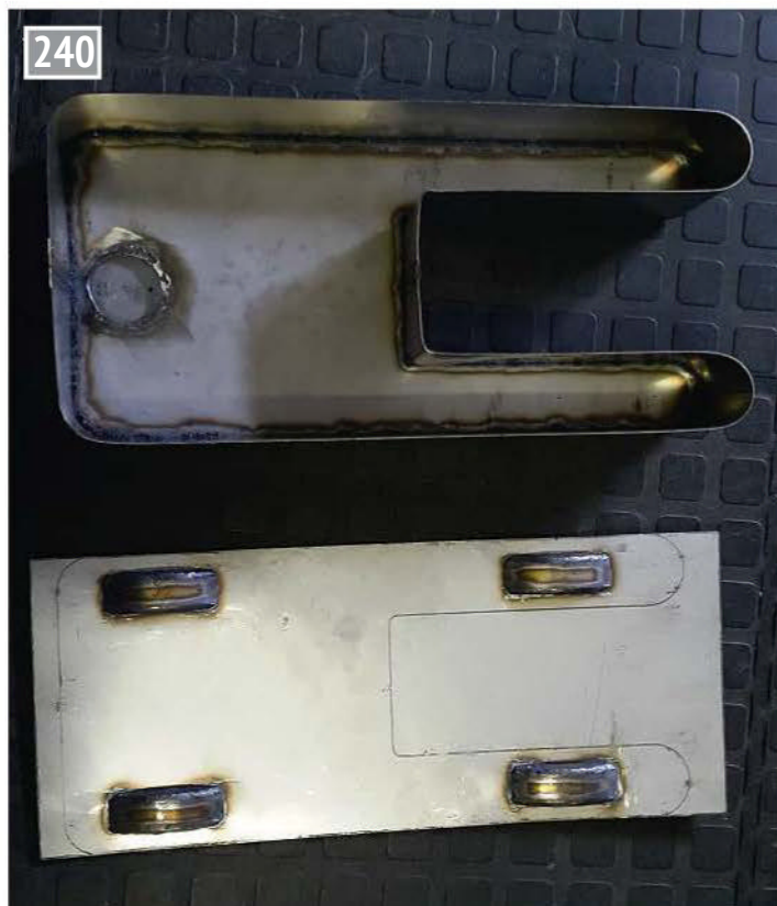
The beginnings of a TIG welded tender tank. The tank consisted of only a few components, with the sides a single piece welded to the top and bottom plates following the engraved line.
