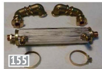
Balsa insulation and the two cladding retaining straps.
