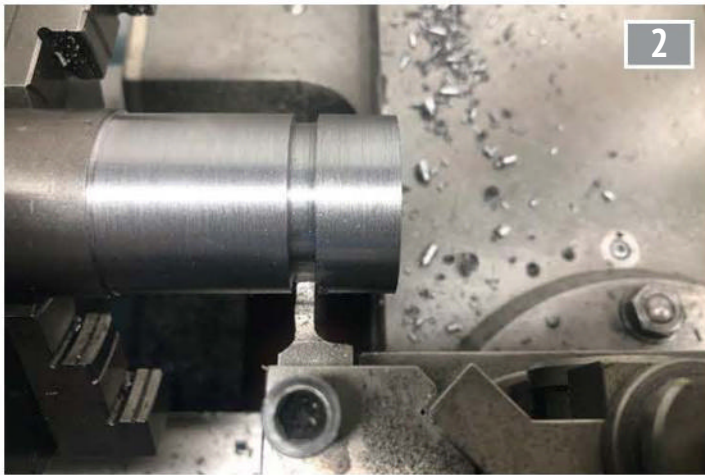
2 A parting cut that was taken into EN1A low-carbon mild-steel bar using an HSS parting-tool. The lathe was stopped and the tailstock removed to improve the image.
