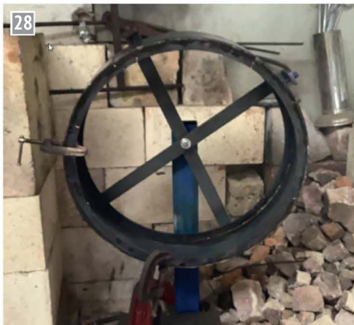
The rear wheel rim on the jig ready for silver solder to be applied.
