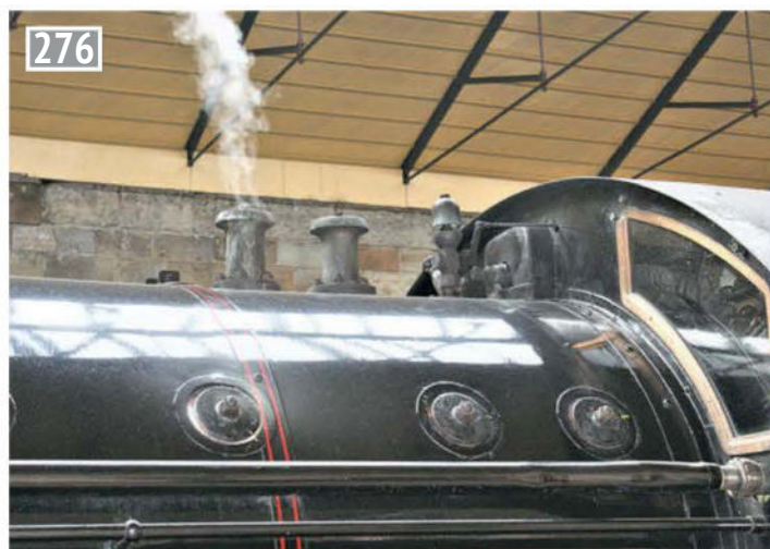
Safety valves on an LNER B1 locomotive.
