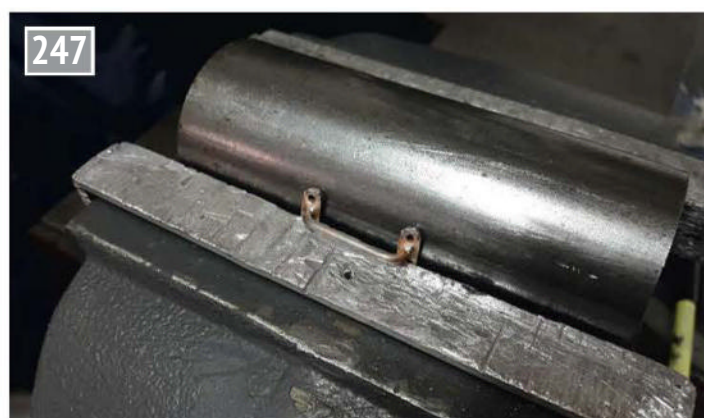
Bending the handle mounts on a suitably sized piece of bar stock with the reaction side held in the soft jaws of the vice. Unseen in the picture is a set of makeshift parallels under the round bar to keep it in place when slipping the handles between the bar and the vice soft jaws.
