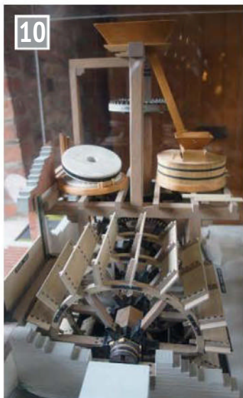
Gear wheel teeth section. Cast iron replaced wooden gears during the 19th Century.
