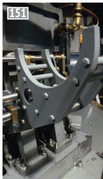
Trial fitting of finished bracket.
