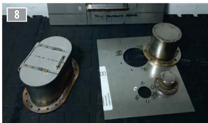
Selected rolled items with flanges already welded in place.
