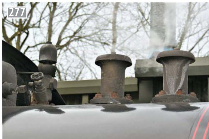
A closer view of the safety valves from the other side.
