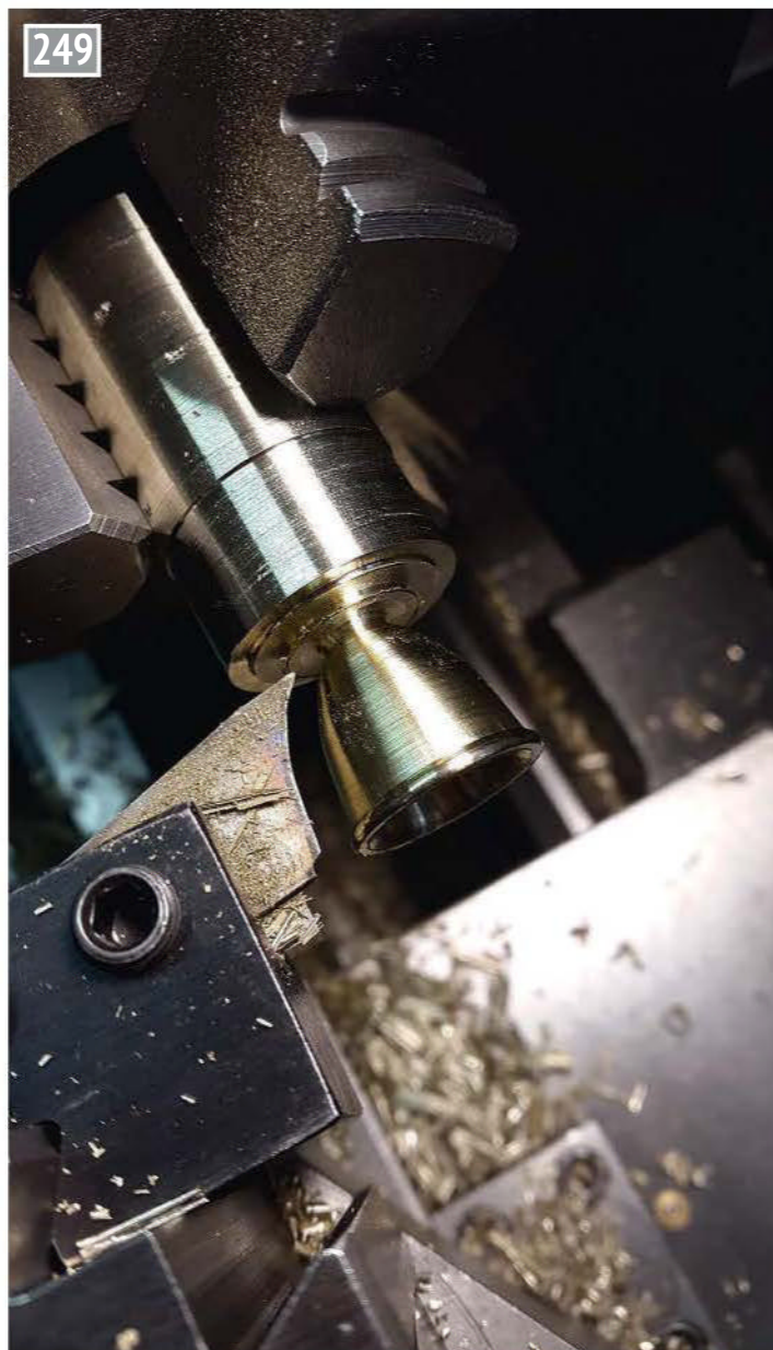
Using the first former to cut the outside of the sanding box. Note the outer lip is part of the forming tool, which is relatively easy to grind by touching the corner of the grinding wheel.
