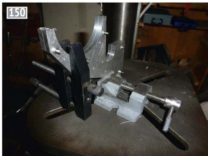
Drilling the strap fixings tapping size.
