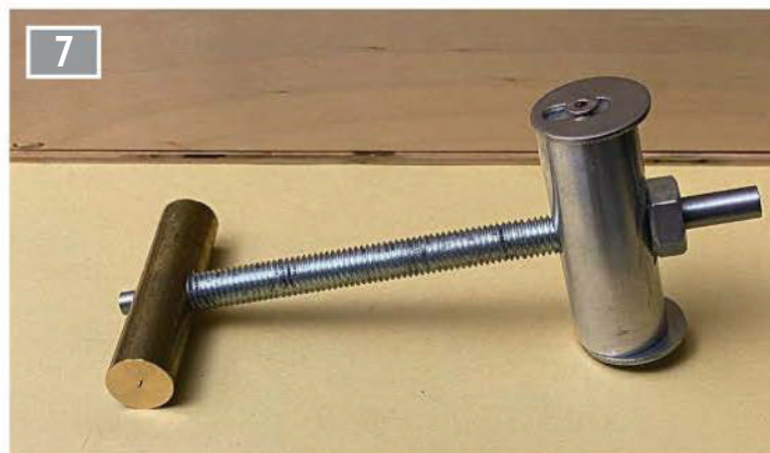
Jig for holding the column.
