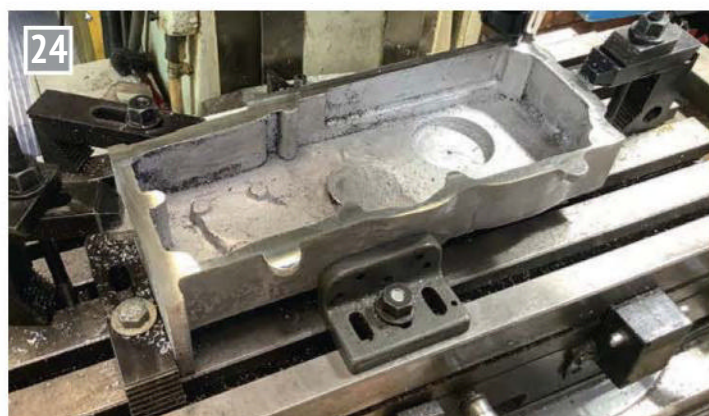
24 Machining the joint surface with a fly cutter.
