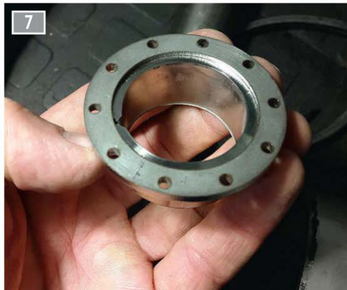
7 A 3mm stainless rolled ring ready to be welded to a laser cut flange.
