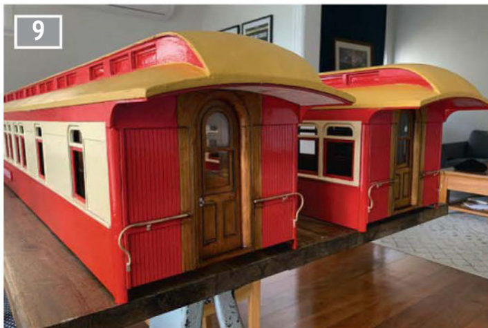
End doors and handrails fitted (mostly hidden with the vestibule added).
