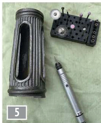
Tools used to remove flashes.
