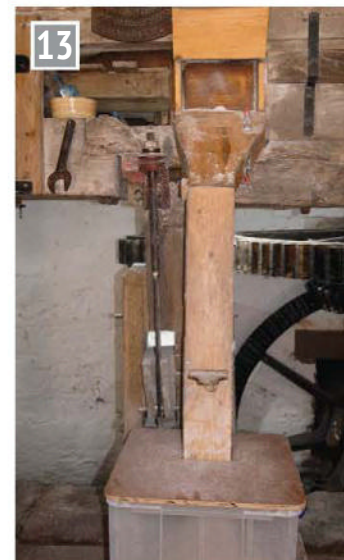
A shoot takes flour from the stones to a container ready for bagging.
