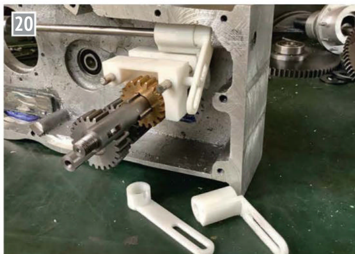
Prototype gear selectors made on the 3D printer. The shapes of these were later changed and made in steel.
