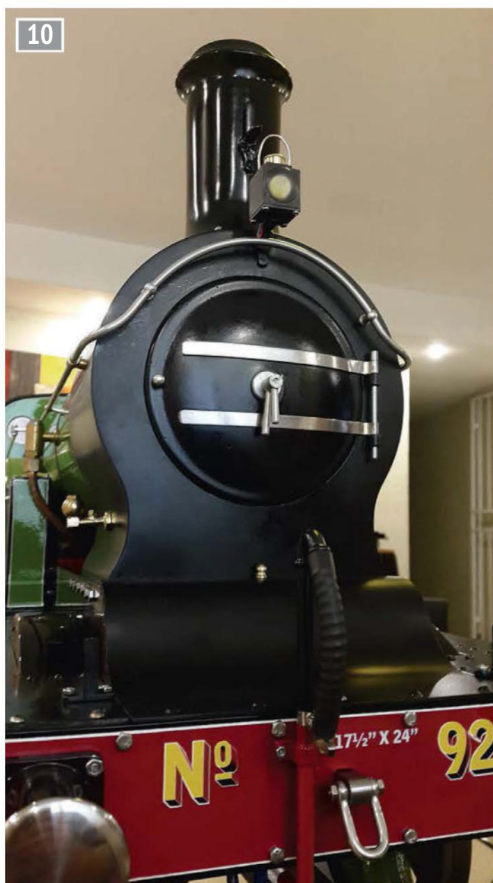
Stirling front hand railing with LED light.
