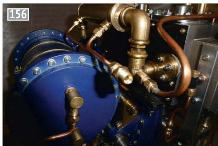
Union on the pipe elbow at the entry to the receiver to accept the steam from the simpling valve.
