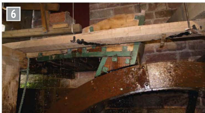
From the launder water falls on to the pitchback wheel which revolves in the opposite direction to the flow in the launder.
