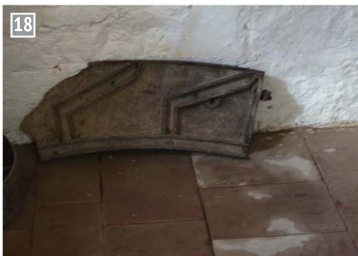
18 A cast iron shroud forms part of the edge of a waterwheel. There are plans to restore the second wheel.
