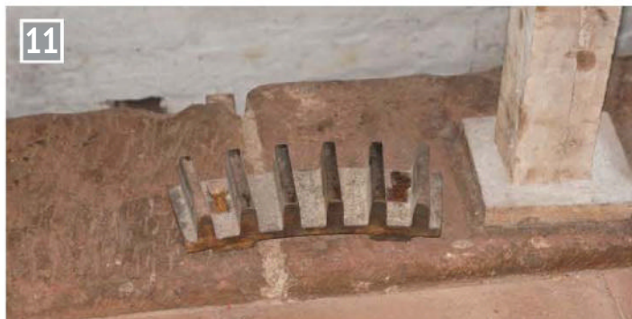
Gear wheel teeth section. Cast iron replaced wooden gears during the 19th Century.
