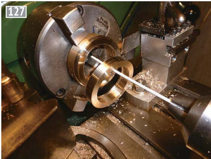
127 Parting off one of the four bearings.
