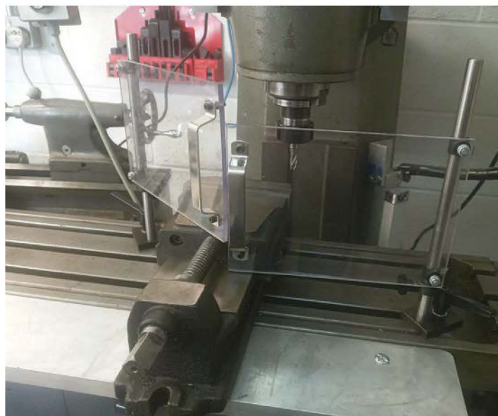
The guards are in place – easily adjustable to avoid clamps, vices etc.
