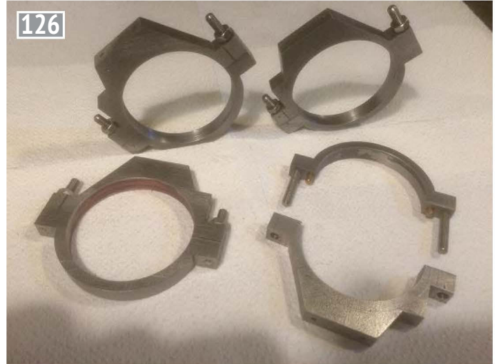
126 The four straps minus the bronze bearing liners.
