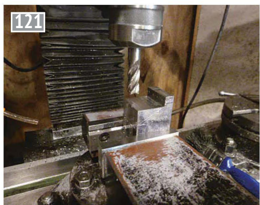
Milling all four halves as a block.
