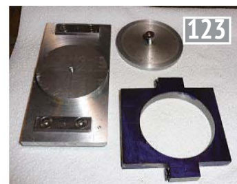
Jig made up to hold the two halves for milling on the rotary table.
