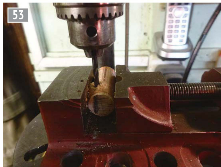
Drilling for the steam pipe.
