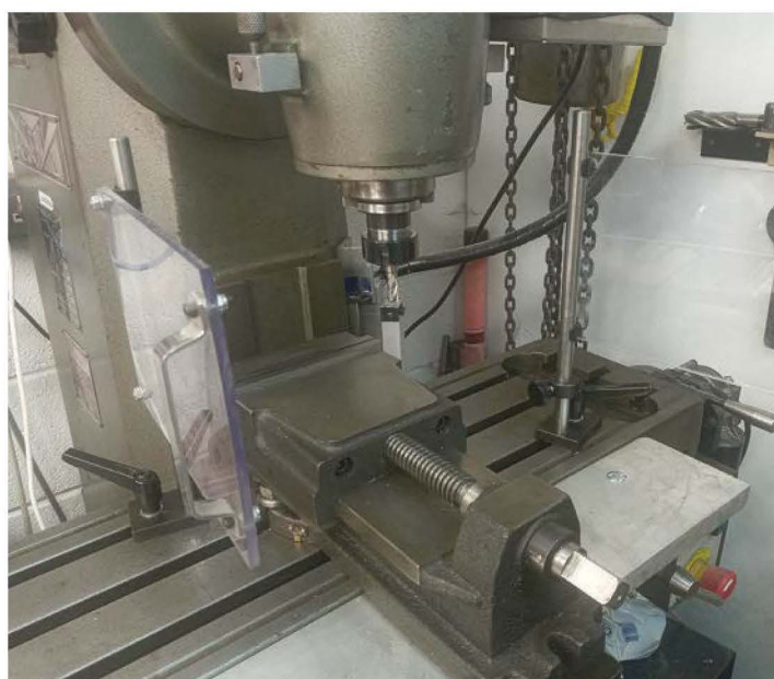
The guards can easily be swung away for setting up.
