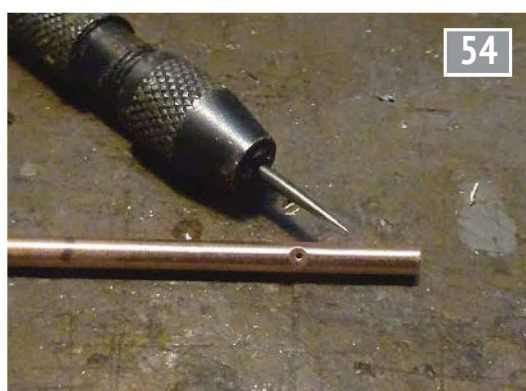
Hole in the steam pipe.
