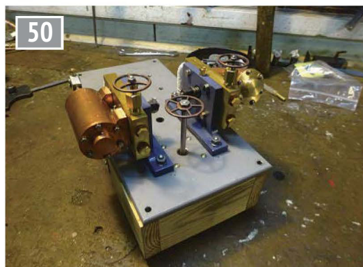
Valve fitted to base plate.
