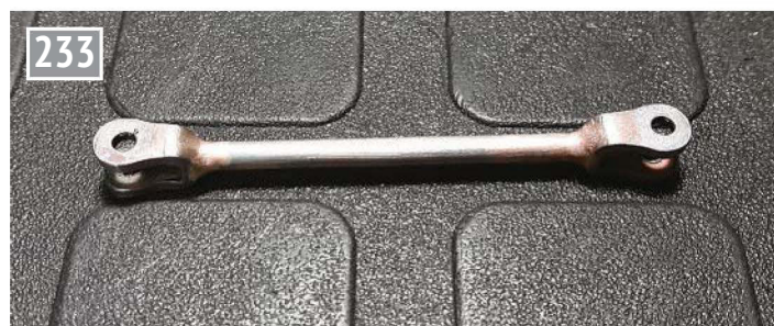
A completed coupling rod brazed and ready for chemical blackening.
