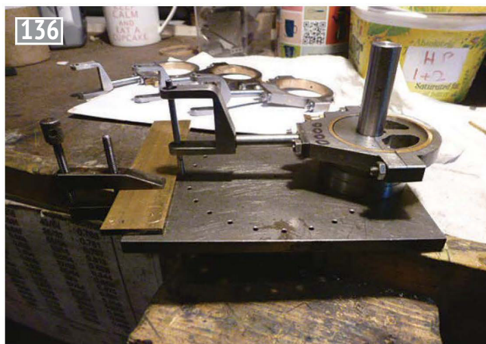
Strap on a measuring jig to ensure all are the same length.
