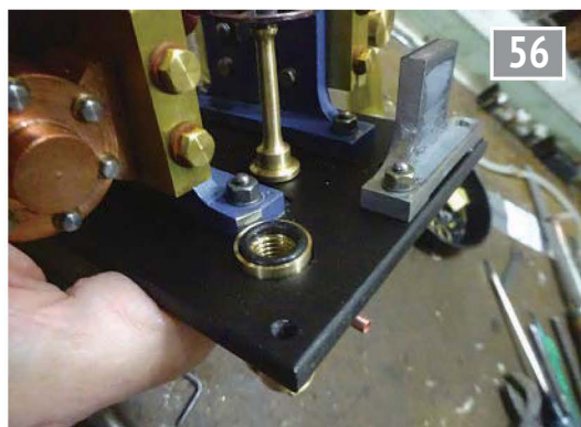
Top soldered in place.
