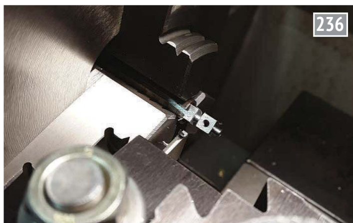
The brake block machined from one piece of key steel for improved strength.
