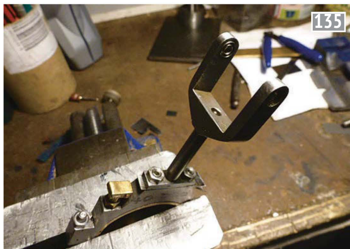
Held in a vice to fit shims under the foot.
