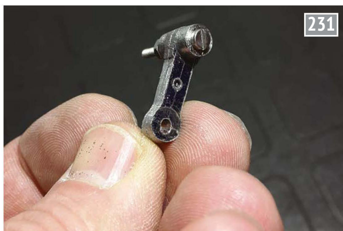
Filing the brake coupling ends using radius guides. Note how they are stacked to decrease manufacturing time.
