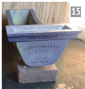
15 The finished casting of the chassis and radiator base showing the lettering detail. The tray part on top of the chassis is the base casting of the radiator.
