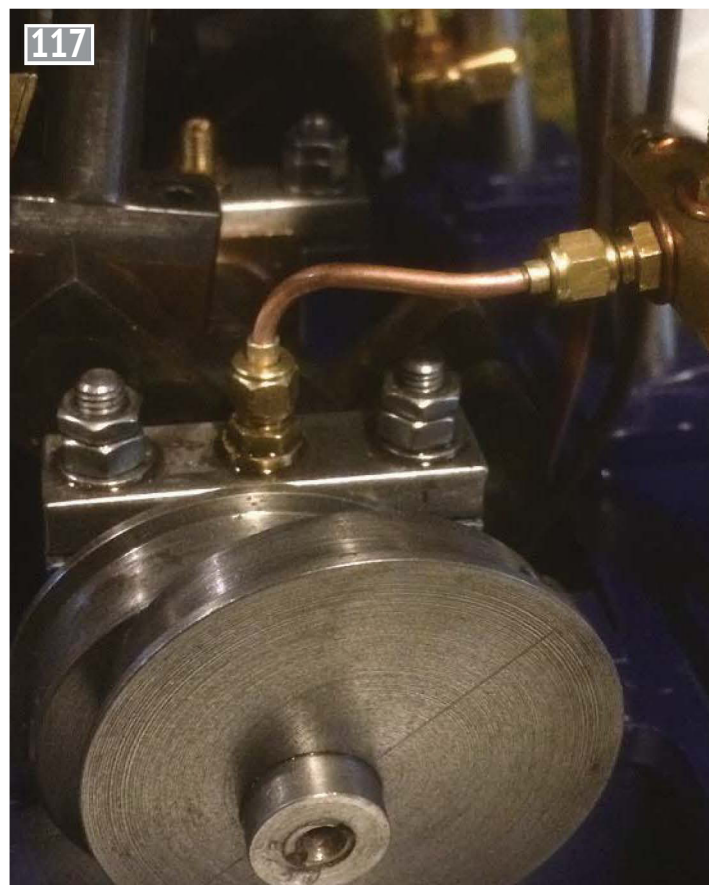
Plain disc eccentric with a flange on one side.
