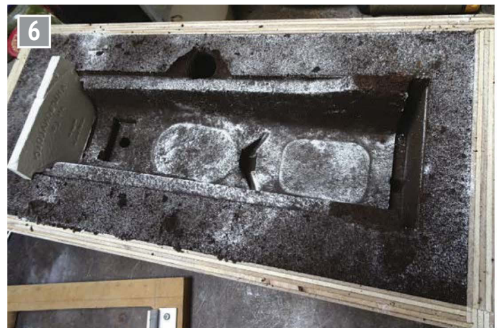
The sand mould showing the name plate at the front.
