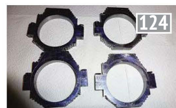
More chain drilling.
