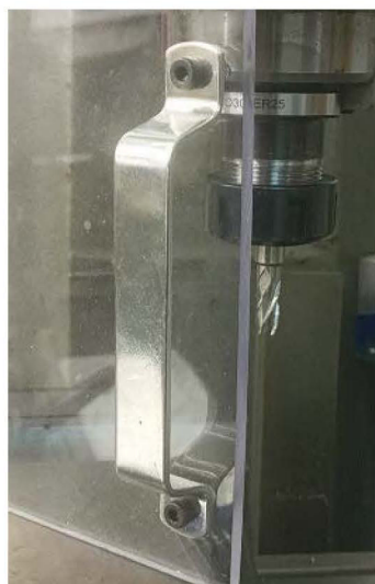
The guards are equipped with handles for easy adjustment.
