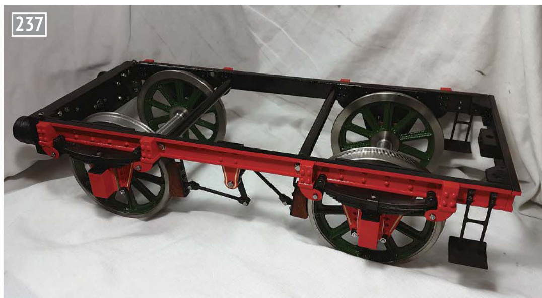
The tender frame completed and painted ready for the tank.
