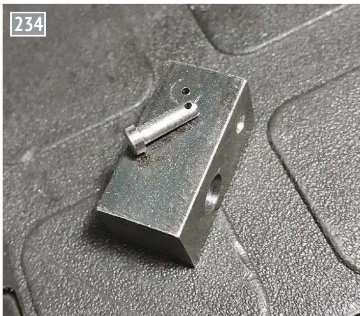
A simple drilling jig made to standardise on the pin lengths, making them interchangeable. One or two spares are worthwhile with such small components that can get lost on the track.
