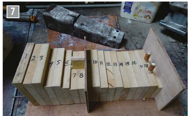
The outside of the laminated core box.
