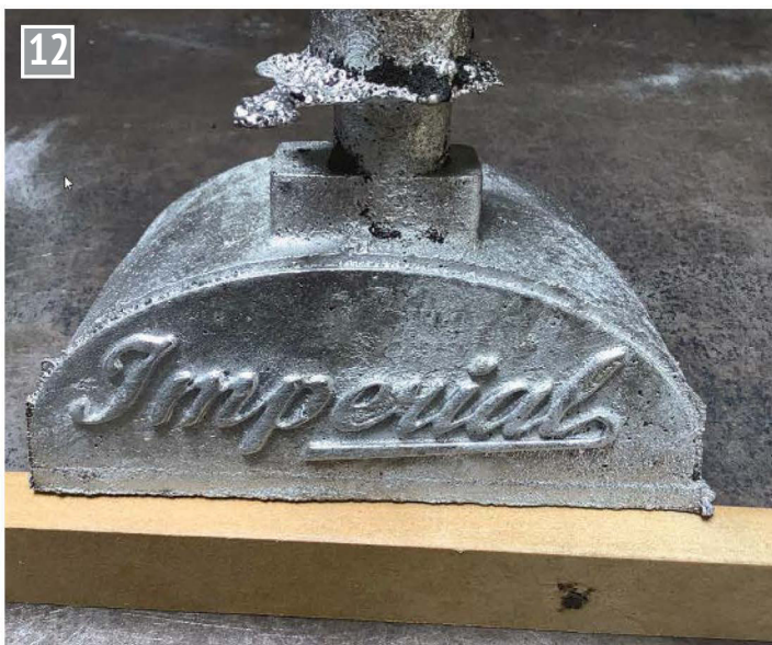
The radiator top as cast and before cleaning up.
