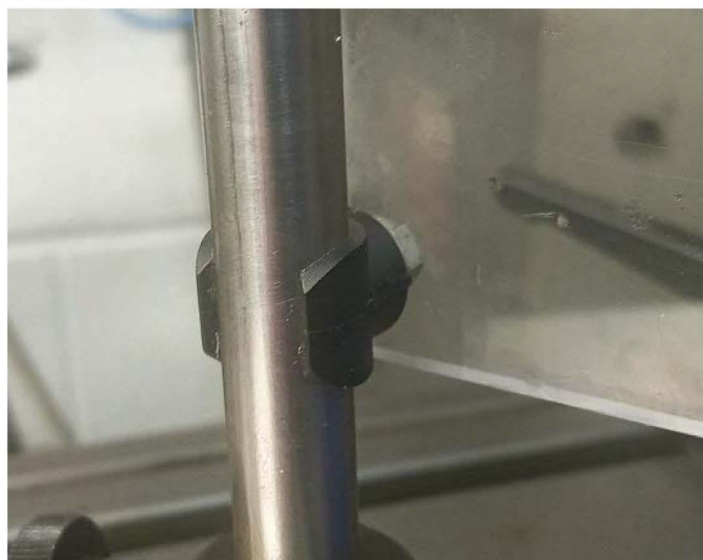
Pipe clips secure the Perspex and allow easy adjustment.
