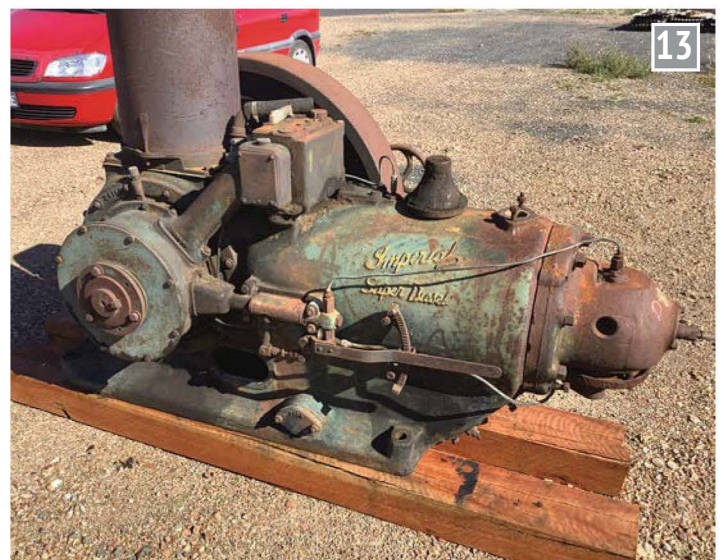
This is a 70bhp two stroke McDonald engine and looks very much like the tractor engine only larger.
