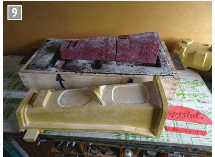
This shows the pattern – the core is ready for the upper box to be placed on top.
