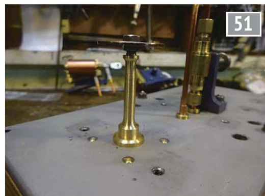
Reversing valve finished.
