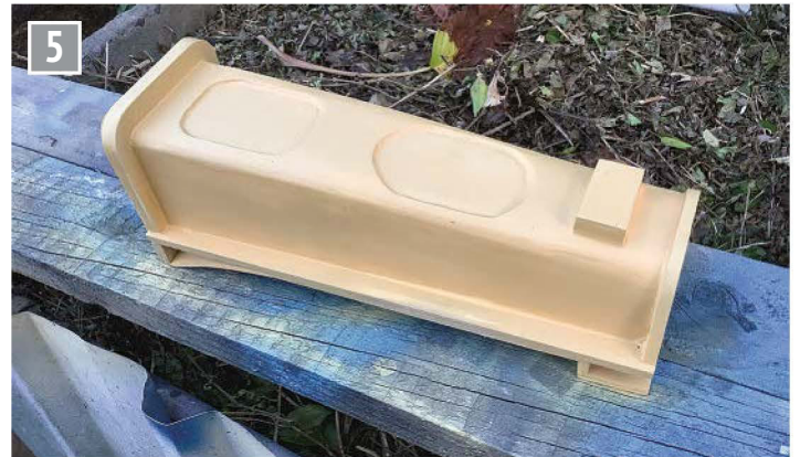
The chassis pattern turned upside down and made from MDF.
