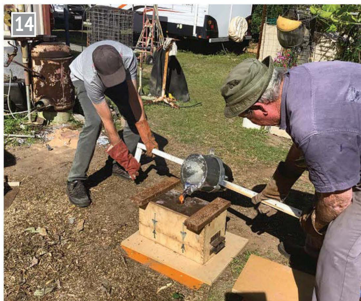
14 Pouring an aluminium casting with my mates John and Ray doing the heavy work while I take the photograph.
