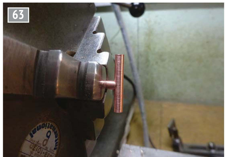
Wringing 'T' connector parts together for soldering.
