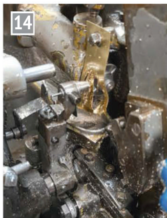
The arm presents the screw to the slitting saw.
