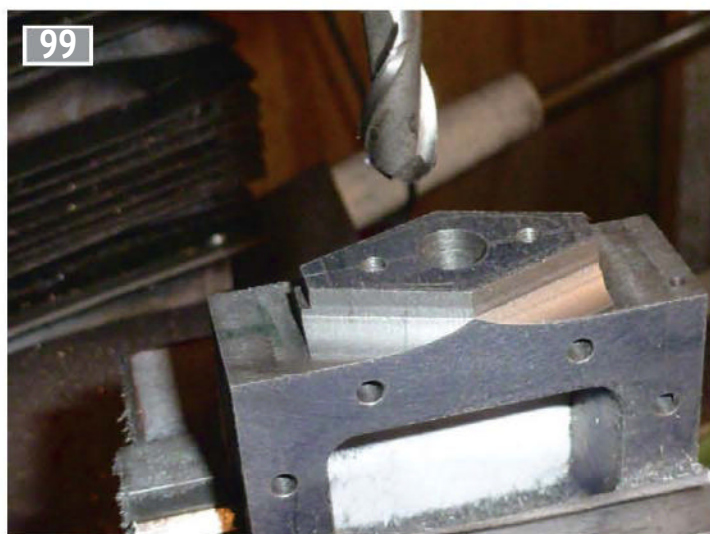
Milling the shape of the gland housing with a ball ended end mill.
