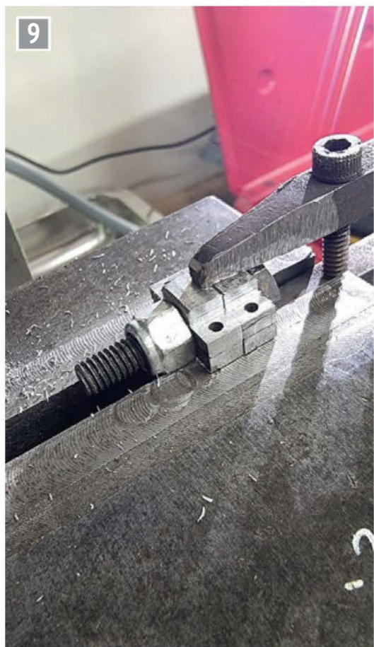
For the other side, I added a small tool clamp (needed a little ground off) and this time sat the blocks on top of the jaws to finish the machining.
