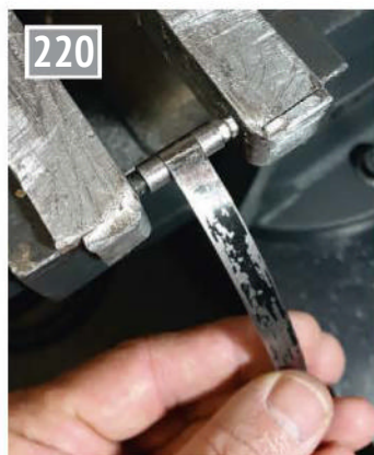
Neatening the ends of the spring using radius guides and a little hand dexterity with the file.
