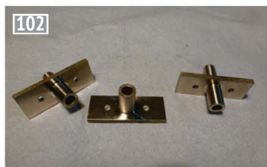
The two types of gland. The top cover with the sealed tube through the flange, and the bottom with the tube on one side to compress the O-ring or packing.
