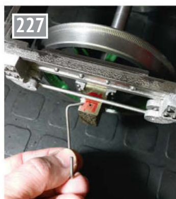
Checking the position of the spring cradle locating hole.
