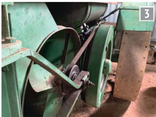
McDonald tractor – flywheel and cooling fan.
