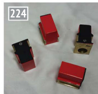
The completed axlebox assemblies all painted with the top plate fitted ready to go onto the frame assembly.
