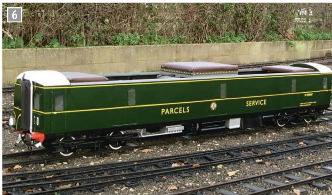
This is a general view of the completed model. It was originally intended to make a pattern for the bogie detail but due to Covid restrictions we ended up fabricating these.
