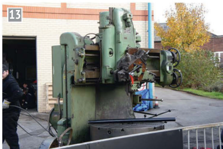
Webster-Bennett vertical boring machine built circa 1950 on the way to the Strathspey Railway. The final disposal of a once well equipped workshop that always interested visitors. This was used for boring locomotive axleboxes producing the so called 'Collett Wedge' which was important for good lubrication in a white metal axle box. Many famous locomotives including Green Arrow, Duchess of Hamilton, City of Truro and the LNWR Super D plus many others were done on the machine. Other machines like an Elliott vertical slotting machine came from the nearby carriage works and were a part of York's railway heritage. That too has gone.
