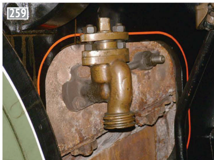
Full-size blow down valve.
