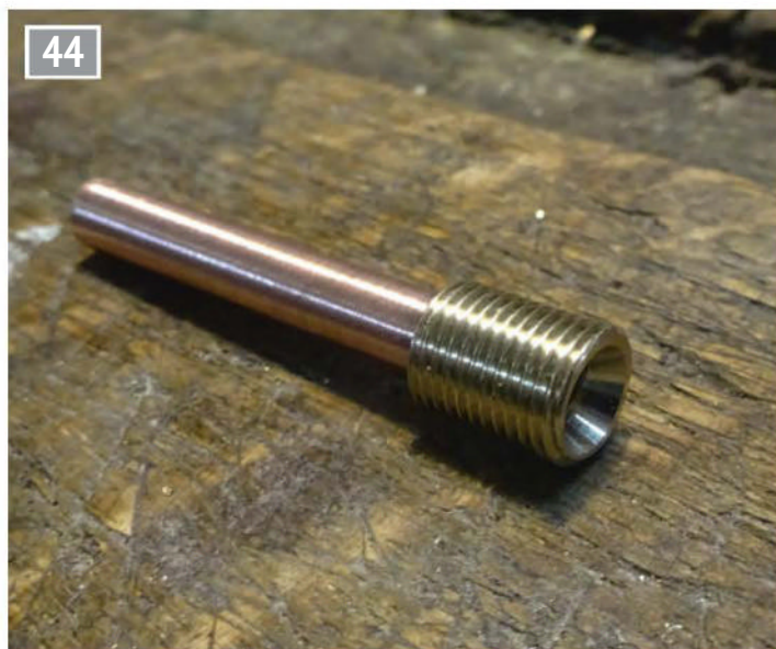
Pipe and union.
