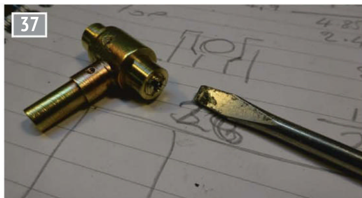
Feed pump ball seating screwed in.
