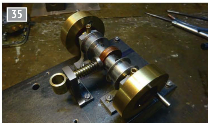
Modified feed pump trial fitted.
