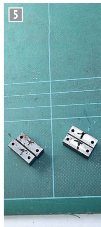
Next job was to make the bearing caps which will eventually be silver soldered in place. I first got four \frac{3}{4} inch lengths of \frac{1}{4} inch square bar. These were overlength to begin with and were then drilled 1.8mm ready for tapping 8BA into the bottom halves fitted to the stand, the top halves then being opened up for clearance.
