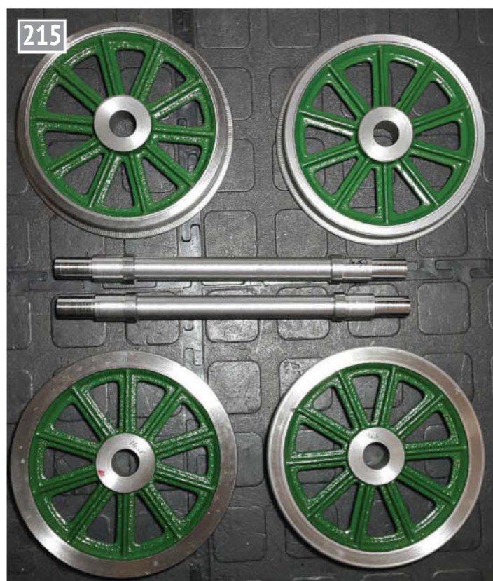
The machined and painted wheels of the tender as well as machined (for) press fit shafts.
