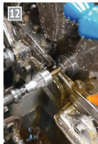
The die moves in to form the thread.
