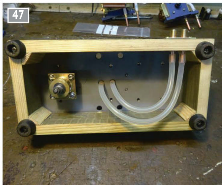
Feed pump connected.
