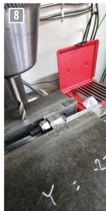
I then needed to profile the blocks to shape. First, I bolted the two assemblies together and held them securely on a pair of parallels in the machine vice. The bolts and the jaws gave enough support to machine the first of the block tabs down.
