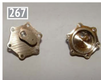
Everlasting blow down valve nearing completion.
