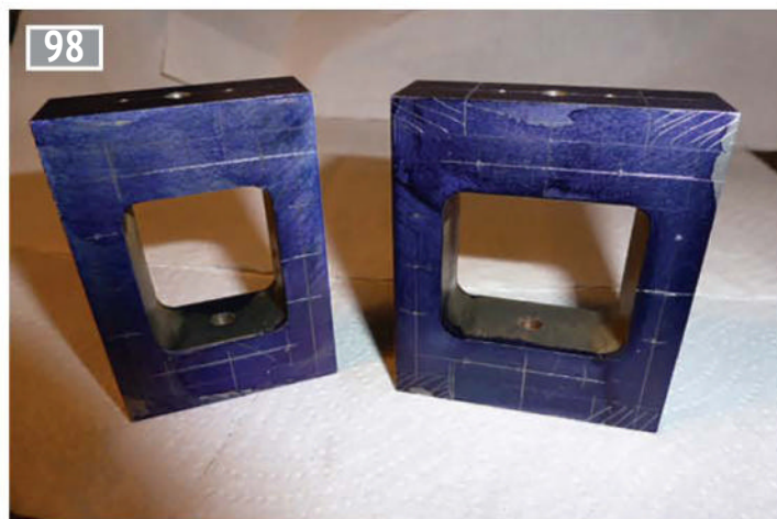
The two chests with the cavities milled out.
