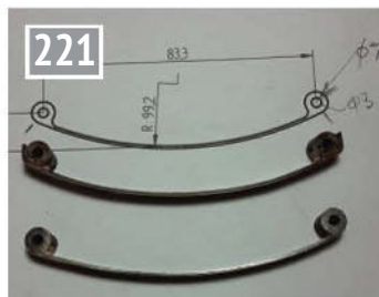
Top leaf springs in various points of manufacture, with the scale plan view used to check the bend and eye position. This is more than accurate enough for spring assemblies. Note how the leaf spring extends under the eye, which ensures the geometry takes the load and not the silver soldered joint.
