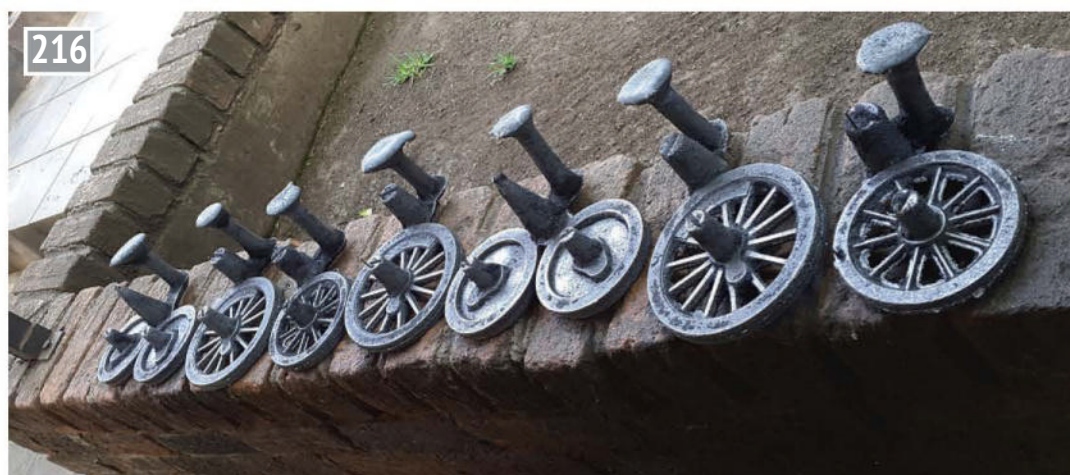
A set of Fire Queen engine and tender wheels as they came out of the sand.
