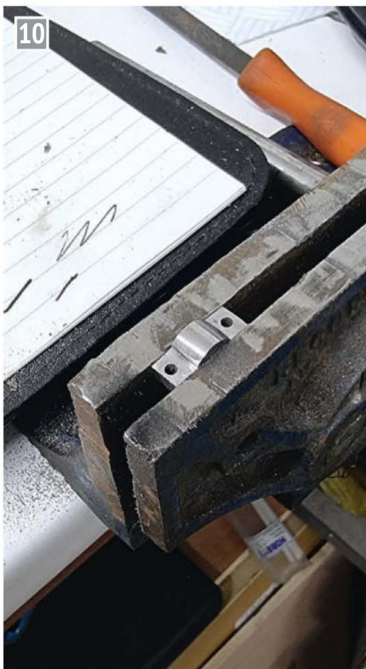
It was then over to the trusty files for a little hand work, the final job involving a Dremel sanding drum to polish.
