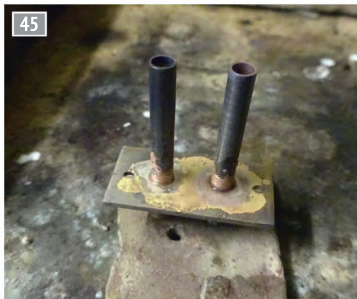
Unions soldered to the plate.
