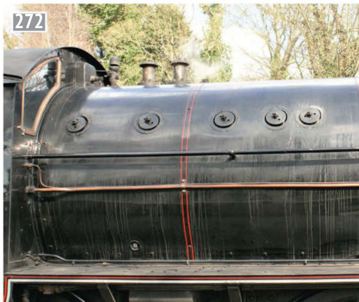
Washout plugs on a full size B1.
