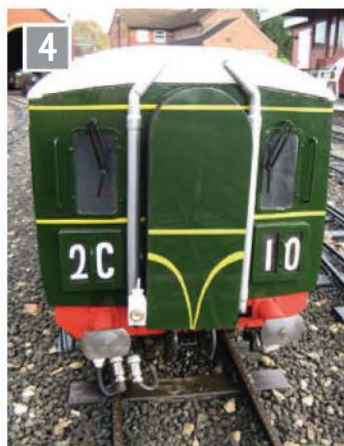
This shows number 1 end with the engine exhaust pipes, corridor connection, windscreen wipers, buffer beam detail and working light. The light can be changed from white to red depending on the direction of travel.
