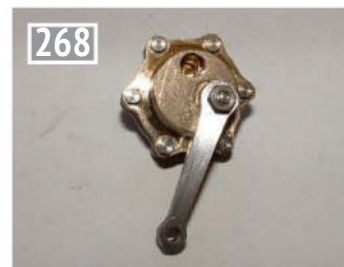
Completed everlasting blow down valve.
