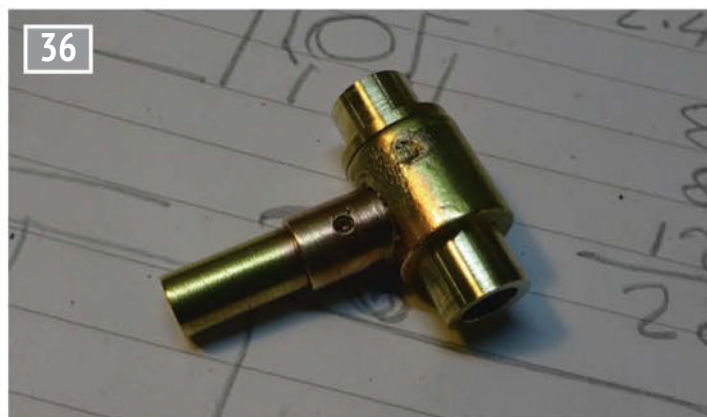
Feed pump body sleeved.
