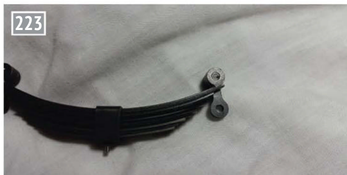
Final assembly of the springs will require the back of the pins to be punched to keep it in place.
