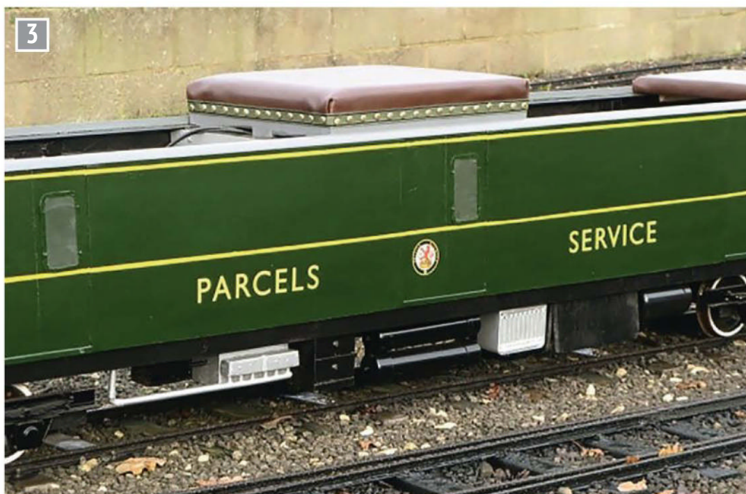
This shows the centre section of the Class 128. The driver's seat is in the centre to enable the unit to easily driven in either direction. Also seen are some of the underfloor details including engine, battery box, cylinders etc.
