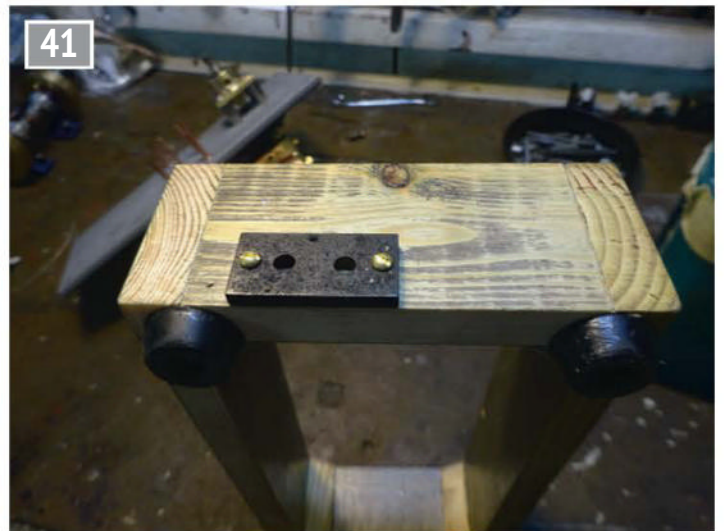
Pipe drilling jig.
