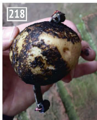
Soldering the round to the end of the top spring in a potato to prevent annealing the spring material. Notice the extra material for trimming and the piece of wire holding everything in place.
