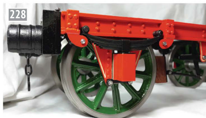
The spring assembly on the frame with the wheels fitted.
