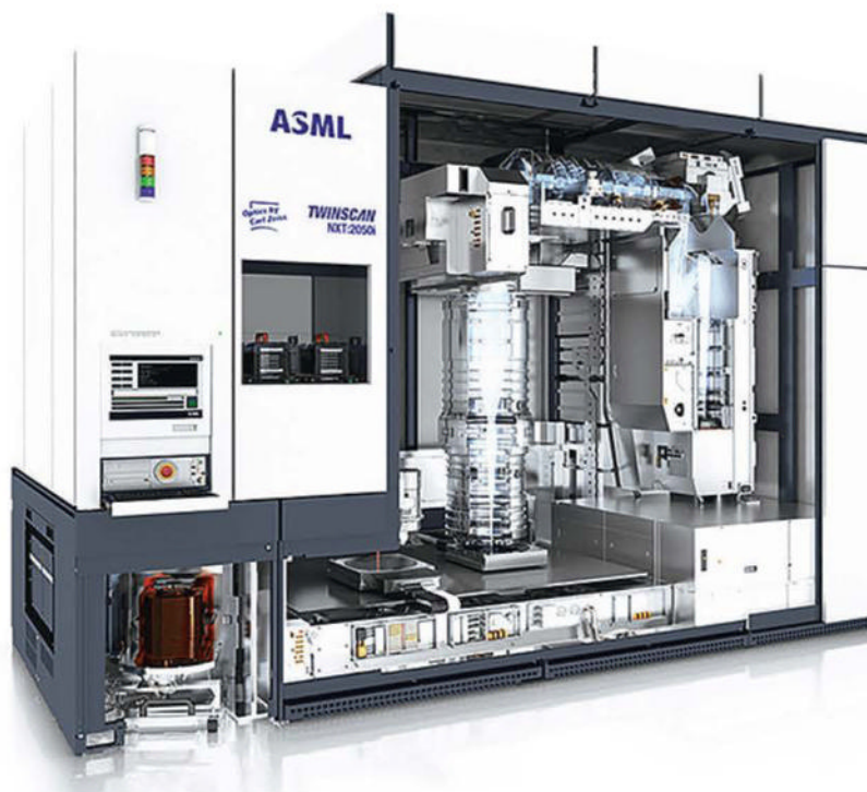
A deep ultraviolet photolithography machine. It takes a big tool to make a small electronic circuit. (Photo credit: ASML N.V.)
