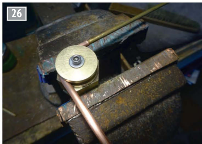
Pipe bending jig in use.
