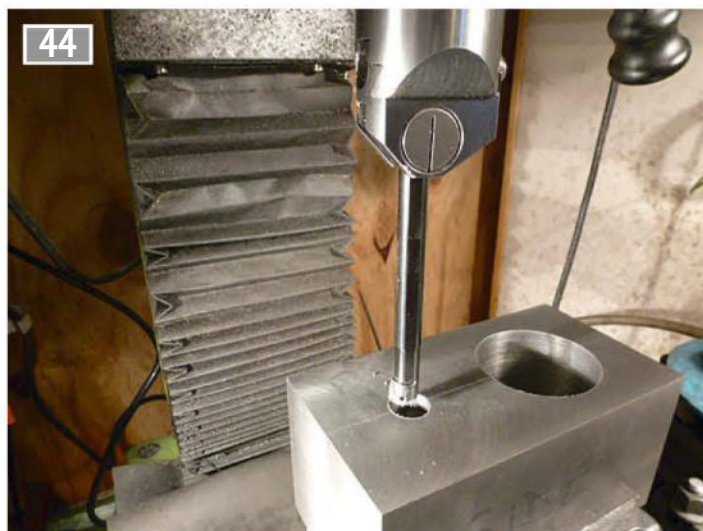
Opening out the bores with a boring head.
