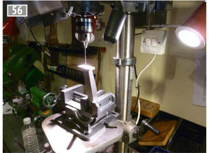
56 Drilling the end of the column for the base screws.
