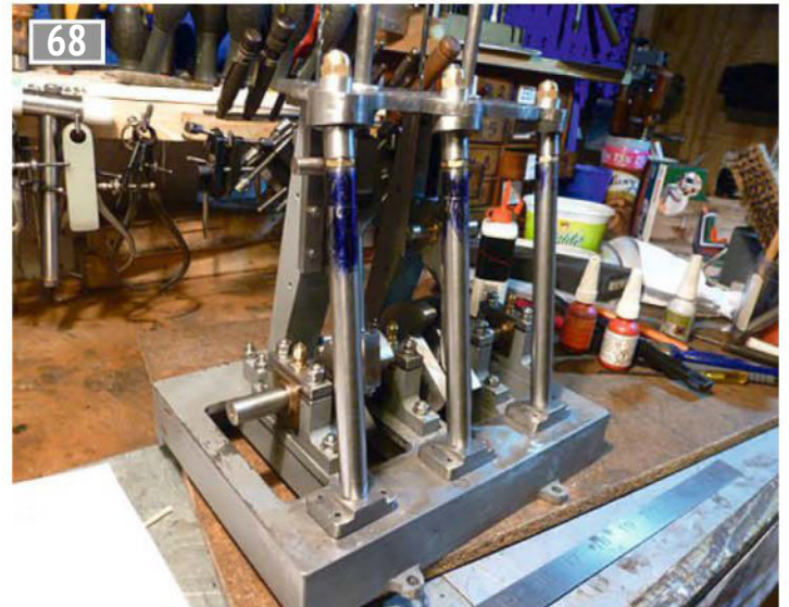
Front support columns. Trial fit of fixings.
