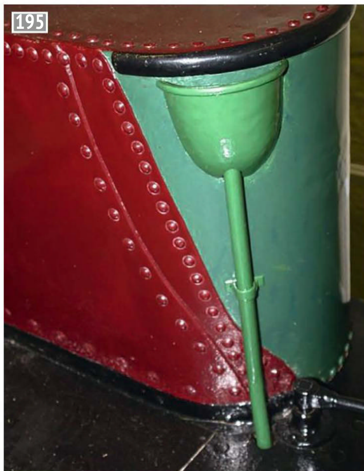
The current sanding gear fitted to the tender isn't the original, which was badly corroded.
