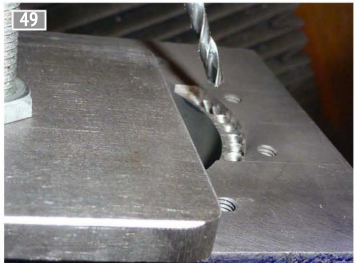
49 Drilling the first of the passages.
