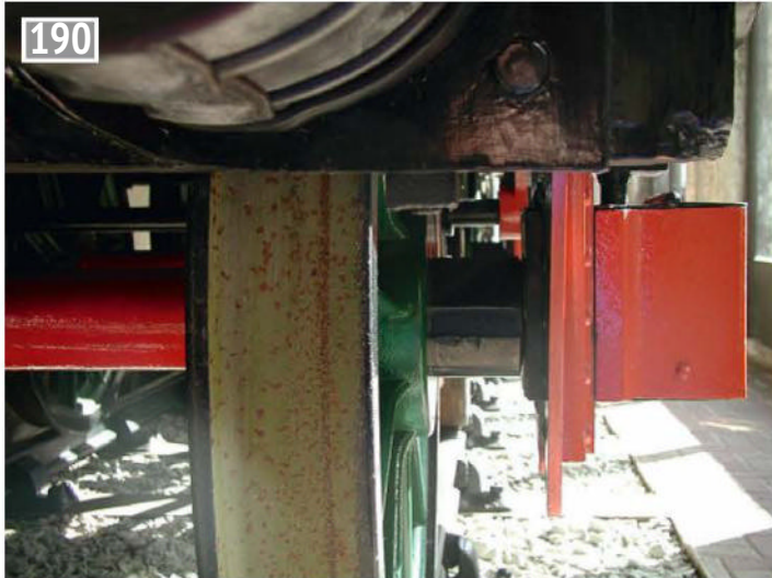
190 Wheels moved inward for the 4 foot gauge with spacers between the axlebox and wheels.
