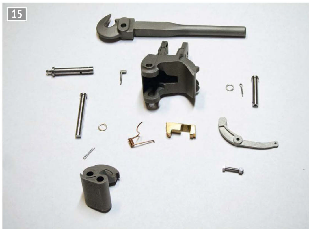
The disassembled components of one complete coupler.
