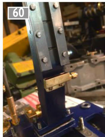
60 Column with the crosshead retainers in position and the brass oil catcher.
