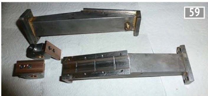
59 Complete units with the crossheads. The flanges have been drilled and tapped for the crosshead keeps and oil channels milled across the bearing surface. The top oil channel is drilled through the column to end in a 3/16 x 40 3/32 inch pipe union on the back.
