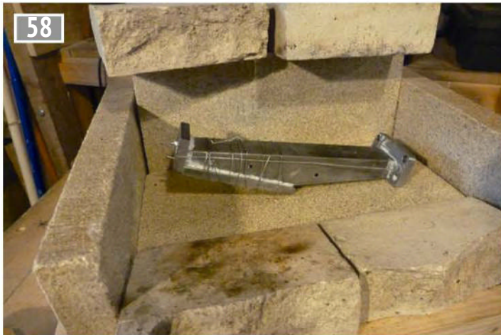
58 Wired and fluxed in the brazing hearth.
