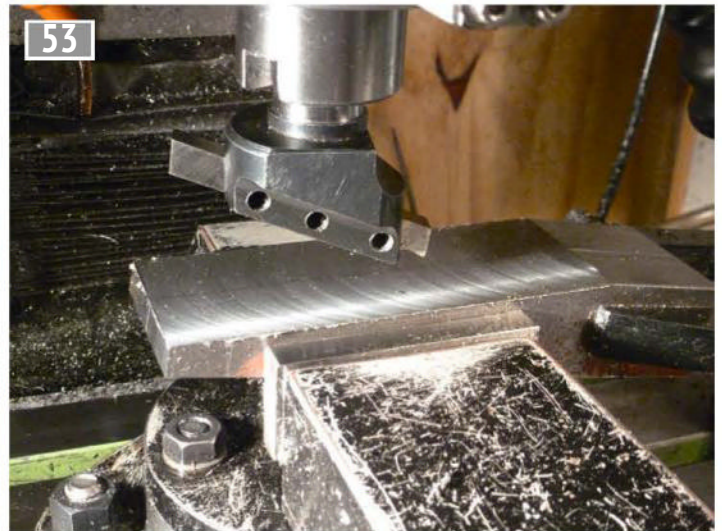
Fly cutting the two columns as a pair.
