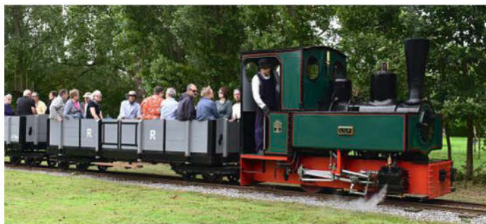
By way of contrast to the previous view, this view of Lily on a passenger working well illustrates the bogie open carriage design using a Robert Hudson chassis acquired from Lydd Ranges married to a body manufactured in-house.
