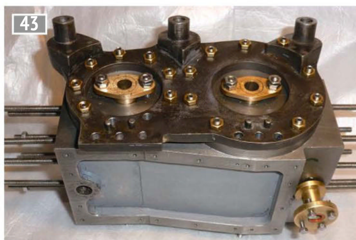
Finished cylinder block. Trial fitting of bottom covers and support plate.
