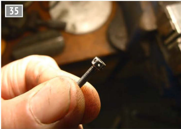
Bolt head drilled for locking wire.
