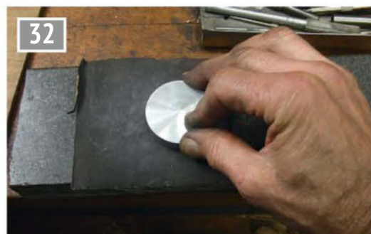
Lapping a ring to width.
