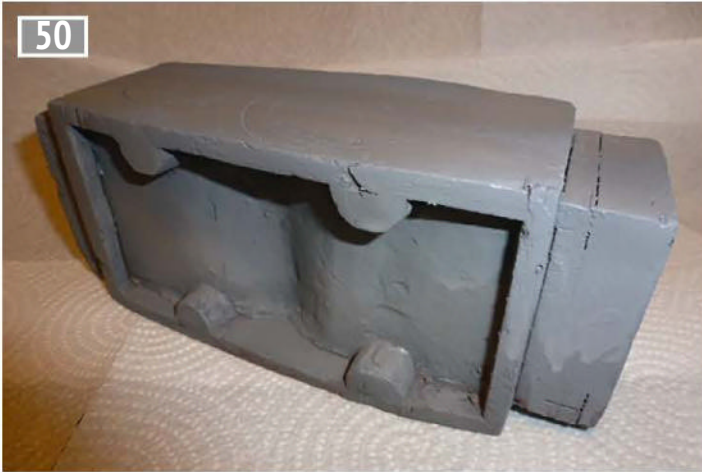
Very rough wooden mock-up of the cylinder block, to enable me to get my head around the shape and position of the various flanges and bosses. I think I'd best leave pattern making to the experts!
