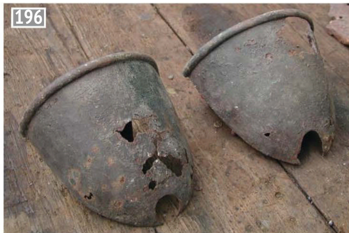
The original sanding funnels which were badly corroded.
