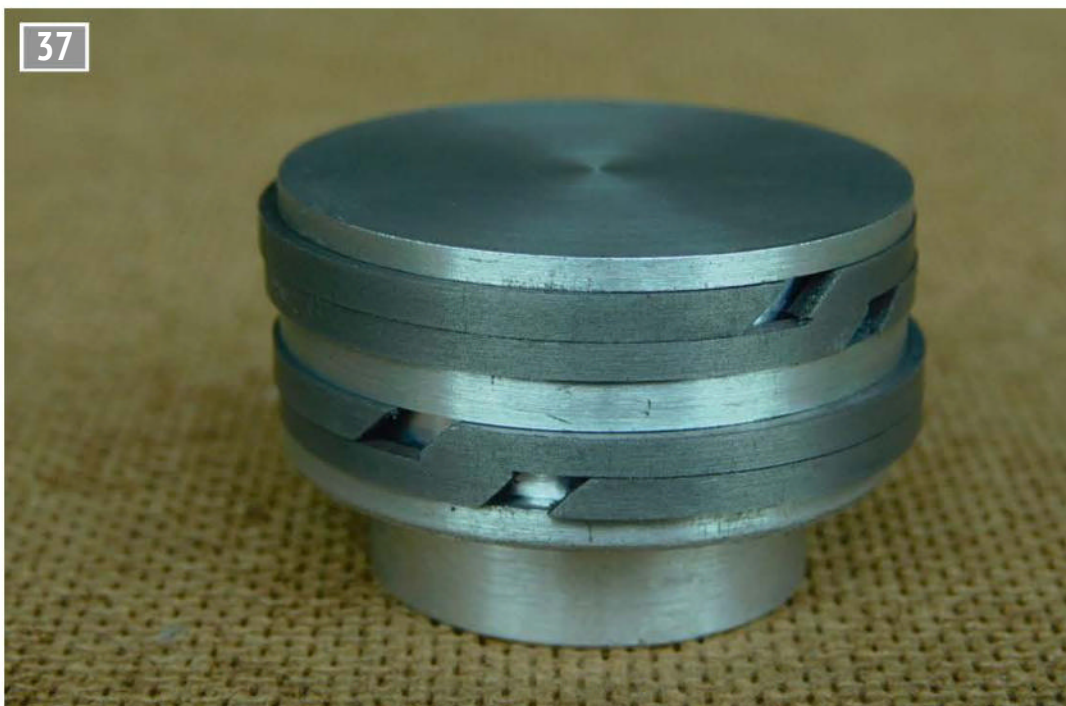
Piston with rings successfully fitted.
