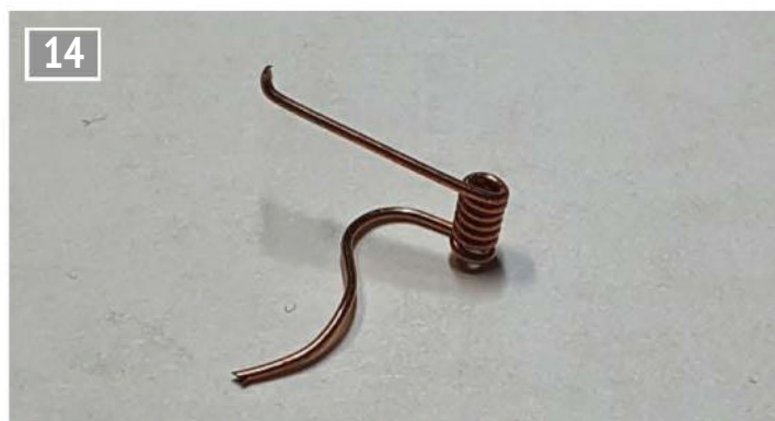
Torsion spring forming complete, prior to de-burring.
