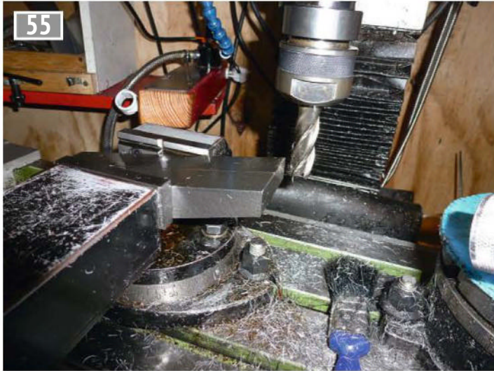
55 Truing up the base of the column.
