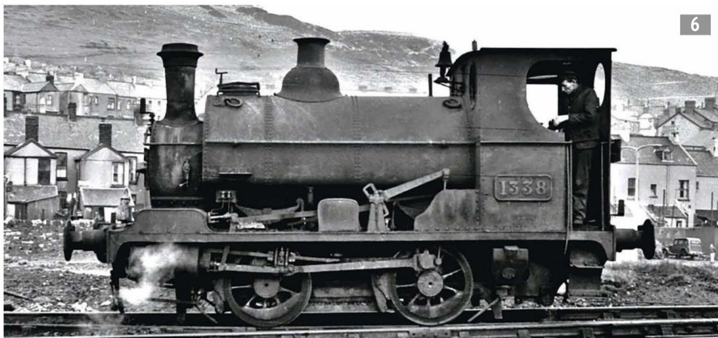
Locomotive with Hawthorne Kitson valve gear (extracted from ref 27 by kind permission of Roger Smith).
