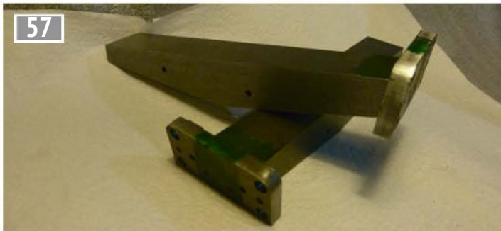
57 Bases attached awaiting brazing.
