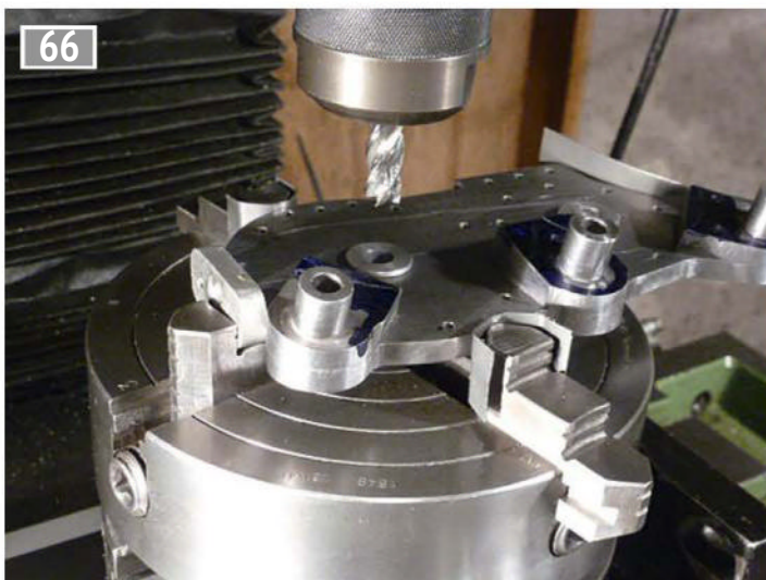
Milling the curved inside surface of the column brackets.
