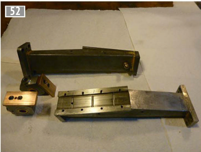
Rear support columns with the two crossheads.
