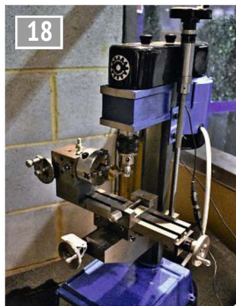
Cutting clock wheels in the Clock Shop.
