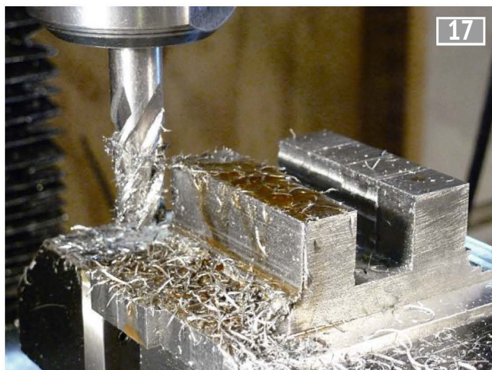
Milling the block of four blanks as a unit.
