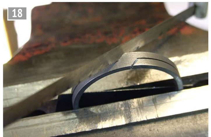
Initial diagonal saw cuts.
