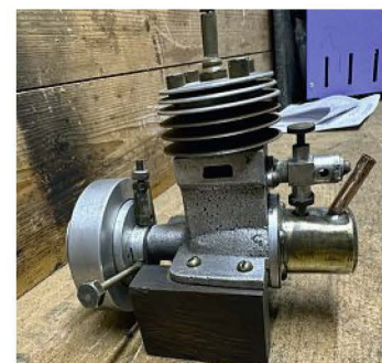
Two stroke internal combustion engine made by a young model engineer.
