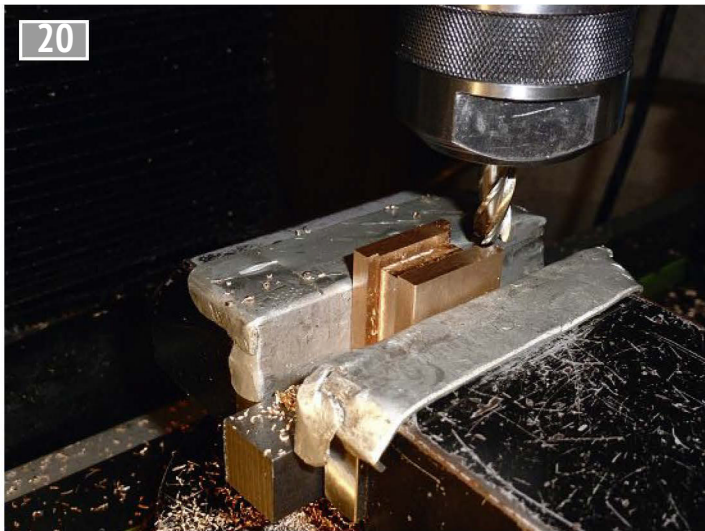
Machining the slot on all four sides.
