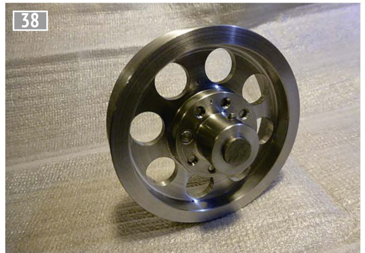
38 Finished flywheel with drive flange.
