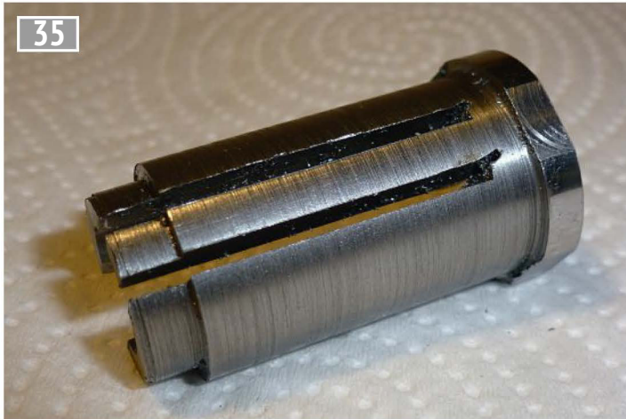
35 Making the key. Key partially cut from its tube.
