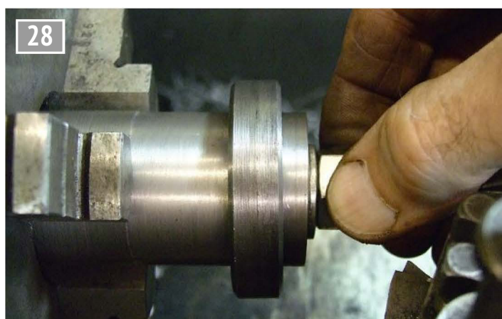
Closure cup mounted on machining mandrel.
