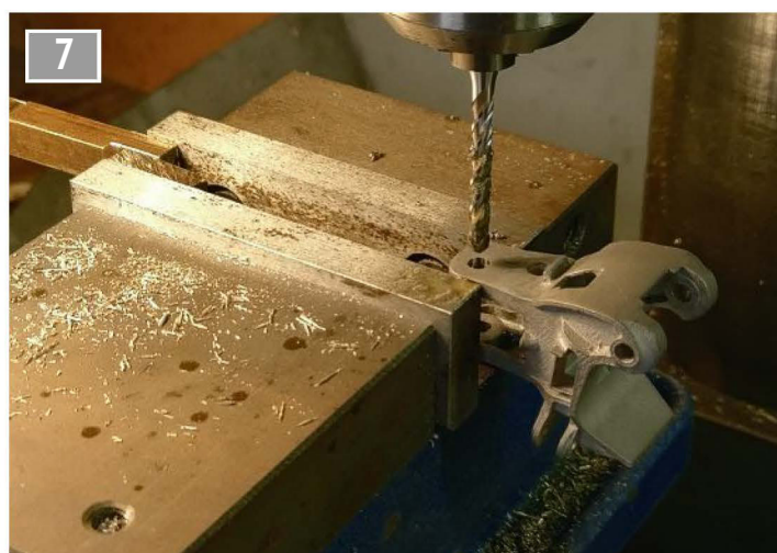
Drilling out coupler pivot pin hole with a 3.5mm extra-long end mill.
