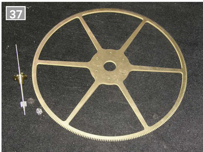
Here is a great wheel completed, with the centre pinions on the left, one mounted on the centre shaft.
