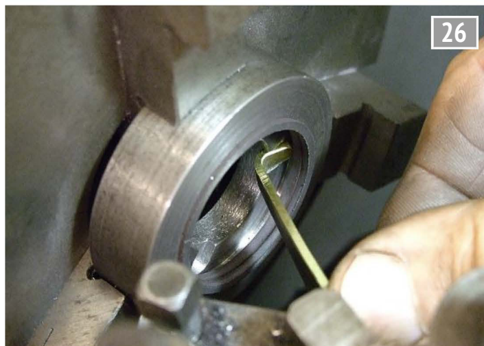
A ring in the 'widthing cup' for final machining.
