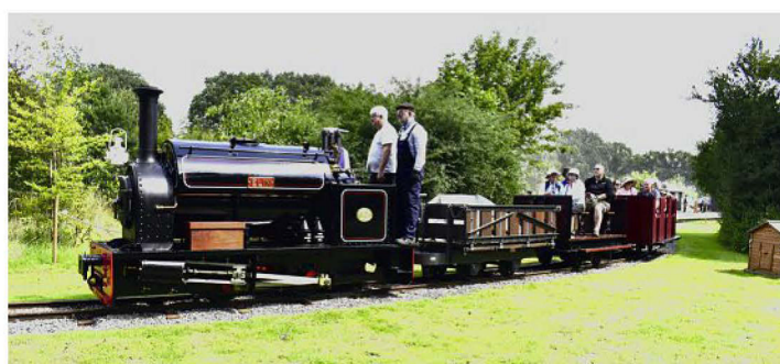
With Richmond station in the background, Elin is seen on an open mixed working on the main loop - a chance to demonstrate two of the smaller passenger vehicles in action and to show off the fine restoration work on the R.A.F. Fauld munitions wagon. Its handbrake column, 'D' platform, bottom-hinged dropsides (with associated uppermost securing catches) and seven vertical dropside timbers, four of which are rebated to take strengthening irons, are well evident in this view.
