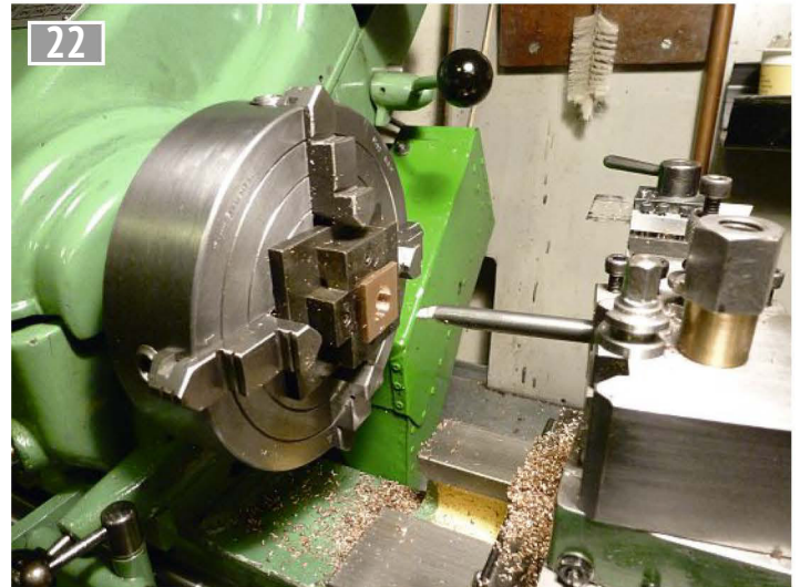
Boring the shaft hole in the bearing.
