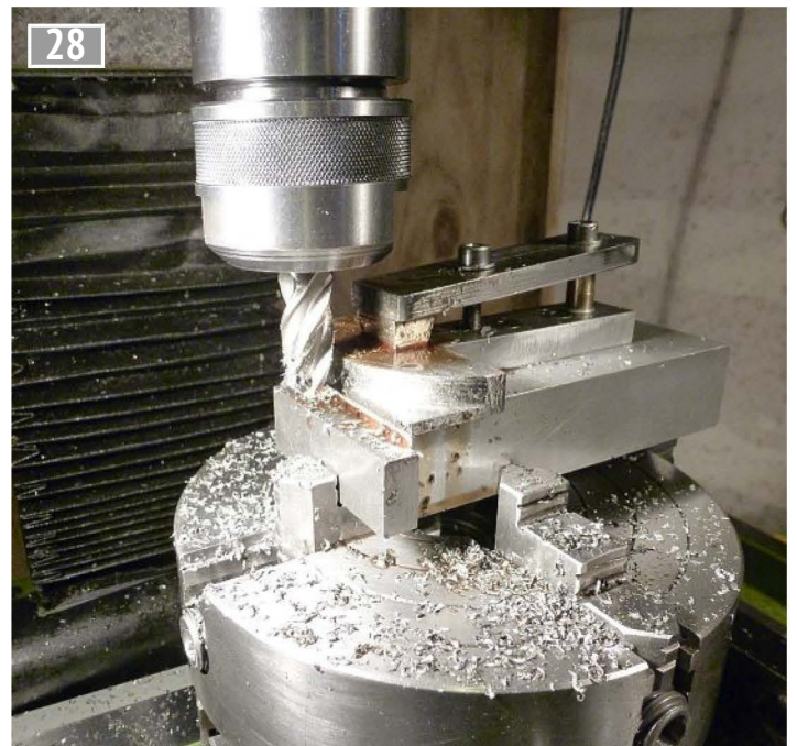
Machining the curved side with an end mill.
