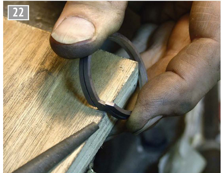
Tidying up the diagonal cut.
