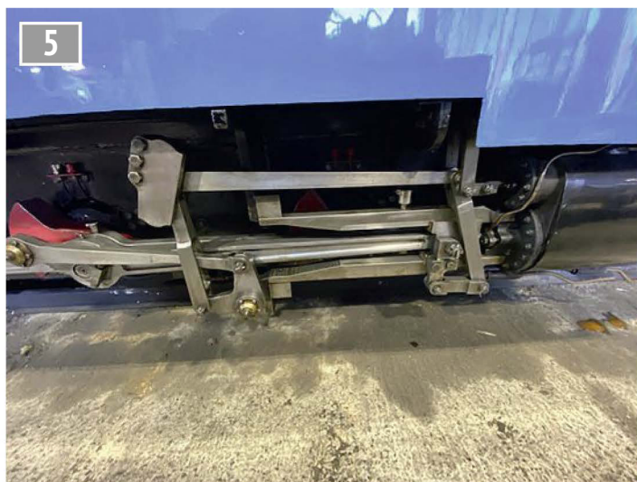
Valve gear of Wroxham Broad (photo courtesy of Bure Valley Railway).
