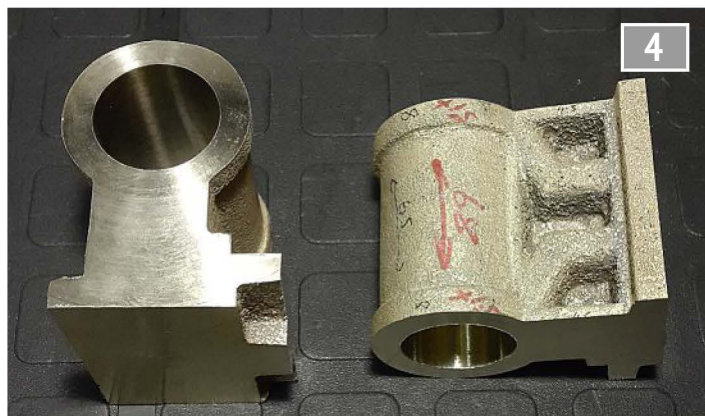
Gunmetal cylinders - note the thinning around the steam channels to improve casting.
