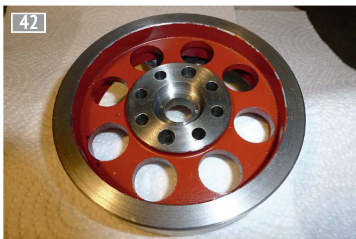
Finished flywheel. Note the rebate in the boss to provide clearance for the head of the saddle key.
