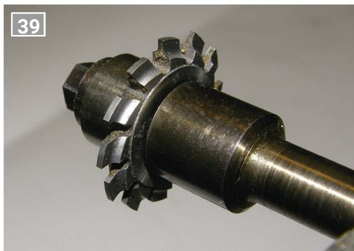
A commercial tooth cutter for clockmaking.
