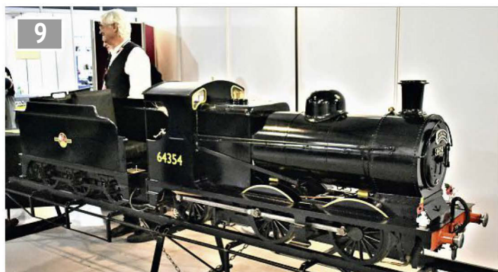
A 10 1/4 inch gauge LNER J11 0-6-0 'Pom Pom' built by Daniel Floyd in three years.
