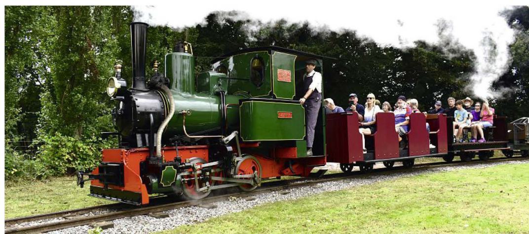
Arnold Jung 0-4-0WT Jenny rounds the main curve on the branch line with another open mixed working in the direction of New Barn Halt. With its combined inside frames and well-tank, high-pitched boiler, outside valve gear (in this case Walschaerts although Stephenson and Hackworth were not unknown, especially on earlier specimens in the former case) and externally mounted regulator and steampipes, Jenny is a classic example of its school of German design. Note also how the leading carriage is inspired by Penrhyn practice.
