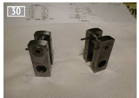
The two crankpins and their webs ready cross drilled with the \frac{1}{16} inch pin.
