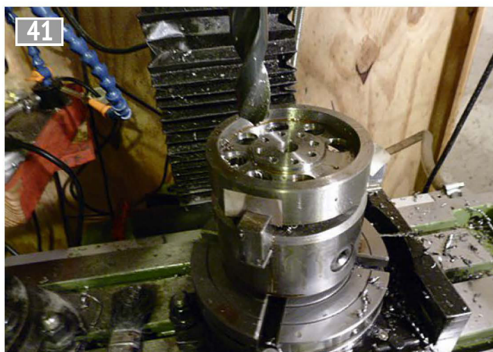
Again, using the PCD function to drill the eight lightening holes.
