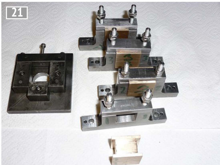
Trying the fit in both the jig and the bearing standards.
