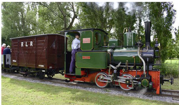
A view of Jenny, again on the branch line, but seen from the other side and working in the opposite direction (i.e., towards Richmond Station). Note that the reach rod is visible in this view, and the shape of the mainframes behind the rear axle. The re-purposing of the ex-R.N.A.D. van as a 4-ton capacity permanent way department vehicle is proclaimed on the sides of its bodywork, now painted in Corris Railway brown livery.
