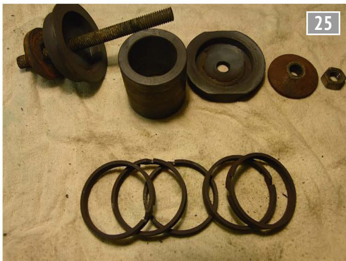
Rings removed from mandrel after heat treatment.
