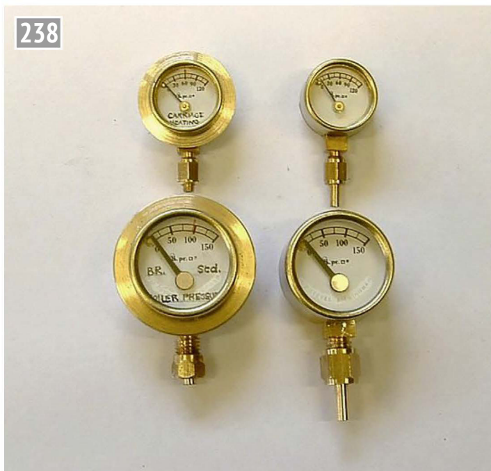
Pressure gauges with flanges.
