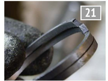
Ragged end of the diagonal cut.
