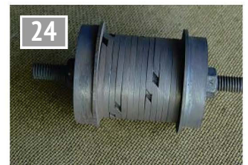
Rings after second heat treatment.
