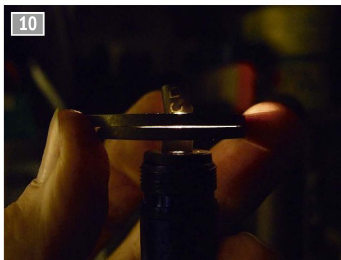
Unwanted gap in a Clupet ring.
