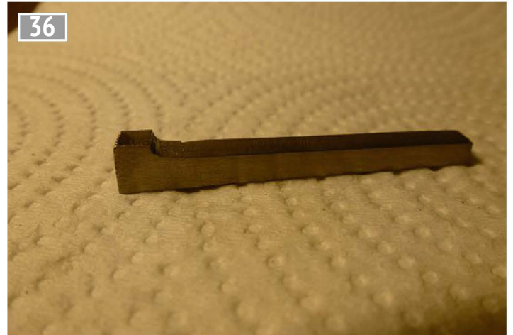
36 Finished key blank. This still requires filing square and fitting.
