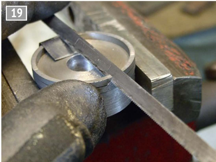
Completing the diagonal cuts.
