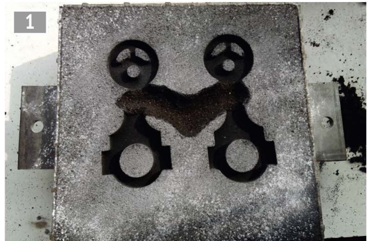
Eccentrics and straps in the same mould.
