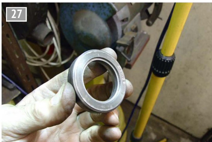
A ring in the 'closure cup' for boring to final internal diameter.
