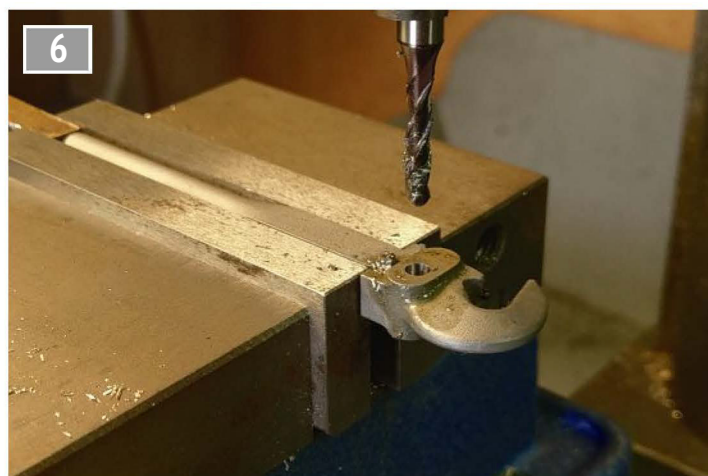
Set-up for finishing pivot hole in coupling hook.
