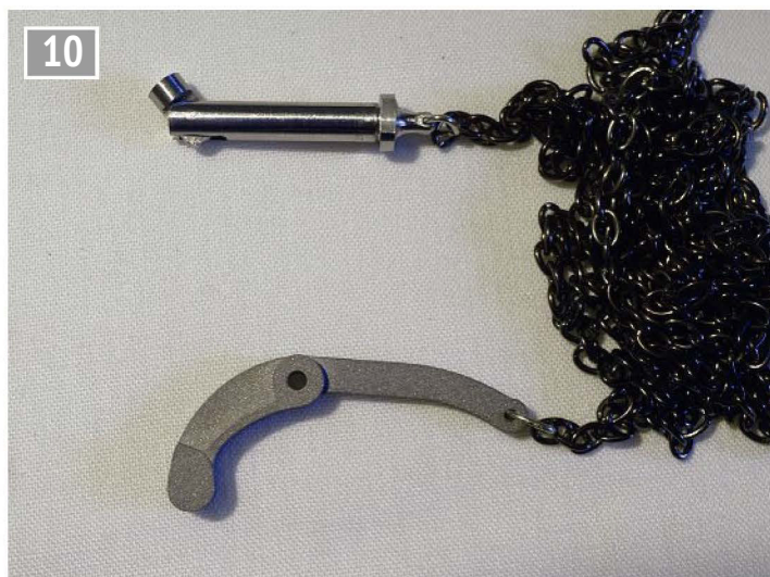
Coupler support pin and unlocking lever.
