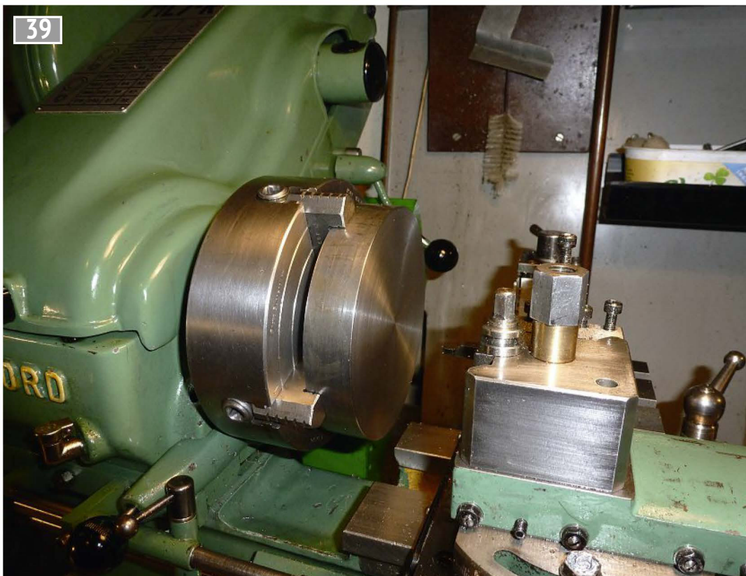
39 The blank turned down to the finished overall size.
