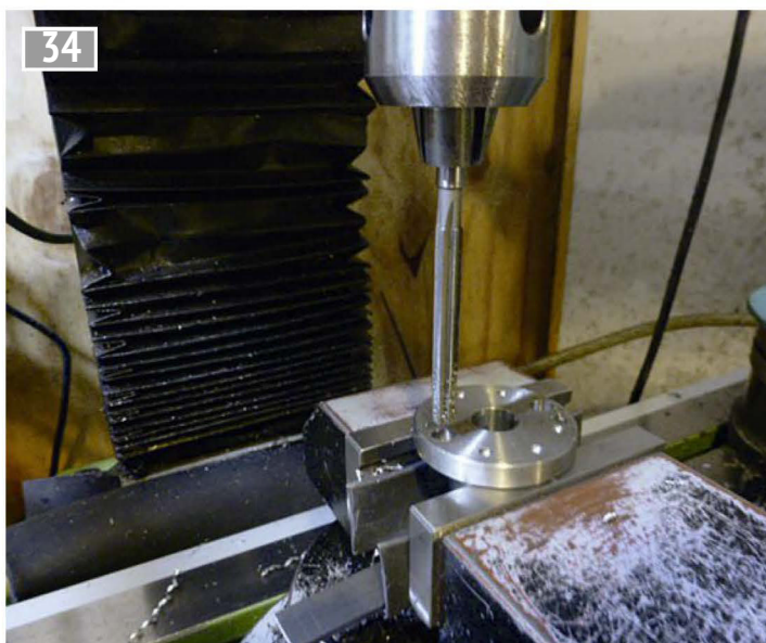
Reaming the two drive pin holes.
