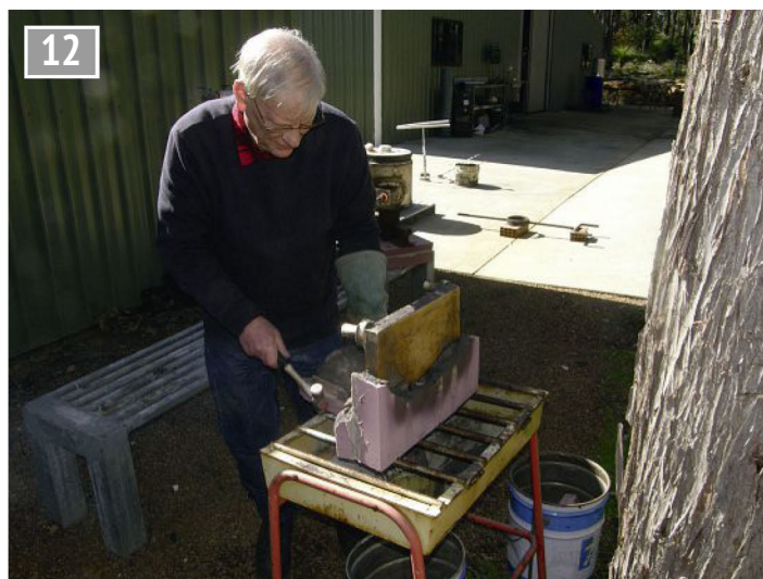
Here is one of the base castings emerging from the sand mould, after being cast at the 'C&C Foundry'.
