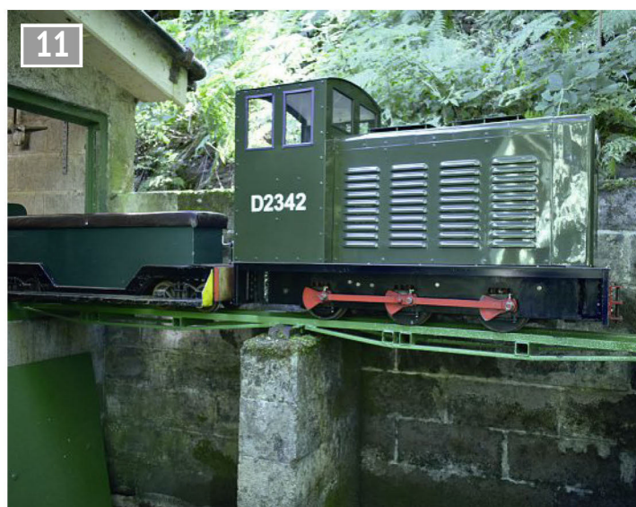
Emerging from storage at the rear of the clubhouse is the petrol hydraulic club 0-6-0 locomotive.
