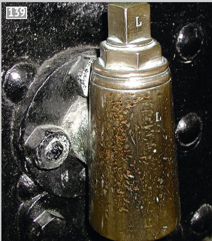
The blow downs on the large scale Fire Queen (photo courtesy E. Lander) and the model.
