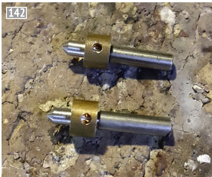
142 Blow down shafts with the phosphor bronze piece to be soldered to the stainless spindle for easier machining and tapping.
