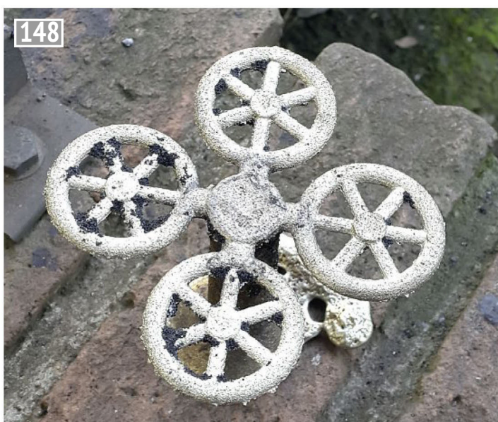
The handles as they came out of the casting sand.
