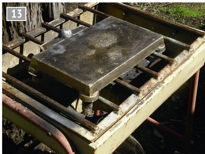
The raw casting, cooling off ready for fettling and machining.
