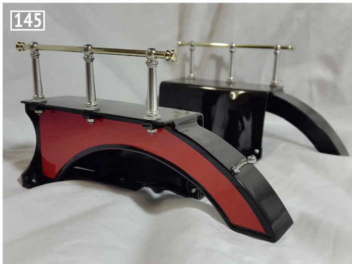
The stanchions and hand railing fitted to the back splasher assembly.
