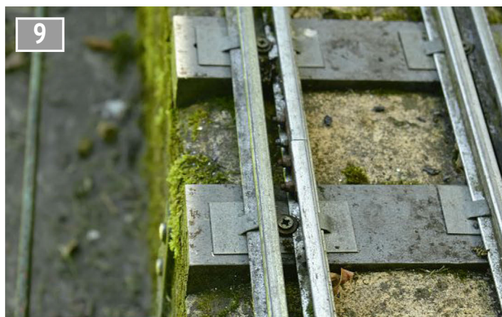
The double track clips used on the raised track.
