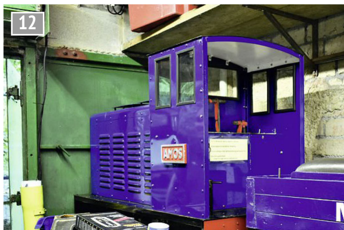
Recently refurbished, the other petrol hydraulic 0-6-0 Amos.
