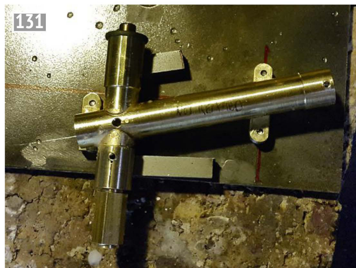
The crosshead pump assembled using screws for silver soldering and hold-down screws to a backing plate to keep the mounting holes closer to drawing.
