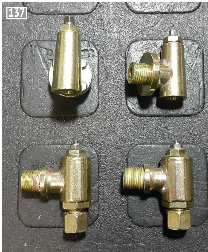
Completed boiler clacks and blow down valves.
