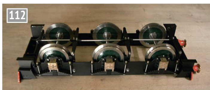
The tender chassis with brake gear fitted.
