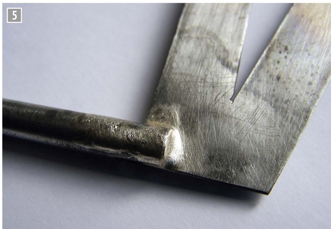
The smooth fillets at the joint using Ag 456a silver solder.
