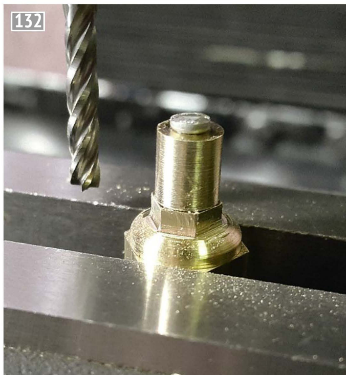
Machining the caps for the crosshead pump and clacks.
