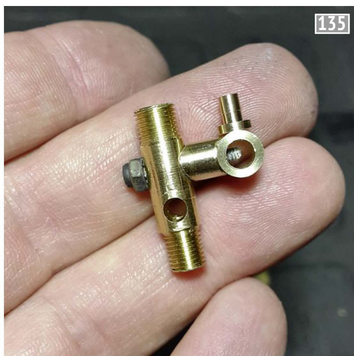
Sight glass bottom assembly prior to soldering, consisting of multiple turned components held together by Tippet covered screws.
