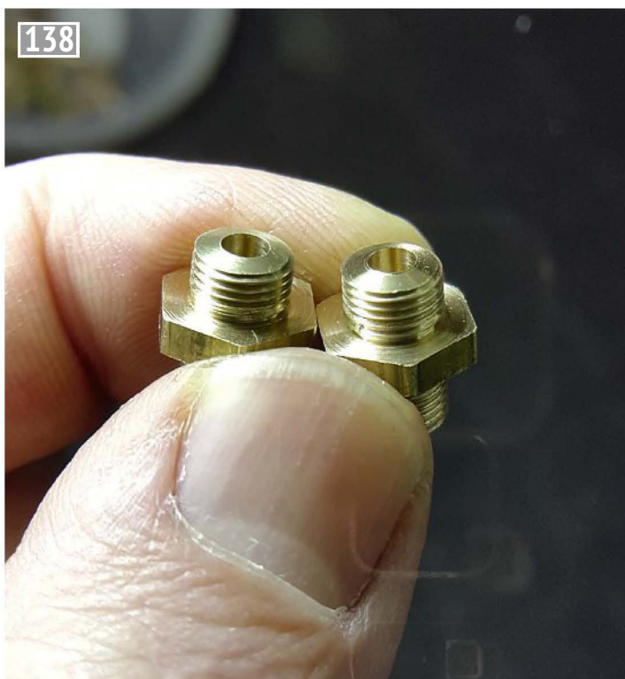
Clack seats showing the coned surface to help sealing by increasing elasticity on the contact surface.
