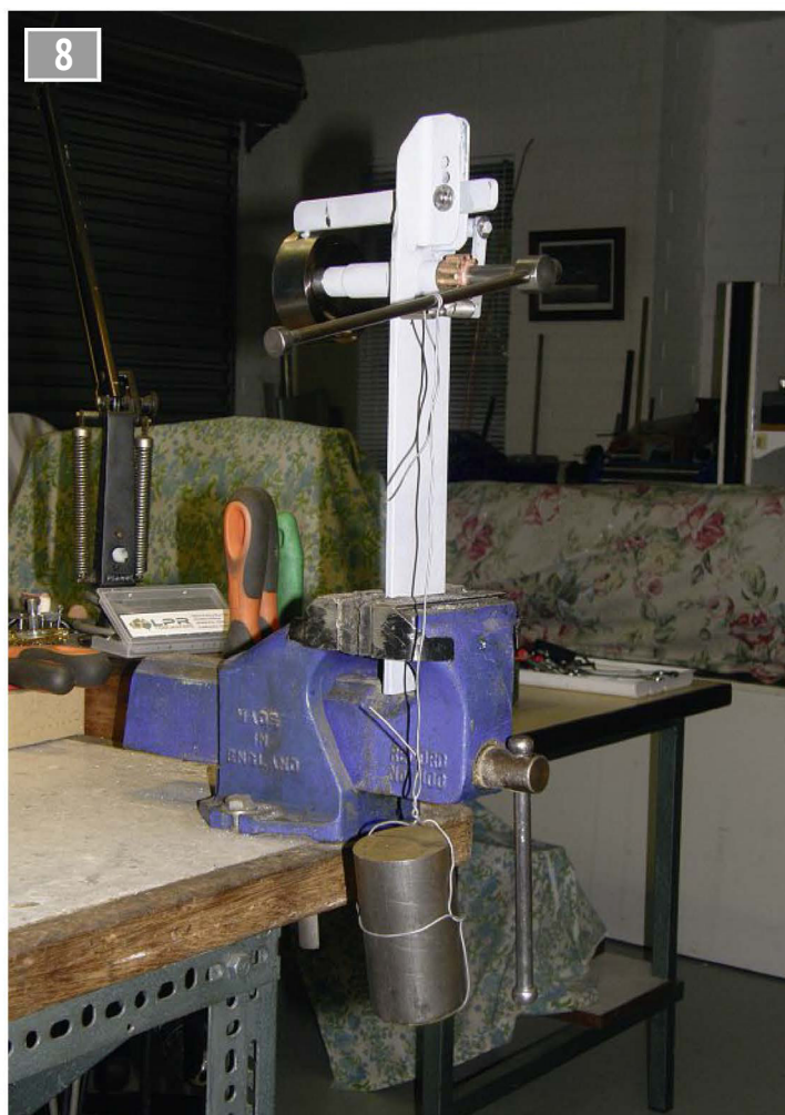
Mainspring winder with improvised measuring weight.
