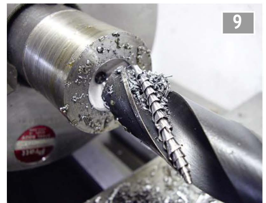
The drill bit was backed out of the work to show the cone impression cut by the point of the drill bit. The centre drilled hole is still visible in the work. (The lathe was stopped).
