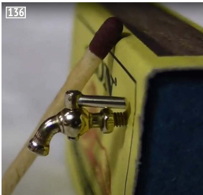
One of the little sight glass taps.
