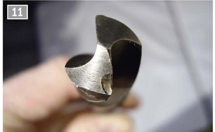
Damage to the cutting edge and flank of a twist drill bit that has reasonable shape - chips of metal have split from the outer aspect of the flank where the stresses of drilling are the greatest.
