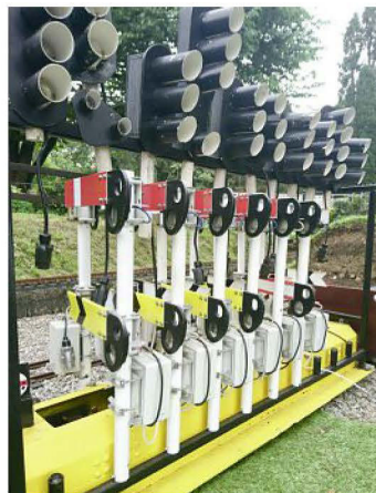
Between running days the signals are safely stored away on a bespoke running car, which facilitates delivery to each gantry as required.
