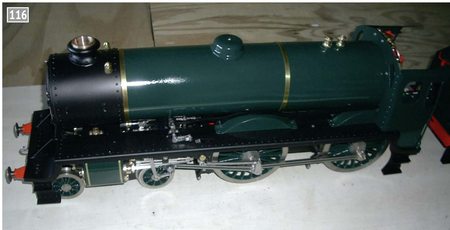
The boiler, installed complete with boiler bands.
