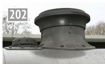
Chimney and anti-vacuum ('snifting') valve.
