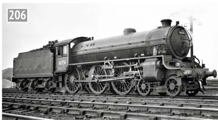
B1 61351 with no visible rivets (photo: Rail Online).
