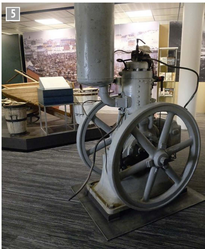
Bollinder engine as was used in many fishing boats.
