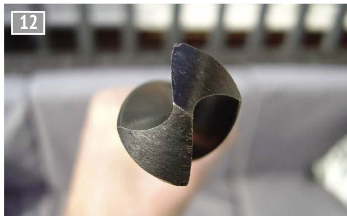
A standard example of a factory ground drill bit with convex flanks.
