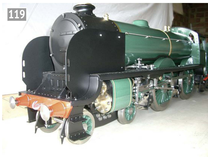
The handrails are added.
