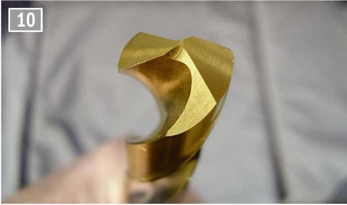
A factory ground drill bit. Photographed to show how the helix is ground to produce two facets on each flank – four facets in total. The flank is convex directly behind the cutting edge and flattened to the rear. Described by the manufacturer as web thinning and a facet point grind.
