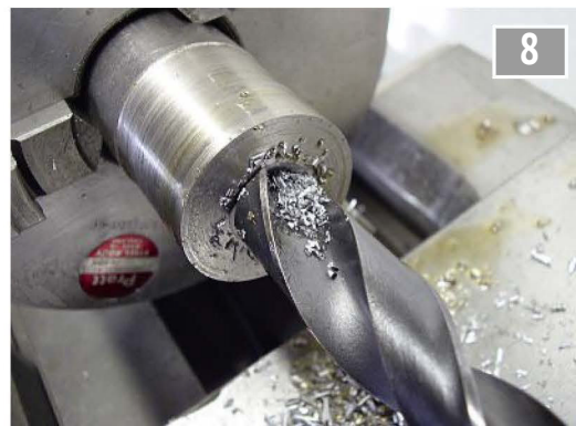
Progressing from a centre drill to a standard twist drill bit. Only the point of the drill bit is embedded in the work as the corner of the flank's cutting edge is still visible at the top of the drill bit. (The lathe was stopped).
