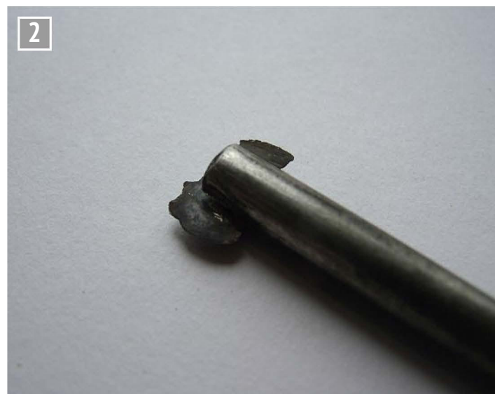
The silver solder still intact after the joint failed.
