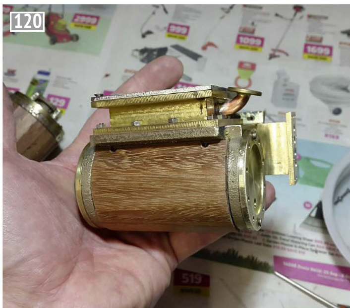
The cylinder lagging fitted and sanded, ready for a little paint.
