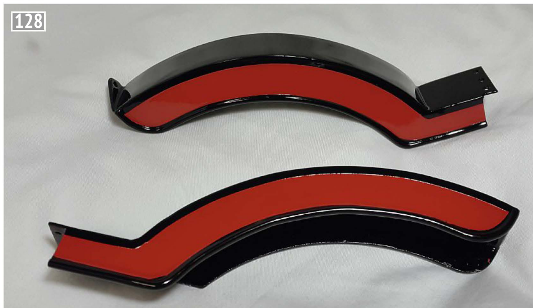
The front splashers completed, ready to be assembled.
