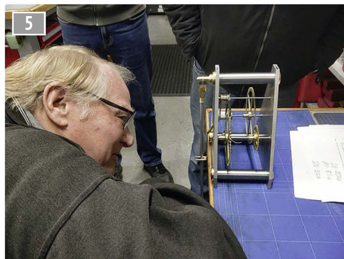
Checking the working of the escapement.
