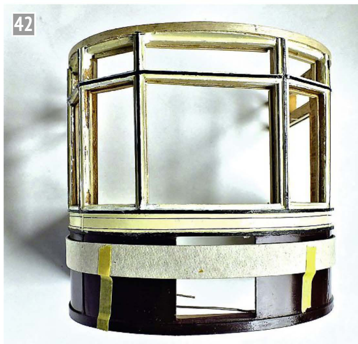
Guide fixed ready for lining.
