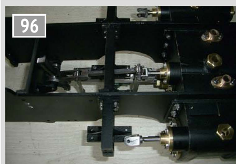
A couple of views of the inside slide bars.
