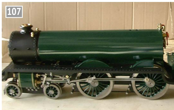
The boiler is fitted to the frames.
