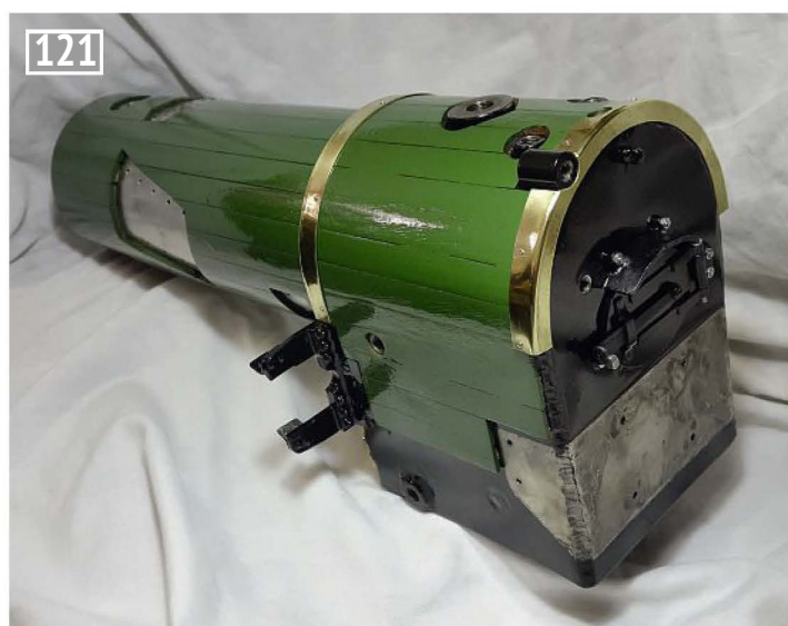
The boiler and wooden lagging painted. The brass edging hides the uneven wood ends rather nicely.
