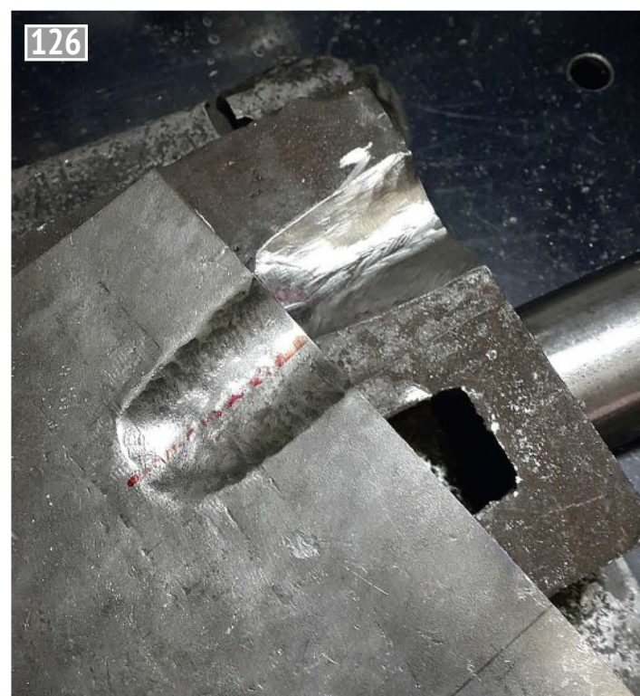
Cold forging the back splasher on a metal former; the bottom edge has already been filed straight.
