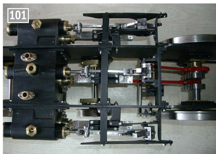
The inside valve gear is now complete.
