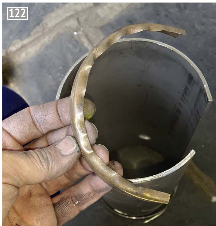
When forcing a strip round a former it buckles under the load, making folds. Further forging and annealing were required to fit the brass edging for the boiler.
