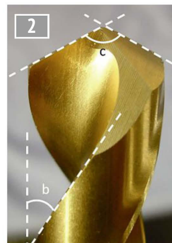
The helix angle of a twist drill (angle 'b') and the point angle ('c').
