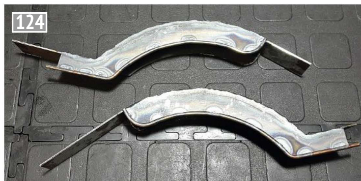
Front splashers fabricated assembly. Note how the plates extend past the edges to prevent the welds getting too hot at the end of the join.
