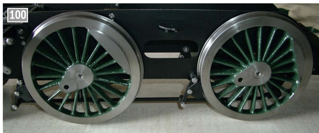
Brake gear is added.
