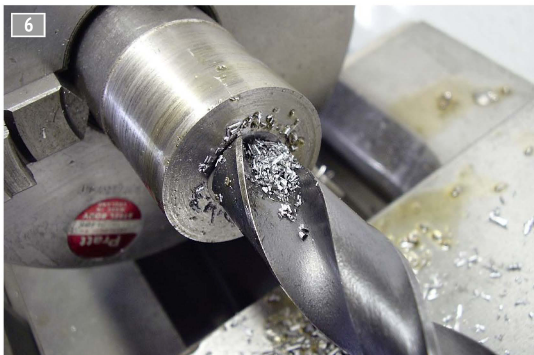
The arriss engaging with the pilot hole.
