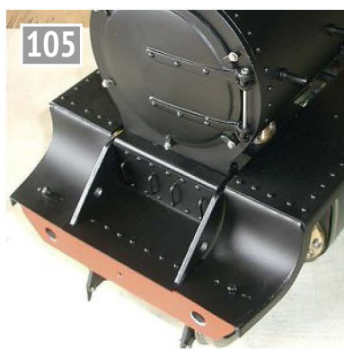
The front apron is in place.
