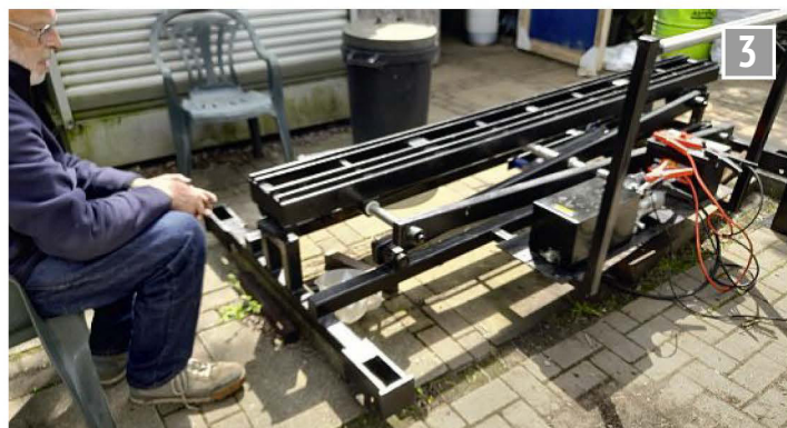
The new traverser and scissors lift in the down position.
