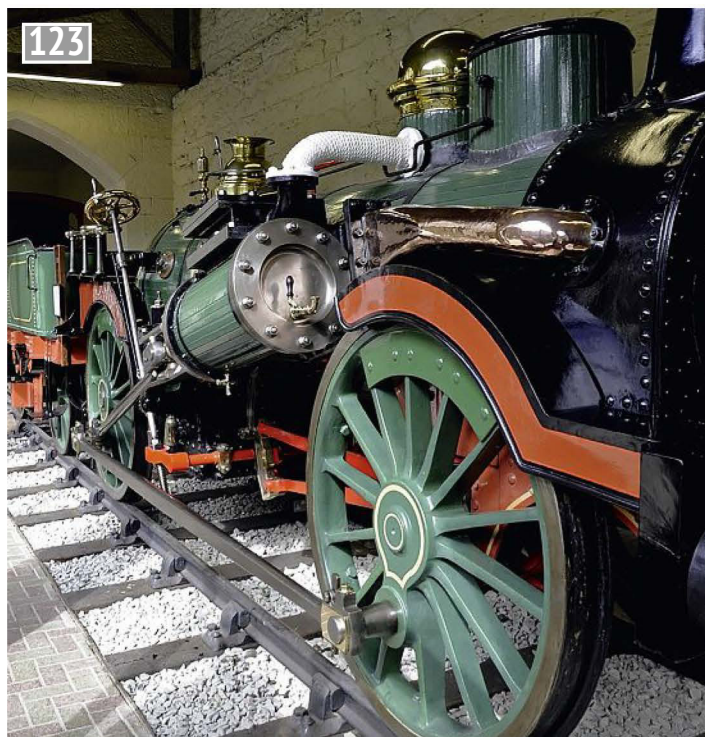
View of the large-scale Fire Queen front splashers (photo courtesy E. Lander).
