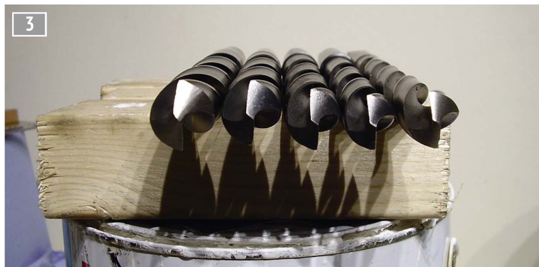
A view of the lands spiraling down the drill to minimise friction while drilling and the flutes to clear swarf.
