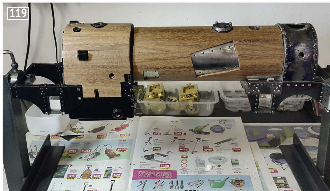
The wooden lagging glued to the boiler and sanded for painting. The maintenance frame helped to orientate the boiler into convenient positions as needed.
