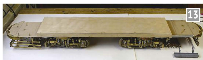
Underframe with floor attached.
