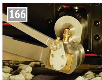
The fly crank, coupling rod, connecting rod and lubricator drive rod with its return crank bolted to the crankpin collar. Without the aid of a milling machine, a lot of handwork went into Jennifer Ann's components.
