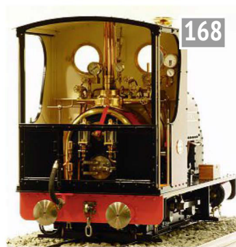
The upper portion of Jennifer Ann's cab is open; sliding doors provide access to the firehole below.
