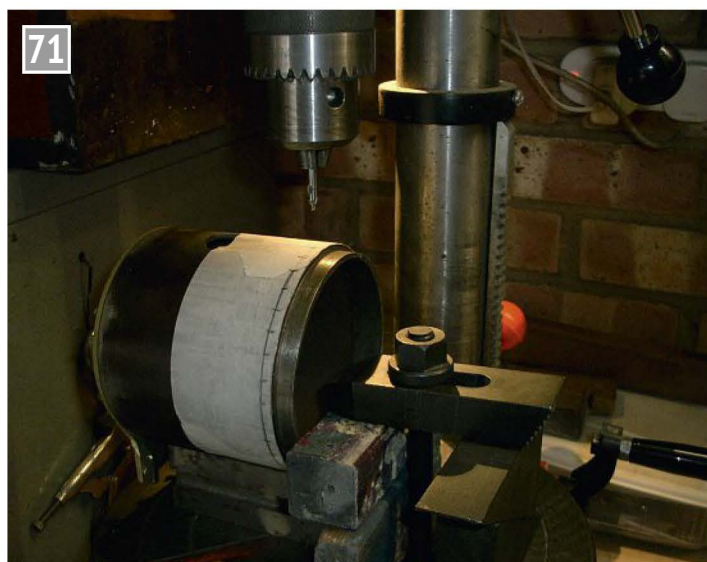
Drilling the rivet holes.
