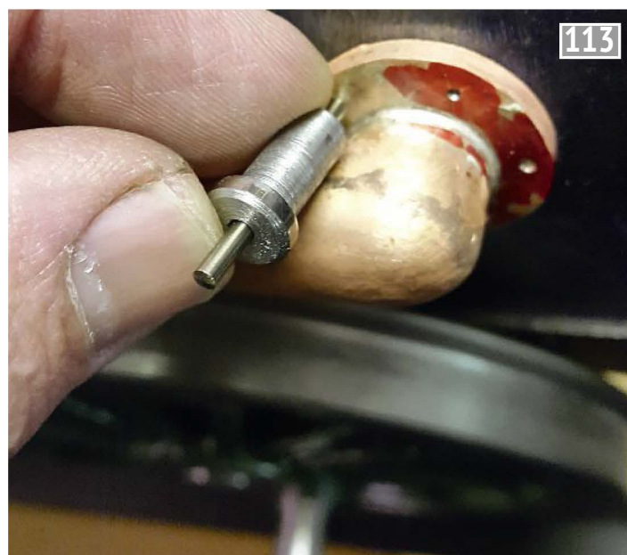
113 Punching guide for the flange holes to make sure the nuts don't foul the main body. The two back holes were done first and the remainder marked out for equal spacing using a pair of dividers.
