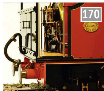
Jennifer Ann's lower cab with oak-planked floor. The firehole access doors are closed in this picture.
