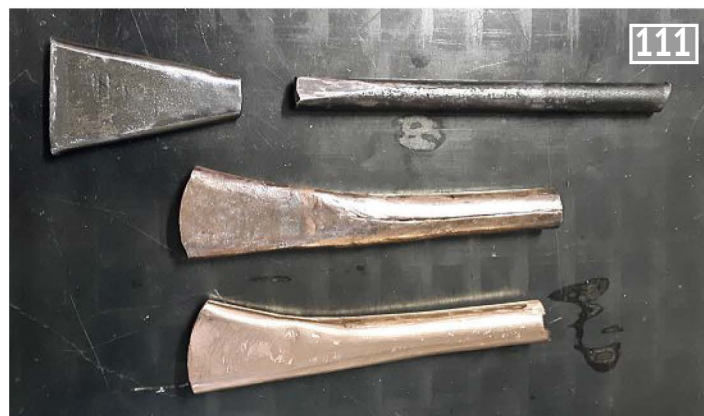
111 The inner forming mandrel and the LH and RH exhaust bodies. The bodies have different bends for the left and right sides. The split former can be used for both with the bend at the split.
