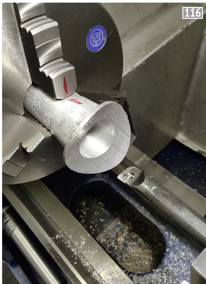
116 Machining the chimney bore. Without the usual chimney cap the casting is easier to hold in a smaller chuck.
