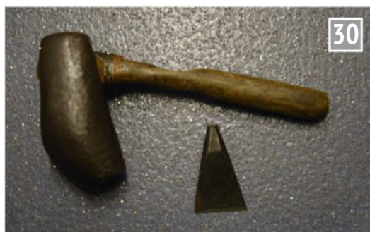
Filemaking was the Sheffield specialism. A museum video shows Ken Hawley demonstrating the use of a similar hammer in cutting file teeth. File cutting machines started to be used from around 1850.
