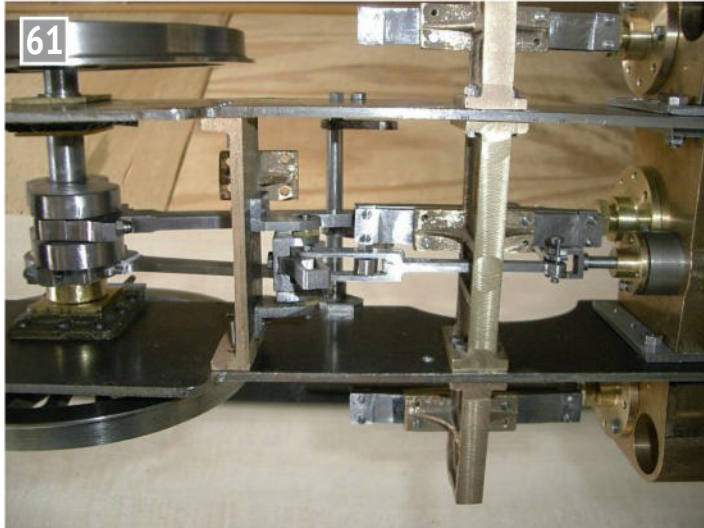
Valve gear mountings in place.
