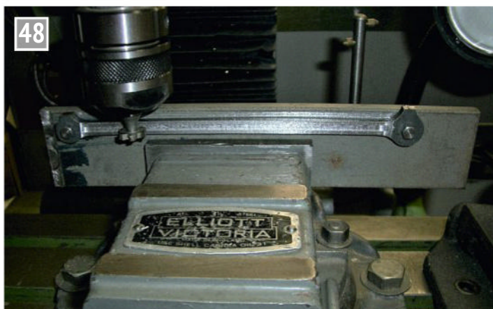
Cutting the flute in a coupling rod.
