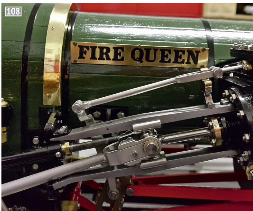
Valve connecting rod and valve rod bearing coming together. Note the slight jog in the valve connecting rod.
