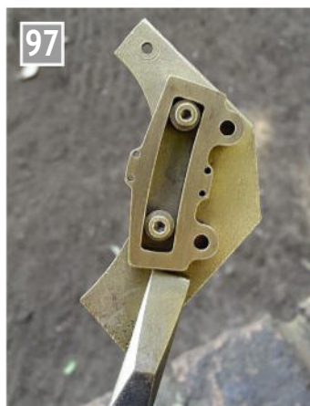
An unconstrained holding jig for heating and brass plating.
