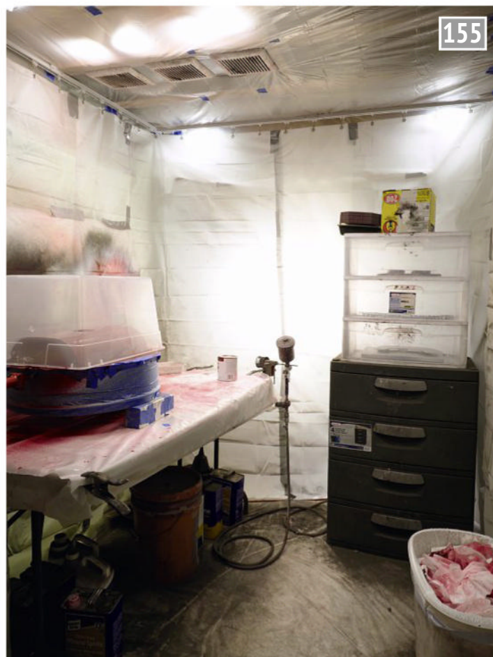
On the left, covered by a large plastic box to banish dust, the freshly painted tank wrapper continues to rotate while drying. In the middle, the spray gun sits cleaned and ready for the next job, and, to its right, the grey drawers contain paint tins and painting tools while the upper transparent drawers hold and protect smaller items between coats. LED lights shine through the walls and ceiling to provide bright but diffuse illumination, and three exhaust fans in the ceiling above help keep the air clear. The drying shelves are to the left of the camera, out of shot.
