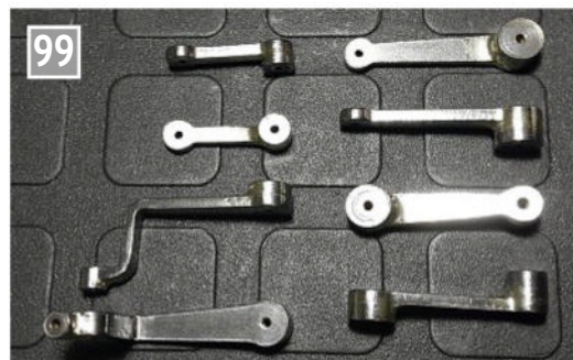
Various valve gear links with the bosses brazed in place, prior to the drilling and reaming of the pin holes.
