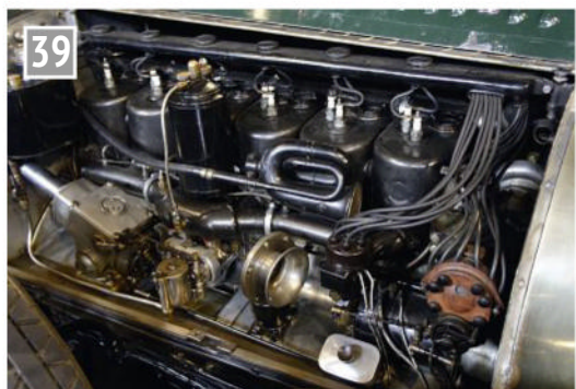
39 Simplex engine with six cylinders and 7778 cc capacity. It made 50hp. This was an expensive car for 1910. This model was built for a wealthy Australian.
