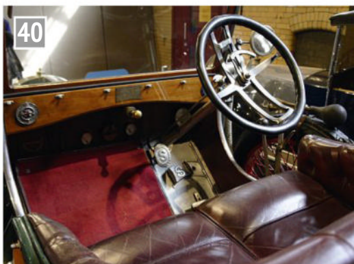
40 An oddity of the Simplex was that a driver moved his foot from side to side to accelerate.
