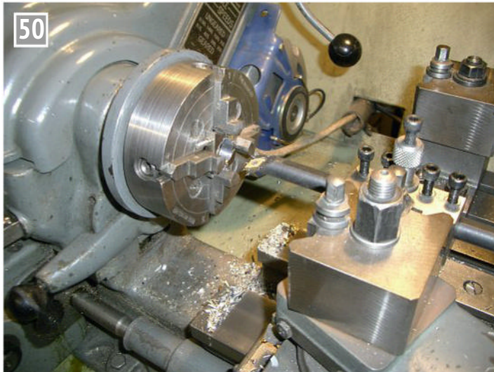
Boring the big end for the inside connecting rod.
