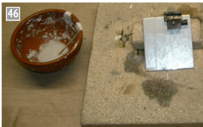
Soldering the two parts of the crosshead.
