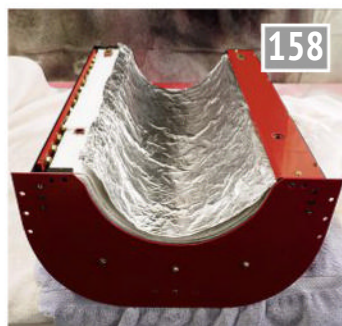
Hidden underneath, heavy-duty aluminium foil provides an additional thermal barrier and helps prevent fibres from shedding.
