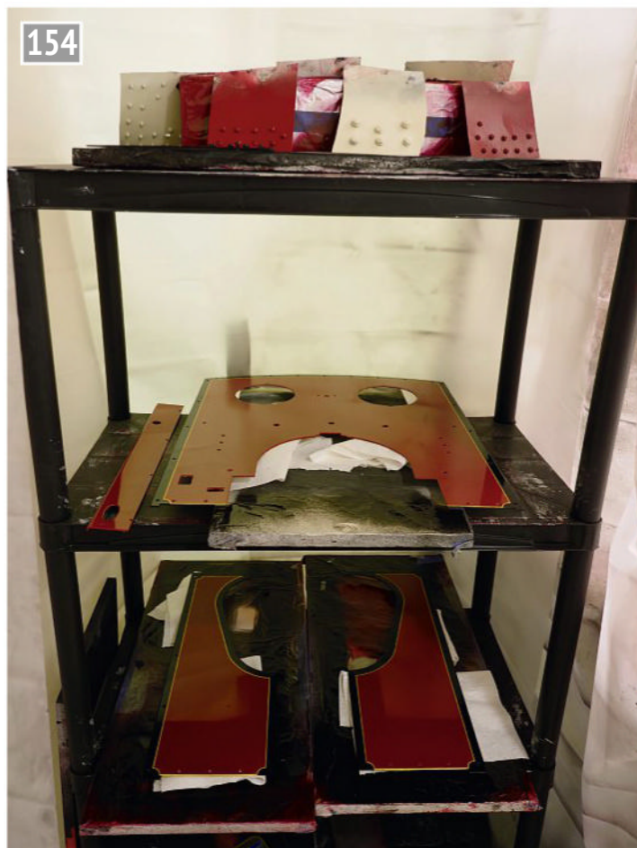
Within the painting booth, a floor-standing shelving unit, fully enclosed by yet more shower curtains, protects larger items from dust and damage between coats.
