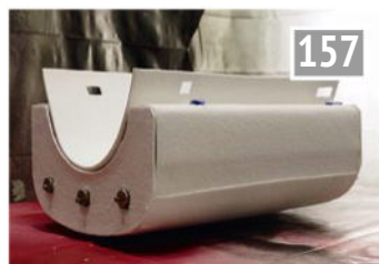
Two layers of ceramic-fibre boiler insulation are glued to the inner tank to help keep the water cool.
