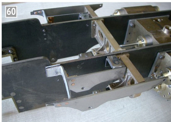
Valve gear mountings in place.
