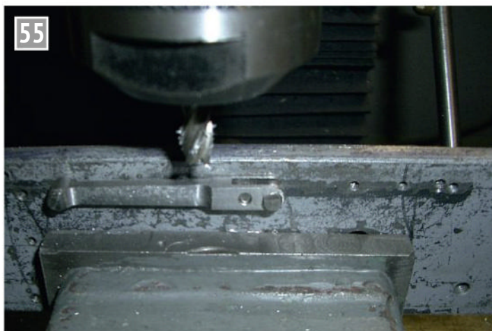
Profiling a combination lever.
