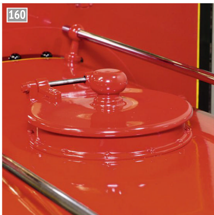
The water filler secures the tank and shell together at the top and completes the assembly.
