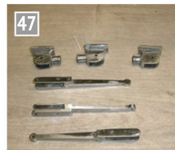
Cleaned up crossheads with radius rods.
