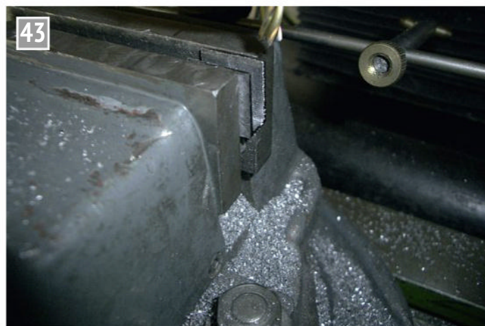
Crosshead throat being cut in the mill.
