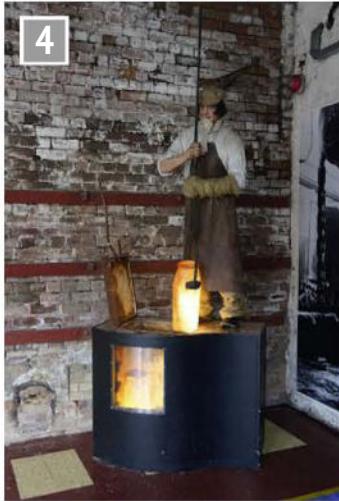
Crucible steel making. Iron and other materials were placed in especially made crucibles and heated for three hours. The resulting steel could be poured and was of consistent quality, ideal for making tools.
