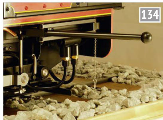
The handle screwed to the handpump, ready for use.
