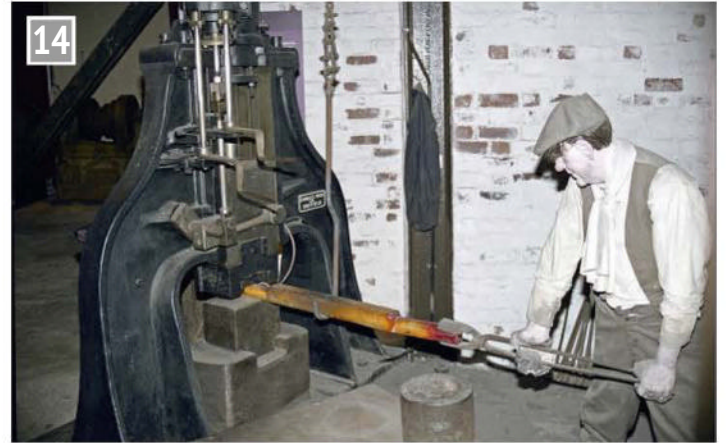
14 Steam hammer. Their use meant that much heavier forgings could be made and access to a source of water power was no longer needed. Later, hydraulic presses took over much of that work.
