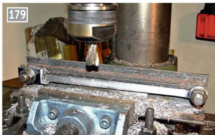
Thinning down a connecting rod.
