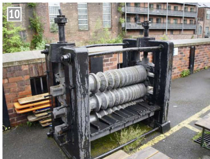
Example of a small rolling mill displayed outside. These could produce different profiles and even patterns on the rolled bars.
