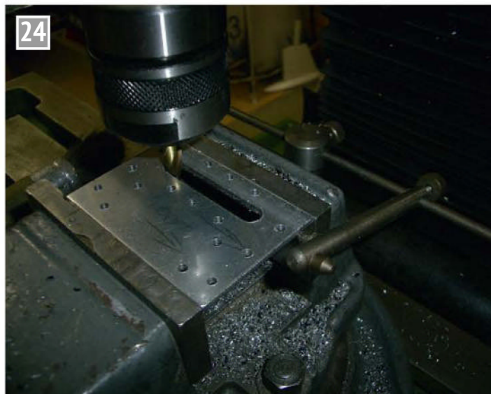
Machining a steam passage in a cylinder mounting plate.
