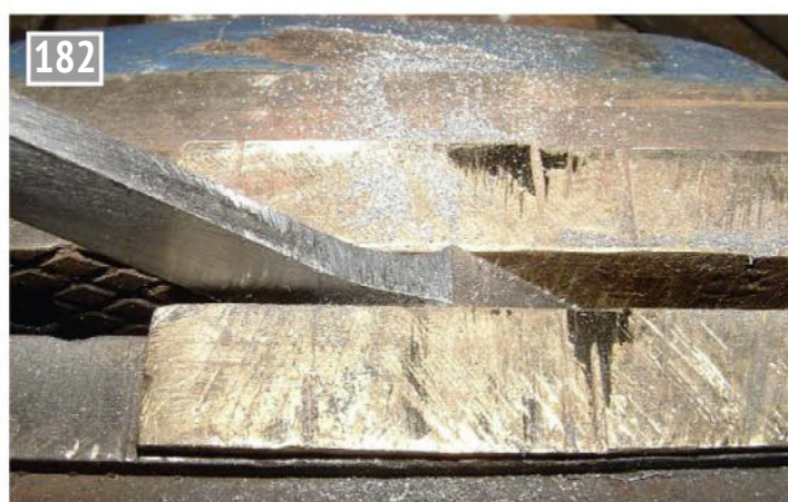
Using brass angle to protect the work while filing.
