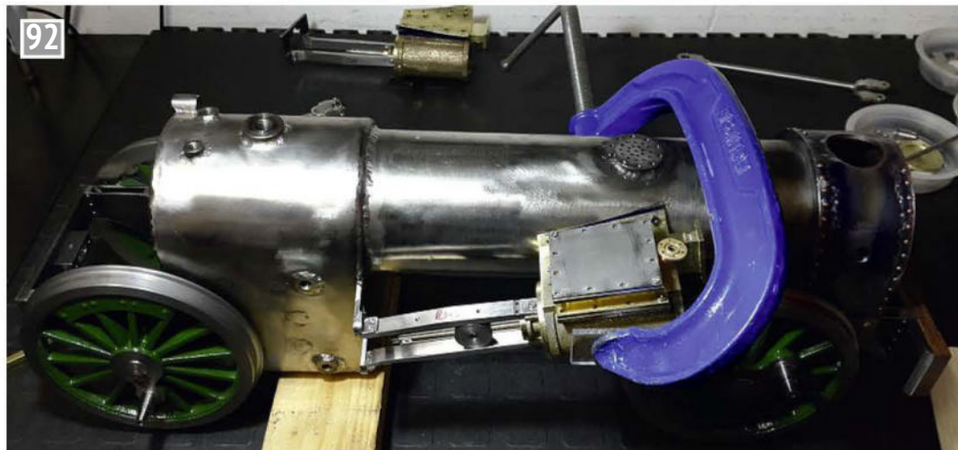
Fitting the cylinder to the boiler. The guide bar jig used to fit the motion plate and drill the guide bar mounting holes is visible. Connecting rod is not shown.
