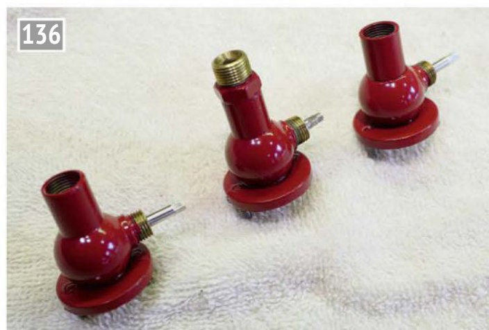
The two injector water valves, sitting on either side of the handpump isolation valve.
