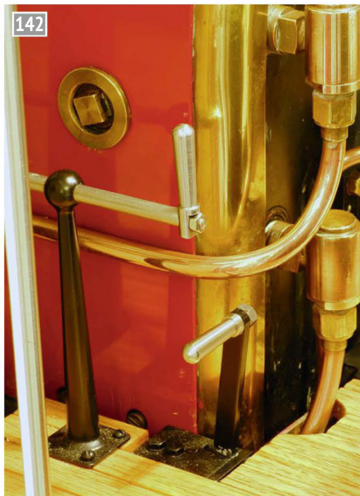
On the other side of the boiler, the left-hand extension rod is similarly supported. The ashpan damper control sits beneath the water valve lever on this side of the cab.
