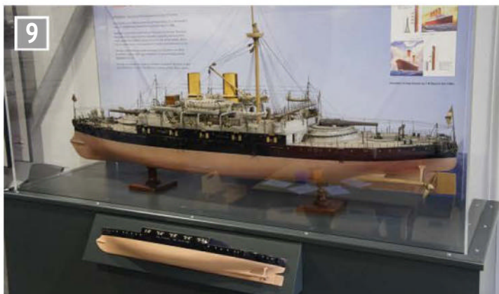
Model of HMS Benbow built by Thames Ironworks in 1888. It used armour plate of up to 45cm thickness rolled by Charles Cammell Ltd. of Sheffield. Most British warships used Sheffield rolled plate armour. Some of the first was used on HMS Warrior, now preserved at Portsmouth.
