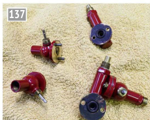
The water valves and the flanged tees to connect them to the tank. The handpump isolation valve is already attached, and the 'O'-ring seals are installed on the other flanges in readiness for the injector valves.
