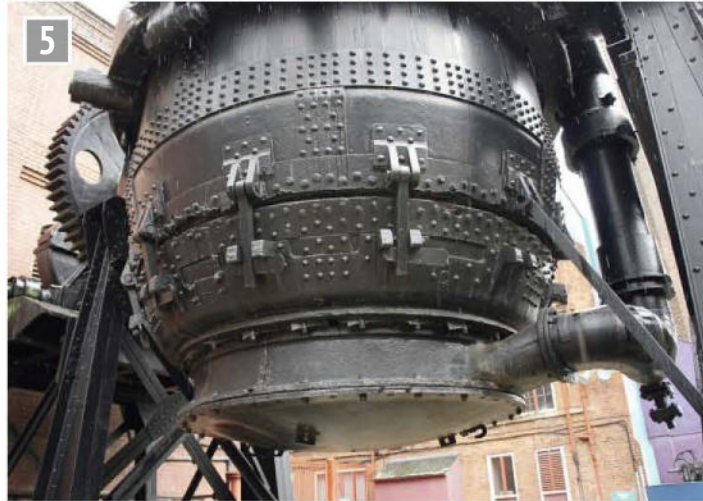
Base of a Bessemer converter. Hot air was blown from the base through molten iron, removing impurities, to make mild steel. There were many examples in Sheffield and blowing a converter was a spectacular sight.
