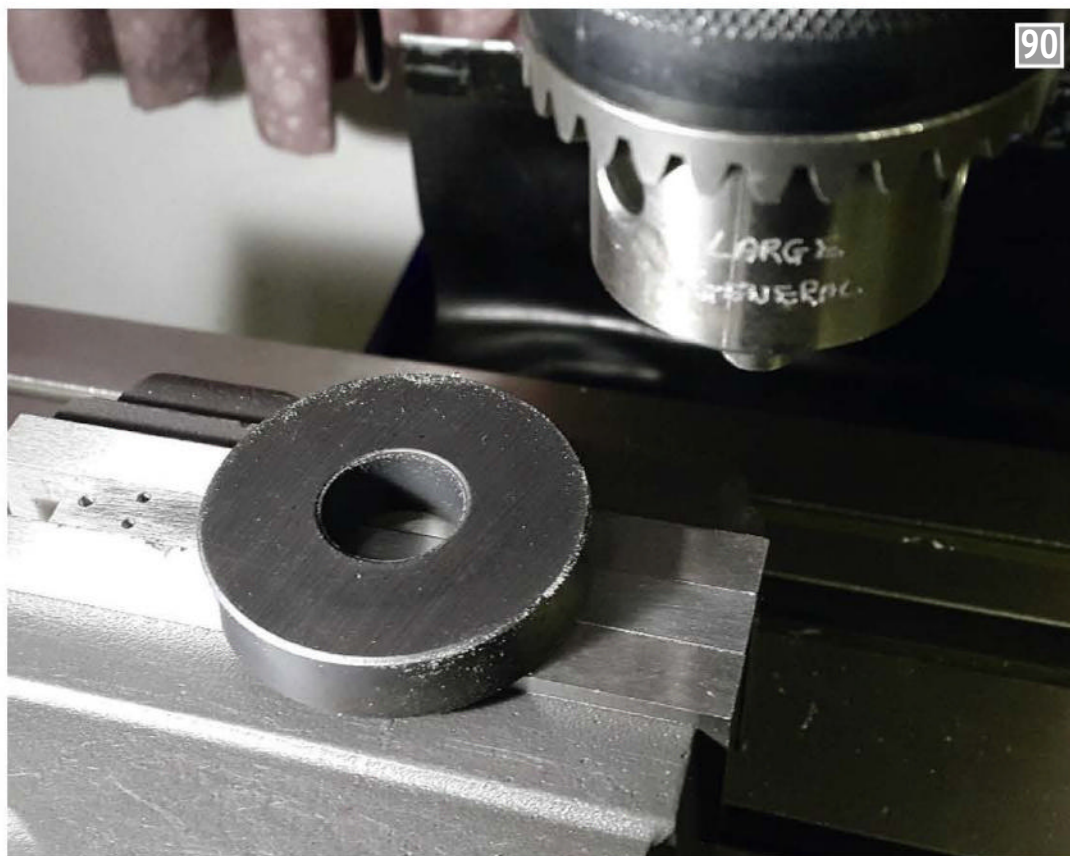
Lining up the guide bars to the top of a vice using a magnet.
