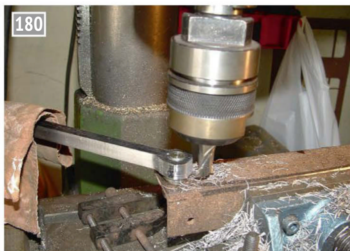
Profiling the end of the rod.
