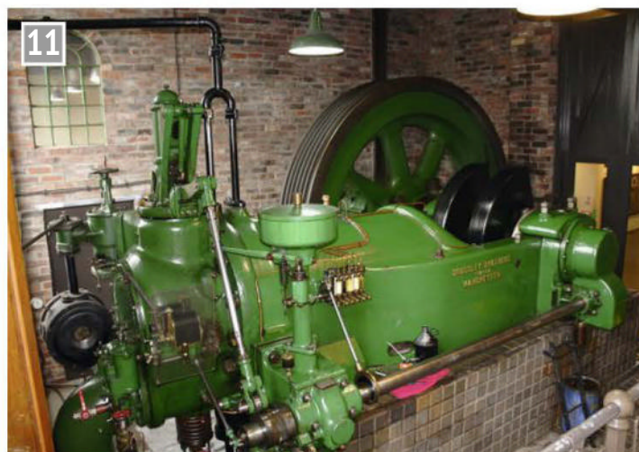
This Crossley gas engine once worked at Hadfield's steel works driving a rolling mill. It was built in Manchester in 1915.
