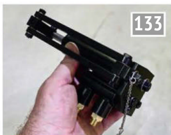
The finished handpump, minus its handle, ready to mount on the locomotive.
