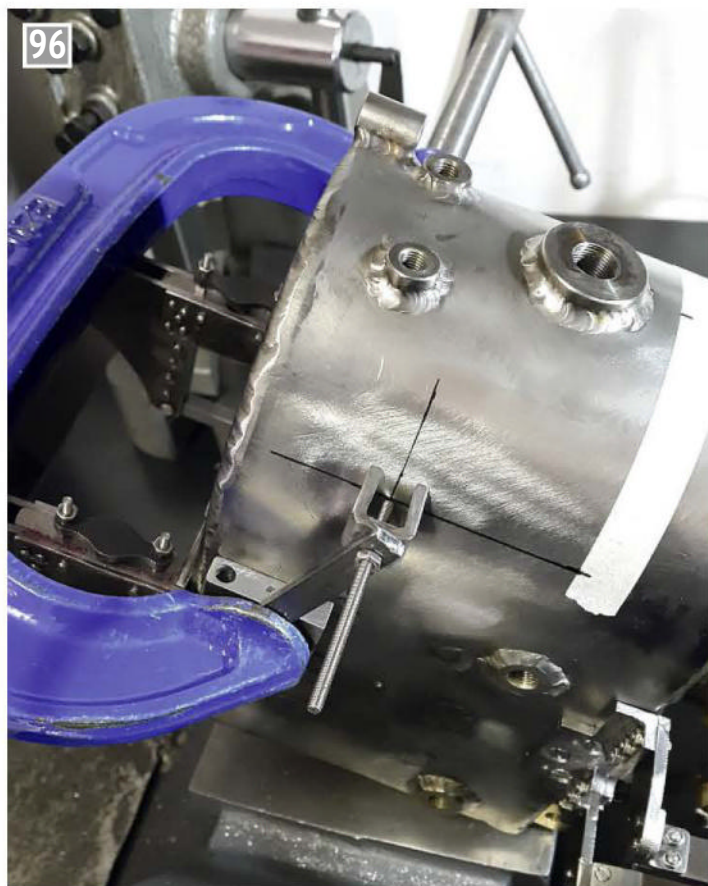
Clamping the reversing lever bracket in position using a threaded pointer and correct packing.
