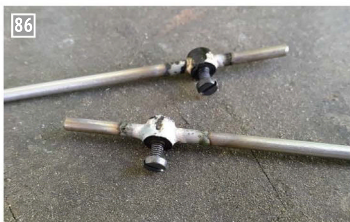
Valve rod spindle boss soldered in position ready for cleaning.
