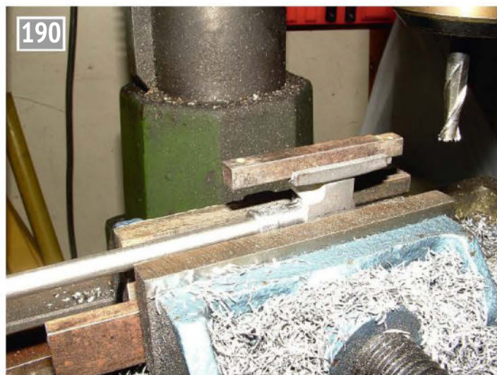
Machining a white metalling crosshead to size.
