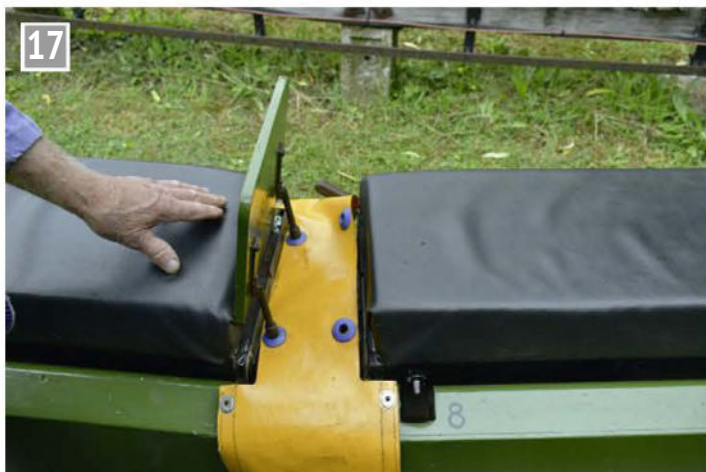
Passenger protection covers between carriages.
