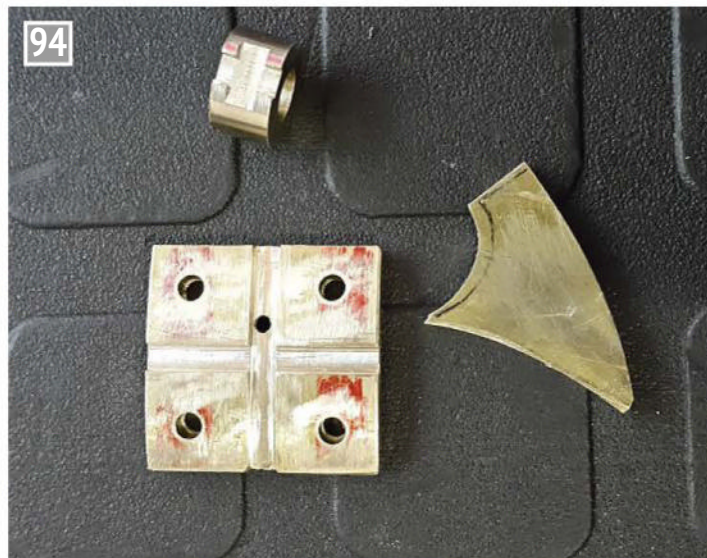
94 The main rocker mount components before (silver) brazing.
