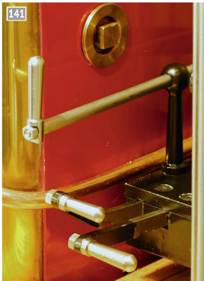
A stanchion supports the right-hand extension rod inside the cab. The cylinder and valve-chest drain cock controls lie below.
