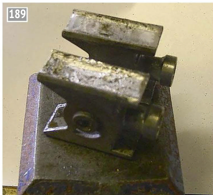
Crossheads white metalling.
