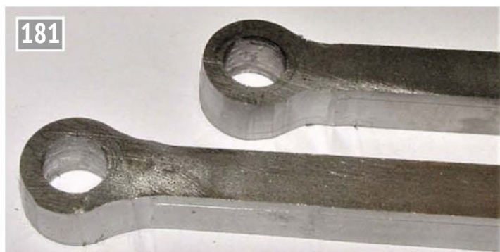
Connecting rod ends ready for finishing off.
