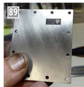
Reed valve fitted to the valve chest cover. The valve was made from automotive feeler gauge.
