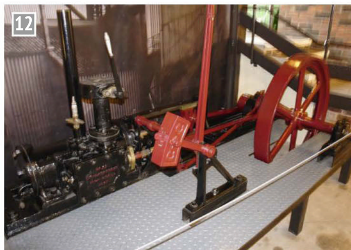
The original Stephenson Link valve motion, the first to allow 'notching up', allowing the expansive power of steam to be used fully.
