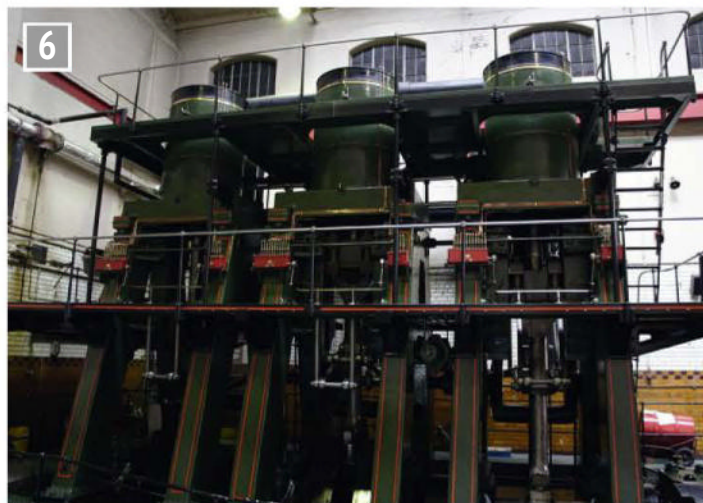
The mighty River Don rolling mill engine. Seeing this working is one of the most spectacular operations in any British industrial museum, even though it is deprived of the rolling mill. Reversing was done in just two seconds. A nearby video shows it as it used to operate.
