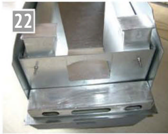
Coal chute sides added.
