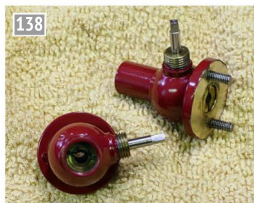
The threaded and screwdriver-slotted internal rings, which hold the 'O'-ring seals against the inlet and outlet side of the ball, and a ball itself, are evident in this picture of the injector water valves.
