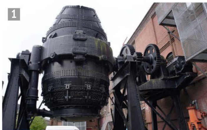
A Bessemer converter outside Kelham Island museum. Steel was key to Sheffield's industry. This example came from Workington in Cumbria and was re-erected under the guidance of Richard Gibbon OBE.
