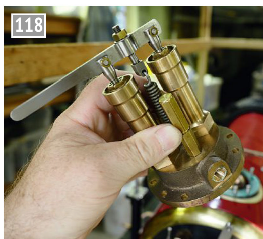
118 The steam-dome and its Ramsbottom safety valves, ready for installation over the regulator valve. A locknut will be added to the adjuster once the safety valves are set.
