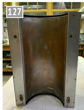
Cover plates enclose the bottom of the tank.
