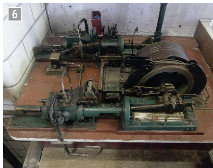
A severely neglected model winder.
