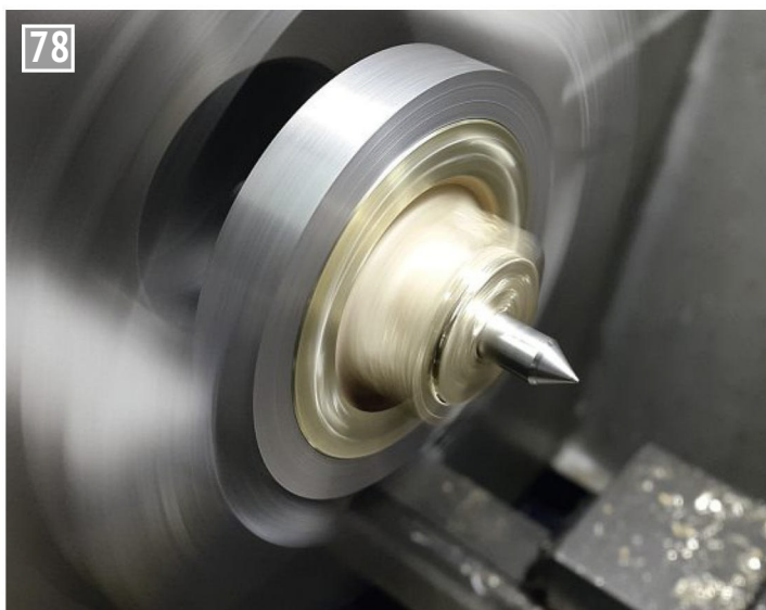
78 Checking the alignment of the centre hole with a pointer; if everything is a blur except the pointer, you're good!
