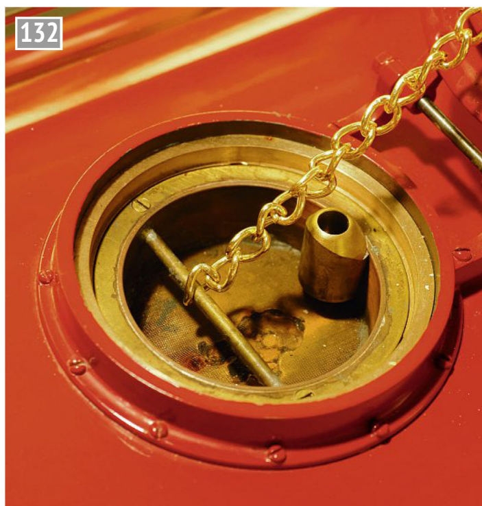
132 A more recent picture of the finished product, now with a snorkel to let the air out of the tank while filling!
