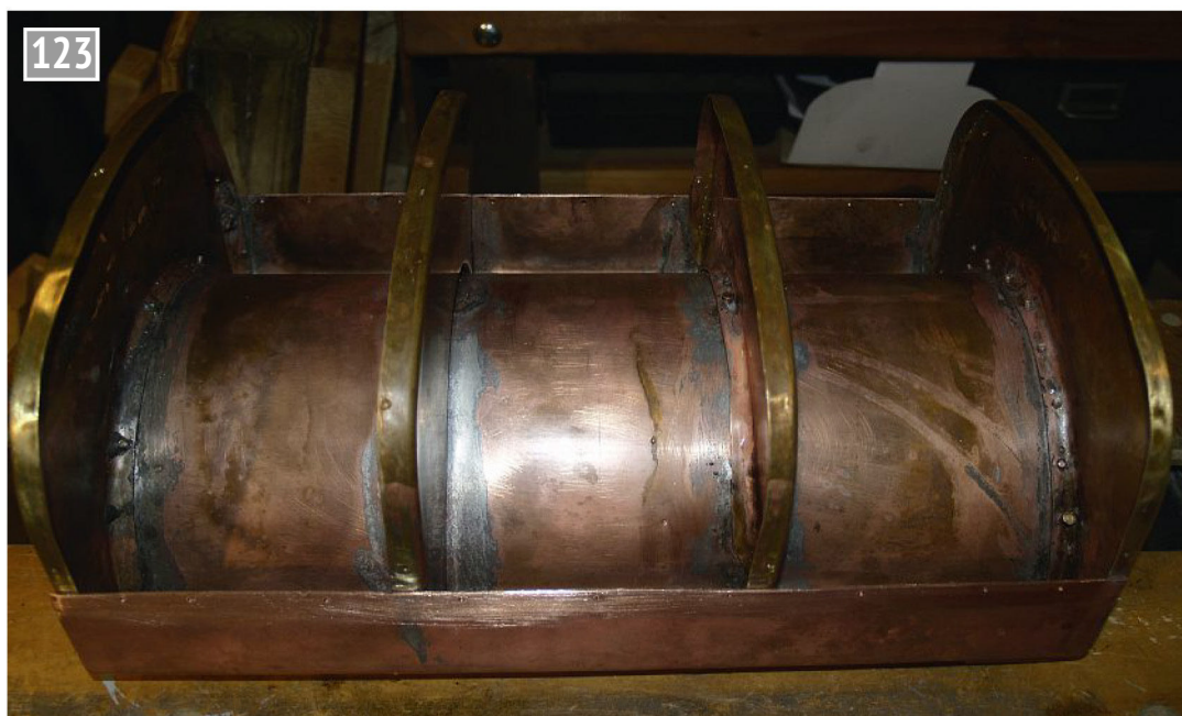
The inner saddle tank during construction, with flanged brass baffles and endplates and the rest in beaten copper.
