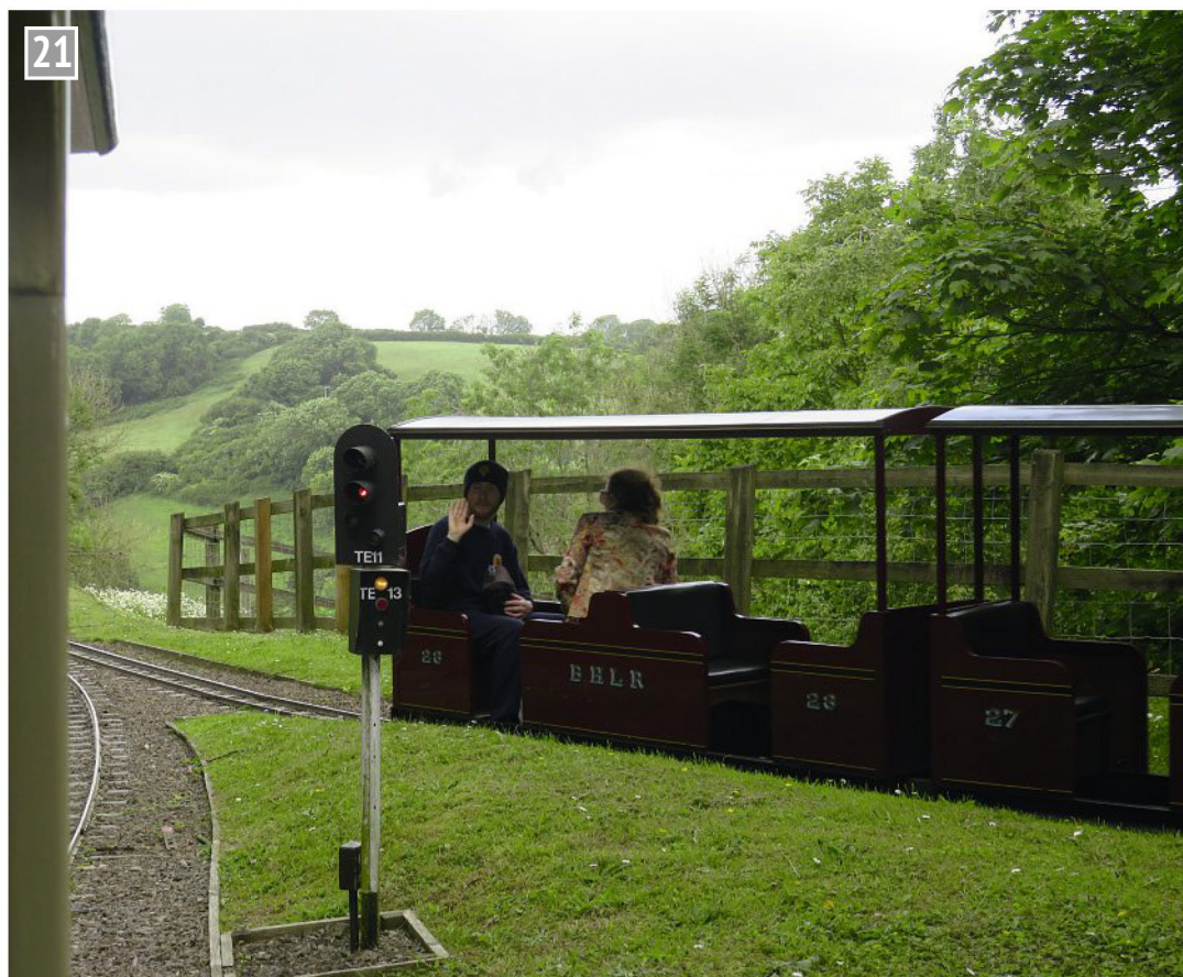
TE13 signal, now showing white as train has just cleared CM track.
