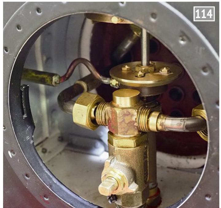
Laurie Lawrence's four-jet blower arrangement and the commercial ball valve to shut off the main steam pipe for boiler testing, pictured during a trial assembly to check that everything fitted and the blast pipe was concentric with the chimney. Fortunately, it did, and it was.
