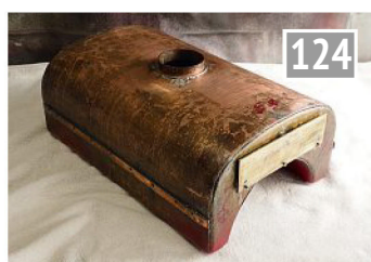
The completed inner tank, ready for its steel outer shell.
