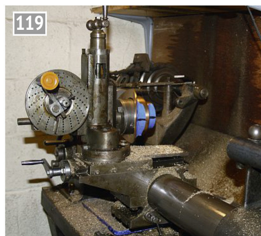
119 After much filing and emery cloth rubbing, the cast dome cover is mounted on the lathe's dividing head to mill the manifold slots.
