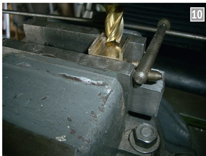
Machining an axlebox.
