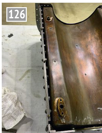
Some of the dozens of false 3/16 inch rivets, screwed and nutted inside.
