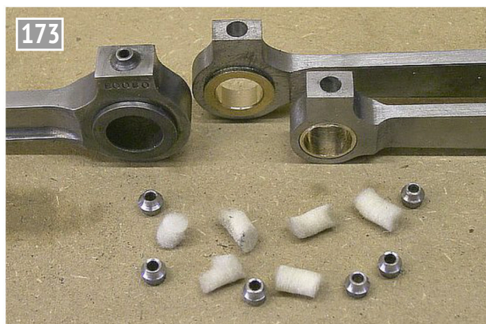
Rods correctly fitted with oil boxes.
