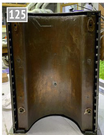
The inner water tank in its shell, a gap all around for future insulation.
