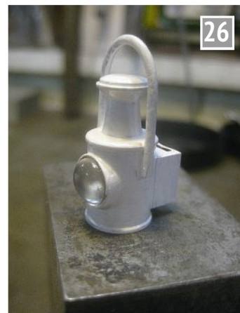
The lens is added to the lamp.
