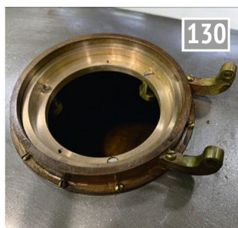
130 The filter housing in place. The cam-shaped lugs are rotated inwards during installation, then outwards once the housing is installed, then each is tightened to secure it against the underside of the inner tank's filler tube.
