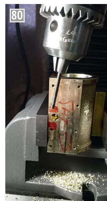
80 Checking alignment of the steam ports to the valve slots.
