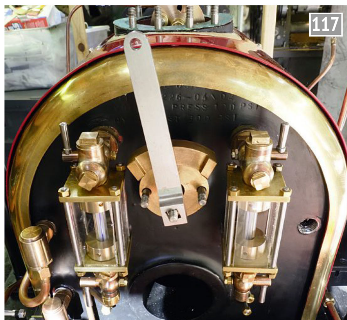
117 The three-cock water gauges, assembled and enclosed by their gauge-glass protectors, straddle the regulator quadrant. The top of the Stroudley-style regulator pokes through the dome flange above.
