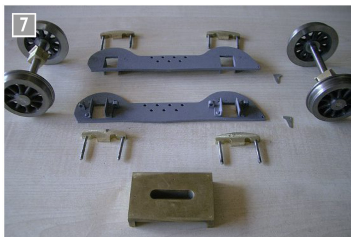
Bogie parts ready for assembly.
