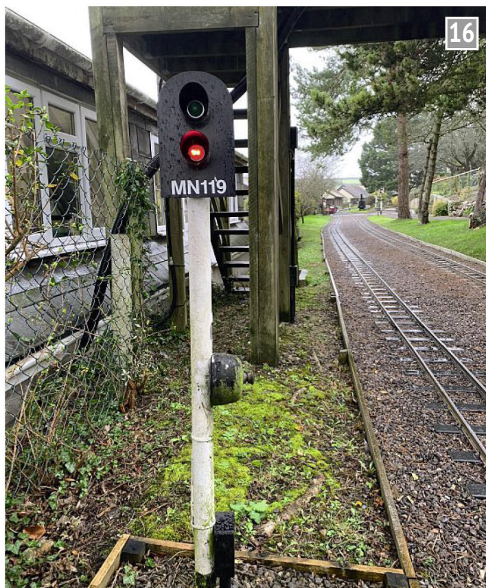
The plunger on Much Natter 119 signal allows drivers to request to go to shed.
