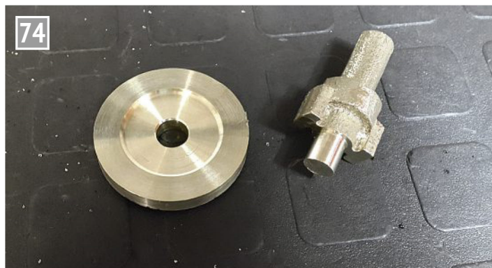
74 Piston side end cap components before soldering. With this configuration the piston rod slides on the stronger AlBr only.
