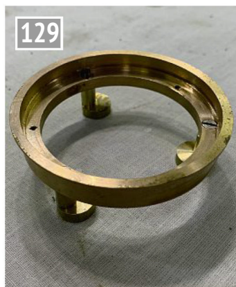
129 The filter housing with its three cam-shaped clamping lugs which secure it to the inner tank.
