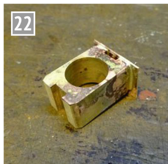
Forming the socket for the lamp iron.
