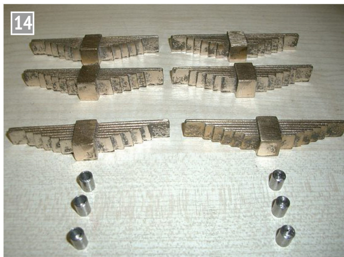
Cast springs for the tender.
