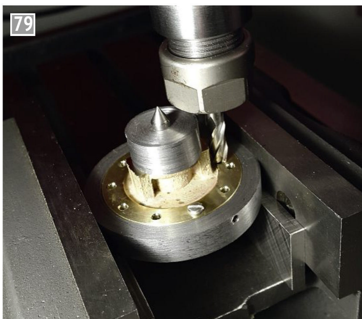
79 Machining the guide bar flats using a guide collar fitted to a shaft, slipped into the piston rod hole.
