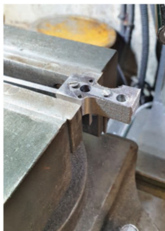
LEFT: 17. Once both blanks had been drilled I bolted the two together and began to profile the lower section. To get the parts to both fit and look like they are how they should be I have changed a few dimensions - in particular, I have used a smaller arc for where the bottom leg meets the upper section. This was done so as to allow the required parallel section to fit between the mounting plate lugs and also to avoid cutting into where the oil reservoir needs to be. RIGHT: 18. With all of the 'square' machining completed I then moved on to the various angles. I began with the angled rear face of the oil reservoir.
