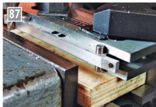
Cutting the tapered profile.
