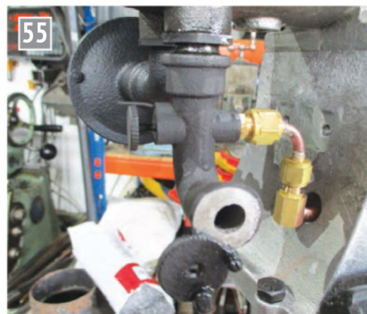
Carburettor and fuel valve in situ.
