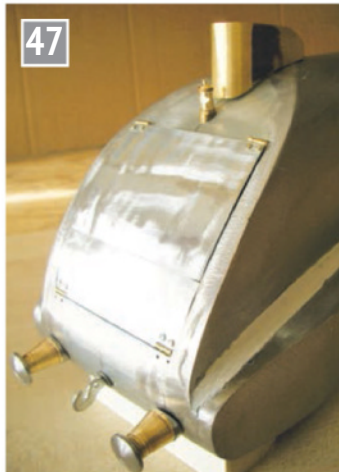
47 Chimney, whistle and buffers fitted.
