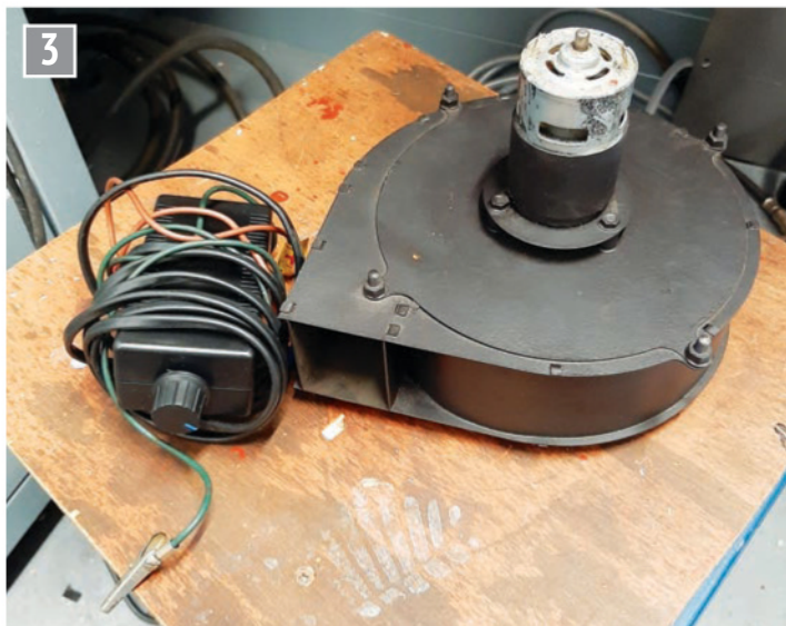
Completed blower and speed controller.
