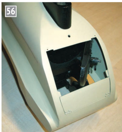
Access to the smokebox.
