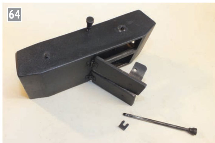
The completed ashpan and grate assembly; in normal operation it is not necessary to remove it as the fire can be cleared through the hopper doors. I wanted to keep the brake linkage as per the prototype.
