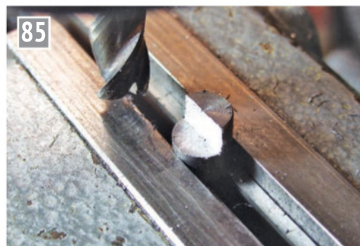
Milling a flat on the setting pin.
