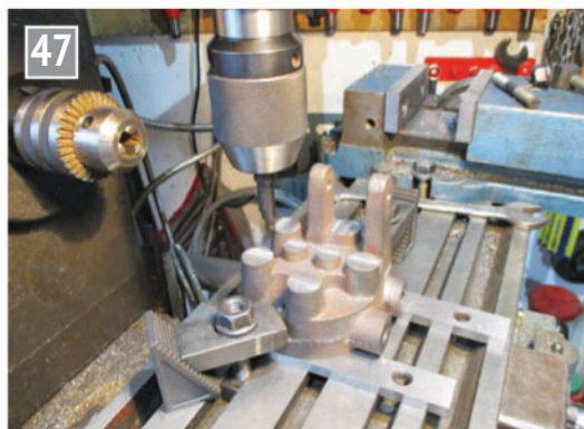
Preparing to machine the cylinder head.
