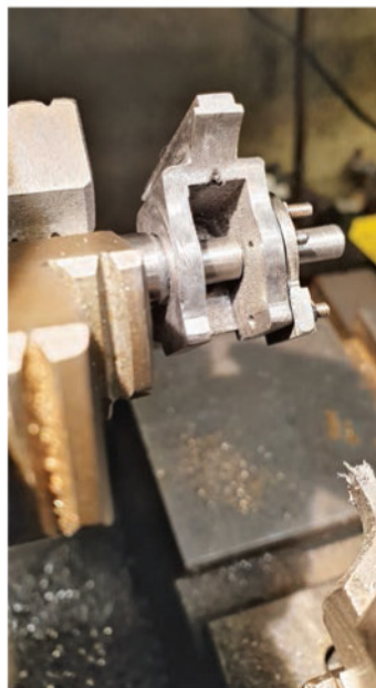
11. Here is a gudgeon pin being checked for fit on the crosshead.
