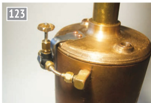
The blower valve support bracket riveted to the top casting and the short steam pipe added.
