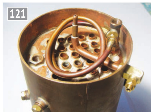
The blower pipe completed and attached to the boiler. The height of the outlet has been extended to ensure it is inside the base of the chimney.
