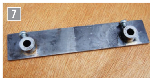
The guide bar with bushes silver soldered in place. Using Araldite didn't work.
