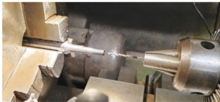
12. I then moved on to the 2BA threaded section, and drilled the oilway hole down the centre. The size drilled is 1.5mm using a cobalt bit and the hole was drilled until it reached just under half way into the journal.
