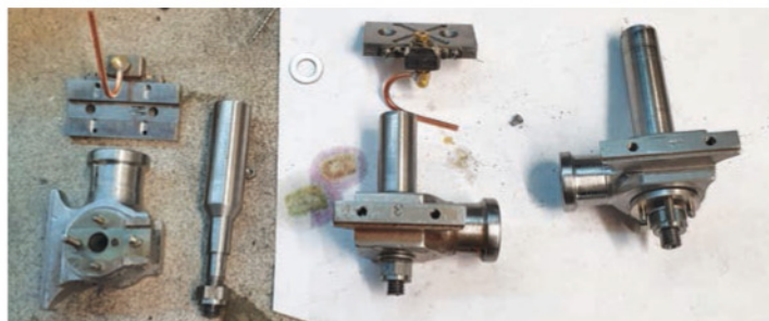
13. The nuts again were simple turning and threading 2BA. I have followed full size and machined a collar around one end which will also be castellated soon. Unlike the other castellated nuts, these will have eight slots instead of the usual six. In this picture, the two on the right have had their central oil way drilled and the one on the left is awaiting the same exercise. Once I have drilled the cross-drill oil way in the journal I'll part off to size.
