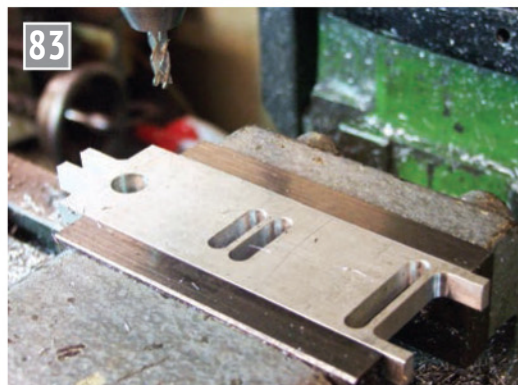
Initial steps in forming the cutouts in the end link.
