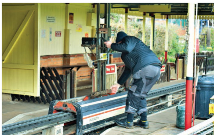
Lowering one of the passenger carriages onto the main track.
