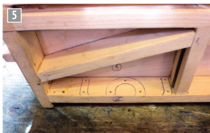
W-iron position marking.
