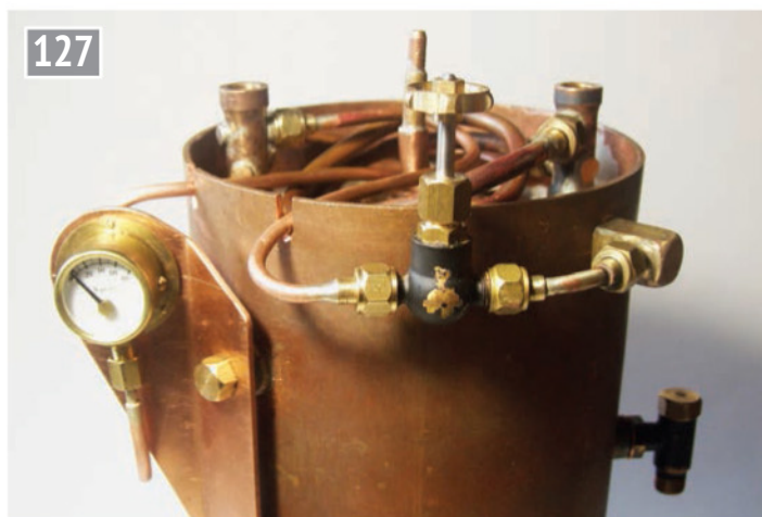
Another view of the mounting plate fitted to the boiler with its pressure gauge.
