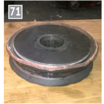
71 This is the water cylinder piston with both new seals and tensioning springs fitted. The steam piston has conventional piston rings fitted.
