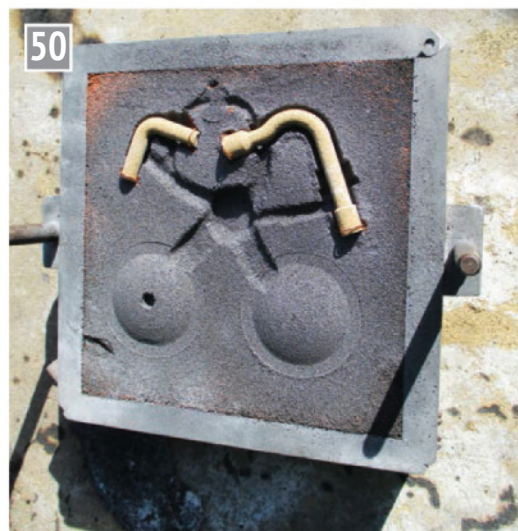
Preparing the mould and cores for the carburettor and silencer.
