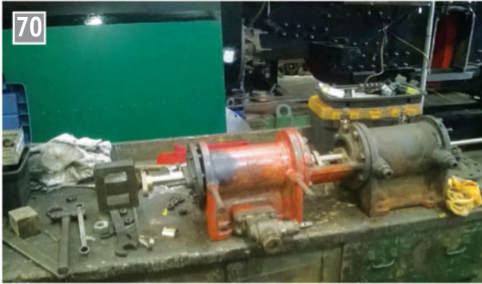
70 The Bulleid reverser during overhaul at Ropley. Apparently, a blend of the SECR and LSWR designs, but the principal and main components remain the same as the L class device.
