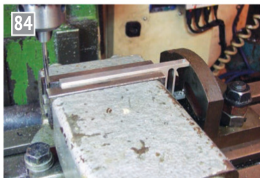
Drilling and reaming the holes in the clevis for the end link pin.
