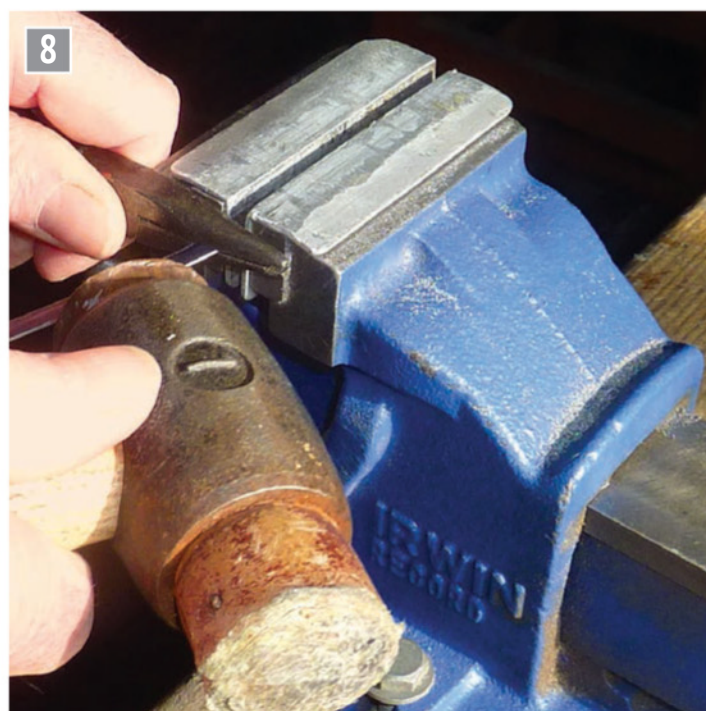
Bending a diagonal strap.
