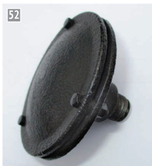
The finished silencer.
