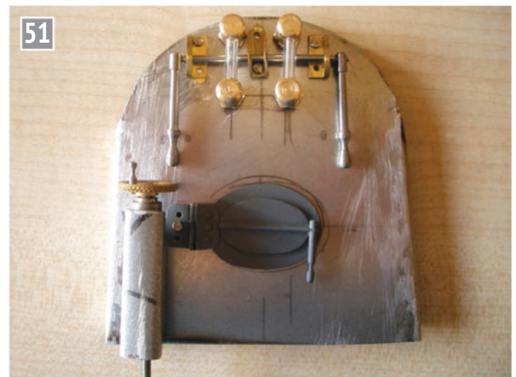
51 Boiler backplate with fittings.
