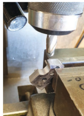
LEFT: 17. Once both blanks had been drilled I bolted the two together and began to profile the lower section. To get the parts to both fit and look like they are how they should be I have changed a few dimensions - in particular, I have used a smaller arc for where the bottom leg meets the upper section. This was done so as to allow the required parallel section to fit between the mounting plate lugs and also to avoid cutting into where the oil reservoir needs to be. RIGHT: 18. With all of the 'square' machining completed I then moved on to the various angles. I began with the angled rear face of the oil reservoir.
