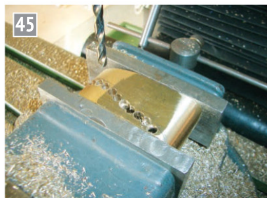
Chain drilling the chimney profile.
