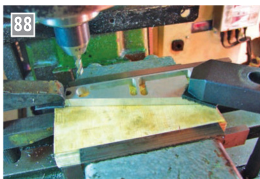
Finishing the cutouts in the end link.
