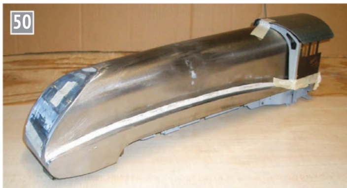
50 Cab united with the casing.
