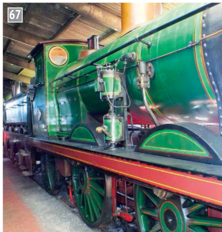
SECR number 65 at the Bluebell. The reverser is the same as the one fitted to the L class and many other SECR designs. Steam cylinder at the top with the slide valve housing on the side. The steam supply is taken from the dome via a pipe inside the boiler. Water cylinder at the bottom with the linkage from the control valve back to the cab prominent.
