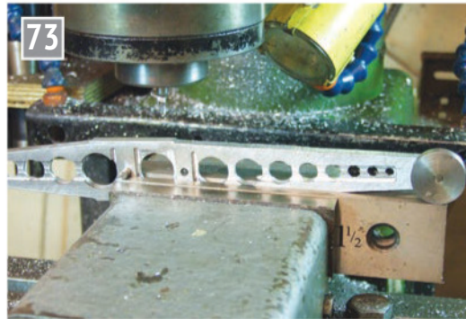
Setting up for profiling the beam.
