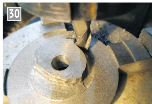
Roughing out the profile on the mill.
