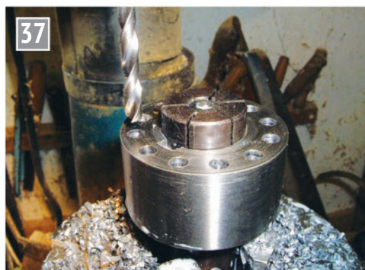
Drilling the positions of the cutter teeth.
