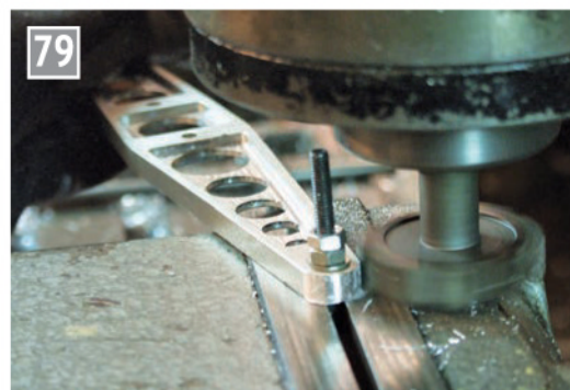
Rounding the ends of the beam.
