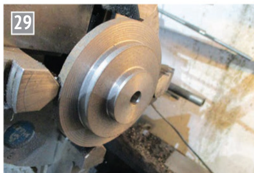
Producing the blank for the cam.
