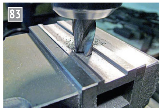
Machining the sides of the axleboxes.
