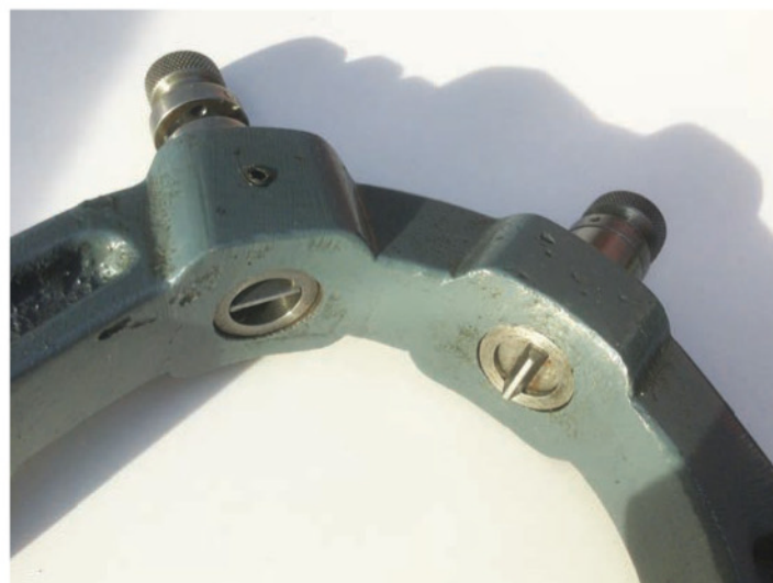
Showing the detent wedges, one in the engaged position, the other withdrawn and locked back.
