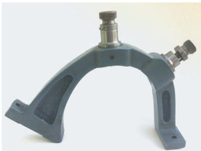
The detents are held in the casting by grub screws - optionally one or two per detent.
