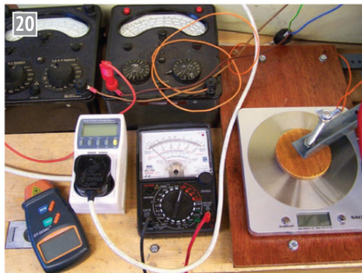
Instruments - Top row (left) main winding amps; (right) auxiliary winding amps; Bottom row from left: tachometer; Power and Energy Monitor for measuring power factor/input watts/ input volt-amps/total amps; capacitor volts; and torque using kitchen scales.
