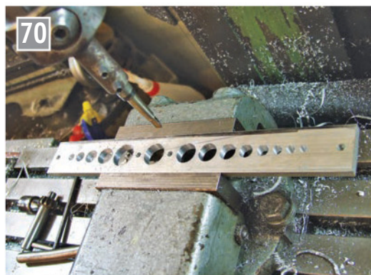
Drilling the lightening holes.
