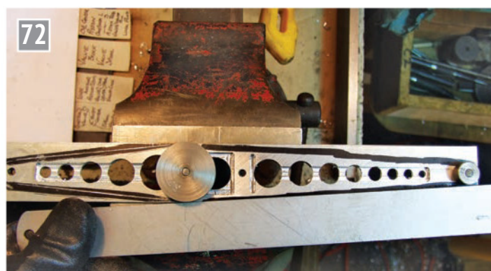
Marking out the outside profile.
