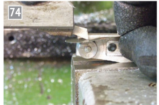
Locating the depth of the cut for profiling.
