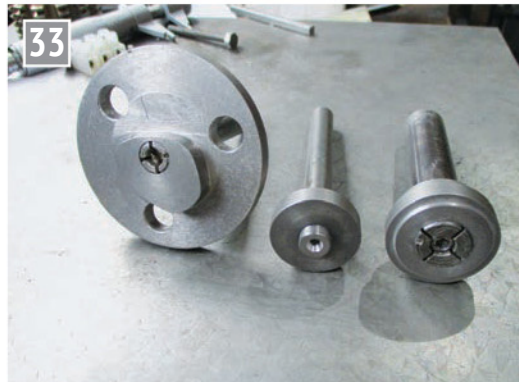
The cam and blanks for the gears.
