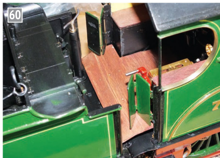
The finished locomotive and tender together, with the floor in place and wooden seats on top of the box splashers and folding cab doors.
