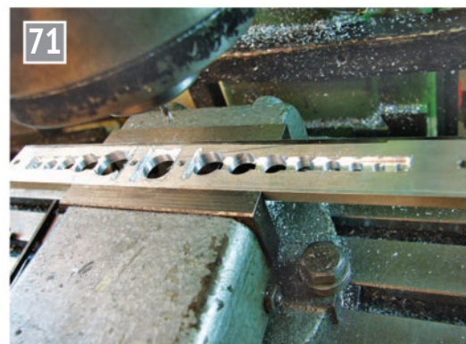
Initial machining of the recesses.
