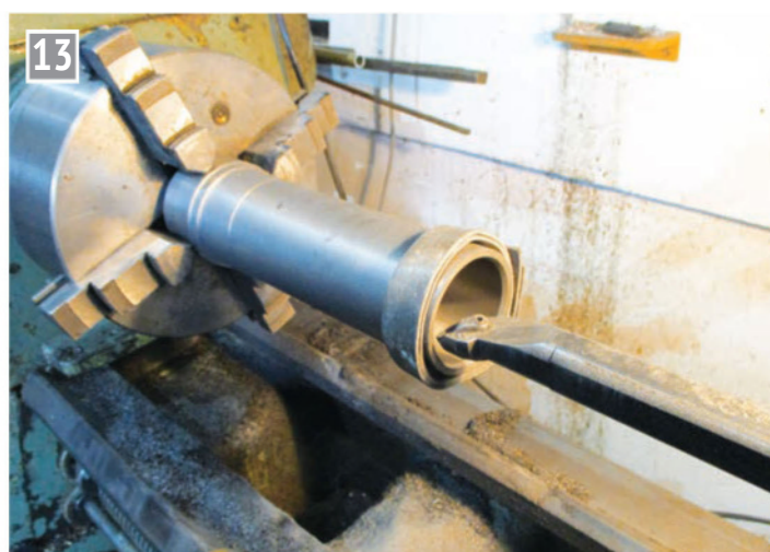
Boring the cylinder sleeve.
