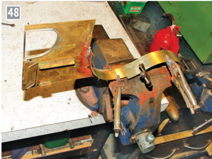
The cab beading has been finished in this photo and I have fixed small brass angle brackets to the sides of the splashers to support the tops. The folding cab doors are also fitted, as is the angle to support the seat tops.
