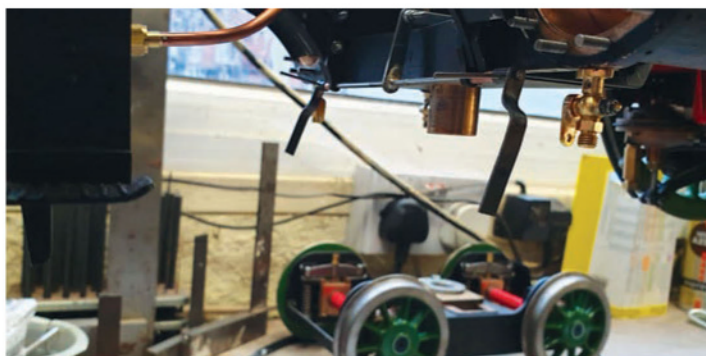
21. Here the cross shaft is temporarily fitted for me to fabricate the end arms so that they line up.
