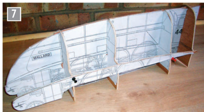
Building jig for the casing.
