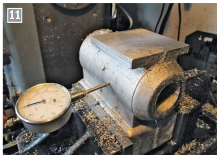
Preparing to skim the casting to get a reference surface.
