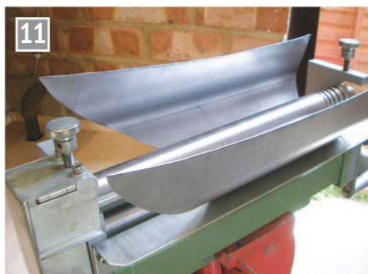
Rolling the front section of the casing.
