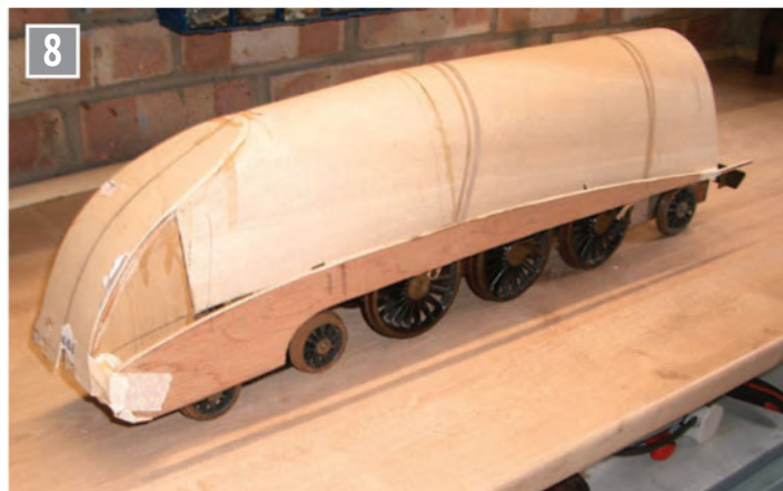
Mock-up made before cutting steel.
