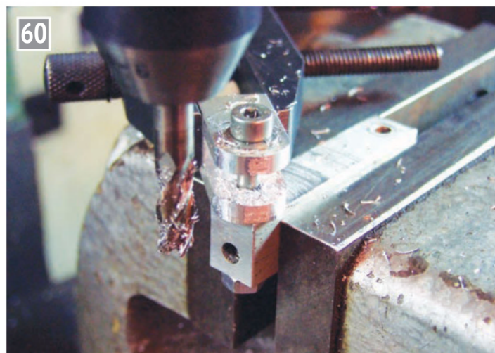
The end result of the rounding operation.
