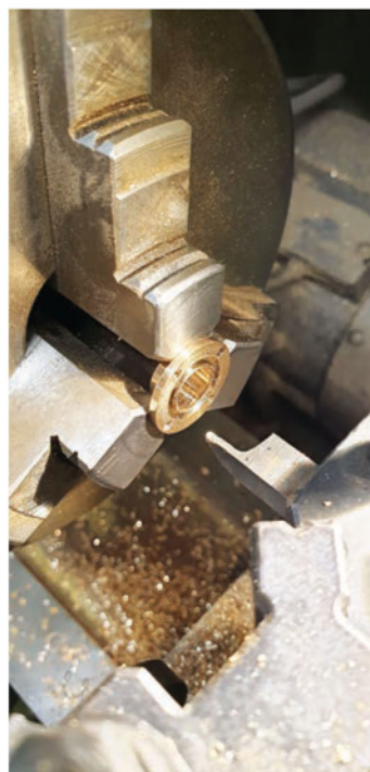
LEFT: 17. This picture shows the first flange being parted off. RIGHT: 18. I added an 'O' ring rather than rely on a plain gasket and here I have machined the groove for the 'O' ring.
