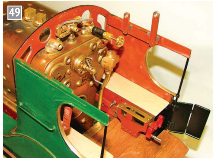
Construction of the cab roof hinges is complete; the next task is to try and fit everything into the limited cab space. Silver soldered elbows for the injector steam valves sit on top of the firebox, either side of the whistle valve.
