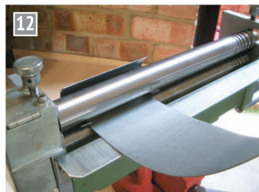
Rolling the front door section.
