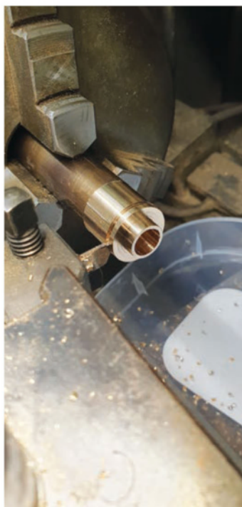
LEFT: 17. This picture shows the first flange being parted off. RIGHT: 18. I added an 'O' ring rather than rely on a plain gasket and here I have machined the groove for the 'O' ring.
