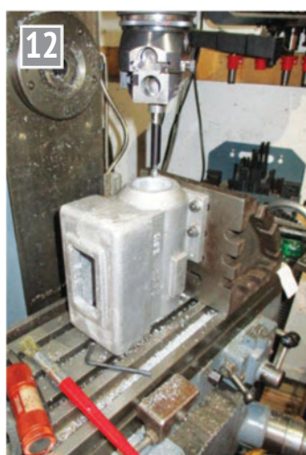
Boring the cylinder casting.
