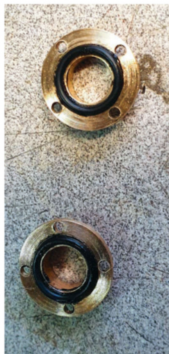
LEFT: 19. To make life easier when mounting the flanges to the cylinders I used a small amount of the high temp silicone used for sealing the exhaust outlets to hold the 'O' rings in place. RIGHT: 20. Here's one of the flanges bolted in place.
