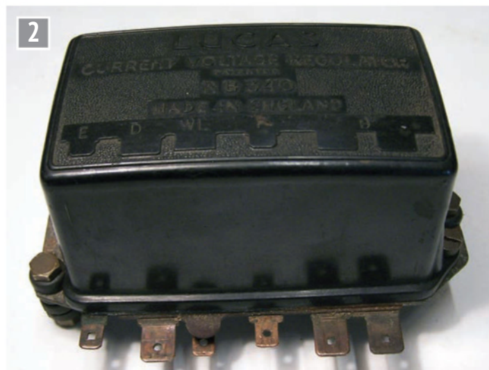
The Lucas RB340 current voltage regulator.
