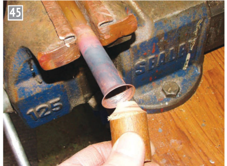
45 There is enough spare tube to be able to cut off the piece that is in the vice which has been squashed a bit out of round.
