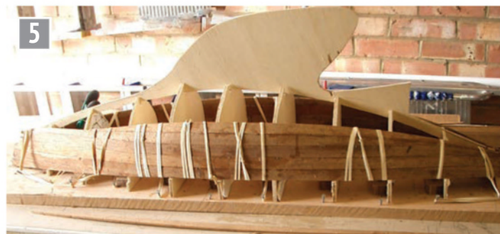
An example of plank on frame construction.
