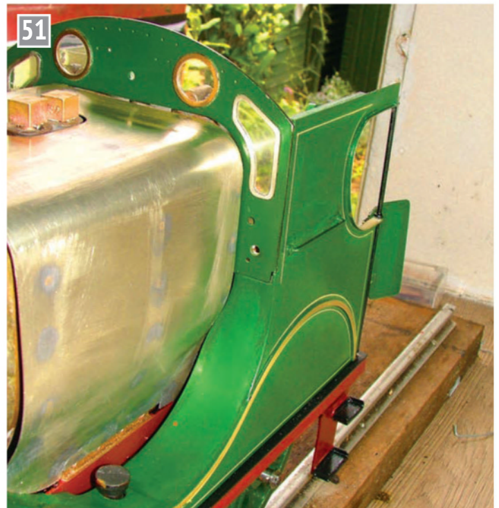
The brass beading has now been fitted to the cab and splasher sides and I have begun the boiler cladding. Unscrewing the rear sandbox filler lids and a couple of screws under the footplating will release cab sides and splashers as one unit for any future dismantling.
