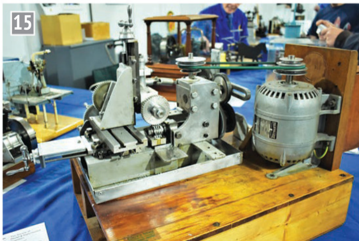
The useful Tom Jacobs gear cutting machine.
