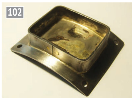
The fabrication looking bright again with the required solder joint all round.
