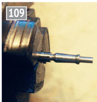
Turning the handle for the latch and leaving extra material for the silver soldering operation.
