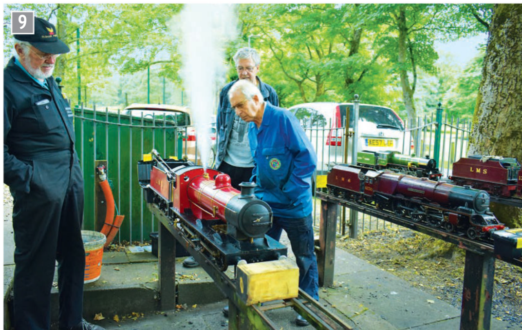
Up to pressure with the boiler inspector checking the safety valves.
