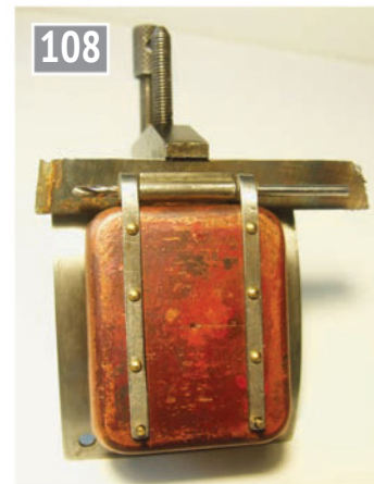
The parts for the door assembly clamped to the frame to check the closing action of the door and rivets added once the alignment is correct.
