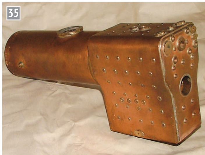
35 Close to scale dimensions the boiler looks the part. Silver soldered throughout, with rod firebox roof stays as per full size. It will operate at 80 psi, hydraulically tested to 160 psi.
