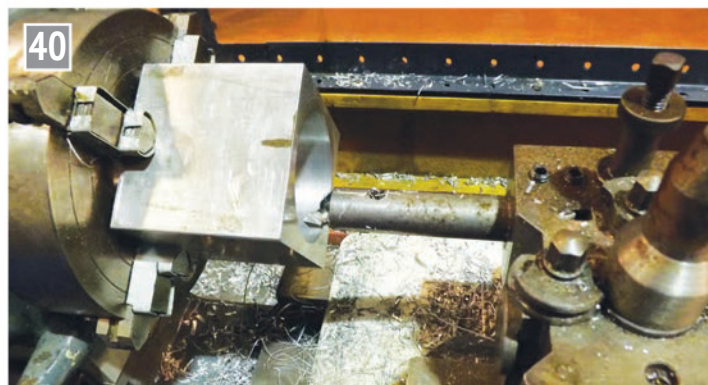
Boring the cylinder block.
