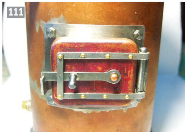
The door frame with the latest parts in place on the boiler.
