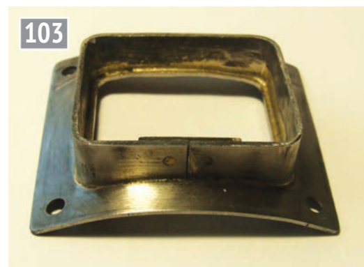
Here the centre of the curved plate has been removed by drilling through each corner and filing up to the edges to the surrounding frame.
