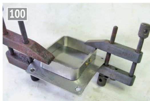
Here the lap strip has been riveted in place and the frame positioned on the cover plate for fluxing and soldering.
