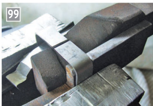
The final corner bend for the door frame with sufficient 'random' packing being used to keep the outline square in the vice. An adjustment was required on the two opposite corners.
