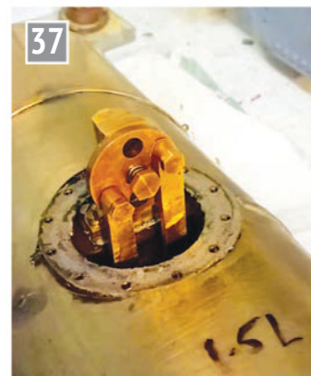
36 LEFT: regulator support cast integrally with the dome ring makes a neat job; a joining ring was also cast to mate the boiler barrel to the front of the firebox. RIGHT: The regulator is in place ready for the hydraulic test. The boiler capacity is 1.5 litres.
