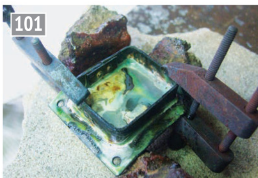
This shows the door frame silver soldered to the fire hole cover plate and ready for cleaning up.
