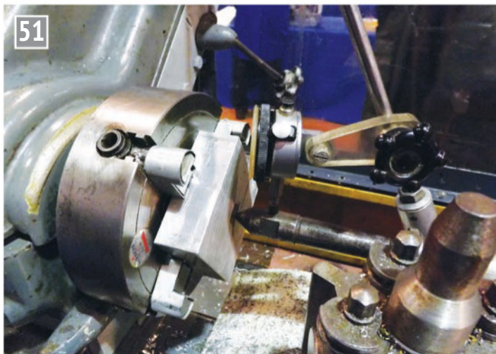
Setting the cylinder cover to run true.
