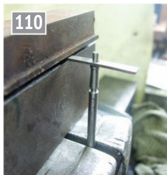
The latch and the embryo handle set up for the soldering whilst still attached to the rod.
