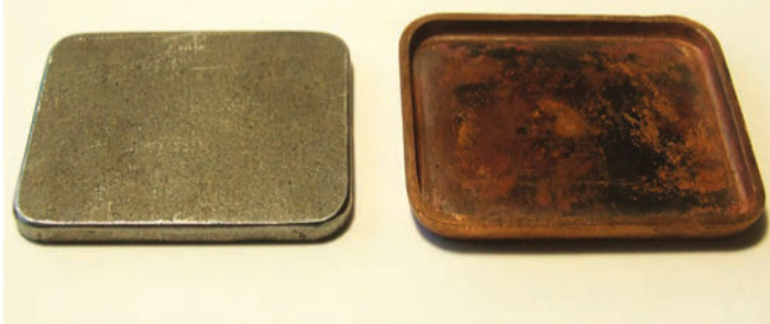
The door made from copper sheet with the forming plate alongside.
