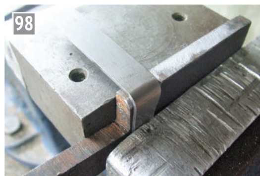
Here the strip is centrally located on a forming bar for the two upper corners to be made.
