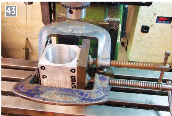
43 Securing the block before drilling and tapping the cover securing holes.
