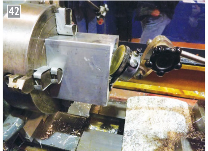
42 Setting the block to run true after turning it round end for end.
