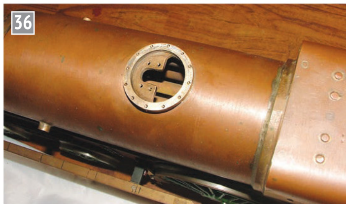
36 LEFT: regulator support cast integrally with the dome ring makes a neat job; a joining ring was also cast to mate the boiler barrel to the front of the firebox. RIGHT: The regulator is in place ready for the hydraulic test. The boiler capacity is 1.5 litres.
