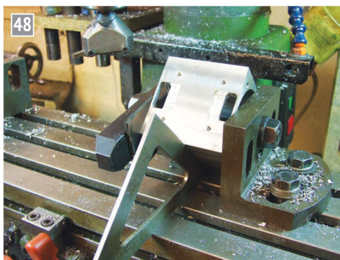
Milling the ports into the cylinder block.
