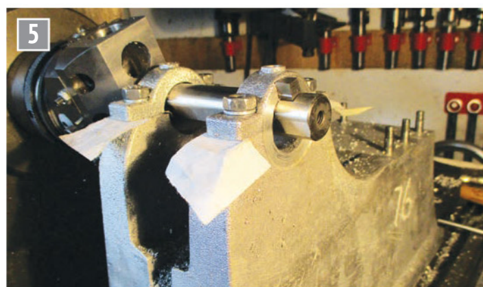
Final machining of the holes for the bearings.
