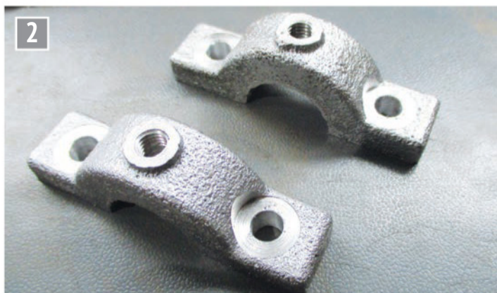
The newly cast bearing caps.
