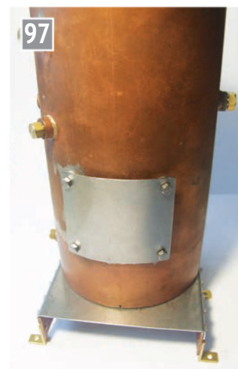
The fire hole cover plate bolted in place on the boiler barrel.
