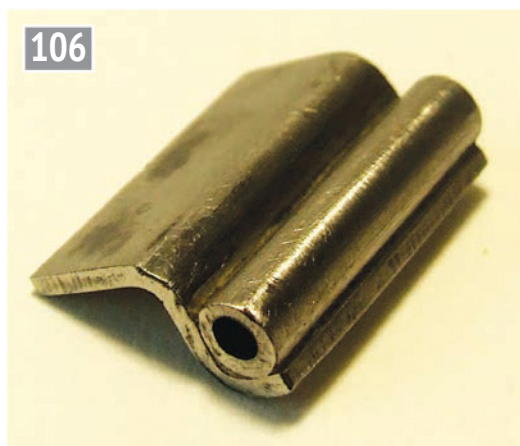
Two views of the door frame hinge bracket silver soldered to the tube.
