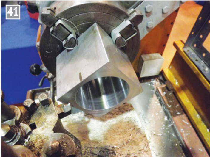
41 Skimming the face of the cylinder block.
