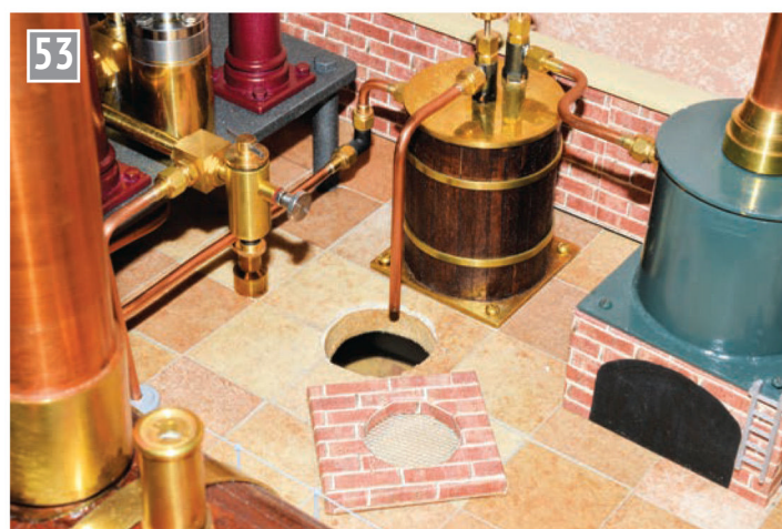
Drain for the condenser.
