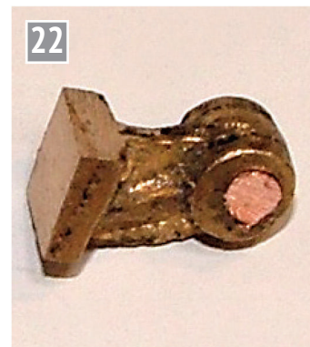
22 One of the rocking lever brackets needed reclamation by silver soldering - the only bad casting on the locomotive fortunately, as there was no opportunity to recast.
