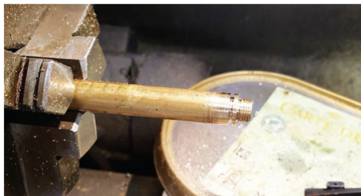
1. Here is one of the glands machined.
