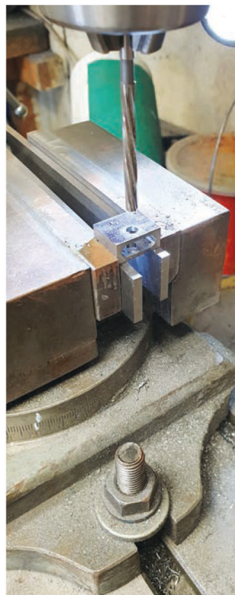
8. I then re-clocked to give me a register for the width of the cross-heads to enable drilling on the other axis. First hole seen here is the hole for the link pins, drilled in steps and reamed to finish. I then drilled all five crossheads for their taper pins.
