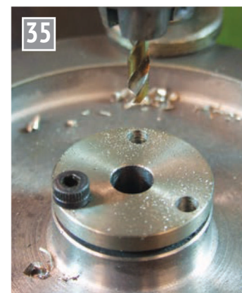
Drilling the collet fixing holes.
