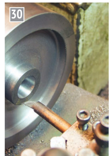
Boring the taper in the flywheel.
