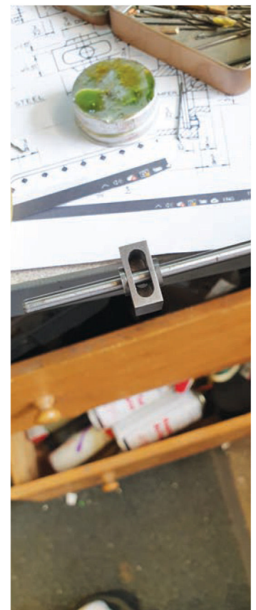
9. To complete the three conjugating lever cross-heads I had one job left to do and that was to add to both top and bottom of the cross-heads. This was simple turning. I decided to use a retainer to bond the parts rather than applying heat and using solder.
