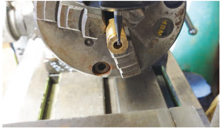
4. Once happy with the gland fits, each in turn had its slots machined on the rotary table.
