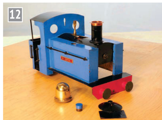
Her dome, the water tank lid and the smokebox front provide access for water, fuel and a match respectively.
