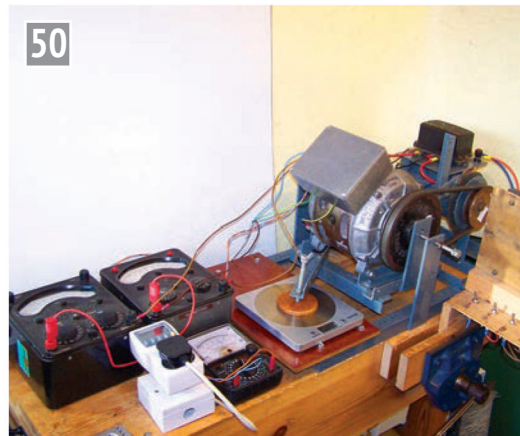
The dynamometer with the motor in place.
