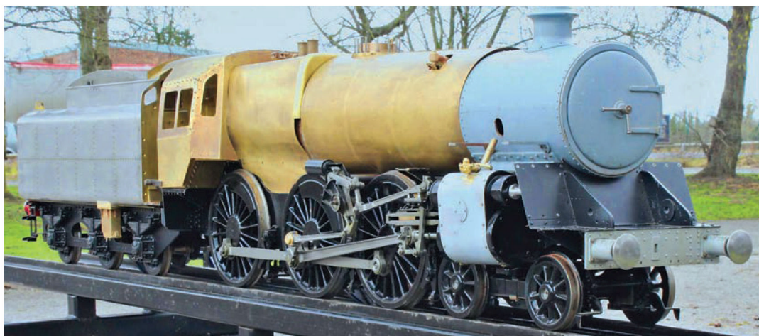
Merlin's unfinished five inch gauge Standard 5. He made several visits to the Watercress Line to ensure that all details were correct. (Photo courtesy of Station Road Steam.)
