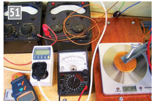
Instruments - Top row from left: main winding amps; auxiliary winding amps; Bottom row from left: tachometer; Energy Monitor for measuring power factor/input watts/ input volt-amps/total amps; capacitor volts; torque using kitchen scales.
