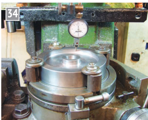
Setting the flywheel taper to run true on the circular table.
