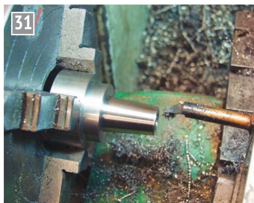
Turning the taper on the flywheel collet.
