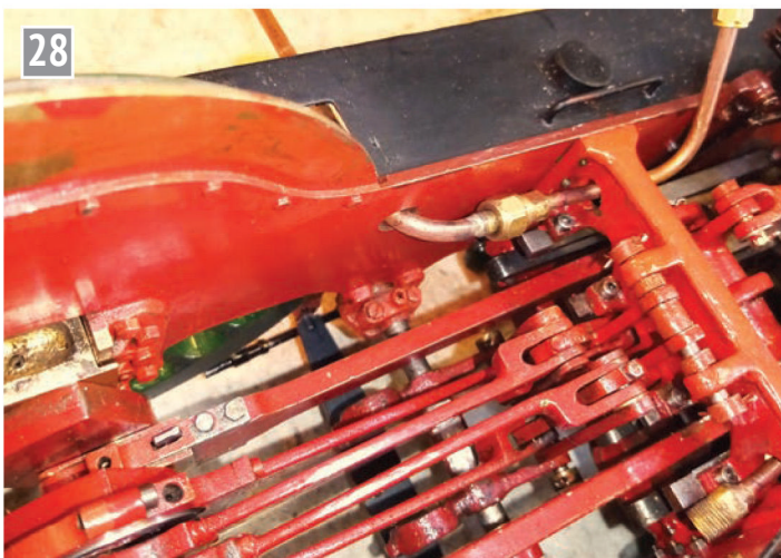
In this view the eccentric rods can be seen. Note also the wedges securing the big end bearings. The feed pipes to the front boiler clacks are threaded through the frames and motion plate as on the full size.
