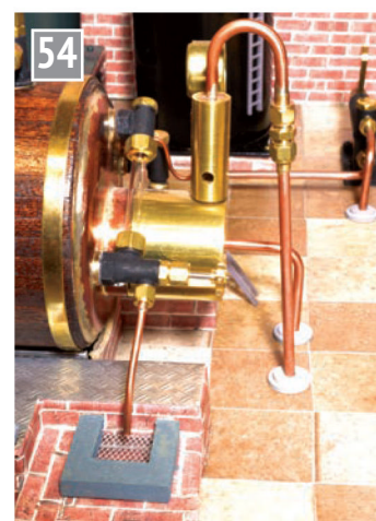
Drain for the sight glass.
