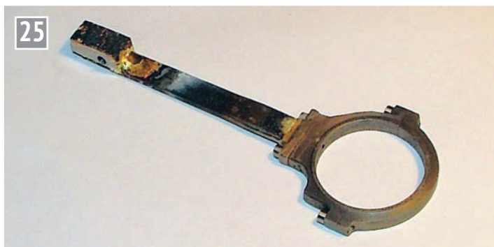
25 A block is brazed to the forward end of the eccentric rod; a hole has been drilled as a guide for milling the slot to form the jaws.
