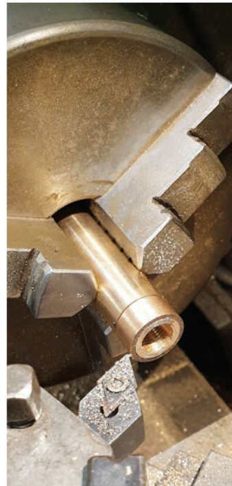
16. Then there were two other parts to make, those being three of each size nuts, one size from \frac{3}{16} inch hex, drilled and tapped \frac{5}{16} inch x 32 tpi to fit the bolt, and the other from \frac{5}{16} inch hex, drilled and tapped \frac{3}{16} inch x 40 tpi to lock the bobbin bolt to the spindle. The picture shows all three made - one is in the steam chest, one complete and the other to show the parts involved.
