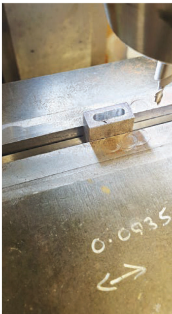
6. Having drilled a row of three holes, I machined an undersized slot using a 3mm cutter. This completed the roughing out stage and the slot is undersized on both axes. Alas I forgot to take a picture of the slot at finished size - it can be seen in later photo's though.
