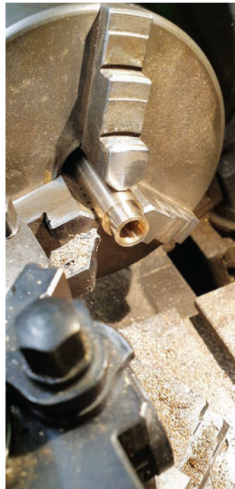
LEFT: 17. First job to do to the bronze bar was to drill the centre and tap for the bobbin end. RIGHT: 18. I then turned down the end for the Fluorosint ring to fit on when machined. The length of the journal here is slightly longer than the slip gauge made.
