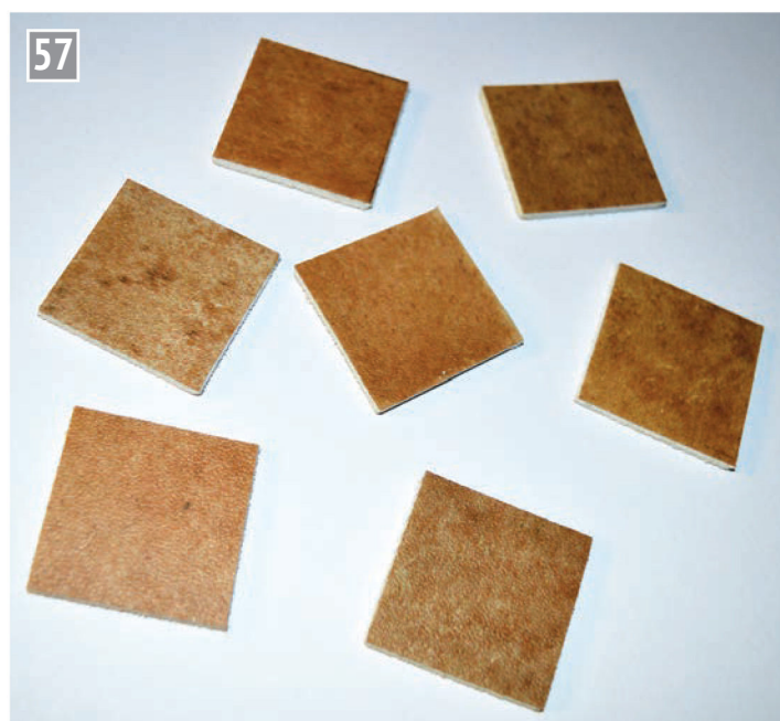
Tiles cut from vinyl sheet.
