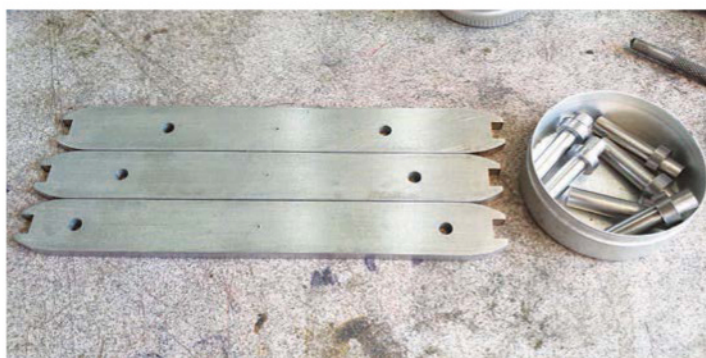
14. The three brake beams with the holes drilled for the pull rod pins - from top to bottom, trailing wheels, centre and leading wheels.
