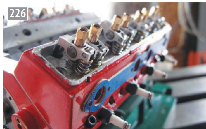
Completed rocker assembly.
