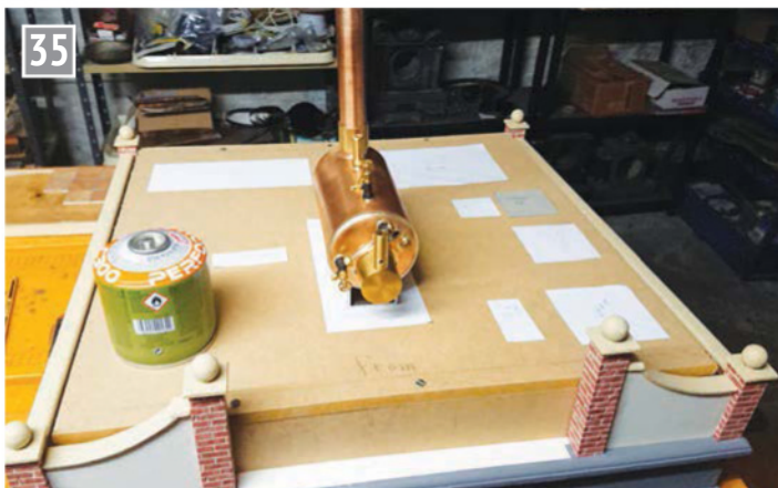
Trial fit of the boiler.
