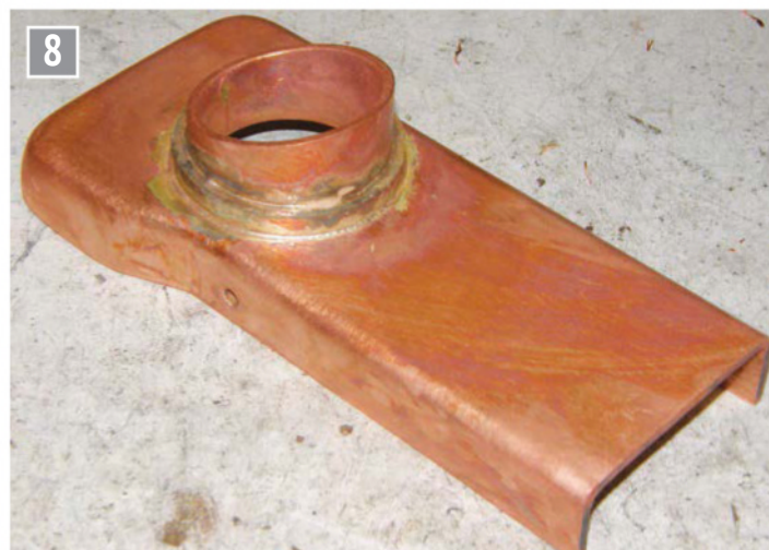
The firebox backhead with fitted firehole ring.
