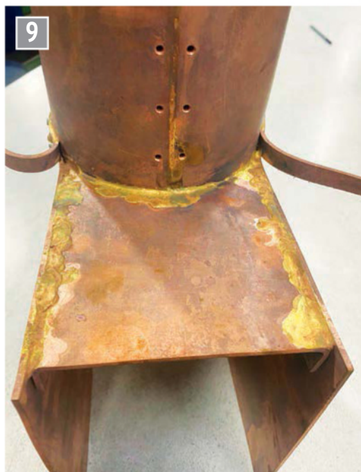
The throatplate brazed to the barrel.
