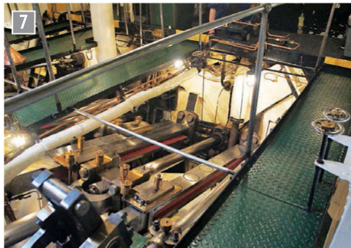
Crossheads run on the slides and Stephenson's valve gear is visible. There are traces of steam in the engine room and there's nothing quite like the smell of warm oil.
