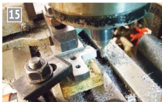
Creating the web on the crank disk.
