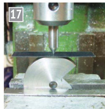
Drilling and tapping for the securing screws.
