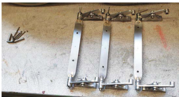
15. Here are the three finished brake beams with their hangers and shoes fitted..
