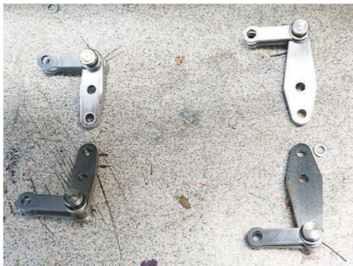
19. Lastly for the compensators and links here they are assembled. I have laid them out as if the locomotive is facing to the right.
