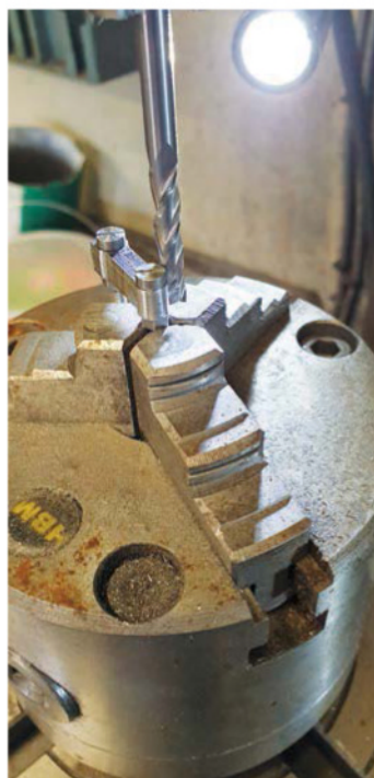
17. It was then over to the rotary table. I didn't trouble myself with making any 'button's as the screw heads are slightly smaller than the required size so I judged it by those and worked by eye - of course, all four ends were machined to the same diameter.
