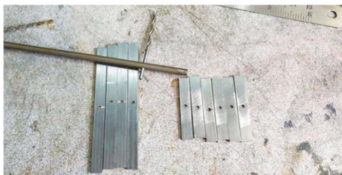
19. Lastly for the compensators and links here they are assembled. I have laid them out as if the locomotive is facing to the right.
