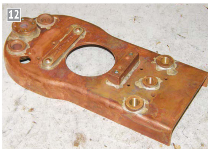
Backhead bushes and label fitted.
