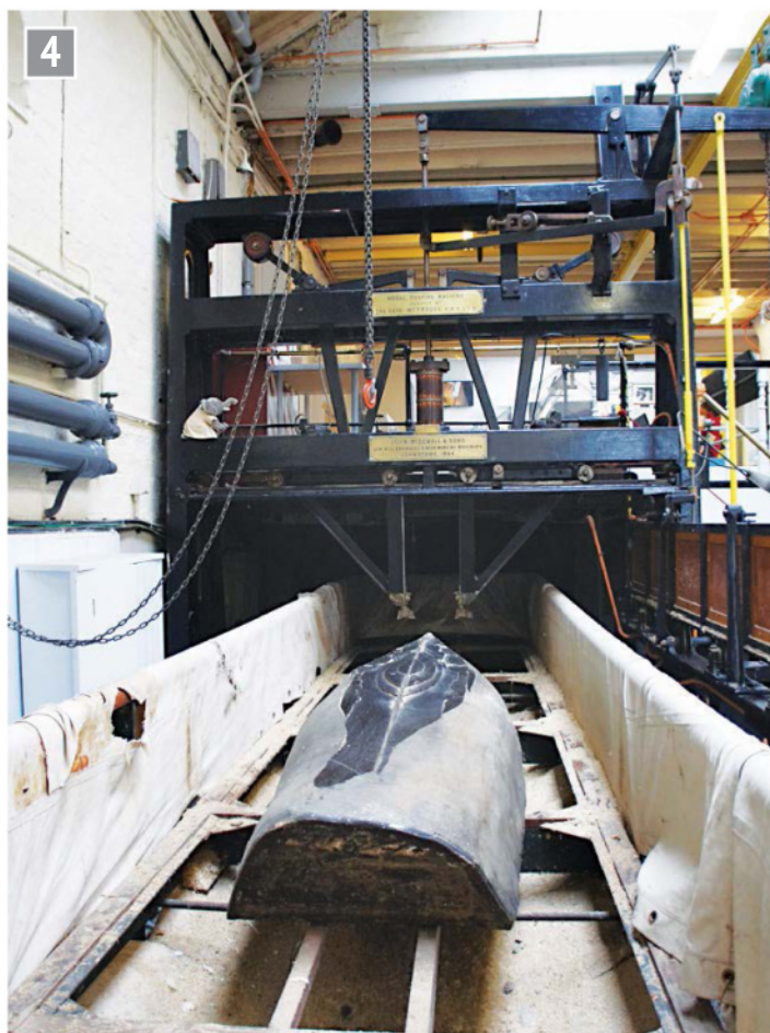
Contouring machine making hull forms for testing in the Denny ship tank.
