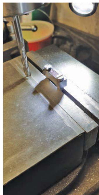
16. This picture shows one of the group of parts held in the machine vice. First the ends were machined square and after that I machined the scallop on either side.
