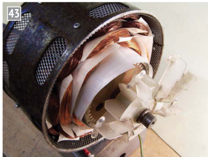
The rotor wrapped in aramid paper to protect the windings whilst inserting the rotor into the stator.
