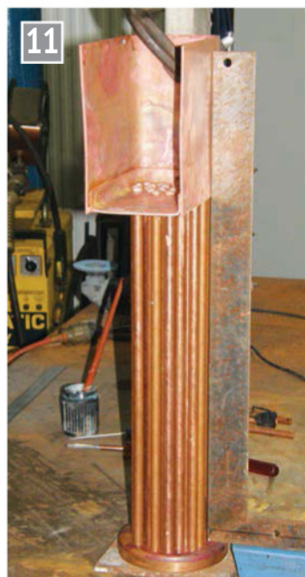
The boiler tubes assembly arrangement.
