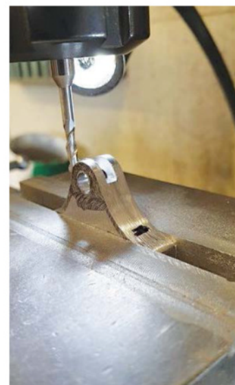
12. To produce the slot for the hanger, they were simply centred in the machine vice, chocked up on parallels and machined with a 3 mm slot drill.
