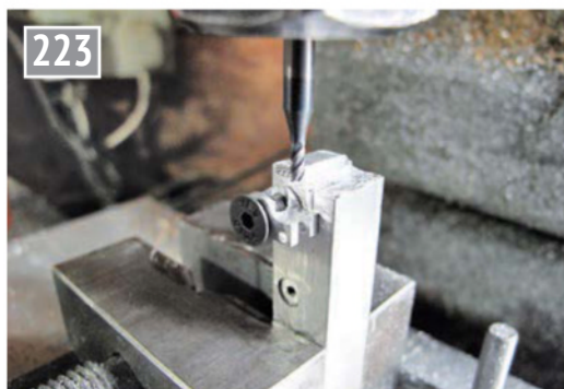
Completing the valve stem roller location slot.
