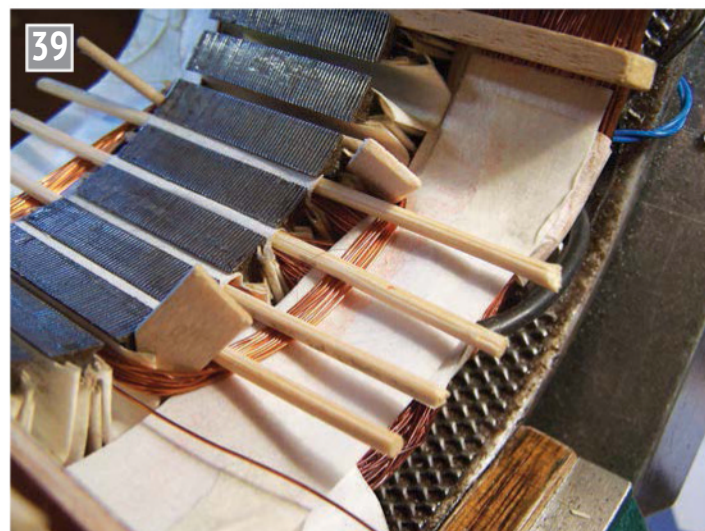
Starting the four-pole second phase winding - note the inter-phase insulation and the tapered craft sticks to space the winding down the slot.
