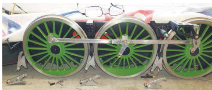
11. Here we are after machining the shoes to their correct thickness, ready for final profiling, remembering to remove the metal from the face that was up tight against the faceplate to remove the resulting lip. I removed most from this side just leaving a few thou to come off the other face.
