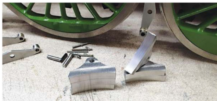
11. Here we are after machining the shoes to their correct thickness, ready for final profiling, remembering to remove the metal from the face that was up tight against the faceplate to remove the resulting lip. I removed most from this side just leaving a few thou to come off the other face.
