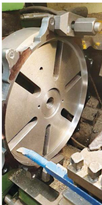
10. Very carefully machining the ring with the top slide set over at three degrees to match the wheel taper.
