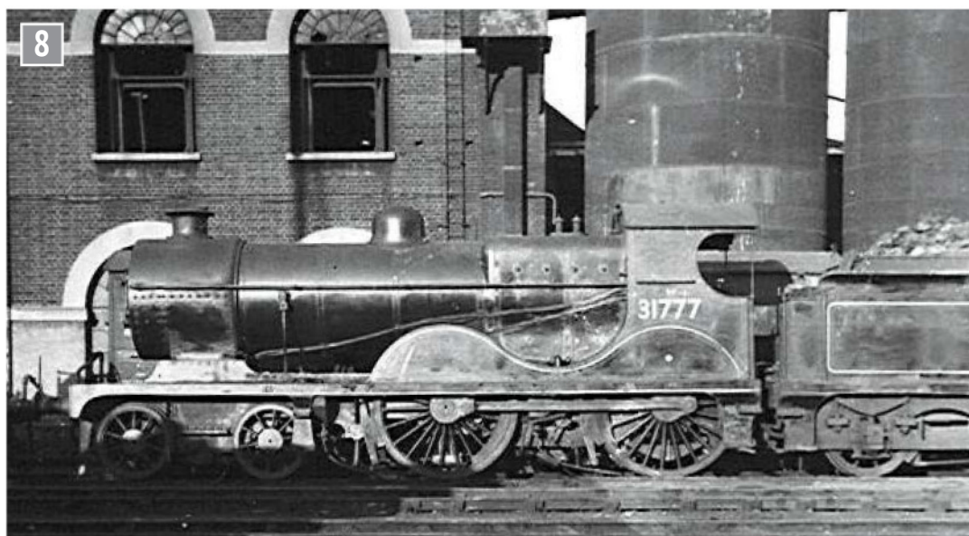
31777 in the evening sun at Brighton, the combination of leaf springs on the trailing axle and coil springs on the driving axle clearly visible. Photo courtesy Geoff Bannister.
