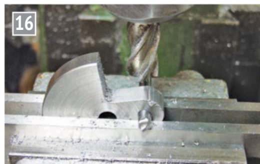
Forming the radius around the crank pin.
