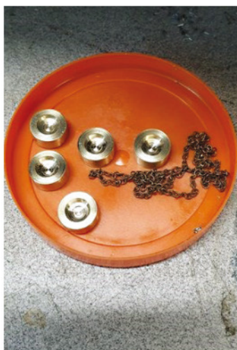
13. Here are the five filler lids (four plus a spare), with the chain that will be used to stop them getting lost. The handles will be added later with soft solder.
