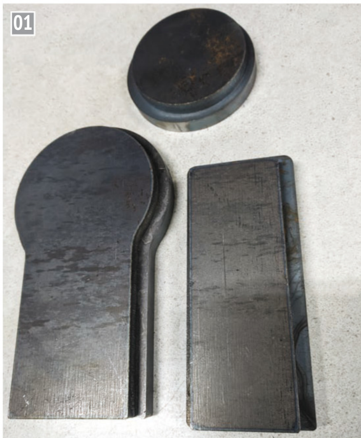
01 Laser cut steel boiler formers and the backing plates (photo: Jim Clark).
