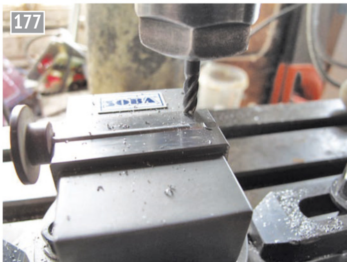
Producing the location flat.
