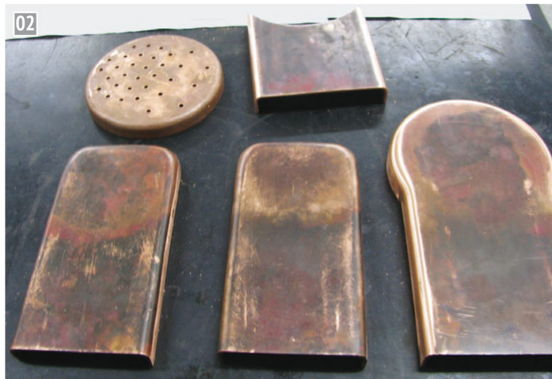
02 Set of flanged boiler plates (photo: Jim Clark).
