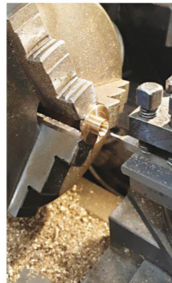
15. Here is the mounting plate in the lathe to machine the cone in the top - this is where the sand enters. I ground up some tool steel and set the cross-slide to 30 degrees for machining.
