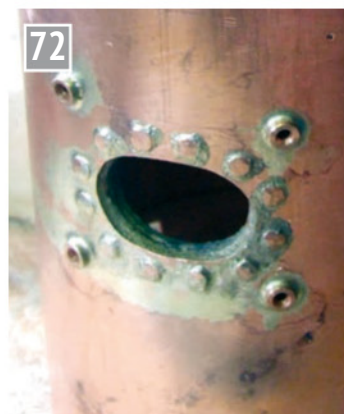
The four simple bushes in place on which to mount the fire door frame assembly.
