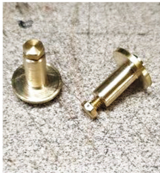
21. Here we have the main parts for the two sand traps. Still to do on this part is the four holes around the flange to bolt to the bottom of the steam sandbox.
