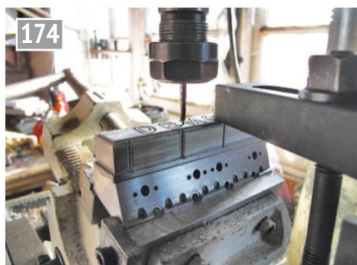
Centring for clearance hole.
