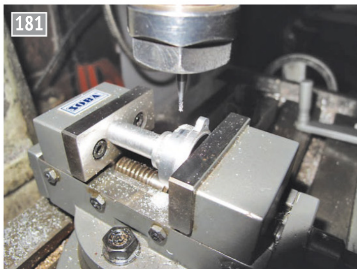
Machining position of the Hall sensor.
