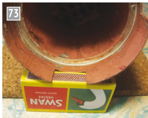
These views show the soldered joints for the top tube plate flange and the foundation ring.
