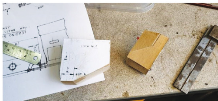
1. Wooden template for one of the sandboxes.
