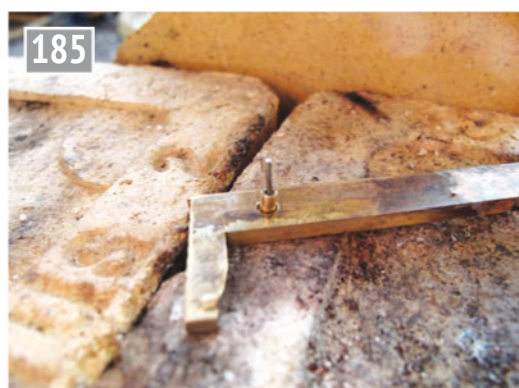
Set up to solder lead to connector.
