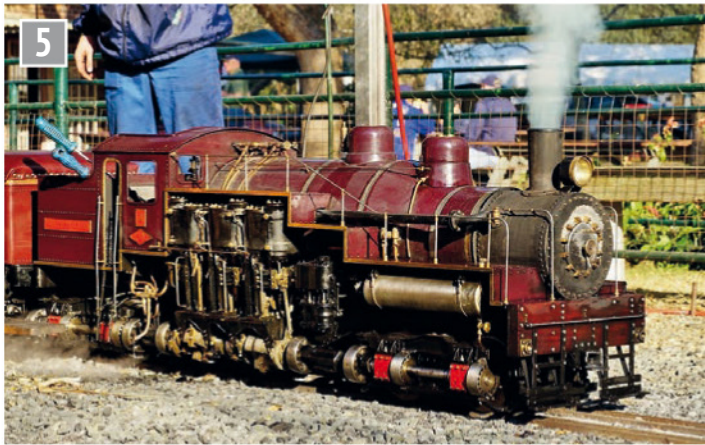
Leon's 7 1/4 inch Shay at the Pietermaritzburg Model Engineering Society – cylinder side (photo courtesy Hannes Paling).
