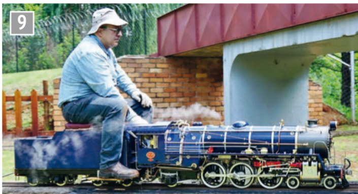
The 16DA which is similar to the 15F with one less coupled wheel set; a regular passenger hauler at the RSME. This locomotive is an outlier, because the frame and some of the valve gear was started by another builder and Leon finished the build to his exceptional standard. Leon's build time was three years (photo courtesy Hannes Paling).
