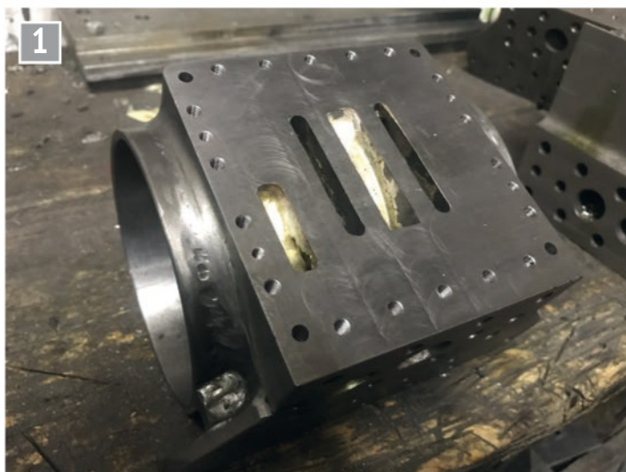
A cylinder fabrication made by combining simple geometric forms into a complex cylinder assembly (photo courtesy Leon Kamffer).
