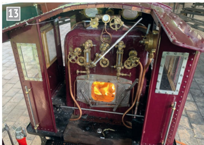
The 5 Class backhead on steam with a roaring fire. Note how something small like the valve handles are perfectly matched and are different for each prototype (photo courtesy Michael Eykelhof).
