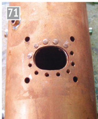
71 The riveting in progress with the ends peened over but not hammered down tightly so that the rivets were still loose and the silver solder could penetrate.
