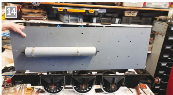
Large vacuum reservoir mounted under the main base plate.
