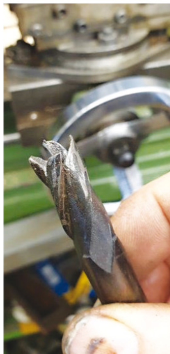
RIGHT: 10. Here's the recess tool before filing and final polishing/sharpening.
