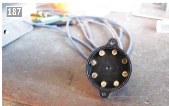
The leads protruding from the connector bores.
