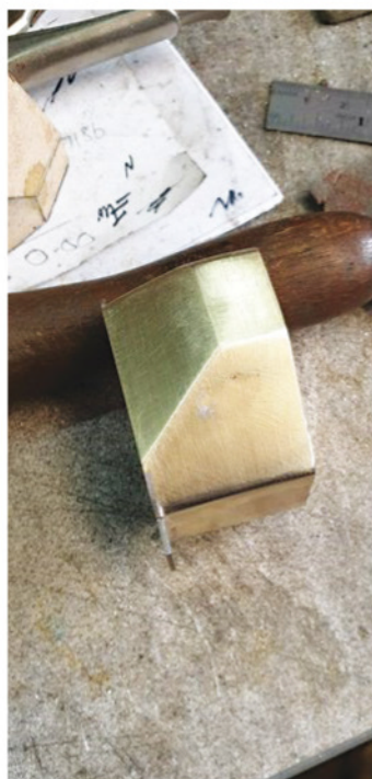
LEFT: 5. Here is the first steam box, now shaped according to the drawing. RIGHT: 6. I needed to plot the exact positions for the various holes. The ones in the bottom were just marked as in the drawing but for the top ones I decided it would be prudent to fit the boxes and check that the positions lined up with the holes that they needed to go through. Here I have temporarily bolted the right-hand gravity box in place.
