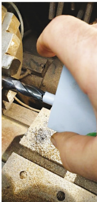
LEFT: 9. Checking the fit with the filler tube.
