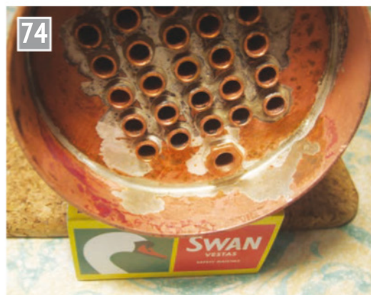
These views show the soldered joints for the top tube plate flange and the foundation ring.
