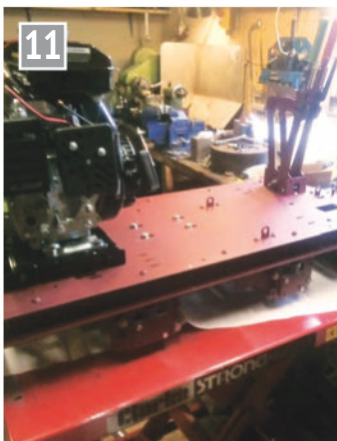
Chassis with engine fitted.
