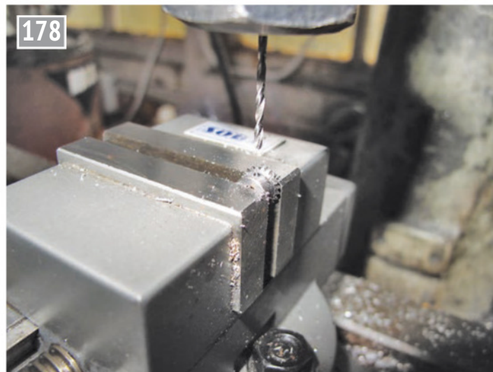
Drilling 1.60 diameter hole for the grub screw.
