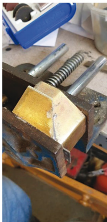
LEFT: 3. This picture shows why I felt it necessary to make the boxes now. As can be seen, the boxes will fill a large part of the area either side of the crank and once the rod is fitted I doubt that I would be able to get to these. RIGHT: 4. This picture shows a start being made on filing the angled face to blend in with the rest of the box.
