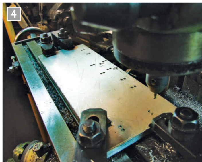
Drilling the base.
