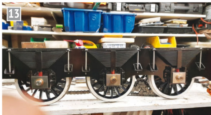
13 Wheels, spring hangers, brackets, connecting chains and a coat of black added.
