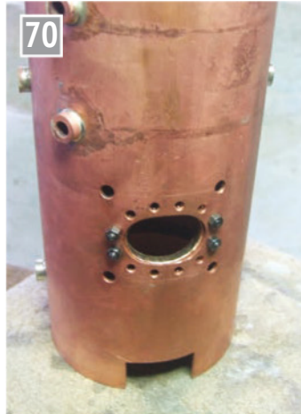
Here the inner firebox assembly has been located and secured with a few nuts and bolts ready for the group of rivets to be added.
