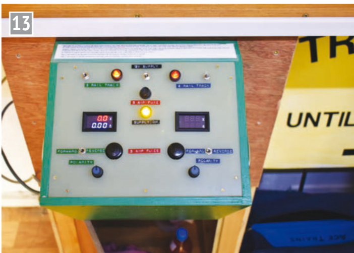
Track controller for all tracks.
