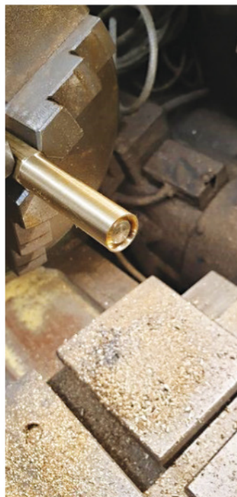
LEFT: 11. Here's the first lid recess machined. As the centre needs to be slightly recessed in the lid, before using the profiled tool I machined a slight recess with a smaller endmill. RIGHT: 12. Here is the dish being formed in the top of the filler lid.
