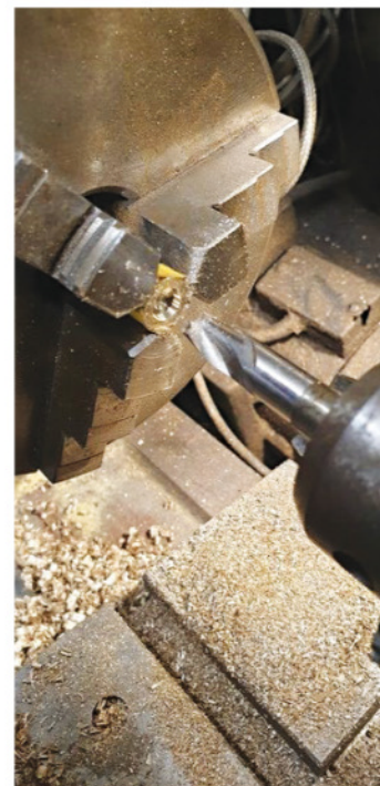
LEFT: 11. Here's the first lid recess machined. As the centre needs to be slightly recessed in the lid, before using the profiled tool I machined a slight recess with a smaller endmill. RIGHT: 12. Here is the dish being formed in the top of the filler lid.
