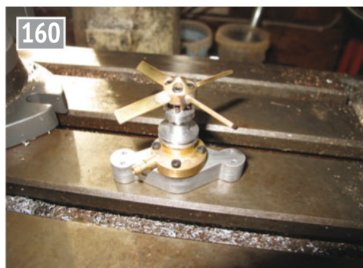
Fan attached to the water pump.
