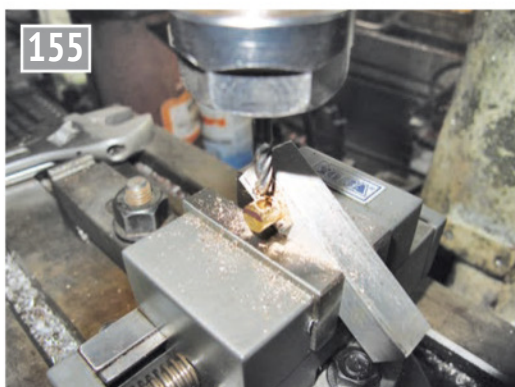
Producing pipe connector hole.
