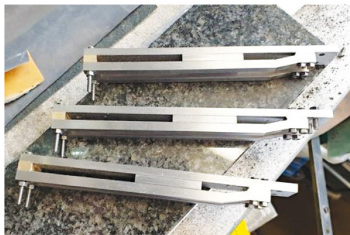
19. The slippers were cut from the gauge plate and machined to size and here they are fitted in between the slide bars.
