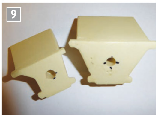
Slot drilled holes are less likely to split the casting than drilled holes.
