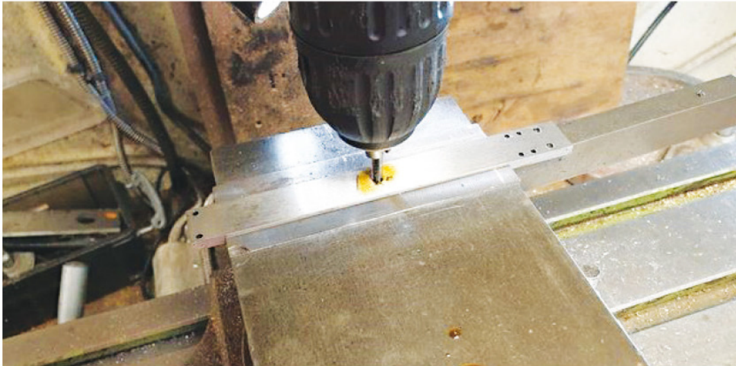
10. All holes have now been drilled in the upper bars and the tapped hole for the oil supply is being cut. This is the centre slide bar; the two outside bars will have two oil holes.
