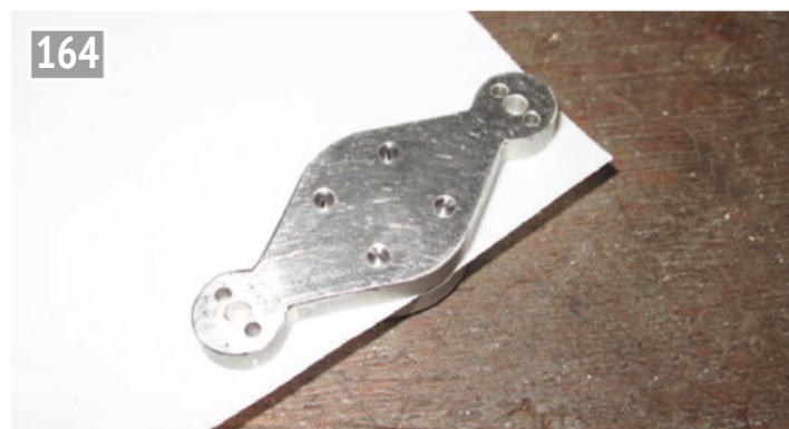
First stage of making the sealing gasket.
