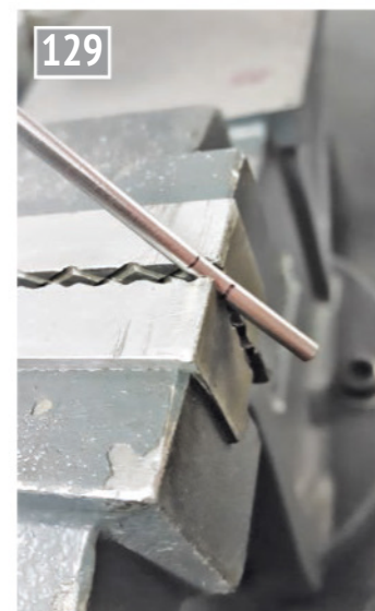
Pressing an interference fit for the hand railing.
