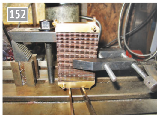
The second water tank left to cure the bonding.
