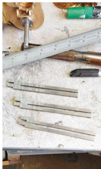
14. The bars were then turned over and the step along most of the bar machined. Here are the six blanks machined to size ready for the angles to be machined.
