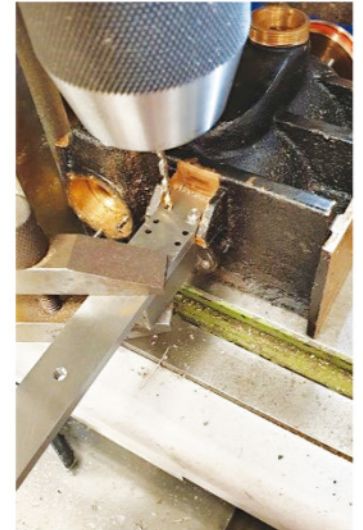
11. The next job was to drill the two mounting holes in the slide bar support. Don suggests doing this the other way around, i.e. holes transferred from the lug, but I chose to do it the other way around as I think it's a more accurate way of doing it. The first job was to set the angle plate squarely on the mill bed and clamp the cylinder to it. I drilled the first hole through the slide, placed a 5BA bolt in this and then on the same 'Y' setting drilled the second, thus ensuring the slide bar will be parallel to the frames.
