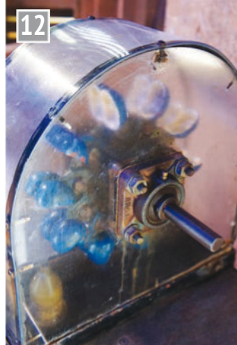
12 Small model of a Pelton wheel at CAT; an effective way to generate electricity where there is a high head of water.
