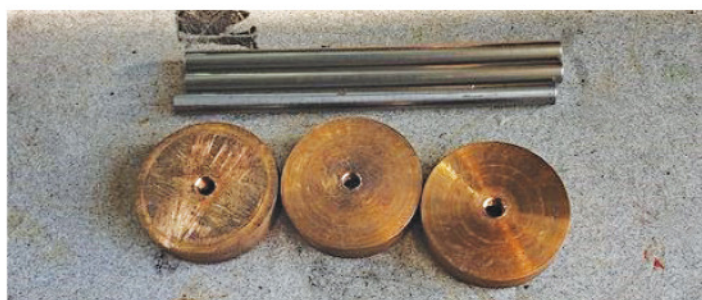
4. To begin with, a picture that shows the piston blanks along with the three rods cut oversize. Note that the piston bores have been chamfered.
