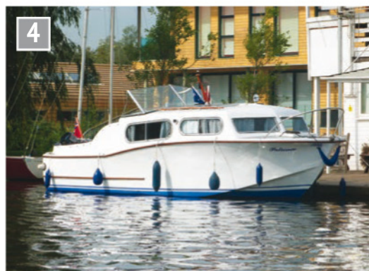
Patience, a 27-foot long motor cruiser I owned for a while, before I decided I much preferred sailing. 50 volts DC at 10 amps pushed her along well for 5 or 6 hours on one battery set.
