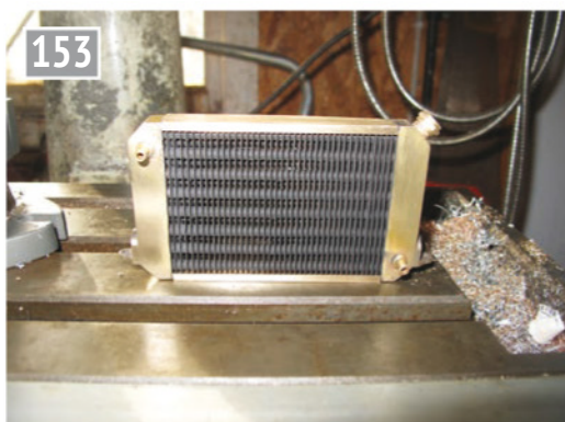
Finished radiator assembly.
