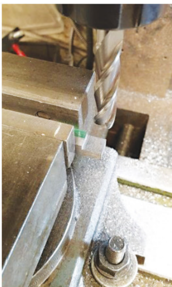
13. After machining the lower bars to size, I needed to machine the underside of the dogleg. All machining operations for these bottom bars were done in pairs to ensure they matched. I have to say all 6 have come out as planned but best to keep them in their machined pairs.
