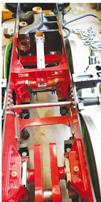
16. Here's a view to show the top slide-bar bolted to the motion bracket.
