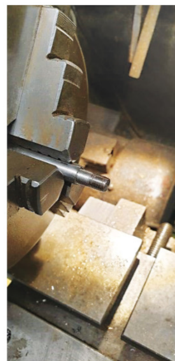
5. The piston rod after having the spigot/thread machined
