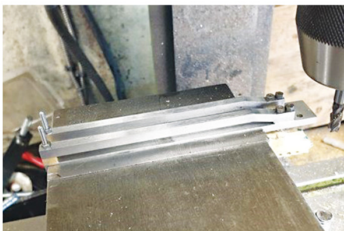
18. I Loctite'd both rear and front packers to the top slide and drilled through them. Once the bottom slides had also been drilled, with the packers now clamped between both slides, I could machine them to width. The picture shows the front brass packers having just been machined.
