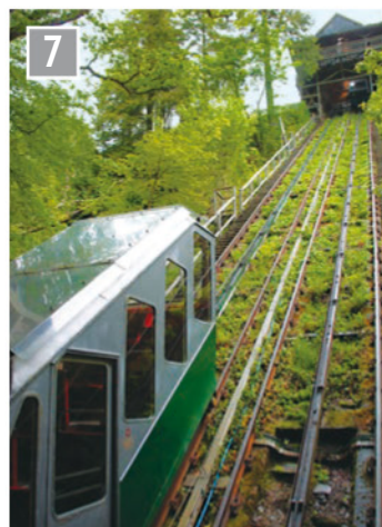
The water powered cliff railway (funicular) looking up from the bottom station.
