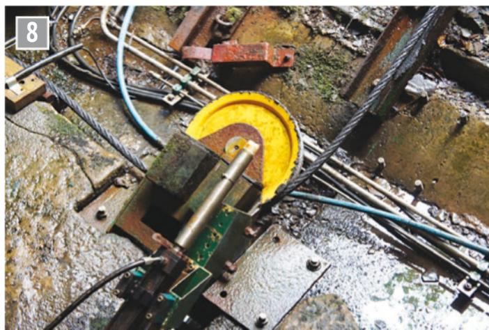
Pulley at the top station, part of a sophisticated control and braking system.
