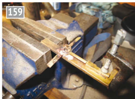
Silver soldering the blades to the hub added by a simple holding fixture.
