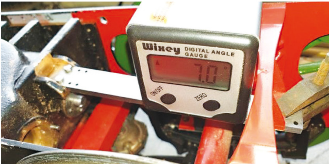
10. All holes have now been drilled in the upper bars and the tapped hole for the oil supply is being cut. This is the centre slide bar; the two outside bars will have two oil holes.
