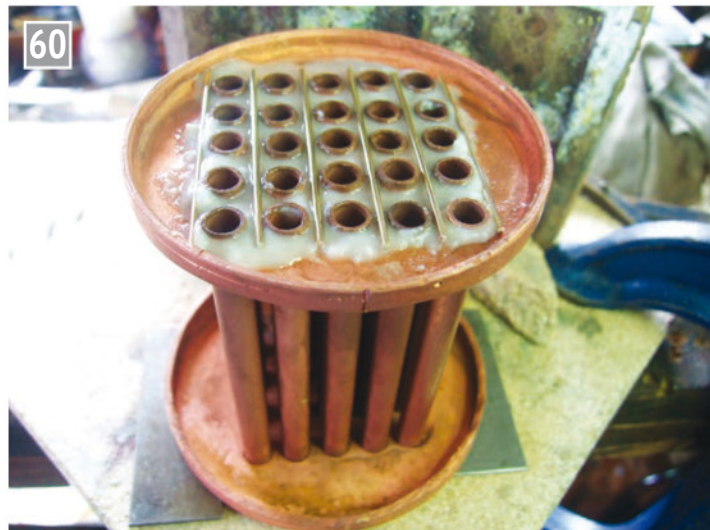
The inner firebox flanged plate ready to silver solder the tubes in place.
