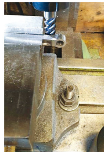
21. With the roughing out of the flute done this left the final machining operation of reducing the thickness of the little end. For this, I held the rod in the machine vice and reduced the little end, the metal being taken off equally from either side.
