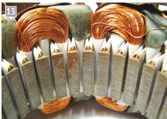
The original 16-pole winding - second phase visible - a full-pitch winding.
