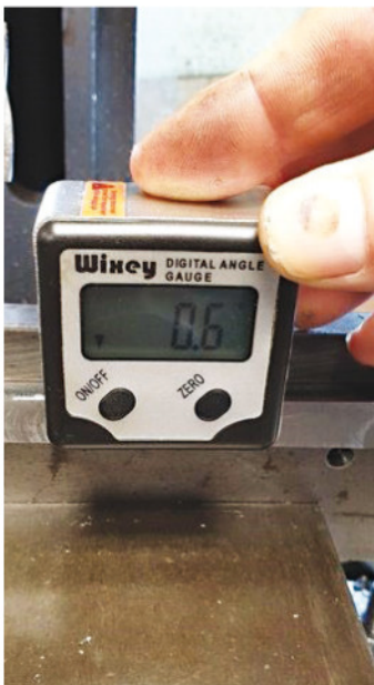
14. I then rested the scale on the rod to measure the angle - as can be seen, it's not very much.
