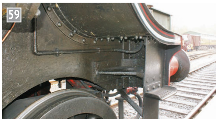
Buffer beam bracket with countersunk rivets.
