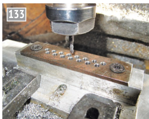
Fixture cover plate being bored.
