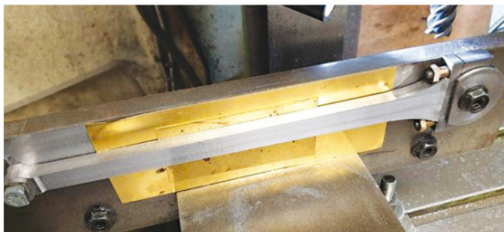
18. With the first side machined, before doing the other side I searched for some suitable shim to pack the back to stop any possible flexing. I may go 'off script' with the big end and add an oil cap with lid for two reasons - firstly to give a larger capacity of oil and secondly to make it easier to reach the oiling point once the locomotive is built. I can't see there being any height restrictions involved but will take a closer look later.
