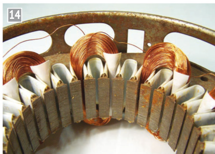
The original 16-pole winding first phase – identical to the visible winding in photo 13.
