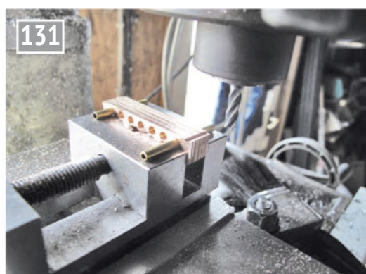
Second rebate machining operation.
