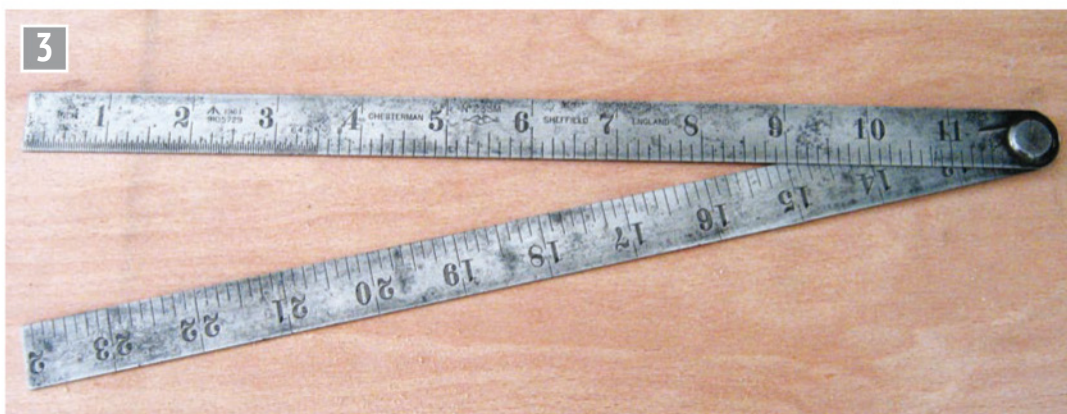
Shipwright's folding steel rule.
