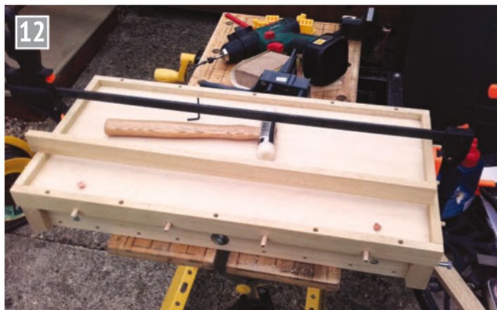
Dry run of the side planking, first row dowelled to the base board with 6mm dowels.
