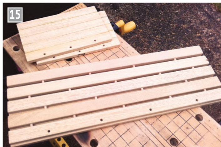
Two of the completed end panels and a pair of side panels before gluing and clamping.
