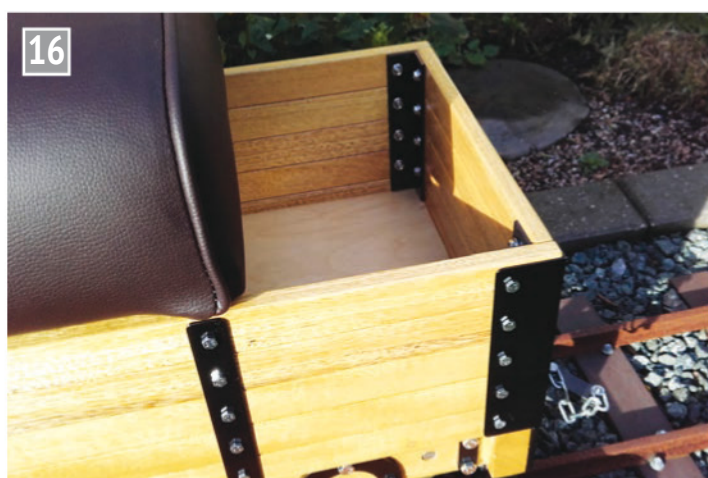
Side planking corner bracing.
