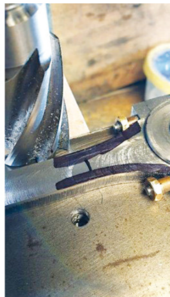
16. For the big end, I also needed to note where to stop cutting for the flare of the rod. The large cutter in the picture was used to line up the angles, not for cutting.
