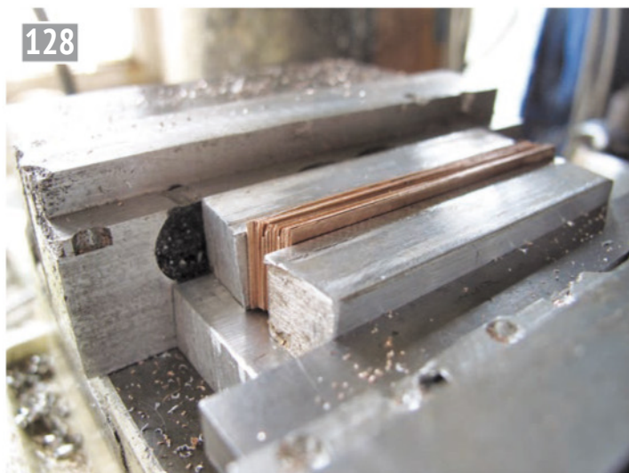
Radiator fins - first operation.
