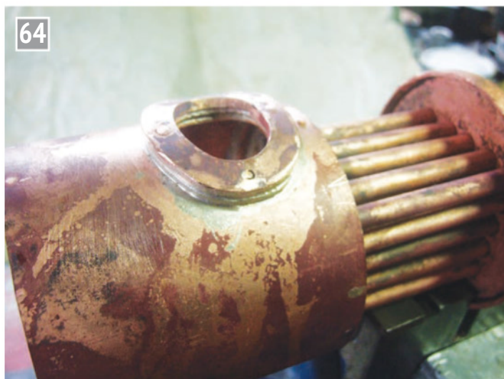
The door spacer added to the inner firebox barrel using just two of the rivet positions.
