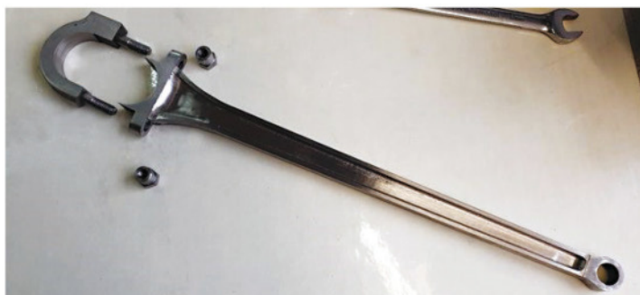
22. Finally, here are the component parts that make up the inside connecting rod on a Gresley Pacific.
