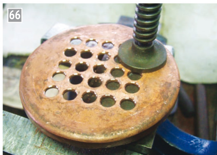
The upper flanged plate has been drilled out and chamfered for the final soldering operation.
