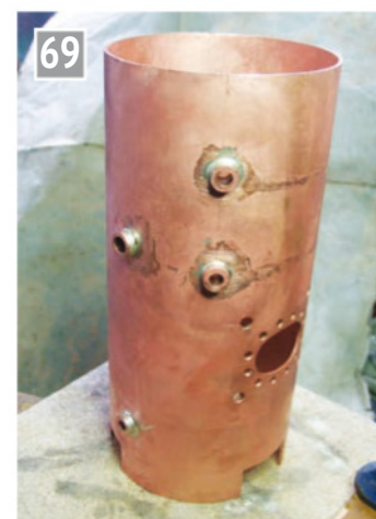
The set of bushes for the boiler fittings has been added and the barrel is ready for the two parts of the boiler to be assembled.
