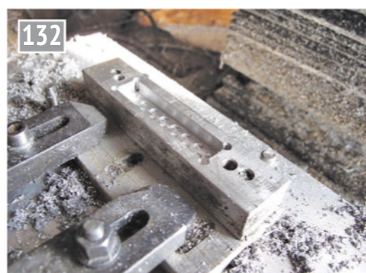
Drilling fixture pocket.
