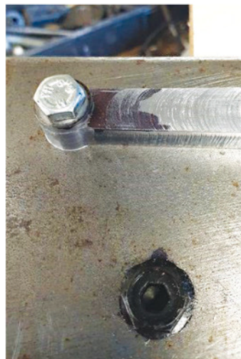
15. Next, I measured the width of the small end neck, halved the difference with the required value and scribed the edge as a guide. I marked both sides but will only use the first, flipping the rod over rather than try to match the same 0.6 degrees on a swivel vice.
