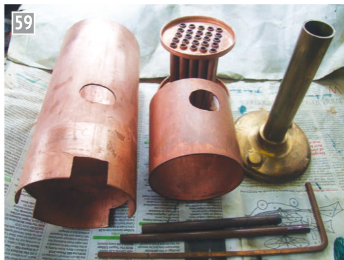
A general view of the vertical boiler kit of parts as received by the author.
