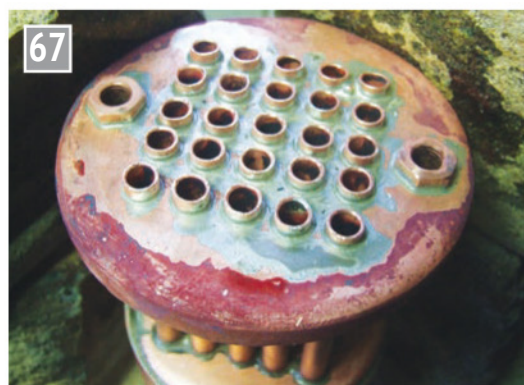
Here are two views of the soldering completed for the top plate with the main steam bushes added.
