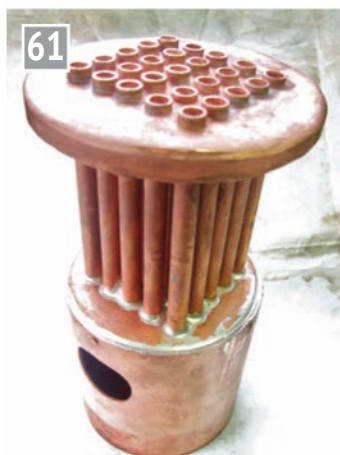
Soldering on the firebox barrel and note the aperture for the door has been placed with the nest of tubes in the same plane.
