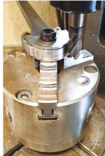
LEFT: 10. With the jig ready I turned my attention to profiling the two ends, beginning with the big end. As can be seen I made a start on machining the curve. The uneven part to the left is just where I have cut away excess metal ready to flair the curve of the strap into the rod itself - this to be done by hand. RIGHT: 11. I've included this picture to show how I held the work in the rotary table. There are two buttons with the lower one (seen here) having a spigot that's larger than the nut below. The spacer in the rod is also threaded so when all are tightened they are not going to come loose. The spigot was held tightly in the rotary table chuck and with the large button between both chuck and job it was very stable. I didn't bother hardening the buttons - I saw no point as they are a one-time only use.
