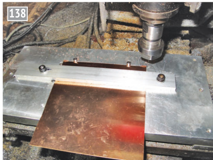
Cutting strips to the correct width.
