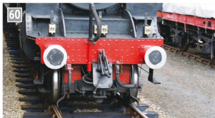
Rivet detail on the front buffer beam.
