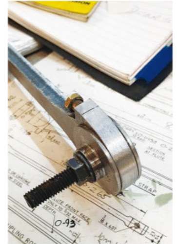
LEFT: 10. With the jig ready I turned my attention to profiling the two ends, beginning with the big end. As can be seen I made a start on machining the curve. The uneven part to the left is just where I have cut away excess metal ready to flair the curve of the strap into the rod itself - this to be done by hand. RIGHT: 11. I've included this picture to show how I held the work in the rotary table. There are two buttons with the lower one (seen here) having a spigot that's larger than the nut below. The spacer in the rod is also threaded so when all are tightened they are not going to come loose. The spigot was held tightly in the rotary table chuck and with the large button between both chuck and job it was very stable. I didn't bother hardening the buttons - I saw no point as they are a one-time only use.
