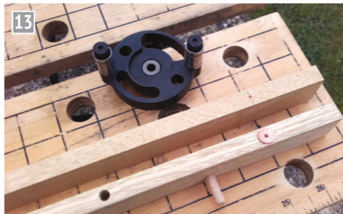
Dowel jig and transfer centre plug in use.
