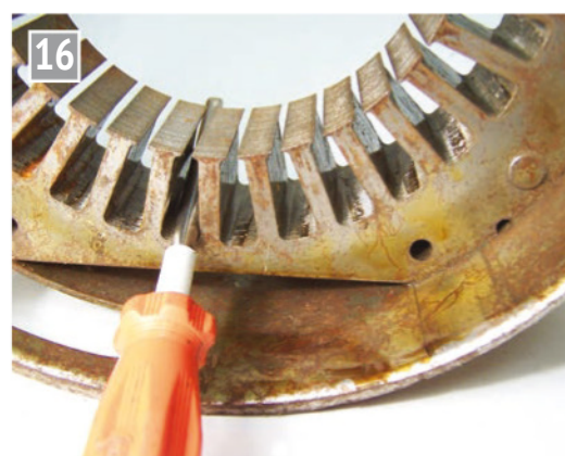
The slots in the two-speed motor stator.
