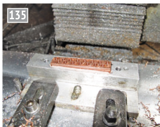
Completed batch of fins.
