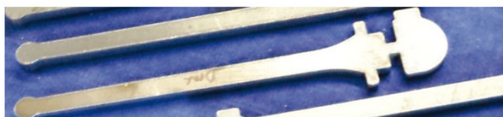
1. Here is the blank as supplied. This particular blank is cut very close to the final dimensions, closer than I would like, which makes life a little harder and setup is crucial.
