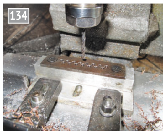
Fins being drilled.
