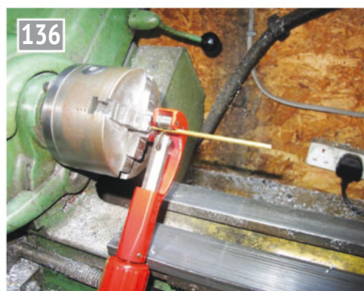
Cutting the tubes to length.
