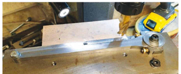
17. Profile almost complete. The step seen near the big end will be done by hand once I have machined the sides and the fluting.
