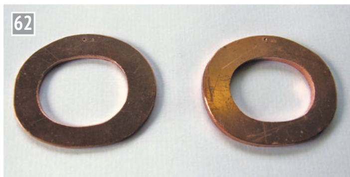
Two pieces of copper plate profiled and formed to be the sandwich spacer ring around the firehole door position.
