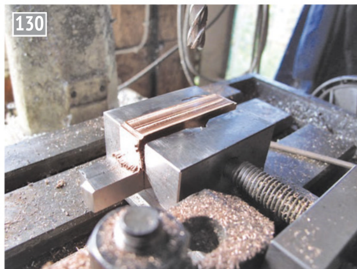
Machining fins' lengths and first rebate.
