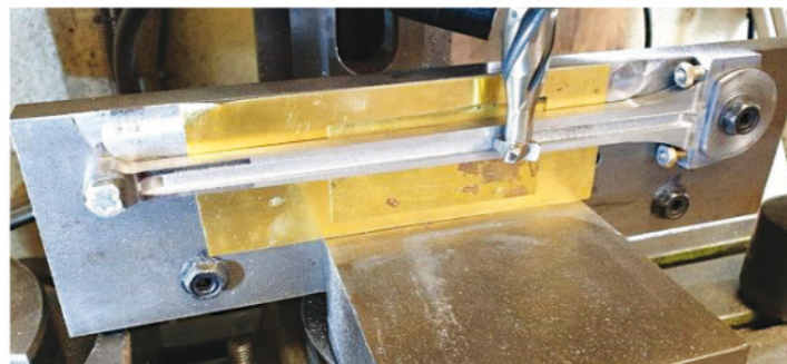
19. For the flutes, I first machined a section down the middle parallel to the middle of the rod. The picture shows the first side so machined, taking care either end not to go too far. For the little end, extra thought is required to allow for the fact that this end still needed to be machined to a thinner width. Once the first side was done I then removed the rod from the jig and flipped it to the other side, leaving the jig in place and thus set for doing either side.
